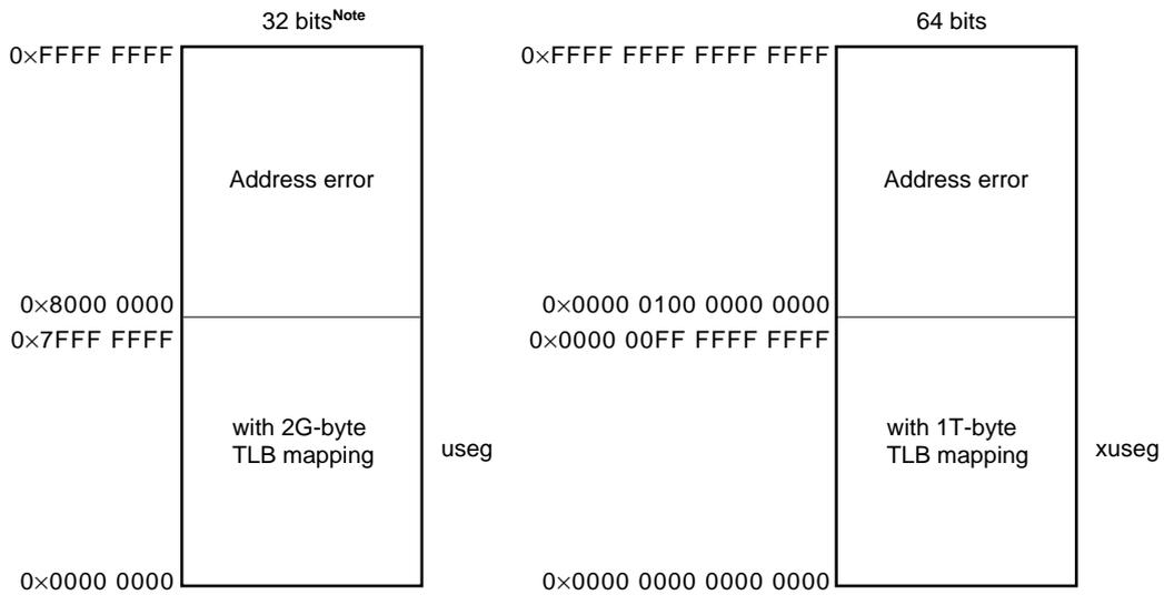
**Note** In the 32-bit mode, the value of bit 31 is sign-extended to bits 32 through 63. For details, refer to **Vr4100 User's Manual**.
