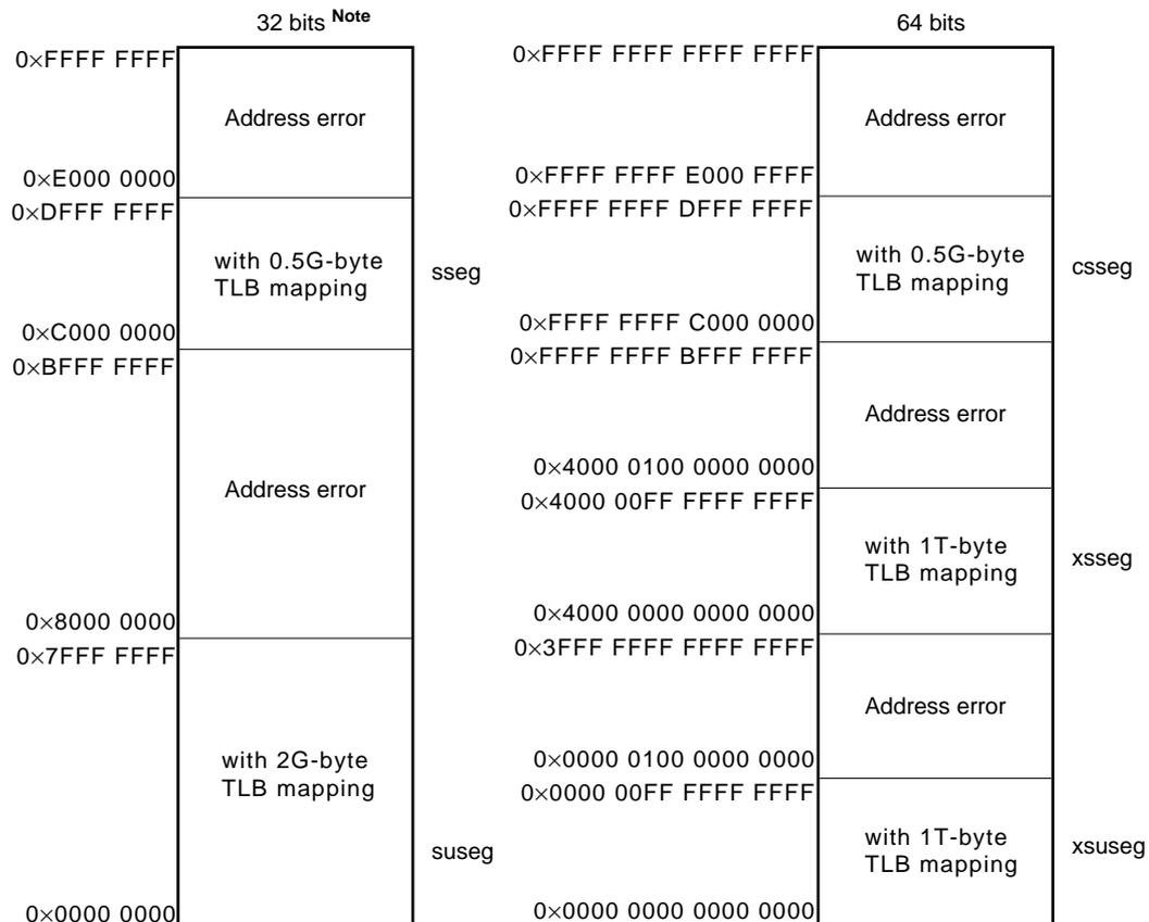
**Note** In the 32-bit mode, the value of bit 31 is sign-extended to bits 32 through 63. For details, refer to **Vr4100 User's Manual**.
