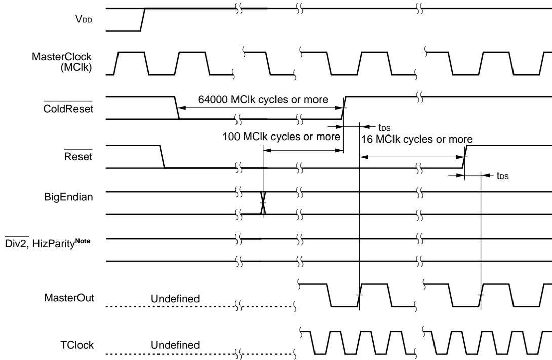
**Note** Fix the status of the  $\overline{\text{Div2}}$  and  $\overline{\text{HizParity}}$  pins on power application.
