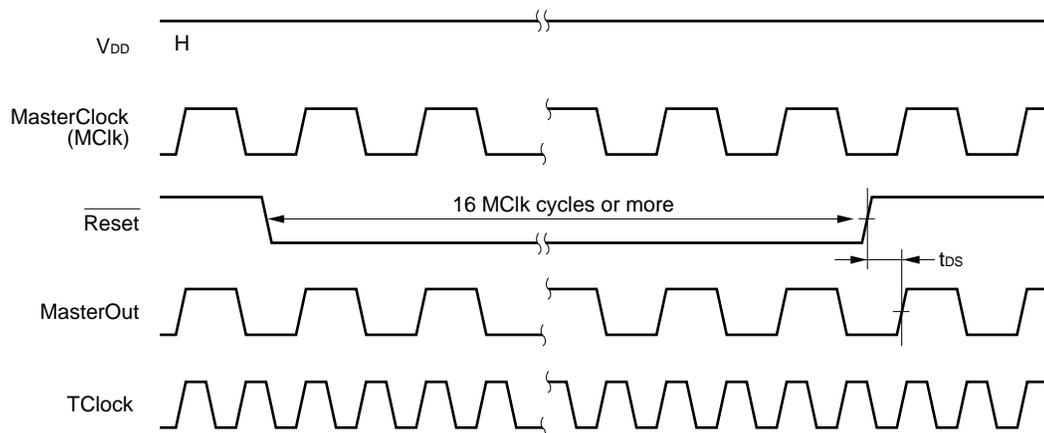
**Remark** For the details on  $t_{bs}$ , refer to **Interrupt/reset edge timing**.
