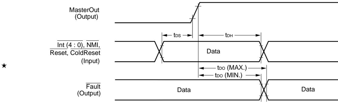
**Relation between clock and system bus (when the Div2 pin is set to low)**
