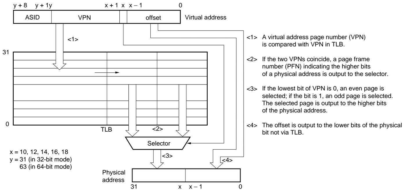
Reading and writing of TLB entries is performed by loading/storing between the TLB entry specified by the index register or the random register, and the entry Hi, entry Lo1, entry Lo0, and page mask registers.
