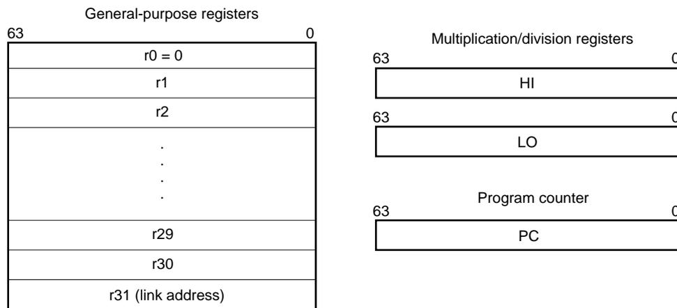
No program status word (PSW) is provided. The function of the program status word is substituted by the status register and cause register of the system control coprocessor (CP0).
