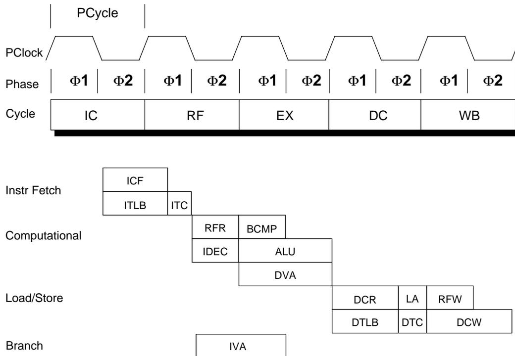
Figure 4-3 Pipeline Operations
