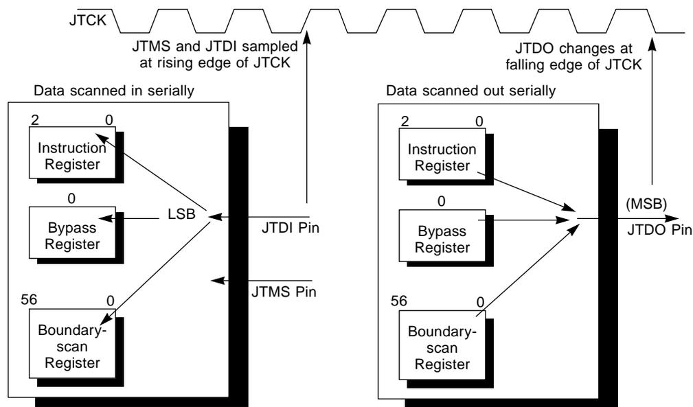
Figure 13-6 JTAG Test Access Port
