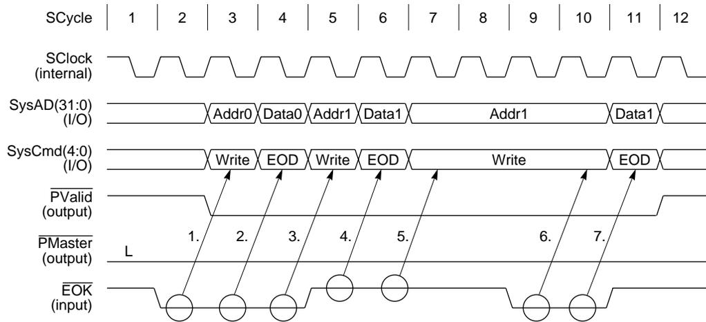
Figure 12-29 Discarding and Re-executing Processor Single Write Request
