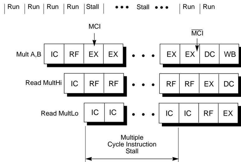
Figure 4-15 Example of a Multicycle Instruction Interlock
