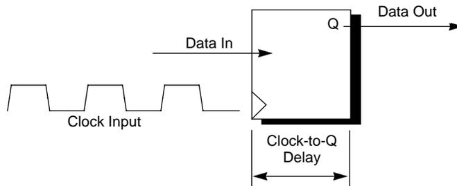
Figure 10-2 Clock-to-Q Delay
