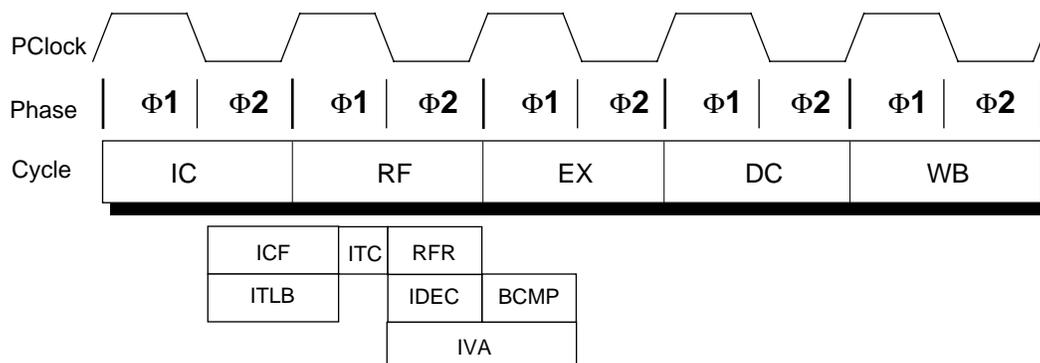
Figure 4-7 Branch on Equal Instruction Pipeline Operations
