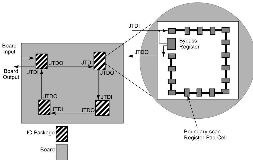
Figure 13-4 Bypass Register Operation
