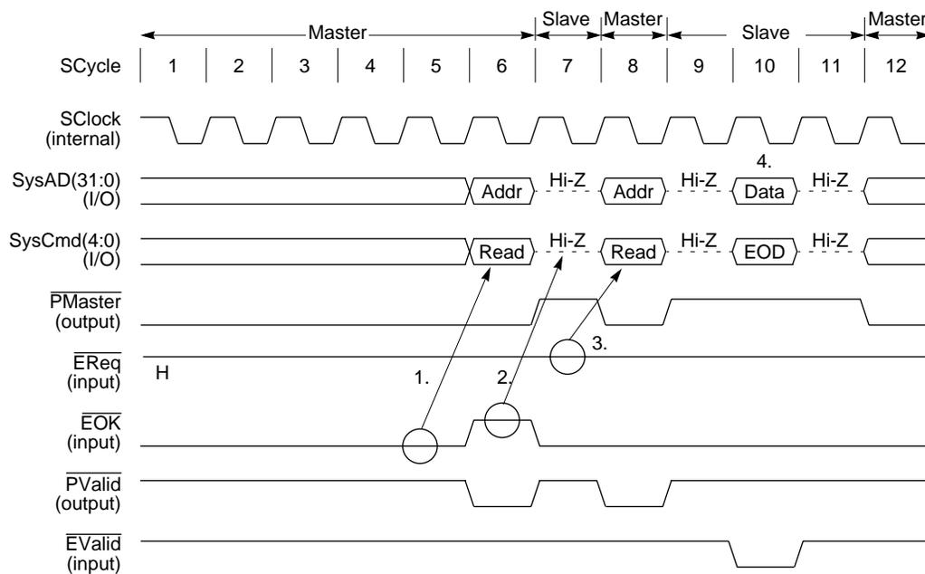
Figure 12-30 Discarding and Re-executing Processor Single Read Request
