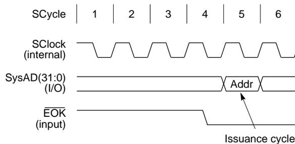
Figure 12-4  $\overline{\text{EOK}}$  Signal Status of Processor Request
