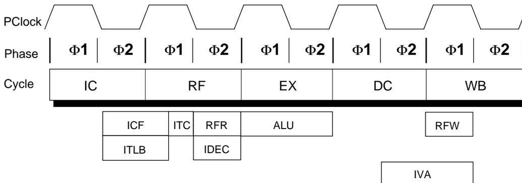
Figure 4-8 Trap if Less Than Instruction Pipeline Operations
