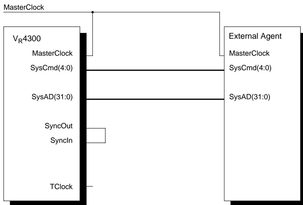
Figure 10-5 Phase-Locked System
