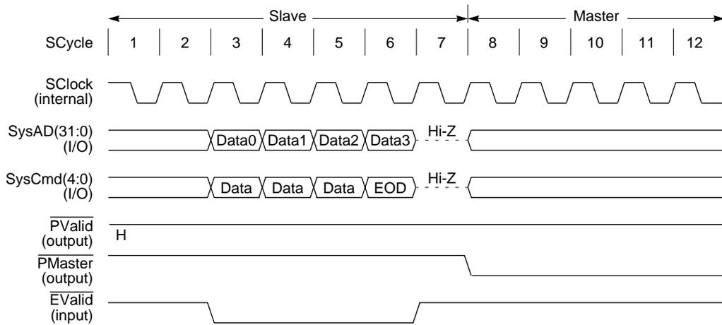
Figure 12-21 Block Read Response in Slave Status
