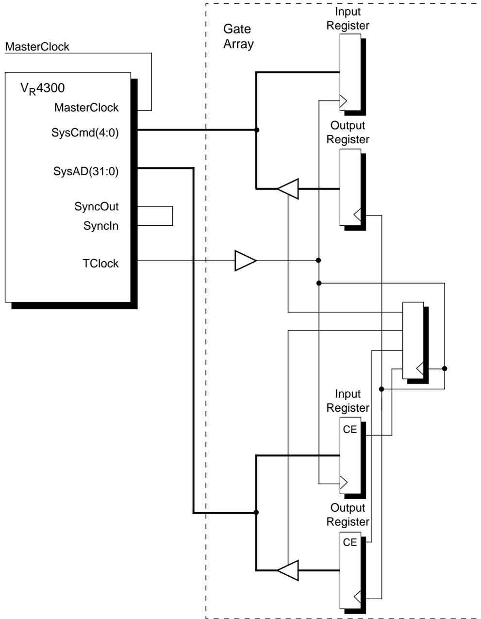
Figure 10-6 Gate-Array System without Phase Lock, Using the V<sub>R</sub>4300 Processor
