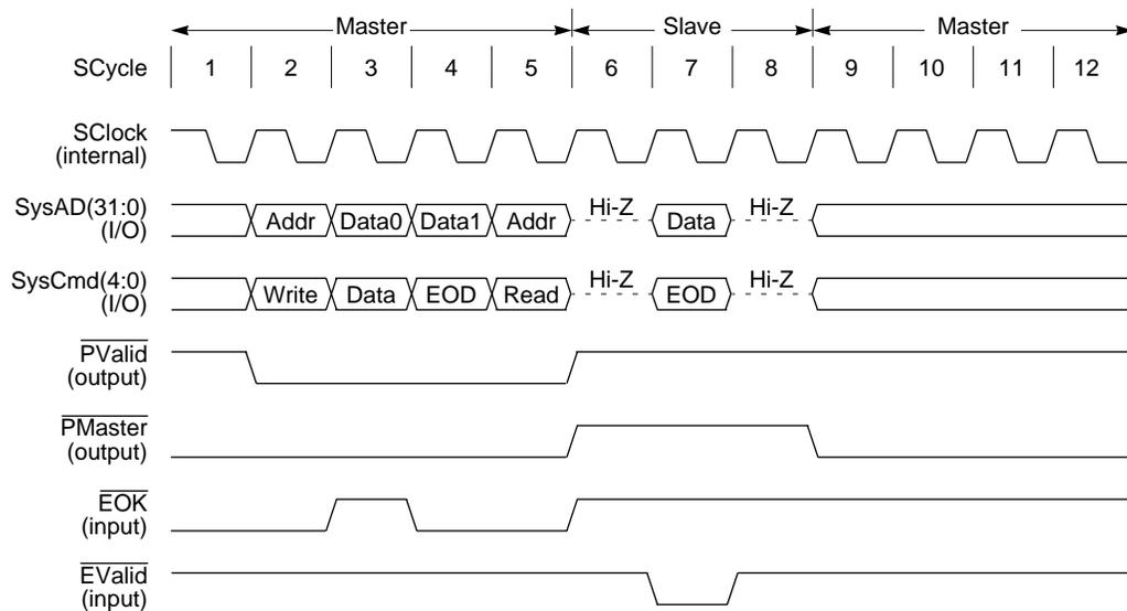
Figure 12-26 Processor Write Request Followed by Processor Read Request
