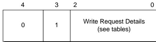
Figure 12-34 Write Request SysCmd(4:0) Bus Bit Definition
