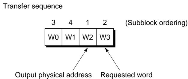
*Figure 12-2 Data Sequence on Data Cache Read Request*
