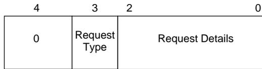
Figure 12-32 System Interface Command Syntax Bit Definition
