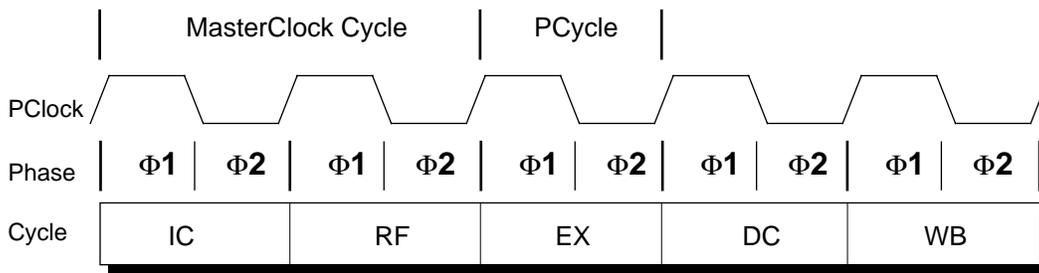
Figure 4-1 Pipeline Stages
