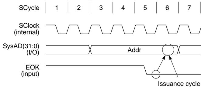
Figure 12-5 Address Cycle Extended by  $\overline{EOK}$  Signal
