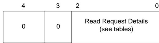
Figure 12-33 Read Request SysCmd(4:0) Bus Bit Definition
