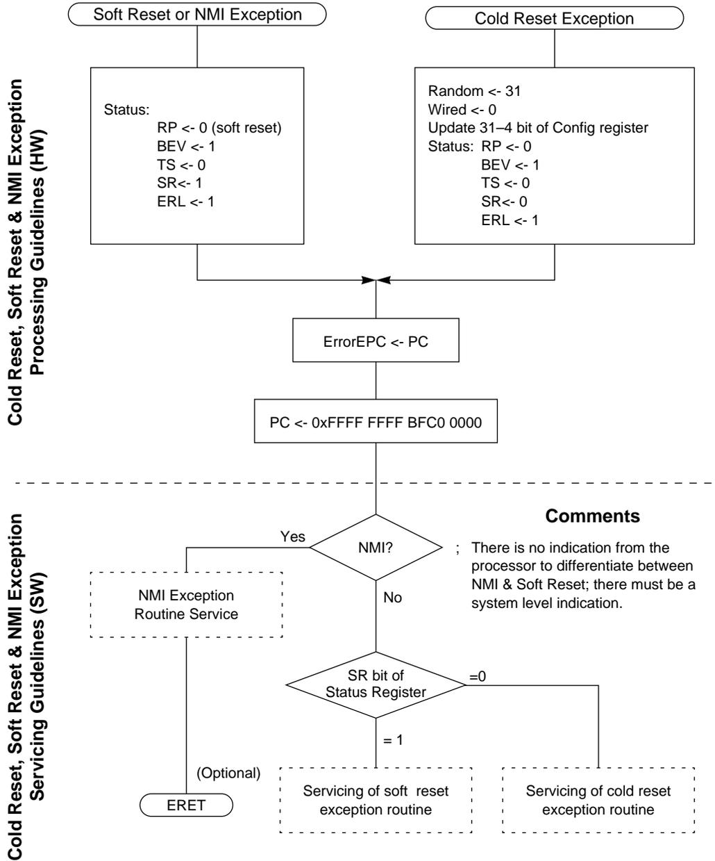
Figure 6-16 Cold Reset, Soft Reset & NMI Exception Handler
