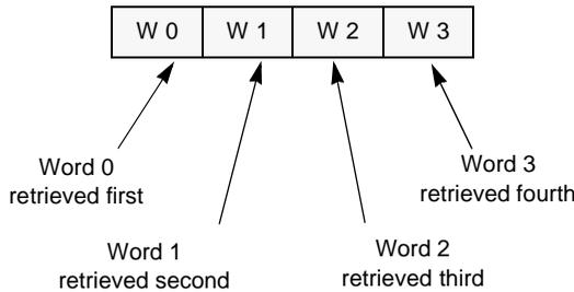
*Figure A-1 Retrieving a Data Block in Sequential Order*
