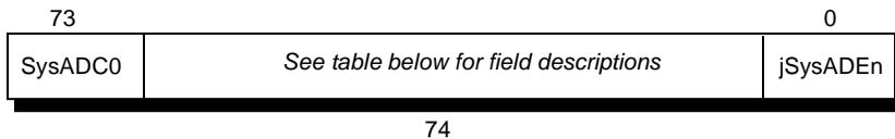
Figure 20-17 JTAG Boundary Scan Register Format
