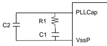
Figure C-2 PLLCap Circuit
