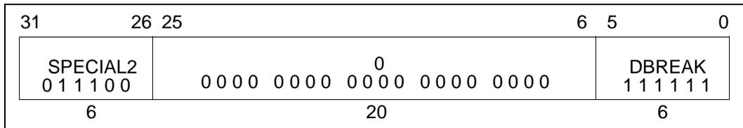
The DBREAK instruction forces entry into Debug mode by causing a trap to the Debug Exception vector address (0xFFFF FFFF BFC0 1000). This instruction may only be executed in Normal (User, Supervisor, or Kernel) mode. Execution in Debug mode results in undefined behavior.
