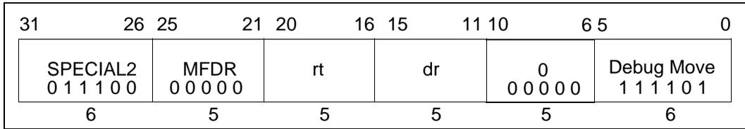
**Format:**MFDR *rt*, *dr* (VR5432 format)**Description:**The contents of debug register *dr* are loaded into general-purpose register *rt*.**Operation:**32, 64T: GPR[*rt*] ← DEBUG[*dr*]**Exceptions:**
