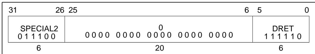
The DRET instruction returns from Debug mode to the mode in effect (User, Supervisor, or Kernel mode) when the last debug break occurred. Control is passed to the instruction pointed to by the Debug Exception PC (DEPC) register. Unlike most jumps and branches, the execution of which also executes the next instruction (the one in the delay slot), DRET does not execute a delay slot instruction. The DRET instruction must not be placed in a branch delay slot.
