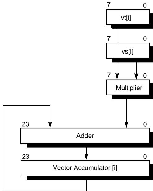
Figure 19-4 24-Bit Accumulator
