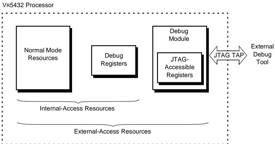
Figure 20-1 Access to Processor Resources in Debug Mode
