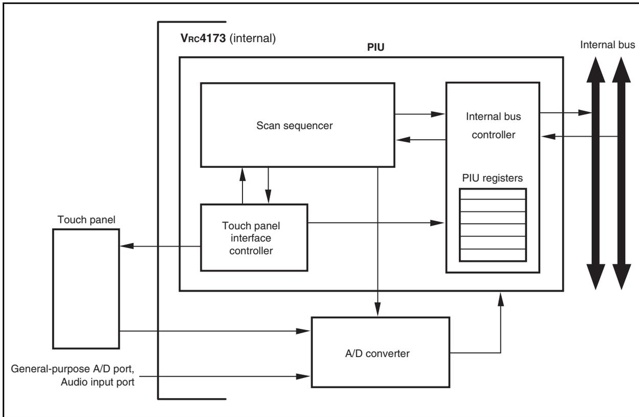
The PIU includes three blocks: an internal bus controller, a scan sequencer, and a touch panel interface controller.
