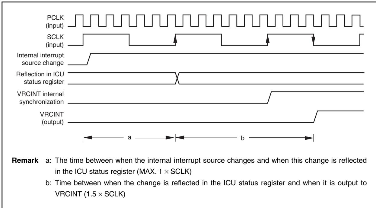
Figure 7-3. Time Lag Until Status Change Is Reflected in VRCINT Signal (When Sampling with PCLK)
