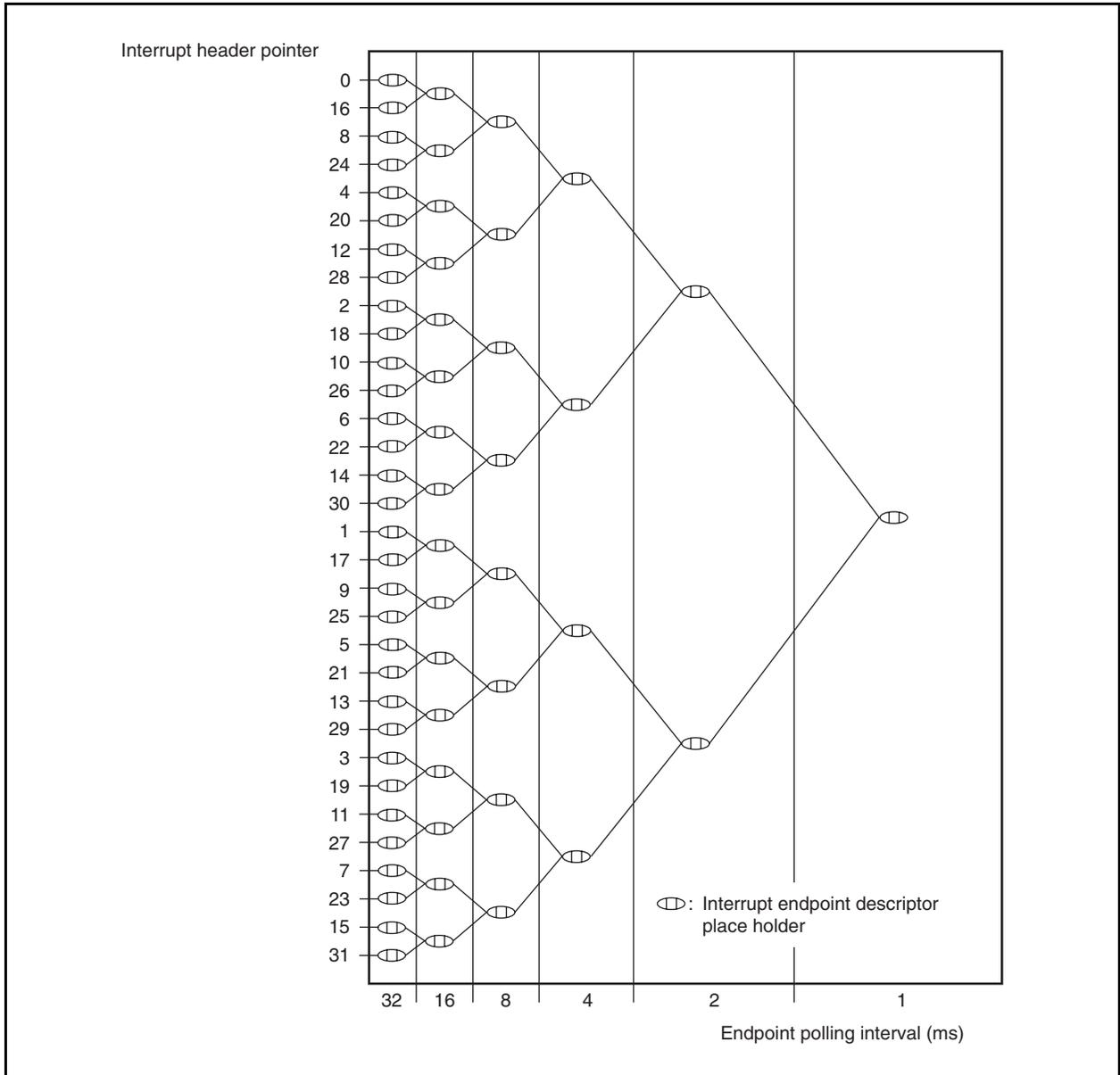
Figure 14-7 shows how OpenHCI allocates bandwidth. The HC selects the list to process based on a priority order algorithm. Control/bulk list processing has priority until the value of the FR area of the HcFmRemaining register from the beginning of the frame is the same as the value of the PS area of the HcPeriodicStart register.
