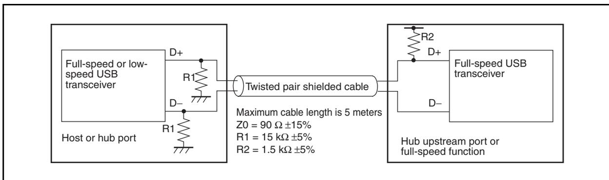
Figure 14-4. Low-Speed Device Cable and Resistor Connections
