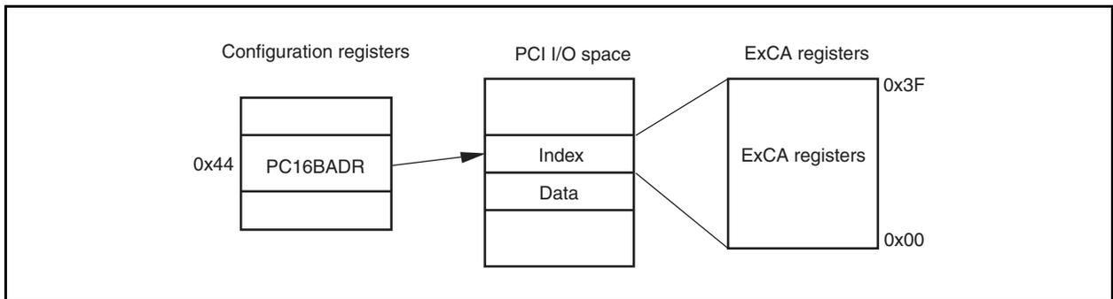
The ExCA registers also contain extended index and extended data registers.
