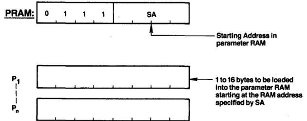
From the starting address, SA, any number of bytes may be loaded into the parameter RAM at incrementing addresses, up to location 15. The sequence of parameter bytes is terminated by the next command byte entered into the FIFO. The parameter RAM stores 16 bytes of information in predefined locations which differ for graphics and character modes. See the parameter RAM discussion for bit assignments.
