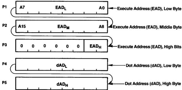
The Execute Address, EAD, points to the display memory word containing the pixel to be addressed. The Dot Address, dAD, within the word is represented as a 1-of-16 code for graphics drawing operations.
