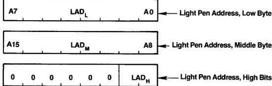
The light pen address, LAD, corresponds to the display word address, DAD, at which the light pen input signal is detected and deglitched.
