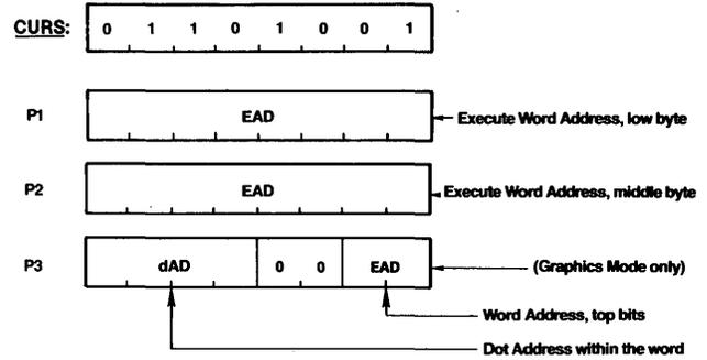
In character mode, the third parameter byte is not needed. The cursor is displayed for the word time in which the display scan address (DAD) equals the cursor address. In graphics mode, the cursor word address specifies the word containing the starting pixel of the drawing; the dot address value specifies the pixel within that word.
