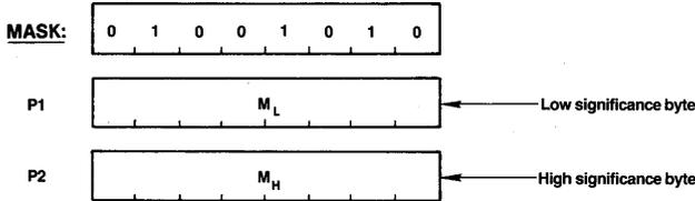
This command sets the value of the 16-bit Mask register of the figure drawing processor. The Mask register controls which bits can be modified in the display memory during a read-modify-write cycle.
