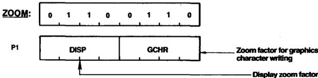
Zoom magnification factors of 1 through 16 are available using codes 0 through 15, respectively.
