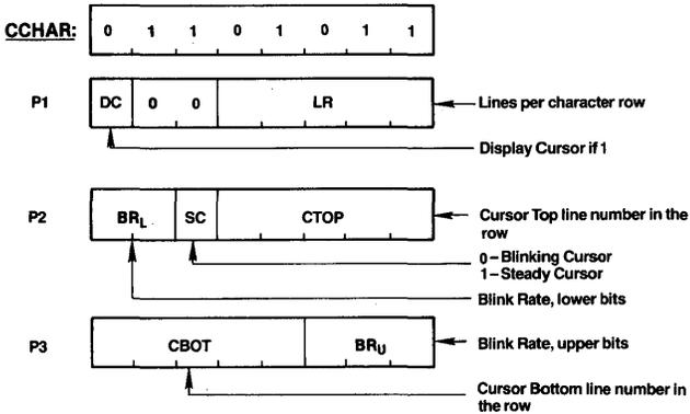
In graphics mode, LR should be set to 1. The blink rate parameter controls both the cursor and attribute blink rates. The cursor blink-on time = blink-off time = 2 x BR (video frames). The attribute blink rate is always 1/2 the cursor rate but with a 3/4 on-1/4 off duty cycle.
