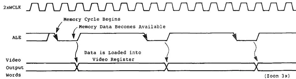
Figure 2.4 Pipelined Video System (Zoom = 3)
