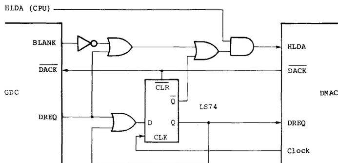
Figure 5.6 System Configuration for DMA Operation with Flashless Mode
