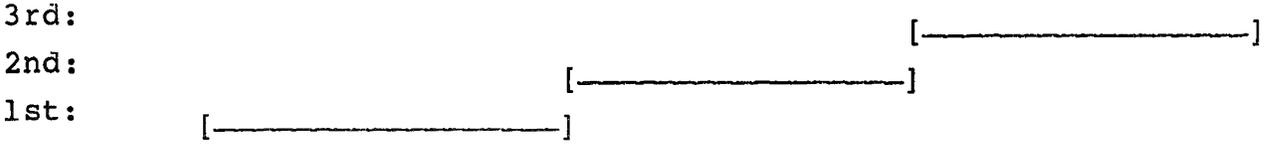
where [----] = a 16 bit word in display memory in the position it would appear in on the CRT screen.
