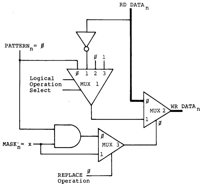
Figure 3.5a RMW Operation with:  $PATTERN_n = 0$ ,  $MASK_n = X$ ,
