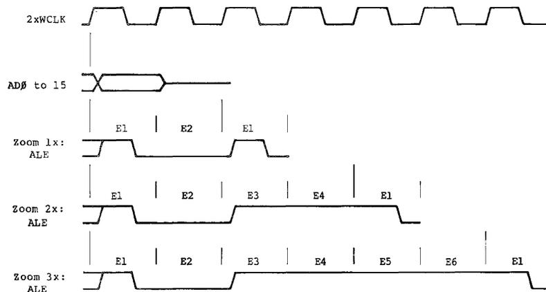
Figure 2.3 Zoom Magnified Display Cycles
