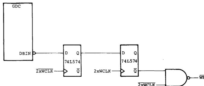
Figure 2.13 RMW Timing Generator
