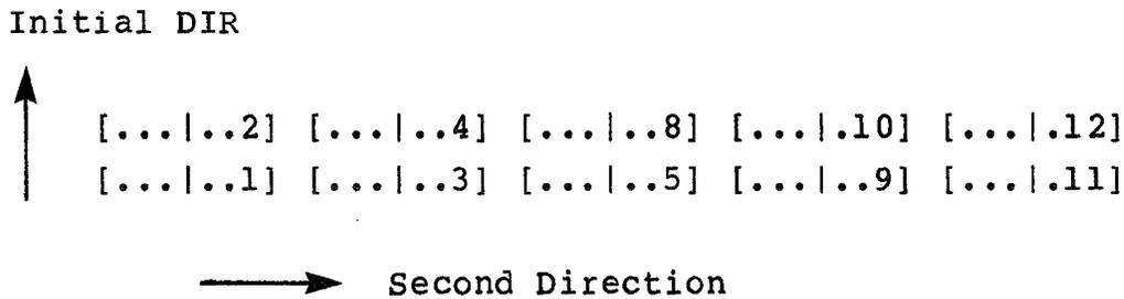
If the DC value is 0, the DMA transfers will be a one-dimensional sequence of accesses, rather than in a two-dimensional area. In this case, D controls the number of bytes to be transferred, up to 2\*\*14 or 16,384 bytes.
