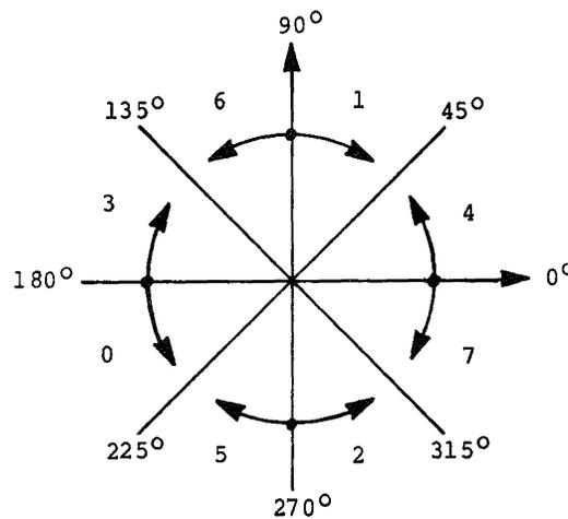
Figure 4.19 Arc Drawing Directions Around a Circle.
