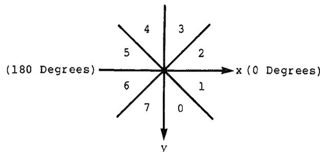
Figure 4.17 Octant Direction Definition
