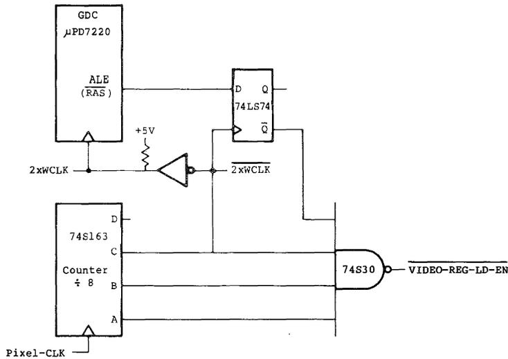
Figure 2.5 Video Register Load Enable Circuit (High Speed)
