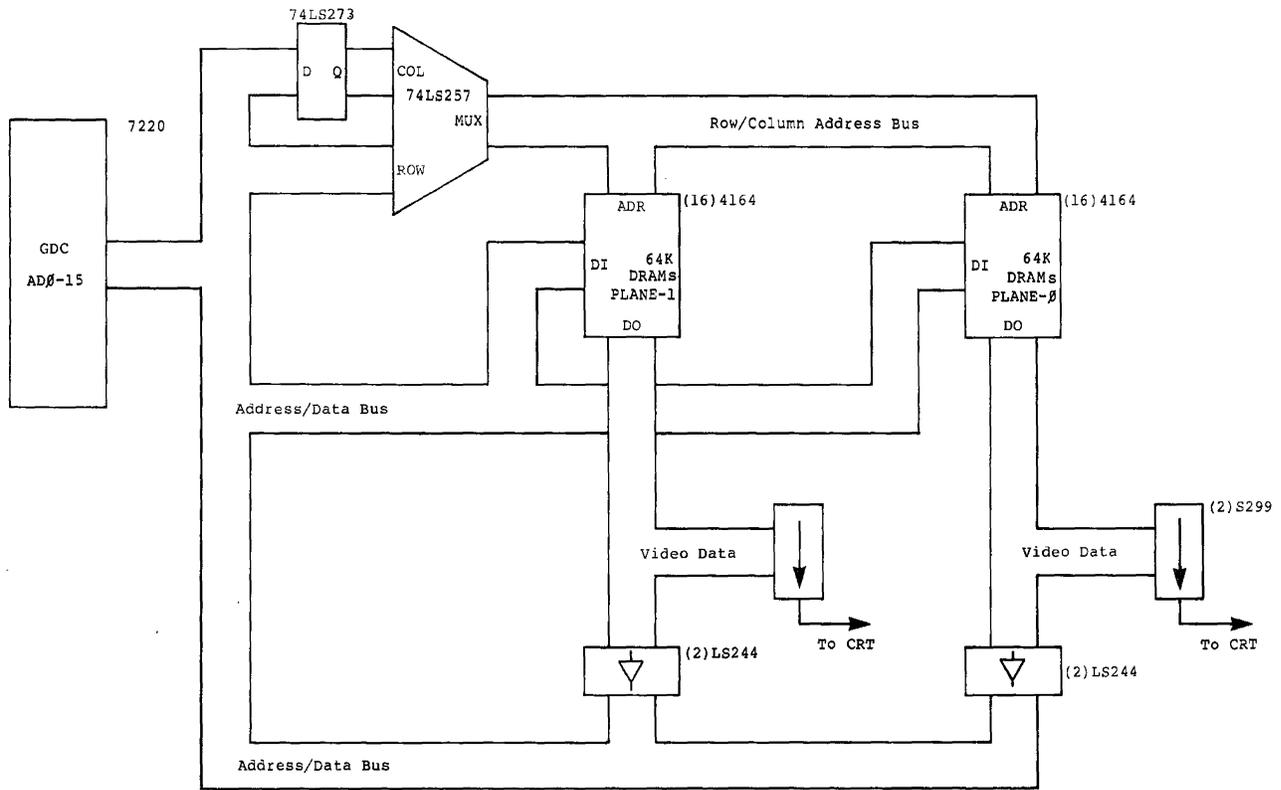
Figure A.1 Wide Display Cycle Memory Configuration
