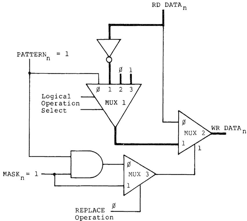
Figure 3.5c RMW Operation with: PATTERN<sub>n</sub> = 1, MASK<sub>n</sub> = 1, Logic Operation = 1, 2, 3
