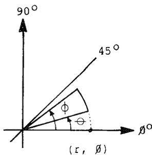
Figure 4.14. Arc Drawing Within an Octant
