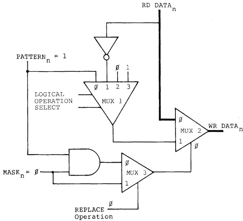
Figure 3.5b RMW Operation with: PATTERN<sub>n</sub> = 1, MASK<sub>n</sub> = 0, Logic Operation = 1, 2, 3
