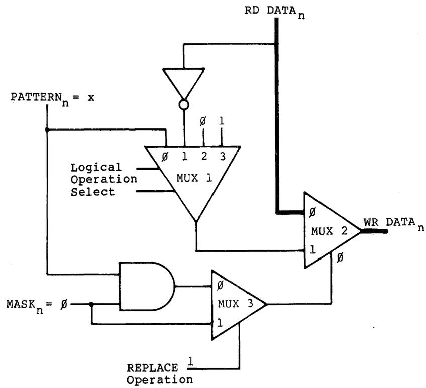
Figure 3.5d RMW Operation with: PATTERN<sub>n</sub> = x, MASK<sub>n</sub> = 0, Logic Operation = 0
