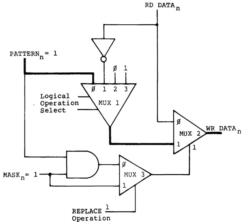
Figure 3.5e RMW Operation with: PATTERN<sub>n</sub> = 1, MASK<sub>n</sub> = 1, Logic Operation = 0
