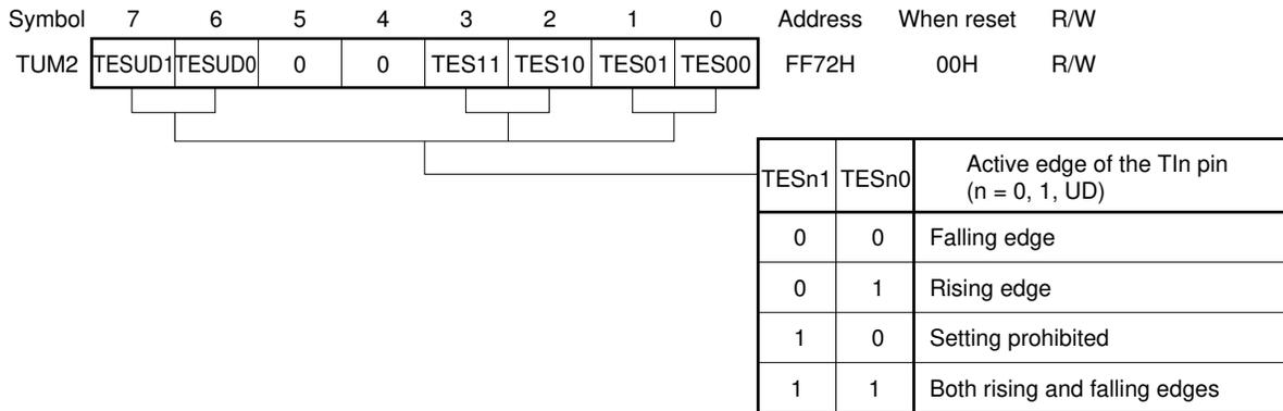
**Caution** When the operating mode for the UDC is specified as mode 4 (by the UDCC register), the specification of an edge for the TIUD pin (settings of the TESUD0 and TESUD1 bits) becomes ineffective.
