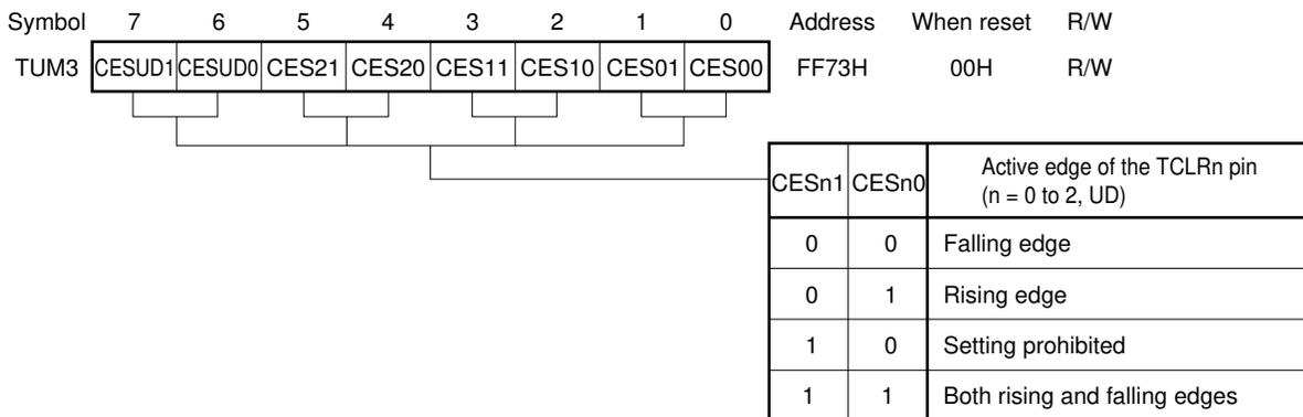
**7.2.2 Timer Control Registers (TMC0 to TMC2 and the UDCC)**
