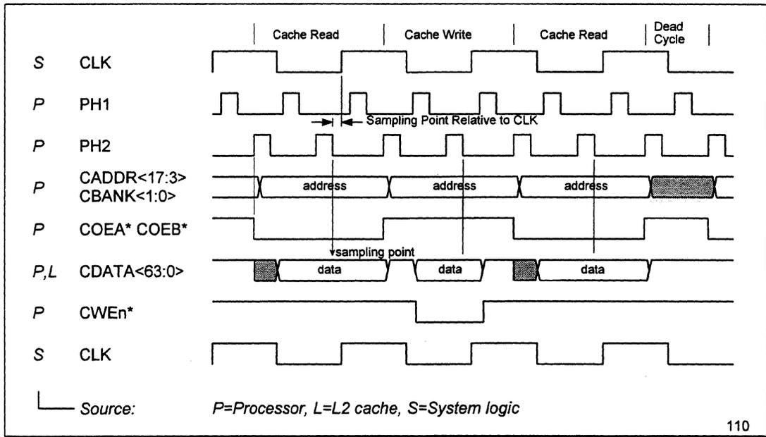
Figure 28 Level-2 Cache Read and Write
