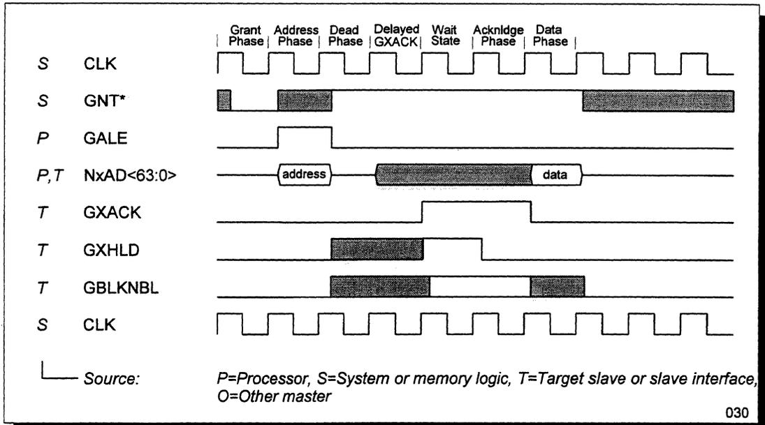
Figure 31 Single-Word Read with Wait States using a delayed GXACK
