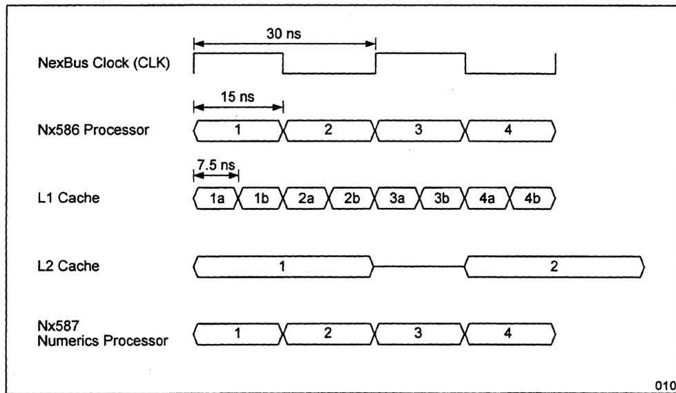
Figure 19 Operating Frequencies (66MHz Processor)
