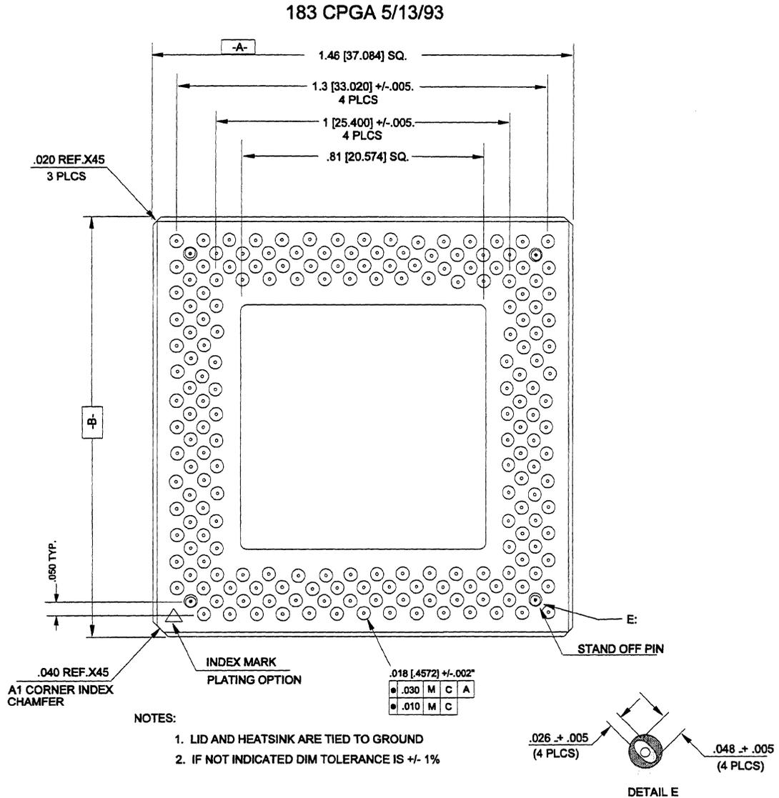
Figure 42 Nx587 Package Diagram (bottom)
