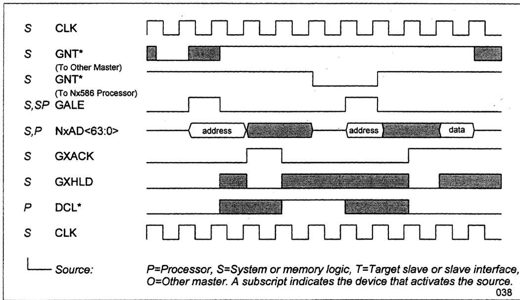
Figure 37 Single-Qword Read Hits Modified Cache Block
