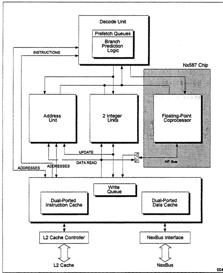
Figure 20 Nx586 Internal Architecture
