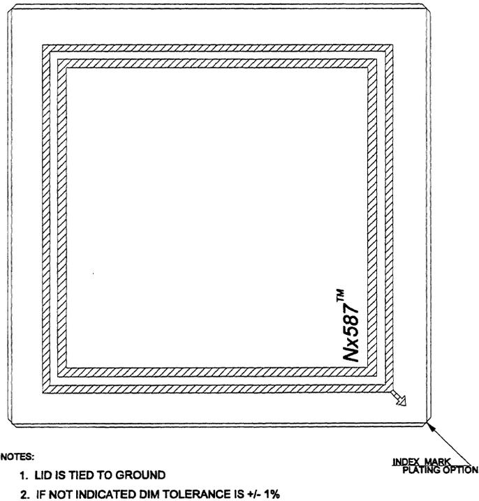
Figure 40 Nx587 Package Diagram (top)
