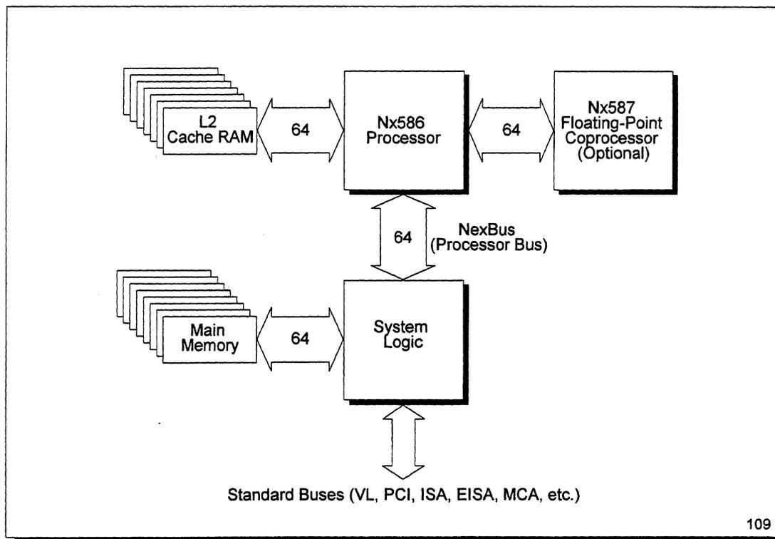
Figure 17 Nx586 based System Diagram
