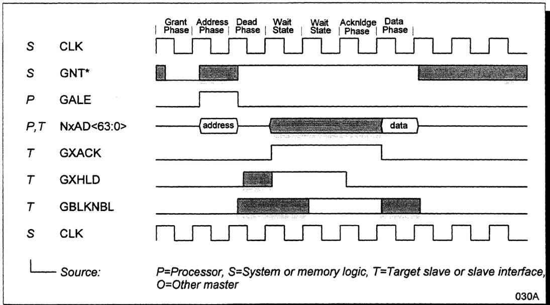
Figure 32 Single-Word Read with Wait States using GXHLD only
