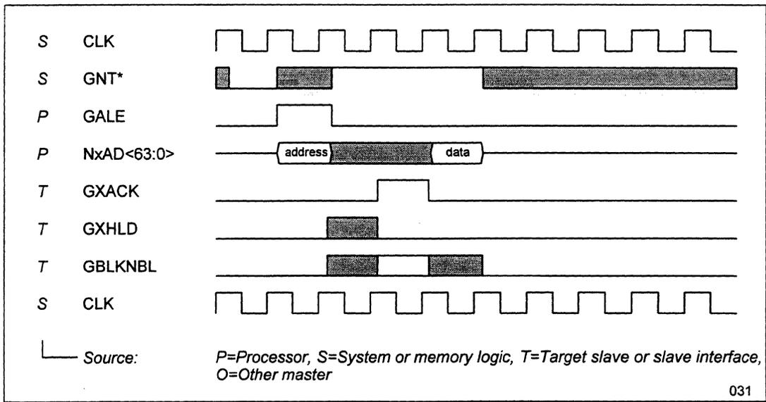
Figure 33 Fastest Single-Qword Write
