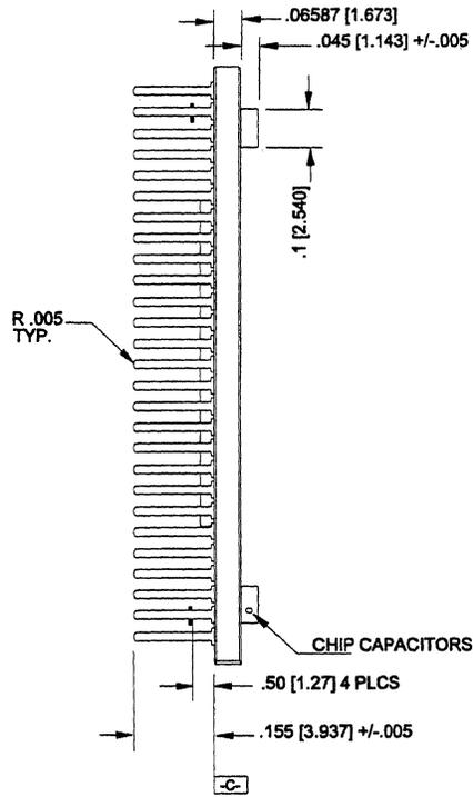
Figure 41 Nx587 Package Diagram (side)
