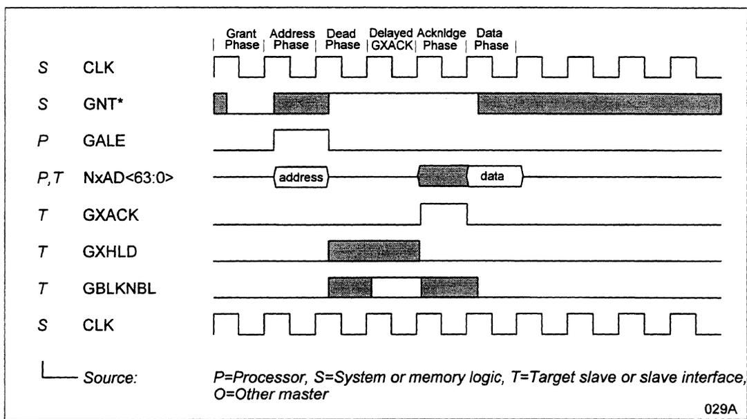
Figure 30 Fast Single-Word Read with a delayed GXACK
