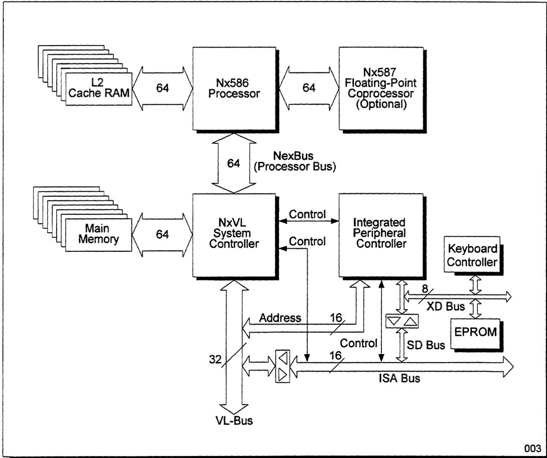
Figure 18 Nx586 based System using the NxVL Diagram
