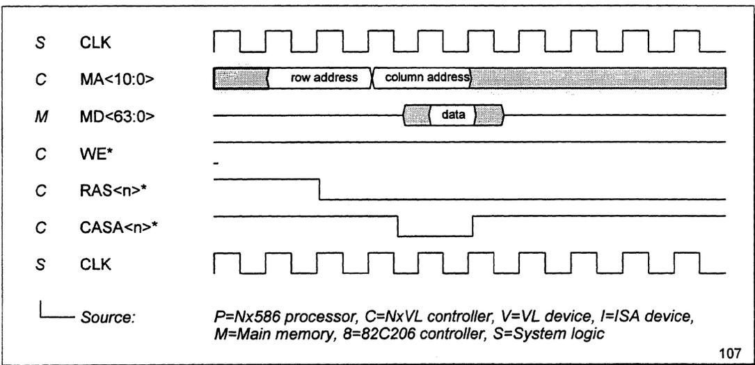
Figure 62 Fast Read from Main Memory (No Precharge)
