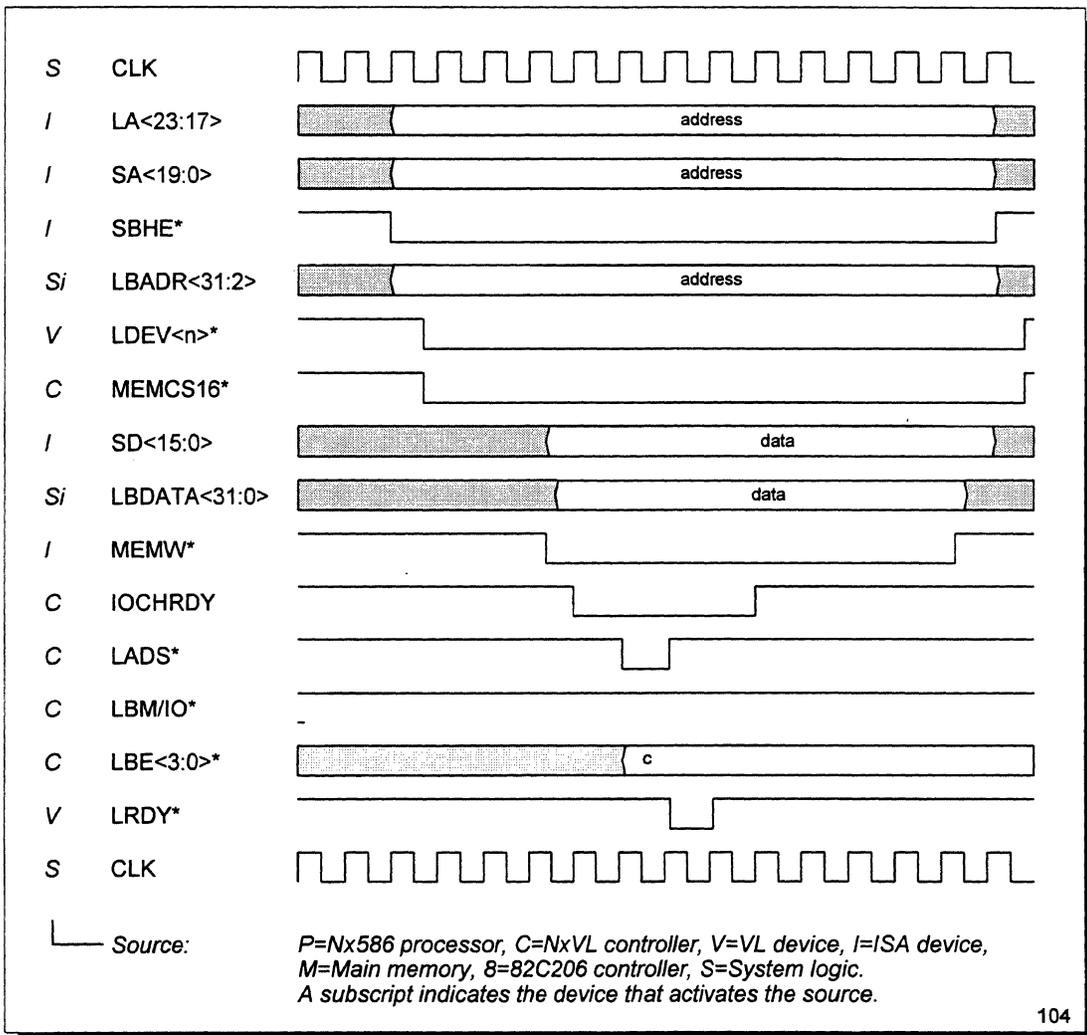
Figure 53 ISA-Master 16-Bit Write to VL-Bus Memory
