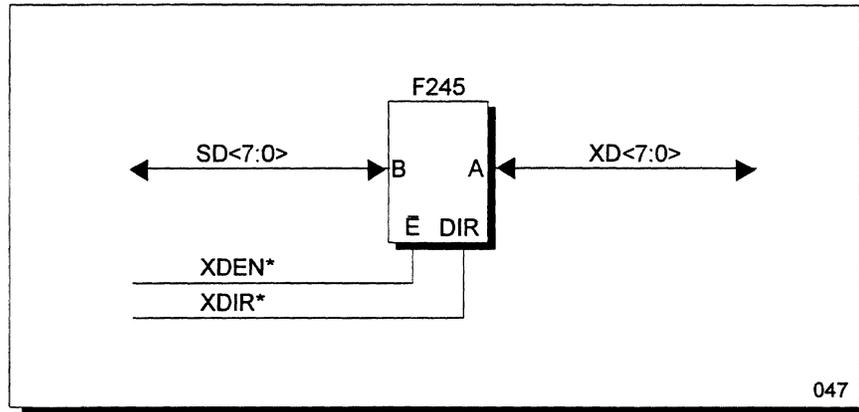
Figure 21 IPC SD-Bus to XD-Bus Data Transceiver
