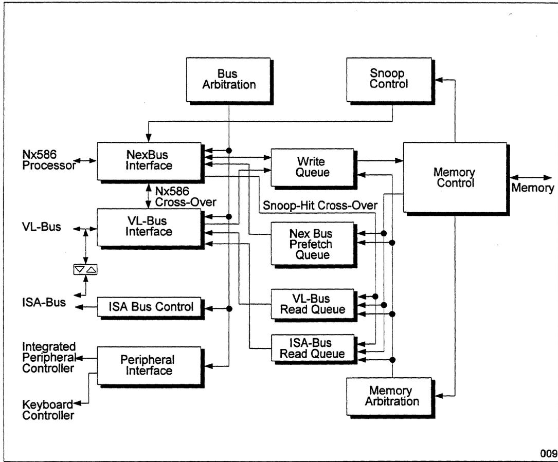
Figure 12 Internal Architecture
