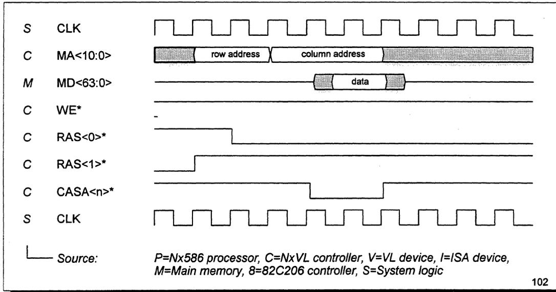
Figure 60 Slow Read from Main Memory (Overlapping Precharge)
