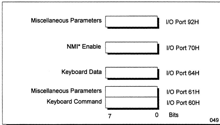
Figure 64 Configuration Registers (I/O-Mapped)
