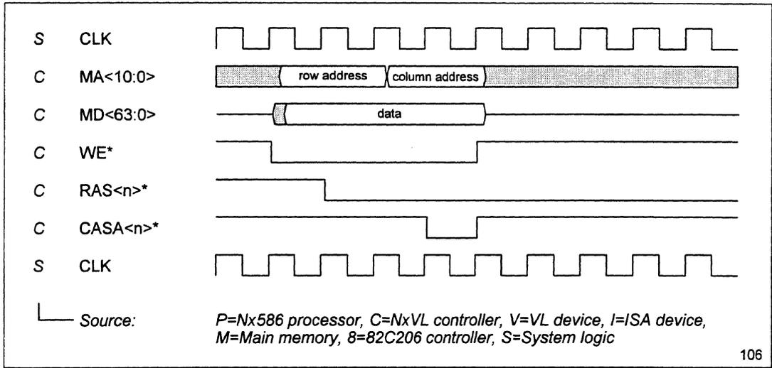
Figure 61 Fast Write to Main Memory (No Precharge)
