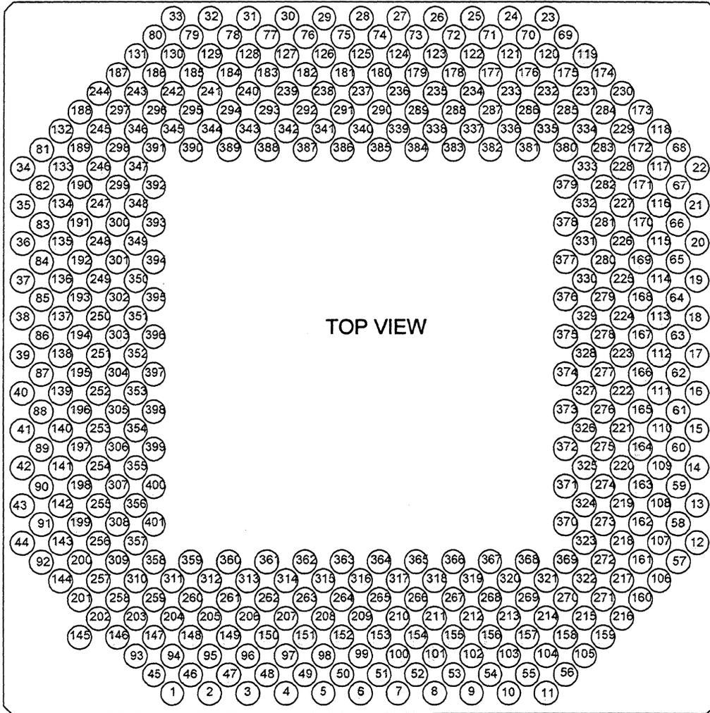
Figure 6 NxVL Pinout Diagram (Top View)
