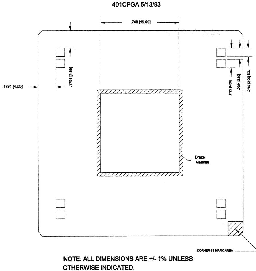
Figure 68 NxVL Package Diagram (top)
