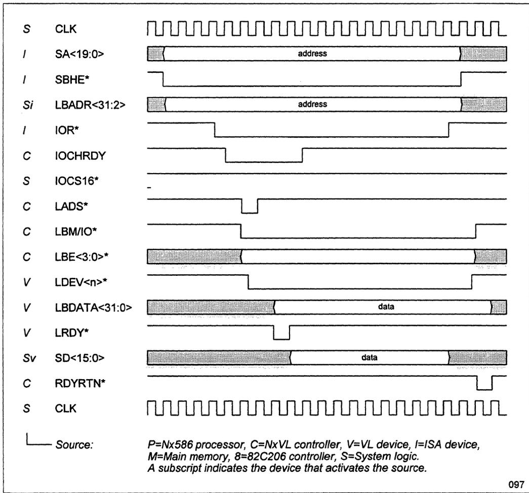
Figure 54 ISA-Master 16-Bit Read from VL-Bus I/O
