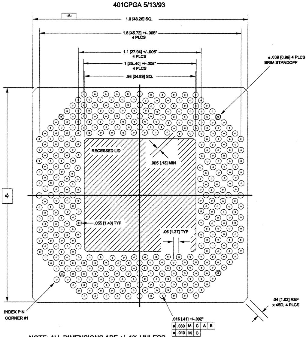
Figure 70 NxVL Package Diagram (bottom)
