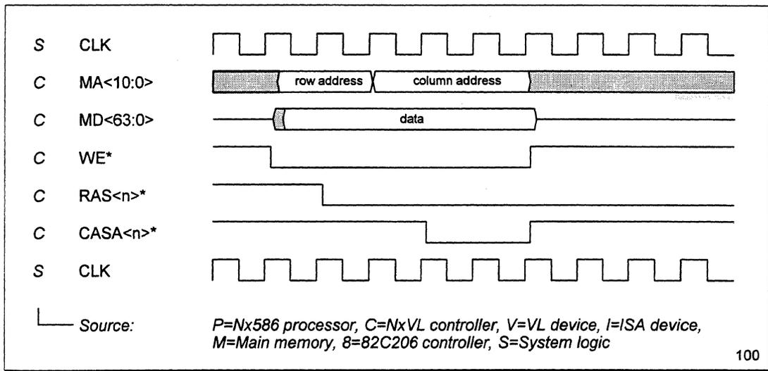
Figure 58 Slow Write to Main Memory (No Precharge)
