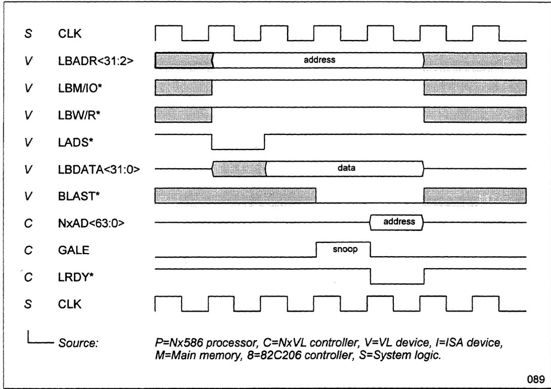
Figure 45 VL-Master 32-Bit Write to Main Memory
