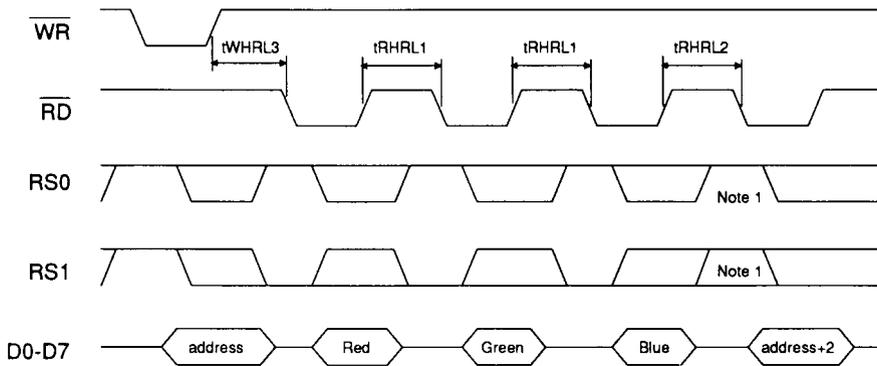
Note 1: The timing for reading from address 0.0 is identical to that for reading from address 1.1.
