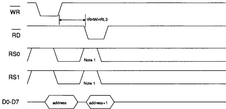
Note 1: The timing for reading from address 0.0 is identical to that for reading from address 1.1.
