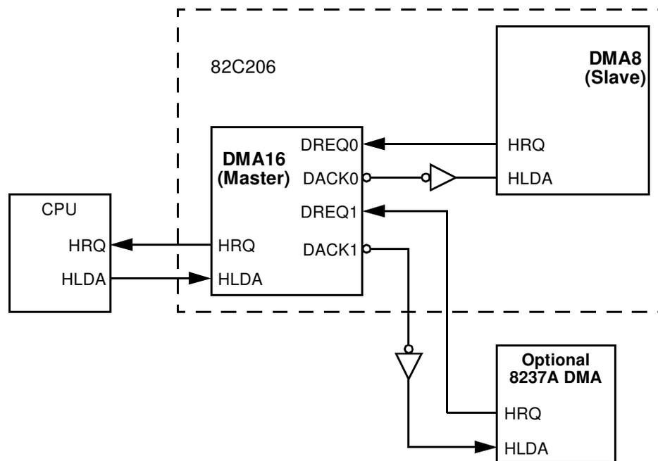
When programming cascaded controllers, begin with the device which is actually generating HRQ to the system (first level device) and then proceed to the second level devices. RESET causes the DACK outputs to become active low and
