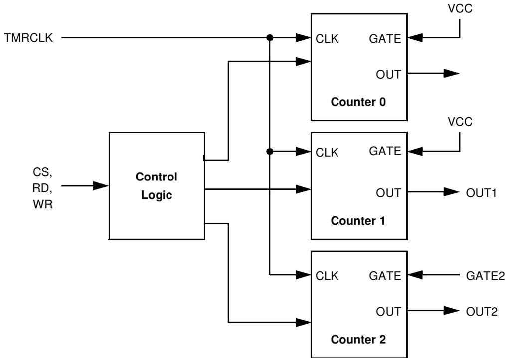
The 16-bit counting component is a loadable synchronous down counter. It is loaded or decremented on the falling edge of TMRCLK. The counting component contains a maximum count when a 0 is loaded, which is equivalent to 65536 in binary operation or 1000 in BCD. The counting component does not stop when it reaches 0. In Modes 2 and 3, the counting component will be reloaded and in all other modes it will wrap around to 0FFFFh in binary operation or 9999 in BCD.
