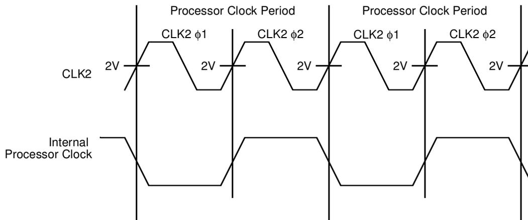
CLK2 is a master 2X clock which is used to drive all host CPU synchronous signals and the 82C295's internal state machines. CLK2 is also used by the cache/DRAM controller logic and to maintain the clock phase between the CPU and the 82C295.
