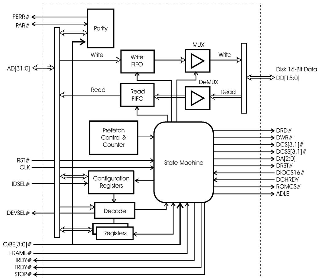
Figure 2-2 Example PCI Controller Block Diagram
