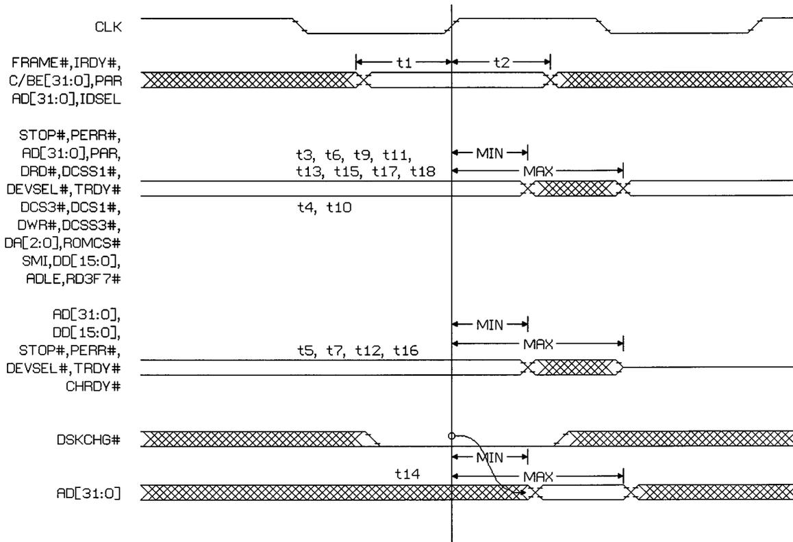
Figure 6-4 32-Bit I/O Access - Buffer Full
