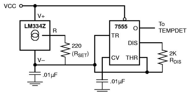
The following equation describes the output frequency of this circuit.
