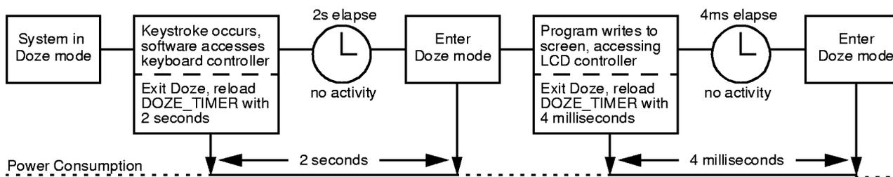
**Setup:** DOZE\_0 = 2 seconds, SYSCFG 41h[7:5] = 110      Link KBD\_ACCESS to DOZE\_0, SYSCFG 76h[6] = 0
