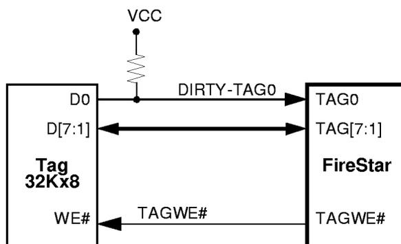
Figure 4-9 32Kx8 and 32Kx8 Combined Tag/Dirty RAM Implementation (Separate Devices)
