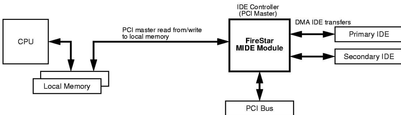
**Figure 4-33 Multi-Word DMA Transfer Mode**
