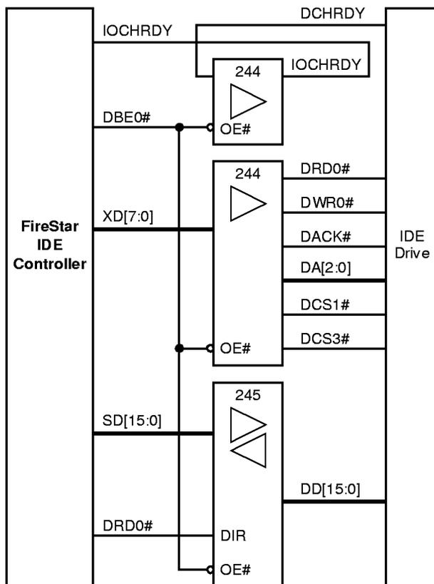
Figure 4-28 IDE Interface Using Zero-TTL
