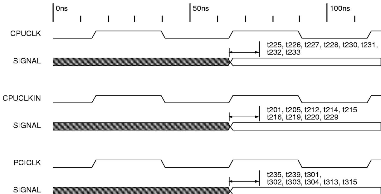
Figure 6-4 Float Delay Timing Waveform
