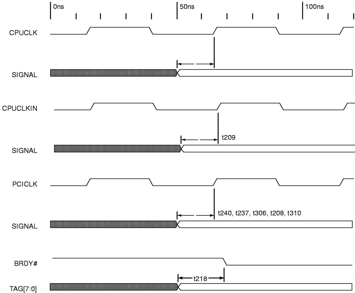
Figure 6-2 Hold Timing Waveform
