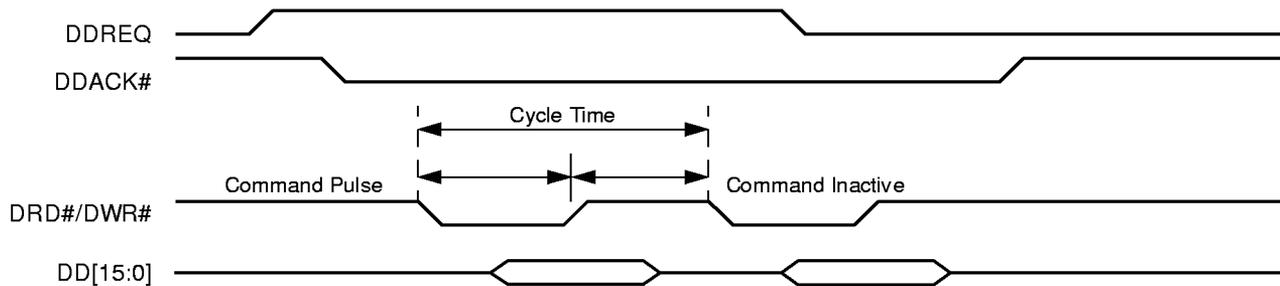
**Figure 4-34 Single-Word DMA Transfer Mode**
