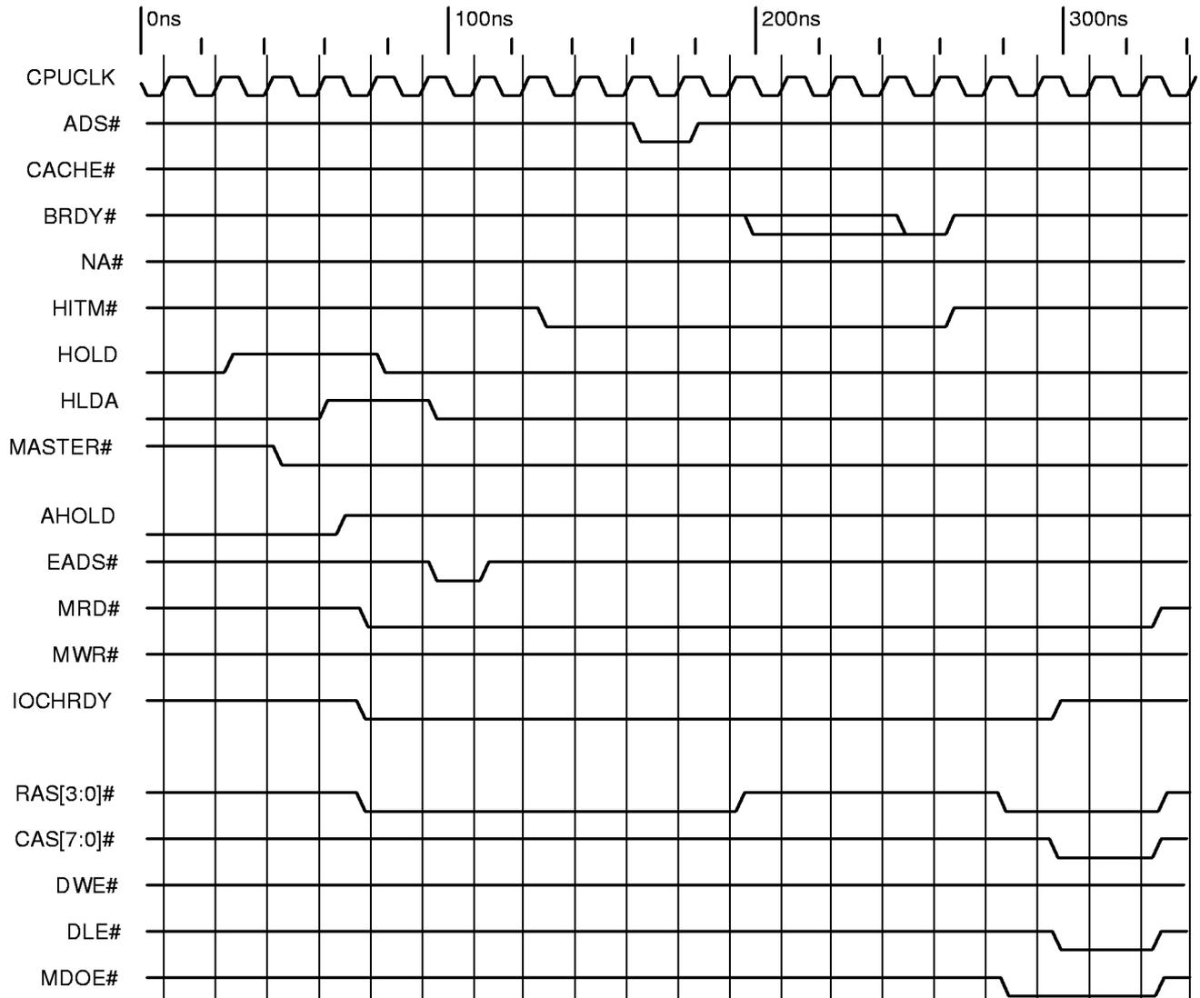
Figure 4-12 ISA DMA/Master Write (L1 cache with modified line)
