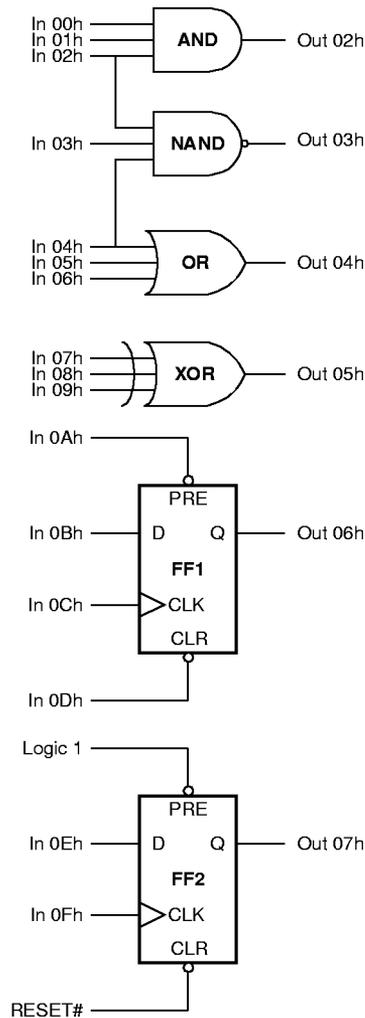
The gate inputs and outputs can be connected directly to PIO pins, or can be connected to each other for multi-level logic development as described in the example below and using the Gate Matrix registers shown in Table 3-5.
