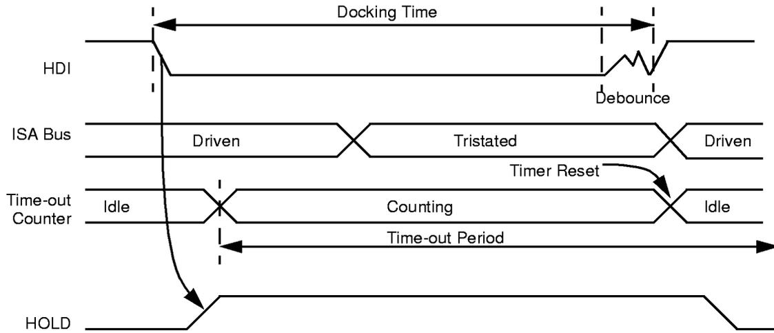
Figure 4-44 HDI Input Not Deasserted Within Time-out Period (SMI generated on time-out)
