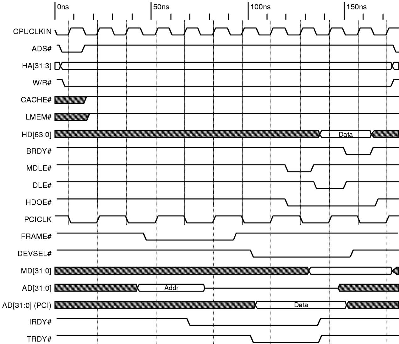
Figure 4-16 CPU 32-Bit Write to PCI
