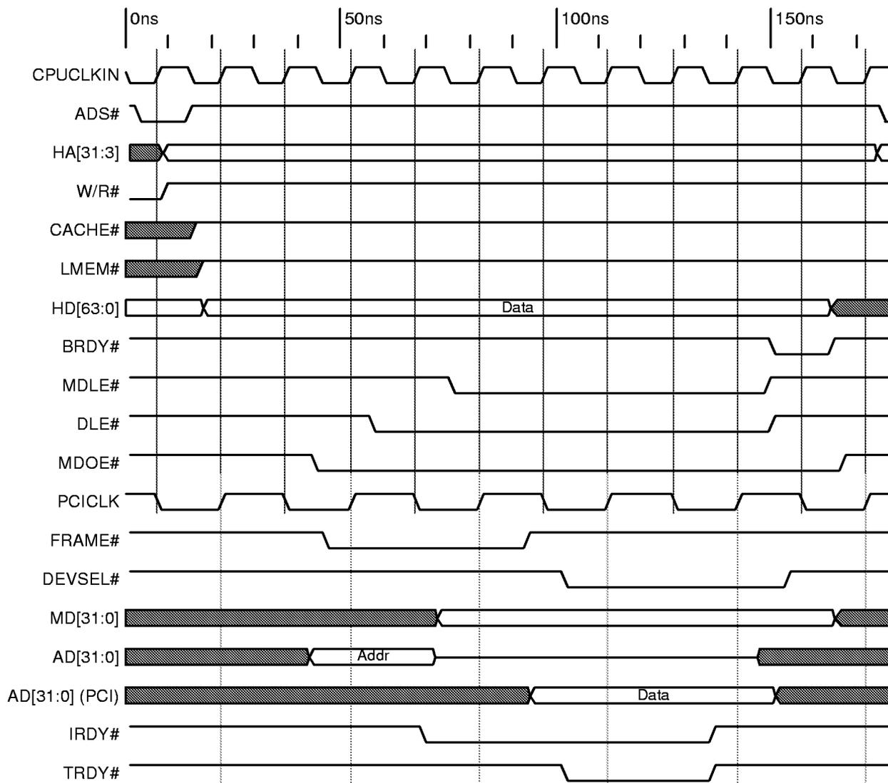
Figure 4-17 CPU 64-Bit Read from PCI
