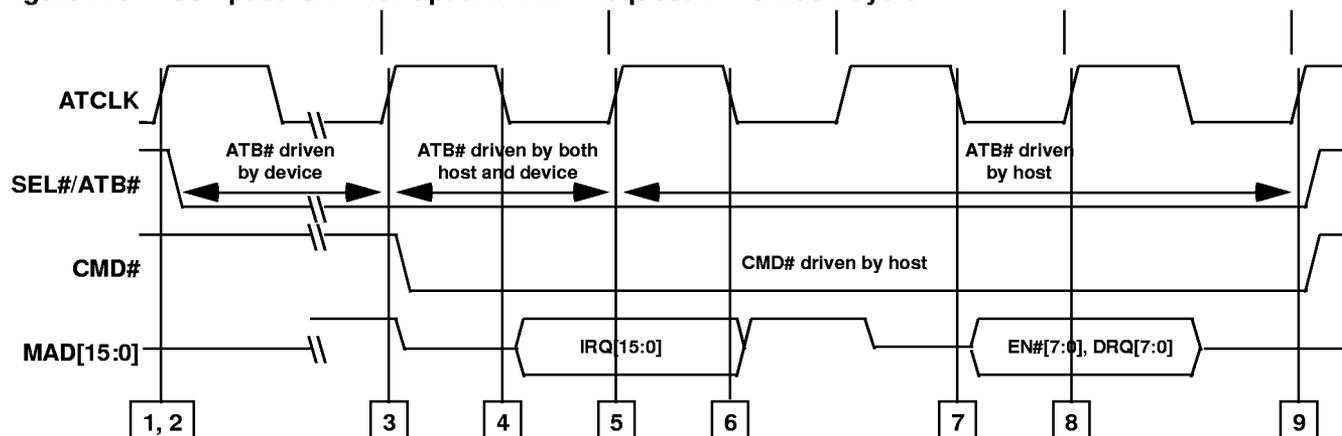
1. CISA Peripheral device must sample SEL#/ATB# and CMD# high, and ALE low, on TWO consecutive rising edges of ATCLK.
