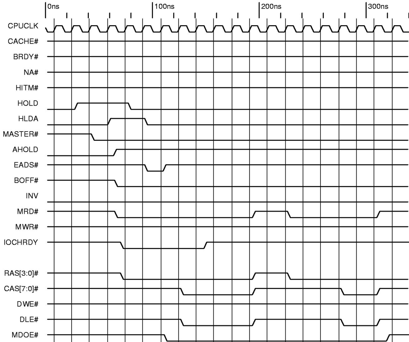
Figure 4-11 ISA DMA/Master Read (L1 cache with modified line)
