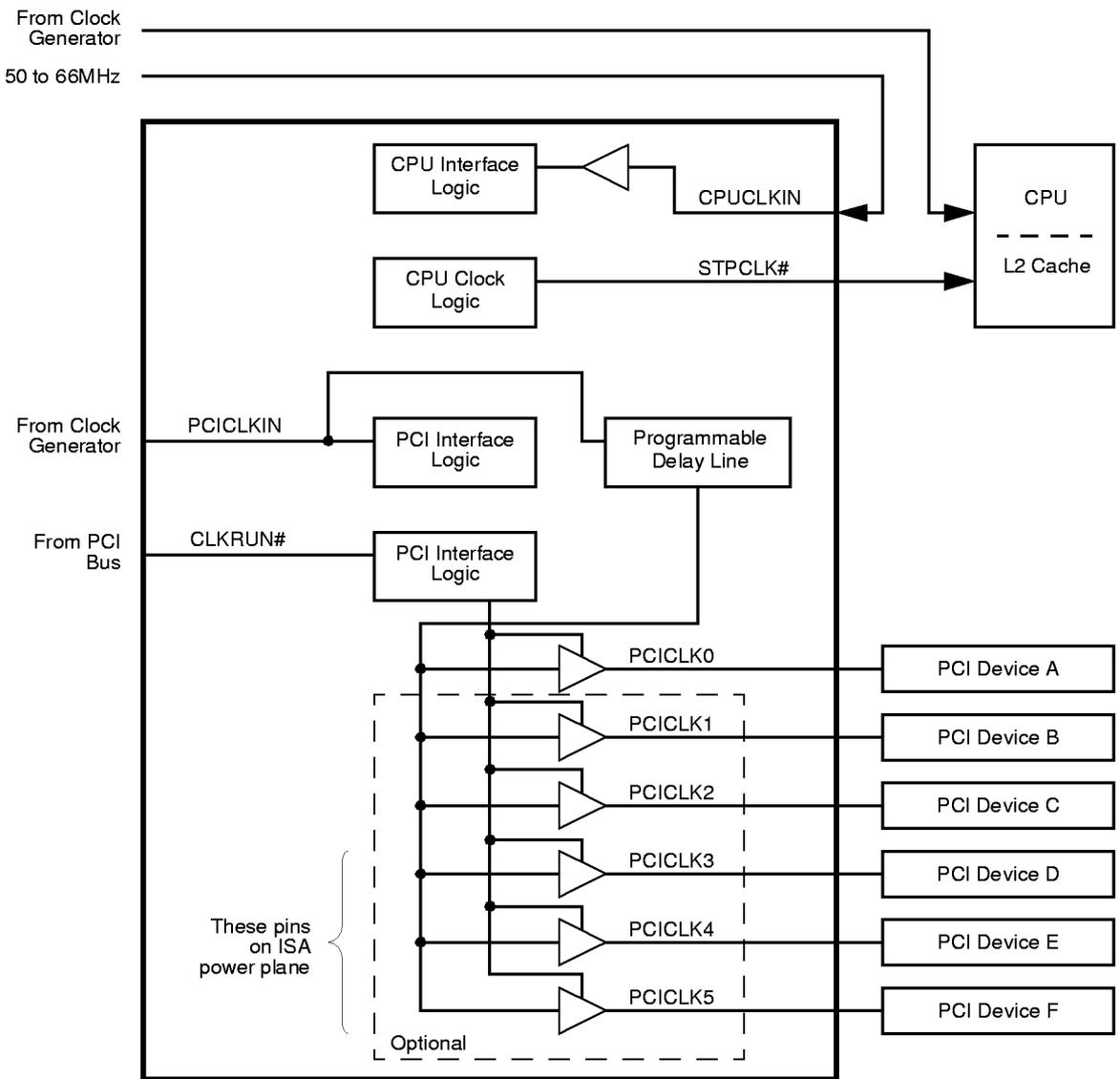
Each PCICLK output is individually controlled by the CLK-RUN# circuitry. In this way, devices that do not support CLK-RUN# can be supported along with those that do.
