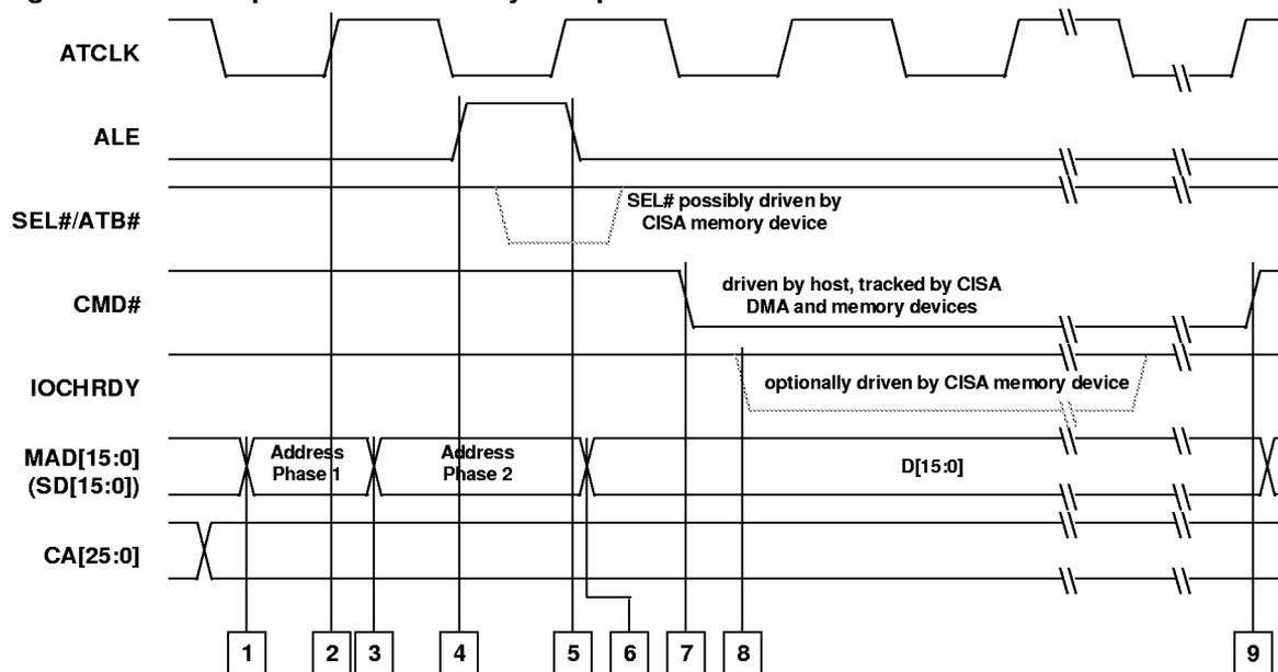
1. CISA host gets address from the CPU address lines and byte enable lines. The host then drives out  $A[23:0] + I/D\# = 0 + M/I\# = 0$  (DACK# cycle).
