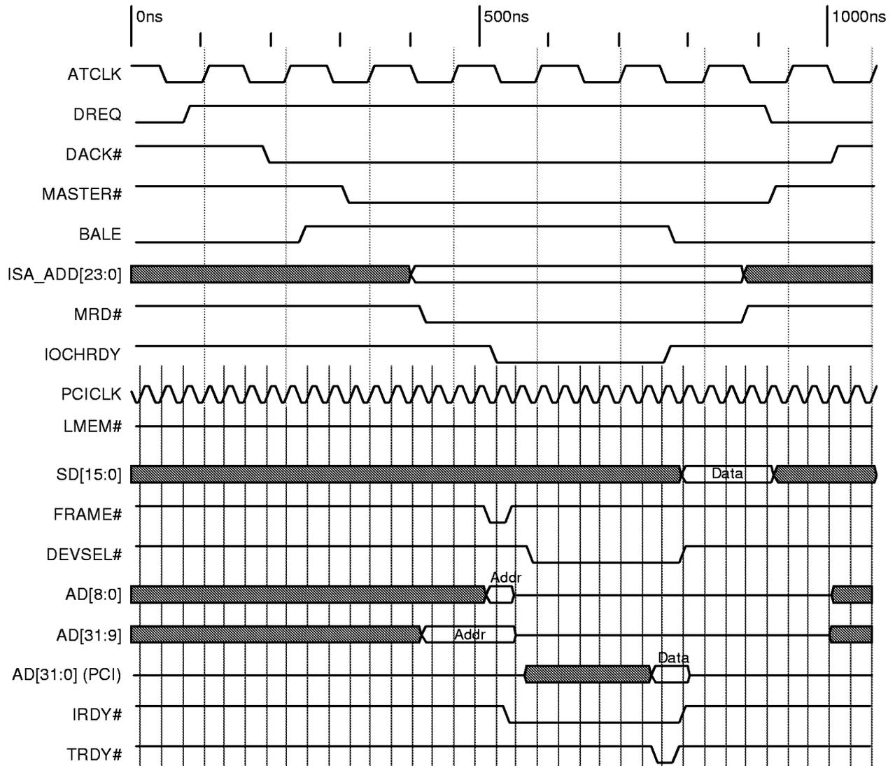
Figure 4-19 ISA Master Write to PCI
