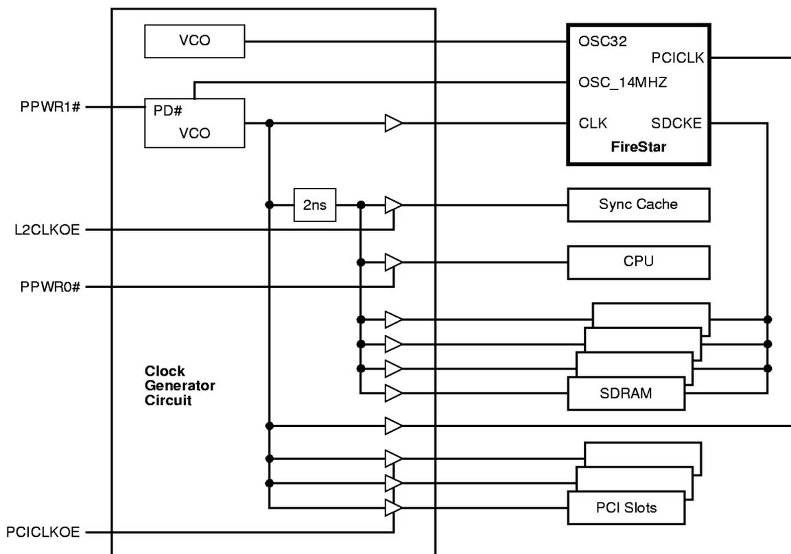
**Note:** All control inputs are high for operation and low for stop.
