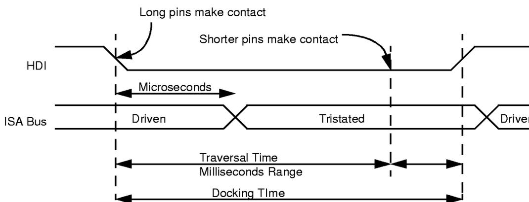
Figure 4-43 HDI Input Deasserted Within Time-out Period
