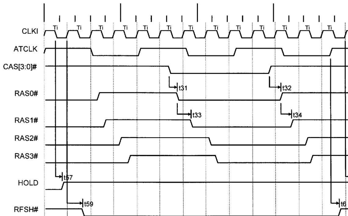
Figure 6-18 DMA Read Cycle
