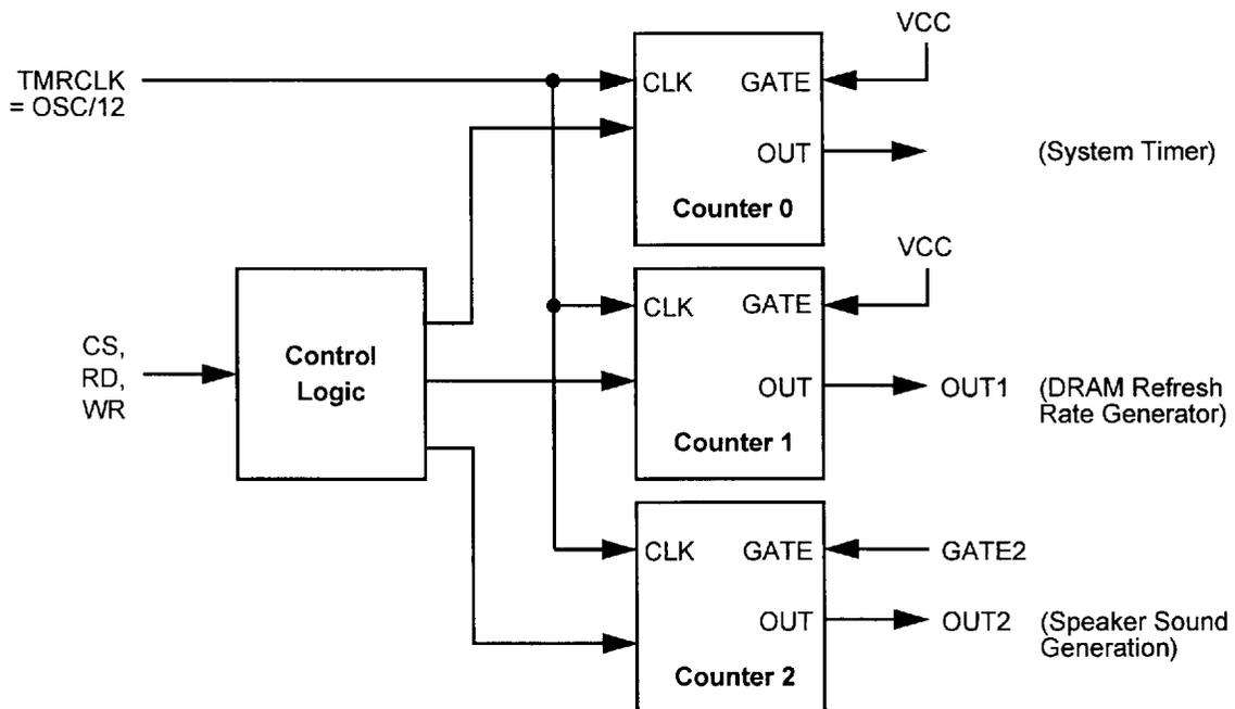
The 16-bit counting component is a loadable synchronous down counter. It is loaded or decremented on the falling edge of TMRCLK. The counting component contains a maximum count when a 0 is loaded, which is equivalent to 65536 in binary operation or 1000 in BCD. The counting component does not stop when it reaches 0. In Modes 2 and 3, the counting component will be reloaded and in all other modes it will wrap around to 0FFFFh in binary operation or 9999 in BCD.
