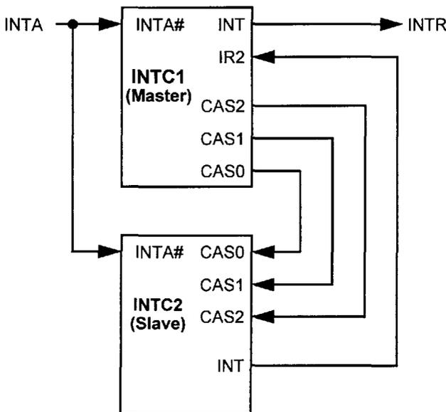
**Note:** INTA will be active when the CPU initiates an interrupt acknowledge cycle.
