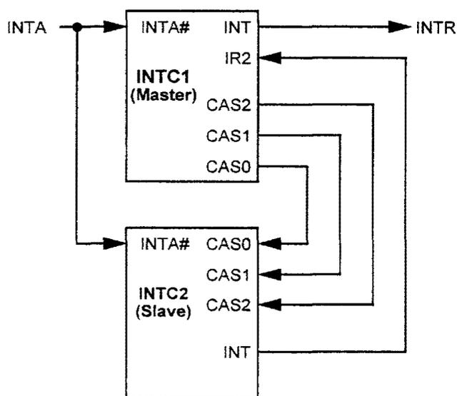
Note: INTA will be active when the CPU initiates an interrupt acknowledge cycle.
