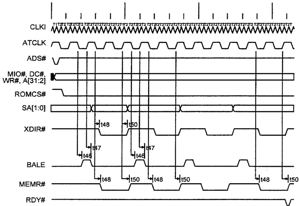
Figure 6-23 Keyboard Controller Access Cycle
