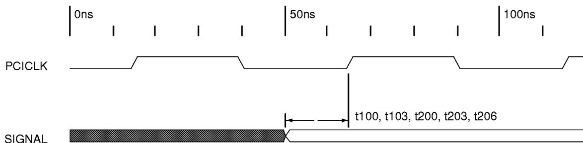
Figure 6-2 Hold Timing Waveform
