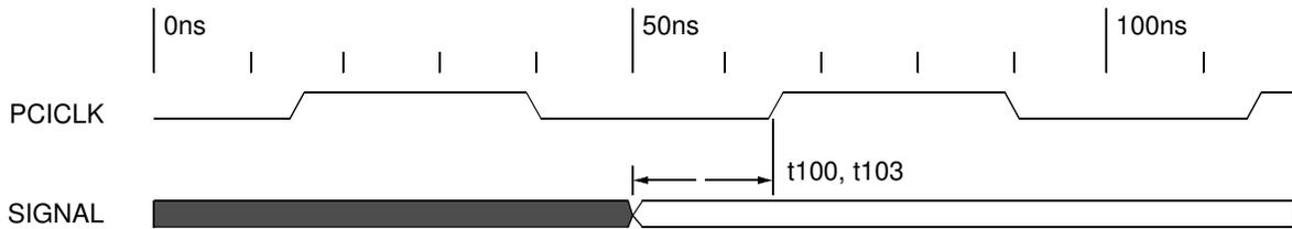
**Figure 6-2 Hold Timing Waveform**
