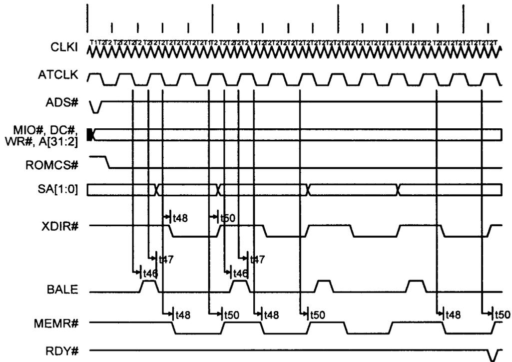
**Figure 6-23 Keyboard Controller Access Cycle**
