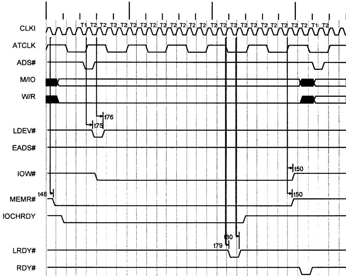
Figure 6-19 DMA Write Cycle
