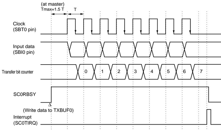
**Figure 11-3-12 Reception Timing (falling edge, start condition is disabled)**
