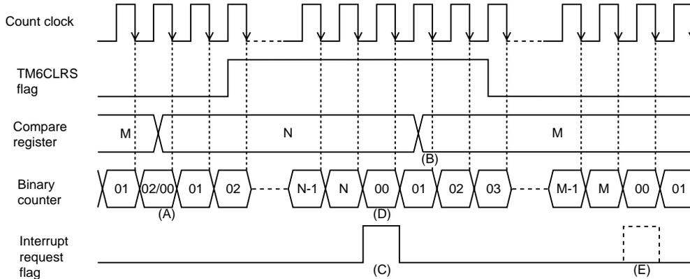
**Figure 8-3-2 Count Timing of Timer Operation (Timer 6)**
