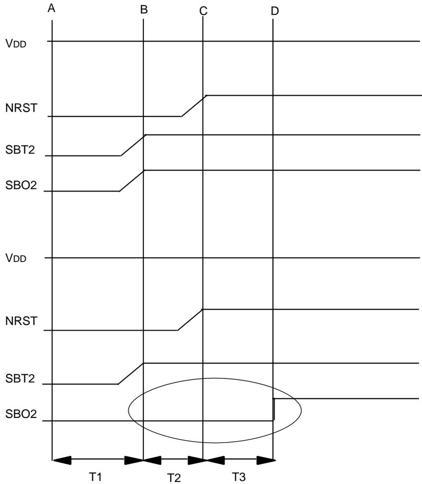
Timing waveform during serial programming
