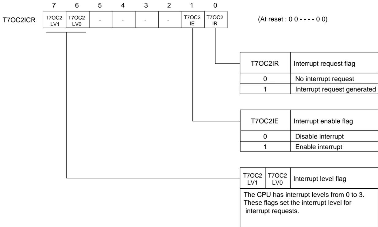
**Figure 3-2-16 Timer 7 Compare Register 2-match Interrupt Control Register (TMO C2ICR : x'03FF2', R/W)**
