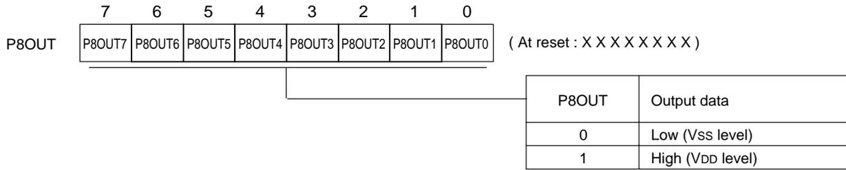
Port 8 output register (P8OUT : x'03F18', R/W)
