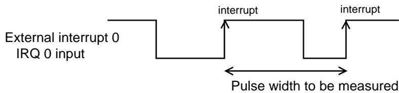
**Figure 7-9-3 Pulse Width Measurement of External Interrupt 0**
