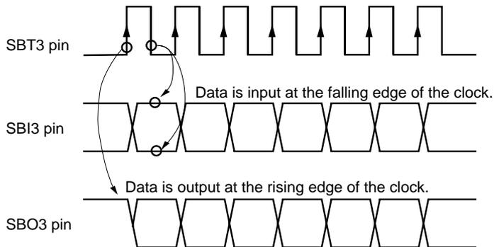
**Figure 14-3-11 Transmission/Reception Timing
