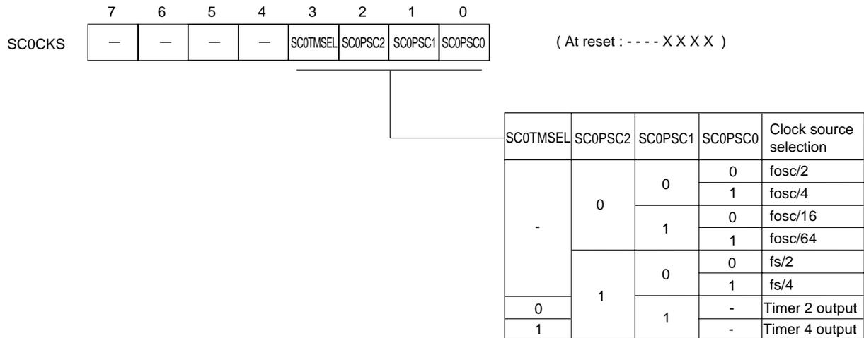
Figure 5-2-7 Serial Interface 0 Transfer Clock Selection Register (SC0CKS : x'03F97', R/W)
