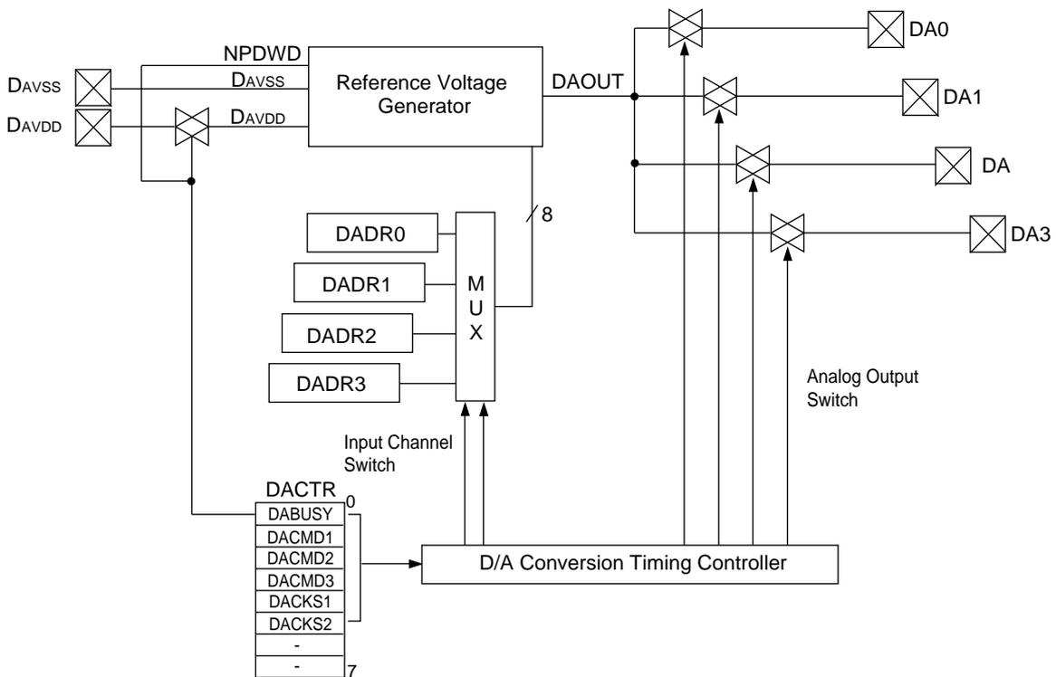
Figure 17-1-1 D/A Converter Block Diagram
