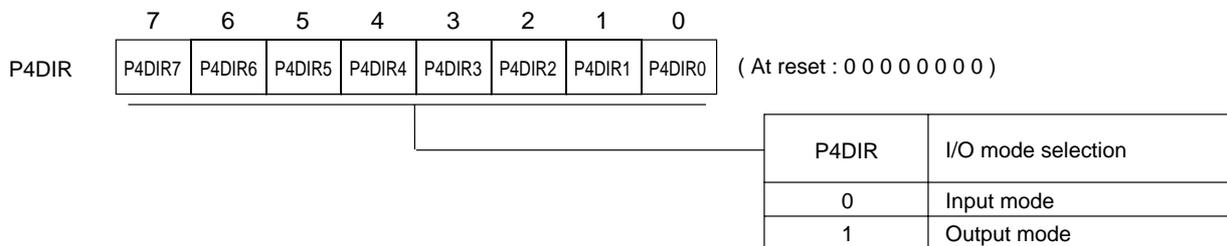
Port 4 direction control register (P4DIR : x'03F34', R/W)
