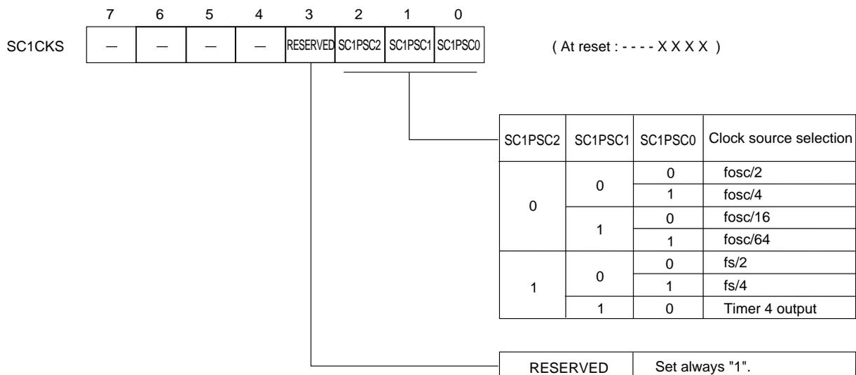
Figure 5-2-8 Serial Interface 1 Transfer Clock Selection Register (SC1CKS : x'03F9F', R/W)
