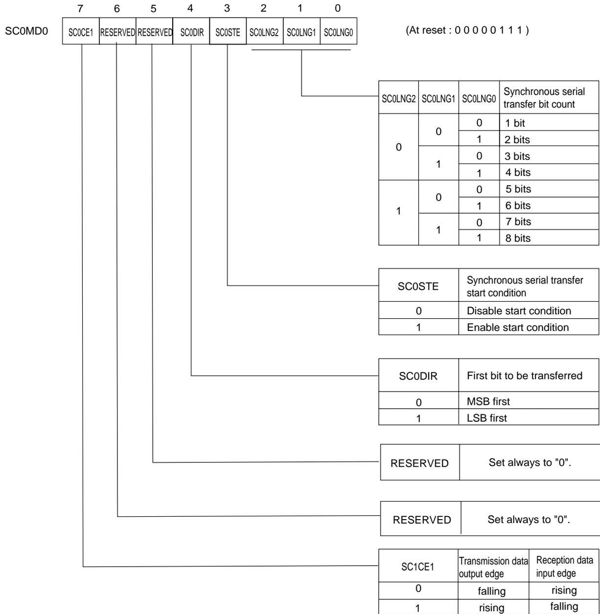
Figure 11-2-3 Serial Interface 0 Mode Register 0 (SC0MD0 : x'03F90', R/W)
