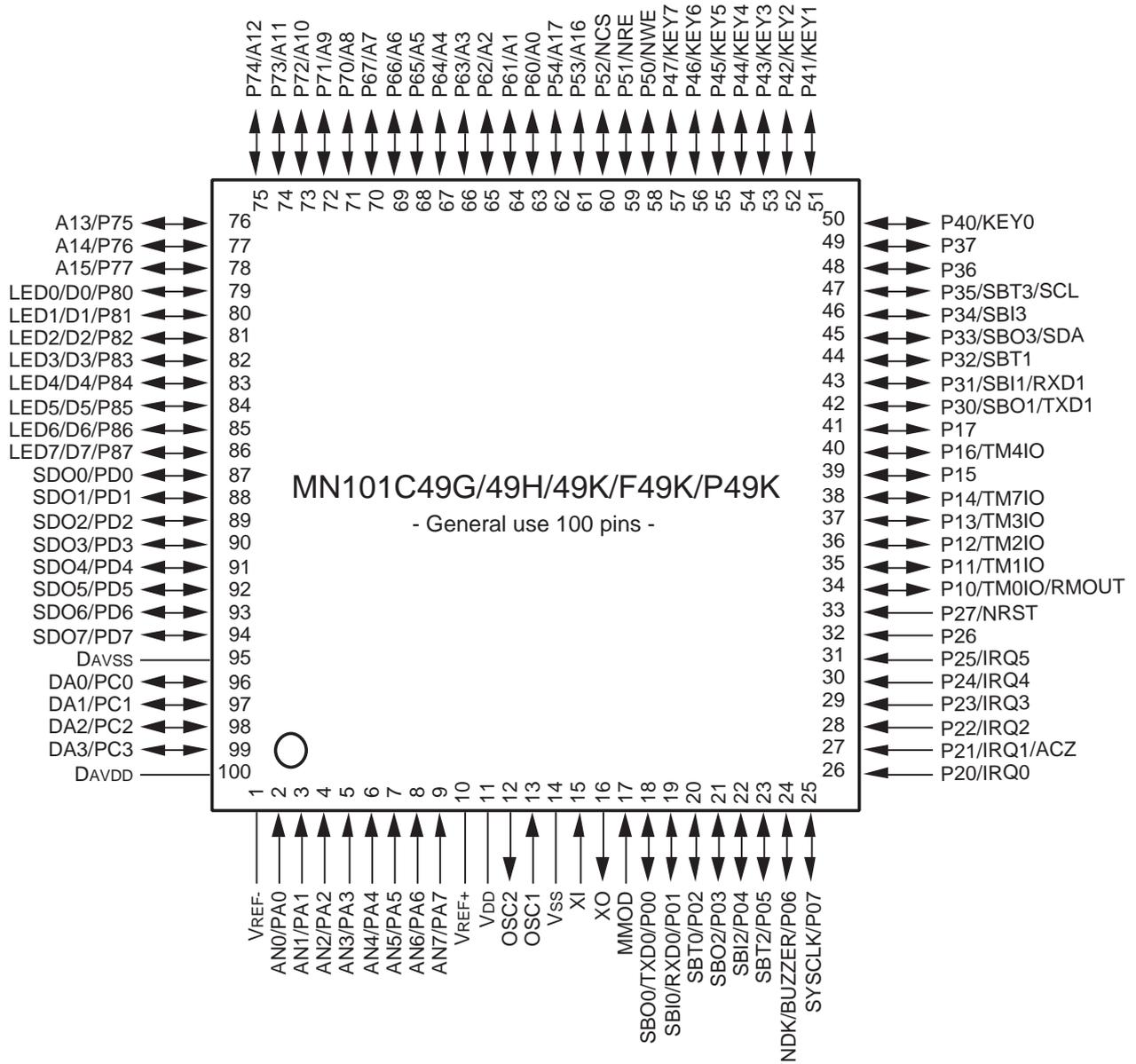
Figure 1-3-1 Pin Configuration ( 100QFP/100LQFP : Top view )
