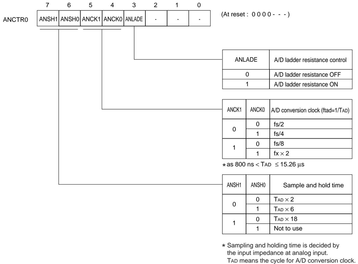
Figure 16-2-1 A/D Converter Control Register 0 (ANCTR0 : x'03FB0', R/W)
