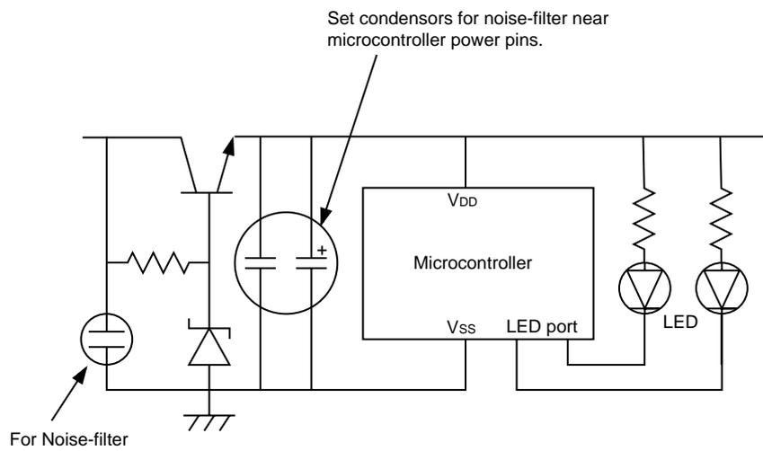
**Figure 1-7-6 An Example for Emitter follower type Power Supply Circuit**
