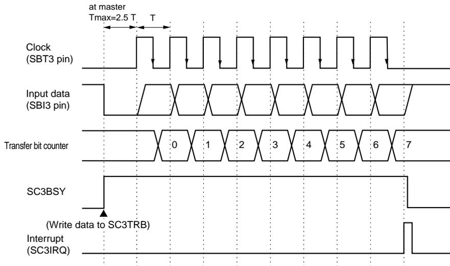
**Figure 14-3-8 Reception Timing (Falling edge, Enable Start Condition)**
