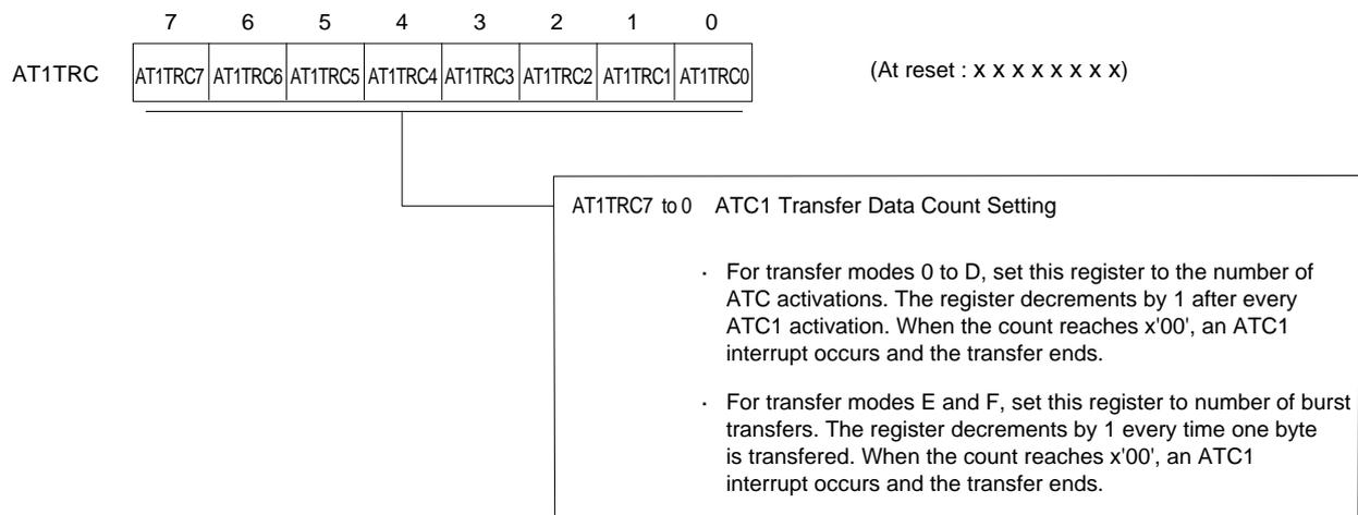
Figure 15-2-3 ATC1 Transfer Data Counter (AT1TRC : x'03FD2', R/W)
