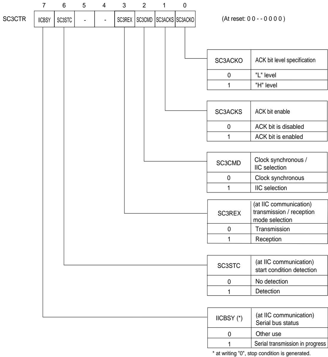
Figure 14-2-4 Serial Interface 3 Control Register (SC3CTR : x'03FAA', R/W)
