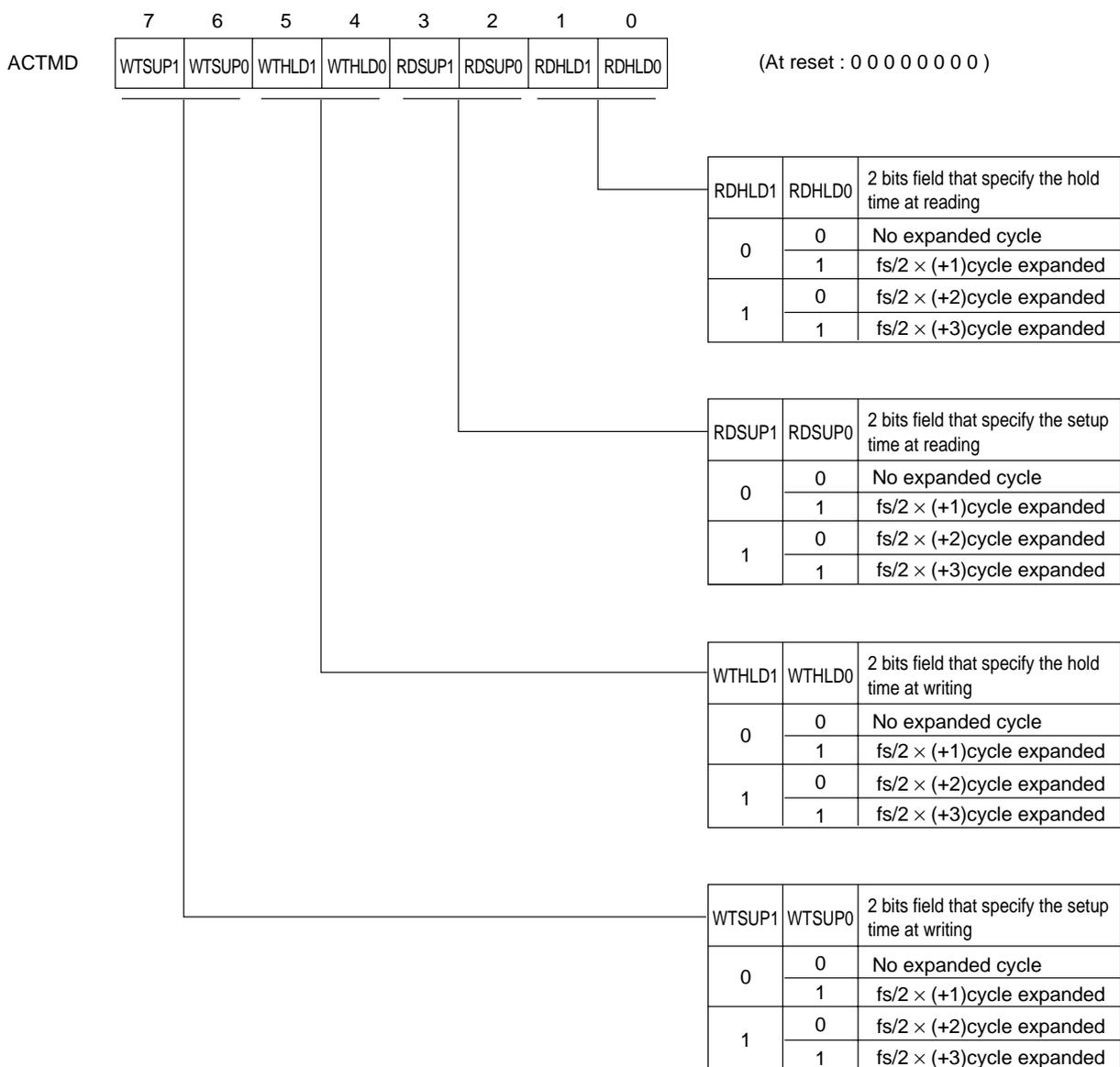
Figure 18-1-1 AC Timing Control Register (ACTMD : x'03F06', R/W)
