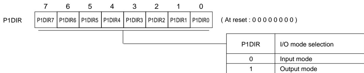
Port 1 direction control register (P1DIR : x'03F31', R/W)
