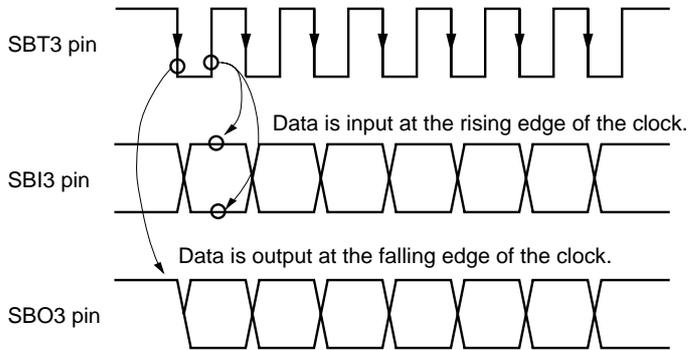
**Figure 14-3-10 Transmission/Reception Timing
