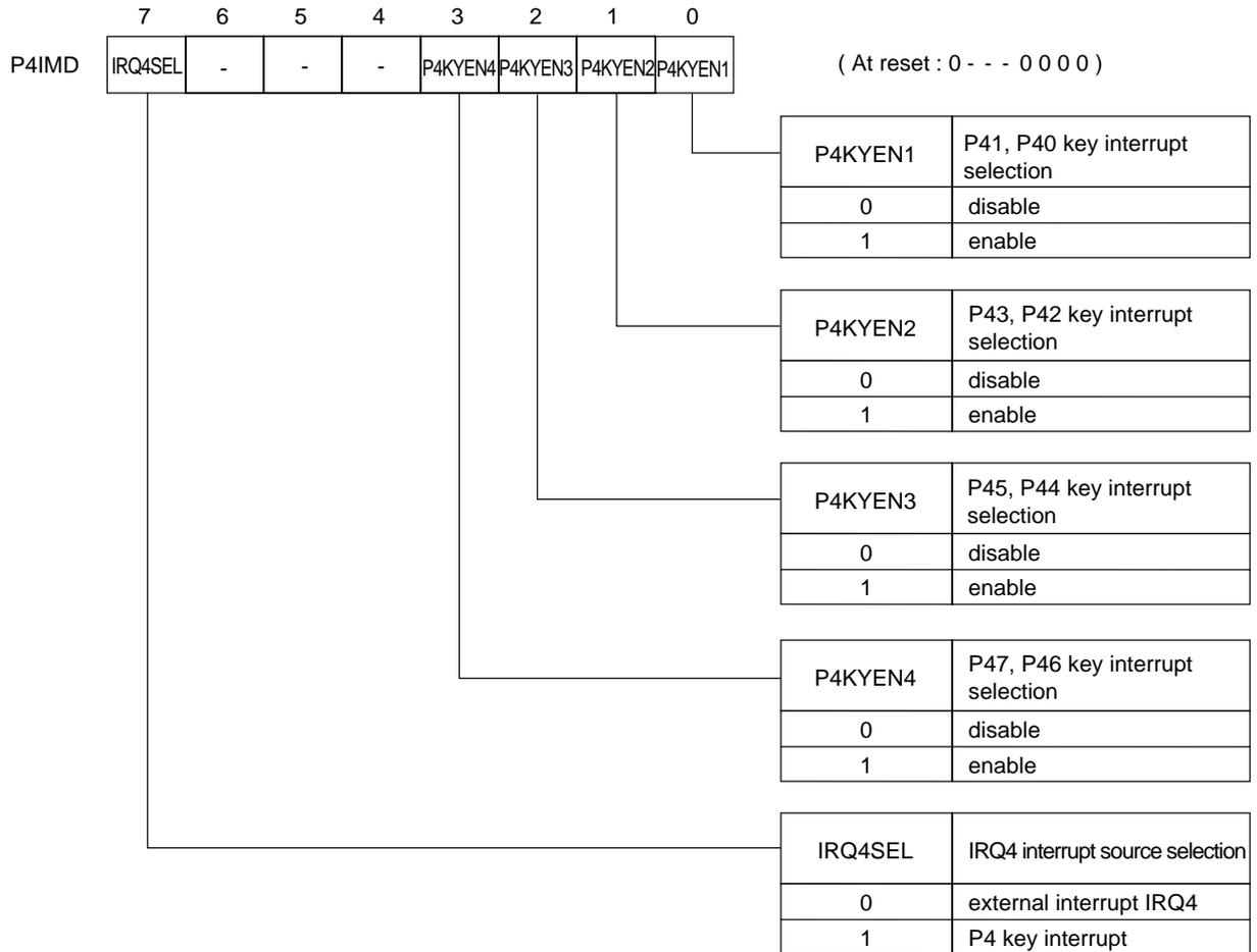
Figure 3-3-6 Port 4 Key Interrupt Control Register (P4IMD : x'03F3E', R/W)
