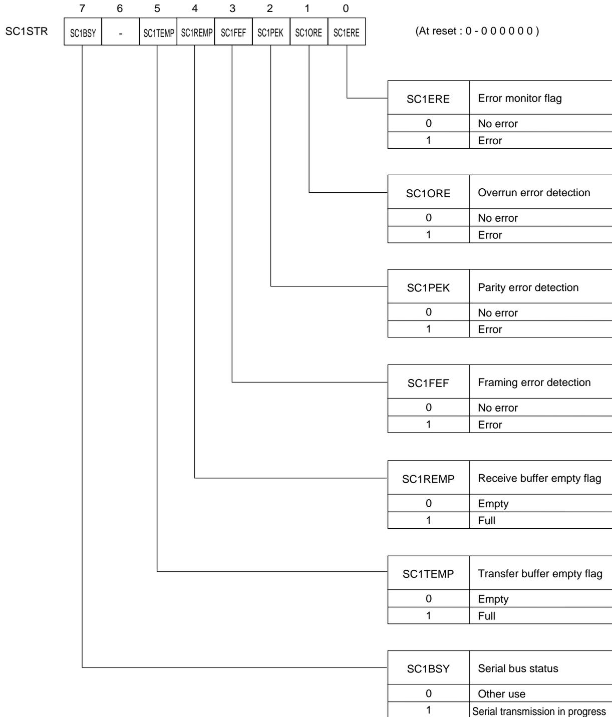
Figure 12-2-6 Serial Interface 1 State Register (SC1STR : x'03F9D', R)
