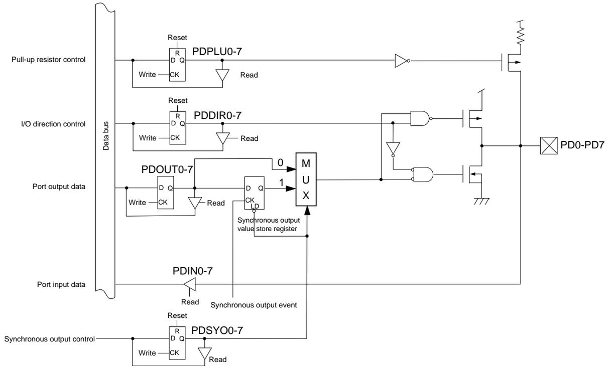
Figure 4-13-3 Block Diagram (PD0 to PD7)
