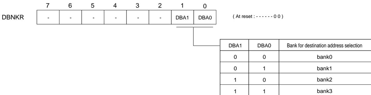
**Figure 2-6-2 Bank Register for Destination Address (DBNKR:x'03F0B', R/W)**
