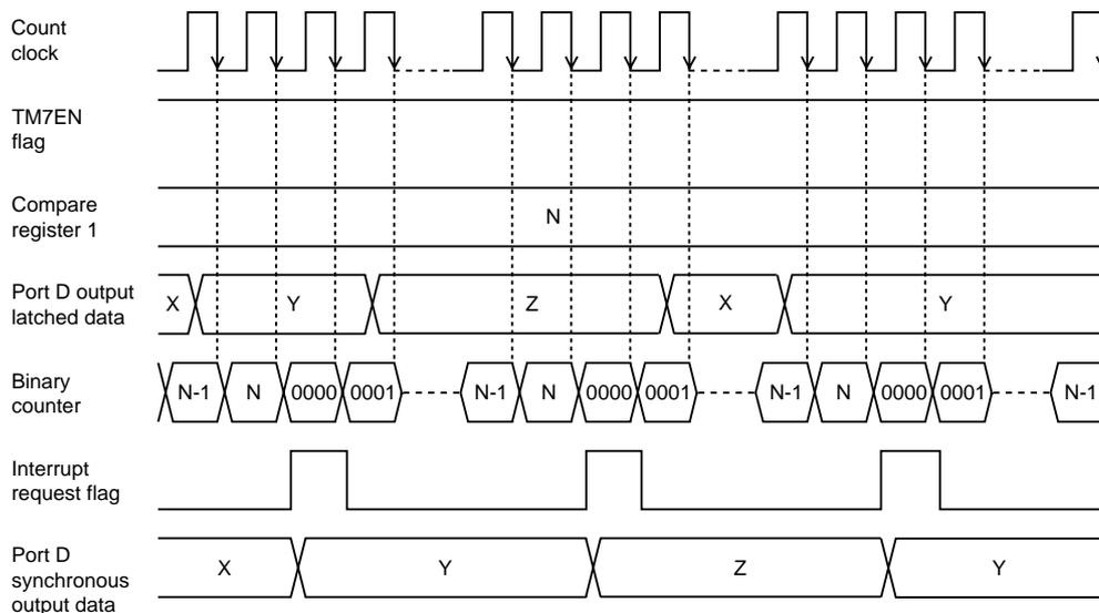
**Figure 7-8-1 Count Timing of Synchronous Output (Timer 7)**
