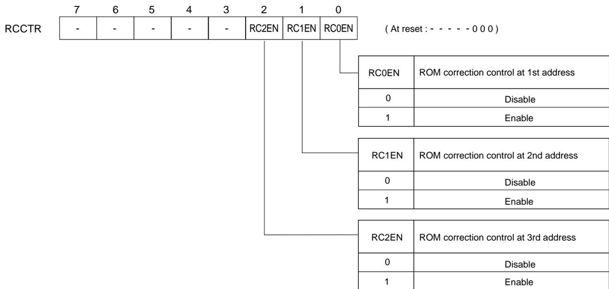
Figure 2-7-2 ROM Correction Control Register (RCCTR : x'03F09', R/W)
