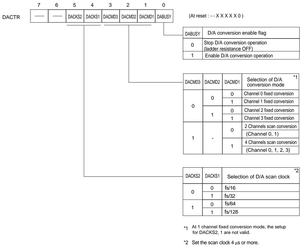
Figure 17-3-1 D/A Converter Control Register (DACTR : x'03FBB' R/W)
