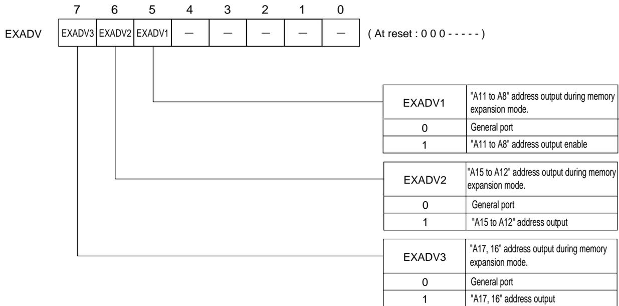
Address output control register (EXADV : x'03F0E', R/W)
