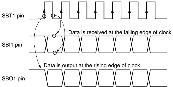
**Figure 12-3-13 Transmission / Reception Timing
