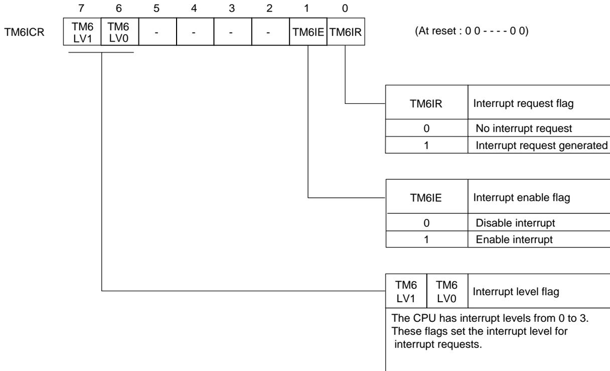
Figure 3-2-13 Timer 6 Interrupt Control Register (TM6ICR : x'03FEF', R/W)
