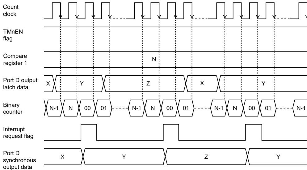
**Figure 6-7-1 Count Timing of Synchronous Output (Timer 1, Timer2)**
