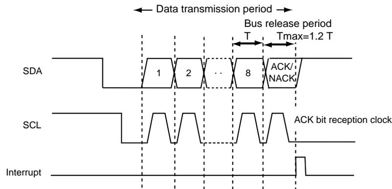
Figure 14-3-13 ACK Bit Reception Timing after Transmission of 8-bit Data
