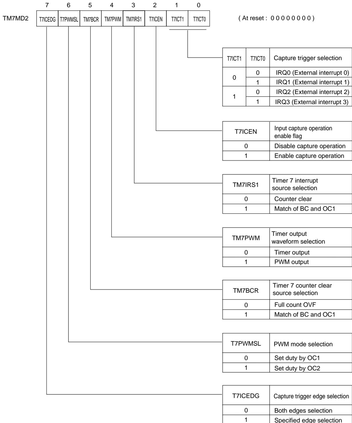
Figure 7-2-14 Timer 7 Mode Register 2 (TM7MD2 : x'03F79', R/W)
