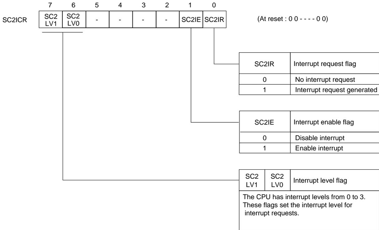
Figure 3-2-20 Serial Interface 2 Interrupt Control Register (SC2ICR : x'03FF8', R/W)
