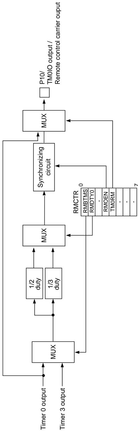
Figure 6-1-4 Remote Control Carrier Output Block Diagram
