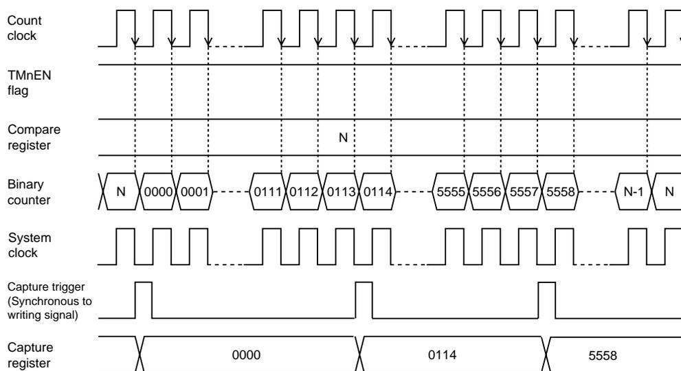
**Figure 7-9-2 Capture Count Timing
