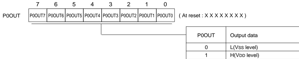
Port 0 output register (P0OUT : x'03F10', R/W)
