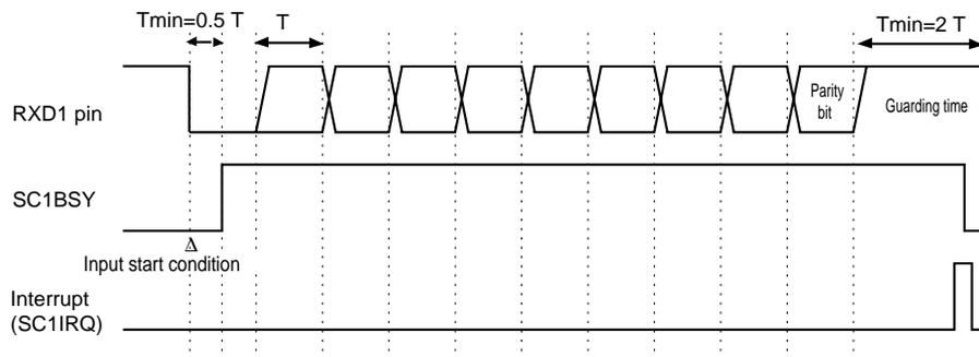
Figure 12-3-23 Reception Timing (T=0, 1 Data Communication)
