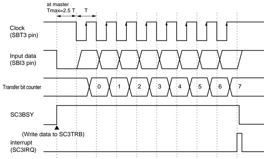
Figure 14-3-6 Reception Timing (Rising edge, Enable Start Condition)
