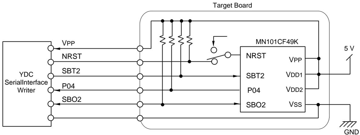
**Figure 20-6-2 Target Board for programming with the clock synchronous communication using Serial writer**
