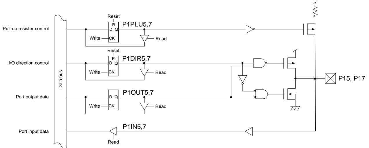
**Figure 4-3-6 Block Diagram (P15, P17)**
