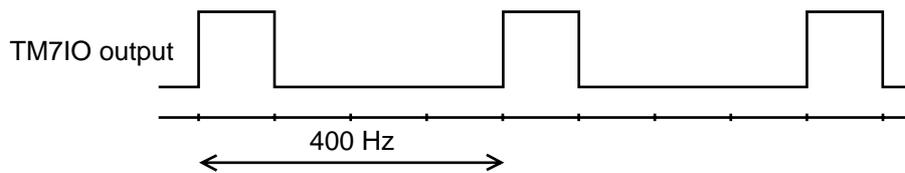
Figure 7-7-4 Output Waveform of TM7IO Output Pin
