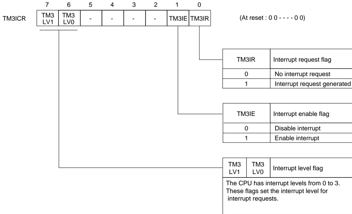
Figure 3-2-11 Timer 3 Interrupt Control Register (TM3ICR : x'03FEC', R/W)
