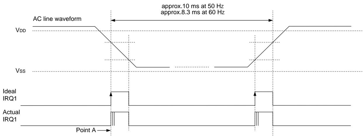
**Figure 3-3-8 AC Line Waveform and IRQ1 Generation Timing**
