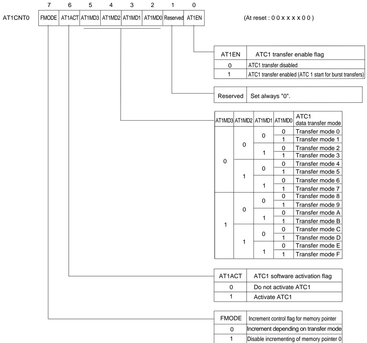
Figure 15-2-1 ATC1 Control Register 0 (AT1CNT0 : x'03FD0', R/W)
