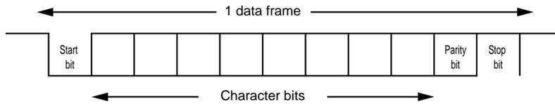
**Figure 12-3-14 UART Serial Interface Transmission / Reception Data Format**
