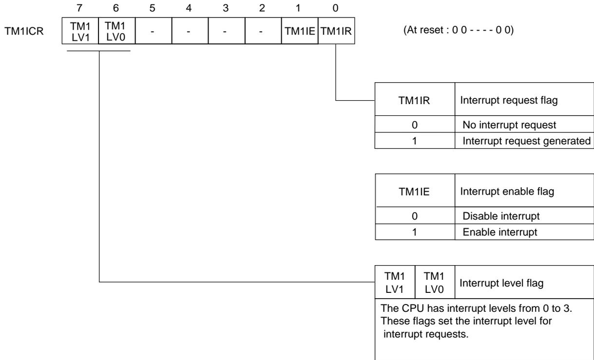
Figure 3-2-9 Timer 1 Interrupt Control Register (TM1ICR : x'03FEA', R/W)
