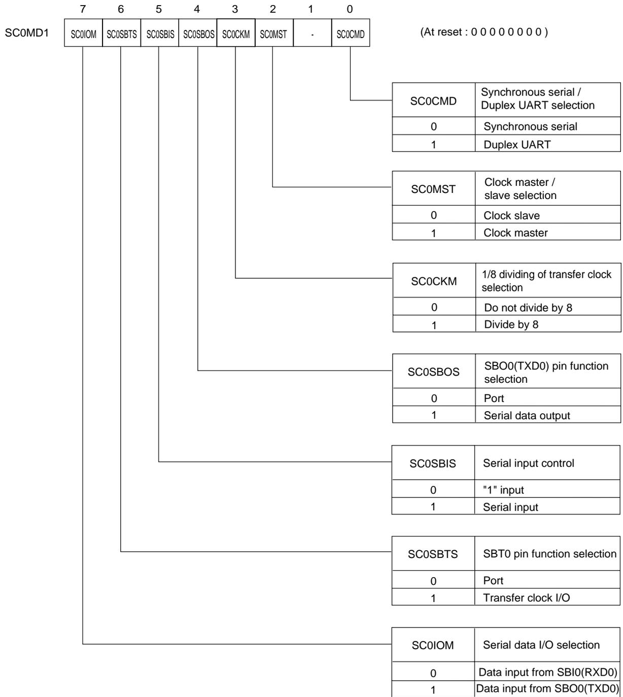
Figure 11-2-4 Serial Interface 0 Mode Register 1 (SC0MD1 : x'03F91', R/W)
