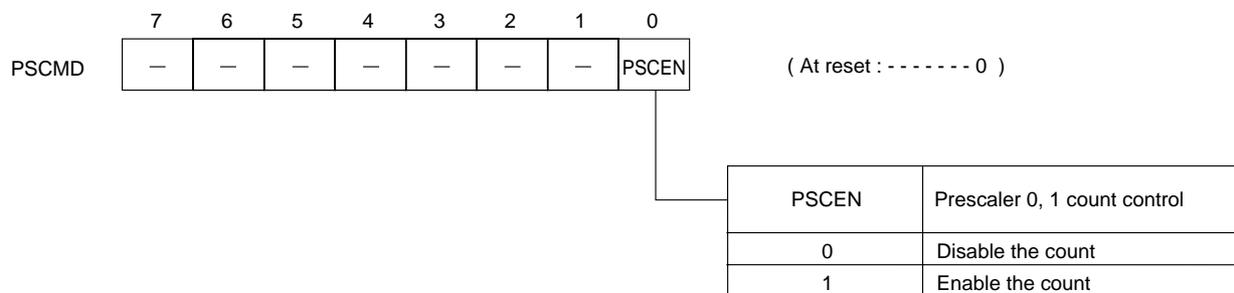
**Figure 5-2-1 Prescaler Control Register (PSCMD : x'03F6F', R/W)**
