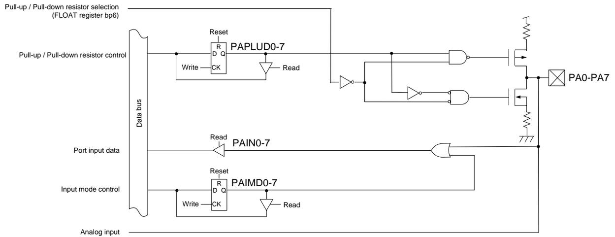
Figure 4-11-3 Block Diagram (PA0 to PA7)
