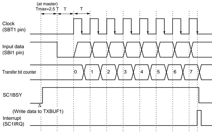
**Figure 12-3-10 Reception Timing (falling edge, start condition is enabled)**
