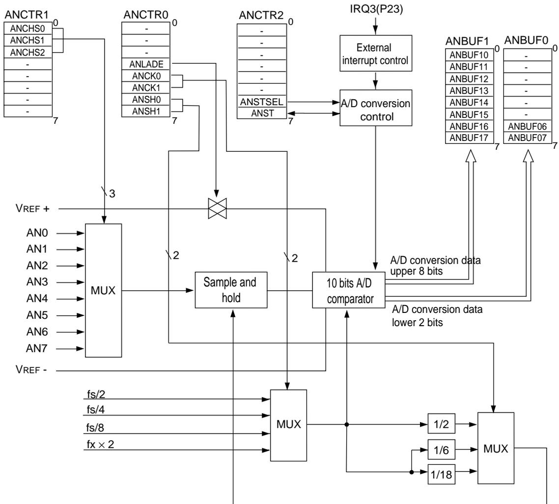
Figure 16-1-1 A/D Converter Block Diagram
