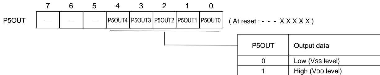
Port 5 output register (P5OUT : x'03F15', R/W)
