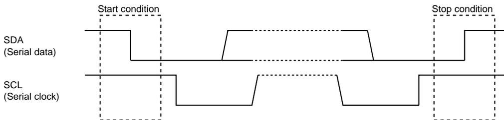
Figure 14-3-12 Start Condition and Stop Condition
