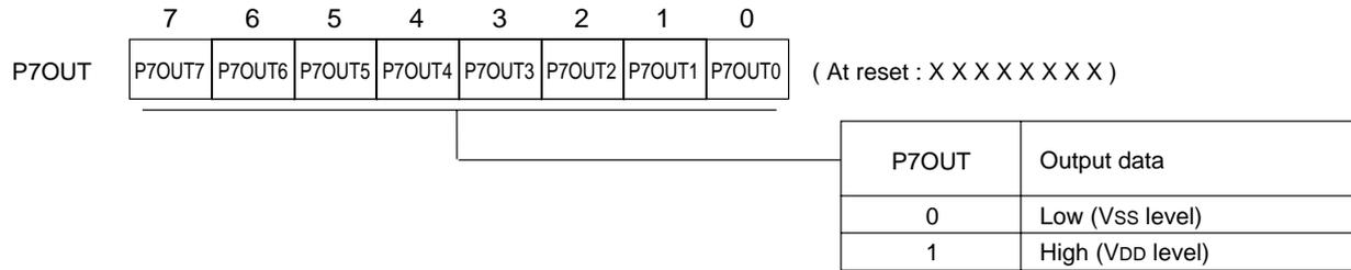
Port 7 output register (P7OUT : x'03F17', R/W)
