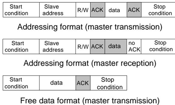
**Figure 14-3-15 Communication Sequence on Each Transfer Format**
