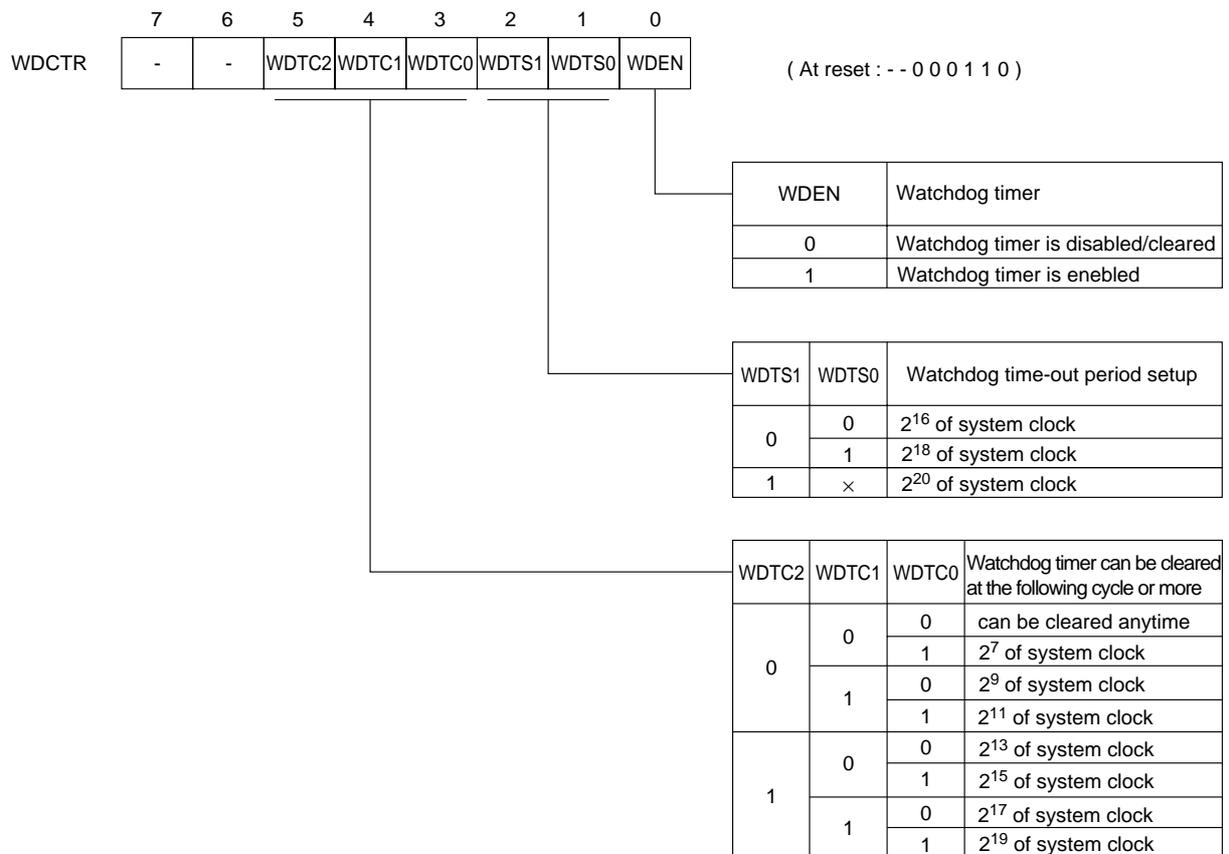
Figure 9-2-1 Watchdog Timer Control Register (WDCTR : x'03F02', R/W)
