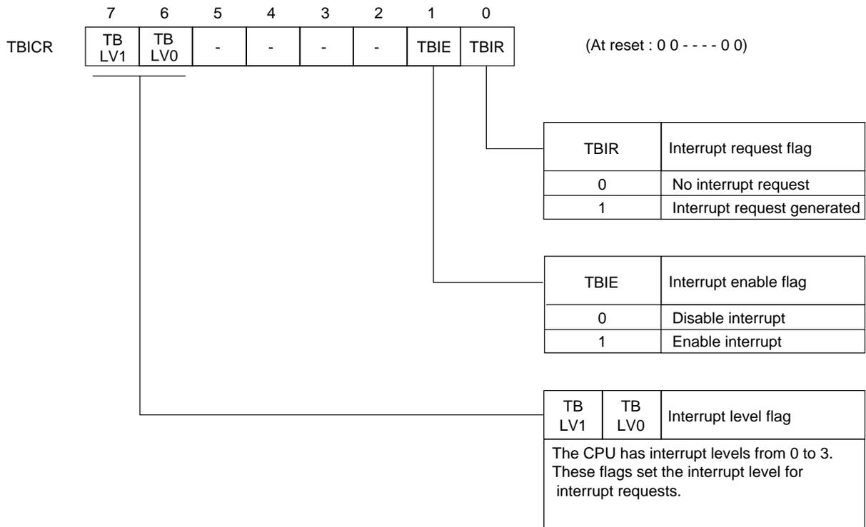
Figure 3-2-14 Time Base Interrupt Control Register (TBICR : x'03FF0', R/W)
