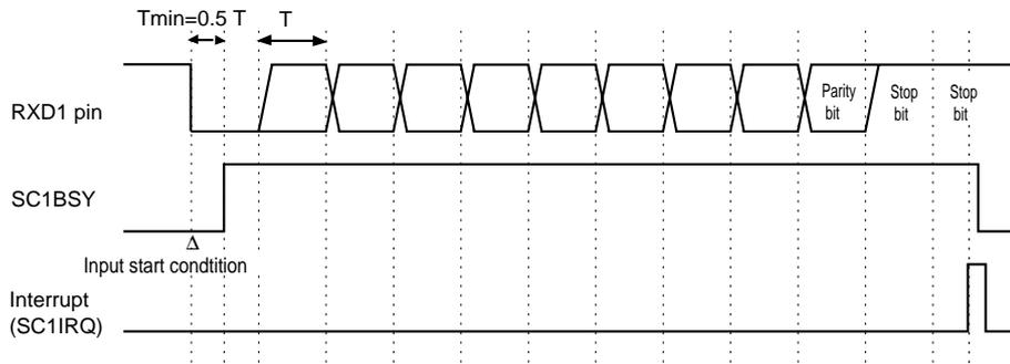
Figure 12-3-17 Reception Timing (parity bit is enabled)
