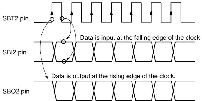
**Figure 13-3-11 Transmission / Reception Timing
