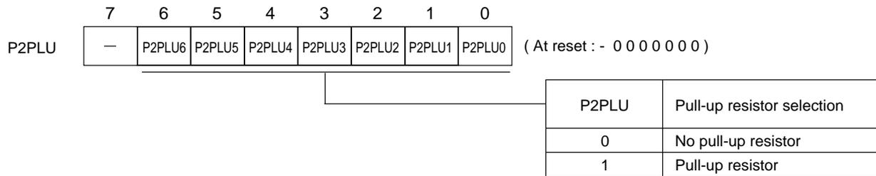
Port 2 pull-up resistor control register(P2PLU : x'03F42', R/W)
