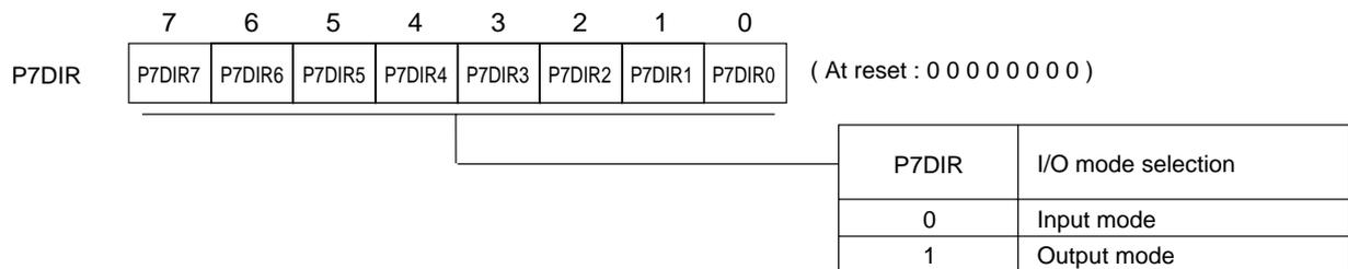
Port 7 direction control register (P7DIR : x'03F37', R/W)
