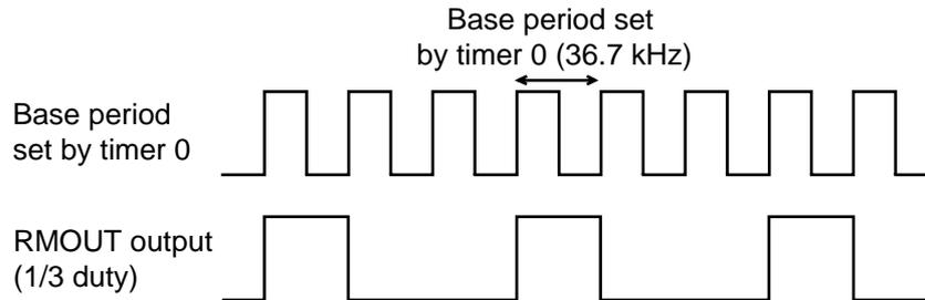
**Figure 6-11-3 Output Wave Form of RMOUT Output Pin**
