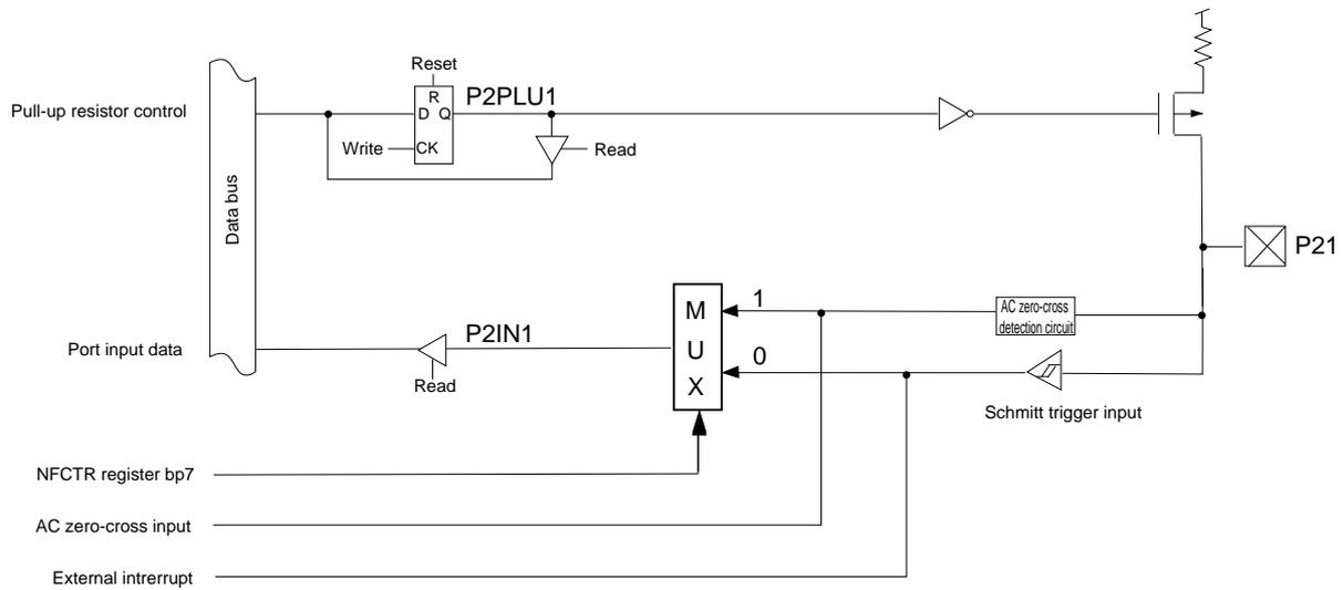
Figure 4-4-3 Block Diagram (P21)
