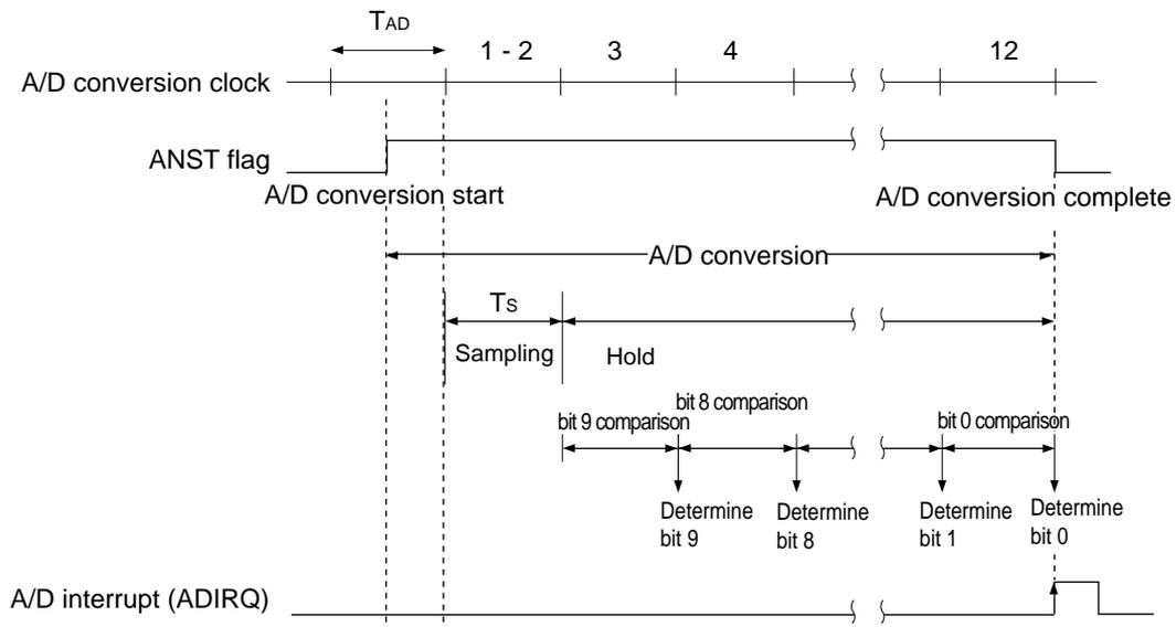
**Figure 16-3-1 Operation of A/D Conversion**
