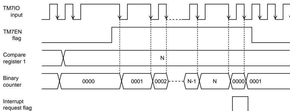
**Figure 7-4-1 Count Timing TM7IO Input (Timer 7)**
