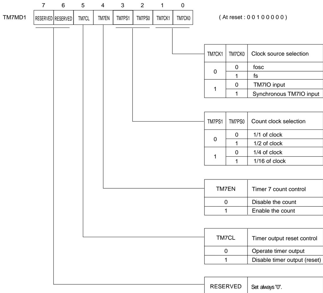
Figure 7-2-13 Timer 7 Mode Register 1 (TM7MD1 : x'03F78', R/W)
