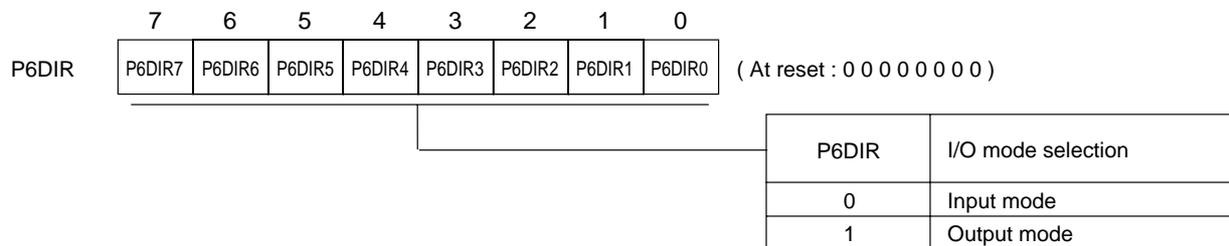
Port 6 direction control register (P6DIR : x'03F36', R/W)
