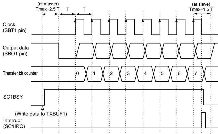
**Figure 12-3-6 Transmission Timing (rising edge, start condition is enabled)**
