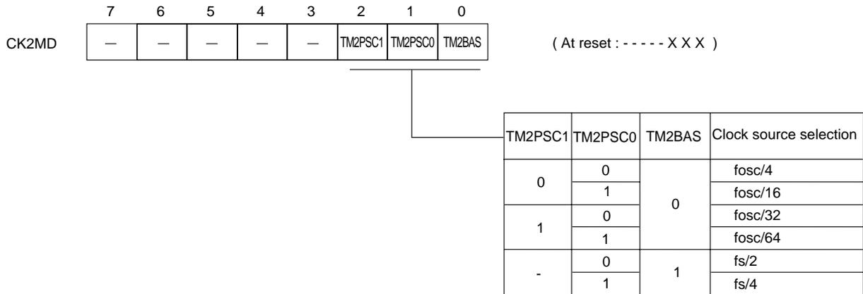
Figure 5-2-4 Timer 2 Prescaler Selection Register (CK2MD : x'03F5E', R/W)
