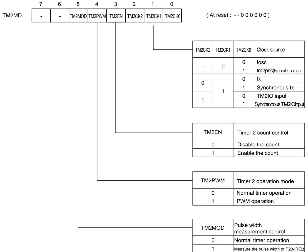
Figure 6-2-13 Timer 2 Mode Register (TM2MD : x'03F5C', R/W)
