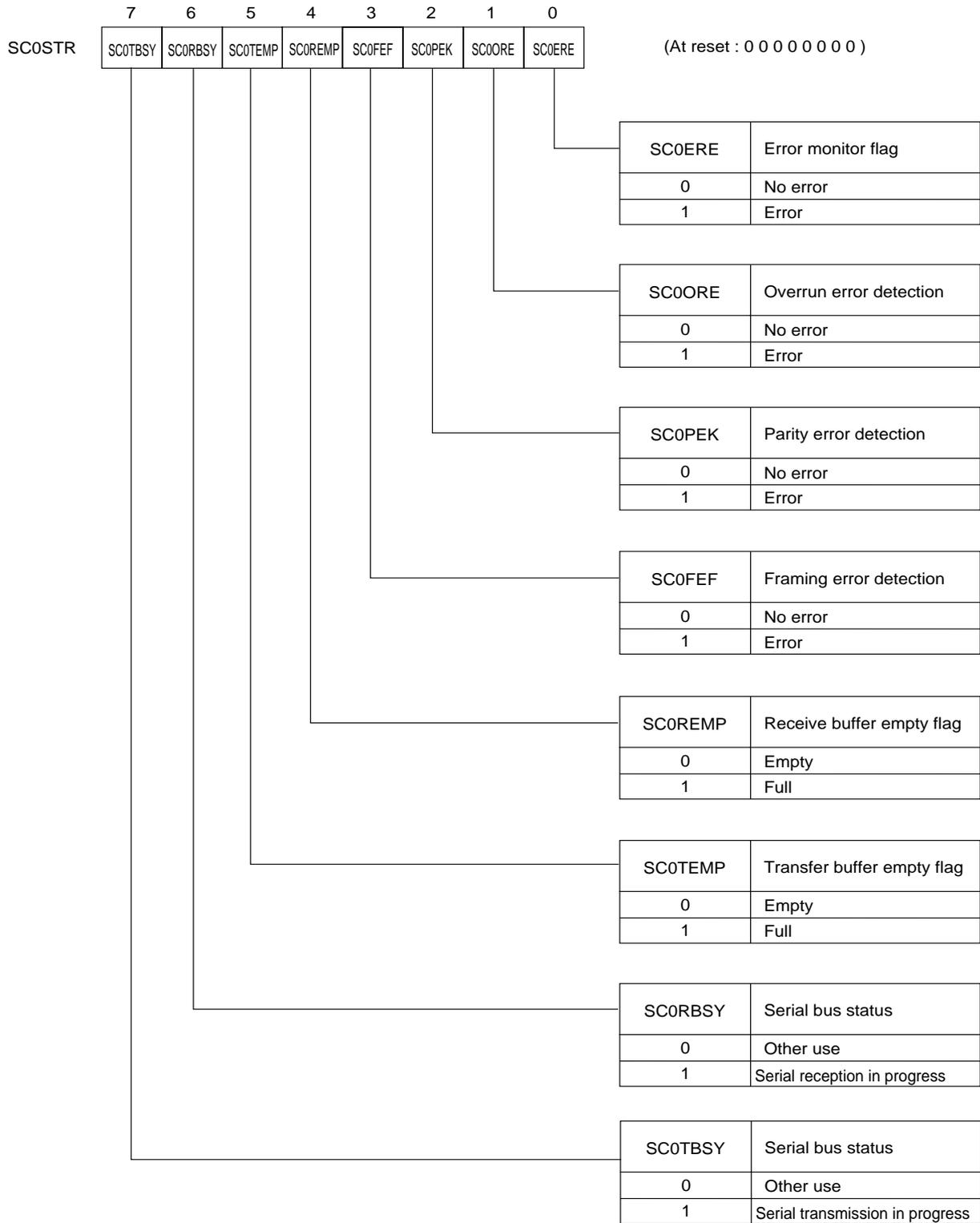
Figure 11-2-6 Serial Interface 0 State Register (SC0STR : x'03F93', R)
