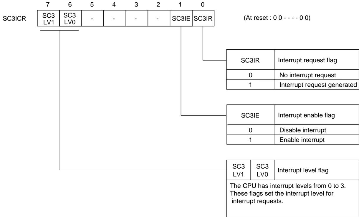
Figure 3-2-21 Serial Interface 3 Interrupt Control Register (SC3ICR : x'03FF9', R/W)
