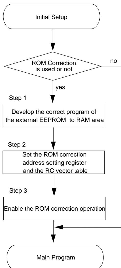
Figure 2-7-12 Initial Routine for ROM Correction
