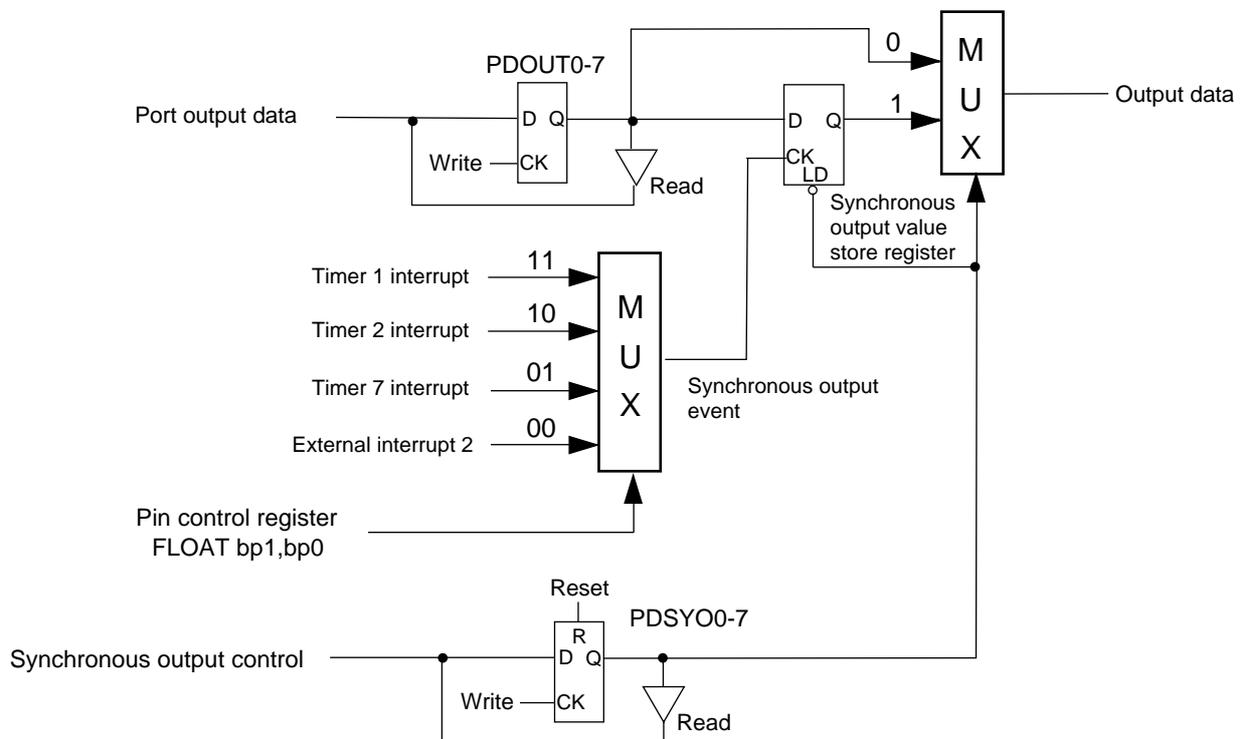
Figure 4-15-1 Synchronous Output Control Block Diagram
