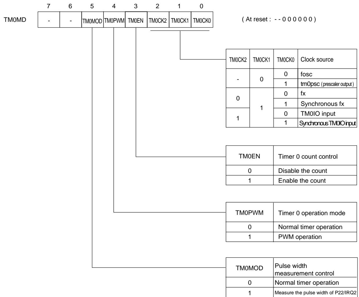
Figure 6-2-11 Timer 0 Mode Register (TM0MD : x'03F54', R/W)
