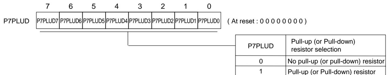
Port 7 pull-up / pull-down resistor control register (P7PLUD : x'03F47', R/W)
