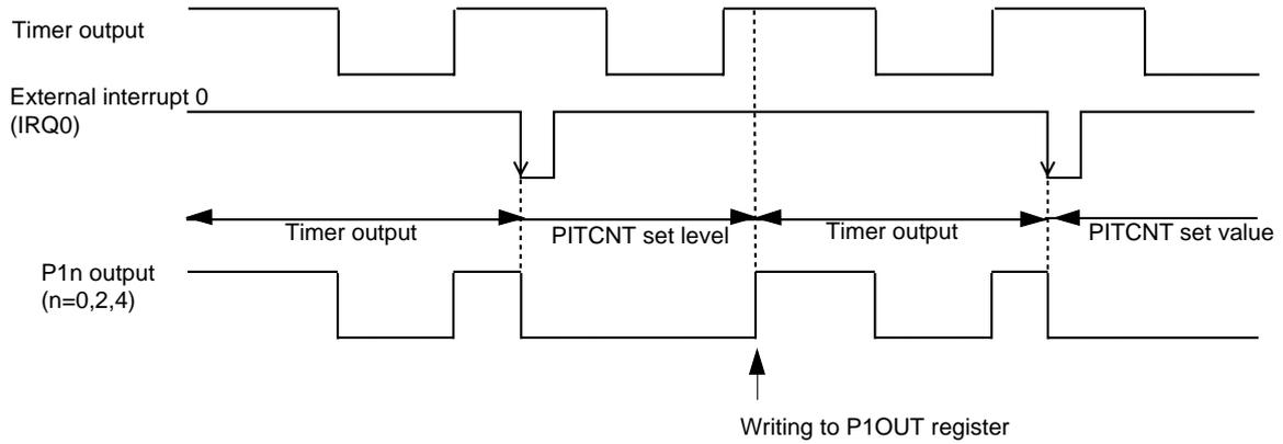
Figure 4-14-1 Real Time Output Control Timing
