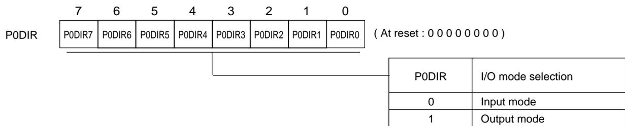
Port 0 direction control register (P0DIR : x'03F30', R/W)
