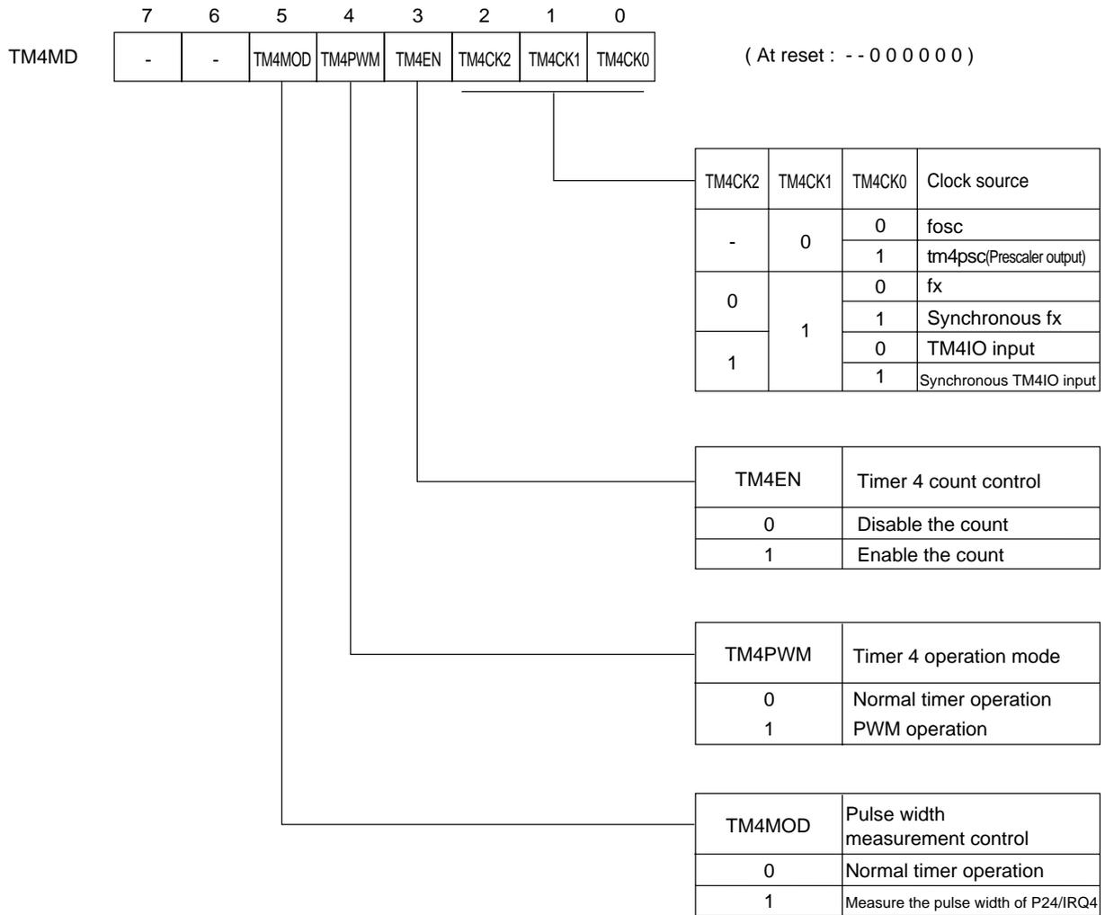
Figure 6-2-15 Timer 4 Mode Register (TM4MD : x'03F64', R/W)
