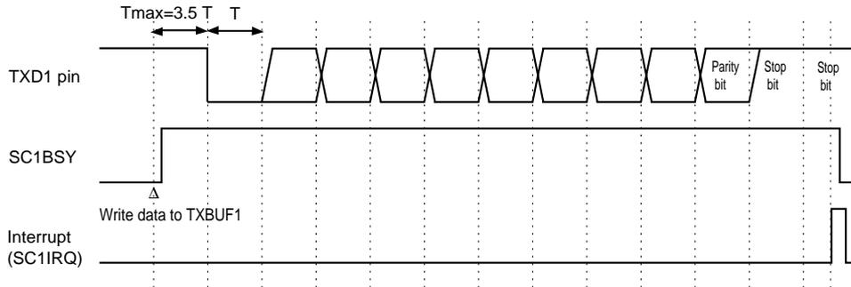
Figure 12-3-15 Transmission Timing (parity bit is enabled)
