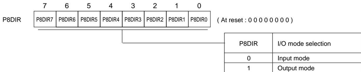
Port 8 direction control register (P8DIR : x'03F38', R/W)
