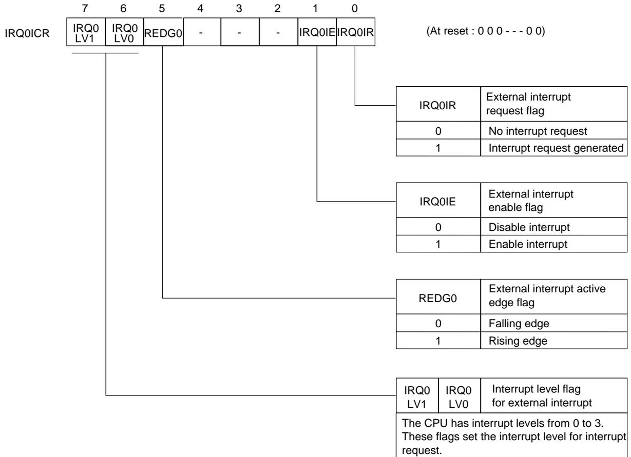
Figure 3-2-2 External Interrupt 0 Control Register (IRQ0ICR : x'03FE2', R/W)
