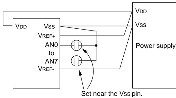
Figure 16-3-3 A/D Converter Recommended Example 2
