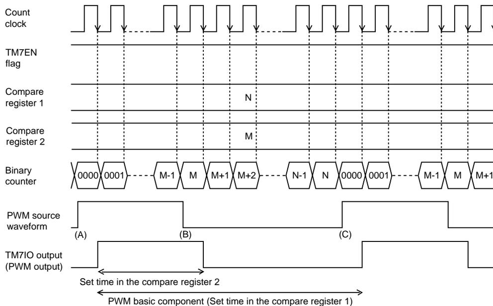
**Figure 7-7-1 Count Timing of High Precision PWM Output (at Normal)**
