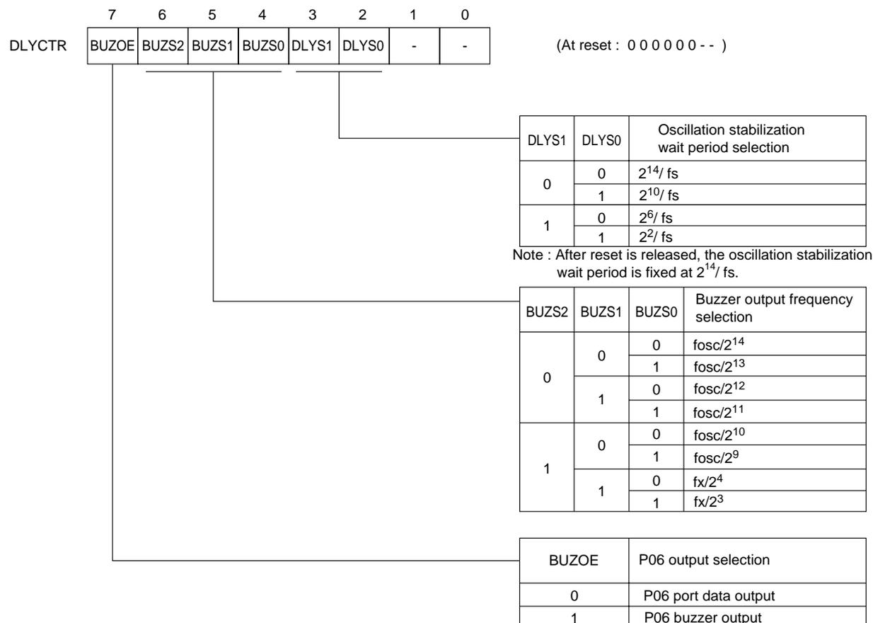
**Figure 10-2-1 Oscillation Stabilization Wait Time Control Register**
