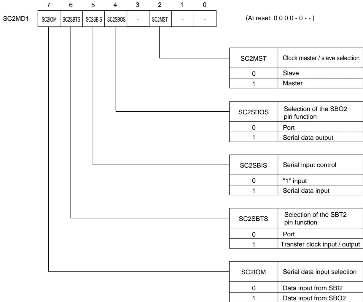
**Figure 13-2-3 Serial Interface 2 Mode Register 1 (SC2MD1 : x'03FA1', R/W)**
