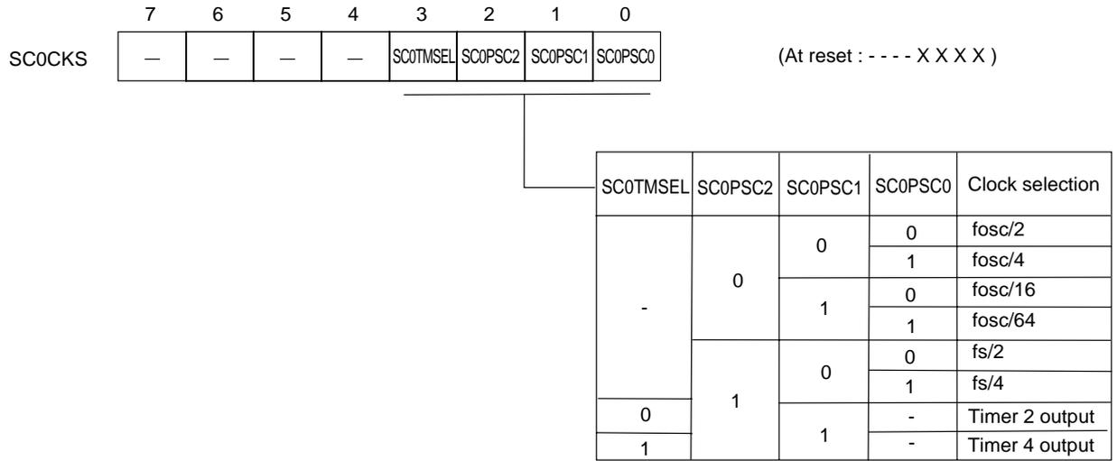
Figure 11-2-8 Serial Interface 0 Transfer Clock Selection Register (SC0CKS : x'03F97', R/W)
