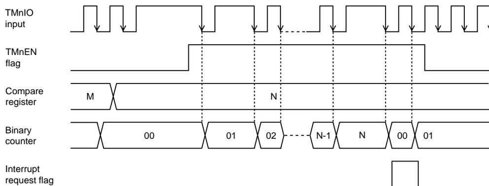
**Figure 6-4-1 Count Timing of TMnIO Input (Timers 0 to 4)**
