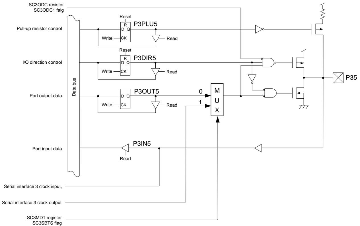
Figure 4-5-7 Block Diagram (P35)
