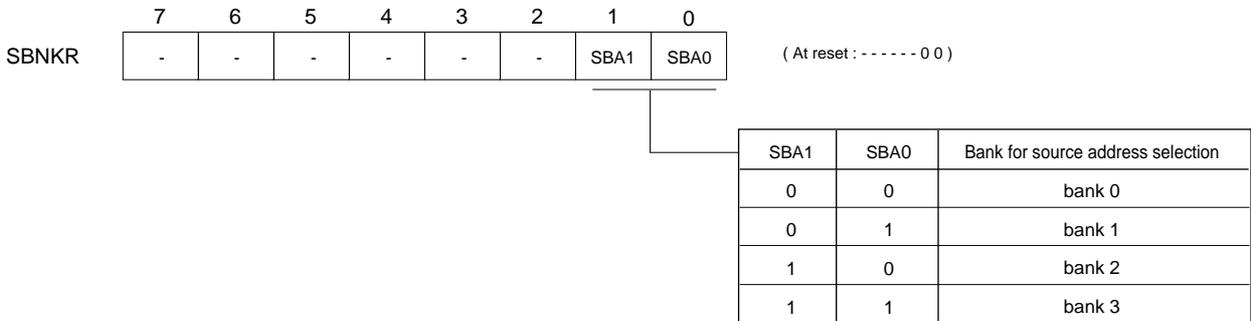
**Figure 2-6-1 Bank Register for Source Address (SBNKR:x'03F0A', R/W)**
