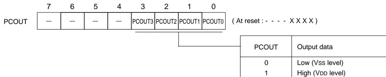
Port C output register (PCOUT : x'03F1C', R/W)
