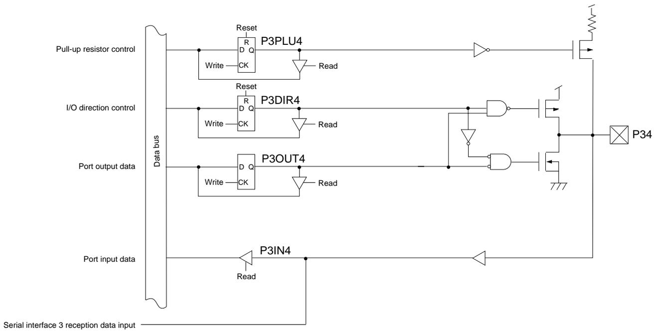
Figure 4-5-6 Block Diagram (P34)
