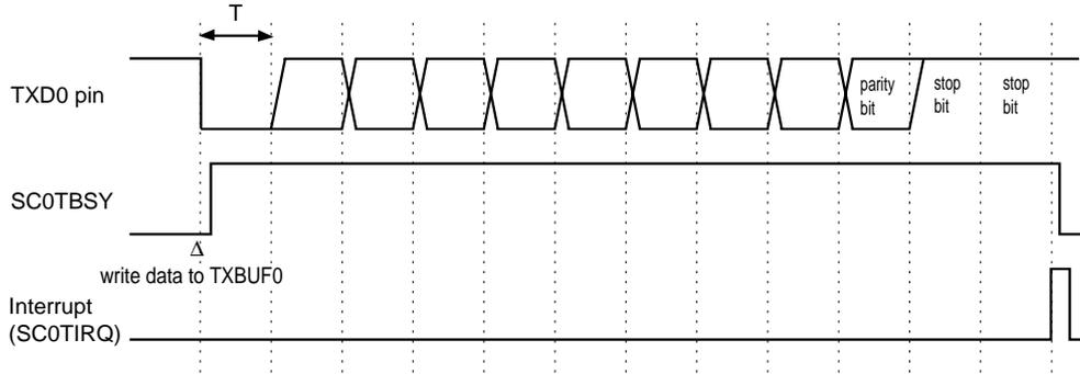
Figure 11-3-20 Transmission Timing (parity bit is enabled)
