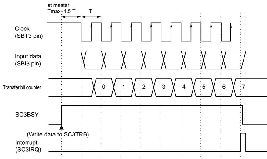
Figure 14-3-7 Reception Timing (Rising edge, Disable Start Condition)
