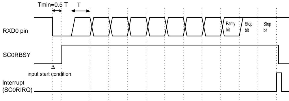
Figure 11-3-22 Reception Timing (parity bit is enabled)
