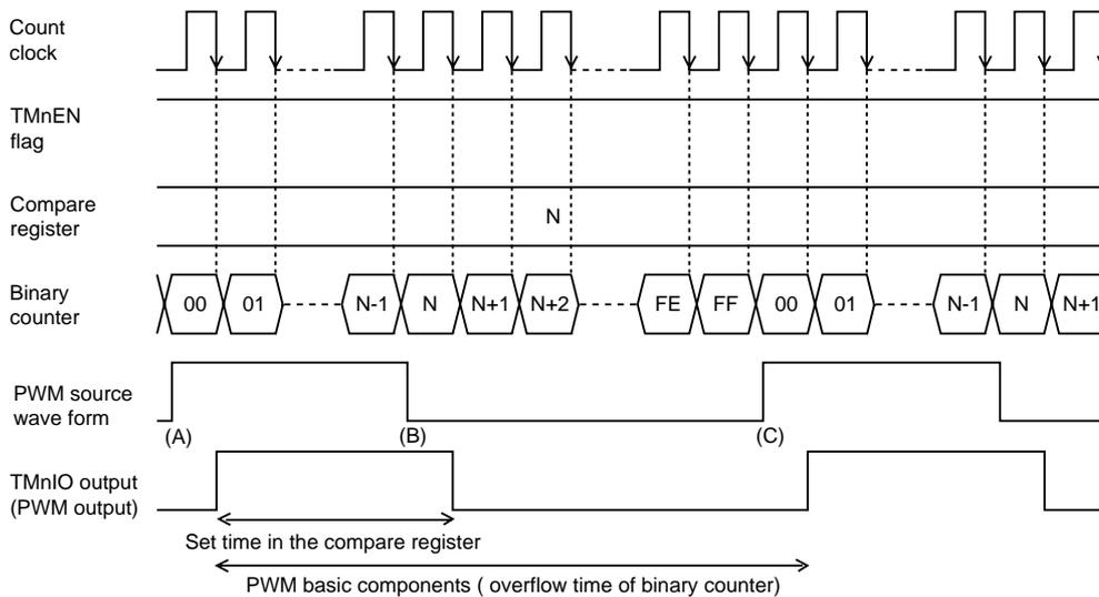
**Figure 6-6-1 Count Timing of PWM Output (at Normal)**
