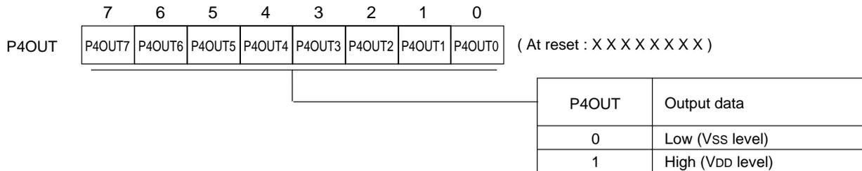
Port 4 output register (P4OUT : x'03F14', R/W)
