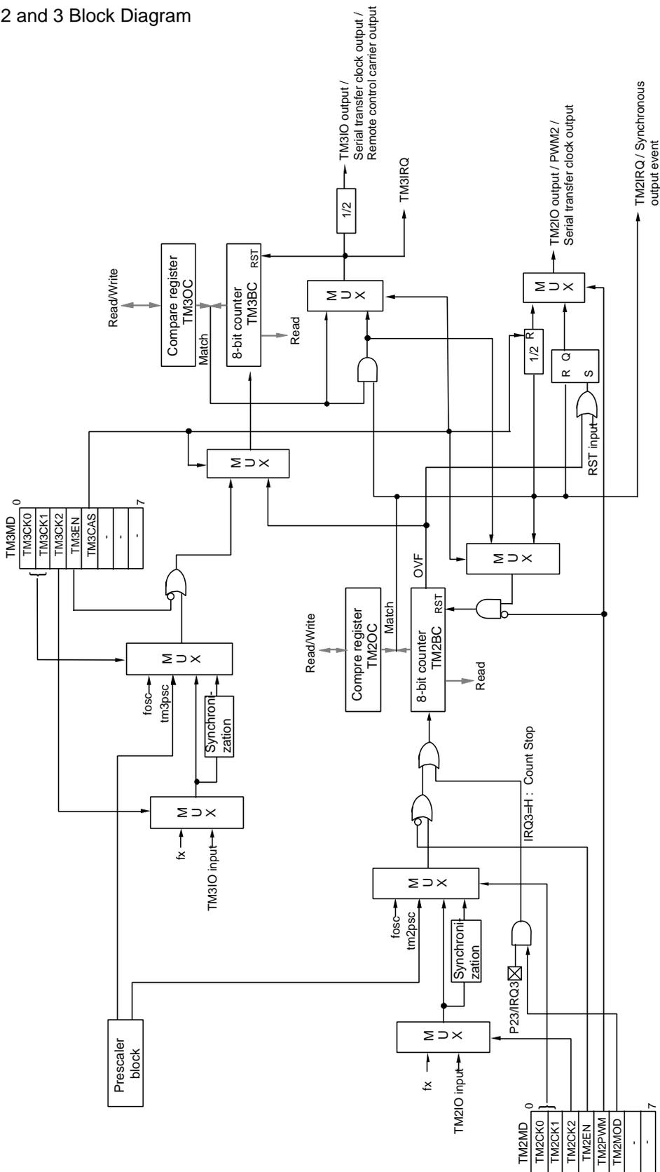
Figure 6-1-2 Timers 2 and 3 Block Diagram
