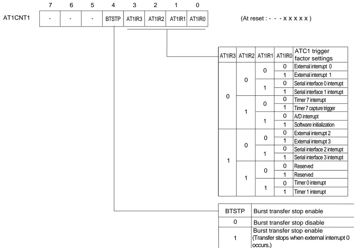
Figure 15-2-2 ATC1 Control Register 1 (AT1CNT1 : x'03FD1', R/W)
