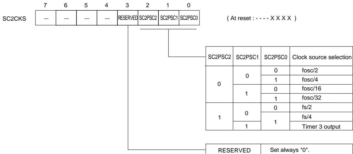
Figure 5-2-9 Serial Interface 2 Transfer Clock Selection Register (SC2CKS : x'03FA7', R/W)
