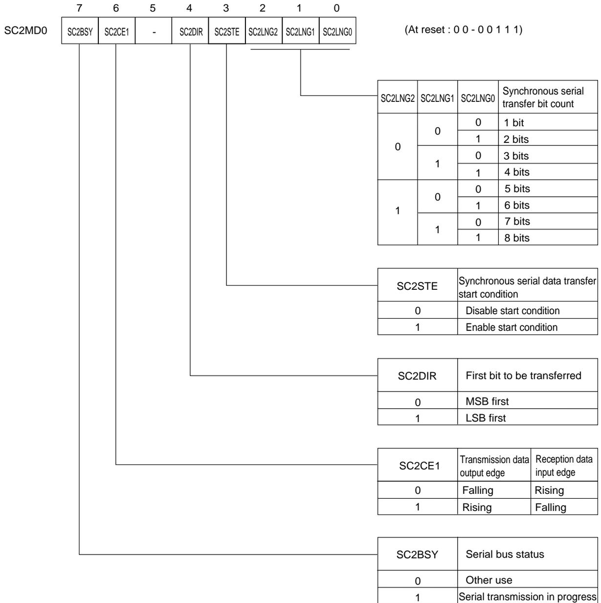
Figure 13-2-2 Serial Interface 2 Mode Register 0 (SC2MD0 : x'03FA0', R/W)
