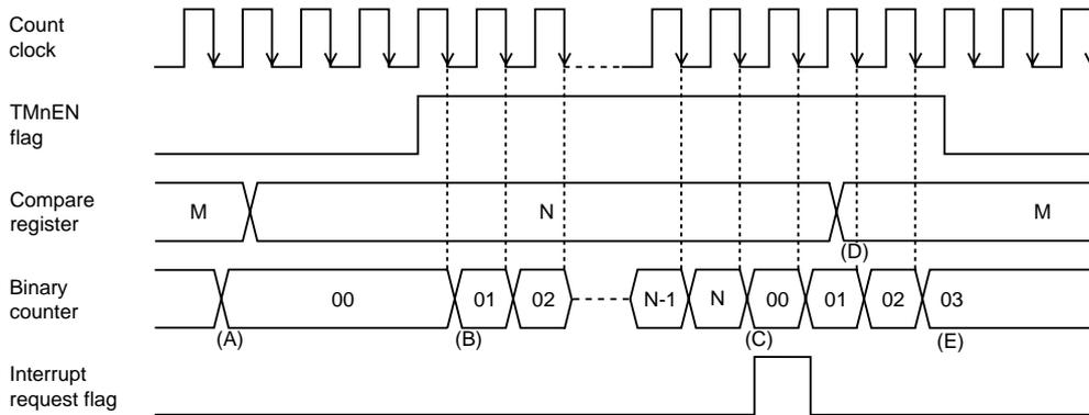
**Figure 6-3-1 Count Timing of Timer Operation (Timers 0, 1, 2, 3 and 4)**
