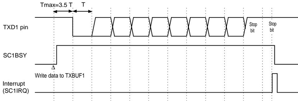
Figure 12-3-16 Transmission Timing (parity bit is disabled)
