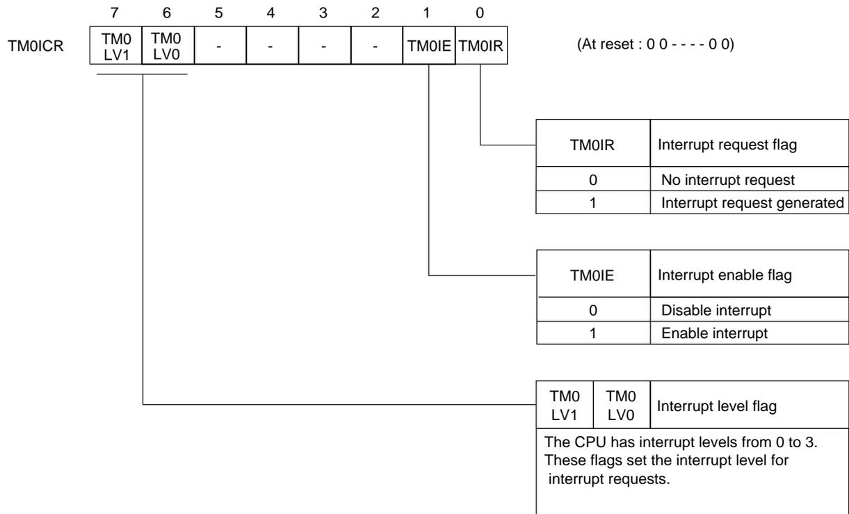
Figure 3-2-8 Timer 0 Interrupt Control Register (TM0ICR : x'03FE9', R/W)
