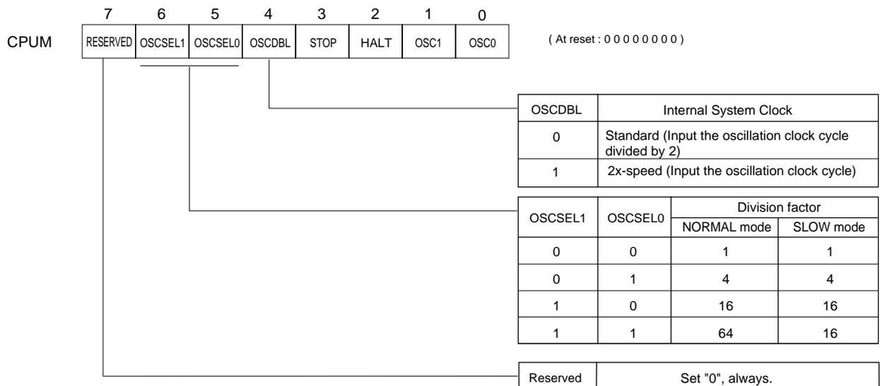
Figure 2-5-2 CPU Mode Control Register (CPUM : x'03F00', R/W)
