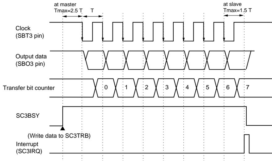
Figure 14-3-2 Transmission Timing (Falling edge, Enable Start Condition)
