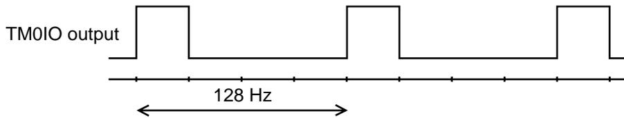
Figure 6-6-4 Output Waveform of TM0IO Output Pin
