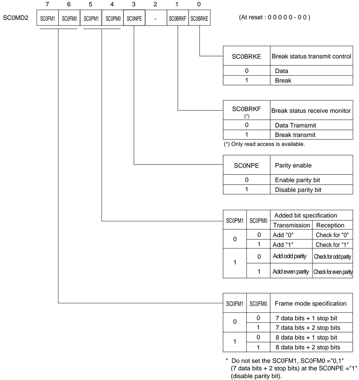
Figure 11-2-5 Serial Interface 0 Mode Register 2 (SC0MD2 : x'03F92', R/W)
