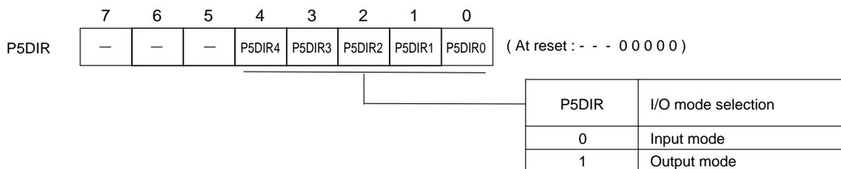
Port 5 direction control register (P5DIR : x'03F35', R/W)
