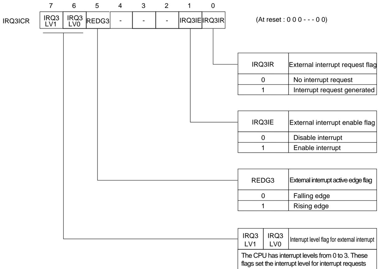
Figure 3-2-5 External Interrupt 3 Control Register (IRQ3ICR : x'03FE5', R/W)
