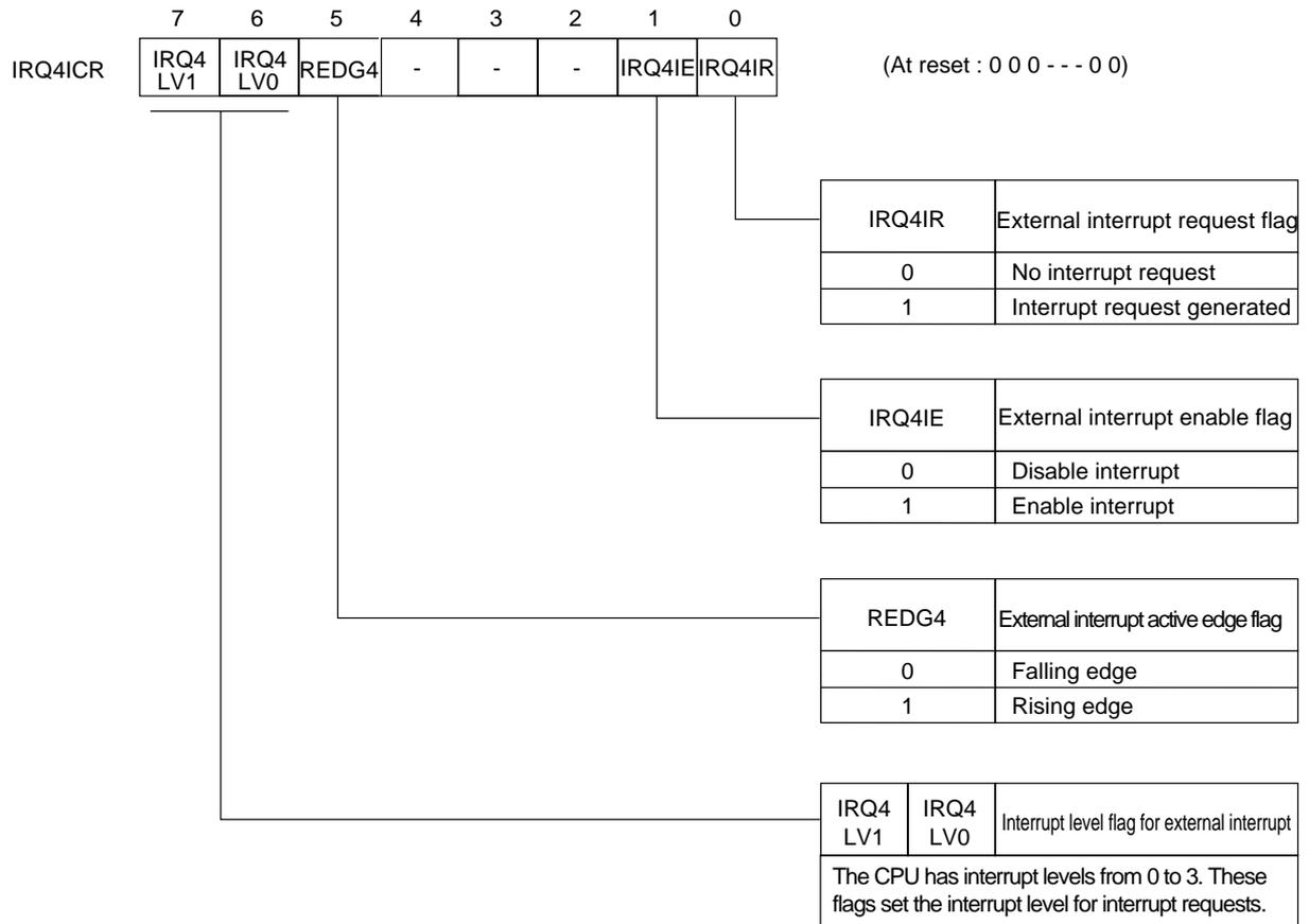
Figure 3-2-6 External Interrupt 4 Control Register (IRQ4ICR : x'03FE6', R/W)
