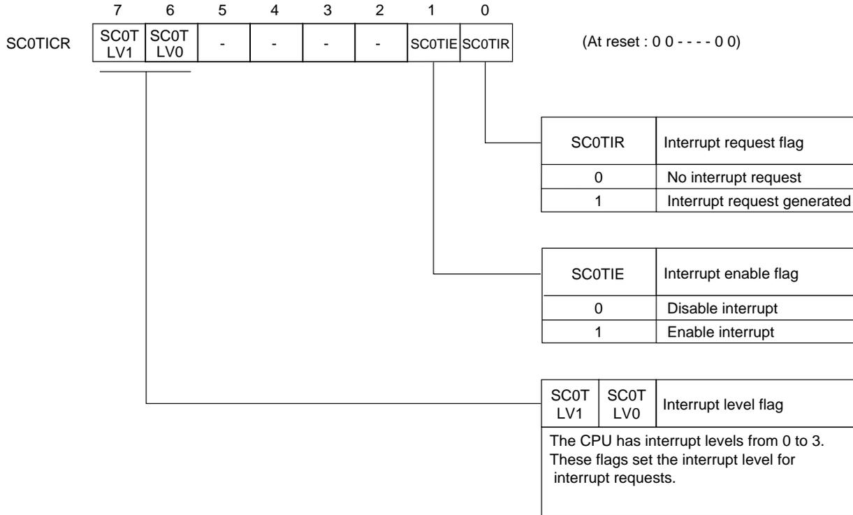
Figure 3-2-18 Serial Interface 0 Interrupt Control Register (SC0TICR : x'03FF6', R/W)
