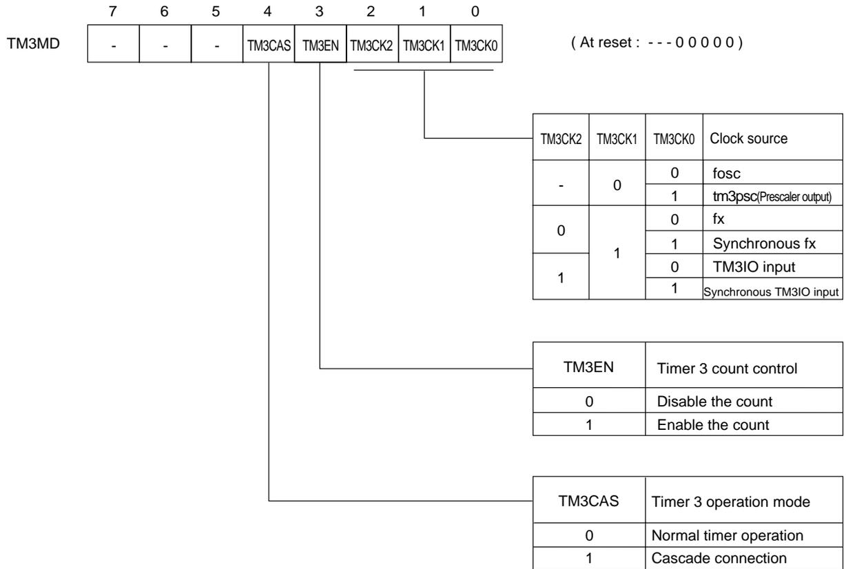
Figure 6-2-14 Timer 3 Mode Register (TM3MD : x'03F5D', R/W)
