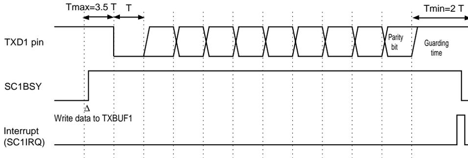
Figure 12-3-22 Transmission Timing (ATR Data, T=0, 1 Data Communication)
