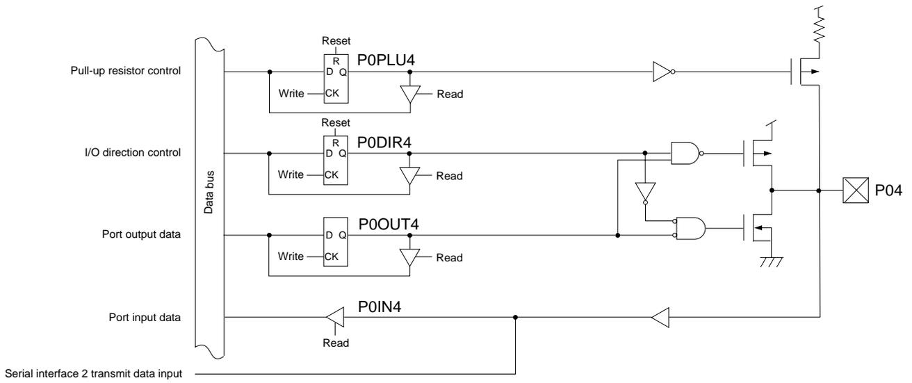
Figure 4-2-6 Block Diagram (P04)
