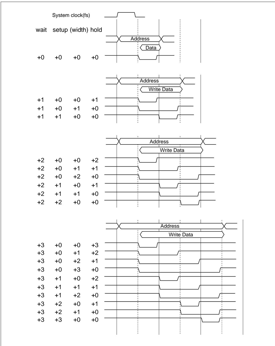
Figure 18-2-1 AC Timing Features of Data Strobe Signal
