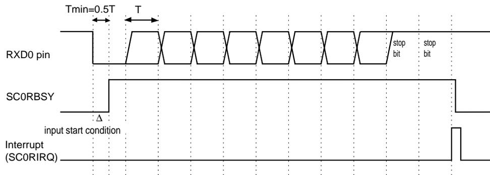
Figure 11-3-23 Reception Timing (parity bit is disabled)
