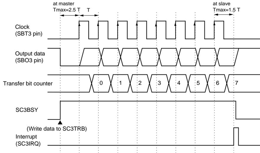
**Figure 14-3-4 Transmission Timing (Rising edge, Enable Start Condition)**
