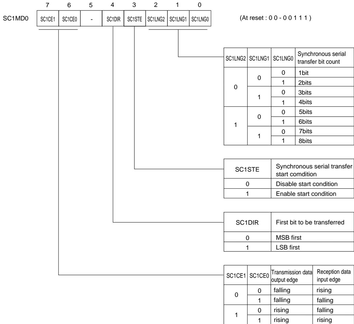
Figure 12-2-3 Serial Interface 1 Mode Register 0 (SC1MD0 : x'03F9A', R/W)
