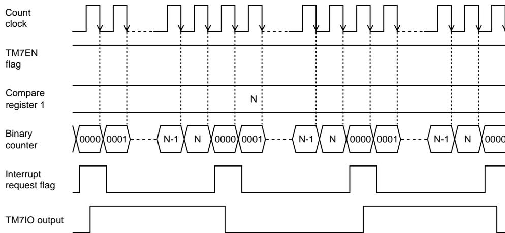
**Figure 7-5-1 Count Timing of Timer Pulse Output (Timer 7)**
