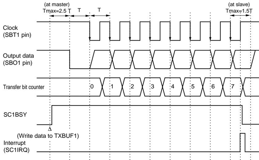
Figure 12-3-4 Transmission Timing (falling edge, start condition is enabled)
