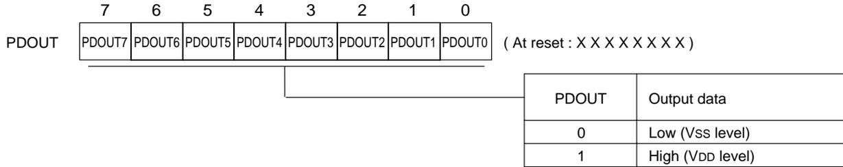
Port D output register (PDOUT : x'03F1D', R/W)
