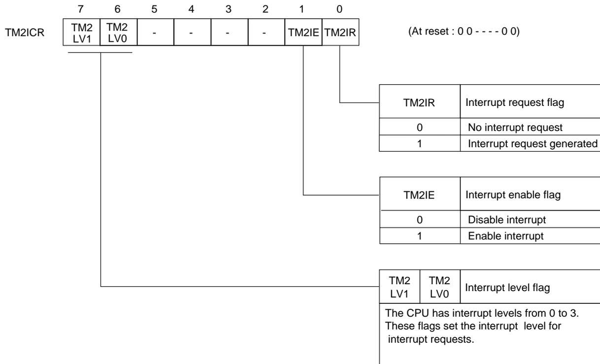
Figure 3-2-10 Timer 2 Interrupt Control Register (TM2ICR : x'03FEB', R/W)
