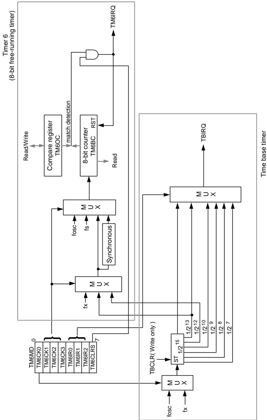
Figure 8-1-1 Block Diagram (Timer 6, Time Base Timer)
