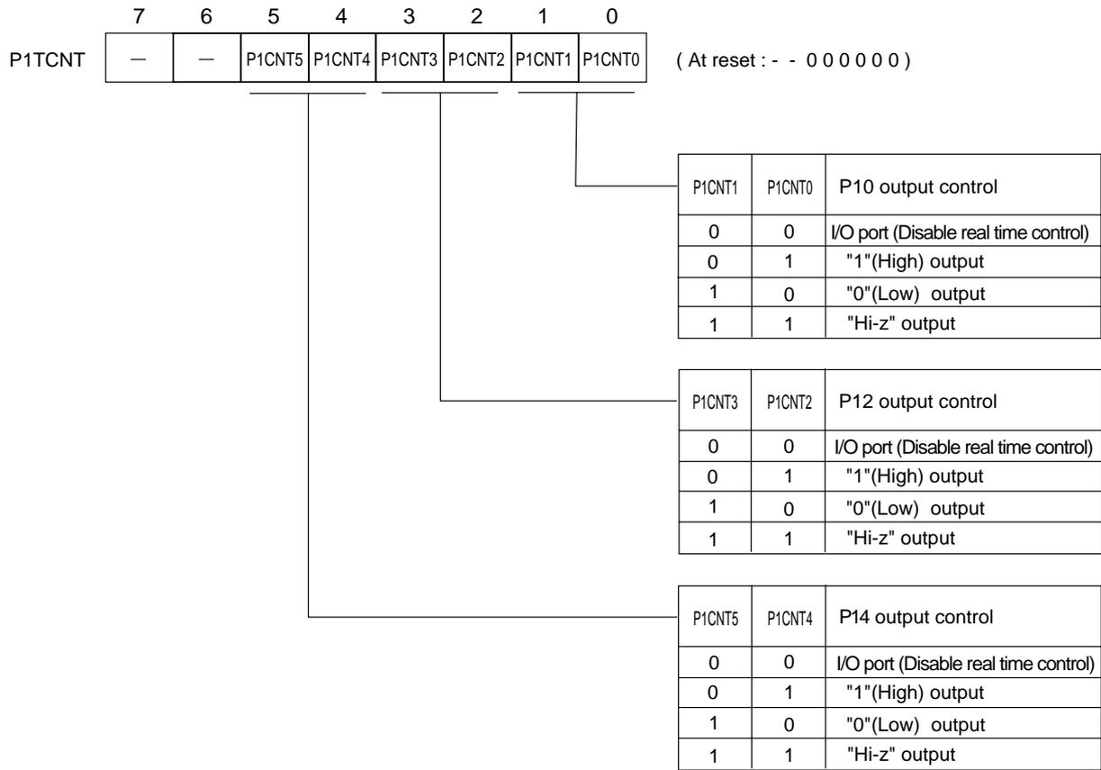
Port 1 output control register (P1TCNT : x'03F7E', R/W)
