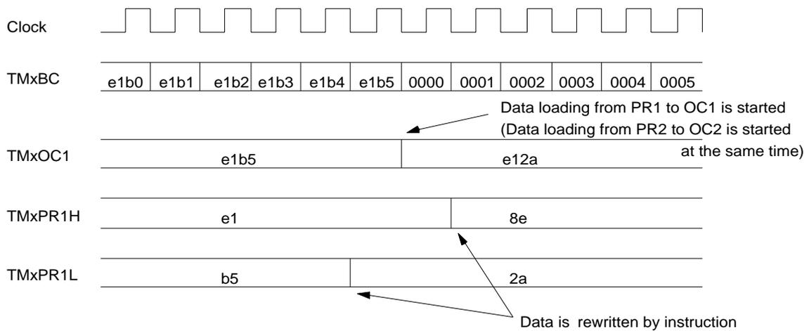
Data e12a is loaded to OC1 as PR1rewriting (e1b5 -> 8e2a) and loading to OC1 are operated at the same time.
