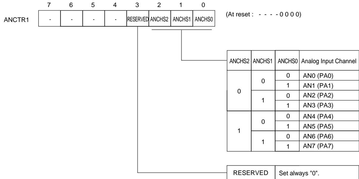
Figure 16-2-2 A/D Converter Control Register 1 (ANCTR1 : x'03FB1', R/W)
