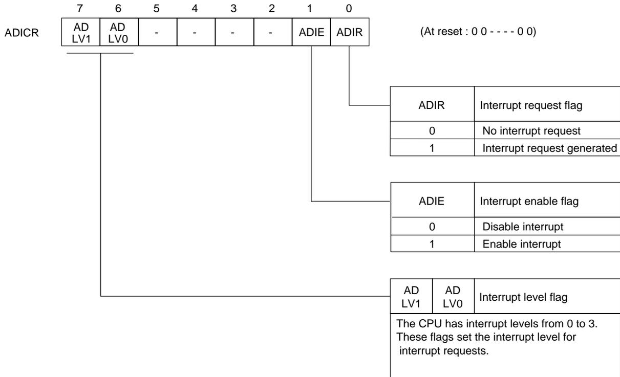
Figure 3-2-22 A/D Converter Interrupt Control Register (ADICR : x'03FFA', R/W)
