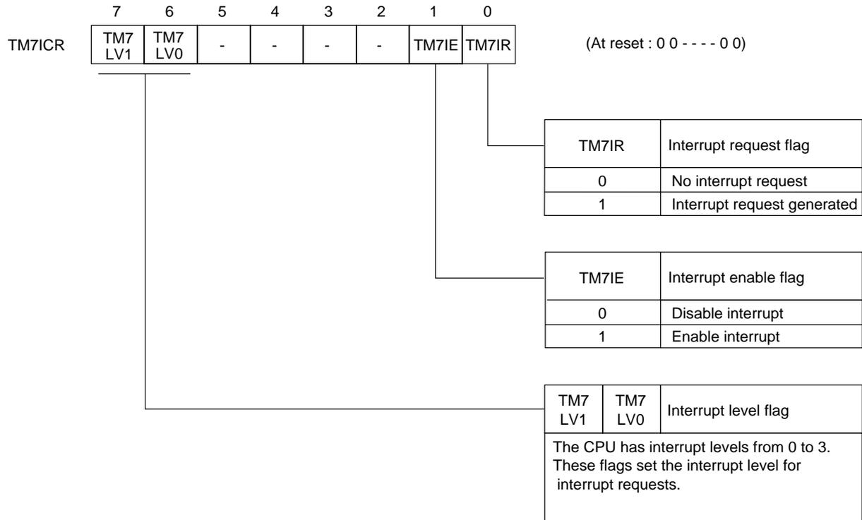
Figure 3-2-15 Timer 7 Interrupt Control Register (TM7ICR : x'03FF1', R/W)
