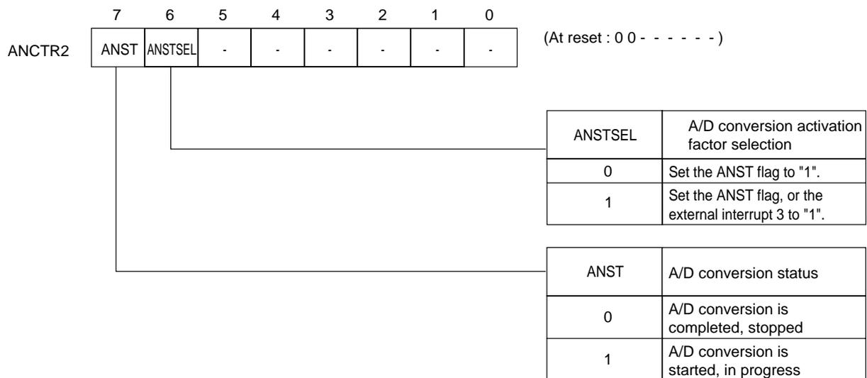
Figure 16-2-3 A/D Converter Control Register 2 (ANCTR2 : x'03FB2', R/W)
