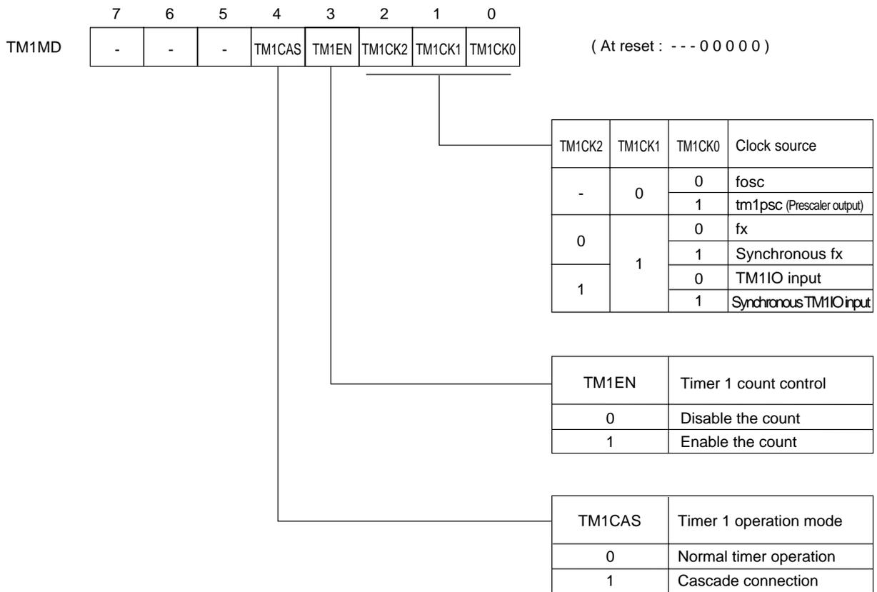
Figure 6-2-12 Timer 1 Mode Register (TM1MD : x'03F55', R/W)
