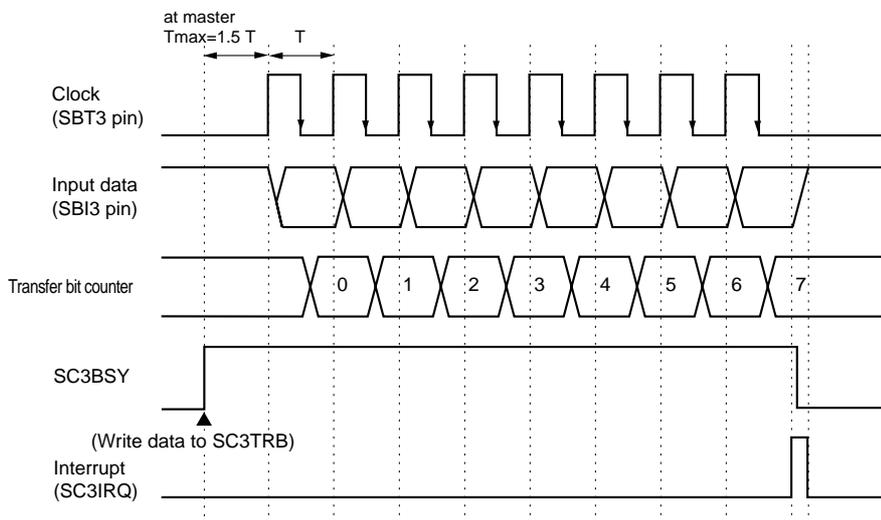
**Figure 14-3-9 Reception Timing (Falling edge, Disable Start Condition)**
