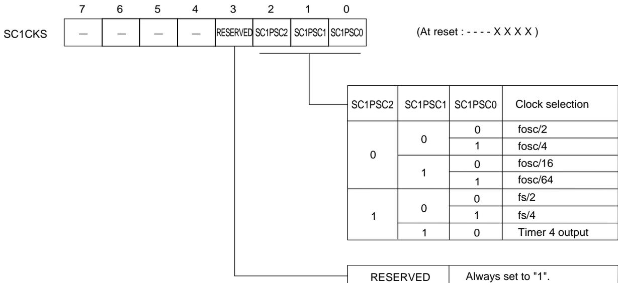
Figure 12-2-8 Serial Interface 1 Transfer Clock Selection Register (SC1CKS : x'03F9F', R/W)
