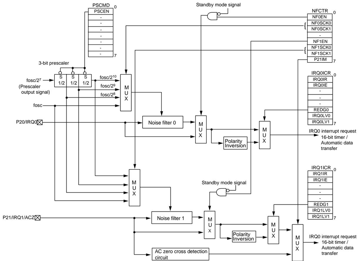
Figure 3-3-1 External Interrupt 0 Interface and External Interrupt 1 Interface Block Diagram
