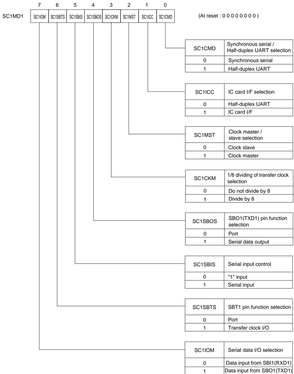
Figure 12-2-4 Serial Interface 1 Mode Register 1 (SC1MD1 : x'03F9B', R/W)
