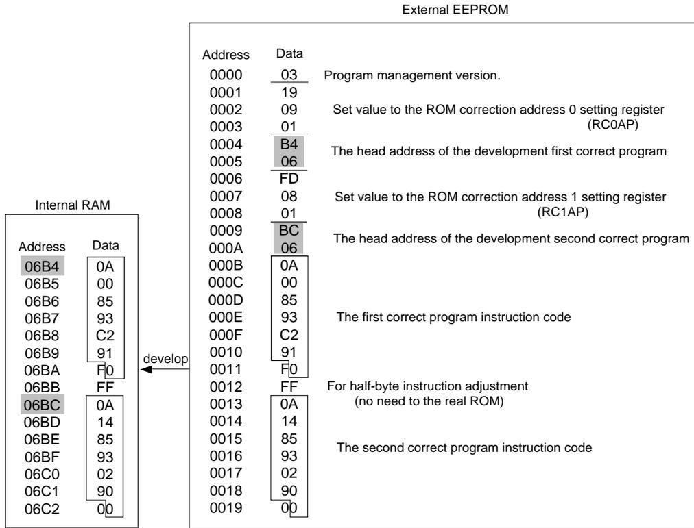
(STEP 2) Set the ROM correction address setting register and the RC vector table.
