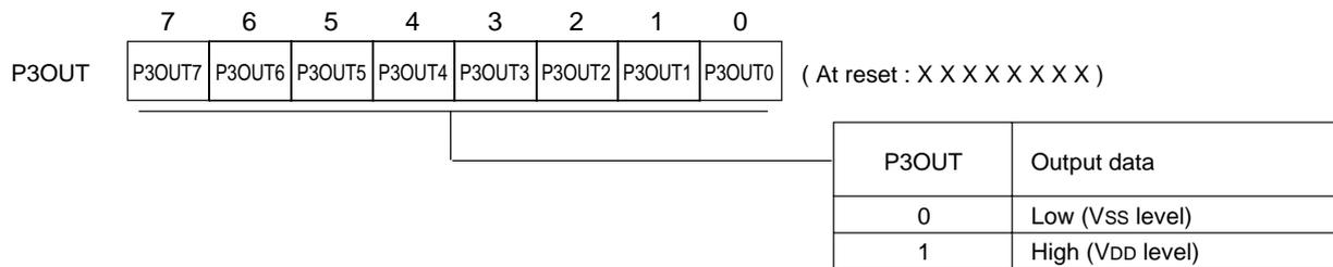
Port 3 output register (P3OUT : x'03F13', R/W)
