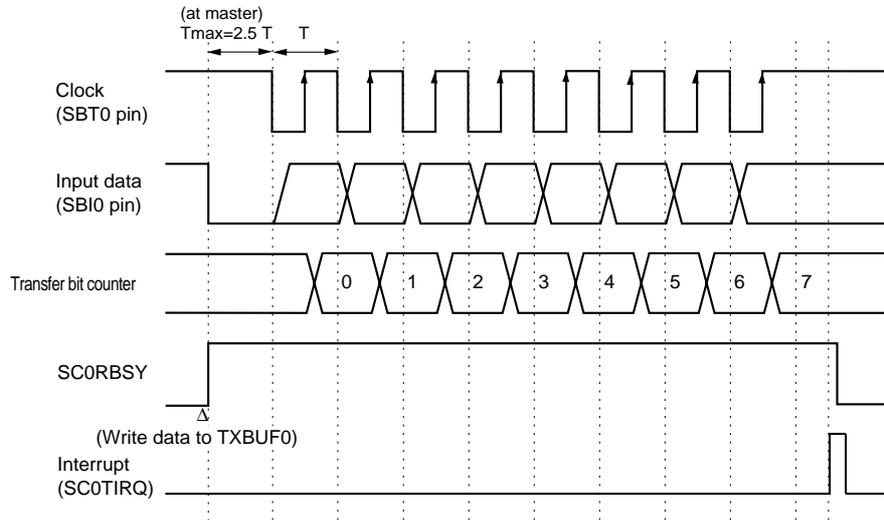
Figure 11-3-9 Reception Timing (rising edge, start condition is enabled)
