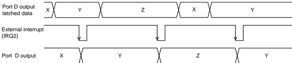
**Figure 4-15-2 Synchronous Output Timing by Event Generation (IRQ2)**
