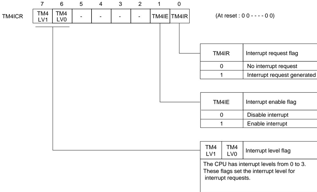
Figure 3-2-12 Timer 4 Interrupt Control Register (TM4ICR : x'03FED', R/W)
