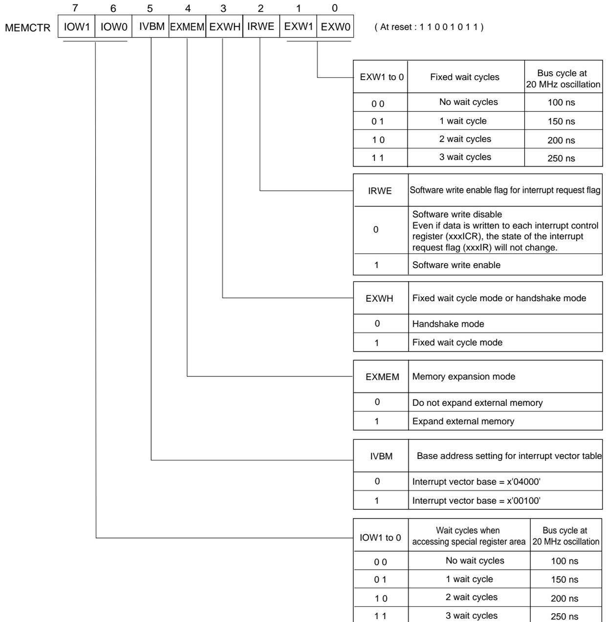
Figure 2-3-2 Memory Control Register (MEMCTR: x'03F01' R/W)
