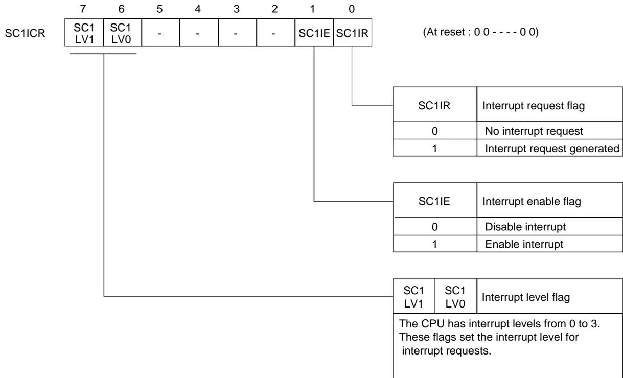
Figure 3-2-19 Serial Interface 1 Interrupt Control Register (SC1ICR : x'03FF7', R/W)
