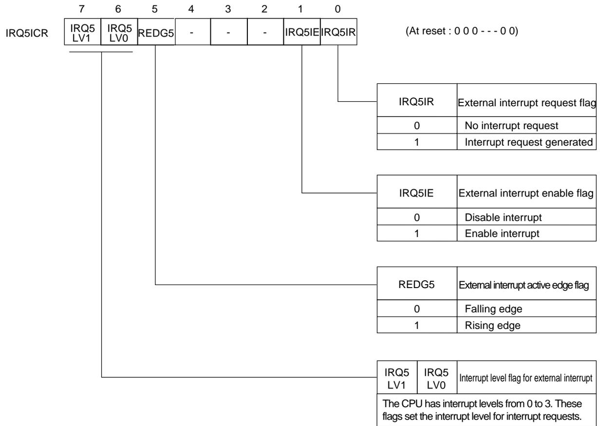
Figure 3-2-7 External Interrupt 5 Control Register (IRQ5ICR : x'03FE7', R/W)
