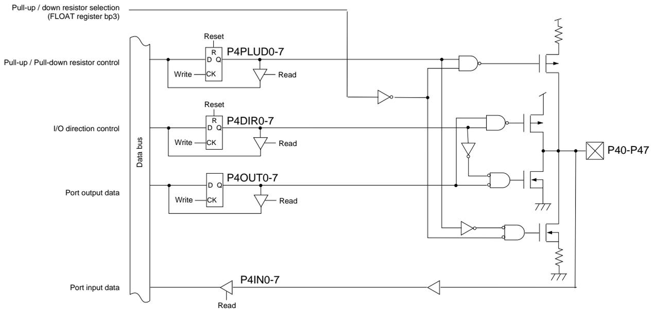
Figure 4-6-3 Block Diagram (P40 to P47)
