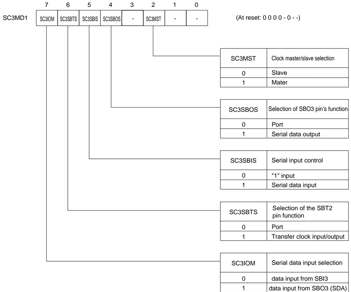
Figure 14-2-3 Serial Interface 3 Mode Register 1 (SC3MD1 : x'03FA9', R/W)
