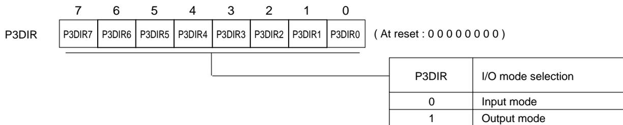
Port 3 direction control register (P3DIR : x'03F33', R/W)
