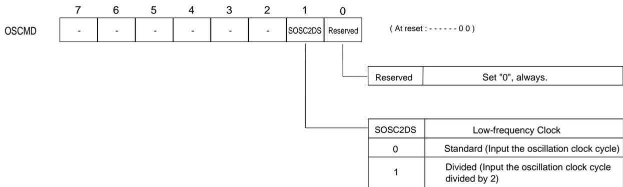
Figure 2-5-1 Oscillator Frequency Control Register (OSCMD : x'03F0D', R/W)
