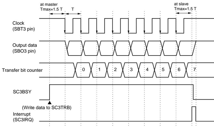
Figure 14-3-3 Transmission Timing (Falling edge, Disable Start Condition)
