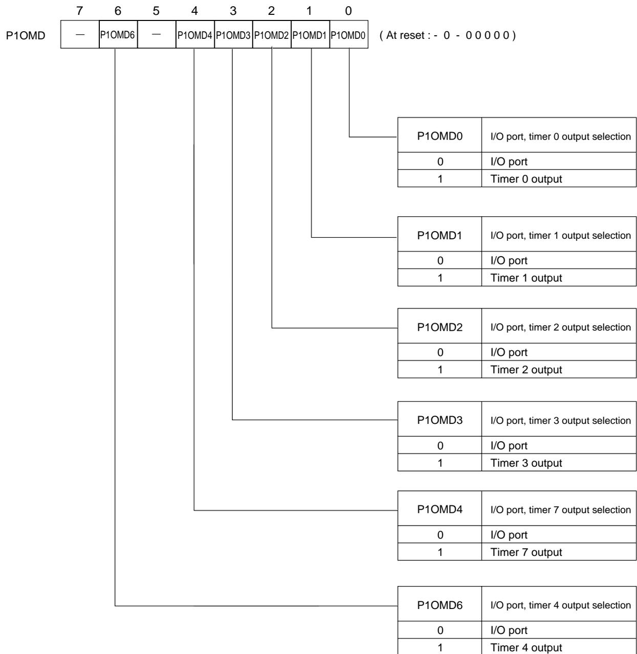
Port 1 output mode register (P1OMD : x'03F2F', R/W)
