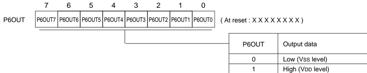
Port 6 output register (P6OUT : x'03F16', R/W)
