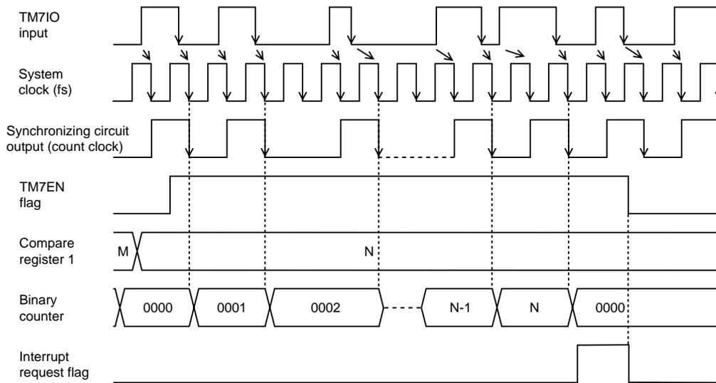
Figure 7-4-2 Count Timing of Synchronous TM7IO Input (Timer 7)
