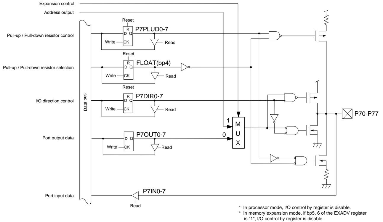
Figure 4-9-3 Block Diagram (P70 to P77)
