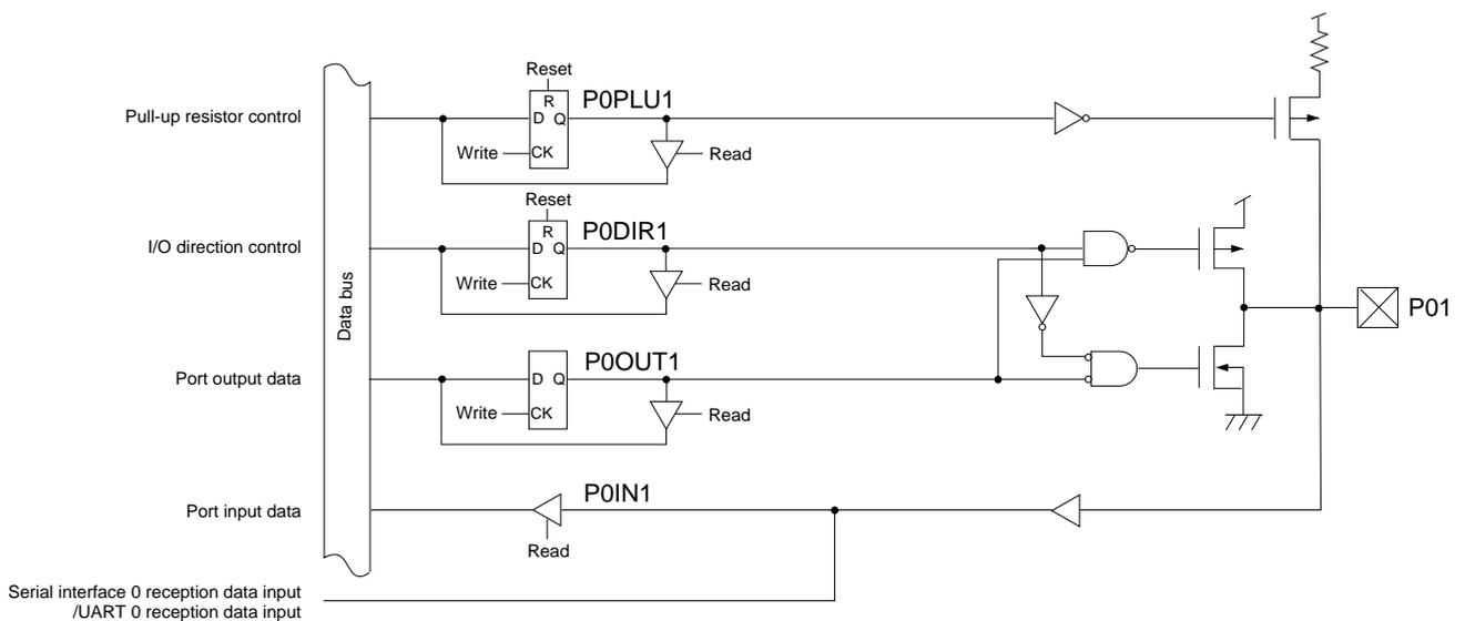
Figure 4-2-3 Block diagram (P01)
