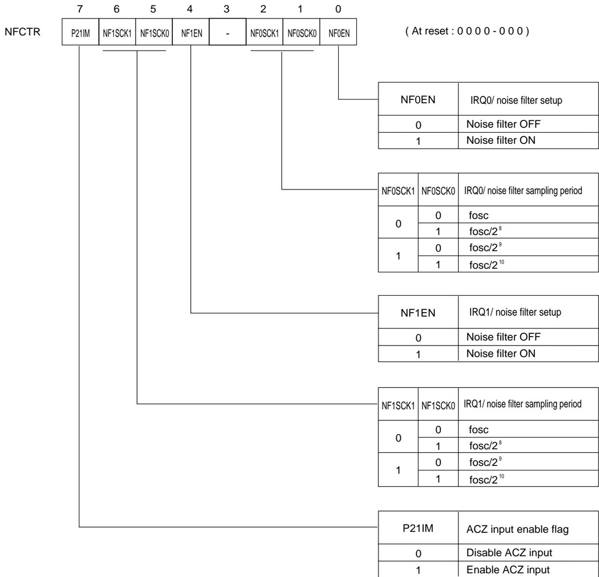
Figure 3-3-4 Noise Filter Control Register (NFCTR : x'03F8E', R/W)
