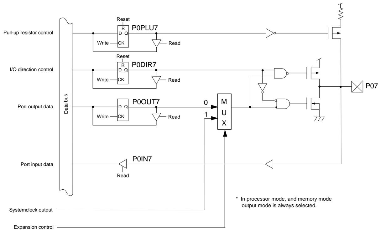
Figure 4-2-9 Block Diagram (P07)
