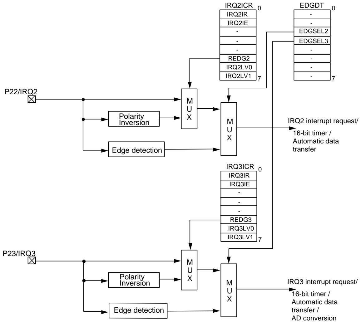
Figure 3-3-2 External Interrupt 2 Interface and External Interrupt 3 Interface, Block Diagram
