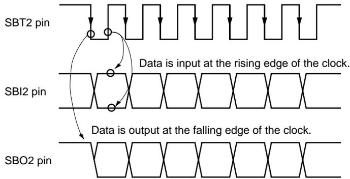
**Figure 13-3-10 Transmission / Reception Timing
