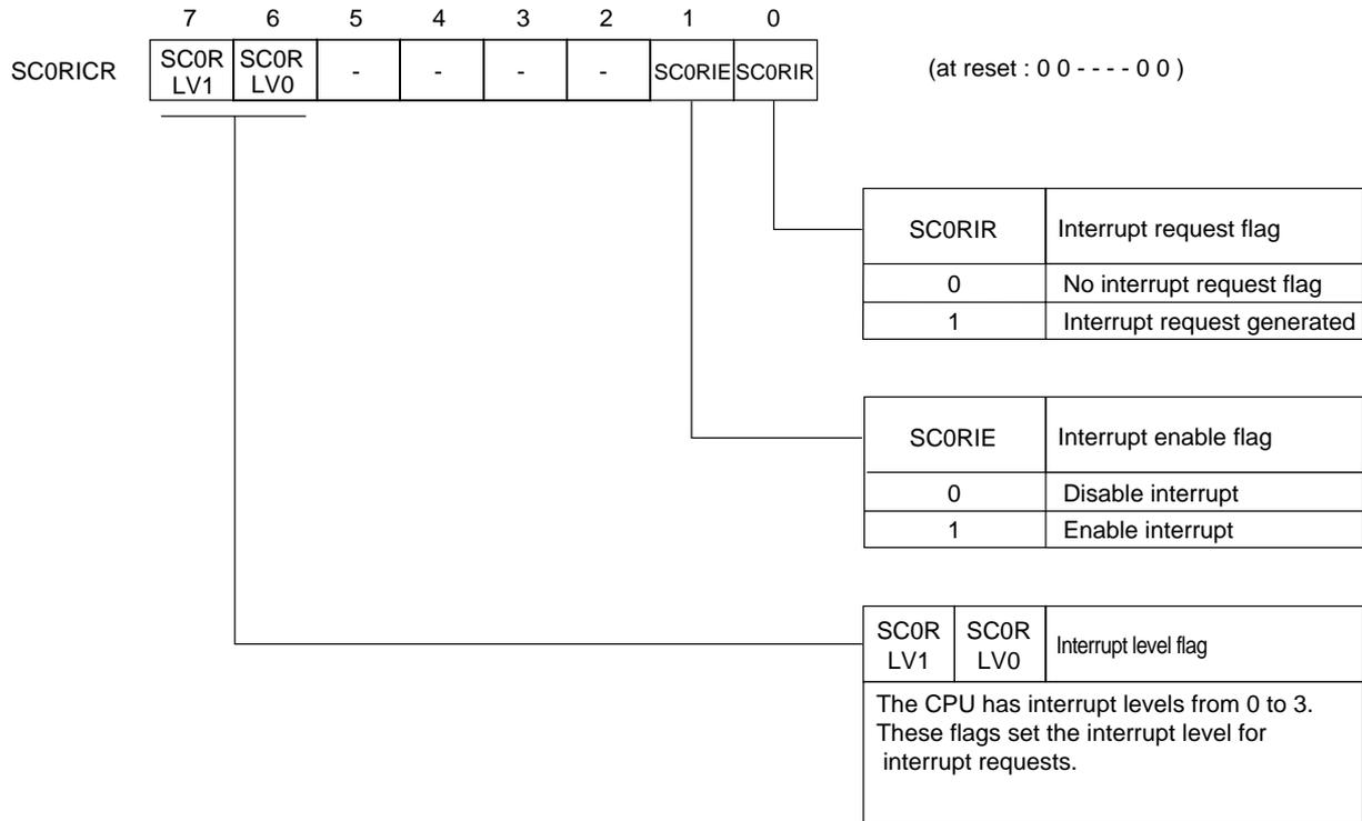
**Figure 3-2-17 Serial Interface 0 UART Reception Interrupt Control register (SC0RICR:x'03FF5', R/W)**
