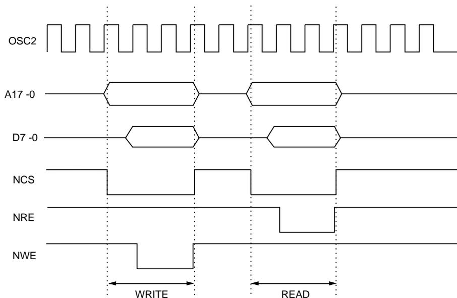
**Figure 2-3-5 ROM and RAM Access Timing with 1 Wait Cycle**
