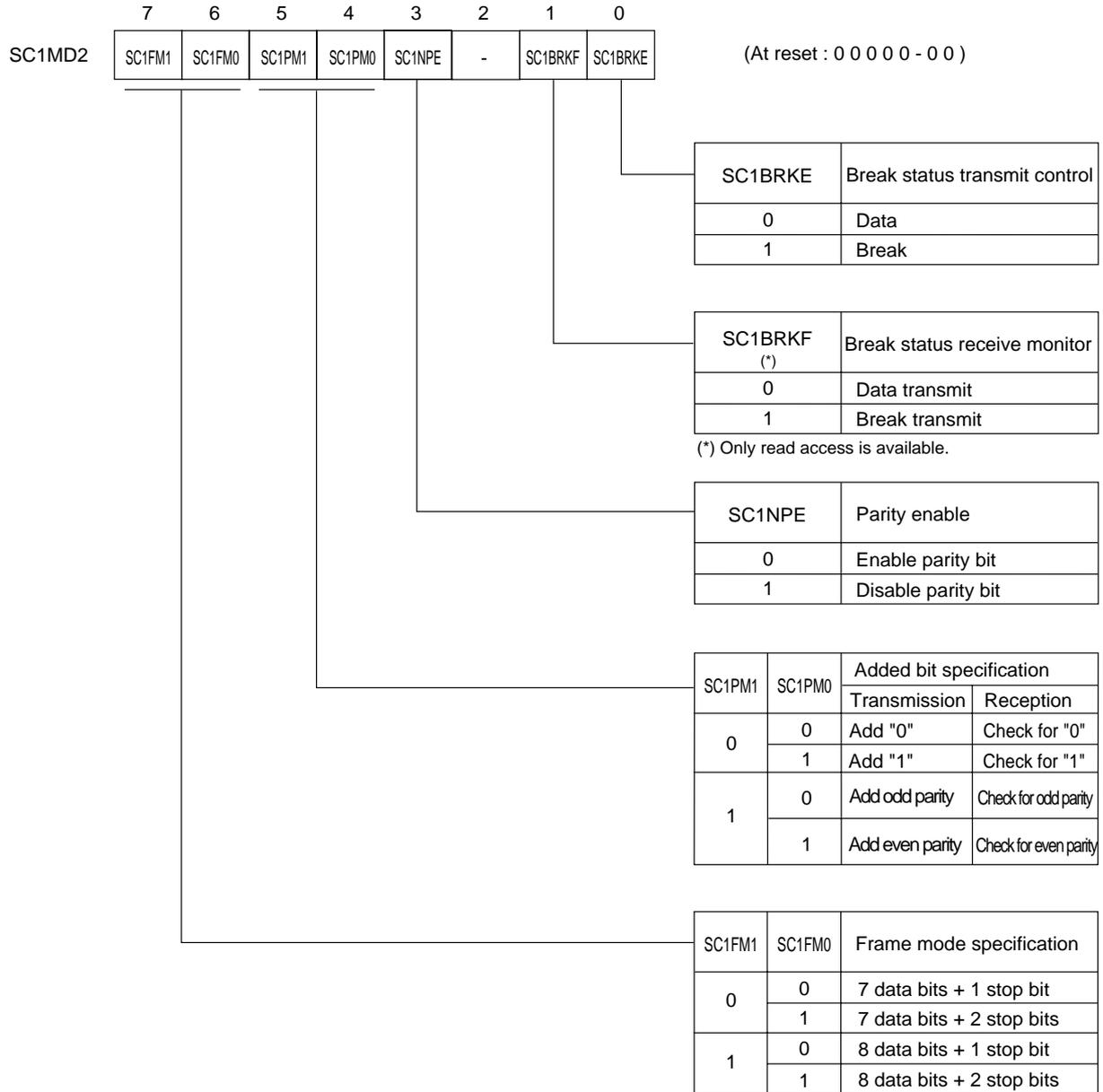
Figure 12-2-5 Serial Interface 1 Mode Register 2 (SC1MD2 : x'03F9C', R/W)
