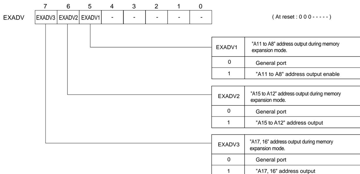
Figure 2-3-3 Expansion Address Control Register (EXADV : x'03F0E', R/W)
