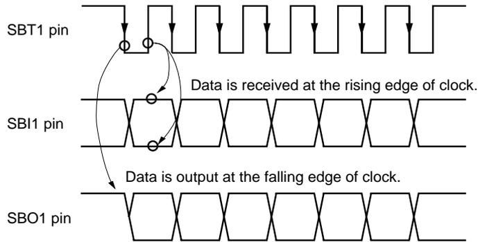
**Figure 12-3-12 Transmission / Reception Timing
