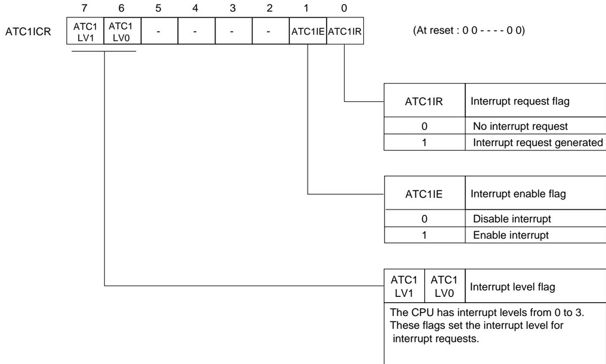
Figure 3-2-23 ATC1 Interrupt Control Register (ATC1ICR : x'03FFC', R/W)
