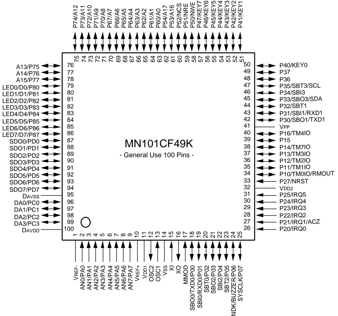
Figure20-2-1 Pin Configuration ( 100QFP : Top view )
