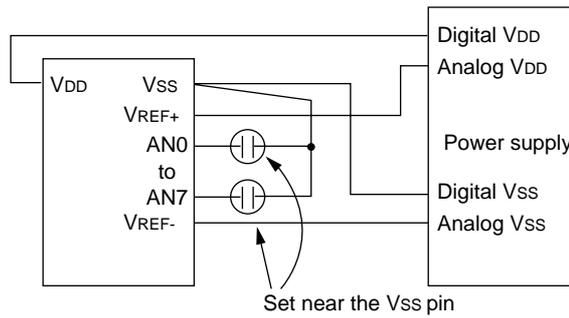
Figure 16-3-2 A/D Converter Recommended Example 1
