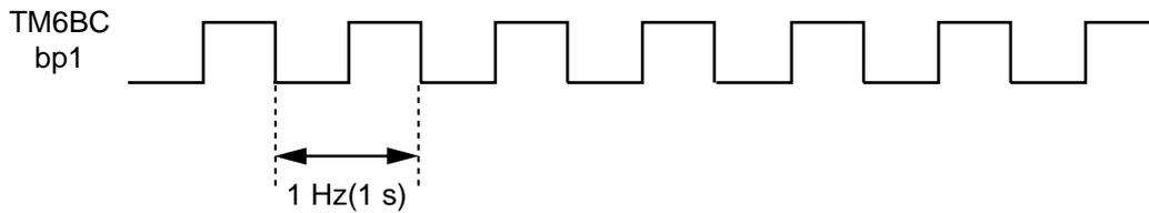
**Figure 8-3-1 Waveform of TM6BC Register bp1 (Timer 6)**
