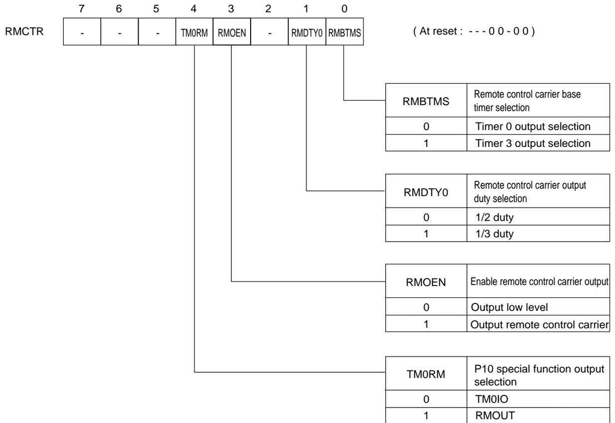
Figure 6-2-16 Remote Control Carrier Output Control Register (RMCTR : x'03F6E', R/W)
