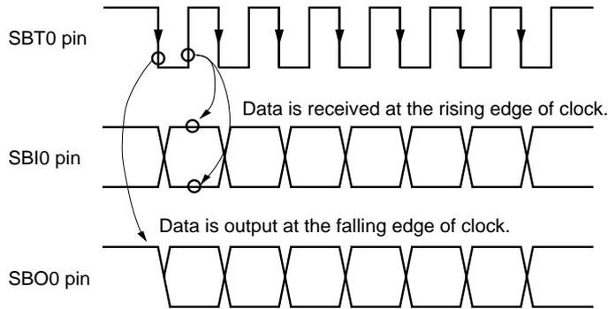
**Figure 11-3-13 Transmission / Reception Timing
