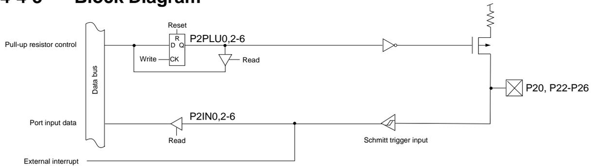
P26 is not used as an external interrupt pin
