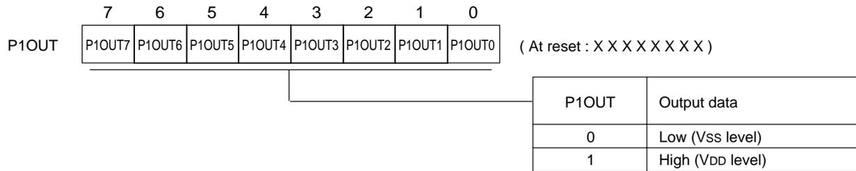
Port 1 output register (P1OUT : x'03F11', R/W)
