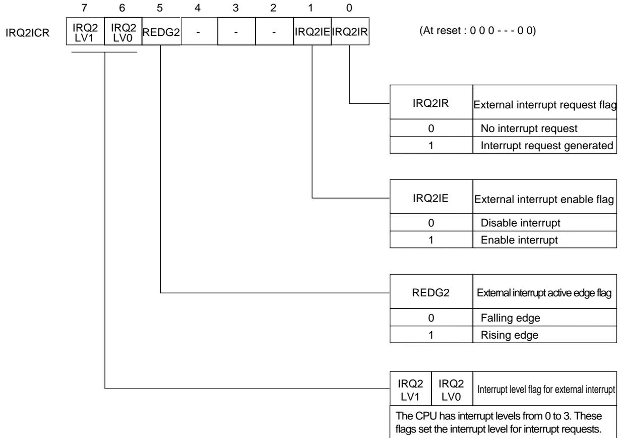
Figure 3-2-4 External Interrupt 2 Control Register (IRQ2ICR : x'03FE4', R/W)
