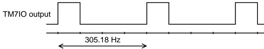
**Figure 7-6-4 Output Waveform of TM7IO Output Pin**
