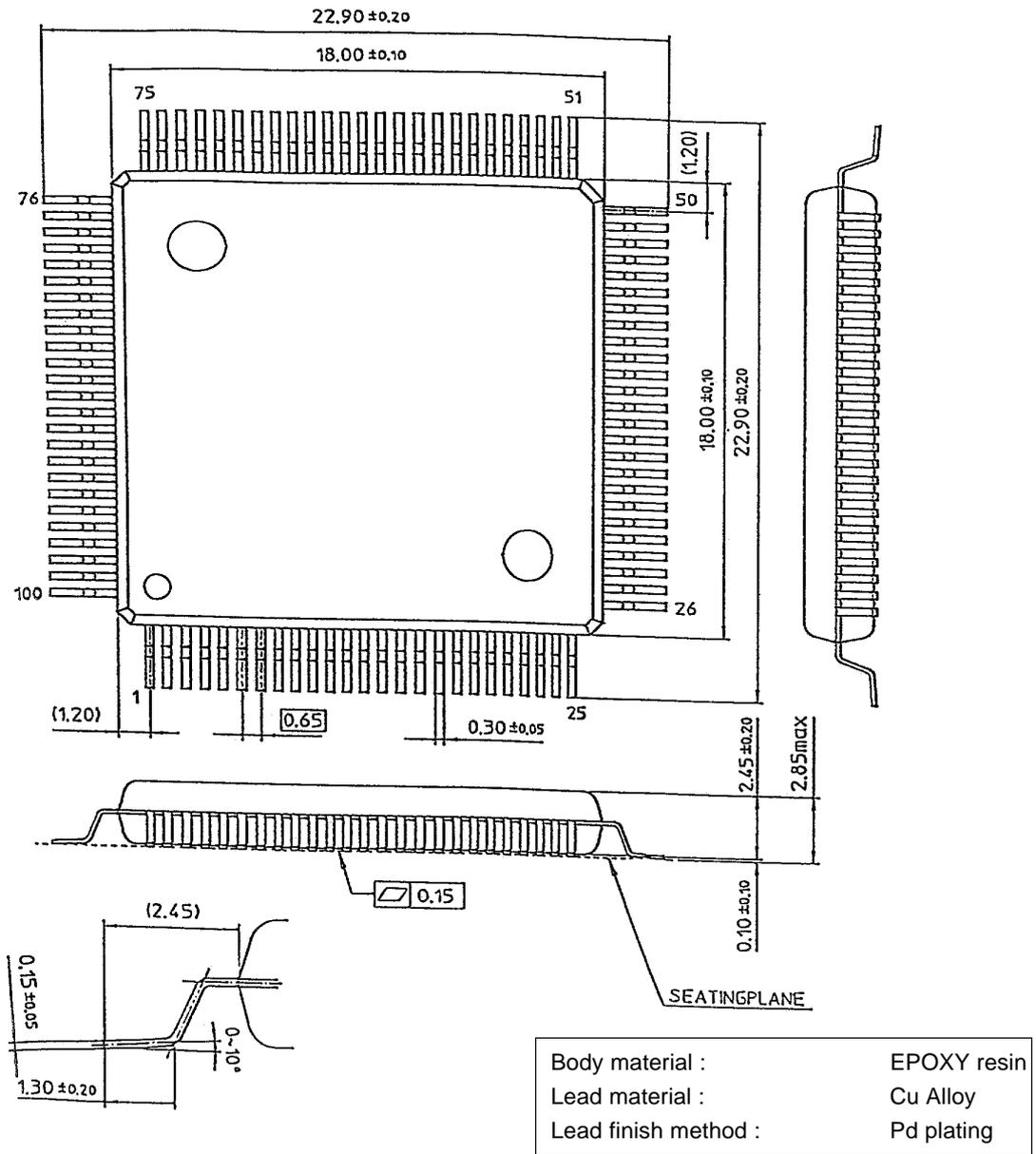
Figure 1-6-1 100-Pin QFP
