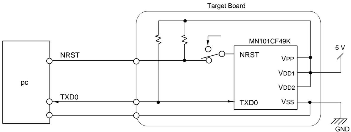
**Figure 20-6-1 Target Board for programming with the UART communication using PC**
