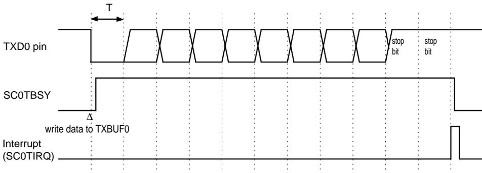
Figure 11-3-21 Transmission Timing (parity bit is disabled)
