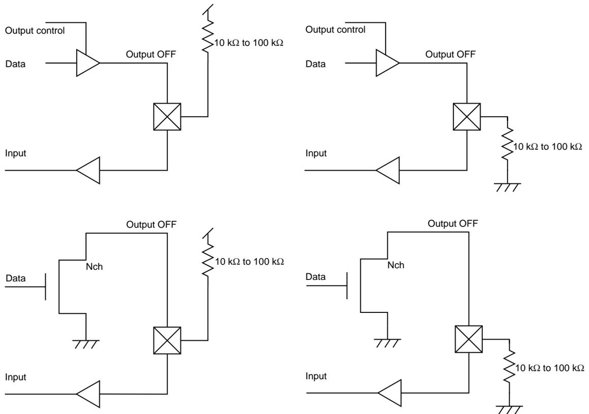
Figure 1-7-3 Unused I/O pins (high impedance output at reset)
