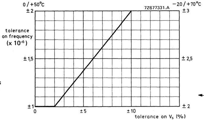
Fig. 4 Frequency tolerance as a function of the tolerance on supply voltage over the entire temperature range.
