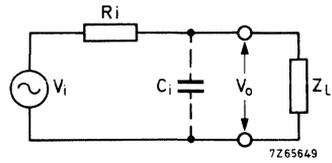
Fig. 3 Equivalent circuit.
