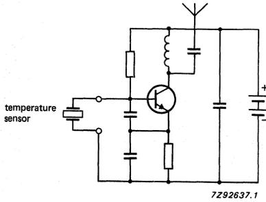
Fig. 4 Miniature wireless temperature sensor.
