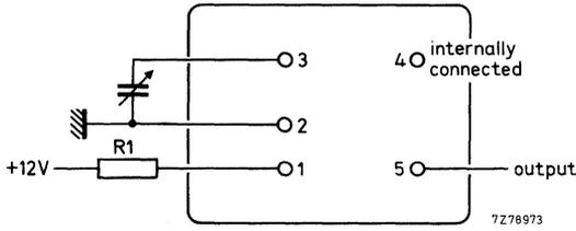
Fig. 2 Connection diagram.
