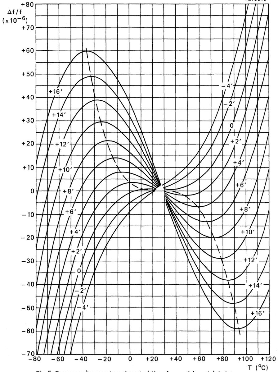
Fig. 5 Frequency/temperature characteristics of a special crystal design.
