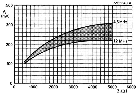
Fig. 4 Output voltage as a function of load impedance (typical values).
