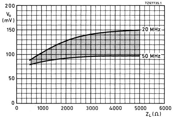
Fig. 5 Output voltage as a function of load impedance (typical values).
