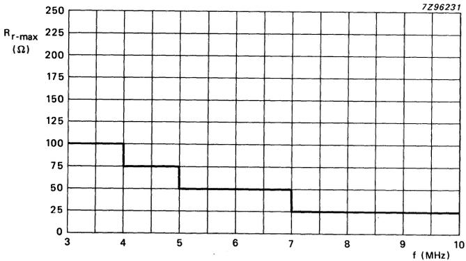
Fig. 2 Resonance resistance  $R_r$  as a function of frequency.
