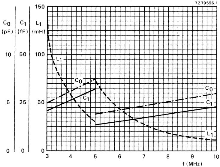
Fig. 1 Typical values for  $C_0$ ,  $C_1$  and  $L_1$  as a function of frequency.
