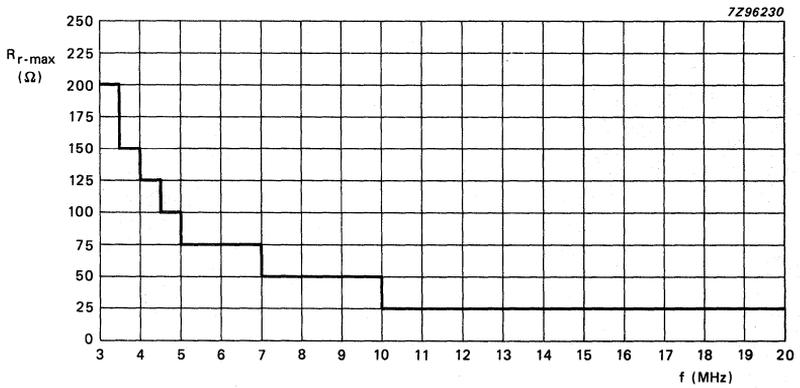
Fig. 2 Resonance resistance,  $R_r$  as a function of frequency.
