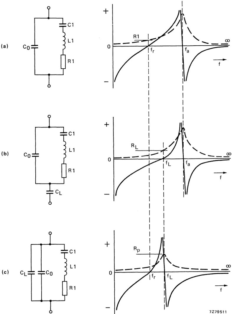
Fig. 2 Resonance, anti-resonance and load resonance frequency.
