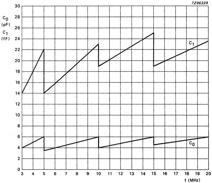
Fig. 1 Motional ( $C_1$ ) and parallel ( $C_0$ ) capacitances as a function of frequency.
