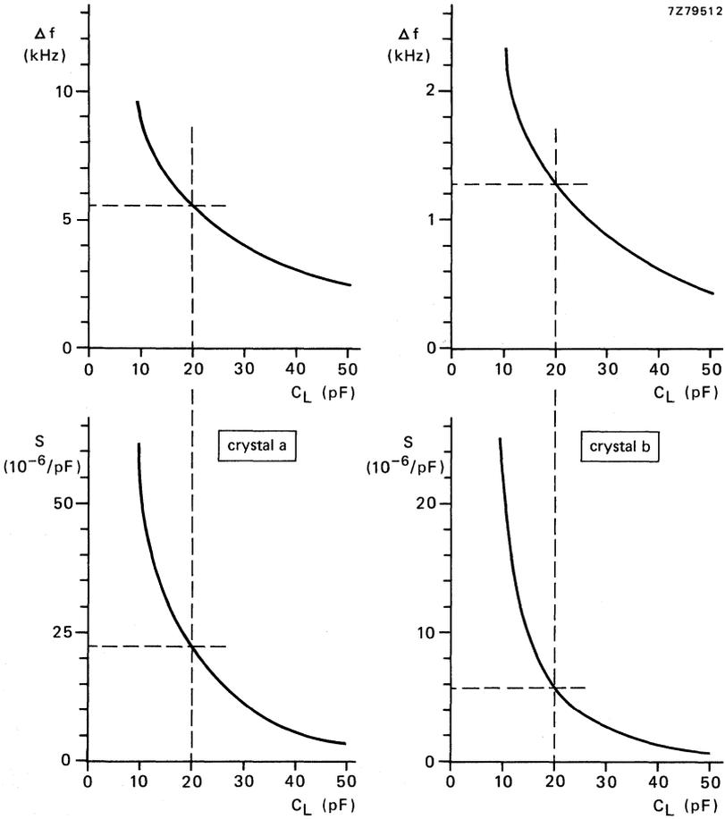
Fig. 3  $\Delta f$  and pulling sensitivity as a function of the load capacitance. Tolerances on the parameters  $f_r$ ,  $C_0$  and  $C_1$  are required for calculating the " $\Delta f$ " and the "pullability at  $f_n$ ".
