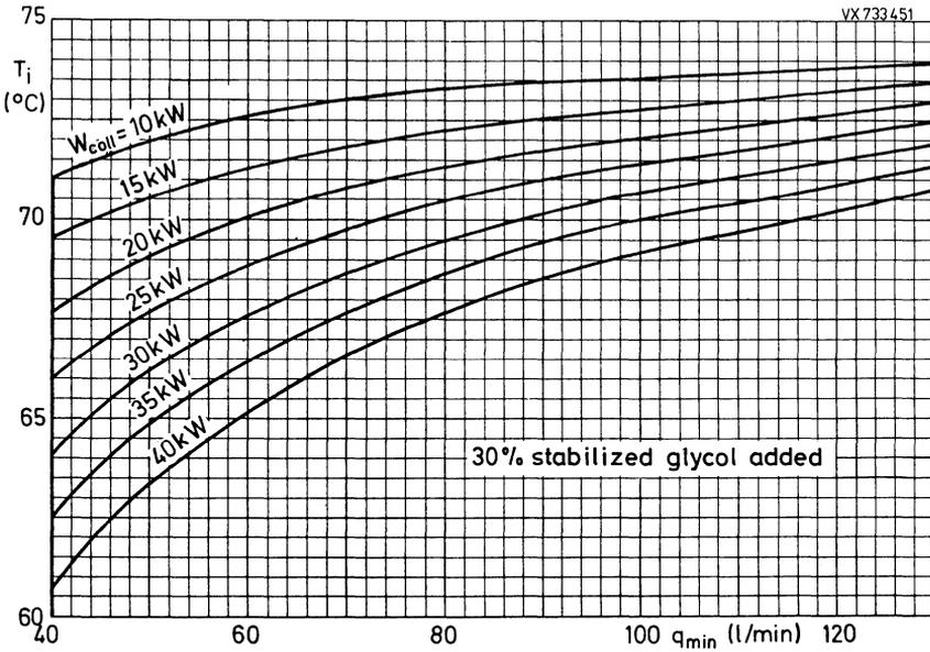
Fig. 9 Cooling curves for closed circuit cooling.
