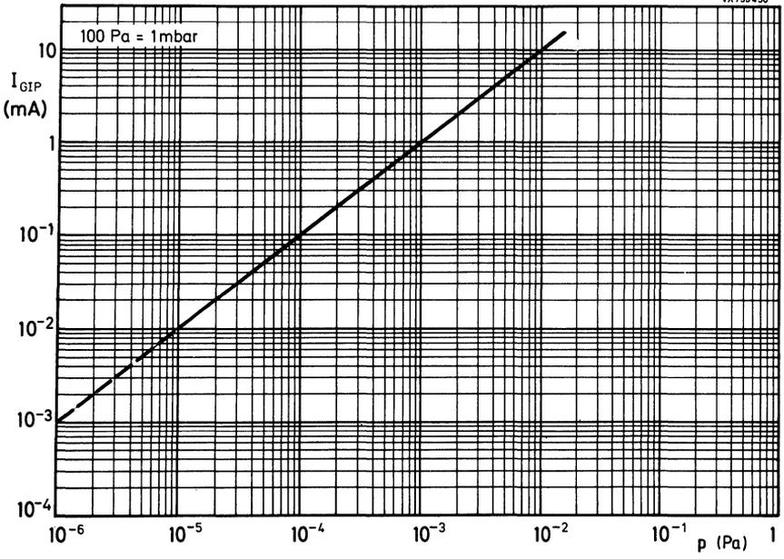
Fig. 4 Ratio of pump current to gas pressure in the klystron.
