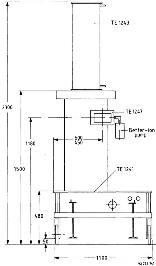
Fig. 3 Complete assembly consisting of tube, trolley, oil tank, focus mount, r.f. transition and operational lead shieldings.
