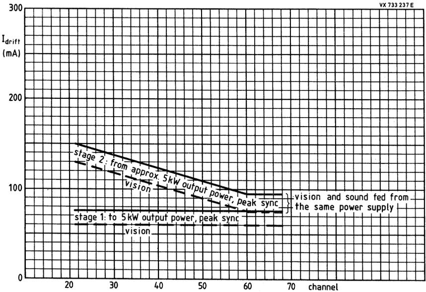
Fig. 7 Drift tube current cut-out at operation without depressed collector voltage for 20 kW transmitter.
