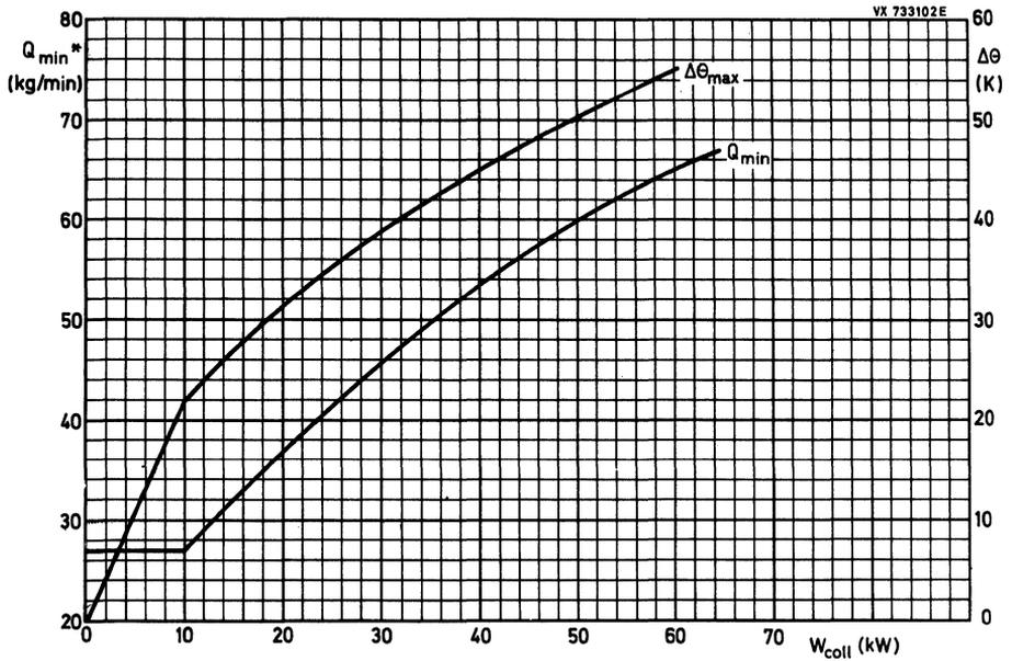
Fig. 3 Required quantity of cooling air  $Q_{min}$  for the inlet temperature  $T_i = 25^\circ\text{C}$  and relative temperature difference  $\Delta\theta$  versus the collector dissipation  $W_{coll}$ .
