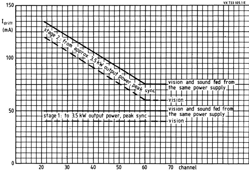
Fig. 8 Drift tube current cut-out at operation with depressed collector voltage for 10 kW transmitter.
