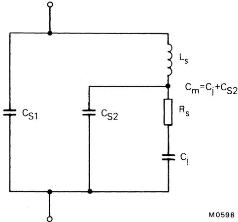
2. Measured at and about the series resonant frequency, in a suitable waveguide holder, enable the values of  $f_o$  and the diode Q factor to be determined. The effective diode capacitance and the cut-off frequency can be calculated taking  $L_s$  to be the typical value.
