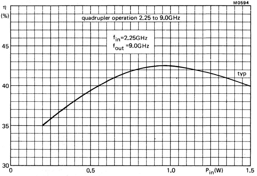
Overall efficiency as a function of input power
