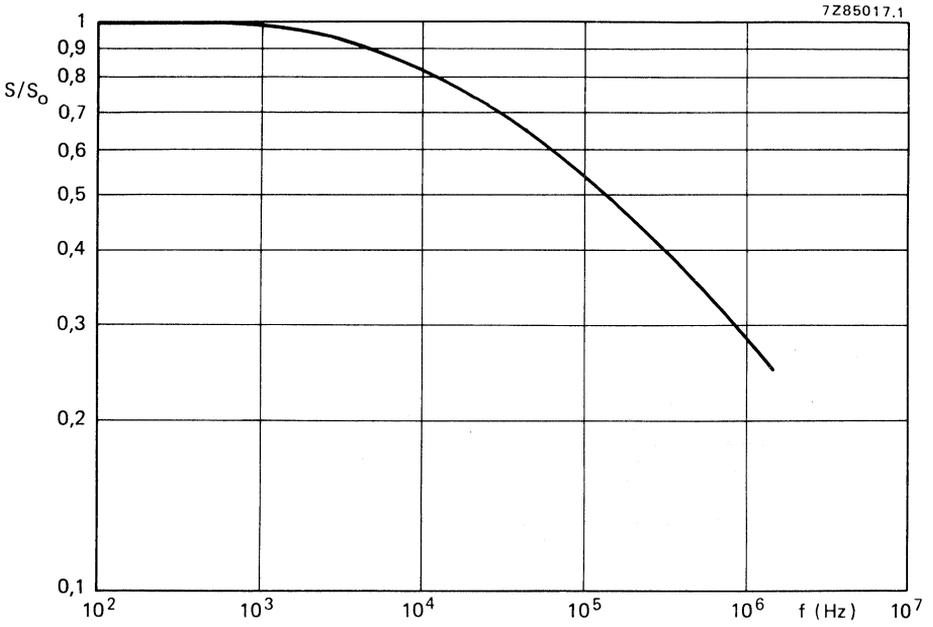
Fig. 4 Typical sensitivity variation of the fast coil versus the sweeping frequency
