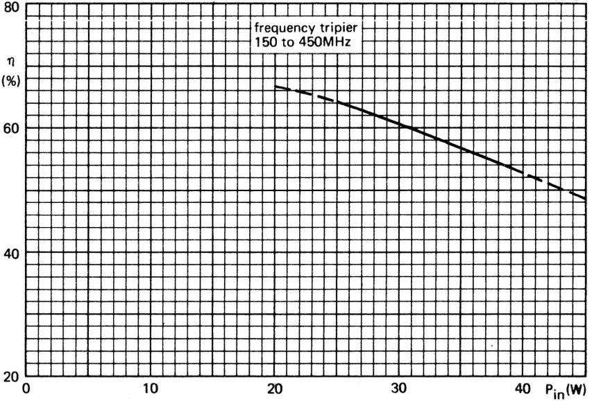
Typical tripler efficiency as a function of input power
