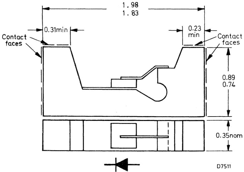
Contact faces are gold plated, 5  $\mu\text{m}$  over 1.27  $\mu\text{m}$  of nickel.
