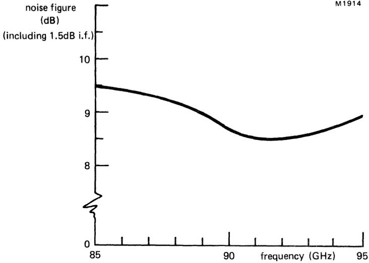
Fig.1 Typical noise figures as a function of frequency
