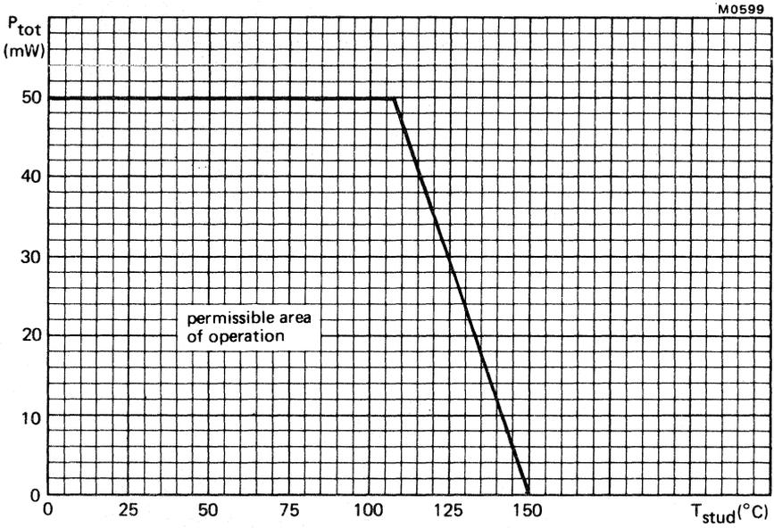
Total dissipation as a function of stud temperature
