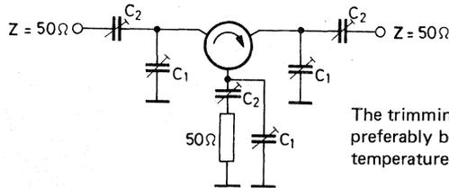
The trimming capacitors should preferably be of a type with low temperature coefficient.
