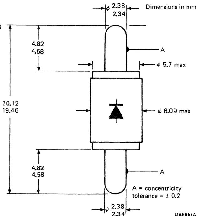
Terminal identification: diode symbol indicates polarity
