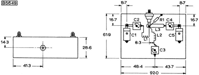
Component layout of tripler circuit
