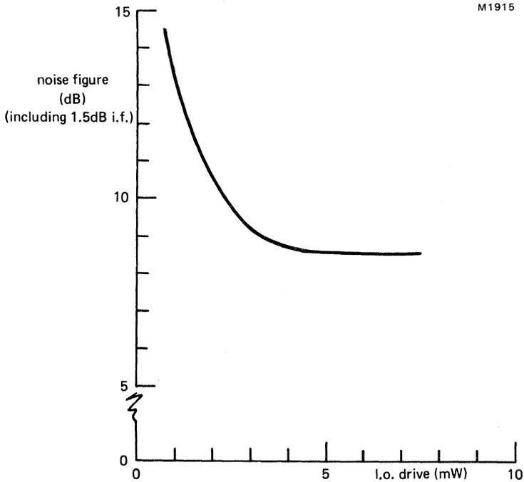
Fig.2 Typical noise figure as a function of local oscillator drive
