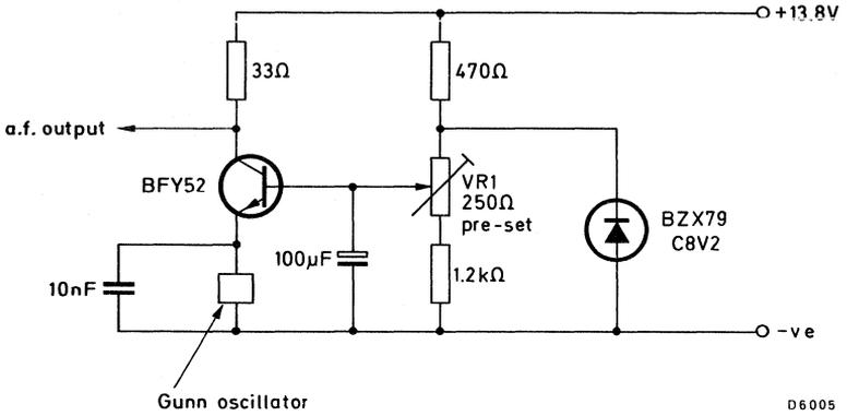
VR<sub>1</sub> is used to set voltage at 7.0 V across Gunn oscillator.
