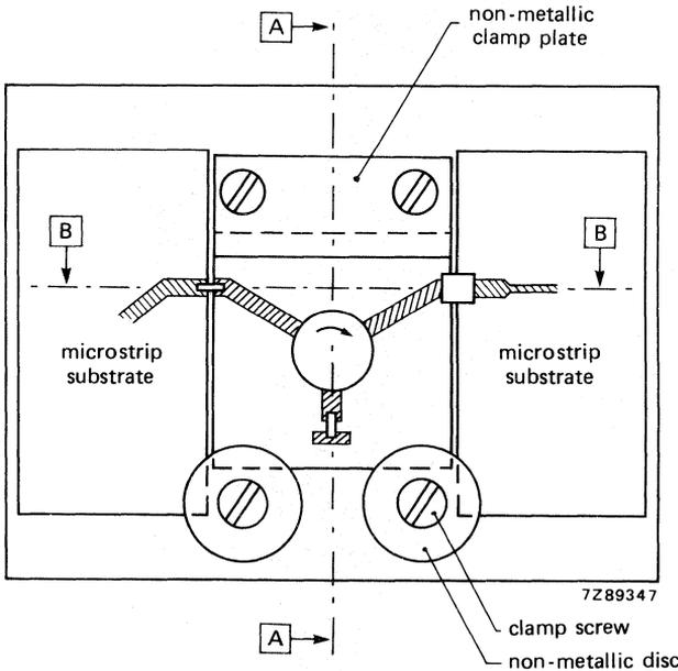
Two methods of mounting an isolator between MIC substrates:
