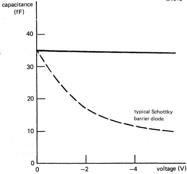
Fig.3 Typical capacitance as a function of voltage
