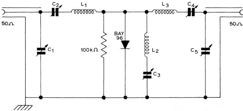
Frequency tripler circuit — 150 to 450 MHz
