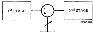
Phase modulation with a variable capacitance diode as a variable reactance
