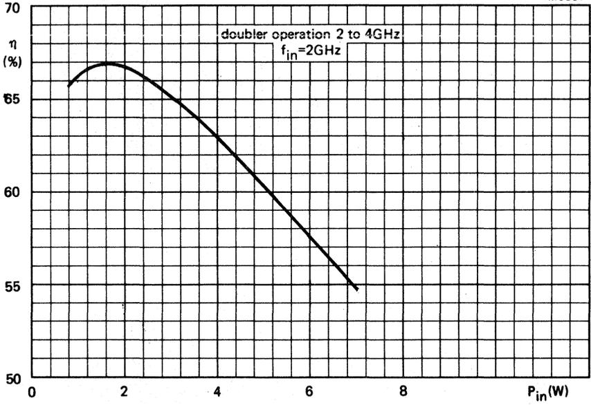
Overall efficiency as a function of input power for doubler operation
