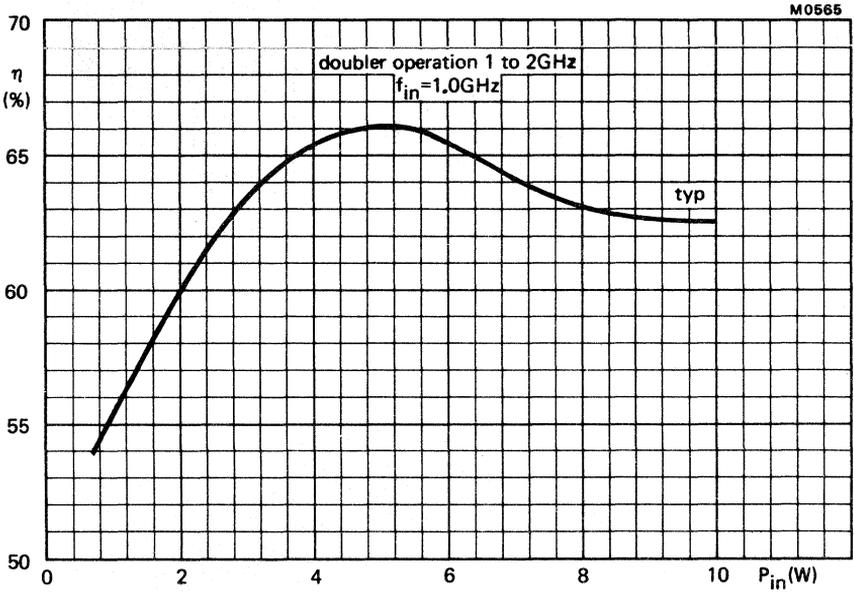
Overall efficiency as a function of input power
