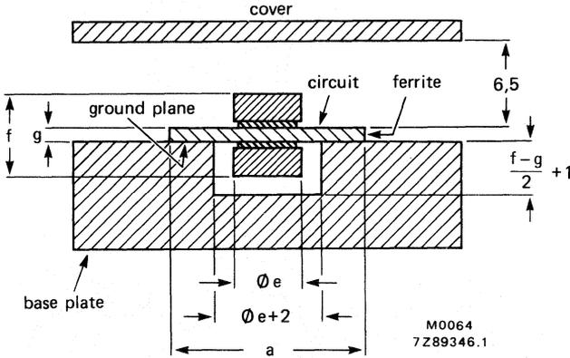
This figure gives the size of the recess in the base-plate and the height of the cover, assuming these parts are made of non-magnetic material. Increase these dimensions if magnetic material is used.
