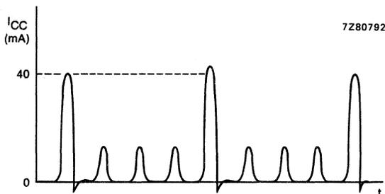
Fig. 3 Typical  $I_{CC}$  waveform with address change.
