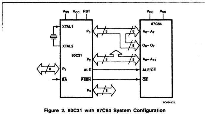
**Figure 2. 80C31 with 87C64 System Configuration**
