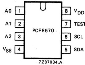
Fig. 2 Pinning diagram.
