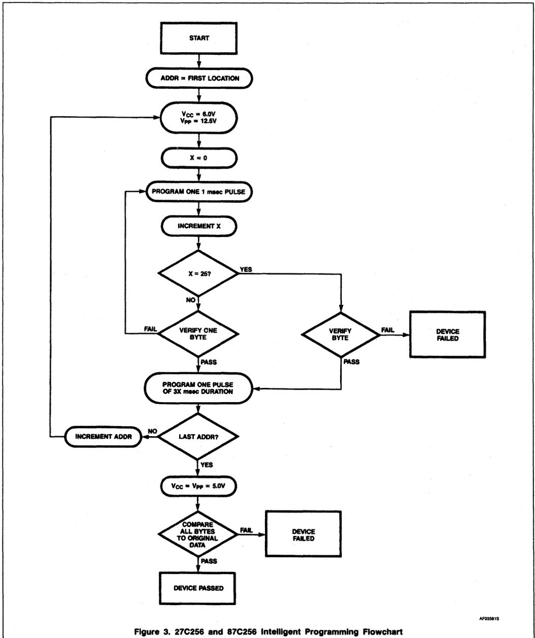
Figure 3. 27C256 and 87C256 Intelligent Programming Flowchart
