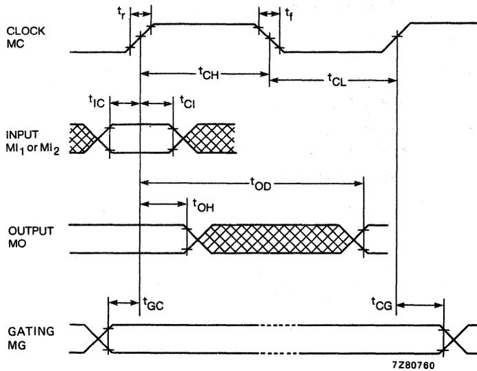
Fig. 7 Timing waveforms for gating and I/O.
