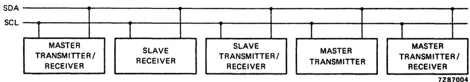
Fig. 5 System configuration.
