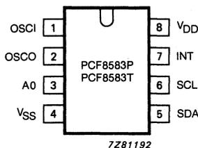
Fig. 2 Pinning diagram.
