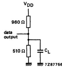
Fig. 4 Test load.
