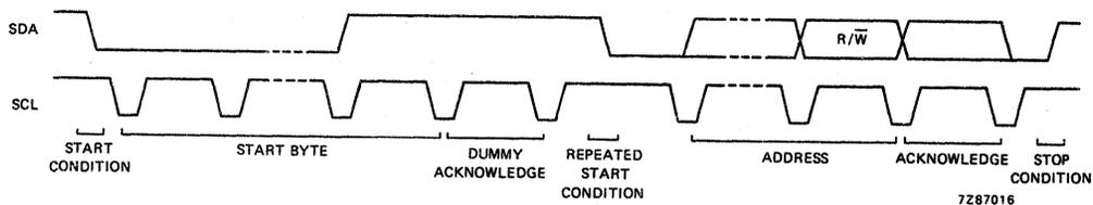
Fig. 10 Complete data transfer in the low-speed mode.
