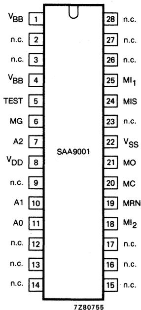
Fig. 2 Pinning diagram.
