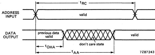
Fig. 6 Read cycle timing (1):  $R/\bar{W}$  is HIGH;  $\bar{CE}$  is LOW for a read cycle.
