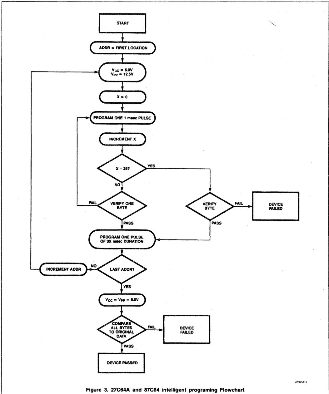
Figure 3. 27C64A and 87C64 intelligent programming Flowchart
