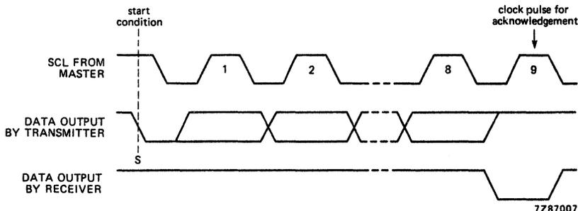
Fig. 6 Acknowledgement on the I<sup>2</sup>C bus.
