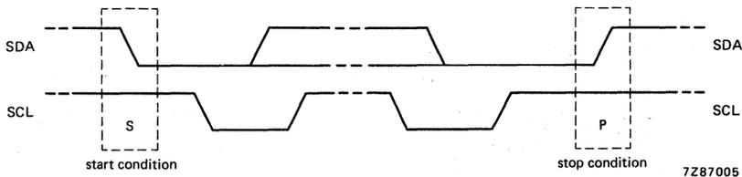
Fig. 4 Definition of start and stop conditions.
