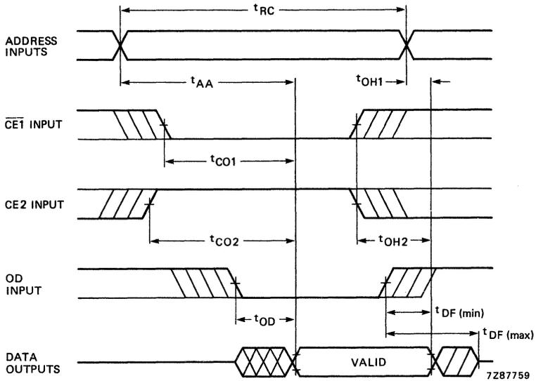
Fig. 6 Read cycle timing;  $R/\bar{W} = \text{HIGH}$ .
