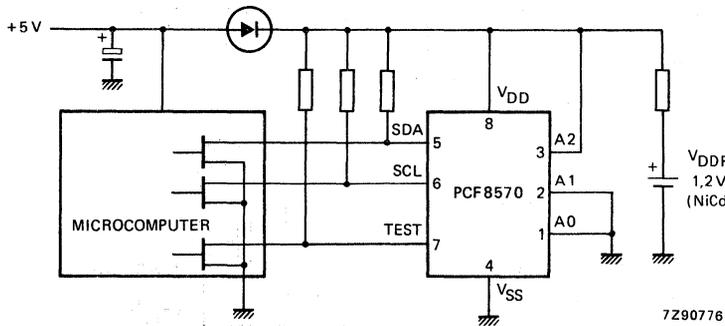
Fig. 15 Application example for power saving mode.
