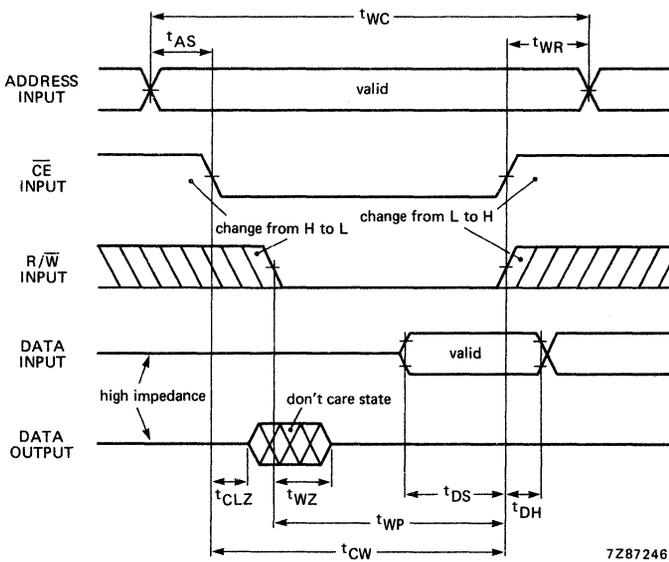
Fig. 9 Write cycle (2):  $\overline{CE}$  controlled.
