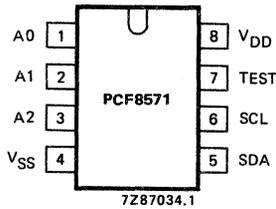
Fig. 2 Pinning diagram.
