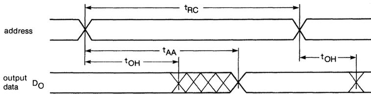
(b) Read cycle 2: device is continuously selected ( $\overline{CS} = V_{IL}$ );  $\overline{OE} = V_{IL}$
