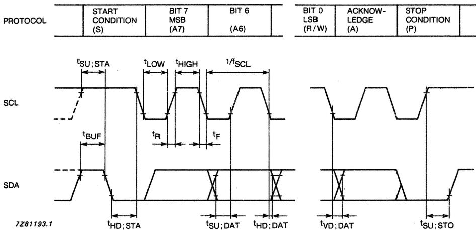
Fig. 14 I<sup>2</sup>C bus timing diagram.
