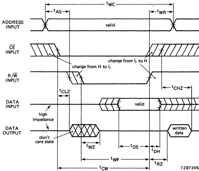
Fig. 8 Write cycle (1):  $\overline{R/W}$  controlled.
