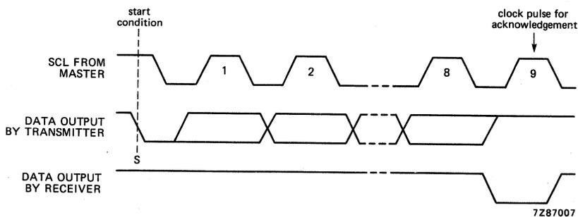
Fig. 13 Acknowledgement on the I<sup>2</sup>C bus.
