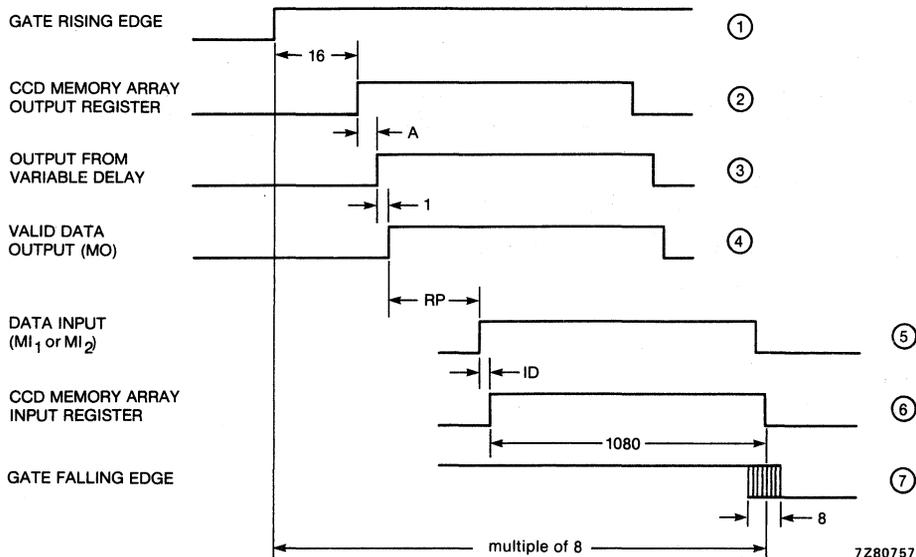
Fig. 4 Determination of memory gating HIGH period.
