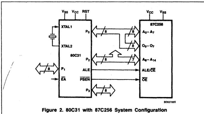
**Figure 2. 80C31 with 87C256 System Configuration**
