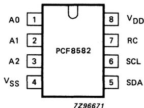
Fig. 2 Pinning diagram.
