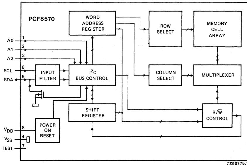
Fig. 1 Block diagram.
