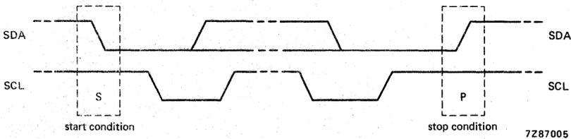
Fig. 4 Definition of start and stop conditions.
