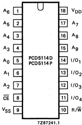
Fig. 2 Pinning diagram: PCD5114D; PCD5114P.
