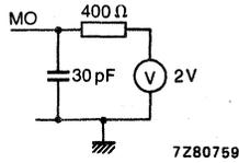
Fig. 6 Output load.
