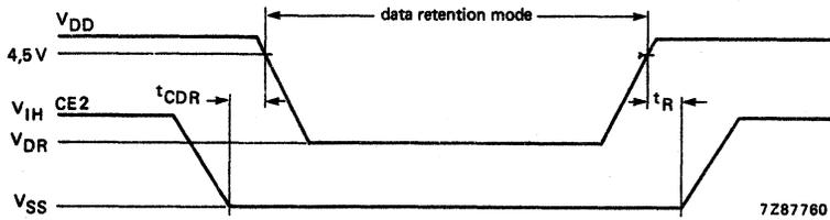
Fig. 8 Low supply voltage data retention characteristics.
