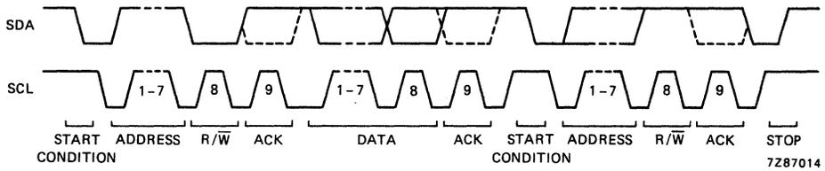
Fig. 8 Complete data transfer in the high-speed mode.
