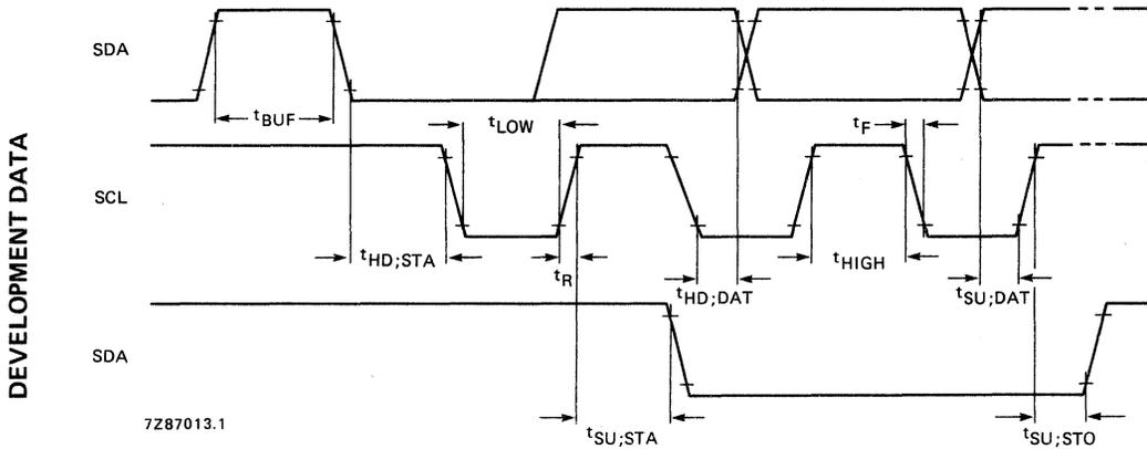
Fig. 4 I<sup>2</sup>C bus timing.
