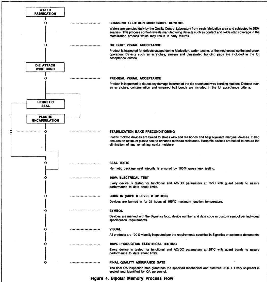
Figure 4. Bipolar Memory Process Flow
