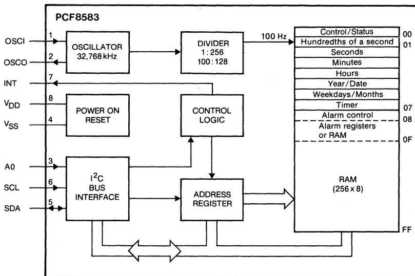
Fig. 1 Block diagram.
