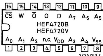
Fig. 2 Pinning diagram.
