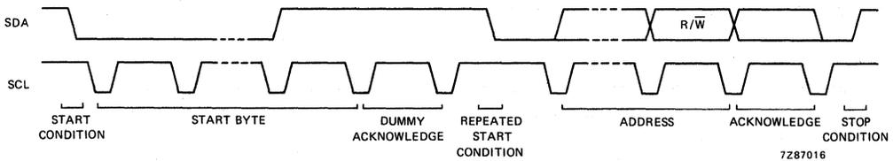
Fig. 10 Complete data transfer in the low-speed mode.
