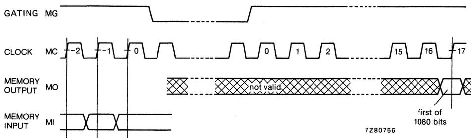
Fig. 3 Memory input and output data timings with respect to the memory clock (MC) for a memory gating (MG) HIGH period that is a multiple of 8 clock periods (no internal rounding of gating period).
