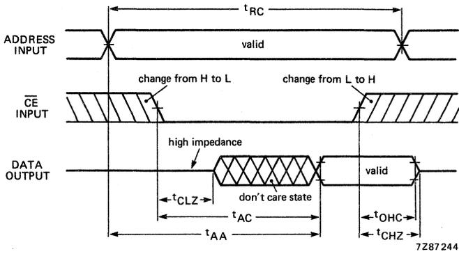
Fig. 7 Read cycle timing (2):  $R/\bar{W}$  is HIGH for a read cycle.
