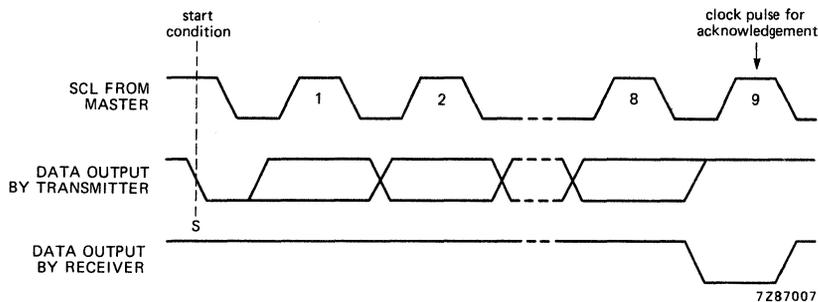
Fig. 6 Acknowledgement on the I<sup>2</sup>C bus.
