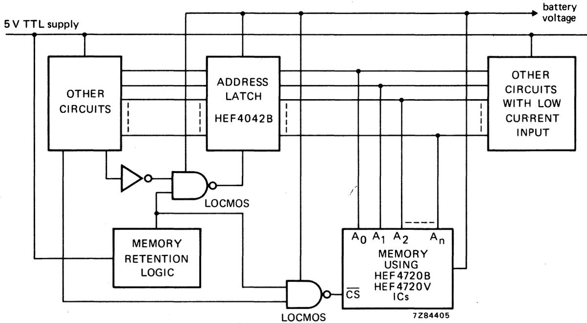
Fig. 11 Preferred solution for memory retention; all interface circuits are battery-fed LOCMOS. Note that maximum sink current of the HEF4042B is about 1,5 mA.
