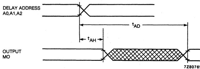
Fig. 8 Timing waveforms for address set-up and hold.
