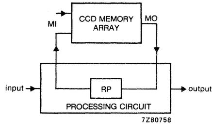
Fig. 5 Recirculation via an external circuit.
