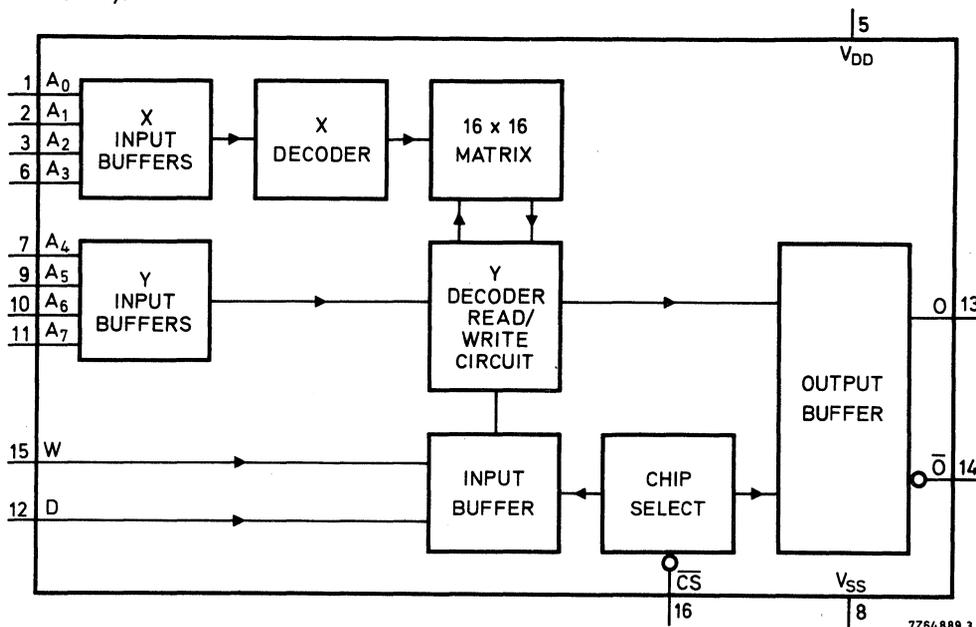
Fig. 1 Functional diagram.
