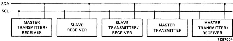
Fig. 12 System configuration.
