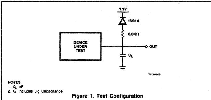
**Figure 1. Test Configuration**
