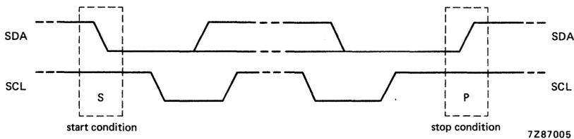
Fig. 11 Definition of start and stop condition.
