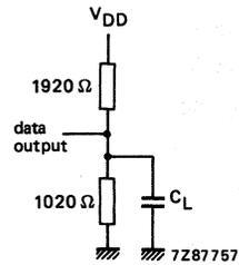
Fig. 5 Test load.
