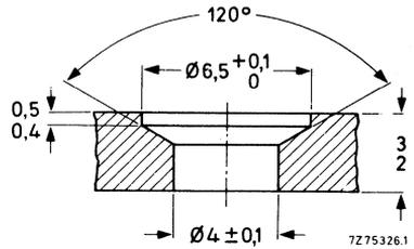
Fig. 5 Heatsink requirements
