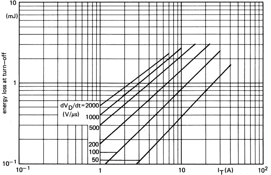
Fig.14 Maximum energy loss at turn-off (per cycle) as a function of anode current and applied  $dV_D/dt$  (calculated from  $I_T/C_S$ );  $dV_D/dt$  linear up to  $V_{Dmax} = 600$  V;  $V_{GR} = 10$  V;  $I_G = 0.5$  A;  $L_G \leq 0.5 \mu H$ ;  $L_S \leq 0.25 \mu H$ ;  $T_j = 120$  °C.
