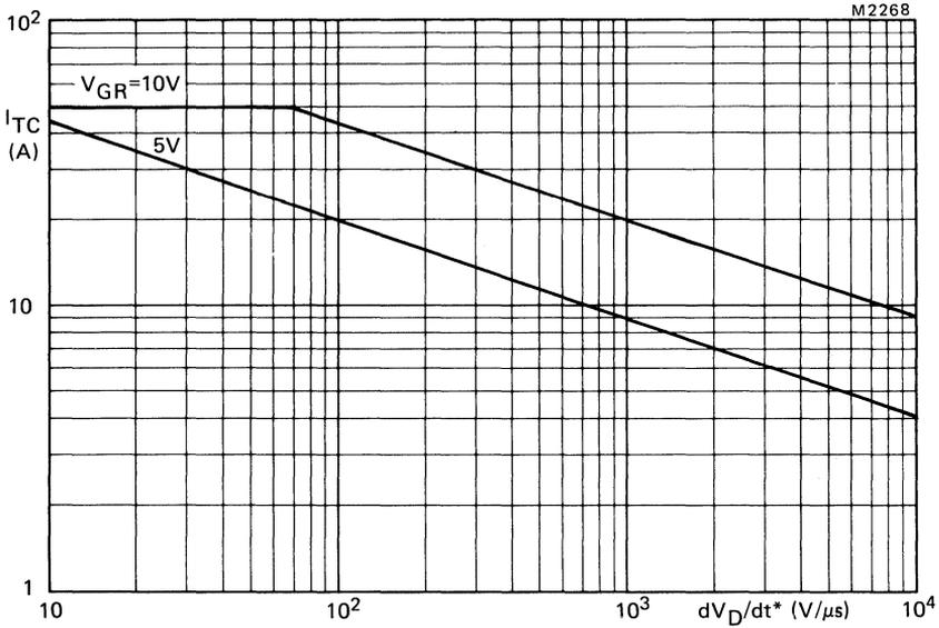
Fig.7 Anode current which can be turned off versus applied  $dV_D/dt^*$ ; inductive load;  $L_G \leq 0.5 \mu H$ ;  $L_S \leq 0.25 \mu H$ ;  $T_j = 120^\circ C$ . \* $dV_D/dt$  is calculated from  $I_T/C_S$ .
