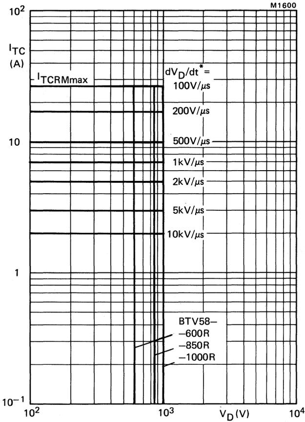
Fig.6 Anode current which can be turned off versus anode voltage; inductive load;  $V_{GR} = 10$  V;  $L_G \leq 1.0 \mu H$ ;  $L_S \leq 0.25 \mu H$ ;  $T_j = 85^\circ C$ .
