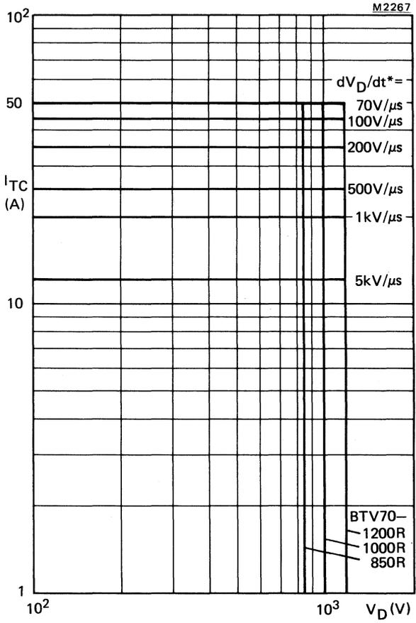
Fig.6 Anode current which can be turned off versus anode voltage; inductive load;
