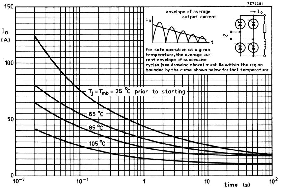
Fig. 10 Limits for starting or inrush currents.
