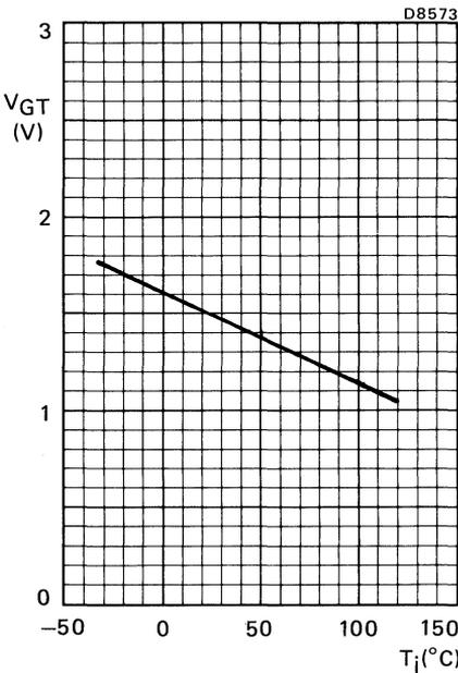
Fig.12 Minimum gate voltage that will trigger all devices; all conditions.
