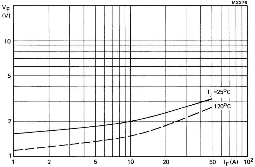
Fig.19 Forward voltage as a function of forward current; maximum values.
