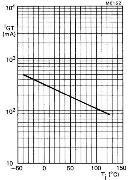
Fig.5 Minimum gate current that will trigger all devices plotted against junction temperature.
