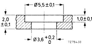
Fig. 11 Heatsink requirements for 800 V insulation.
