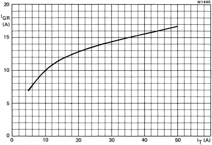
Fig.11 Peak reverse gate current versus anode current at turn-off; inductive load;  $V_{GR} = 10\text{ V}$ ;  $I_G = 0.5\text{ A}$ ;  $L_G = 0.4\text{ }\mu\text{H}$ ;  $T_j = 120\text{ }^\circ\text{C}$ ; maximum values.
