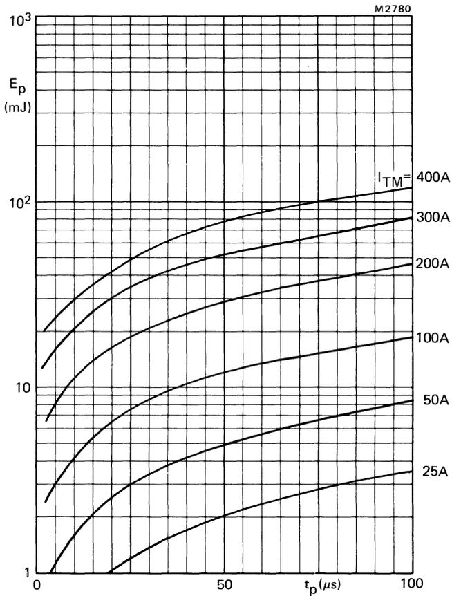
Fig.7 Maximum total energy loss per pulse when switching a half-sinusoidal pulse from 600 V.
