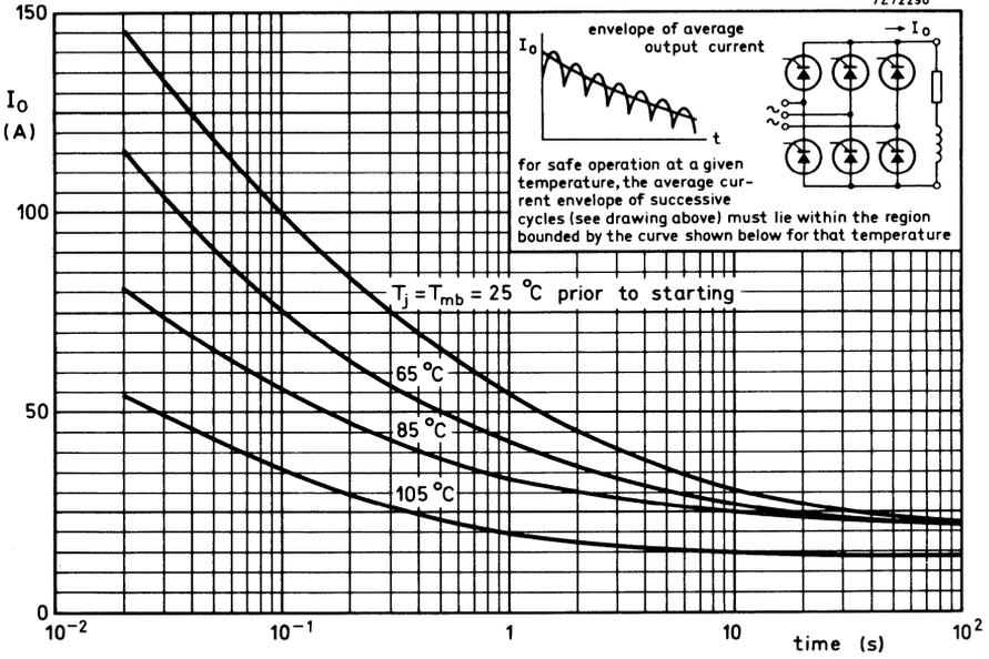
Fig. 11 Limits for starting or inrush currents.
