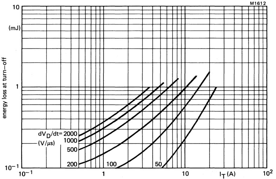
Fig.17 Maximum energy loss at turn-off (per cycle) as a function of anode current and applied  $dV_D/dt$  (calculated from  $I_T/C_S$ ); reapplied voltage sinusoidal up to  $V_{DRM} = 1200$  V;  $V_{GR} = 10$  V;  $I_G = 0.2$  A;  $L_G \leq 1.0 \mu H$ ;  $L_S \leq 0.25 \mu H$ ;  $T_j = 120$  °C.
