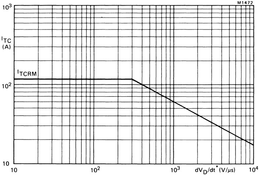
Fig.7 Anode current which can be turned off versus applied  $dV_D/dt^*$ ; inductive load;  $V_{GR} = 10$  V;  $L_G \leq 0.5 \mu H$ ;  $L_S \leq 0.25 \mu H$ ;  $T_j = 120$  °C. \* $dV_D/dt$  is calculated from  $I_T/C_S$ .
