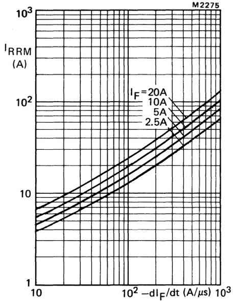
Fig.15 Peak reverse recovery current versus  $-di_F/dt$ ;  $T_j = 25^\circ\text{C}$ ; maximum values.
