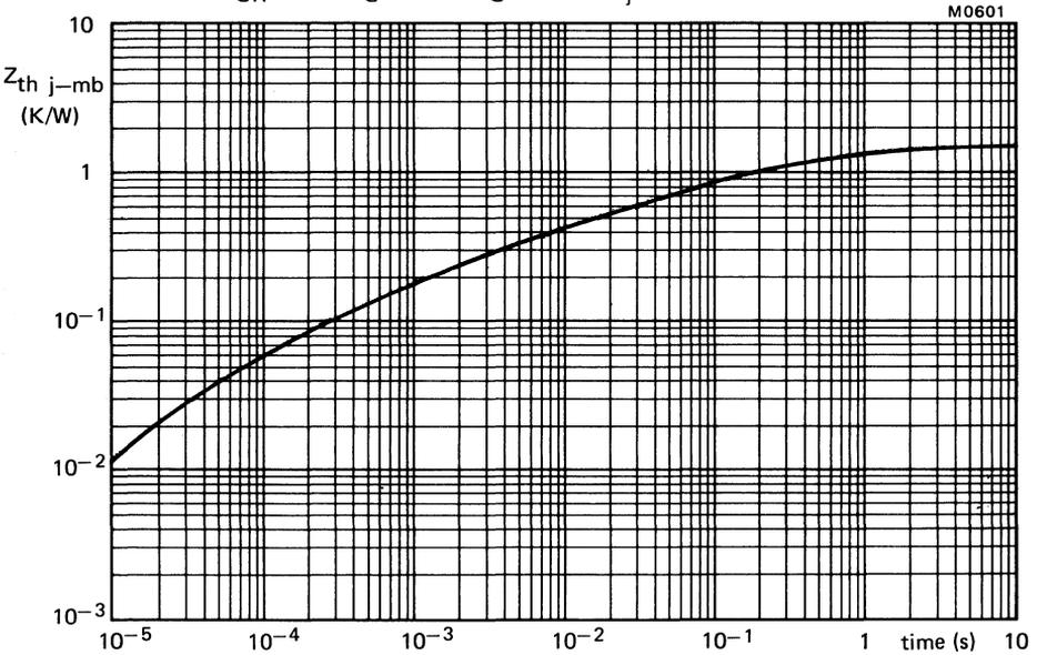
Fig.12 Transient thermal impedance.
