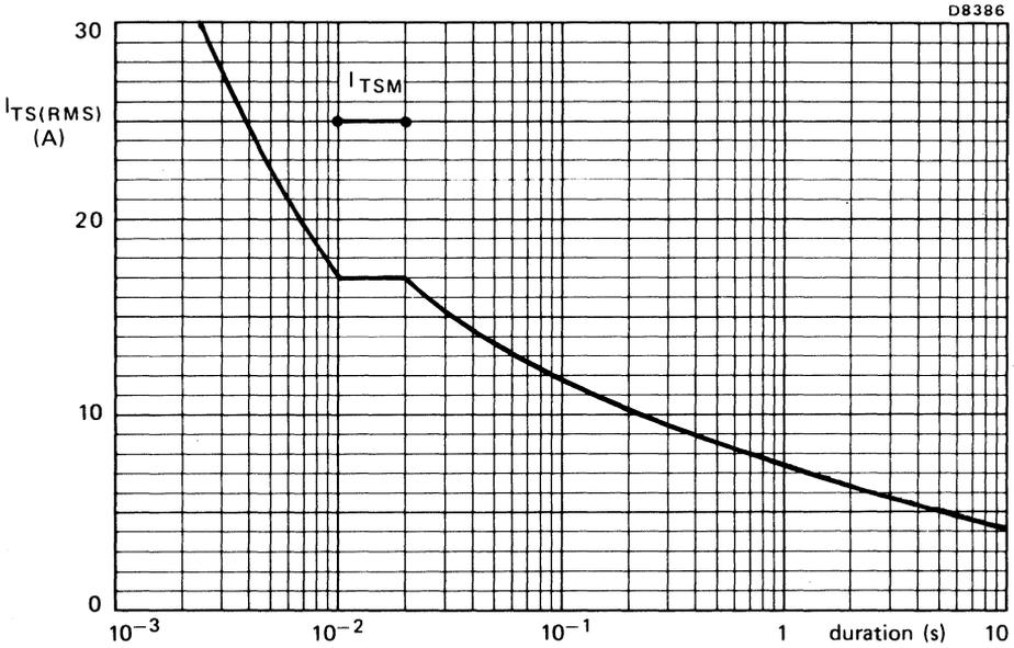
Fig.7 Maximum permissible non-repetitive r.m.s. on-state current based on sinusoidal currents ( $f = 50$  Hz);  $T_j = 120$  °C prior to surge. The triac may temporarily lose control following the surge.
