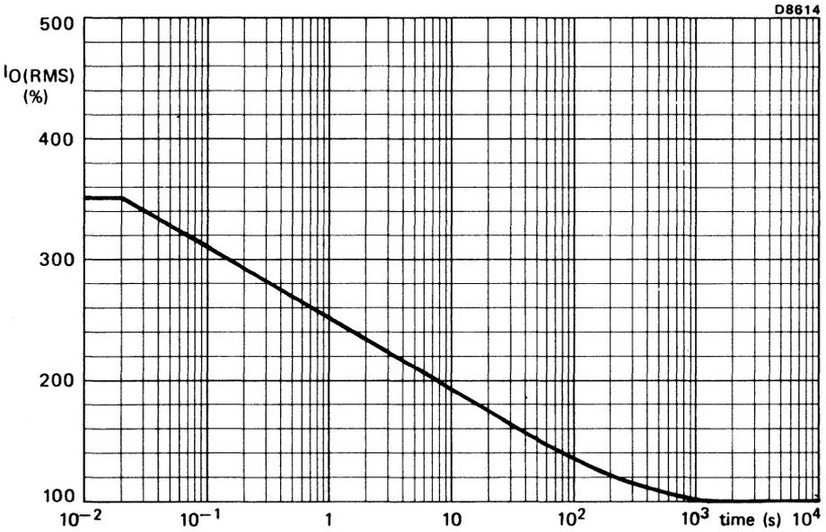
Fig.5 Maximum permissible duration of steady overload (provided that  $T_{mb}$  does not exceed  $120^{\circ}\text{C}$  during and after overload) expressed as a percentage of the steady state r.m.s. rated current. For high r.m.s. overload currents precautions should be taken so that the temperature of the terminals does not exceed  $125^{\circ}\text{C}$ . During these overload conditions the triac may lose control. Therefore the overload should be terminated by a separate protection device.
