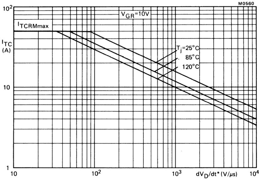
Fig.7 Anode current which can be turned off versus applied  $dV_D/dt^*$ ; inductive load;  $V_{GR} = 10 V$ ;  $L_G \leq 0.5 \mu H$ ;  $L_S \leq 0.25 \mu H$ . \* $dV_D/dt$  is calculated from  $I_T/C_S$ .
