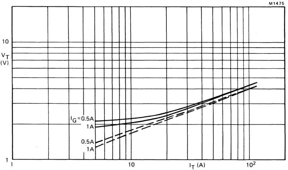
Fig.10 Maximum  $V_T$  versus  $I_T$ ; —  $T_j = 25^{\circ}C$ ; - - -  $T_j = 120^{\circ}C$ .
