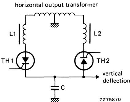
Fig. 8 Basic circuit of a vertical deflection system.
