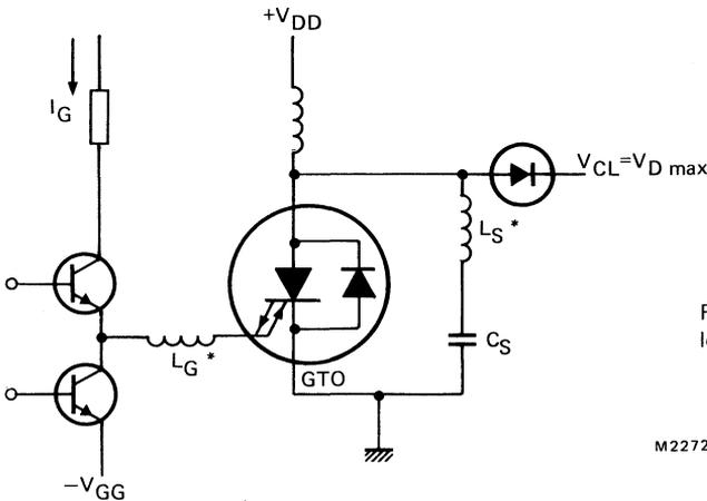
Fig.5 Inductive load test circuit.
