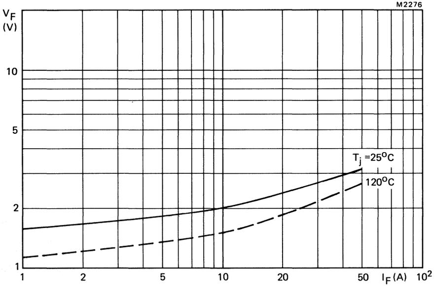
Fig.18 Forward voltage as a function of forward current; maximum values.
