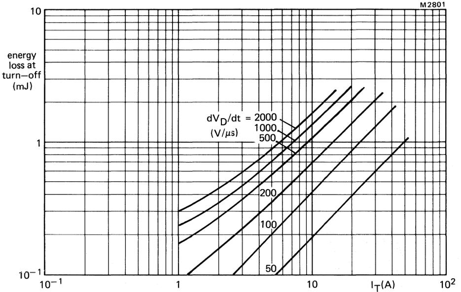
Fig.16 Maximum energy loss at turn-off (per cycle) as a function of anode current and applied  $dV_D/dt$  (calculated from  $I_T/C_S$ );  $dV_D/dt$  linear up to  $V_D = V_{DWmax}$ ;  $V_{GR} = 10$  V;  $I_G = 0.5$  A;  $L_G < 0.5$   $\mu$ H;  $L_S < 0.25$   $\mu$ H;  $T_j = 120$   $^{\circ}$ C.
