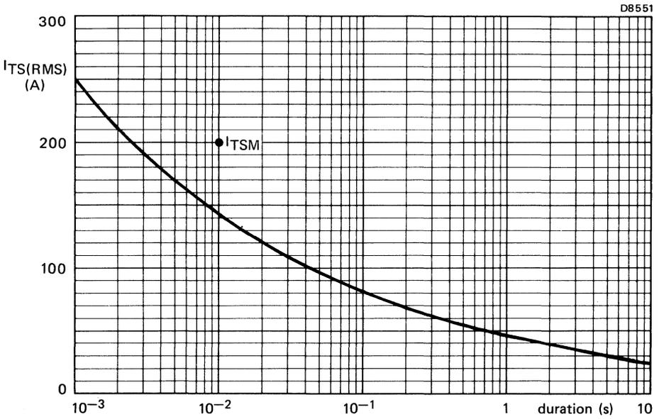
Fig.6 Maximum permissible non-repetitive r.m.s. on-state current based on sinusoidal currents ( $f = 50$  Hz);  $T_j = 115^\circ\text{C}$  prior to surge; with reapplied  $V_{RWMmax}$ .
