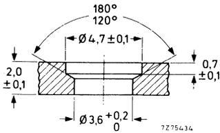
Fig. 10 Heatsink requirements for 500 V insulation.
