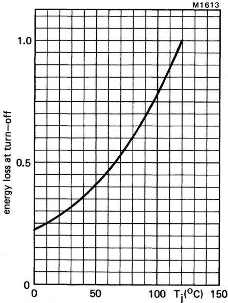
Fig.18 Energy loss at turn off as a function of junction temperature;  $I_G = 0.2$  A;  $V_{GR} = 10$  V. Normalised to  $T_j = 120$  °C.
