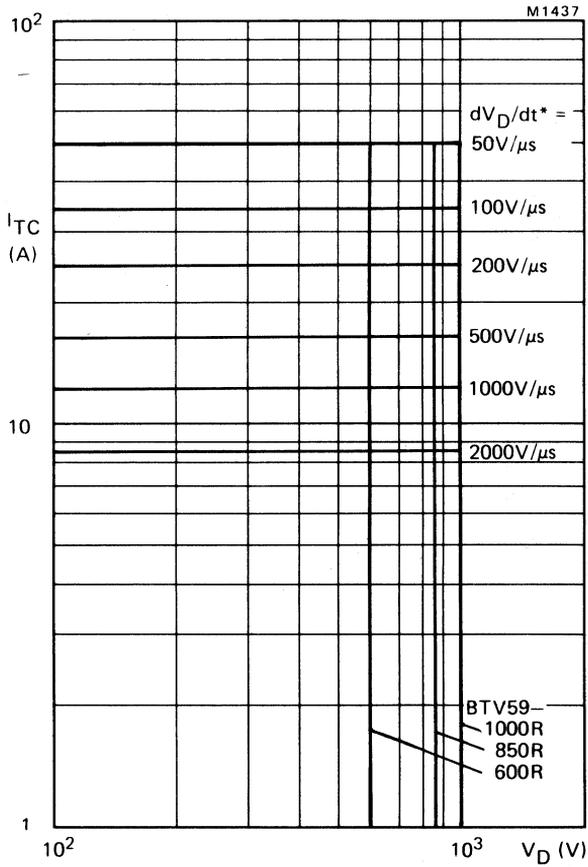
Fig. 6 Anode current which can be turned off versus anode voltage; inductive load;  $V_{GR} = 10$  V;  $L_G \leq 0.5 \mu H$ ;  $L_S \leq 0.25 \mu H$ ;  $T_j = 85^\circ C$ .
