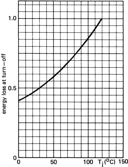
Fig.15 Energy loss at turn off as a function of junction temperature;  $I_G = 0.5$  A;  $V_{GR} = 10$  V. Normalised to  $T_j = 120$  °C.
