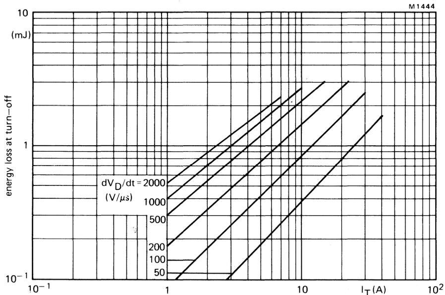
Fig.17 Maximum energy loss at turn-off (per cycle) as a function of anode current and applied  $dV_D/dt$  (calculated from  $I_T/C_S$ );  $dV_D/dt$  linear up to  $V_{Dmax} = 600$  V;  $V_{GR} = 10$  V;  $I_G = 0.5$  A;  $L_G \leq 0.5 \mu H$ ;  $L_S \leq 0.25 \mu H$ ;  $T_j = 120$  °C.
