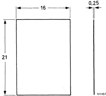
\*Because alumina is brittle, extreme care must be taken when mounting devices not to crack the alumina, particularly when used without heatsink compound.
