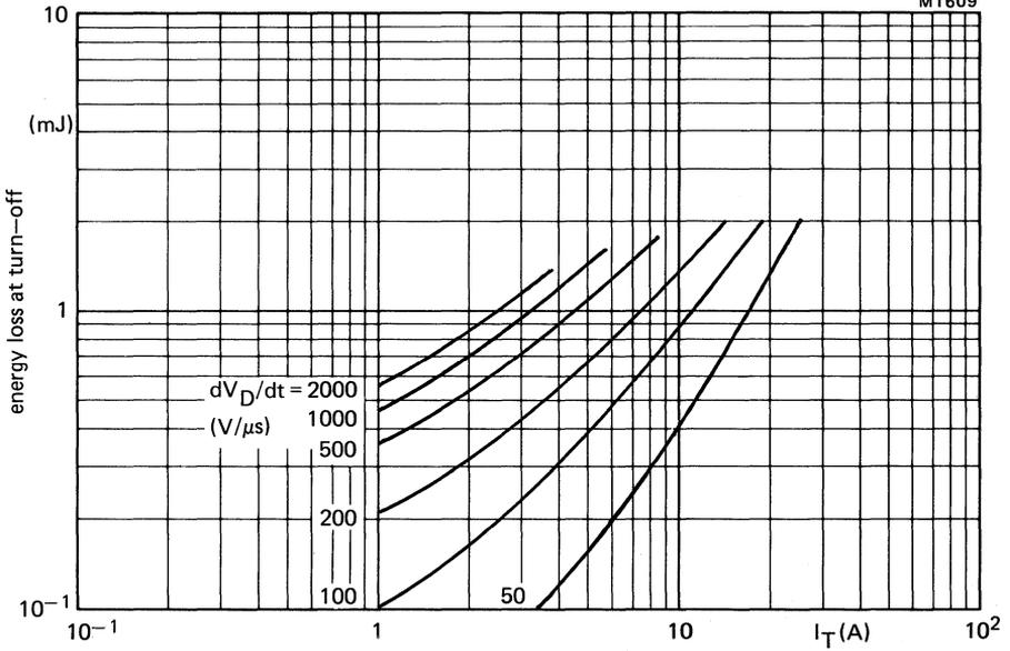
Fig.17 Maximum energy loss at turn-off (per cycle) as a function of anode current and applied  $dV_D/dt$  (calculated from  $I_T/C_S$ );  $dV_D/dt$  linear up to  $V_{Dmax} = 600$  V;  $V_{GR} = 10$  V;  $I_G = 0.2$  A;  $L_G \leq 1.0 \mu H$ ;  $L_S \leq 0.25 \mu H$ ;  $T_j = 120$  °C.
