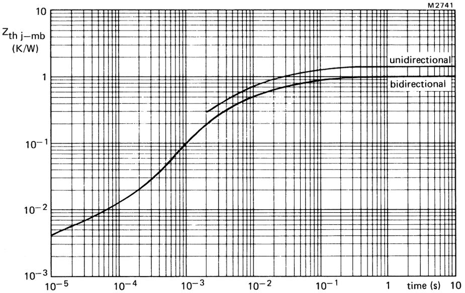
Fig.10 Transient thermal impedance.
