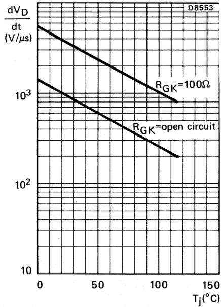
Fig. 9 Maximum rate of rise of off-state voltage that will not trigger any device as a function of junction temperature.
