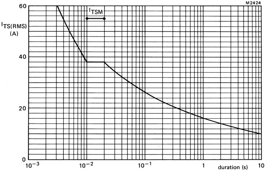
Fig.7 Maximum permissible non-repetitive r.m.s. on-state current based on sinusoidal currents ( $f = 50$  Hz);  $T_j = 120^\circ\text{C}$  prior to surge. The triac may temporarily lose control following the surge.
