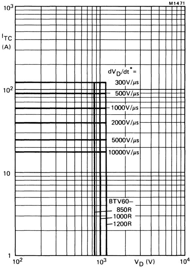
Fig.6 Anode current which can be turned off versus anode voltage; inductive load;  $V_{GR} = 10$  V;  $L_G \leq 0.5 \mu$ H;  $L_S \leq 0.25 \mu$ H;  $T_j = 120$  °C.
