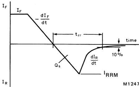
Fig.15 Definition of  $t_{rr}$  and  $Q_s$ .
