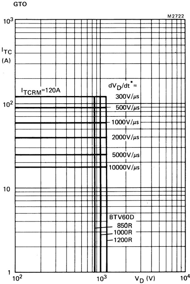
Fig.7 Anode current which can be turned off versus anode voltage; inductive load;  $V_{GR} = 10$  V;  $L_G \leq 0.5 \mu$ H;  $L_S \leq 0.25 \mu$ H;  $T_j = 120^\circ$ C.
