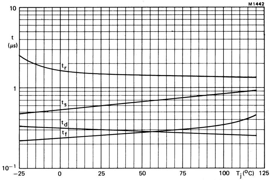
Fig.14 Switching times as a function of junction temperature;  $V_D \geq 250$  V;  $I_T = 10$  A;  $I_{GF} = 1.0$  A;  $V_{GR} = 10$  V;  $I_G = 0.5$  A;  $L_G = 0.4 \mu H$ ; maximum values.
