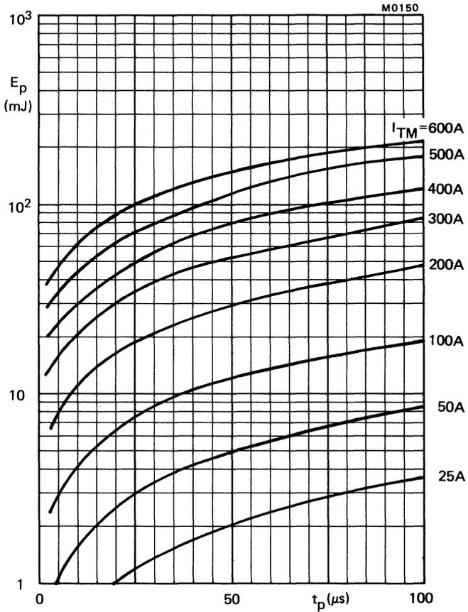
Fig.7 Maximum total energy loss per pulse when switching a half-sinusoidal pulse from 600 V.
