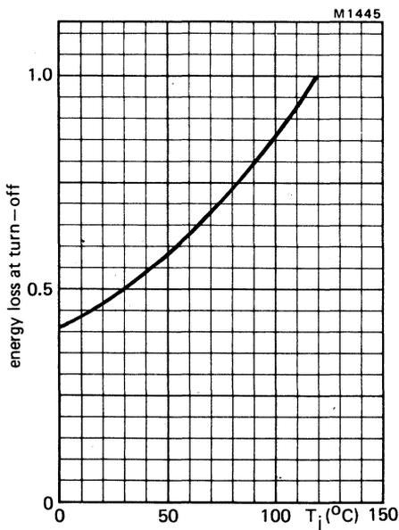
Fig.18 Energy loss at turn off as a function of junction temperature;  $I_G = 0.5$  A;  $V_{GR} = 10$  V. Normalised to  $T_j = 120$  °C.
