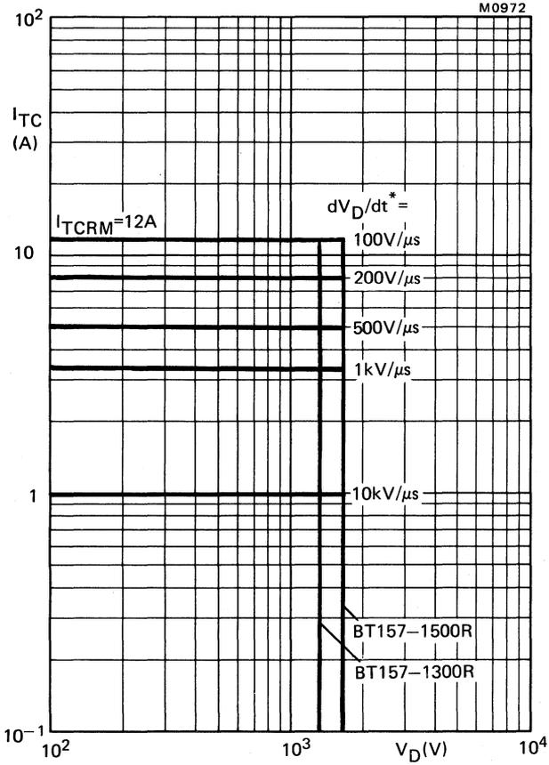
Fig.6 Anode current which can be turned off versus anode voltage; inductive load,  $V_{GR} = 10 V$ ;  $L_G \leq 1.5 \mu H$ ;  $L_S \leq 0.25 \mu H$ ;  $T_j = 85 \text{ }^\circ C$
