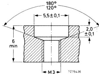
Fig. 14 Heatsink requirements for 1000 V insulation.
