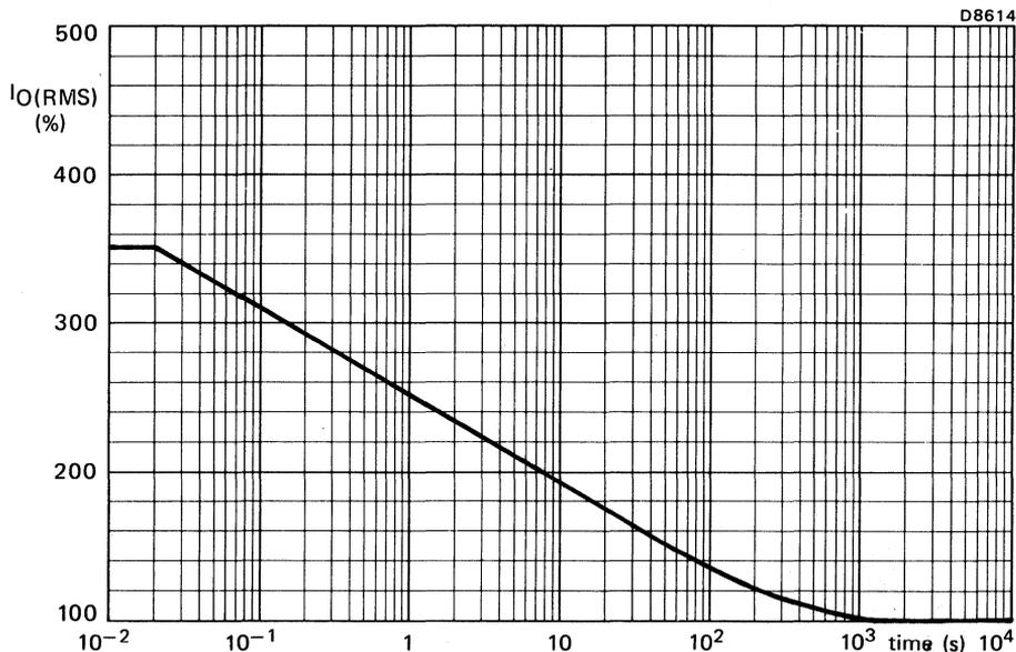
Fig.6 Maximum permissible duration of steady overload (provided that  $T_h$  does not exceed  $120^\circ\text{C}$  during and after overload) expressed as a percentage of the steady state r.m.s. rated current. For high r.m.s. overload currents precautions should be taken so that the temperature of the terminals does not exceed  $125^\circ\text{C}$ . During these overload conditions the triac may lose control. Therefore the overload should be terminated by a separate protection device.
