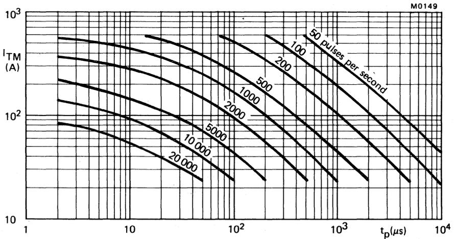
Fig.4 Maximum allowable peak on-state current versus pulse width;  $T_{mb} = 85 \text{ }^\circ\text{C}$ .
