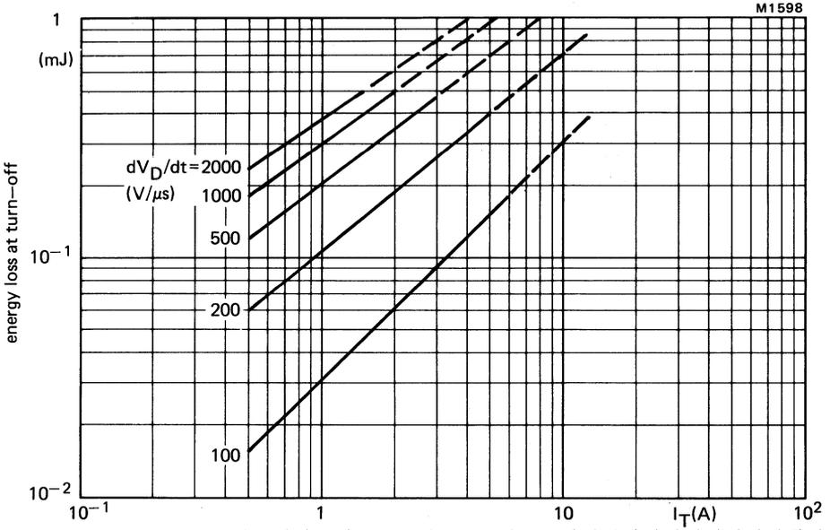
Fig.17 Maximum energy loss at turn-off (per cycle) as a function of anode current and applied  $dV_D/dt$  (calculated from  $I_T/C_S$ ); reapplied voltage sinusoidal up to  $V_{DRM} = 1200$  V;  $V_{GR} = 10$  V;  $I_G = 0.2$  A;  $L_G \leq 1.5 \mu$ H;  $L_S \leq 0.25 \mu$ H;  $T_j = 120$  °C.
