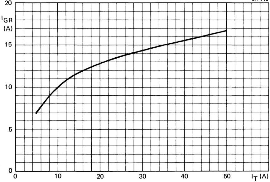
Fig.12 Peak reverse gate current versus anode current at turn-off; inductive load;  $V_{GR} = 10 \text{ V}$ ;  $I_G = 0.5 \text{ A}$ ;  $L_G = 0.4 \mu\text{H}$ ;  $T_j = 120 \text{ }^\circ\text{C}$ ; maximum values.
