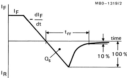
Fig.11 Definition of  $t_{rr}$  and  $Q_s$ .
