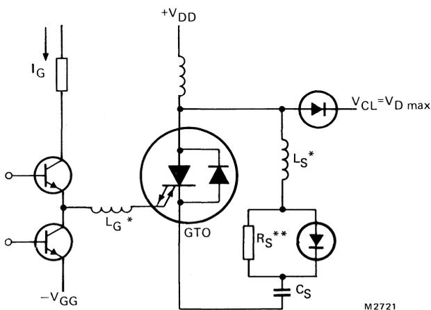
Fig.5 Inductive load test circuit.
