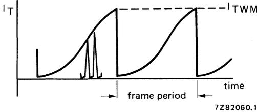
Fig. 7 Waveform defining  $I_{TWM}$ .
