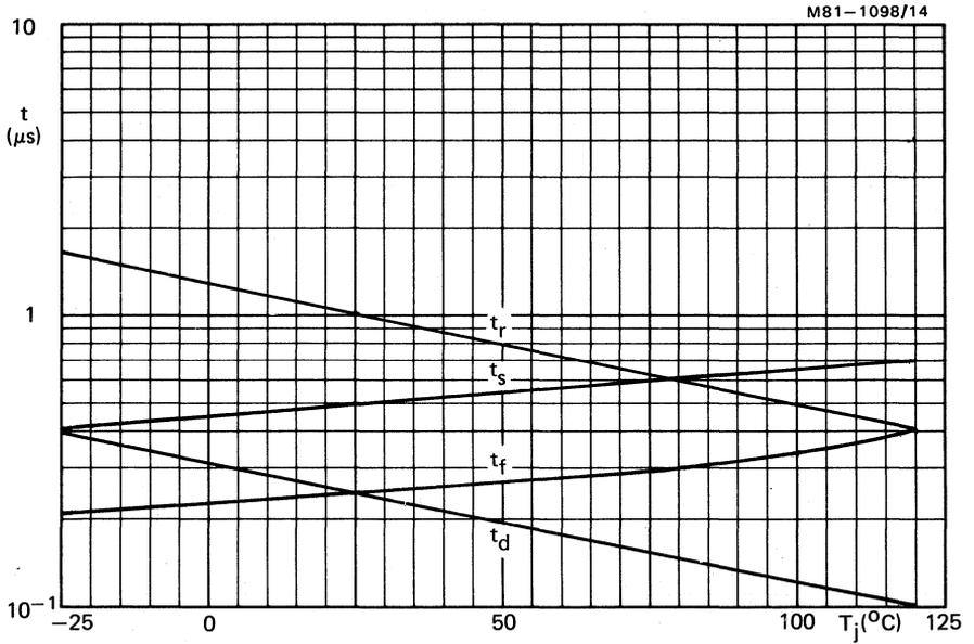
Fig.14 Switching times as a function of junction temperature;  $V_D \geq 250 \text{ V}$ ;  $I_T = 5 \text{ A}$ ;  $I_{GF} = 0.5 \text{ A}$ ;  $V_{GR} = 10 \text{ V}$ ;  $I_G = 0.2 \text{ A}$ ;  $L_G = 0.8 \mu\text{H}$ ; maximum values.
