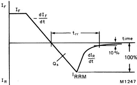
Fig.16 Definition of  $t_{rr}$  and  $Q_s$ .
