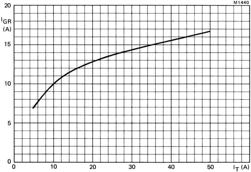
Fig.11 Peak reverse gate current versus anode current at turn-off; inductive load;
