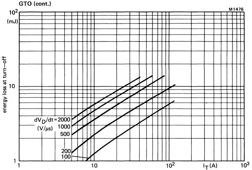
Fig.12 Maximum energy loss at turn-off (per cycle) as a function of anode current and applied  $dV_D/dt$  (calculated from  $I_T/C_S$ );  $dV_D/dt$  linear up to  $V_{Dmax} = 600$  V;  $V_{GR} = 10$  V;  $I_G = 0.5$  A;  $L_G \leq 0.5 \mu$ H;  $L_S \leq 0.25 \mu$ H;  $T_j = 120$  °C.
