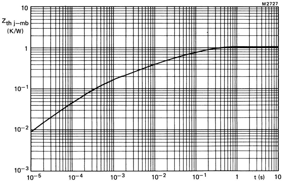
Fig.6 Transient thermal impedance.
