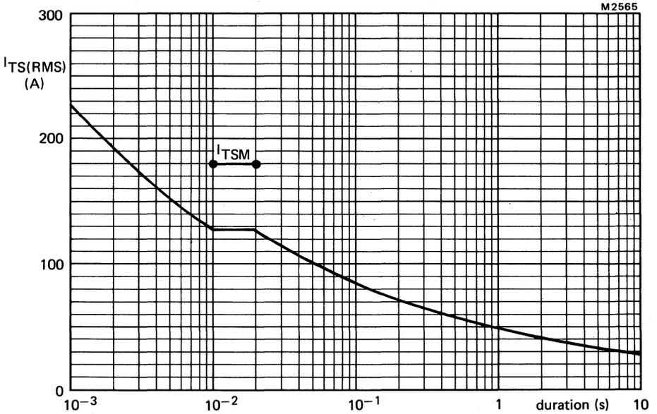
Fig.8 Maximum permissible non-repetitive r.m.s. on-state current based on sinusoidal currents ( $f = 50$  Hz;  $T_j = 120$  °C prior to surge. The triac may temporarily lose control following the surge.
