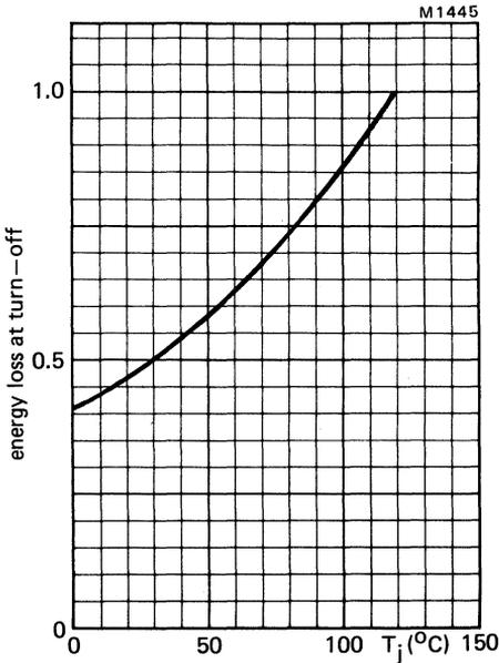
Fig.17 Energy loss at turn off as a function of junction temperature;  $I_G = 0.5$  A;  $V_{GR} = 10$  V. Normalised to  $T_j = 120$  °C.
