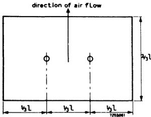
Fig. 3 Plain cooling fin with two diodes
