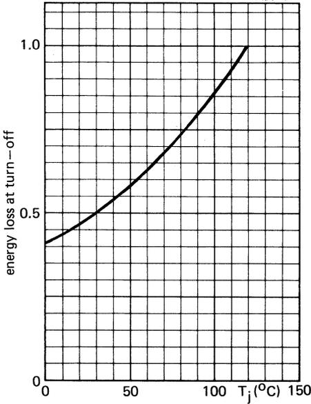
Fig.17 Energy loss at turn-off as a function of junction temperature;  $I_G = 0.5$  A;  $V_{GR} = 10$  V. Normalised to  $T_j = 120$  °C.
