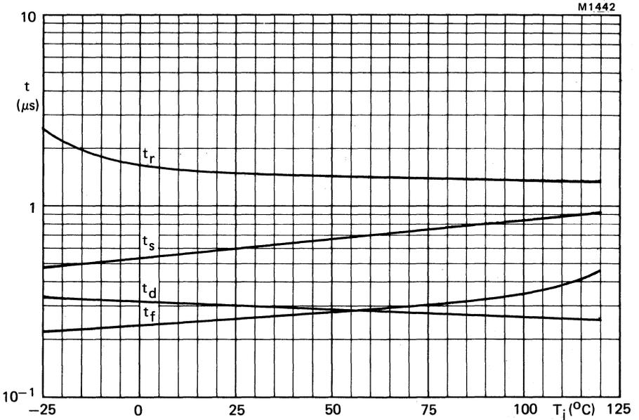
Fig.13 Switching times as a function of junction temperature;  $V_D \geq 250 \text{ V}$ ;  $i_T = 10 \text{ A}$ ;  $I_{GF} = 1.0 \text{ A}$ ;  $V_{GR} = 10 \text{ V}$ ;  $I_G = 0.5 \text{ A}$ ;  $L_G = 0.4 \mu\text{H}$ ; maximum values.
