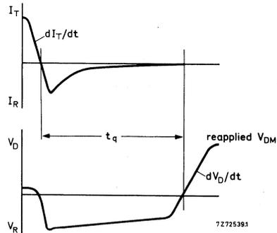
Fig.3b Circuit-commutated turn-off time definition.
