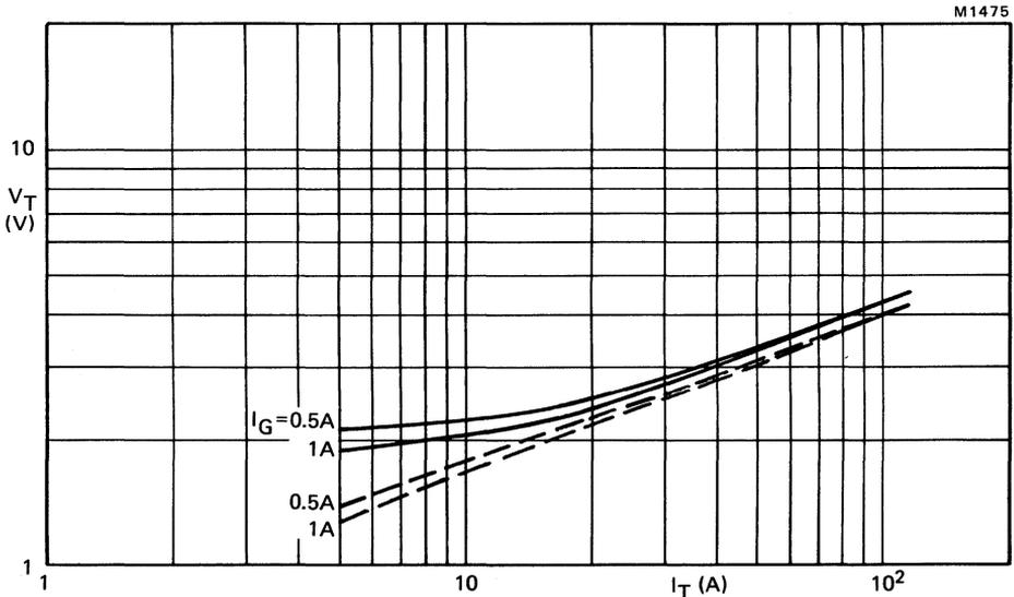
Fig.11 Maximum  $V_T$  versus  $I_T$ ; —  $T_j = 25$  °C; - - -  $T_j = 120$  °C.
