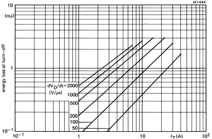
Fig.13 Maximum energy loss at turn-off (per cycle) as a function of anode current and applied  $dV_D/dt$  (calculated from  $I_T/C_S$ );  $dV_D/dt$  linear up to  $V_{Dmax} = 600$  V;  $V_{GR} = 10$  V;  $I_G = 0.5$  A;  $L_G \leq 0.5 \mu H$ ;  $L_S \leq 0.25 \mu H$ ;  $T_j = 120^\circ C$ .
