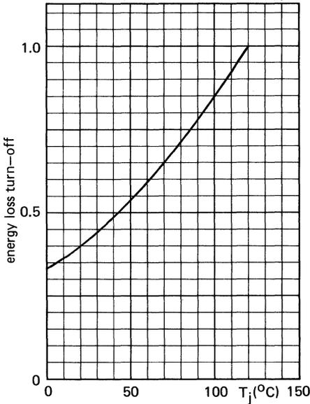
Fig.18 Energy loss at turn off as a function of junction temperature;  $I_G = 0.2$  A;  $V_{GR} = 10$  V. Normalised to  $T_j = 120$  °C.
