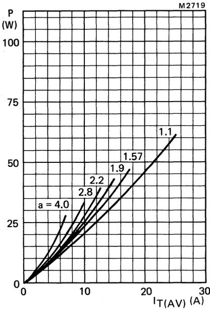
Fig.6 (a,b) Power dissipation as a function of average current (maximum values).
