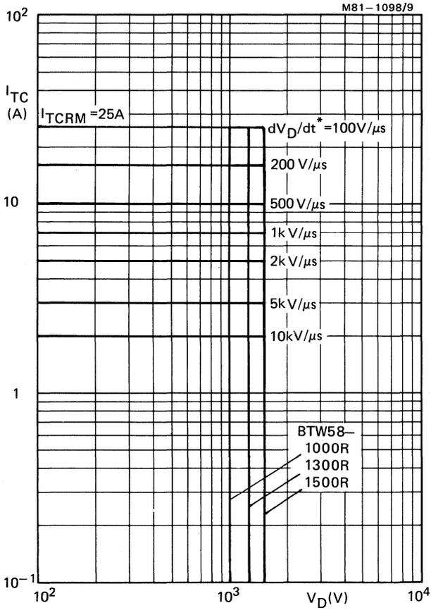
Fig.6 Anode current which can be turned off versus anode voltage; inductive load;  $V_{GR} = 10 V$ ;  $L_G \leq 1.0 \mu H$ ;  $L_S \leq 0.25 \mu H$ ;  $T_j = 85^\circ C$ .
