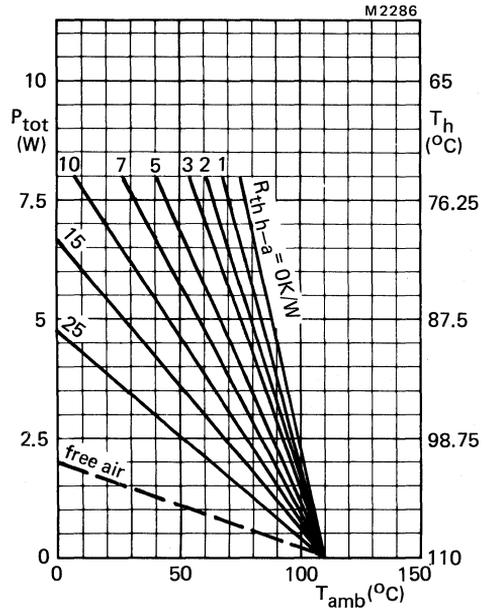
Fig.5c With heatsink compound.
