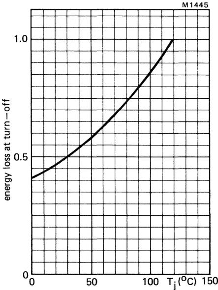
Fig.17 Energy loss at turn-off as a function of junction temperature;  $I_G = 0.5$  A;  $V_{GR} = 10$  V. Normalised to  $T_j = 120$   $^{\circ}$ C.
