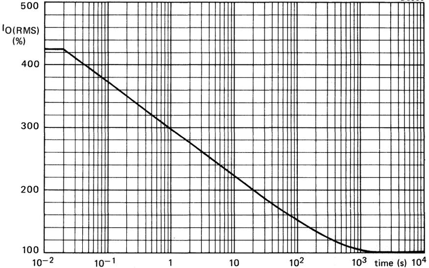
Fig.6 Maximum permissible duration of steady overload (provided that  $T_{mb}$  does not exceed  $120^\circ\text{C}$  during and after overload) expressed as a percentage of the steady state r.m.s. rated current. For high r.m.s. overload currents precautions should be taken so that the temperature of the terminals does not exceed  $125^\circ\text{C}$ . During these overload conditions the triac may lose control. Therefore the overload should be terminated by a separate protection device.
