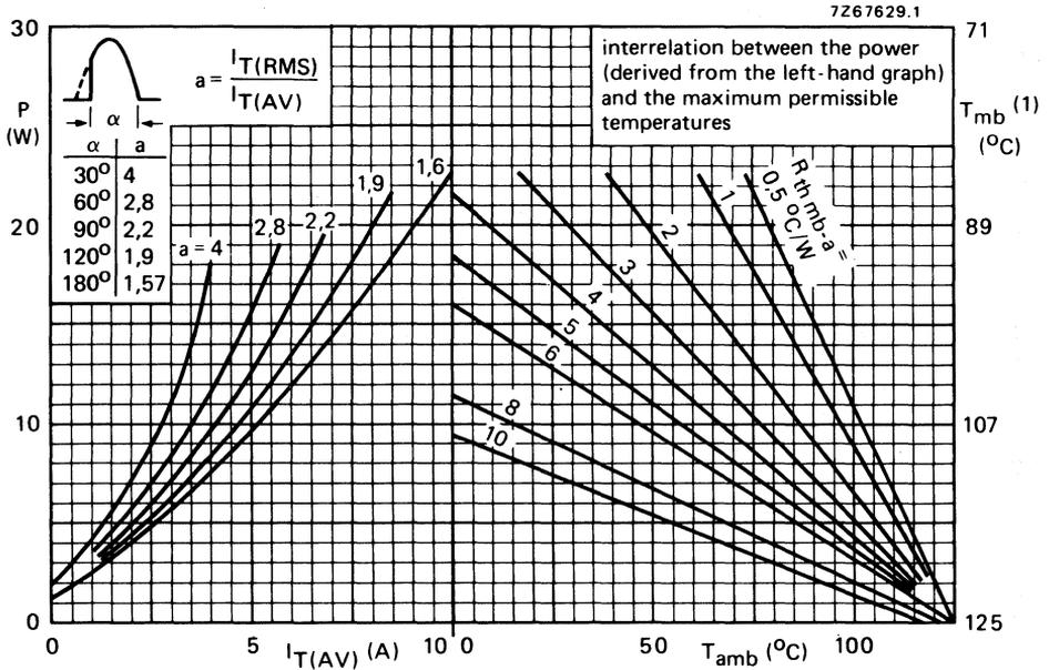
(1)  $T_{mb}$ -scale is for comparison purposes only and is correct only for  $R_{thmb-a} \leq 6 \text{ } ^\circ\text{C/W}$ .
