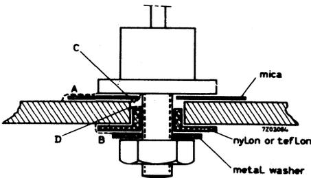
Fig. 2 Creepage distances with an insulated diode
