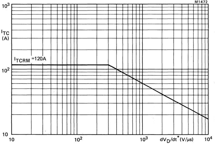
Fig.8 Anode current which can be turned off versus applied  $dV_D/dt^*$ ; inductive load;  $V_{GR} = 10$  V;  $L_G \leq 0.5 \mu H$ ;  $L_S \leq 0.25 \mu H$ ;  $T_j = 120$  °C.
