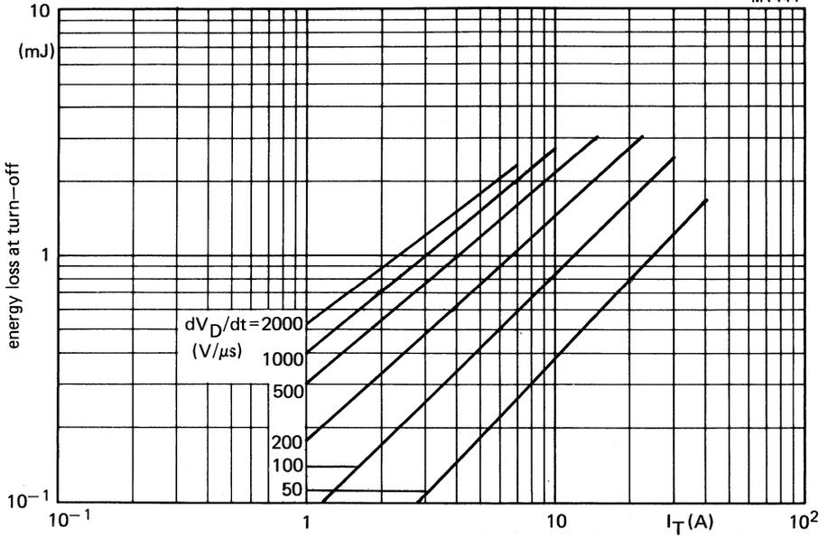
Fig.16 Maximum energy loss at turn-off (per cycle) as a function of anode current and applied  $dV_D/dt$  (calculated from  $I_T/C_S$ );  $dV_D/dt$  linear up to  $V_{Dmax} = 600$  V;  $V_{GR} = 10$  V;  $I_G = 0.5$  A;  $L_G \leq 0.5 \mu$ H;  $L_S \leq 0.25 \mu$ H;  $T_j = 120$  °C.
