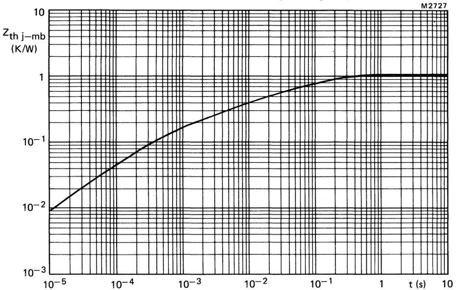
Fig.10 Transient thermal impedance.
