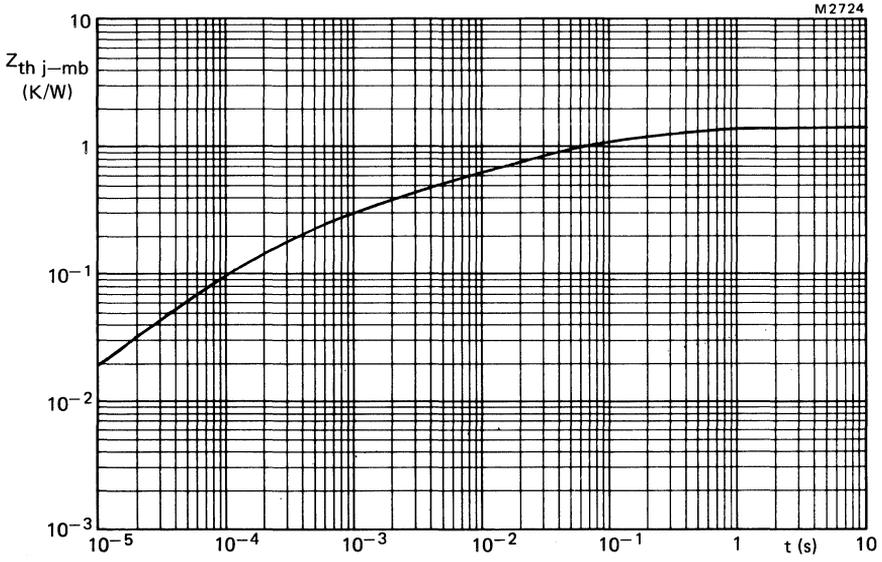
Fig.18 Transient thermal impedance.
