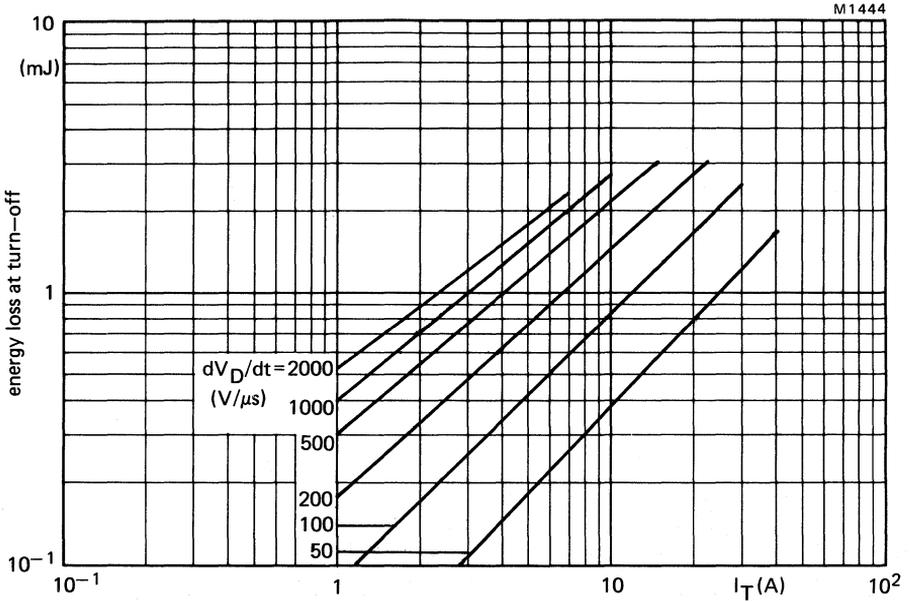
Fig.16 Maximum energy loss at turn-off (per cycle) as a function of anode current and applied  $dV_D/dt$  (calculated from  $I_T/C_S$ );  $dV_D/dt$  linear up to  $V_{Dmax} = 600$  V;  $V_{GR} = 10$  V;  $I_G = 0.5$  A;  $L_G \leq 0.5 \mu$ H;  $L_S \leq 0.25 \mu$ H;  $T_j = 120$  °C.
