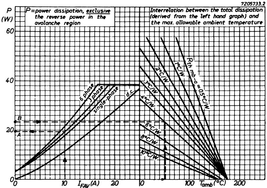
From the lefthand graph it follows that  $P_{tot} = 19,5\text{ W}$  per diode (point A). The average reverse power in the avalanche region, averaged over any cycle, follows from
