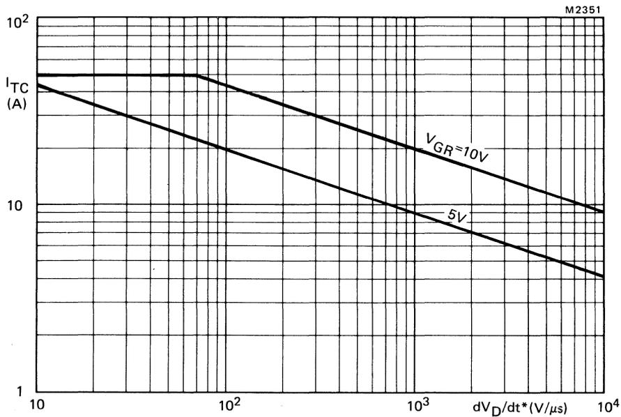
Fig.7 Anode current which can be turned off versus applied  $dV_D/dt^*$ ; inductive load;
