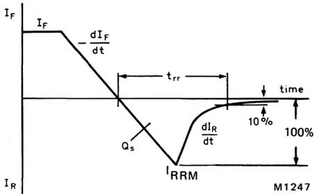
Fig.14 Definition of  $t_{rr}$  and  $Q_s$ .
