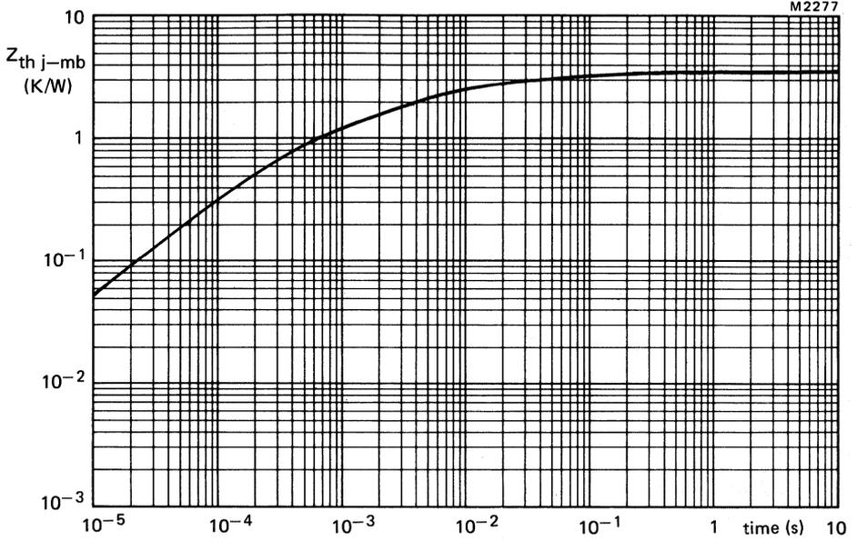
Fig.21 Transient thermal impedance.
