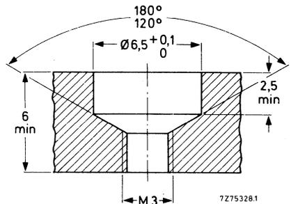
Fig. 7 Heatsink requirements
