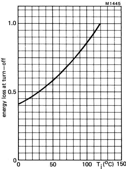
Fig.14 Energy loss at turn off as a function of junction temperature;  $I_G = 0.5$  A;  $V_{GR} = 10$  V. Normalised to  $T_j = 120^\circ C$ .
