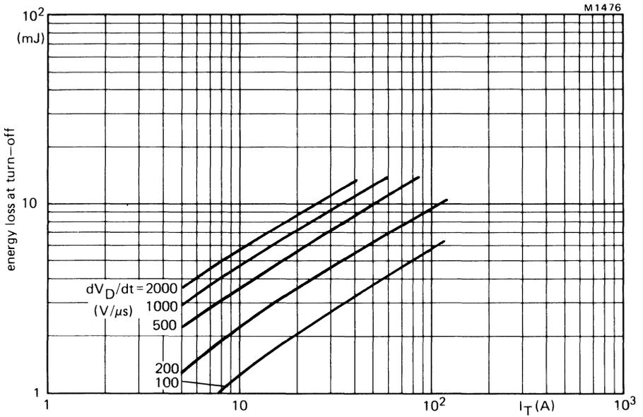
Fig.11 Maximum energy loss at turn-off (per cycle) as a function of anode current and applied  $dV_D/dt$  (calculated from  $I_T/C_S$ );  $dV_D/dt$  linear up to  $V_{Dmax} = 600$  V;  $V_{GR} = 10$  V;  $I_G = 0.5$  A;  $L_G \leq 0.5 \mu H$ ;  $L_S \leq 0.25 \mu H$ ;  $T_j = 120$  °C.
