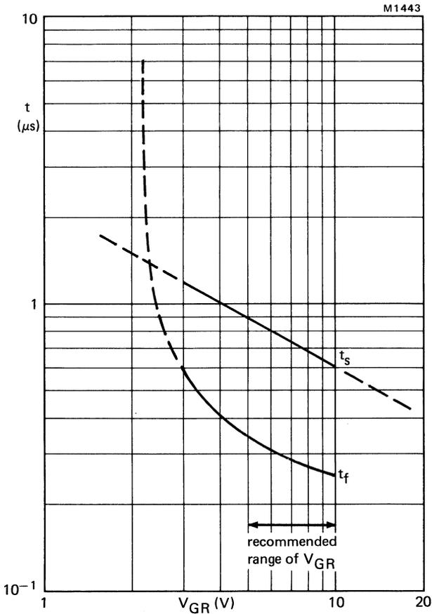
Fig.15 Storage and fall times versus applied reverse gate voltage; inductive load;
