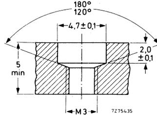
Fig. 13 Heatsink requirements for 500 V insulation.
