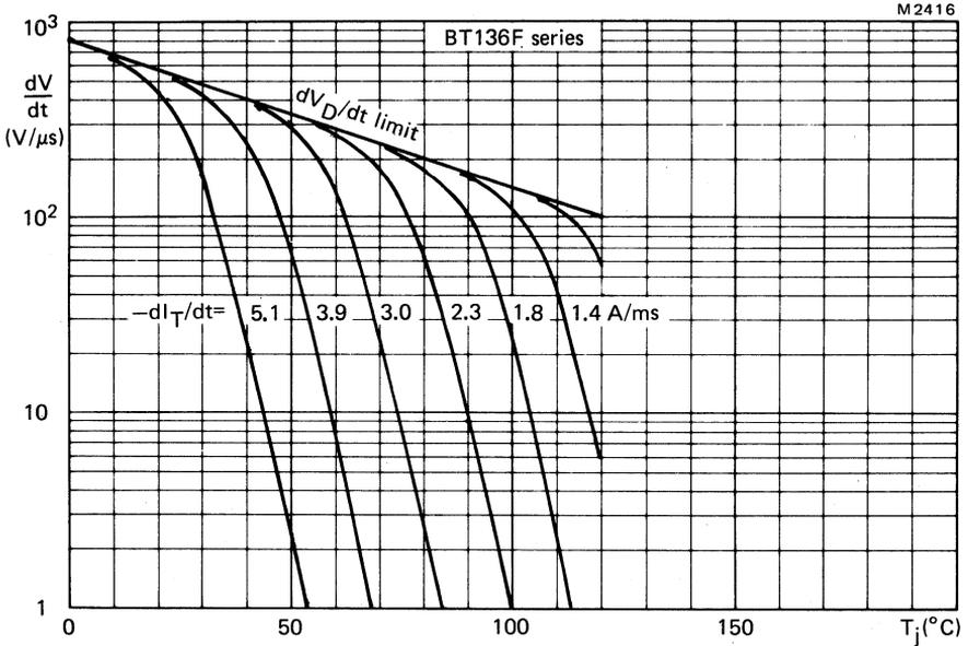
Fig.9 Typical commutation  $dV/dt$  for BT136F series versus  $T_j$ . The triac should commute when the  $dV/dt$  is below the value on the appropriate curve for pre-commutation  $dI_T/dt$ .
