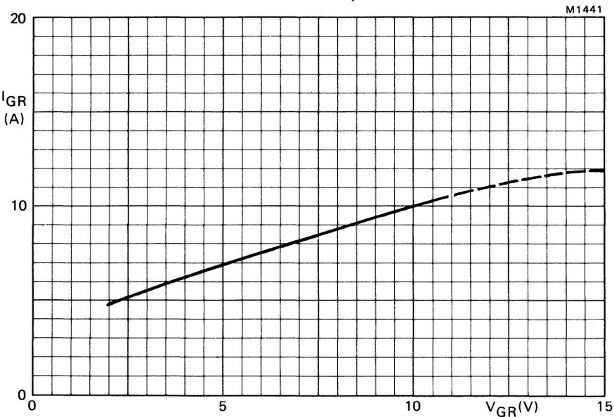
Fig.12 Peak reverse gate current versus applied reverse gate voltage; inductive load;
