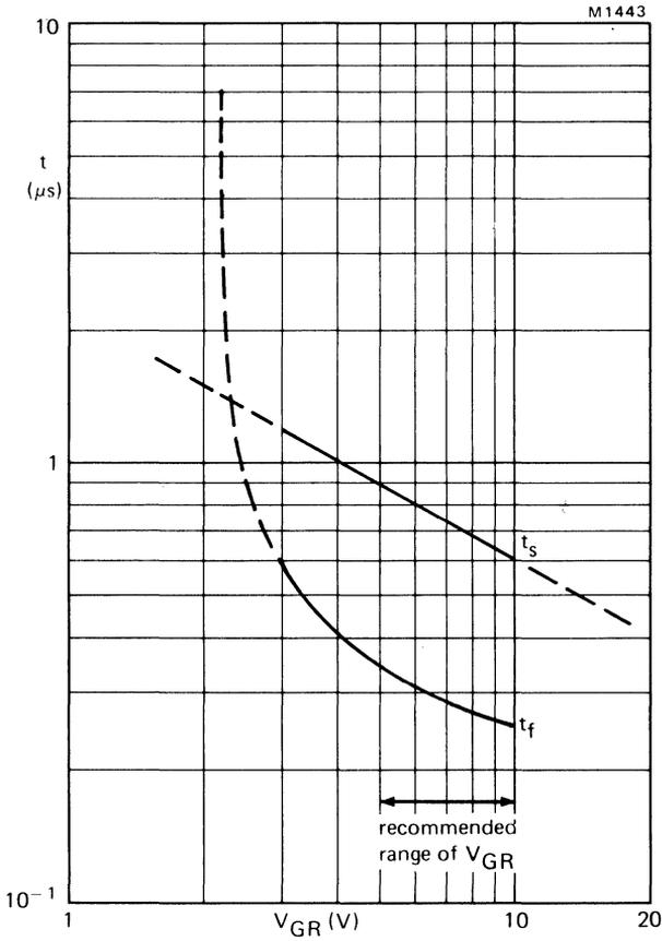
Fig.16 Storage and fall times versus applied reverse gate voltage; inductive load;  $I_T = 10$  A;  $I_G = 0.5$  A;  $L_G = 0.4 \mu H$ ;  $T_j = 25$  °C; maximum values.
