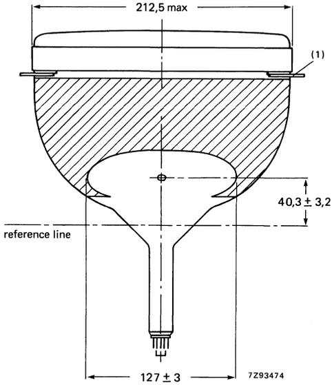
(1) The displacement of any lug with respect to the plane through the other three lugs is max. 2 mm.
