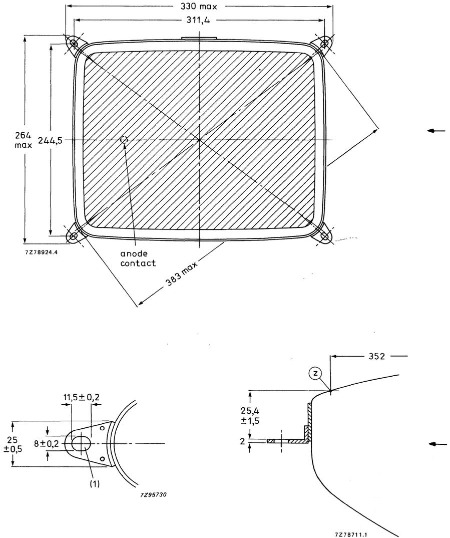
(1) The mounting screws in the cabinet must be situated inside a circle of 5 mm diameter drawn around the true geometrical positions i.e. at the corners of a rectangle of 311,4 mm x 244,5 mm.
