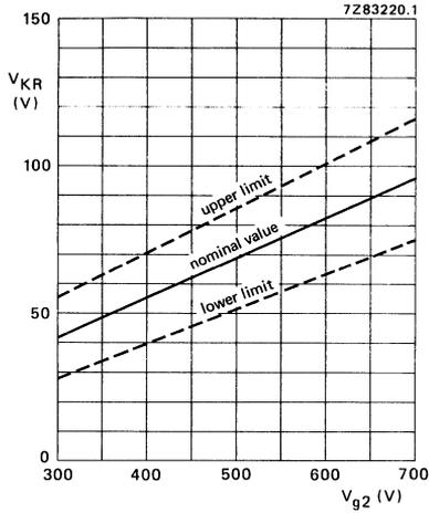
Limits of cathode raster cut-off voltage as a function of grid 2 voltage.
