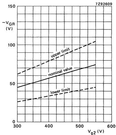
Limits of grid 1 cut-off voltage as a function of grid 2 voltage.
