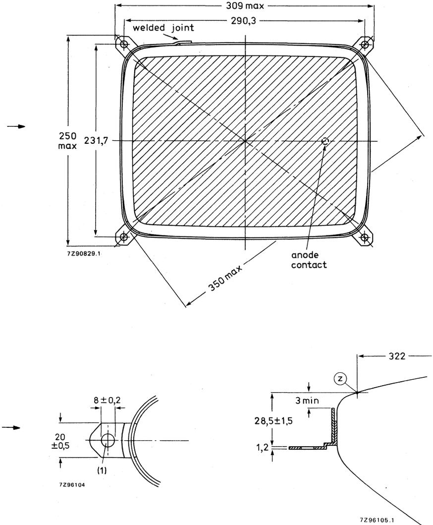
(1) The mounting screws in the cabinet must be situated inside a circle of 4 mm diameter drawn around the true geometrical positions i.e. at the corners of a rectangle of 290,3 mm x 231,7 mm.
