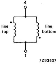
Fig. 2a Line coils.
