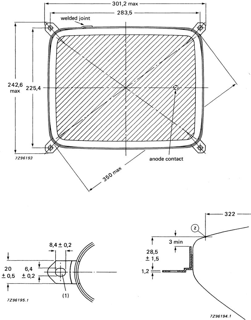
(1) The mounting screws in the cabinet must be situated inside a circle of 4 mm diameter drawn around the true geometrical positions i.e. at the corners of a rectangle of 283,5 mm x 225,4 mm.
