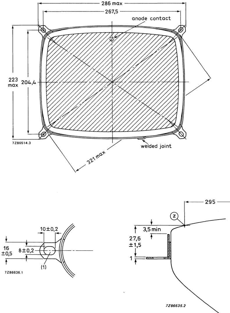
(1) The mounting screws in the cabinet must be situated inside a circle of 5 mm diameter drawn around the true geometrical positions i.e. at the corners of a rectangle of 267,5 mm x 204,4 mm.
