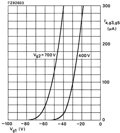
Anode current as a function of grid 1 voltage.
