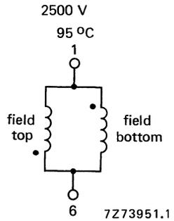
Fig. 2b Field coils, AT1040/04.
