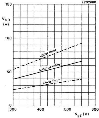
Limits of cathode cut-off voltage as a function of grid 2 voltage.
