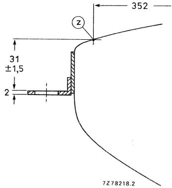
(1) The mounting screws in the cabinet must be situated inside a circle of 8 mm diameter drawn around the true geometrical positions i.e. at the corners of a rectangle of 327 mm x 247,7 mm.
