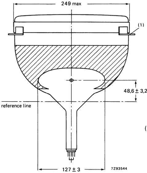
(1) The displacement of any lug with respect to the plane through the other three lugs is max. 1,5 mm.
