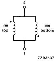
Fig. 2a Line coils.
