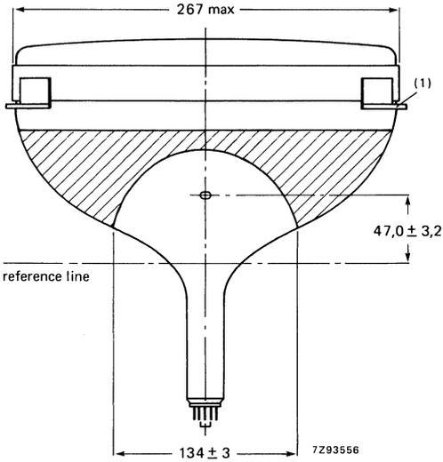
(1) The displacement of any lug with respect to the plane through the other three lugs is max. 1,5 mm.
