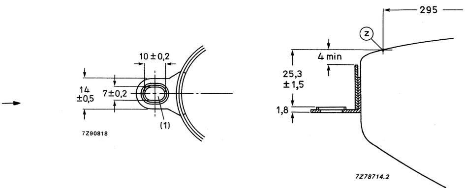
(1) The mounting screws in the cabinet must be situated inside a circle of 4 mm diameter drawn around the true geometrical positions i.e. at the corners of a rectangle of 273,3 mm x 190,2 mm.
