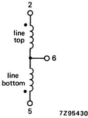
Fig. 2a Line coils.
