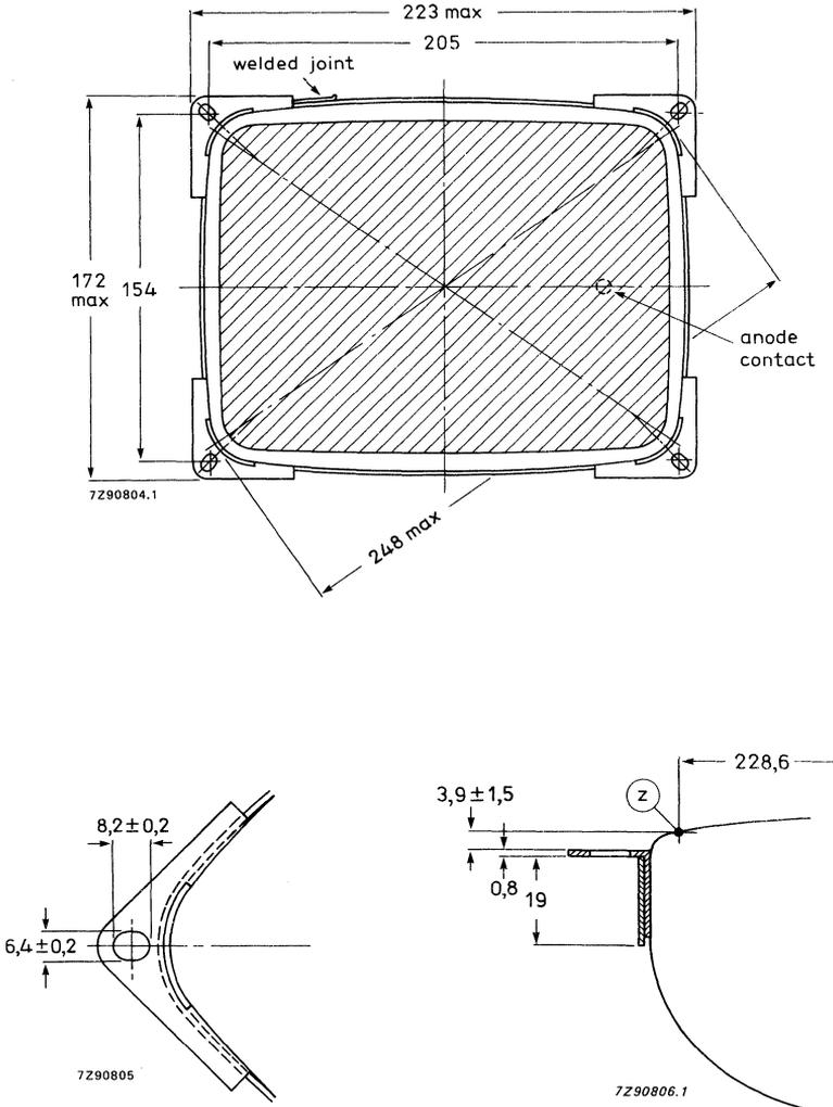
(1) The position of the mounting screws in the cabinet must be within a circle of 3,4 mm diameter drawn around the true geometrical positions, i.e. the corners of a rectangle of 205 mm x 154 mm.
