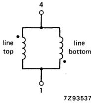
Fig. 2a Line coils.
