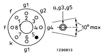
(1) The displacement of any lug with respect to the plane through the three other lugs is max. 1,5 mm.
