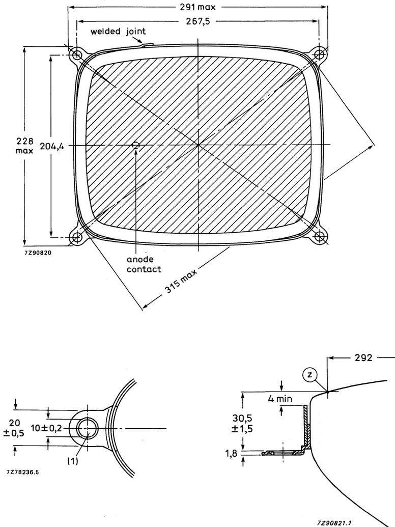
(1) The position of the mounting screws in the cabinet must be within a circle of 7 mm diameter drawn around the true geometrical positions, i.e. corners of a rectangle of 267,5 mm x 204,4 mm.
