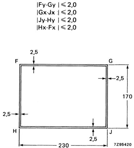
Fig. 4 The edges of the displayed raster fall within the two rectangles.
