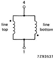
Fig. 2a Line coils.
