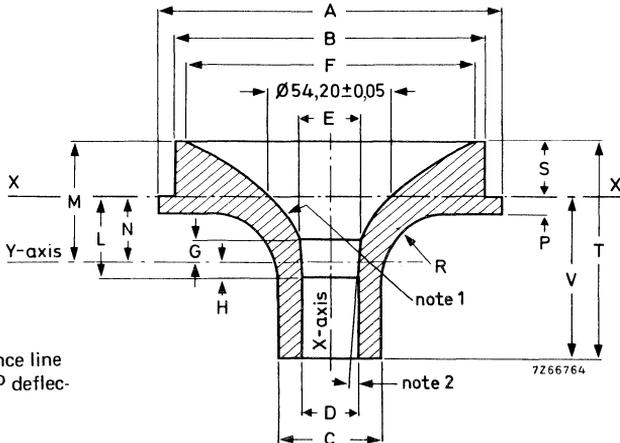
Fig. 1 Reference line gauge for  $110^\circ$  deflection angle.
