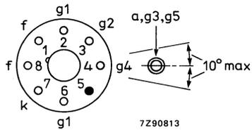
(1) The displacement of any lug with respect to the plane through the three other lugs is max. 1,5 mm.
