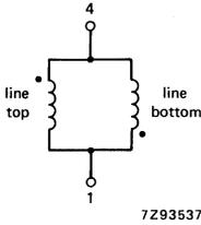
Fig. 2a Line coils.
