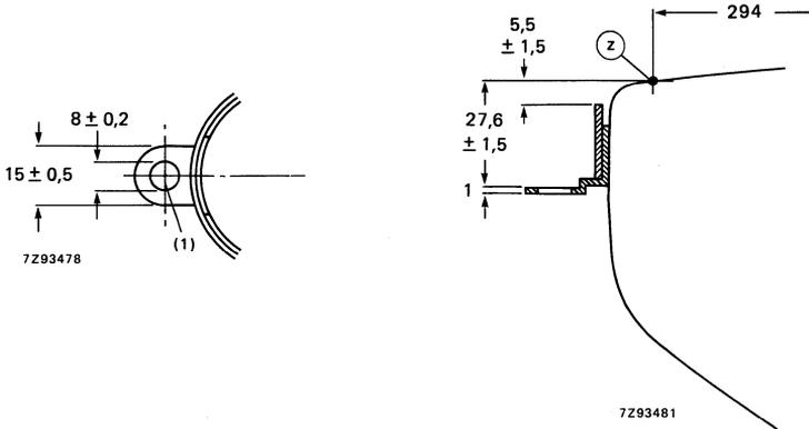
(1) The mounting screws in the cabinet must be situated inside a circle of 5 mm diameter drawn around the true geometrical positions i.e. at the corners of a rectangle of 273,3 mm x 190,2 mm
