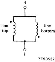
Fig. 2a Line coils.
