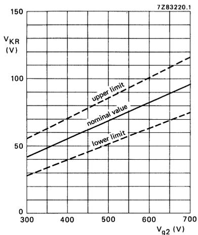
Limits of cathode raster cut-off voltage as a function of grid 2 voltage.
