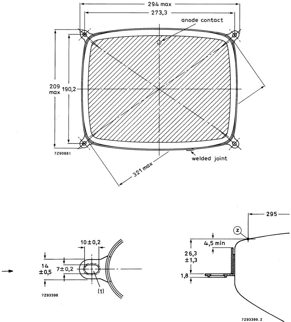
(1) The mounting screws in the cabinet must be situated inside a circle of 4 mm diameter drawn around the true geometrical positions i.e. at the corners of a rectangle of 273,3 mm x 190,2 mm.
