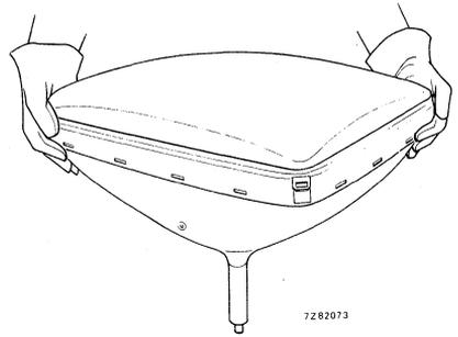
Fig. 3 Lifting picture tube from face-down position.
