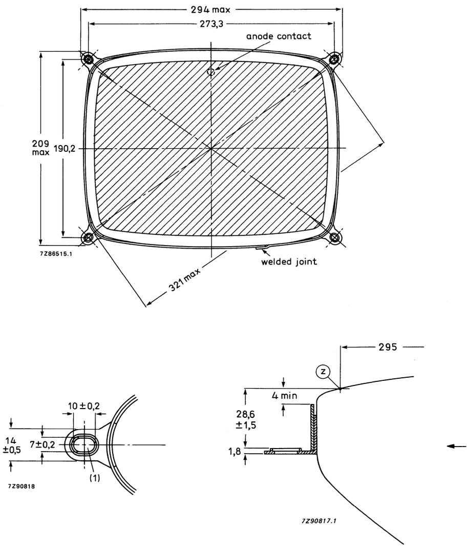
(1) The mounting screws in the cabinet must be situated inside a circle of 4 mm diameter drawn around the true geometrical positions i.e. at the corners of a rectangle of 273,3 mm x 190,2 mm.
