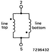
Fig. 2a Line coils.
