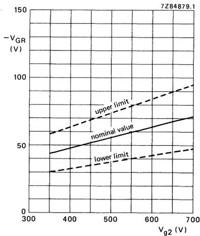
Limits of grid 1 raster cut-off voltage as a function of grid 2 voltage.
