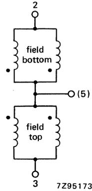
Fig. 2b Field coils.
