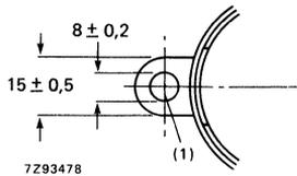
(1) The mounting screws in the cabinet must be situated inside a circle of 5 mm diameter drawn around the true geometrical positions i.e. at the corners of a rectangle of 273,3 mm x 190,2 mm.
