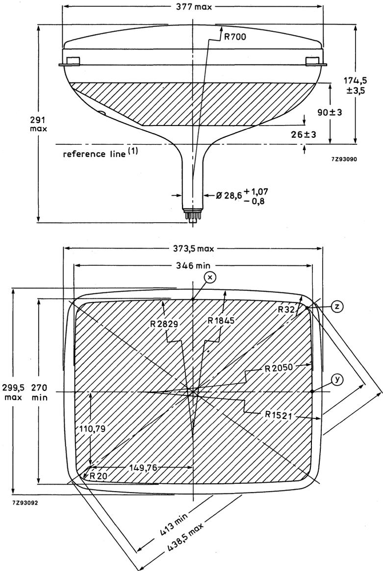
(1) The reference line is determined by the plane of the upper edge of reference line gauge C when the gauge is resting on the cone.
