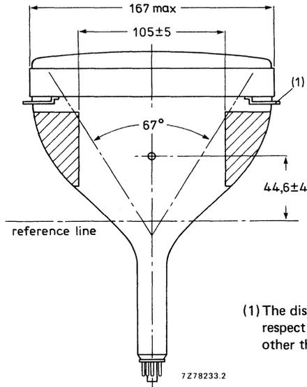
(1) The displacement of any lug with respect to the plane through the other three lugs is max. 1,8 mm.
