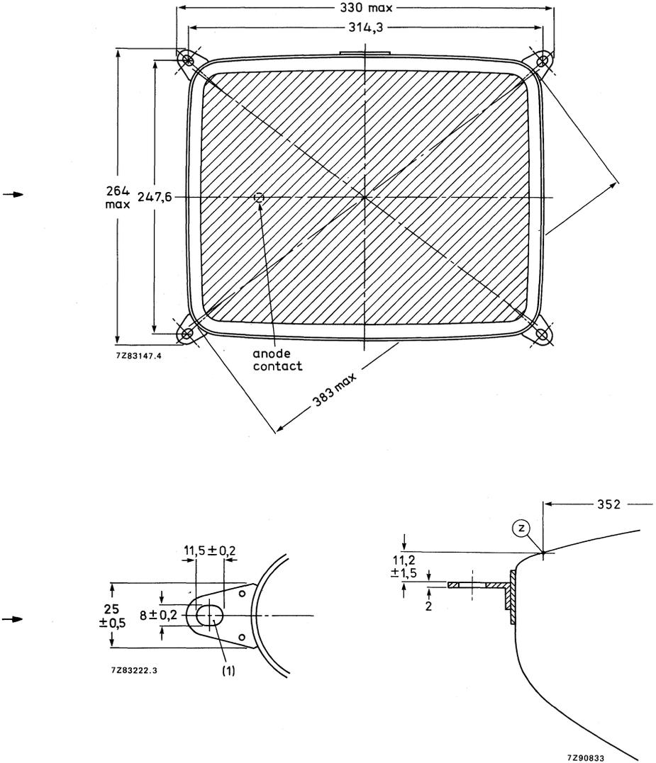
(1) The mounting screws in the cabinet must be situated inside a circle of 5 mm diameter drawn around the true geometrical positions i.e. at the corners of a rectangle of 314,3 mm x 247,6 mm.
