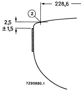
Front view and lug dimensions of tube M24-512W
