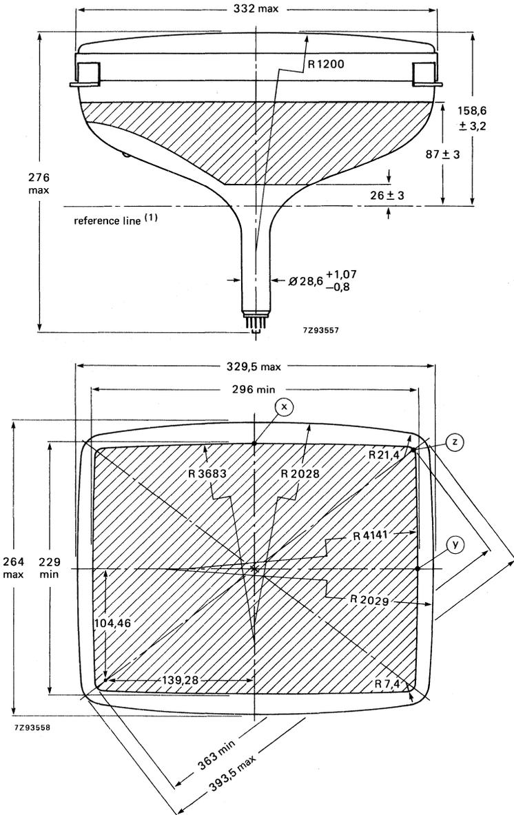
(1) The reference line is determined by the plane of the upper edge of reference line gauge C when the gauge is resting on the cone.
