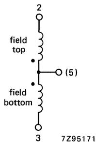
Fig. 2b Field coils.
