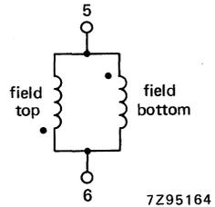
Fig. 3b Field coils, AT1040/17.
