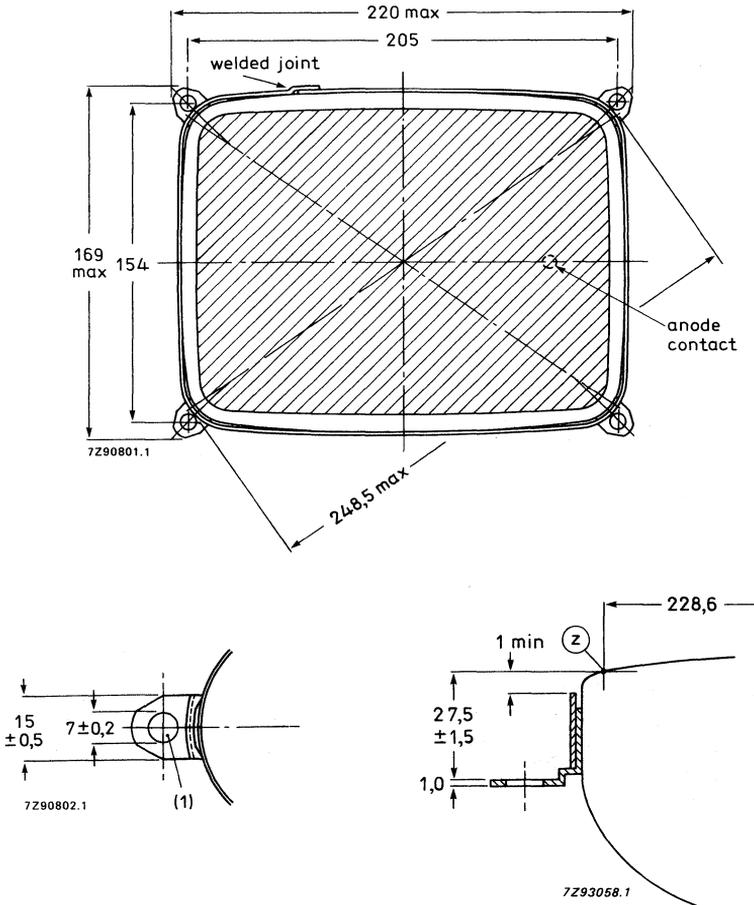
(1) The position of the mounting screws in the cabinet must be within a circle of 4 mm diameter drawn around the true geometrical positions, i.e. the corners of a rectangle of 205 mm x 154 mm.
