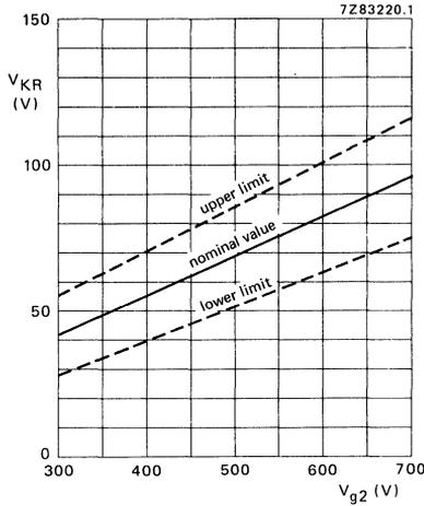
Limits of cathode cut-off voltage as a function of grid 2 voltage. Cathode drive;  $V_{a,g3,g5} = 17$  kV.
