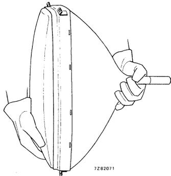
Fig. 2 Lifting picture tube from edge-down position.
