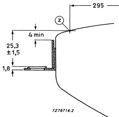
(1) The mounting screws in the cabinet must be situated inside a circle of 4 mm diameter drawn around the true geometrical positions i.e. at the corners of a rectangle of 273,3 mm x 190,2 mm.
