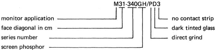
In the **new system**, used for type numbers M29EAA, M32EAA, etc., surface treatment and type of screen glass are identified as shown in the example below.
