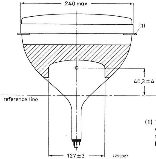
(1) The displacement of any lug with respect to the plane through the other three lugs is max. 2 mm.
