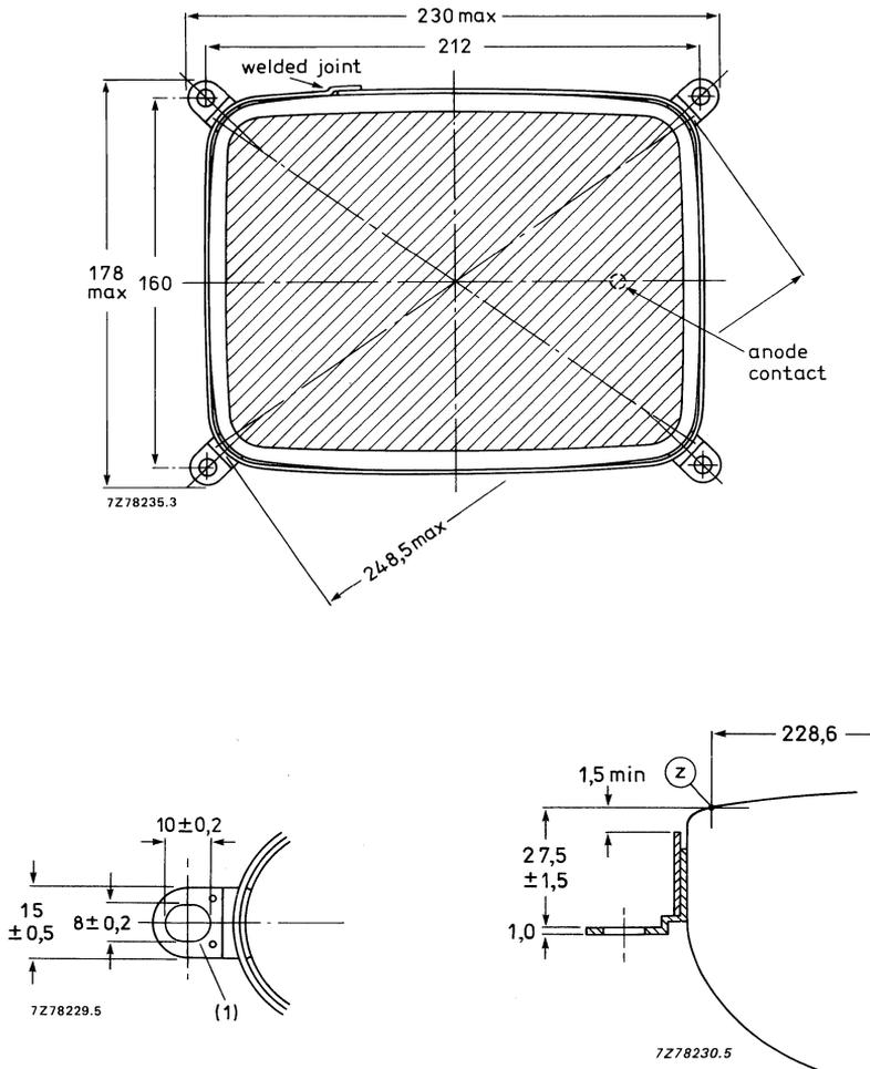
(1) The position of the mounting screws in the cabinet must be within a circle of 5 mm diameter drawn around the true geometrical positions, i.e. the corners of a rectangle of 212 mm x 160 mm.
