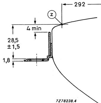
(1) The position of the mounting screws in the cabinet must be within a circle of 7 mm diameter drawn around the true geometrical positions, i.e. the corners of a rectangle of 273,3 mm x 190,2 mm.
