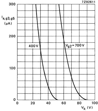
Anode current as a function of cathode voltage.
