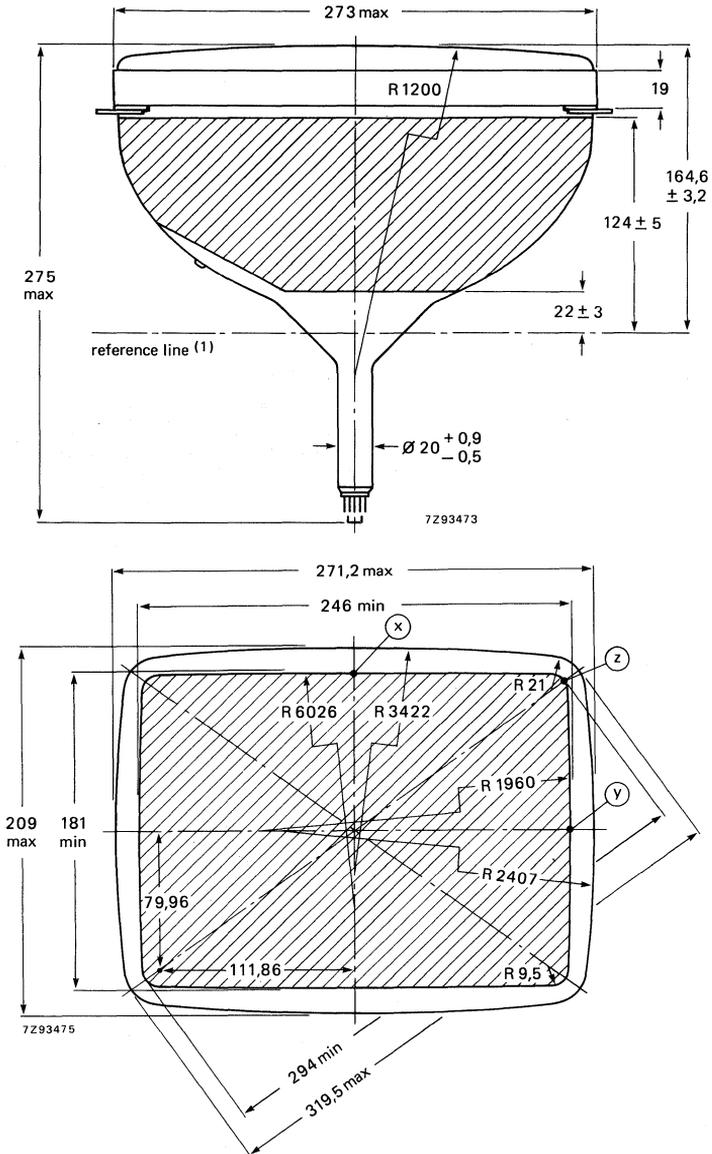
(1) The reference line is determined by the plane of the upper edge of reference line gauge D when the gauge is resting on the cone.
