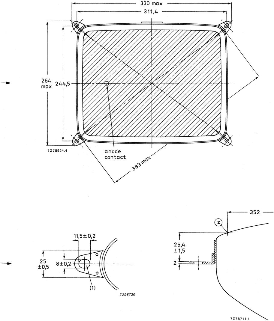
(1) The mounting screws in the cabinet must be situated inside a circle of 5 mm diameter drawn around the true geometrical positions i.e. at the corners of a rectangle of 311,4 mm x 244,5 mm.
