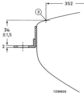
(1) The mounting screws in the cabinet must be situated inside a circle of 8 mm diameter drawn around the true geometrical positions i.e. at the corners of a rectangle of 314,3 mm x 247,6 mm.
