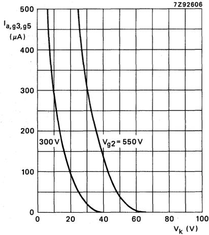
Anode current as a function of cathode voltage.
