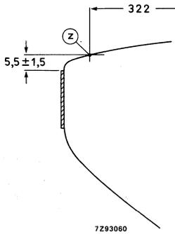
Front view and lug dimensions of tube M32EAK
