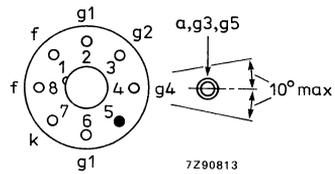
(1) The displacement of any lug with respect to the plane through the three other lugs is max. 2 mm.
