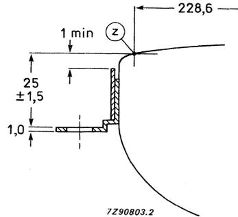
(1) The position of the mounting screws in the cabinet must be within a circle of 4 mm diameter drawn around the true geometrical positions, i.e. the corners of a rectangle of 205 mm x 154 mm.
