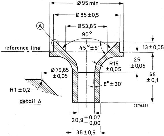
Fig. 2 Reference line gauge for 90° deflection angle.
