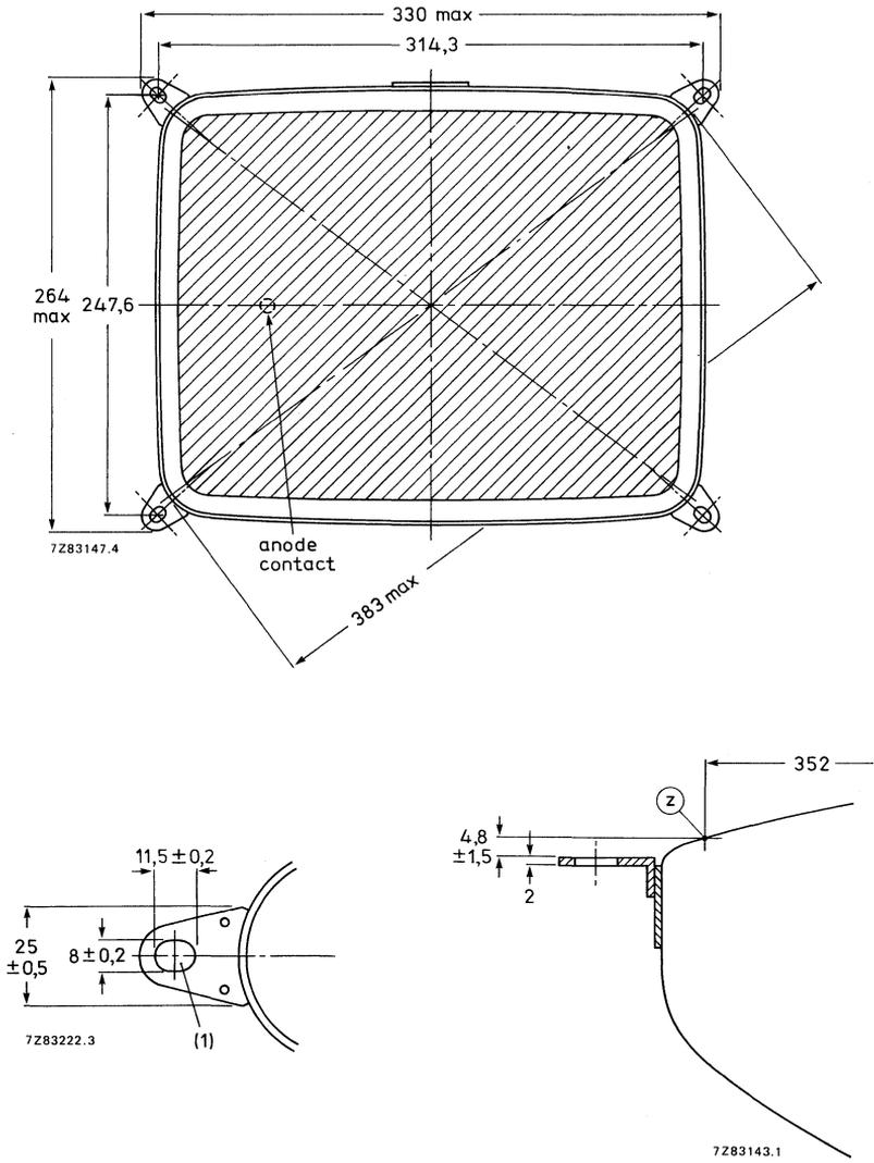
(1) The mounting screws in the cabinet must be situated inside a circle of 5 mm diameter drawn around the true geometrical positions i.e. at the corners of a rectangle of 314,3 mm x 247,6 mm.
