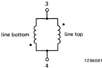
Fig. 2a Line coils, AT1040/04.
