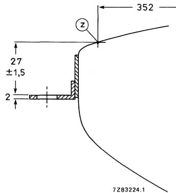
(1) The mounting screws in the cabinet must be situated inside a circle of 5 mm diameter drawn around the true geometrical positions i.e. at the corners of a rectangle of 314,3 mm x 247,6 mm.
