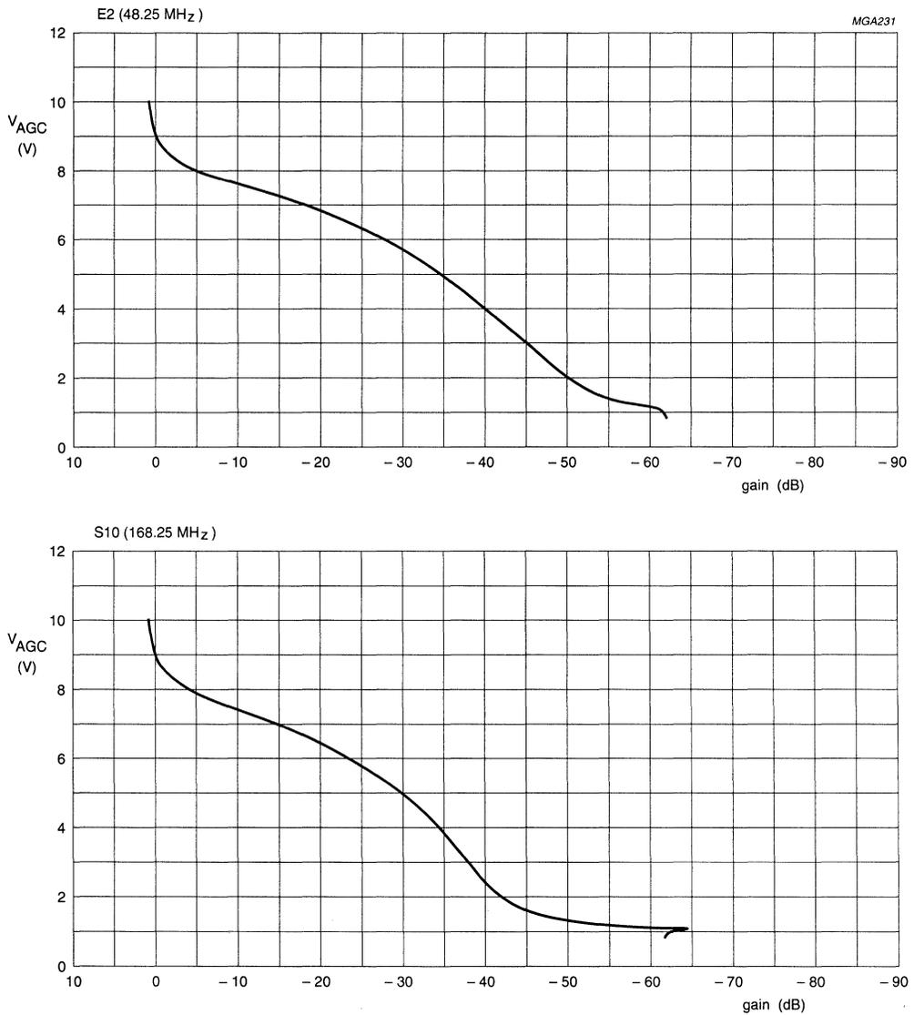
Fig.10 Typical low band AGC curves.
