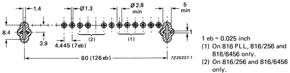
Fig.3 Piercing diagram viewed from solder side of board; unless otherwise stated the tolerance is  $\pm 0,05 \text{ mm}$ .
