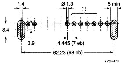
Fig.2 Piercing diagram viewed from solder side of board.
