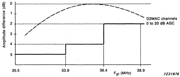
Fig.8 Tilt overall response curves.
