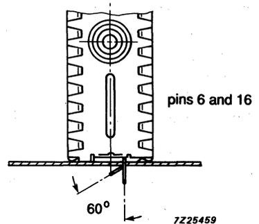
In order to prevent any stress to the printed-wiring board, the tuner should be supported at its aerial connector.
