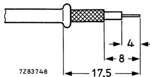
Fig. 3 Recommended cable stripping.
