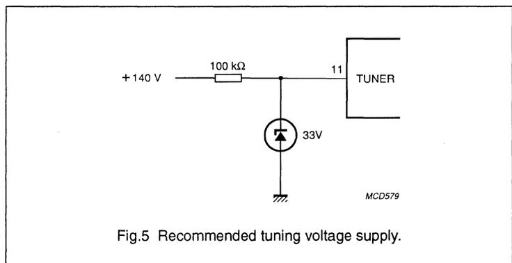
Fig.5 Recommended tuning voltage supply.
