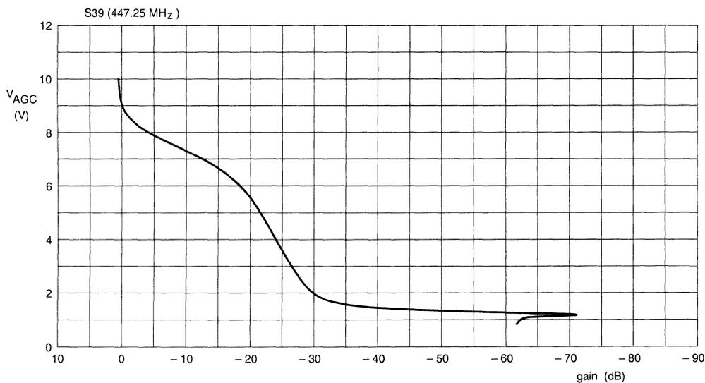
Fig.11 Typical mid band AGC curves.
