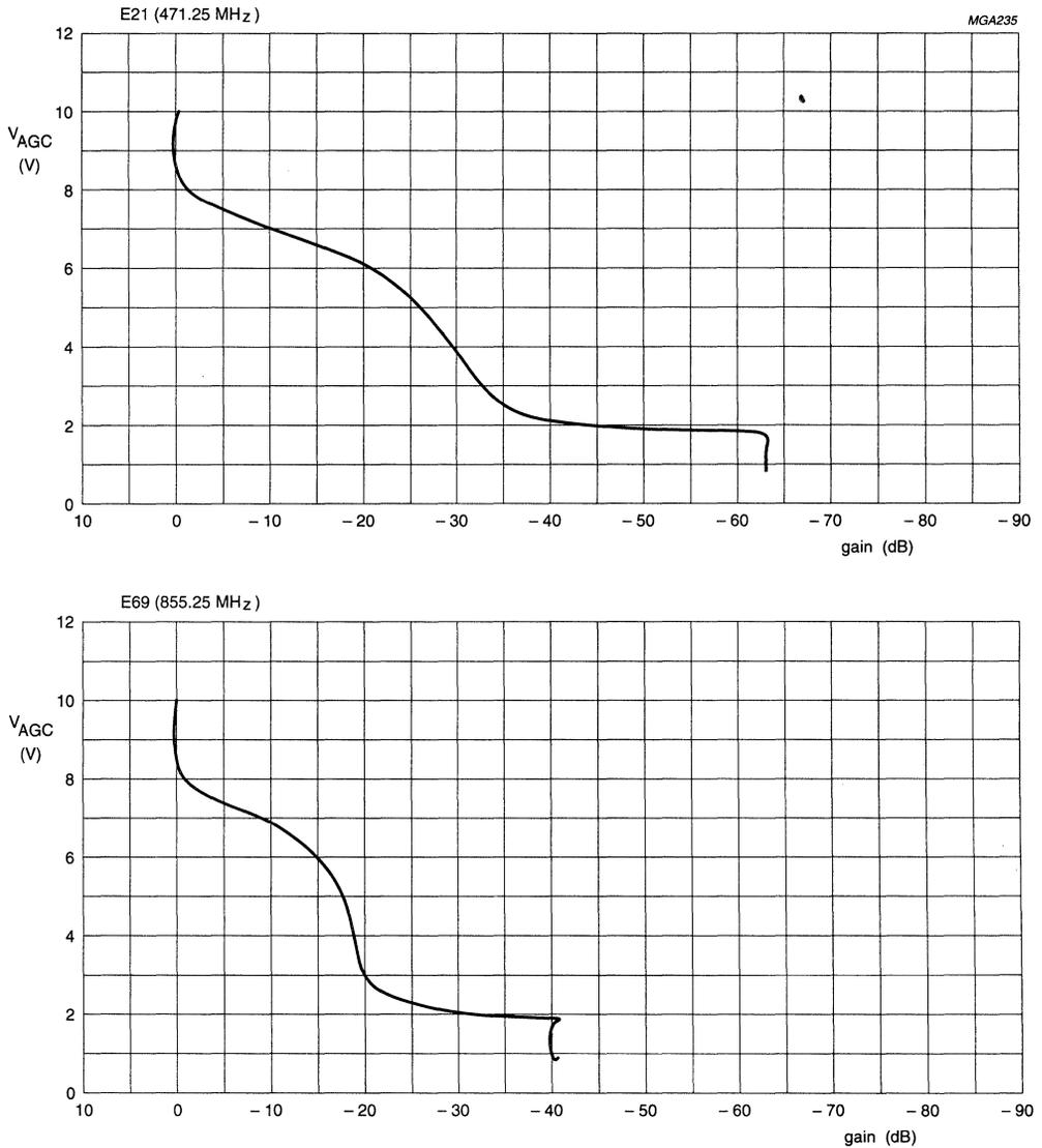
Fig.12 Typical high band AGC curves.
