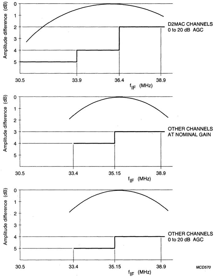
Fig.4 Tilt of overall response curves.
