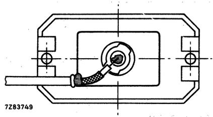
Fig. 3 Recommended fixing of the aerial cable.
