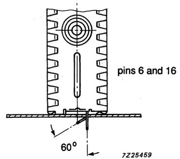
Fig.3 Bending of connecting pins and mounting tabs.
