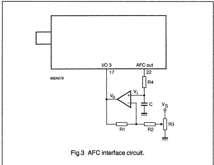
Fig.3 AFC interface circuit.
