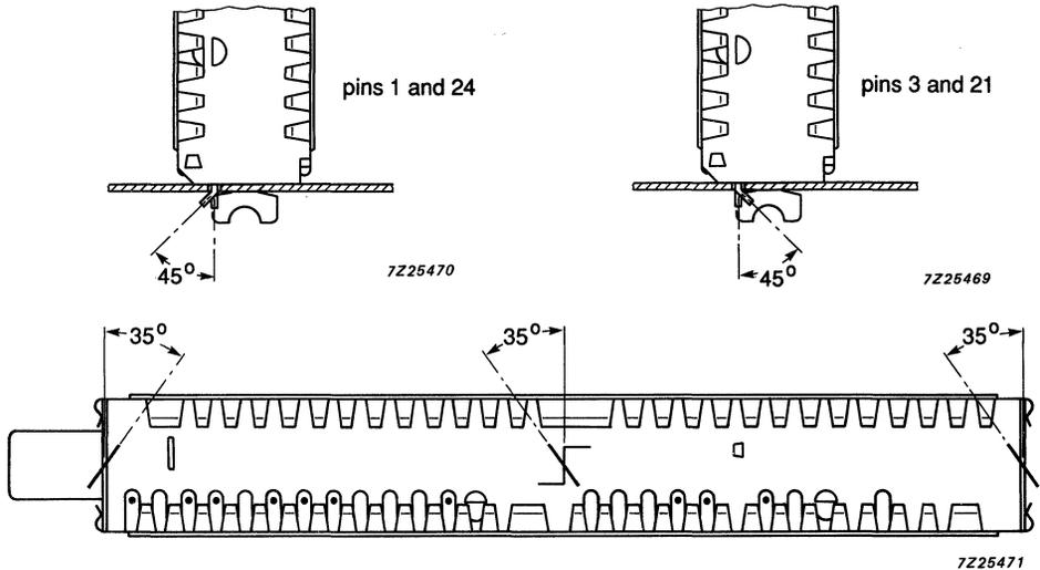
Fig.5 Bending of connecting pins and mounting tags.
