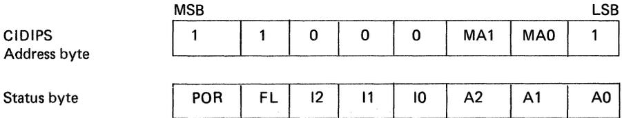
FL is set to 1 when the tuning loop is in lock.
