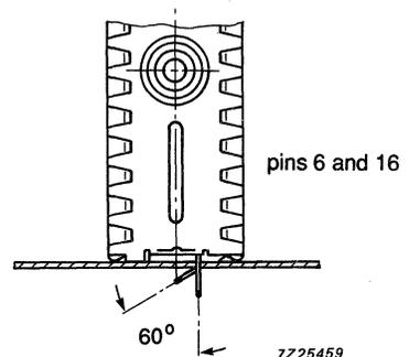
**Note:** In order to prevent any stress to the printed-wiring board, the tuner should be supported at its aerial connector.
