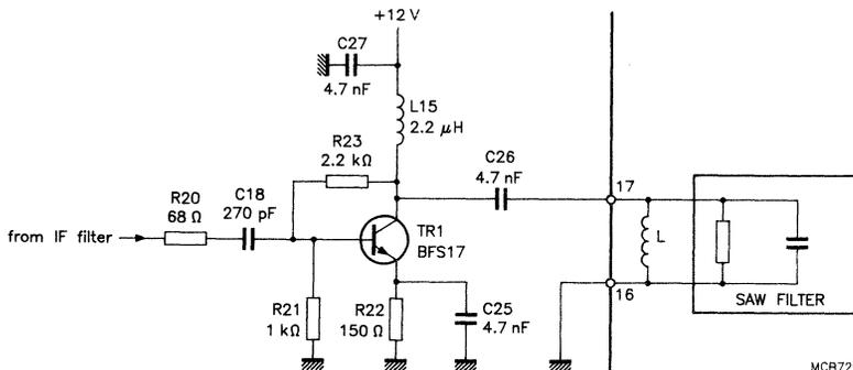
Fig.7 IF output circuit.
