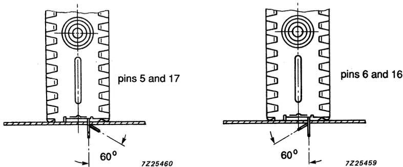
**Note:** In order to prevent any stress to the printed-wiring board, the tuner should be supported at its aerial connector.
