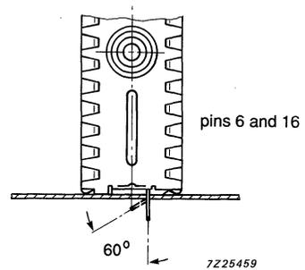
Fig.3 Bending of connecting pins and mounting tabs.
