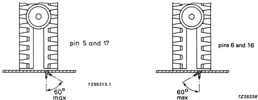
**Note:** In order to prevent any stress to the printed-wiring board, the tuner should be supported at its aerial connector.
