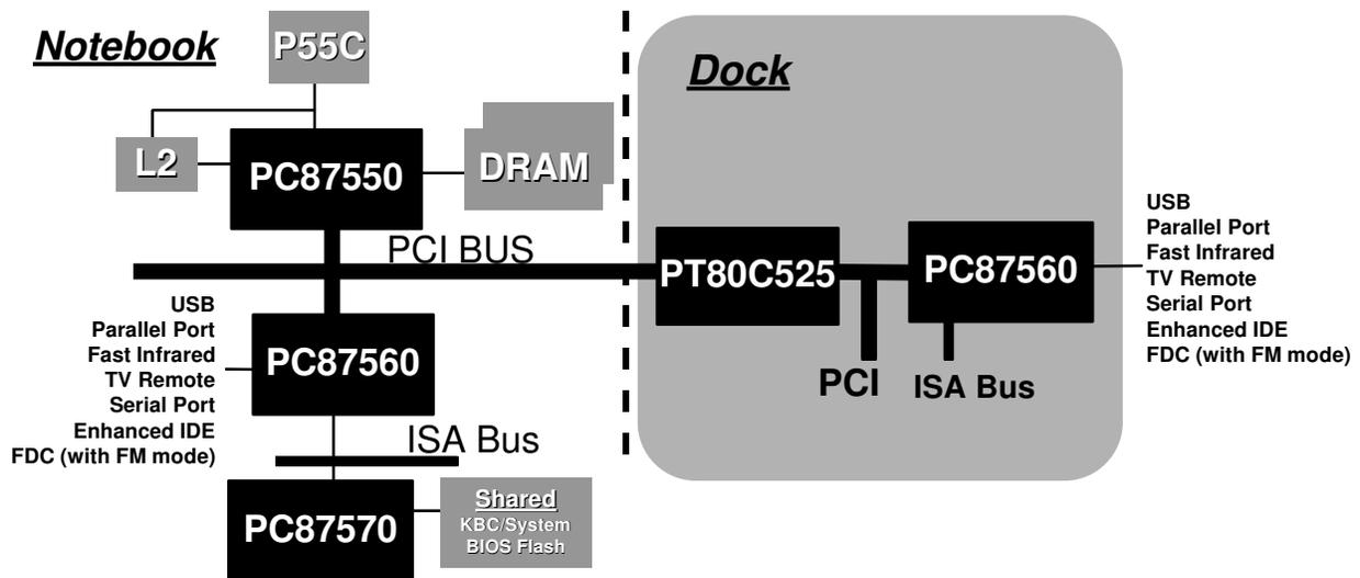
Figure 1. National Semiconductor Mobile System Solution
