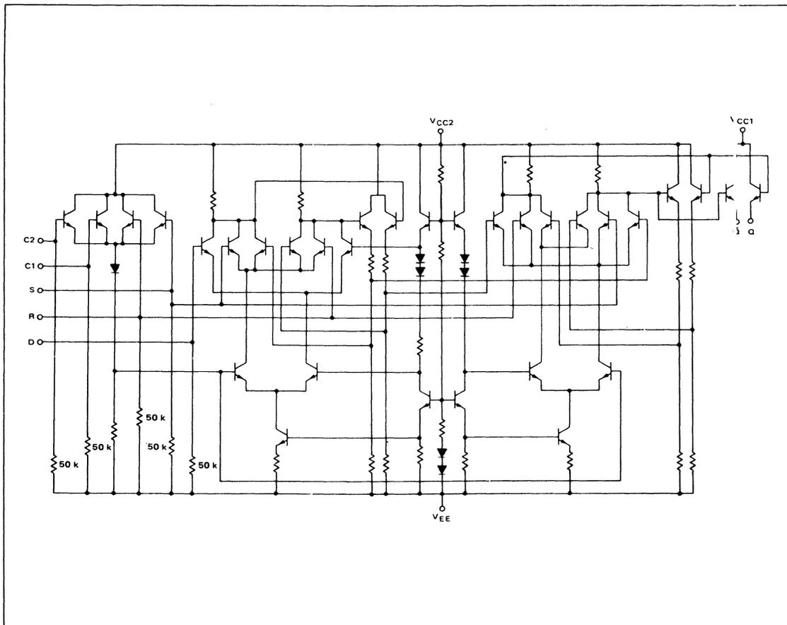
FIGURE 10 - SP1670 CIRCUIT SCHEMATIC
