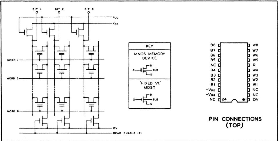
Fig.1 NOM401C circuit and pin connections
