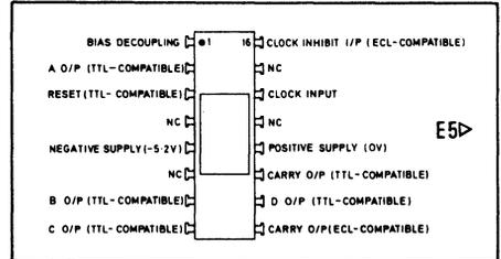
Fig. 1 Pin connections (top)
