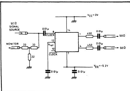
Fig. 3 Toggle frequency test circuit
