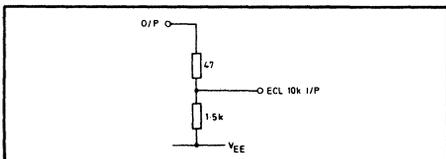
Fig. 4 SP8685 output – ECL 10K i/p and ECL I (or ECL 10K o/p/s unloaded) – ECL 10K i/p
