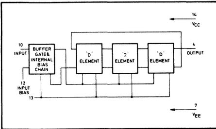
Fig. 2 Functional diagram
