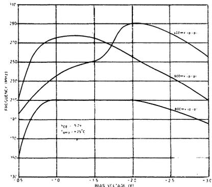
Fig.3 Maximum input frequency v. bias voltage at single input drive levels of 400, 600 and 800 mV (typical device)
