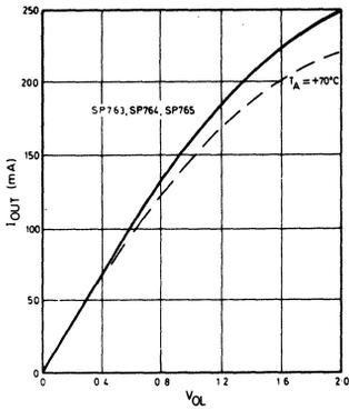
Fig. 5 Output characteristics ( $T_A = +25^\circ\text{C}$ )
