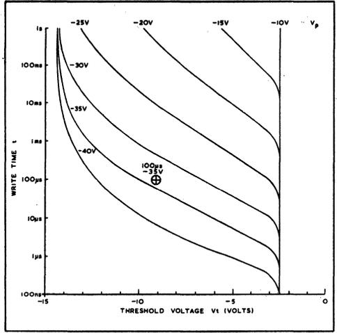
Fig. 3 Speed curves for negative values of  $V_p$
