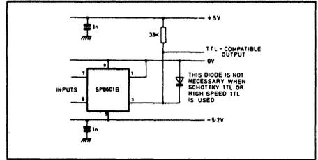
Fig.8 TTL interface (fanout = 1 TTL gate)
