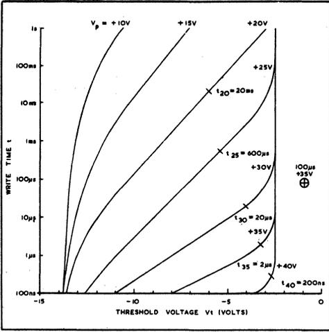
Fig. 2 Speed curves for positive values of  $V_p$
