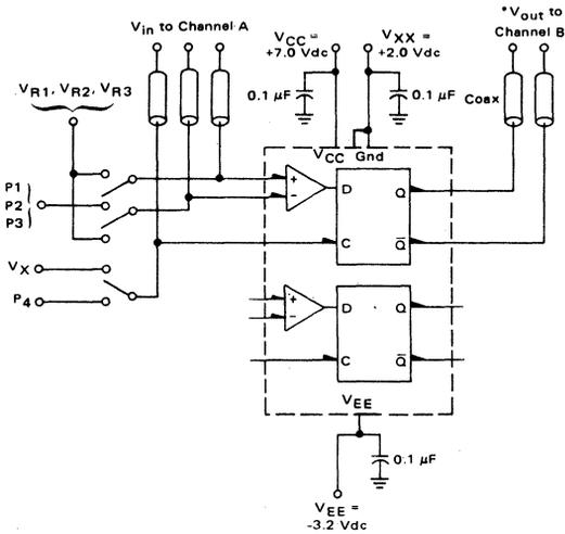
50-ohm termination to ground located in each scope channel input
