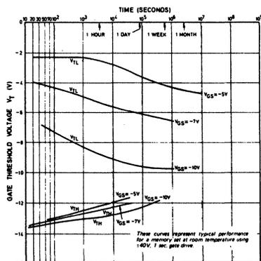
Fig. 8 Threshold voltage retention with continuously applied gate read voltages at  $T_A = +25^\circ\text{C}$
