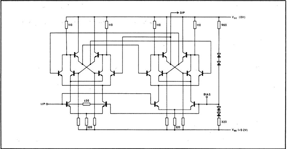
Fig.2 Circuit diagram of 1st element (1-2) showing input biasing arrangement.
