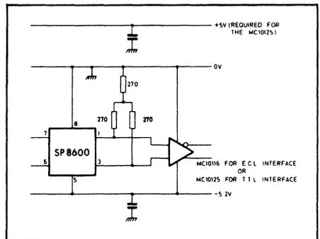
Fig. 7 ECL and Schottky TTL interfacing
