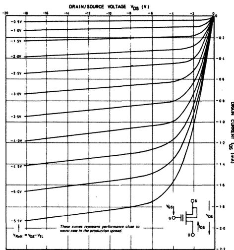
Fig. 4 Drain current  $V_{DS}$  vs  $V_{GS}$  with  $V_T$  set low
