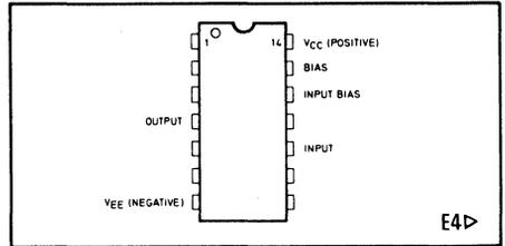
Fig. 1 Pin connections
