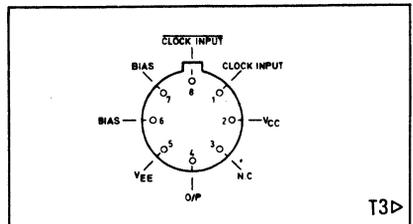
Fig.2 Pin connections (viewed from beneath)
