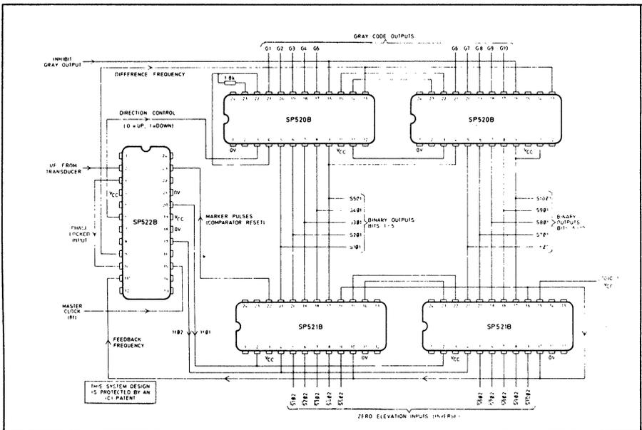
Fig. 5 Frequency-to-digital encoder
