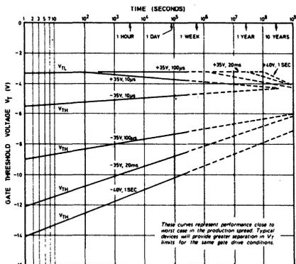
Fig. 5 Threshold voltage retention at  $T_A = +25^\circ\text{C}$
