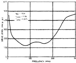
Fig.6 Minimum single input drive level for correct operation v. input frequency (typical device)
