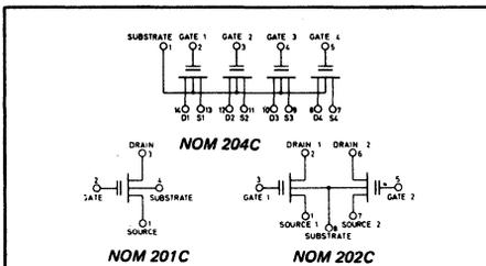
Fig.1 Transistor configurations
