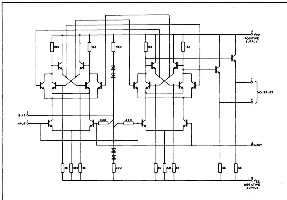
Fig.1 Circuit diagram (all resistor values are nominal)
