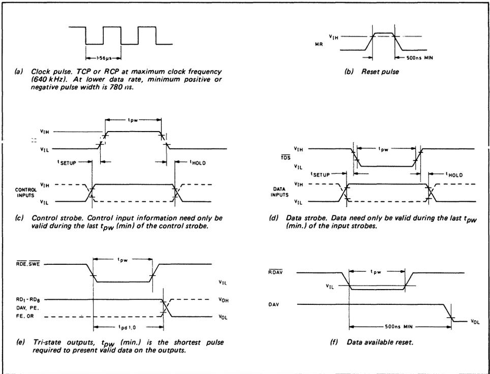
Fig.3 Timing diagrams
