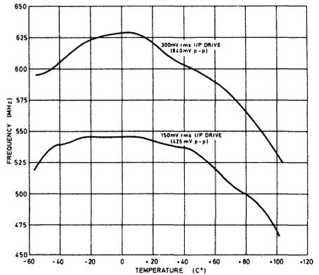
Fig.6 Max. operating frequency v. ambient temperature for a typical SP8631B ( $V_{CC} = -5.2\text{V}$ ).
