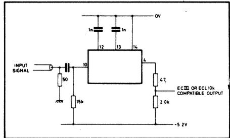
Fig. 5 Interfacing to ECL III or ECL 10,000
