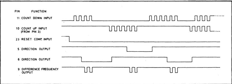
Fig. 4 Frequency comparator and filter timing
