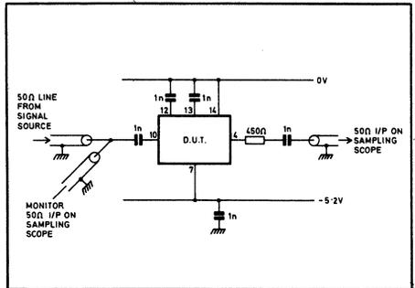
Fig.3 Test circuit.
