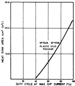
Fig. 9 Operating characteristics, stud package with heatsink ( $T_A = +70^\circ\text{C}$  max.)
