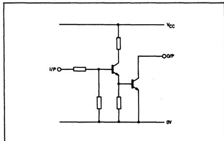
Fig. 2 Functional diagram (one driver)
