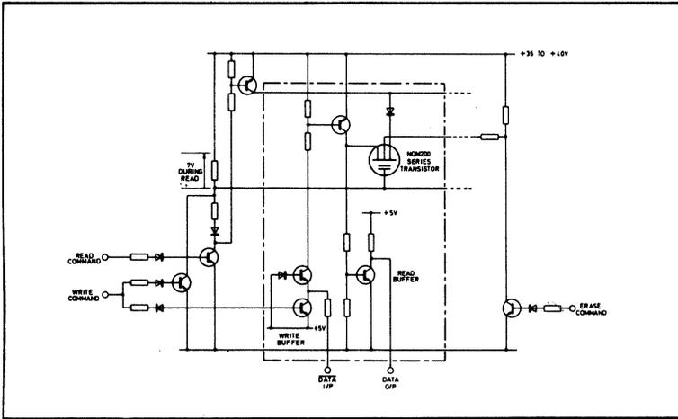
Fig.9 TTL – compatible memory application
