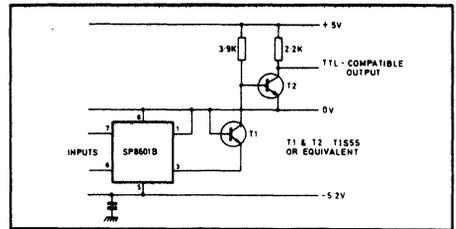
Fig.9 High fanout TTL interface
