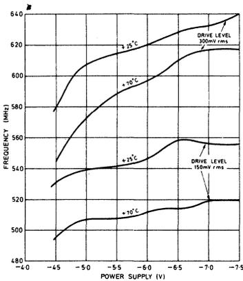
Fig.5 Max. operating frequency v. power supply voltage for a typical SP8631B.
