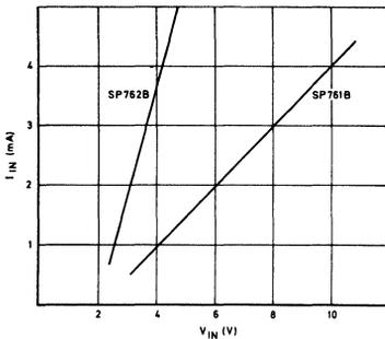
Fig. 3 Input characteristic (including strobe)  $T_{amb} = +25^{\circ}\text{C}$
