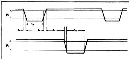
Fig. 3 Clock waveforms
