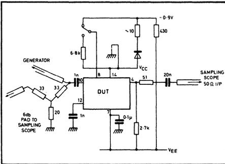
Fig. 3 Test circuit
