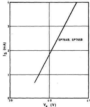
Fig. 4 Strobe input characteristics ( $T_A = +25^\circ\text{C}$ )
