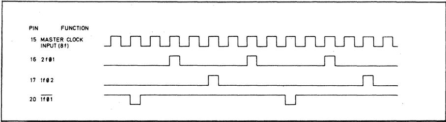
Fig. 2 Frequency divider logic timing
