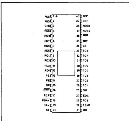
Fig. 1 Pin connections
