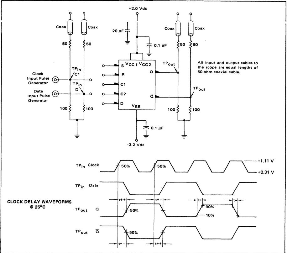
FIGURE 2 – SET-RESET DELAY WAVEFORMS @ 25°C
