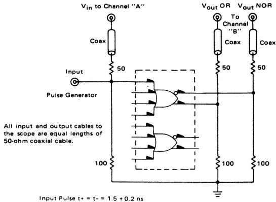
Unused outputs connected to a 50-ohm resistor to ground
