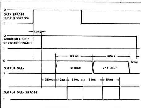
Fig. 4 Output timing Note: times specified are minimum.
