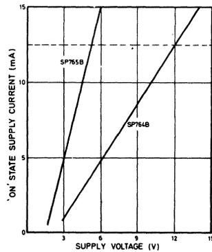
Fig. 10 Current drain per element ( $T_A = +70^\circ\text{C}$  max.)
