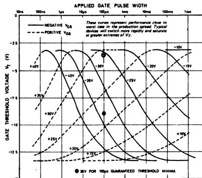
Fig. 7 Write/Erase switching speed characteristics
