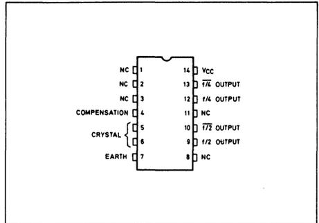
Fig.1 Pin connections
