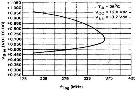
Figure 6 illustrates the variation in toggle frequency with the dc offset voltage ( $V_{Bias}$ ) of the input clock signal.  $V_{Bias}$  is defined by the test circuit in Figure 4, and waveform Figure 5.
