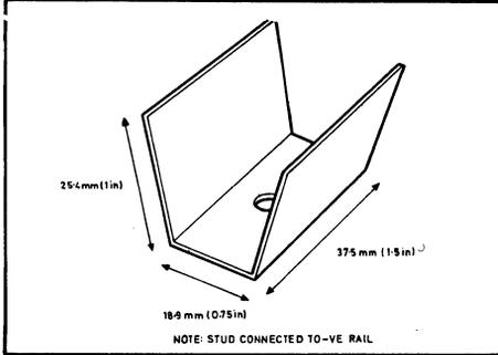
Fig. 13 Heatsink details for stud package
