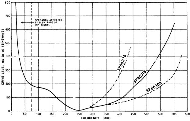
Fig.4 Minimum drive level v.  $1/P$  frequency at  $+25^{\circ}\text{C}$ .
