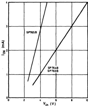
Fig. 3 Input characteristics ( $T_A = +25^\circ\text{C}$ )
