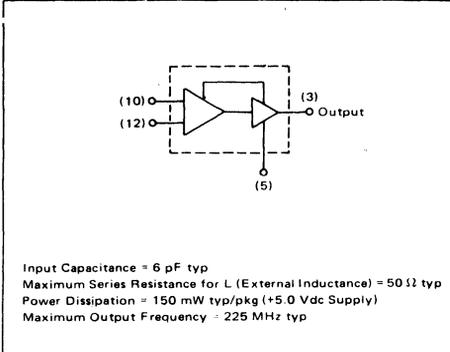
FIGURE 1 – CIRCUIT SCHEMATIC
