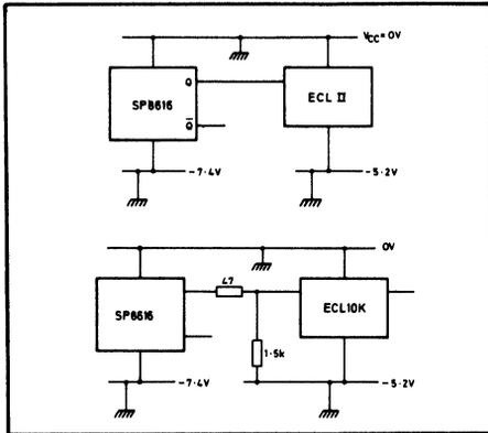
Fig. 6 Interfacing SP8616 series to ECL II and ECL III
