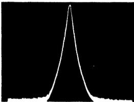
B.W. = 10 kHz      Scan Width = 50 kHz/div
