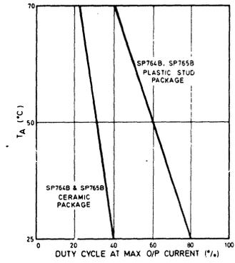
Fig. 6 Operating characteristics ( $T_A = +25^\circ\text{C}$  to  $+70^\circ\text{C}$ )
