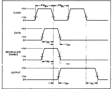
Fig. 3 Timing diagram and voltage wave forms
