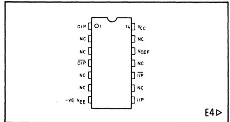
Fig. 1 Pin connections
