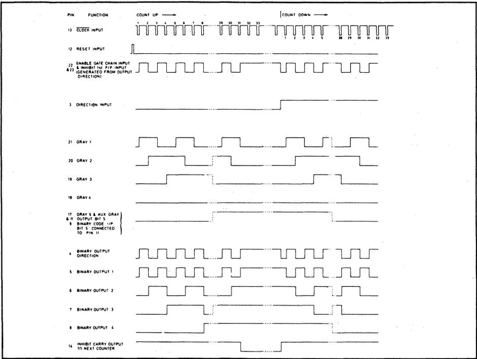
The enable gate chain output is normally in the '0' state and goes to the '1' state only when all the Gray outputs are low and the enable input high.
