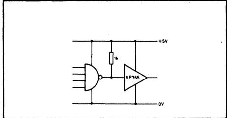
Fig.12 TTL interface to SP765 strobe input
