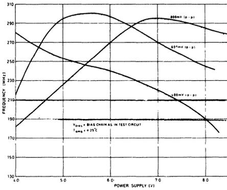
Fig.4 Maximum input frequency v. power supply voltage at single input drive levels of 400, 600 and 800 mV (typical device)
