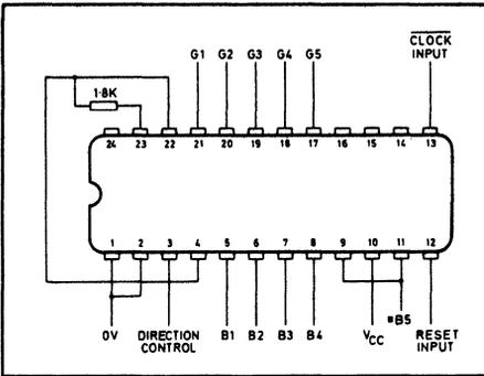
Fig.2 SP520 connected as a 5-bit counter
