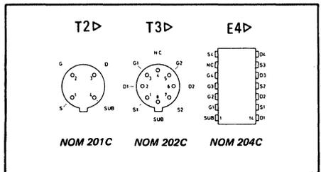
Fig.2 Pin connections (viewed from beneath)
