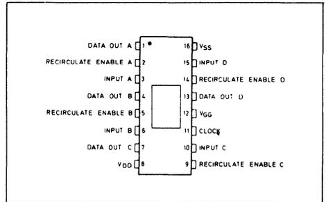
Fig. 1 Pin connections
