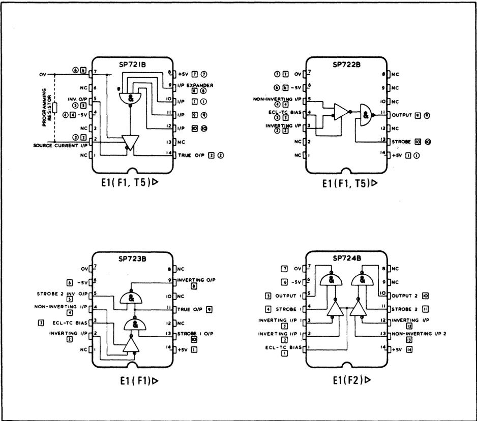
Fig. 1 Logic and dual-in-line package connection diagrams. Connections for package options shown thus: □ = Flatpack, ○ = TO-5.
