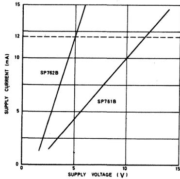
Fig. 7 On state supply current drain per element
