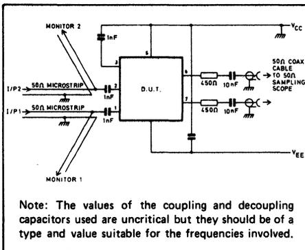
Fig.2 Test circuit
