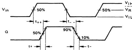
Test pulses:  $t_{p+}, t_{p-} = 1.5 \pm 0.2$  ns (10% to 90%)
