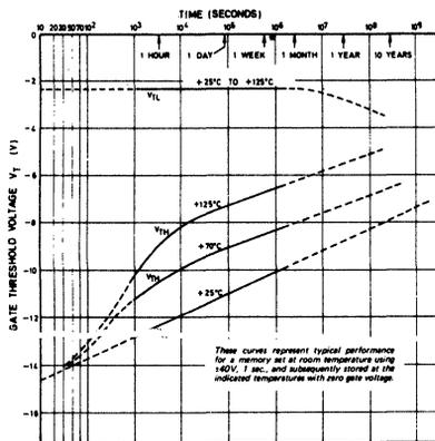
Fig. 6 Threshold voltage retention at high ambient temperatures
