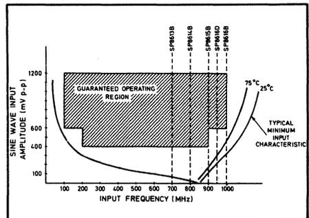
Fig. 3 Specified range of operation
