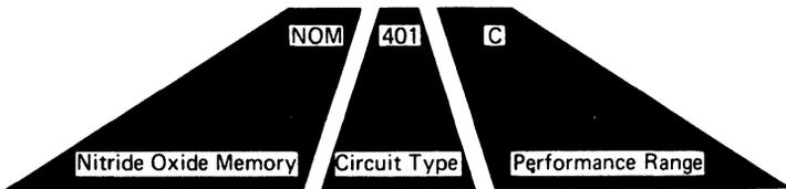
The term 'performance range' refers to the relationship between storage time and writing conditions. All devices are available, as standard, in performance grade C, which provides a minimum storage time of 1 year with typical write conditions of 35V for 100µs. Other performance grades offering 100 years minimum storage time or 1µs write time can be made available to special order.
