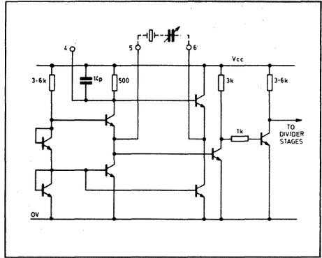
Fig. 3 Circuit diagram of SP705B oscillator
