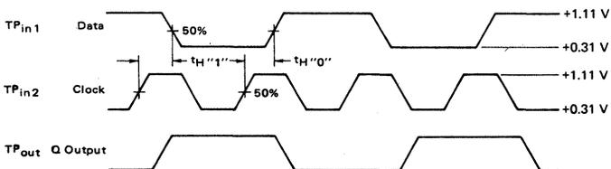
Set up time is the minimum time before the positive transition of the clock pulse (C) that information must be present at the data (D) input.
