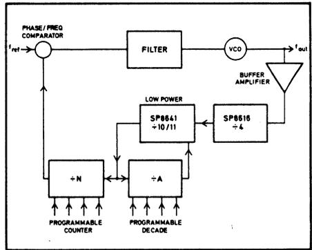
Fig. 8 A 1GHz synthesiser loop
