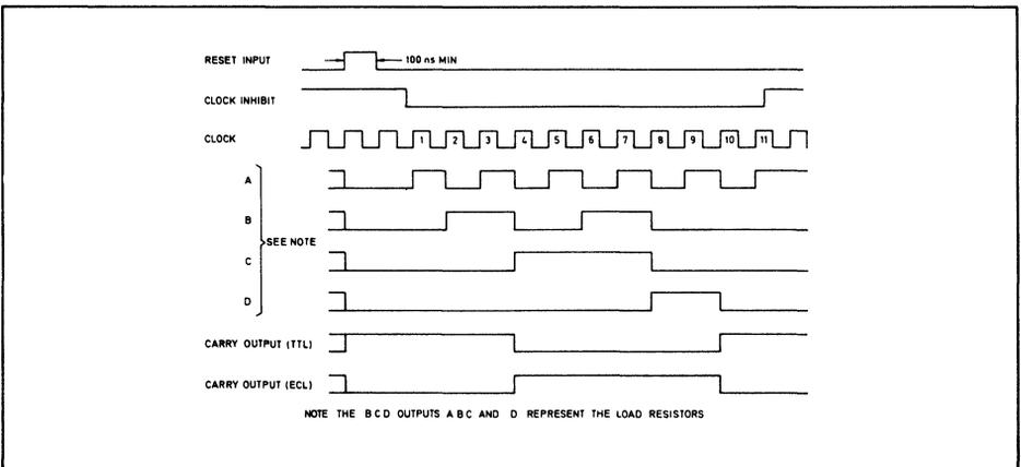
Fig. 5 Decade counter timing diagram
