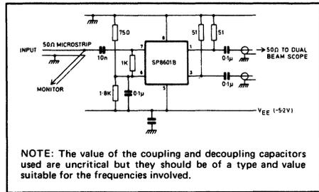
NOTE: The value of the coupling and decoupling capacitors used are uncritical but they should be of a type and value suitable for the frequencies involved.
