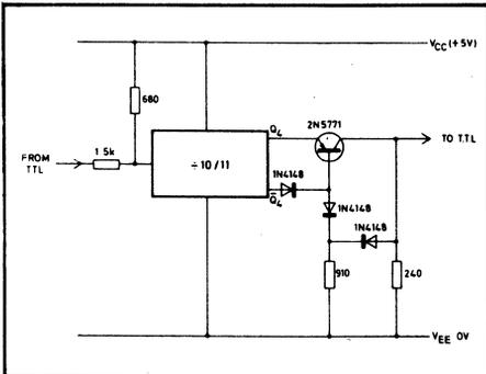
Fig. 7 TTL to ECL and ECL/TTL interfaces (for SP8640 devices and TTL operating from the same supply rails)
