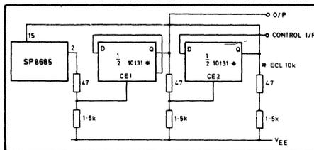
Fig. 6 Divide-by-20/22. Control loop delay time approximately 40ns.
