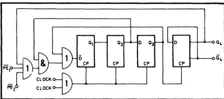
Fig. 2 Logic diagram (positive logic)
