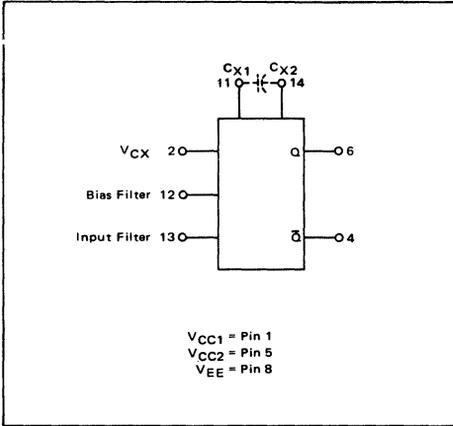
The SP1658 is a voltage-controlled multivibrator which provides appropriate level shifting to produce an output compatible with RECU III and RECU 10,000 logic levels. Frequency control is accomplished through the use of voltage-variable current sources which control the slew rate of a single external capacitor.
