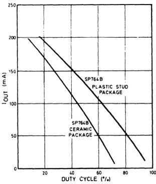
Fig. 7 SP764 operating characteristics ( $T_A = +70^\circ\text{C}$  max.)
