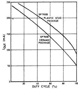
Fig. 8 SP765 operating characteristics ( $T_A = +70^\circ\text{C}$  max.)
