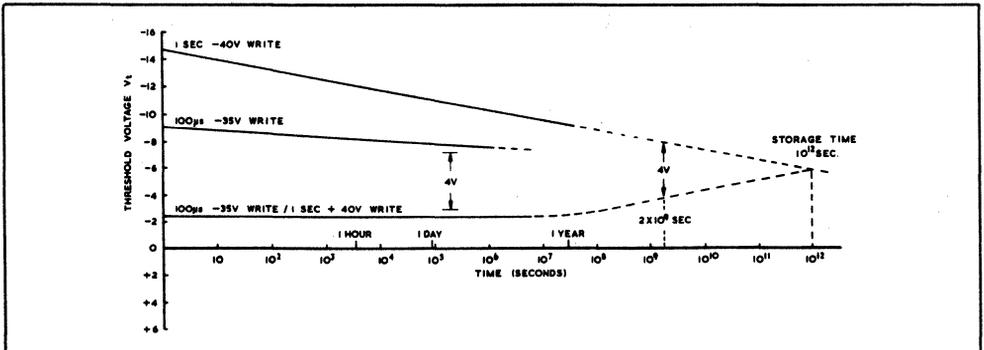
Fig. 5 Memory retention characteristic
