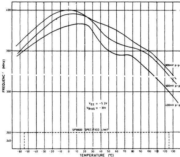
Fig. 5 Maximum input frequency v. temperature
