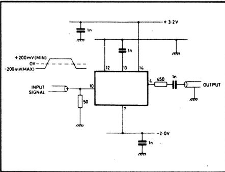
Fig. 4 Directly connecting the input signal
