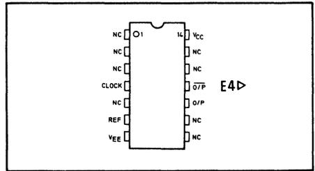
Fig. 1 Pin connections
