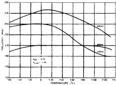
Fig.5 Maximum input frequency v. temperature at single input drive levels of 400, 600 and 800 mV (typical device)
