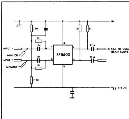
Fig. 3 Test circuit
