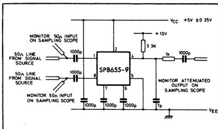
Fig.3 Test circuit
