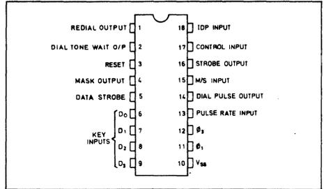
Fig. 1 Pin connections (top)
