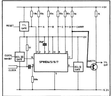
Fig. 4 Typical application configuration
