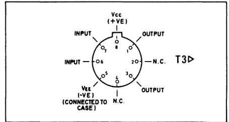
Fig. 1 Pin connections (viewed from beneath)
