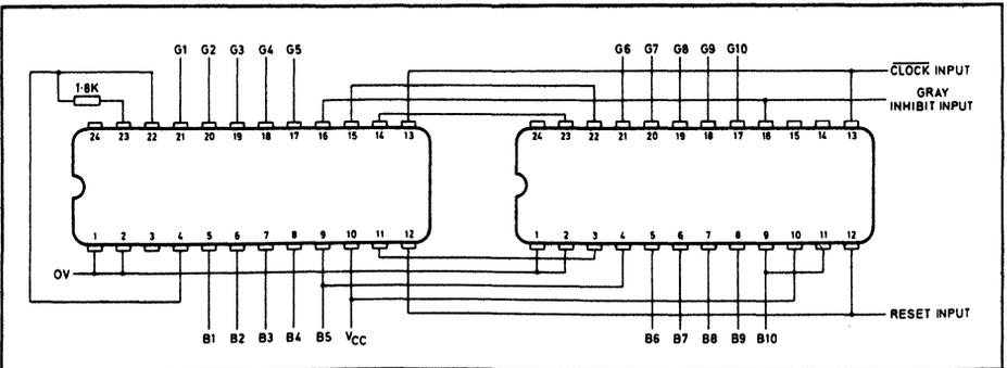
Fig.3 Two SP520s connected as a 10-bit counter
