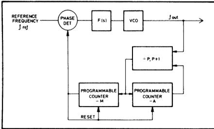
Fig. 9 Synthesiser block diagram (simplified)
