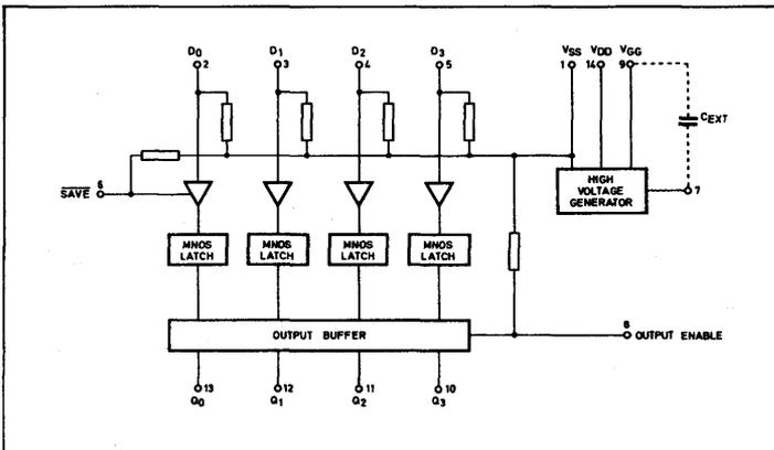
Fig. 2 Block diagram of MN9102
