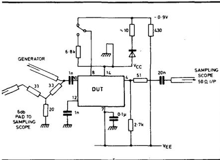
Fig. 3 Test circuit
