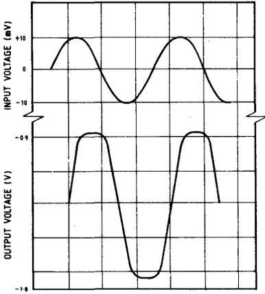
Fig. 6 Response to a 100MHz sine wave
