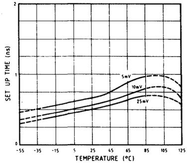
Fig. 9 Set-up time as a function of temperature
