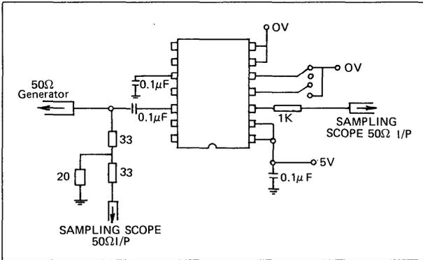
Fig. 5 - Test Circuit
