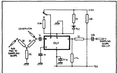
Fig. 3 Test circuit
