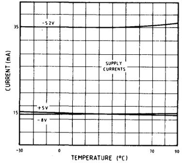
Fig. 7l Supply current variation with temperature
