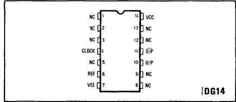
Fig. 1 Pin connections
