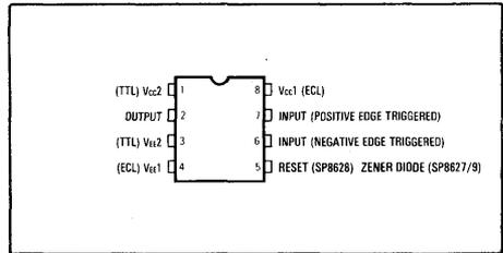
Fig. 1 Pin connections
