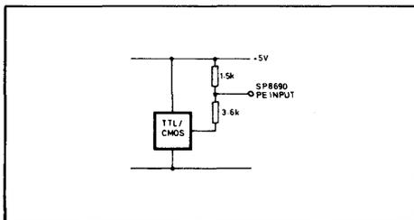
Fig.3 TTL/CMOS interface
