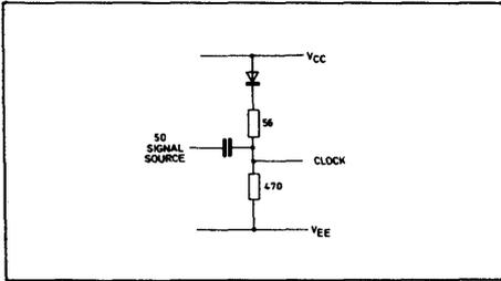
Fig. 6. Recommended input bias configuration for capacitive coupling to a continuous 50  $\Omega$  signal source
