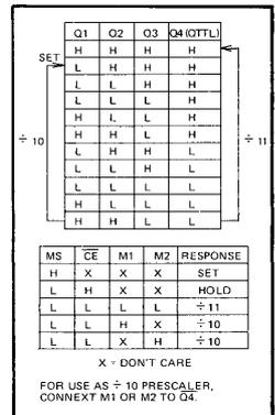
Fig. 3 — Count Sequence & Control Input Truth Table
