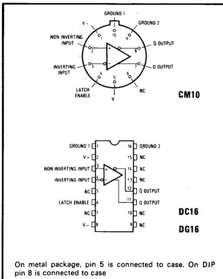
On metal package, pin 5 is connected to case. On DIP pin 8 is connected to case
