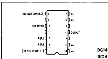
Fig. 1 Pin Connections
