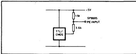
Fig.3 TTL/CMOS interface
