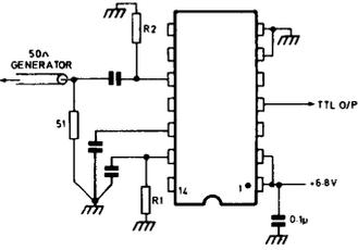
Capacitors are 1 nf unless otherwise stated. Values should be increased if operation below 10 MHz is desired.
