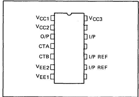
Fig. 1 – Pin Configuration
