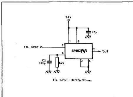
Fig. 4 TTL input (DC <  $f_{in}$  <  $f_{max}$ )
