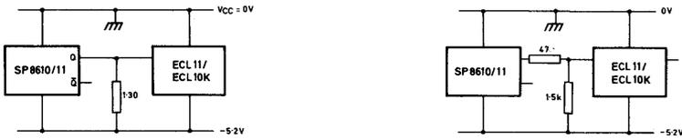
Fig. 5 Interfacing SP8610/11 to ECL10K and ECL III
