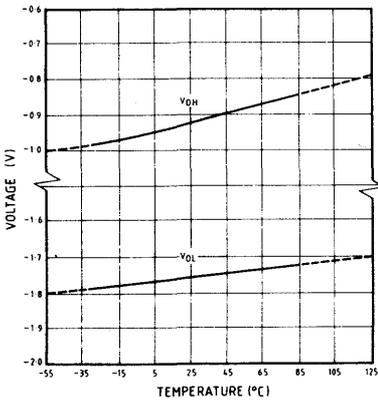
Fig. 16 Output levels as a function of temperature
