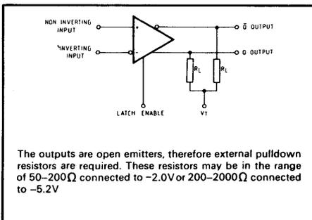
The outputs are open emitters, therefore external pulldown resistors are required. These resistors may be in the range of 50-200 $\Omega$  connected to -2.0V or 200-2000 $\Omega$  connected to -5.2V
