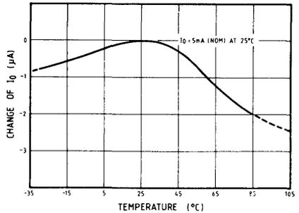
Fig. 7M Analogue output current variation with temperature
