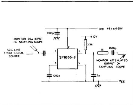
Fig. 3 Test circuit
