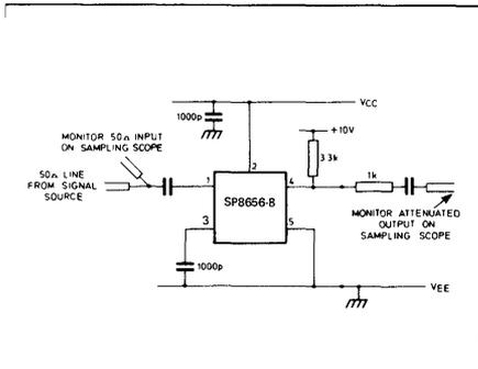
Fig. 3 Test circuit
