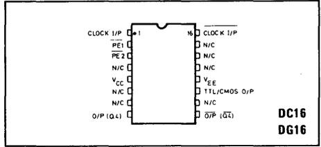
Fig. 1 Pin connections
