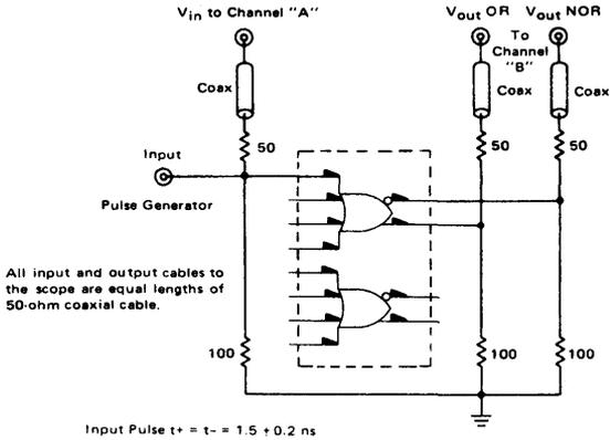
Unused outputs connected to a 50-ohm resistor to ground
