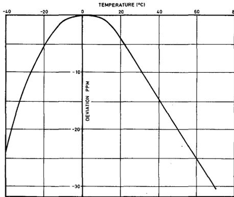
Fig. 5 Frequency/temperature characteristics of CB 10.24 MHz crystal oscillator
