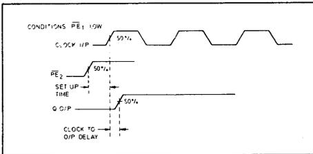
Fig. 3 Set-up timing diagram
