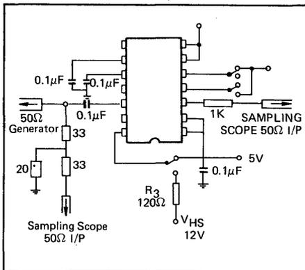
Fig. 5 - Test Circuit
