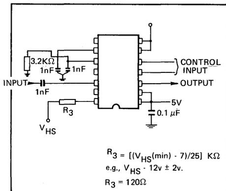
Fig. 6. - Application Circuit
