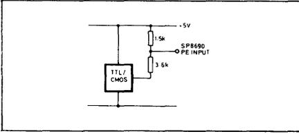
Fig.3 TTL/CMOS interface
