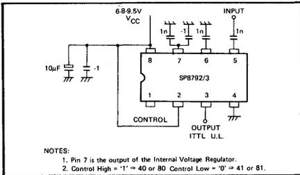
Fig. 3 - SP8792/3 Application Diagram
