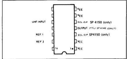
Fig. 1 - Pin connections
