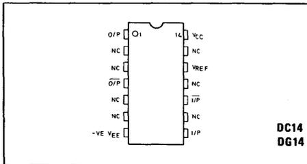
Fig. 1 Pin connections
