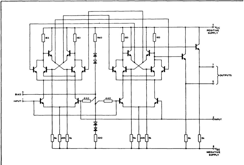
Fig. 2 Circuit diagram (all resistor values are nominal)
