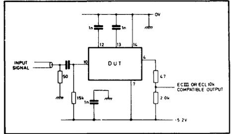
*Fig. 5 Interfacing to ECL III or ECL 10,000*
