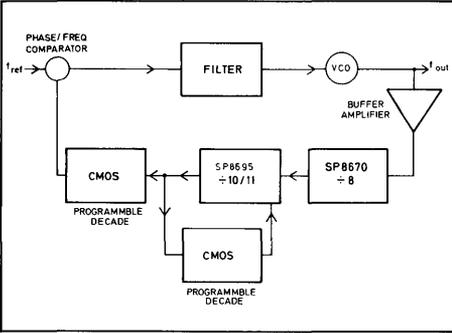
Fig. 5 A low power synthesizer loop
