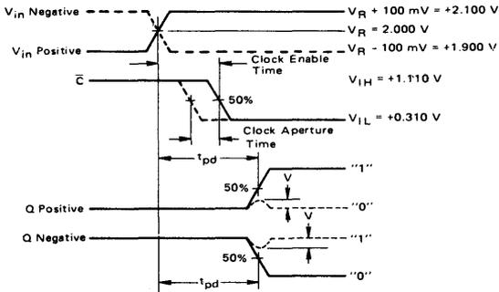
————— Clock enable time = minimum time between analog and clock signal such that output switches, and  $t_{pd}$  (analog to Q) is not degraded by more than 200 ps.
