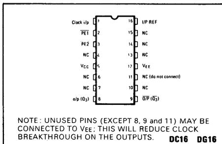
Fig. 1 Pin connections
