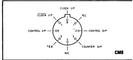
Fig. 1 Pin connections
