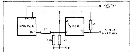
Fig. 5 40/42 control loop delay time 24ns typ.
