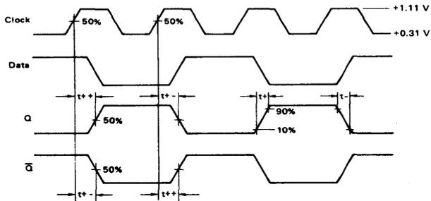
FIGURE 2 – SETUP AND HOLD TIME TEST CIRCUIT
