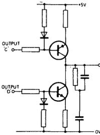
Fig. 5 Low voltage charge pump and filter
