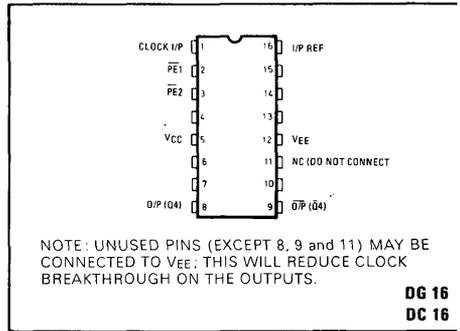
Fig. 1 Pin connections
