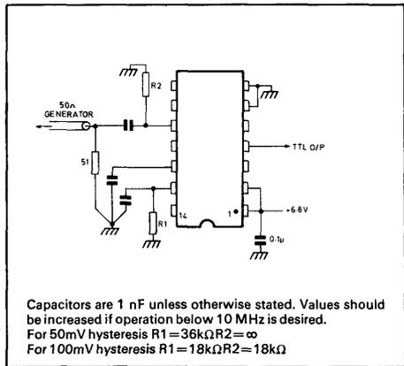
Capacitors are 1 nF unless otherwise stated. Values should be increased if operation below 10 MHz is desired.
