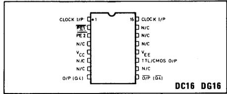
Fig.1 Pin connections
