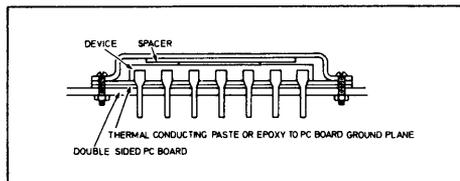
Fig. 5 Heat sink for 'M' grade devices
