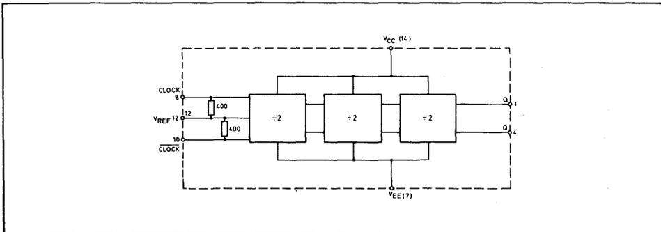
Fig. 2 Functional diagram
