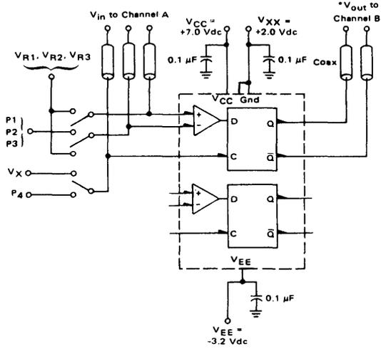
50-ohm termination to ground located in each scope channel input
