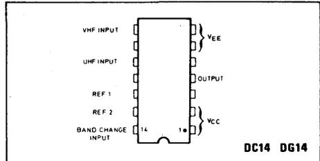
Fig. 1 Pin connections
