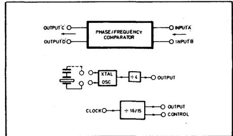
Fig. 2 SP8760 block diagram
