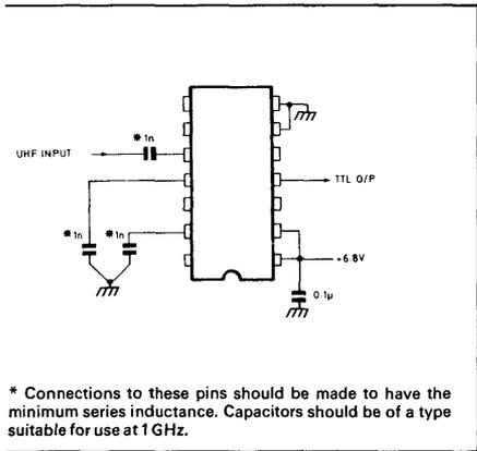
Fig. 3 Application circuit
