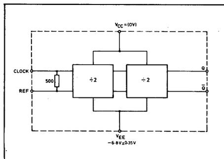
Fig. 2 Functional diagram
