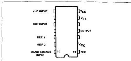
Fig. 1 Pin connections
