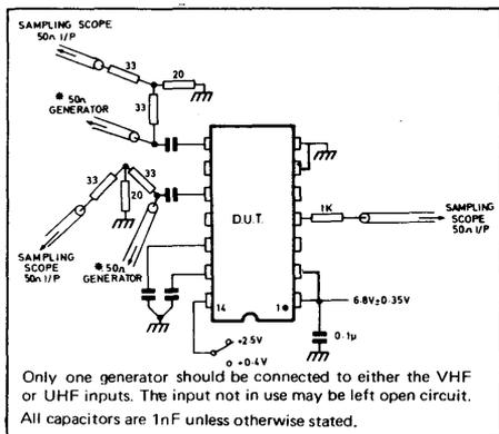
Only one generator should be connected to either the VHF or UHF inputs. The input not in use may be left open circuit. All capacitors are 1nF unless otherwise stated.
