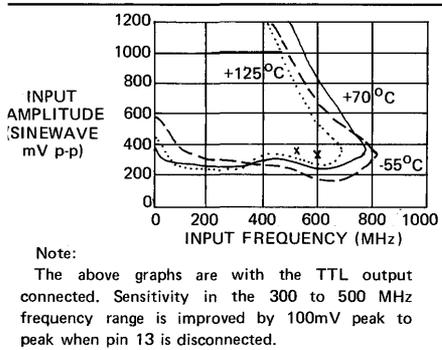
Fig. 4 Clock Input Frequency versus Amplitude (a.c. coupled)
