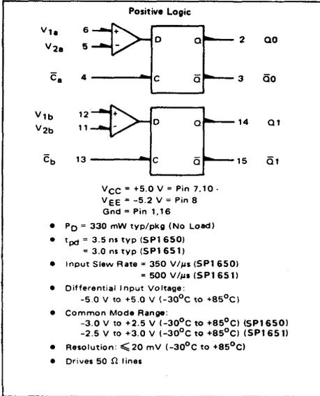
The SP1650 and the SP1651 are very high speed comparators utilizing differential amplifier inputs to sense analog signals above or below a reference level. An output latch provides a unique sample-hold feature. The SP1650 provides high impedance Darlington inputs, while the SP1651 is a lower impedance option, with higher input slew rate and higher speed capability.
