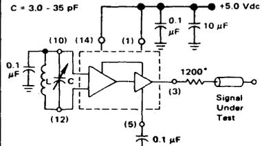
\*The 1200 ohm resistor and the scope termination impedance constitute a 25:1 attenuator probe. Coax shall be CT-070-50 or equivalent.
