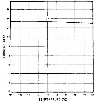
Fig. 15 Supply current as a function of temperature
