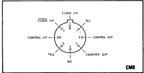
Fig. 1 Pin connections.
