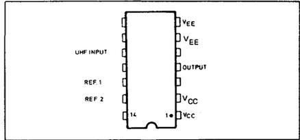
Fig. 1 - Pin connections
