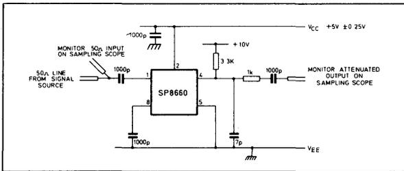
Fig. 3 Test circuit
