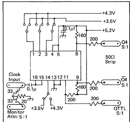
Fig. 5 - Dynamic Test Circuit
