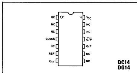
Fig. 1 Pin connections
