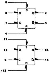
This device is a Dual Clocked Latch/R-S Flip-Flop. Whenever the Clock is low, the R-S inputs control the output state. Whenever the Clock is high, the output follows the data (D) input.
