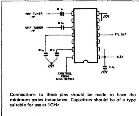
Fig. 4 Application circuit
