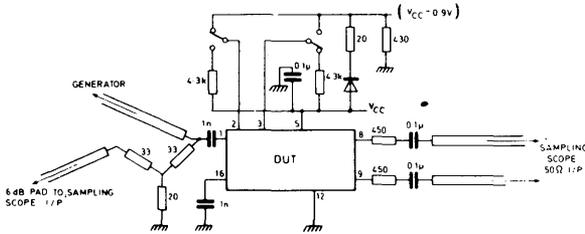
Fig. 3 Test circuit
