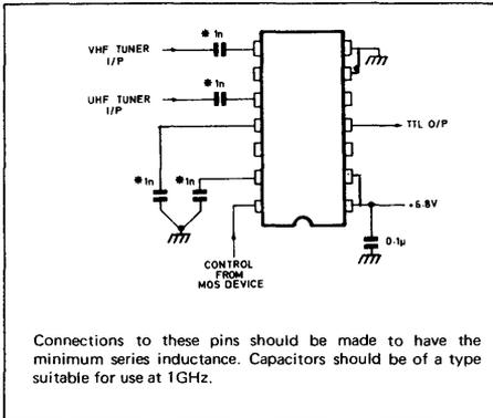
Fig. 4 Application circuit
