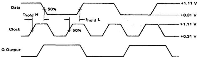
Setup time is the minimum time before the positive transition of the clock pulse (C) that information must be present at the data (D) input.
