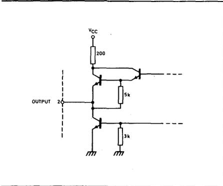
Fig. 7 Output circuit diagram
