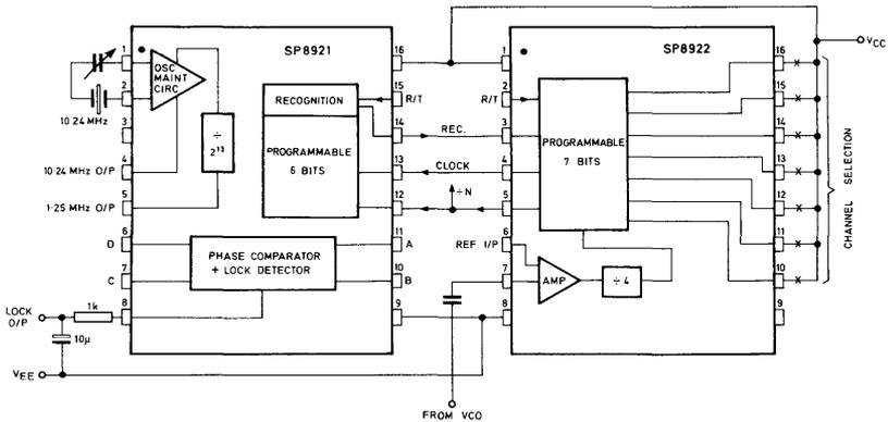
Fig. 2 SP8921/SP8922 interconnections (10.695MHz receive offset)
