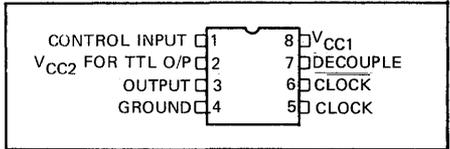
Fig. 1 — Pin connections
