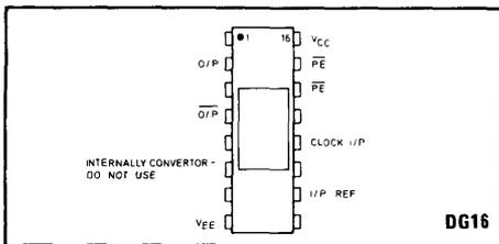
Fig. 1 Pin connections
