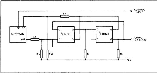
Fig. 6 ÷ 80/81 control loop delay time 55ns typ.
