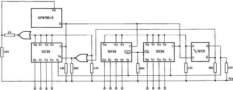
Fig. 7 1.3 GHz variable divider (200—2000 in steps of 2)
