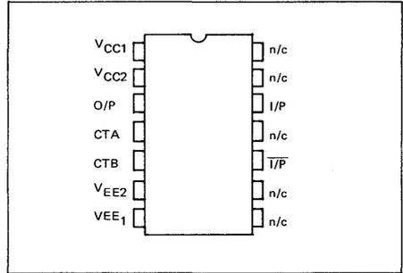
Fig. 1 Pin Configuration
