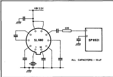
Fig. 17 High stability crystal reference oscillator using SL680
