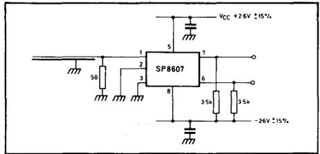
Fig. 4 Direct coupling using split power supplies
