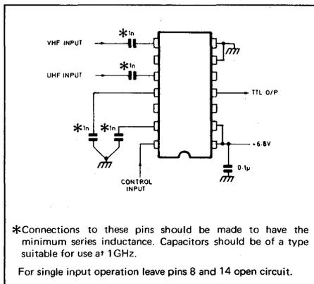
Fig. 4 Application circuit
