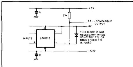
Fig. 9 TTL interface (fanout = 1 TTL gate)
