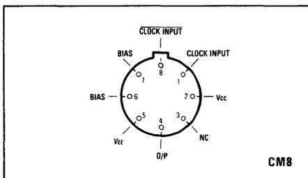
Fig. 1 Pin connections (viewed from beneath)
