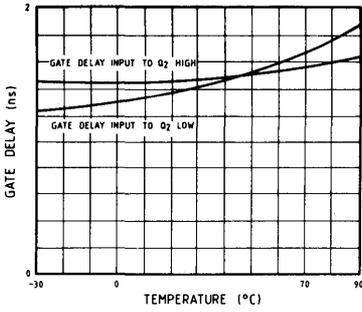
Fig. 7i Gate input to Q<sub>1</sub> - Q<sub>4</sub> delay variation with temperature
