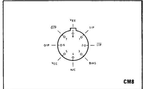
Fig. 1 Pin connections
