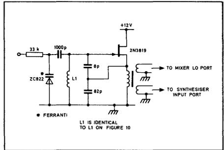
Fig. 18 Voltage controlled oscillator for 27MHz CB synthesiser
