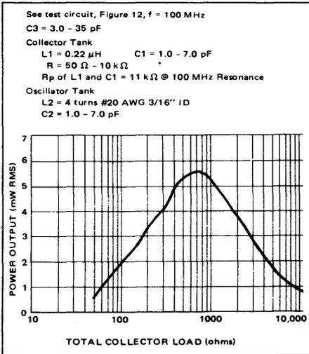
FIGURE 14 – POWER OUTPUT versus COLLECTOR LOAD
