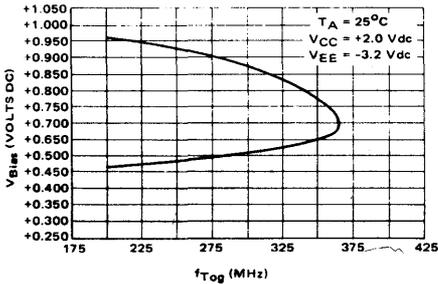
Figure 6 illustrates the variation in toggle frequency with the dc offset voltage ( $V_{Bias}$ ) of the input clock signal.  $V_{Bias}$  is defined by the test circuit in Figure 4, and waveform Figure 5.
