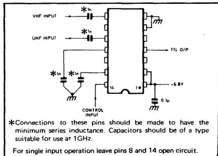
Fig. 4 Application Circuit
