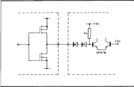
Fig. 3 CMOS and TTL compatible control I/P.
