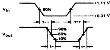
All input and output cables to the scope are equal lengths of 50-ohm coaxial cable.
