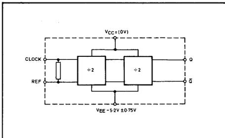
Fig. 2 Functional diagram
