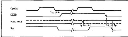
Fig. 4 Output control timing
