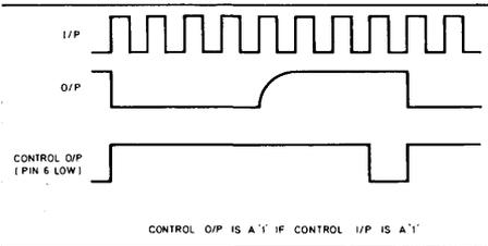
Fig. 4 SP8794 waveforms
