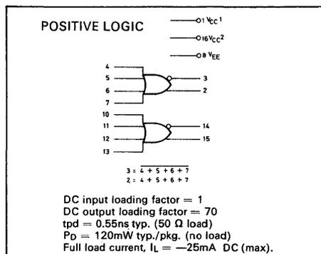
Fig. 1 Logic diagram
