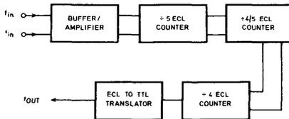
Fig. 2 SP8627/8/9 logic diagram
