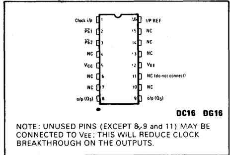
Fig. 1 Pin connections
