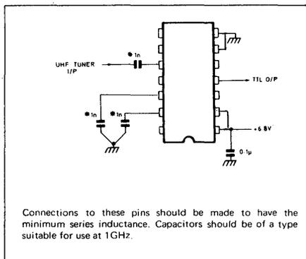
Fig. 4 - Application circuit
