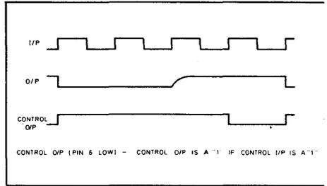
Fig. 4 SP8790 waveforms
