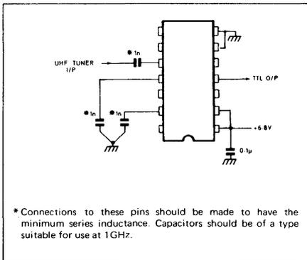
Fig. 4 — Application circuit
