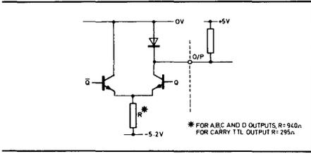
Fig. 4 TTL carry and ABCD output structure
