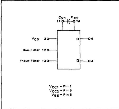
The SP1658 is a voltage-controlled multivibrator which provides appropriate level shifting to produce an output compatible with PECL, III and PECL, 10,000 logic levels. Frequency control is accomplished through the use of voltage-variable current sources which control the slew rate of a single external capacitor.
