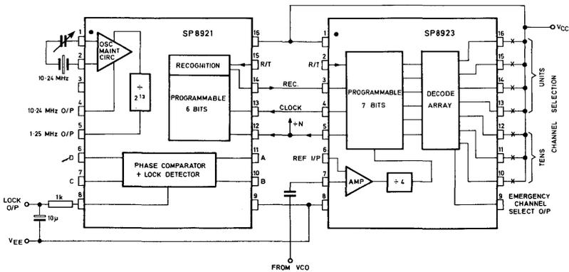
Fig. 3 SP8921/SP8923 interconnections (10.695MHz receive offset)
