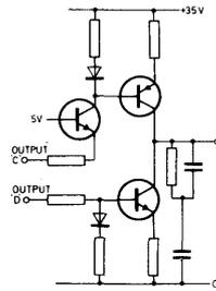
Fig. 6 High voltage charge pump and filter
