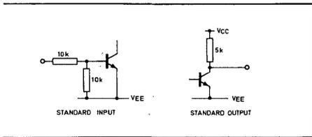
Fig. 11 Standard input and output
