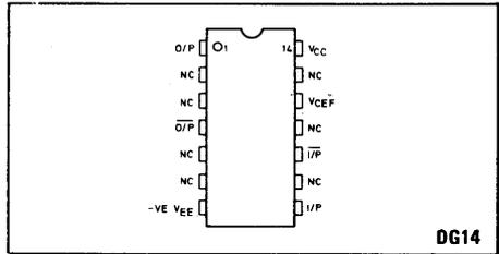
Fig. 1 Pin connections
