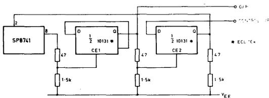
Fig. 6 Divide-by-12/14. Control loop delay time approximately 40ns.
