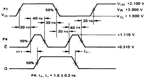
FIGURE 3 – PROPAGATION DELAY ( $t_{pd}$ ) versus INPUT PULSE AMPLITUDE AND CONSTANT OVERDRIVE
