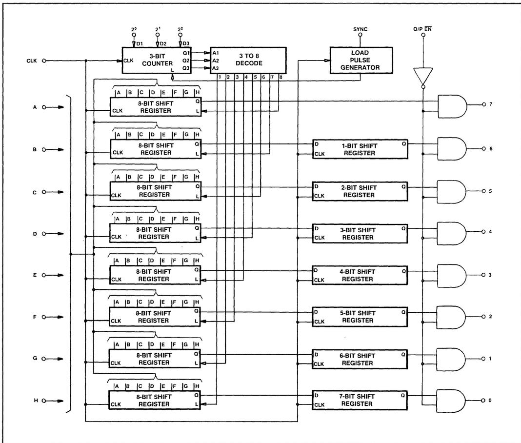
Fig.2 Block diagram
