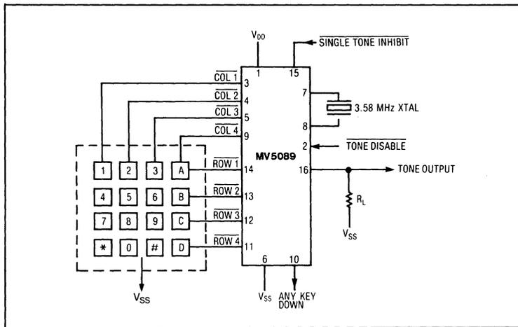
Fig.7 connection diagram
