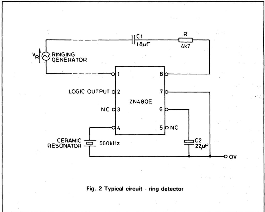
Fig. 2 Typical circuit - ring detector
