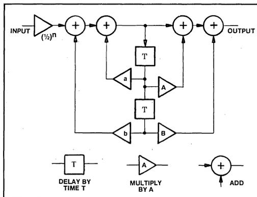
Fig.3 Basic 2nd order filter section
