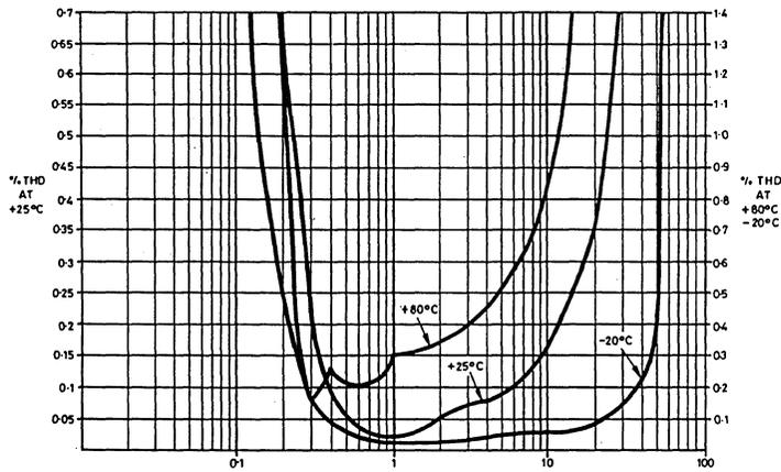
Fig.7 Total harmonic distortion v current (ZN482Z)
