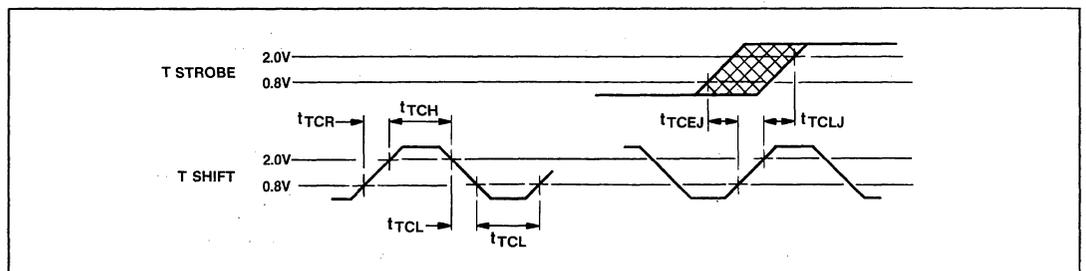
Fig.12 Timing - receive clock
