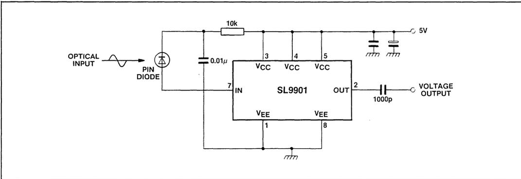
Fig.5 Typical application circuit
