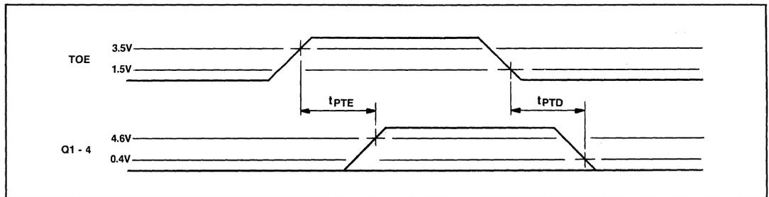
Fig.15 Timing - output enable and disable
