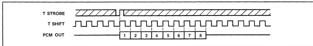
Fig.4 Transmit alignment
