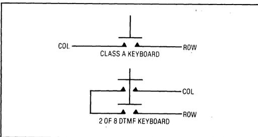
Fig.3 Keyboard configuration
