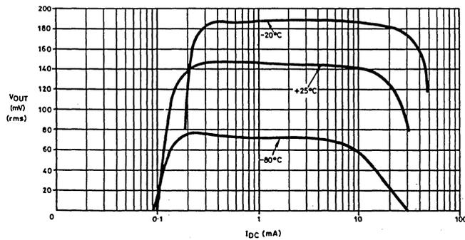
Fig.8 Output voltage v current at 2% THD (ZN482Z)
