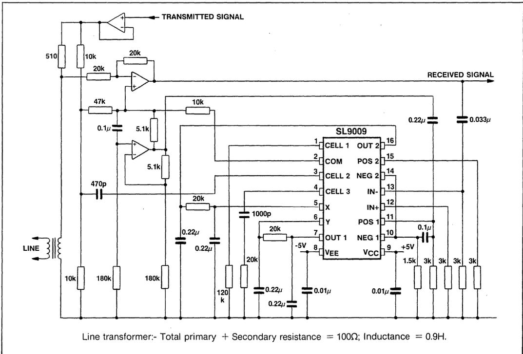
Fig.9 Complete circuit
