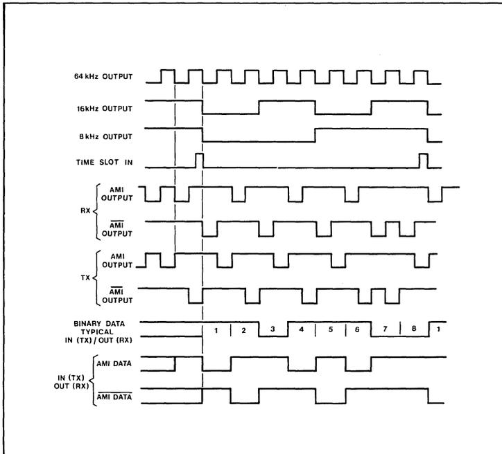
Fig.4 64kBit/s operation
