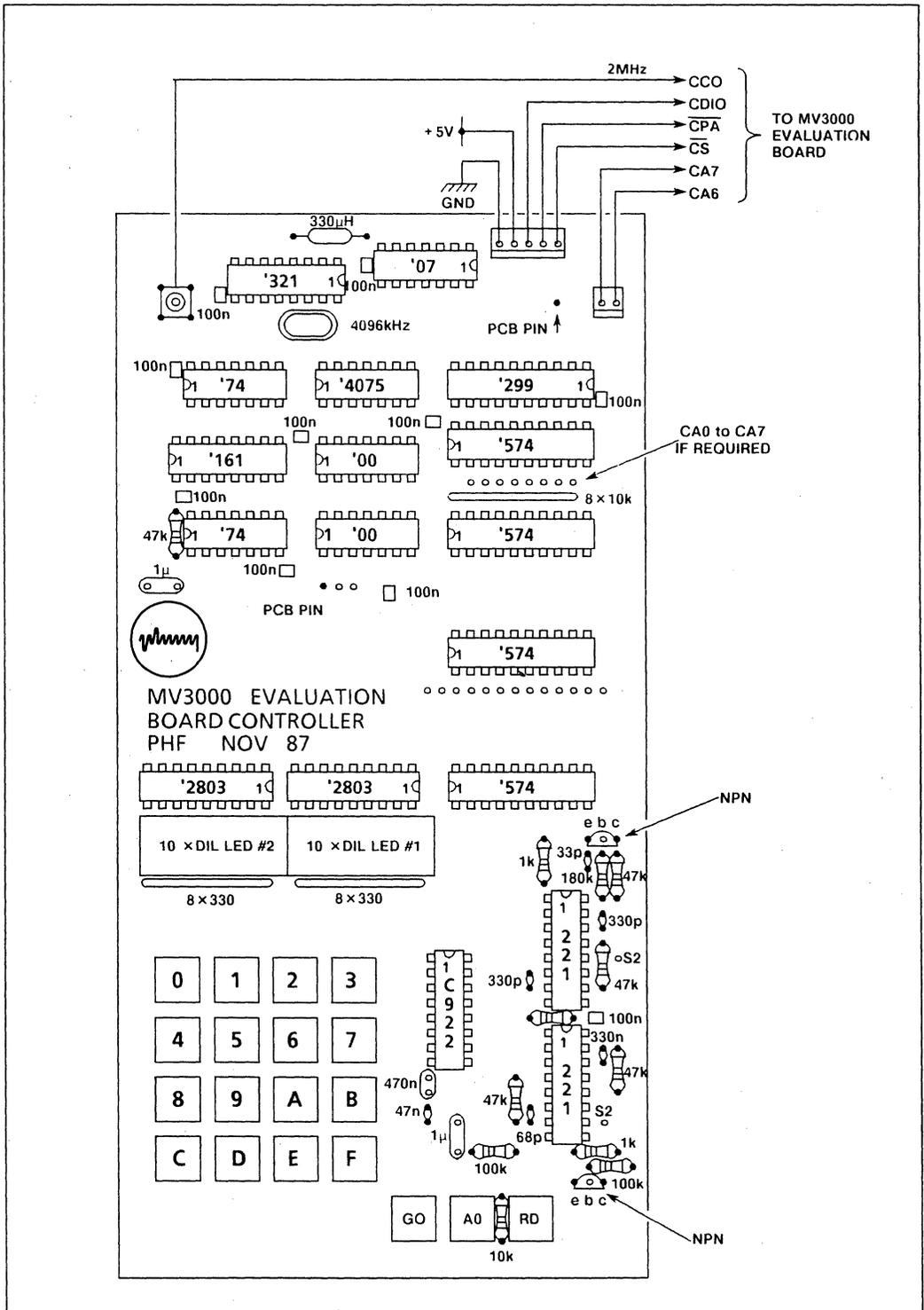
Fig.5 Controller PCB component layout
