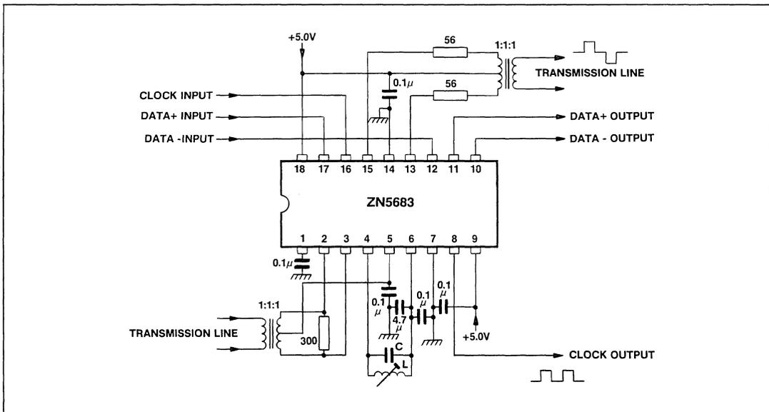
Fig.4 Recommended circuit
