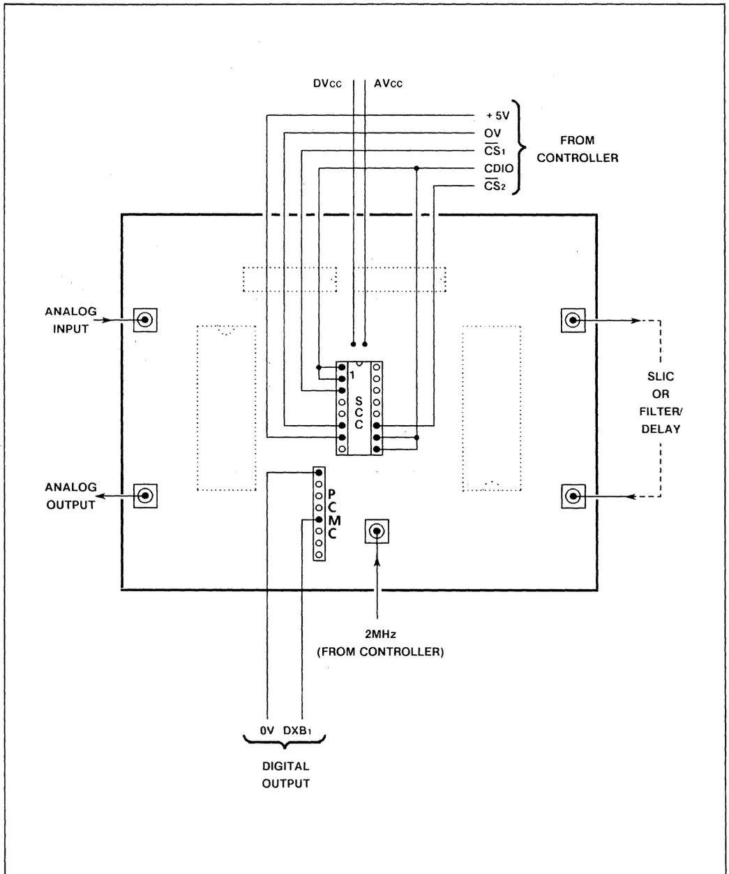
Fig.3 MV3000 evaluation board, test set-up 4
