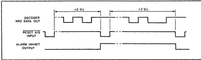
Fig. 6 AIS error and reset waveforms
