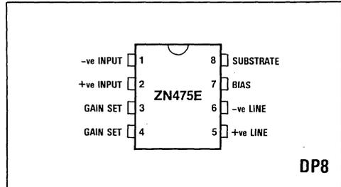
Pin connections - top view
