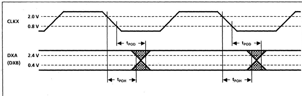
Fig. 26 Timing - PCM output changing during burst (see Fig. 4)
