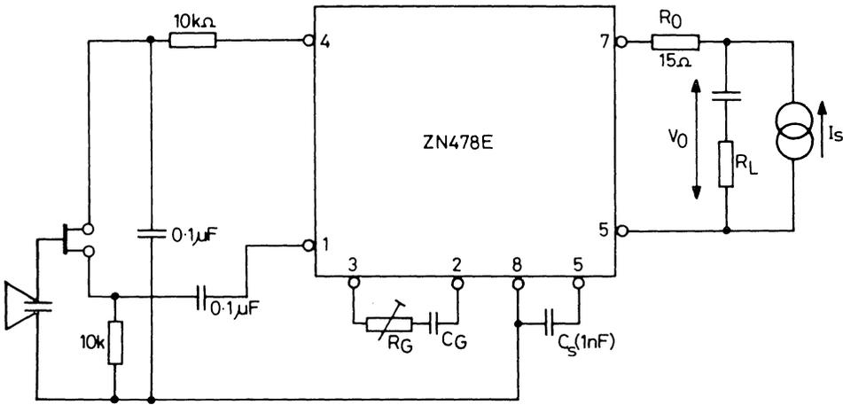
Fig. 2 Typical Application Circuit
