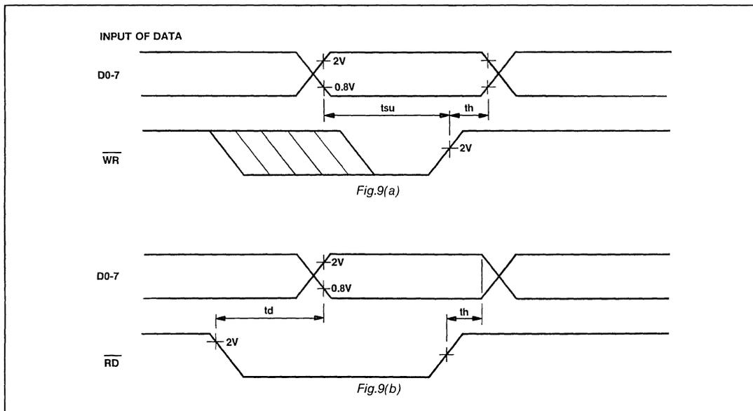
Fig.9 Register timing
