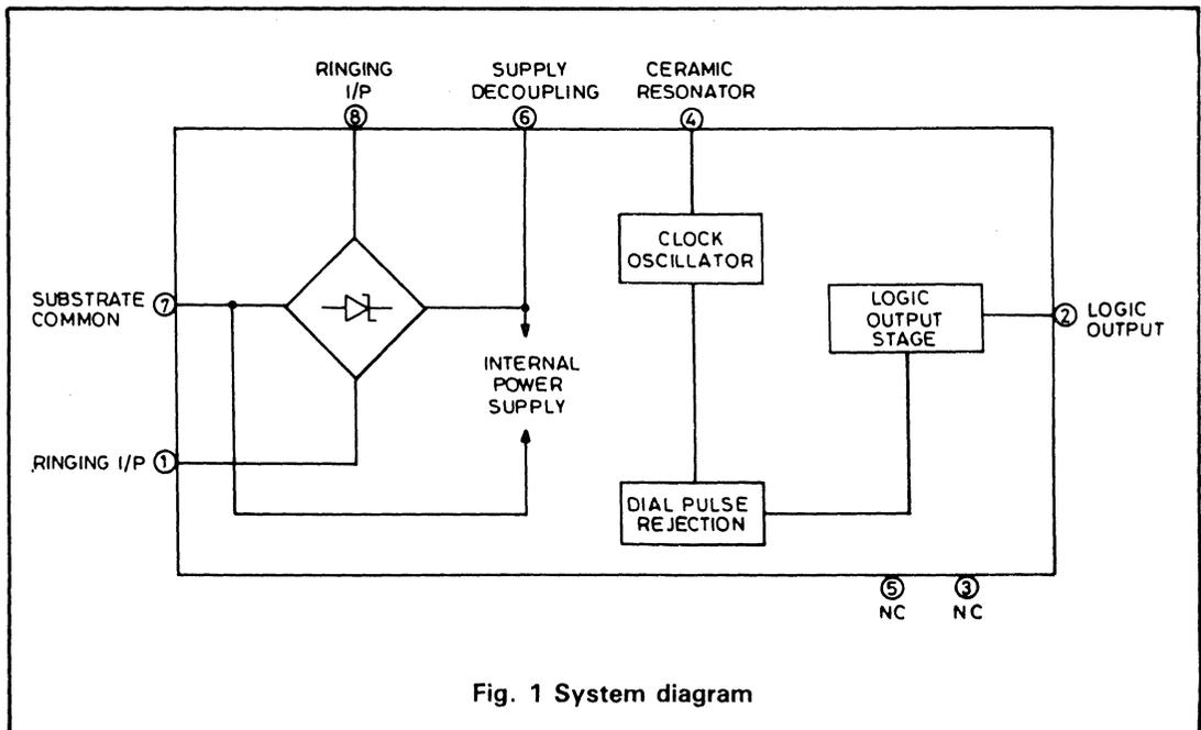
Fig. 1 System diagram
