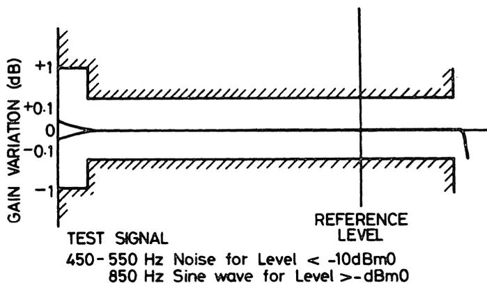
Fig. 8(b). Gain to Signal Level, 'A law'
