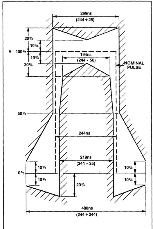
Fig.3 Input signal pulse mask
