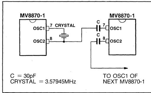
Fig.10 Oscillator circuit
