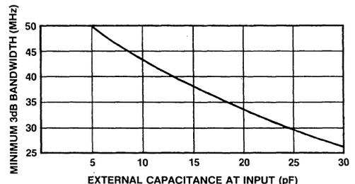
Fig.3 Minimum 3dB bandwidth against external capacitance at input
