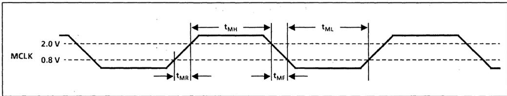
Fig. 22 Timing - master clock
