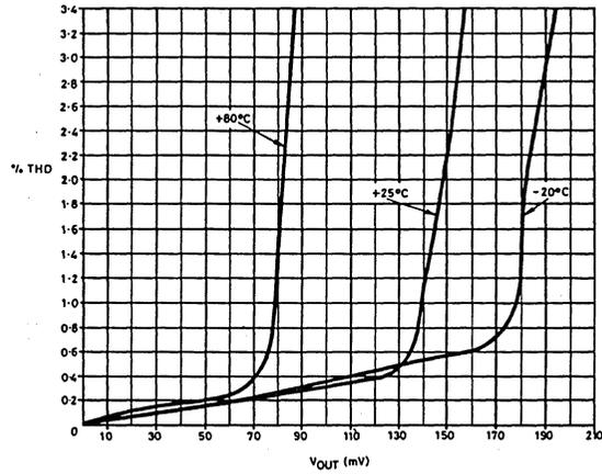
Fig.6 Distortion v output voltage (ZN482Z)
