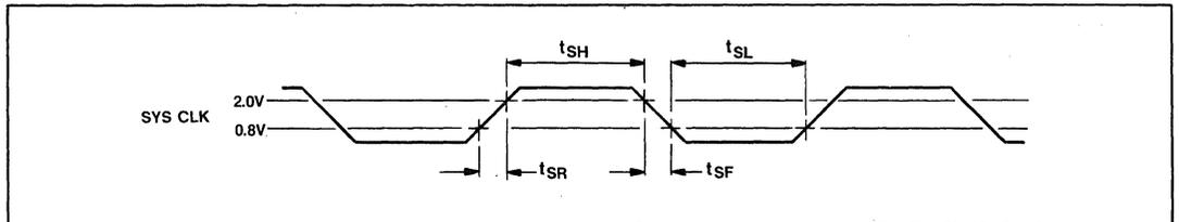
Fig.7 Timing - system clock
