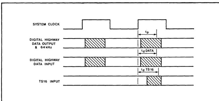
Fig.5 Timing diagram
