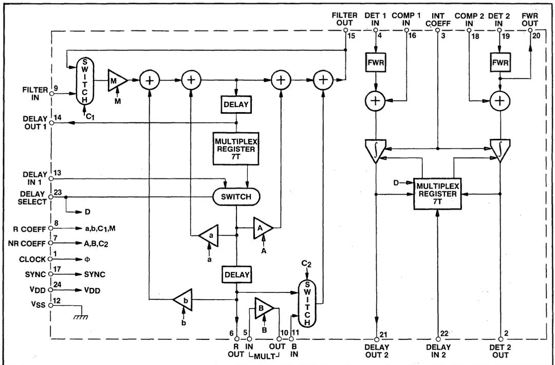
Fig.2 Block diagram
