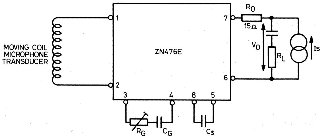
Fig. 2 Typical Application Circuit
