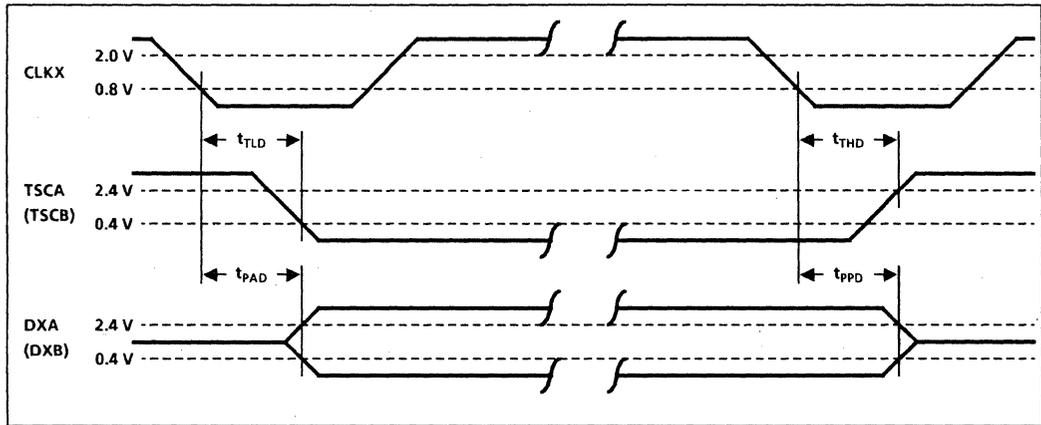
Fig. 25 Timing - PCM Output Start and Stop of Burst (see Fig. 4)
