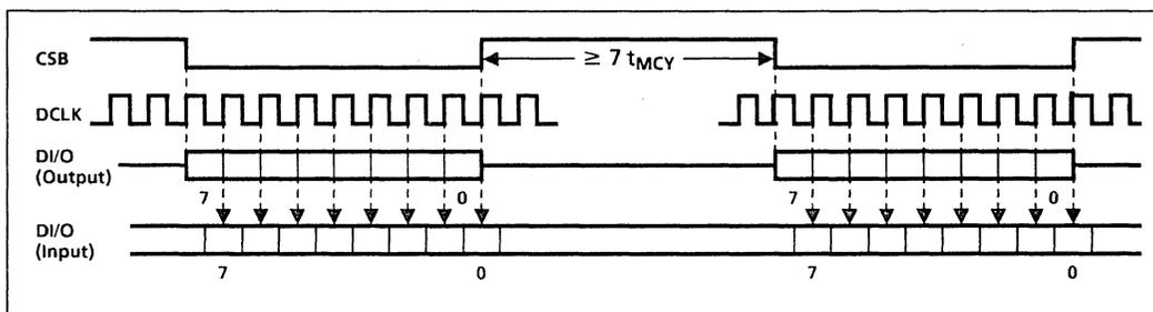
Fig. 9 Control timing diagram - normal operation
