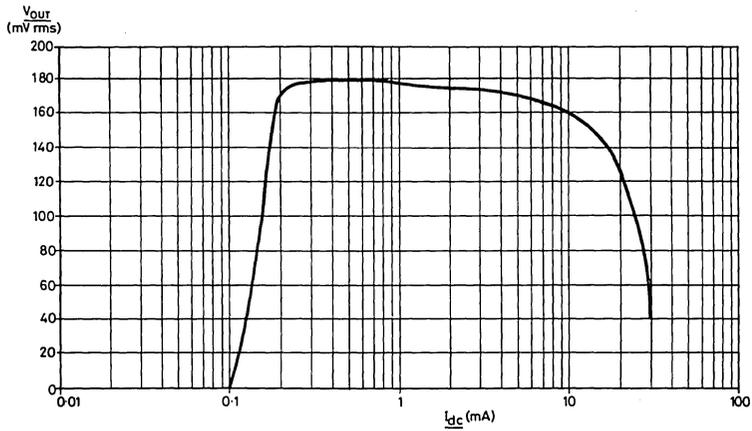
Fig.16 Output voltage v current at 2% THD (ZN483Z)
