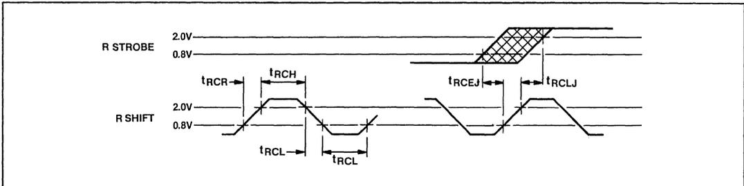
Fig.9 Timing - receive clock
