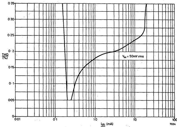
Fig.15 Total harmonic distortion v current (ZN483Z)
