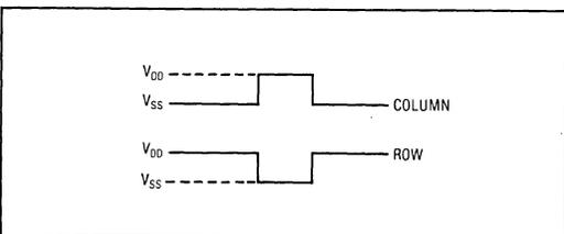
Fig.4 Electronic input
