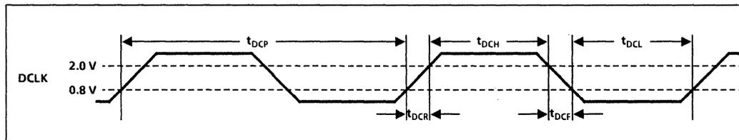
Fig. 28 Timing - PCM clocks
