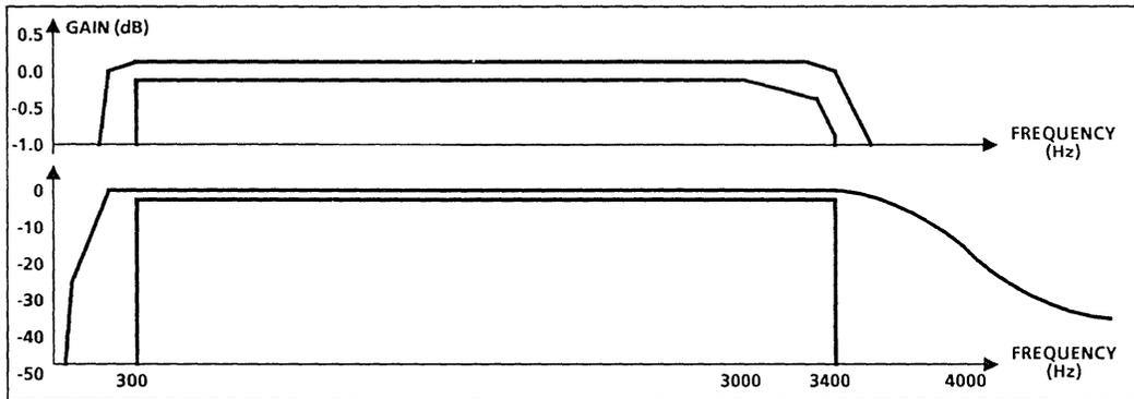
Fig. 33 Transmit channel gain
