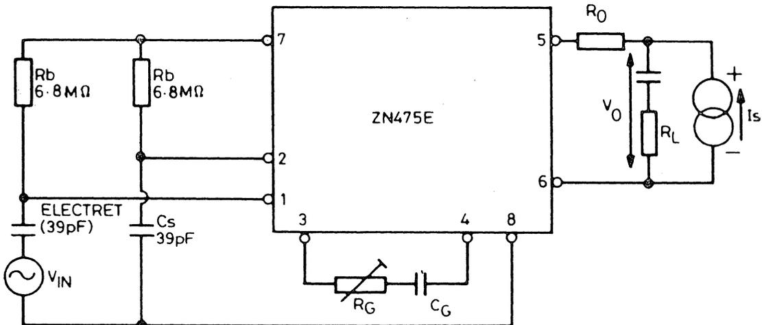
Fig. 2 Typical Electret Microphone Amplifier
