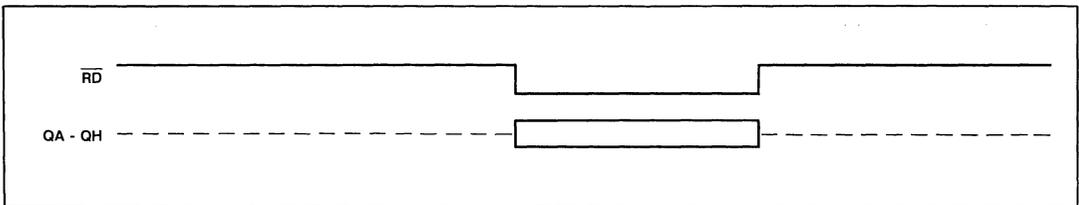
Fig.2(c) Microprocessor read
