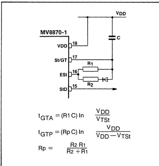
Fig.8 Guard time adjustment ( $t_{GTP} > t_{GTA}$ )
