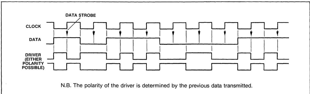
N.B. The polarity of the driver is determined by the previous data transmitted.
