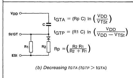
Fig.8 Guard time adjustment
