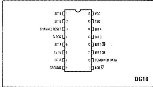
Fig.1 Pin connections
