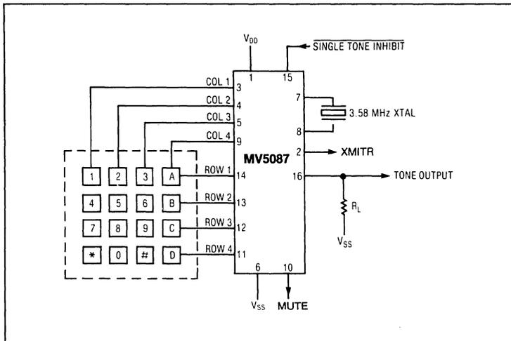
Fig.7 Connection diagram
