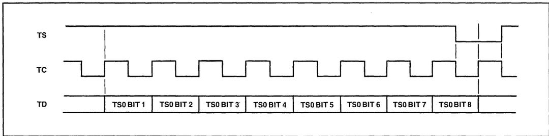
Fig.3 Transmit signal alignment
