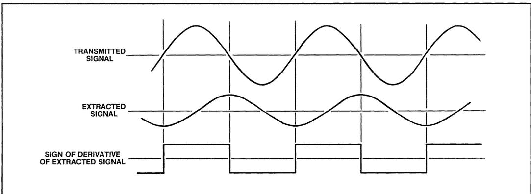
Fig.6 Signal relationship for 90° of lag on extracted signal
