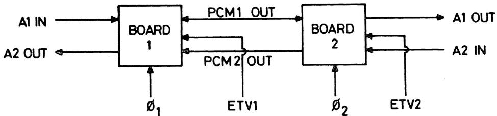
$\phi_1$  and  $\phi_2$  must be the same frequency and ETV1 and ETV2 can be common or up to 30 clock periods displaced.
