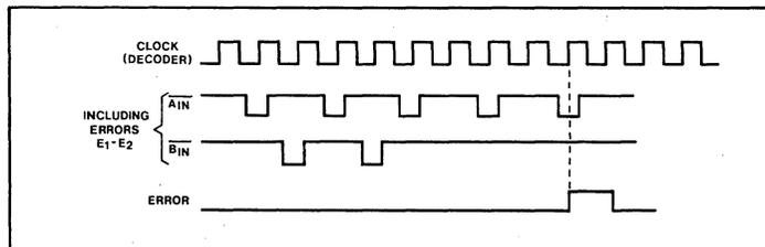
Fig. 5 HDB3 error output waveforms
