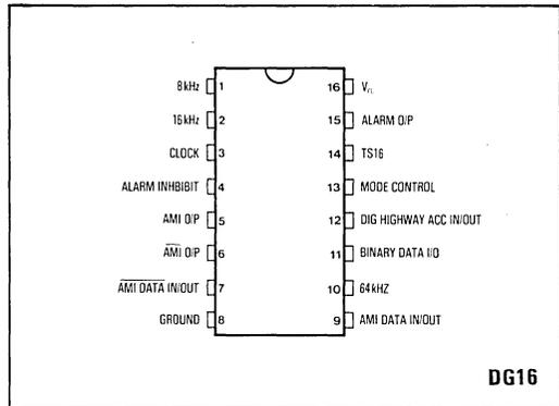
Fig.1 Pin connections
