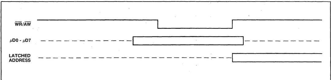
Fig.2(b) Microprocessor write
