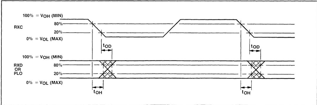
Fig.10 Timing - receive data and phase lock out
