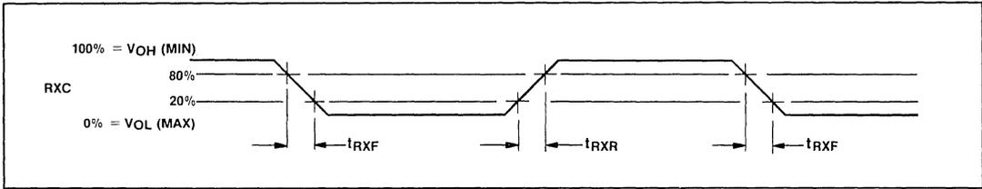
Fig.9 Timing - receive clock
