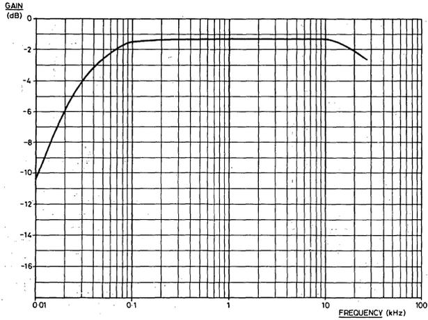
Fig.13 Gain v frequency (ZN483Z)
