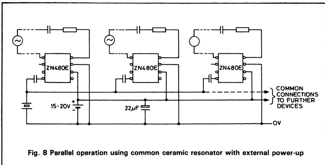
**Fig. 8 Parallel operation using common ceramic resonator with external power-up**
