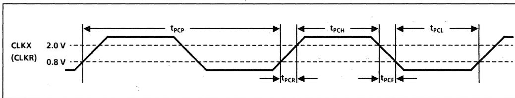
Fig. 23 Timing - PCM clocks
