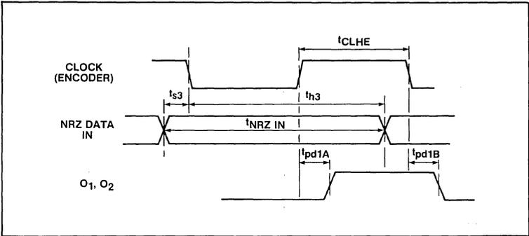
Fig.8 Encoder timing relationship
