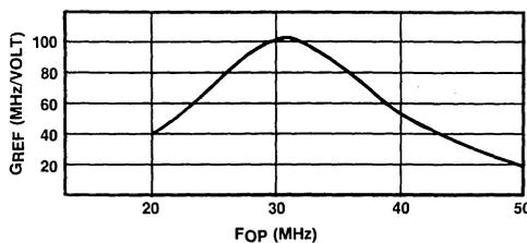
Fig.7 Typical reference loop gain characteristic
