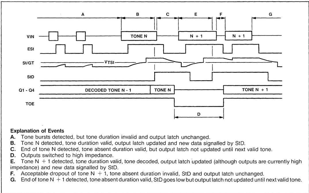
Fig.5 Timing diagram
