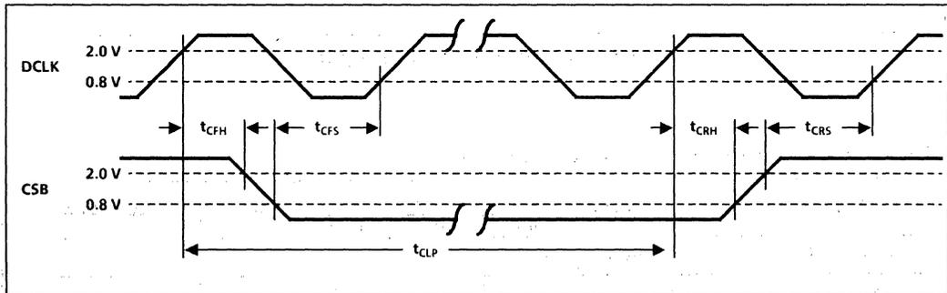
Fig. 29 Timing - chip select (see Fig. 9)
