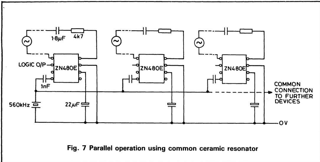
**Fig. 7 Parallel operation using common ceramic resonator**
