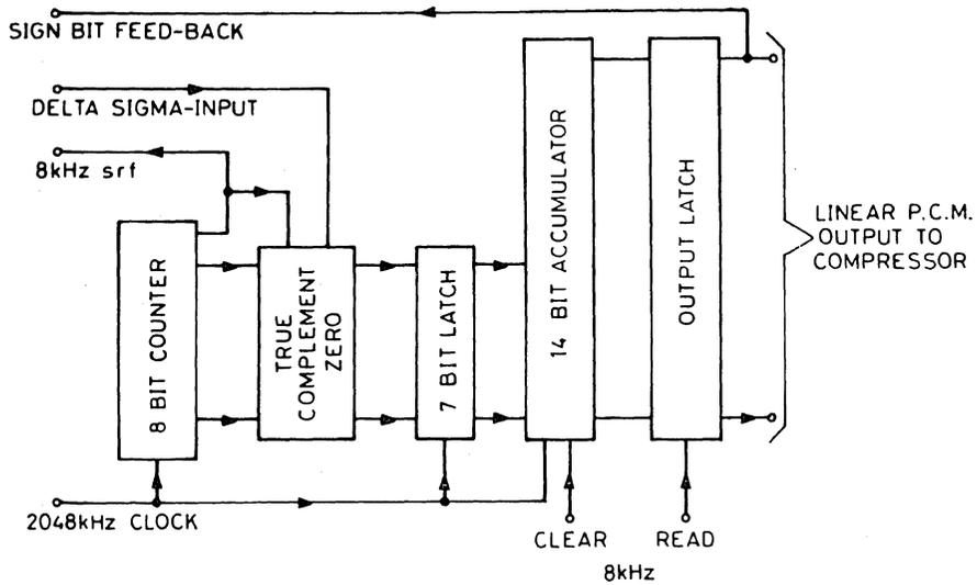
Fig. 5. Delta sigma to Linear pcm Converter
