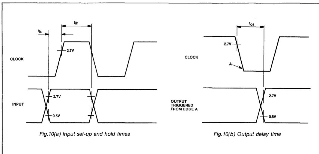
Fig.10(a) Input set-up and hold times
