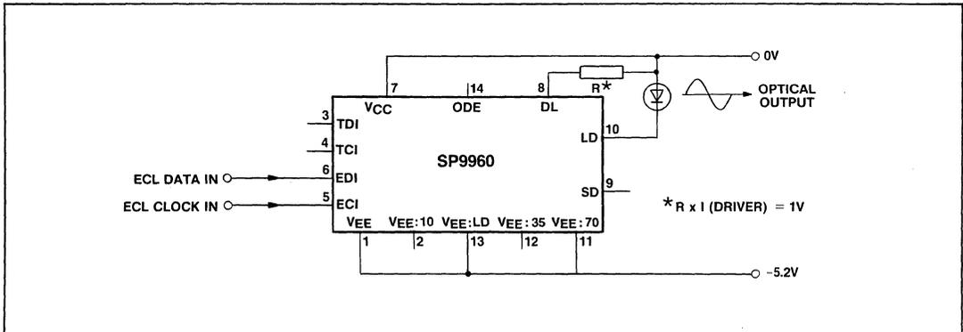
Fig.6 Typical ECL application circuit - large driver at 115mA (nominal) chosen **NB** For TTL applications the TTL inputs should be used,  $V_{CC}$  should be 5V and  $V_{EE}$  should be 0V (DG package pin out)
