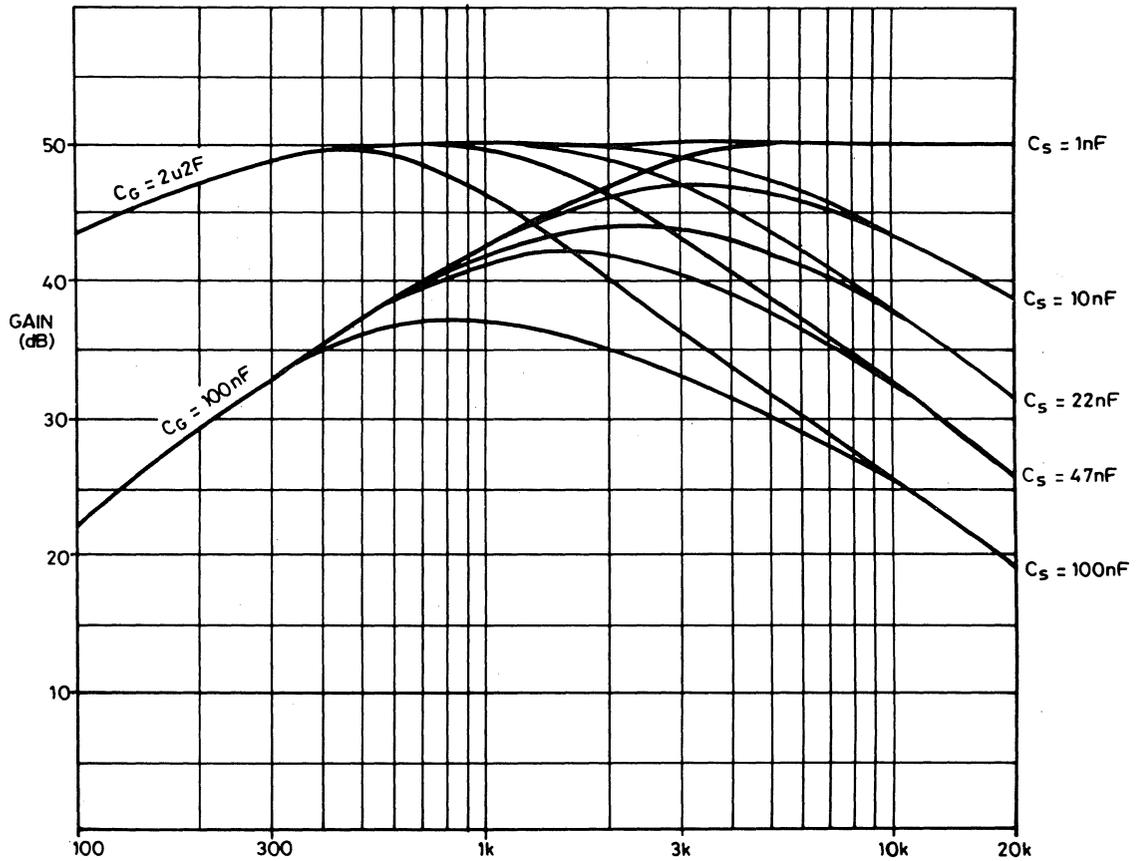
Gain (dB) vs Frequency (Hz)
