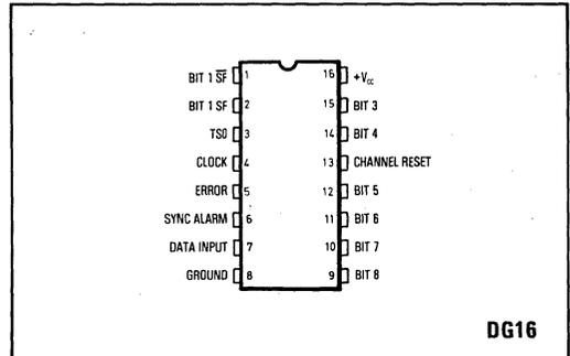
Fig.1 Pin connections
