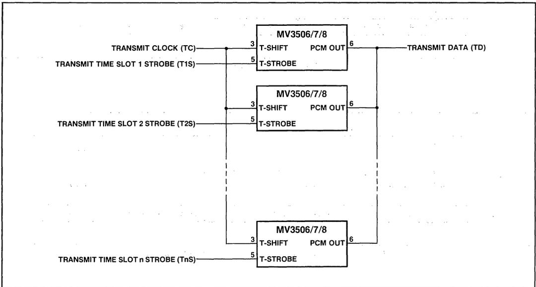
Fig.5 Transmit data from Codecs
