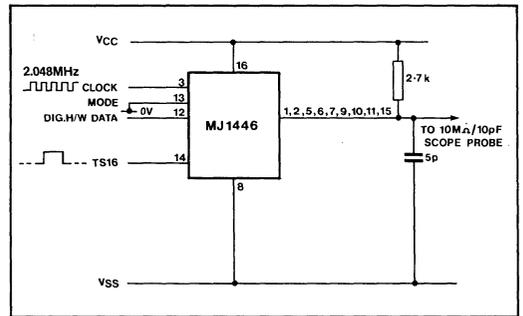
Fig.8 Test conditions (receive mode)
