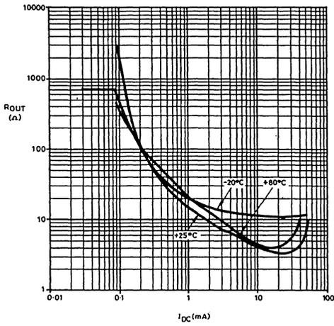
Fig.9 Output resistance v current (ZN482Z)
