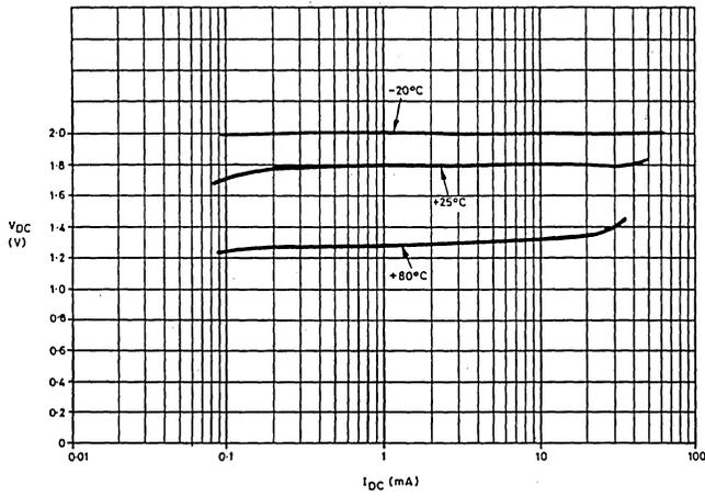
Fig.3 DC voltage v current (ZN482Z)
