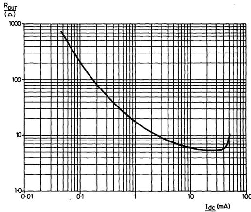
Fig.17 Output resistance v current (ZN483Z)
