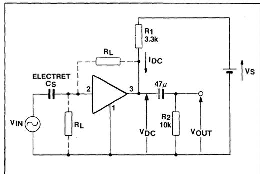
Fig.2 Typical buffer amplifier application circuit
