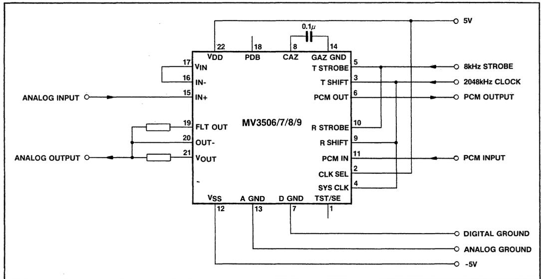
Fig.14 Simple application circuit
