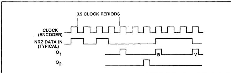
Fig.3 Encode waveforms
