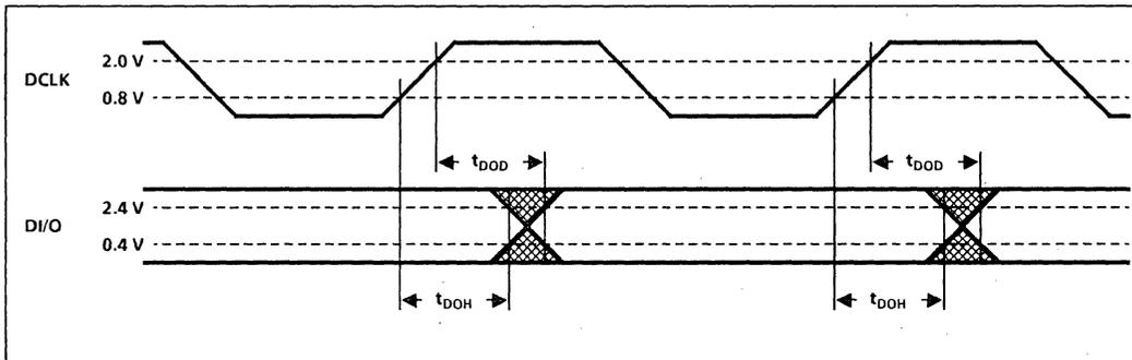
Fig. 32 Timing - data output changing during burst (see Fig. 9)
