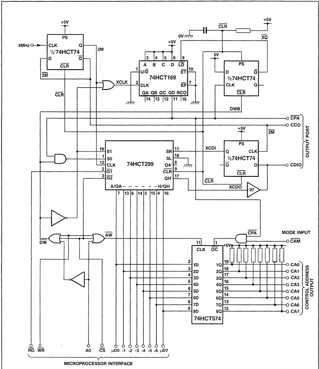
Fig.1 Line card controller logic diagram
