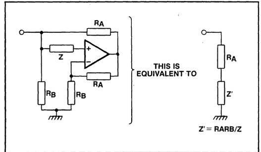
Fig.7 Gyrator circuit
