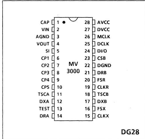
Fig. 1 Pin Connection - top view
