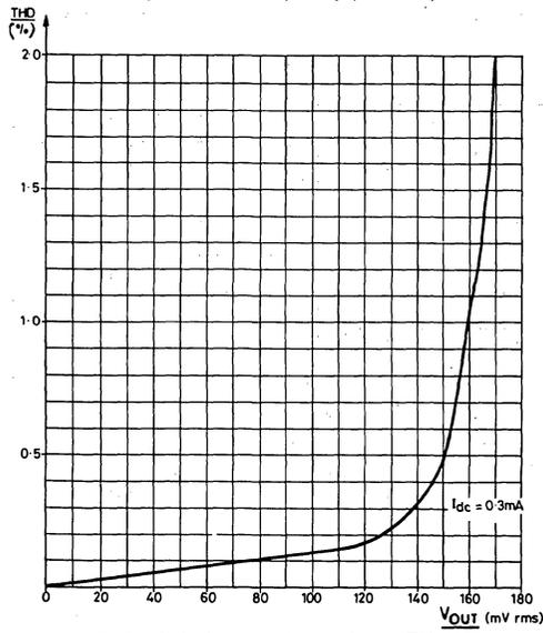
Fig.14 Distortion v output voltage (ZN483Z)
