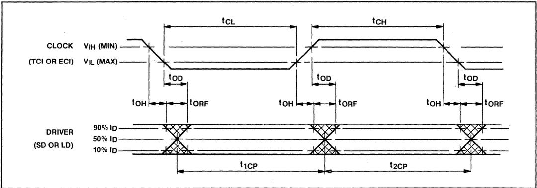
Fig.5 Digital switching characteristics - output
