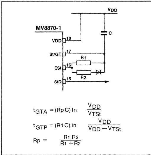
Fig.7 Guard time adjustment ( $t_{GTP} < t_{GTA}$ )
