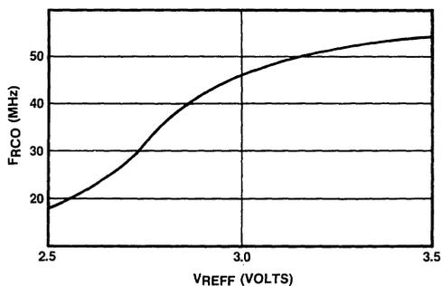
Fig.6 Typical reference VCO characteristic
