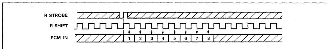
Fig.6 Receive alignment
