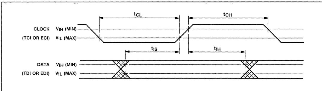
Fig.4 Digital switching characteristics - input
