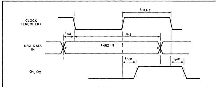
Fig. 8 Encoder timing relationship
