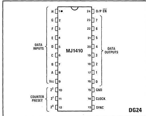
Fig.1 Pin connections
