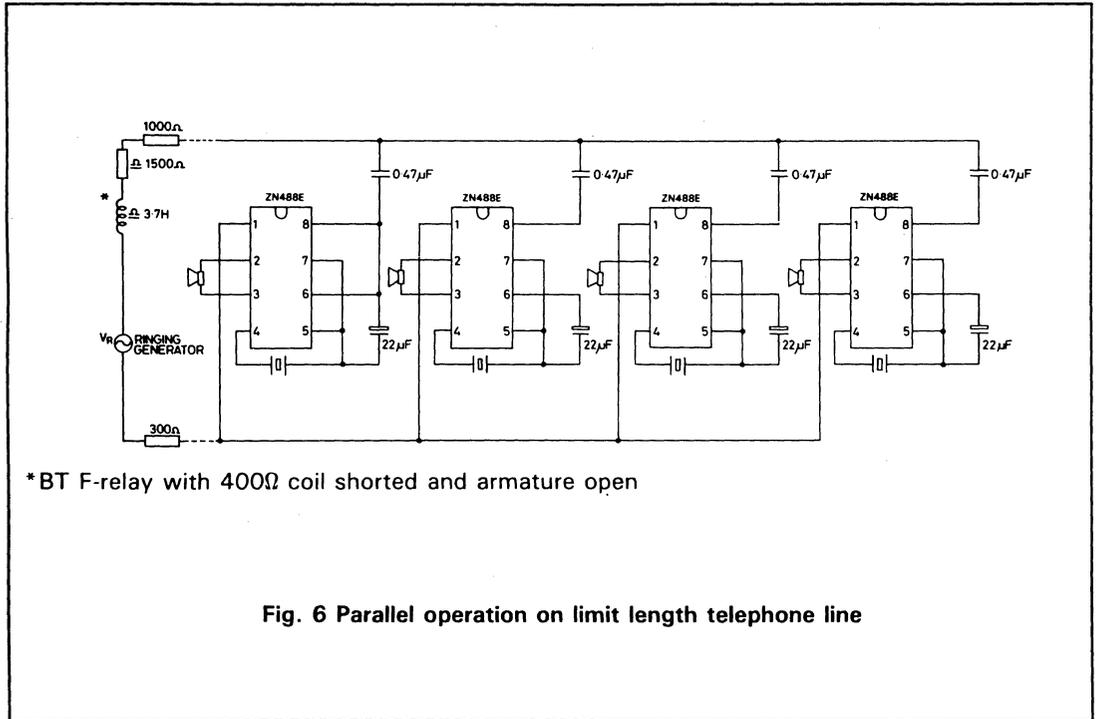
Fig. 6 Parallel operation on limit length telephone line
