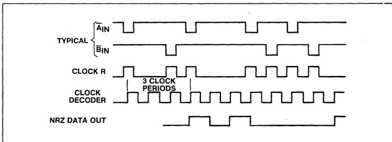
Fig.4 Decode waveforms
