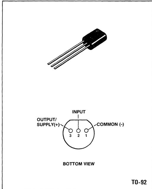
Fig.1 Pin connections
