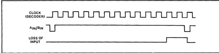
Fig. 7 Loss of input waveforms
