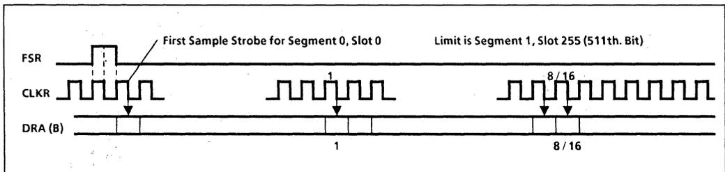
Fig. 3 Receive timing diagram
