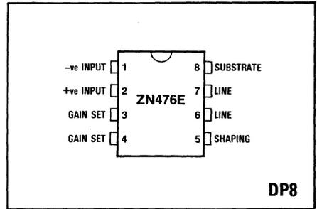
Pin connections - top view
