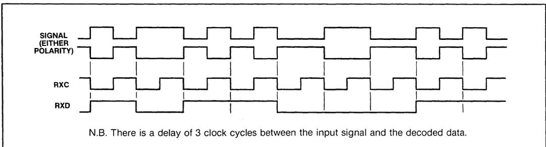
Fig.3 Biphase-mark decoding
