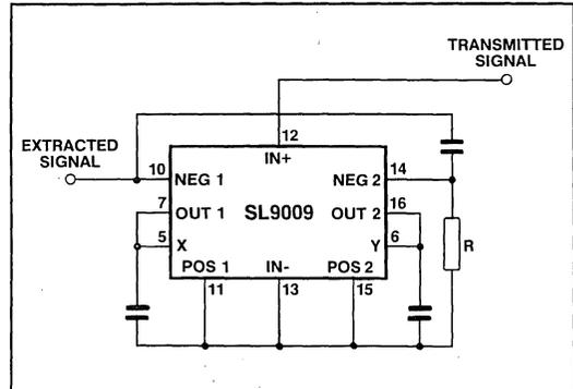
Fig.5 Feedback arrangement
