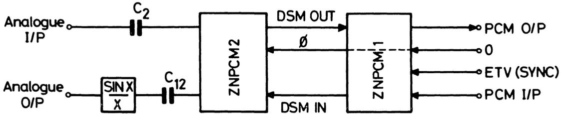
Single Channel Codec System Operating in Internal Mode (PCM at 64K bits/sec. without ADI).
