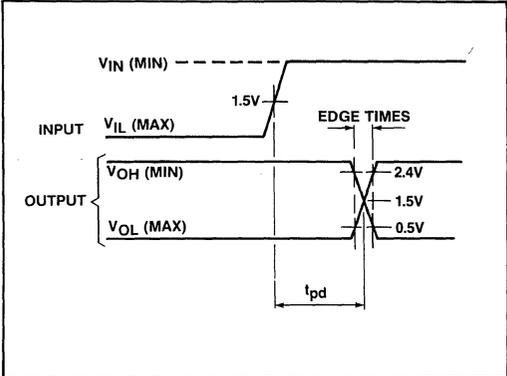
Fig.15 Test timing definitions
