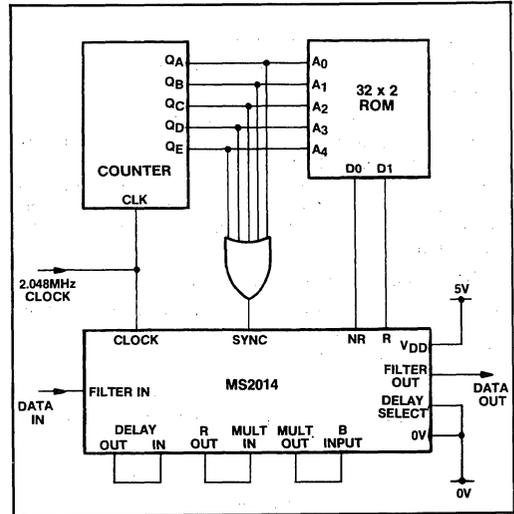
Fig.8 2nd order 32kHz bandwidth filter
