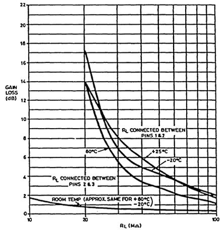
Fig.10 Gain leakage loss v leakage resistance (ZN482Z)
