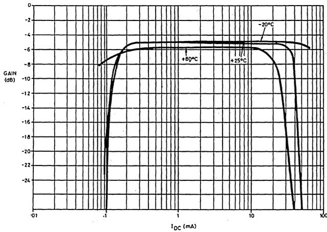
Fig.4 Gain v current (ZN482Z)
