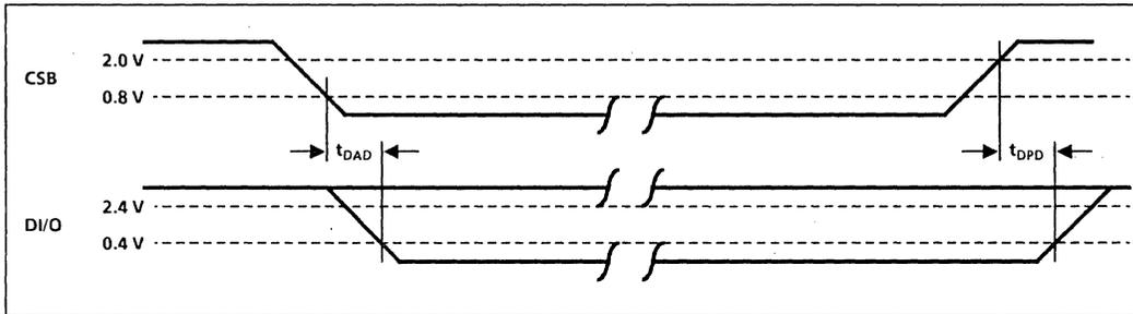
Fig. 31 Timing - data output start and stop of burst (see Fig. 9)
