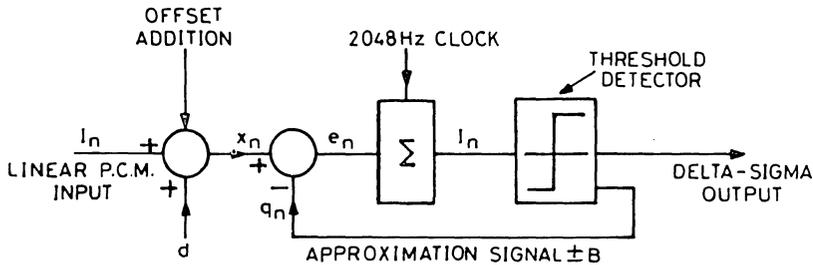
Fig. 9. The Digital DSM
