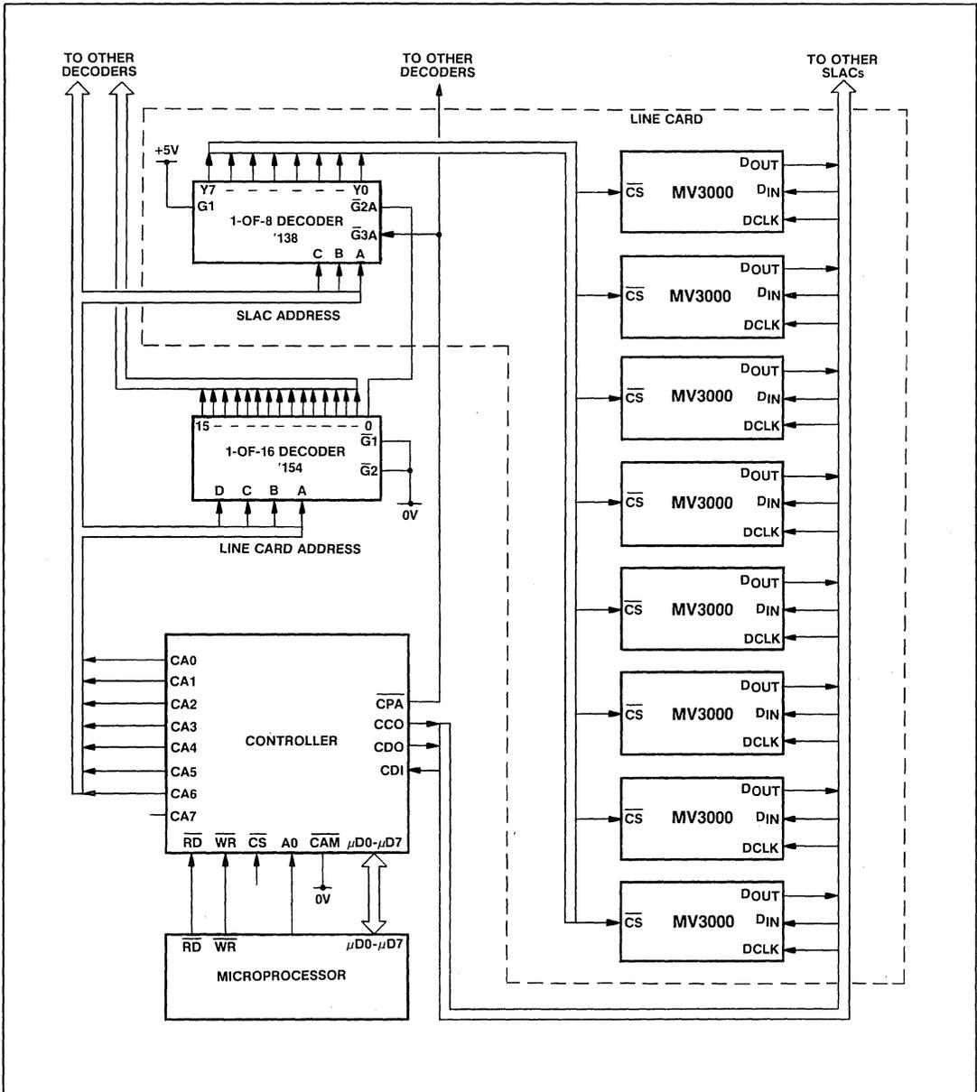
Fig.4  $\overline{CAM} = 0$  mode/PABX application
