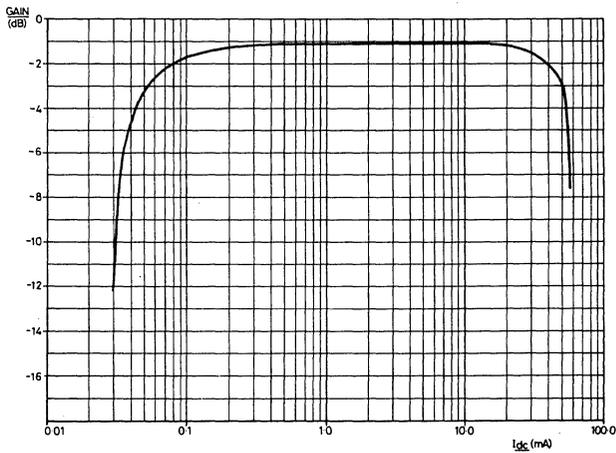
Fig.12 Gain v current (ZN483Z)
