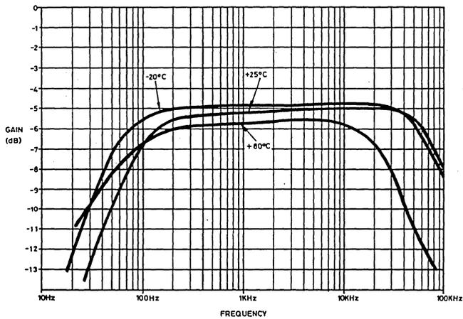
Fig.5 Gain v frequency (ZN482Z)
