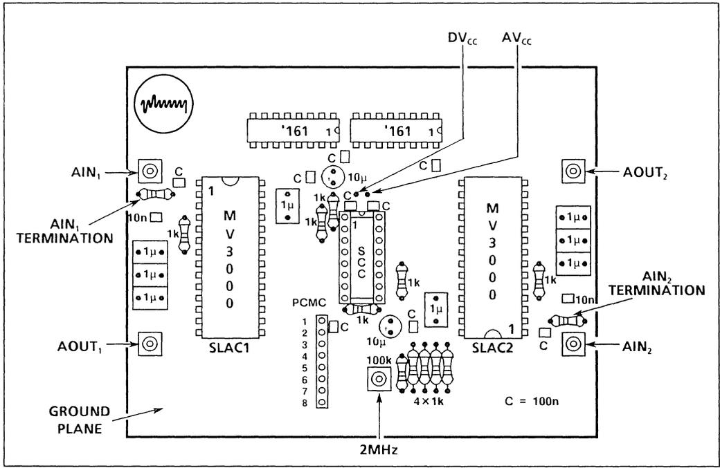
Fig.2 MV3000 evaluation board, component layout
