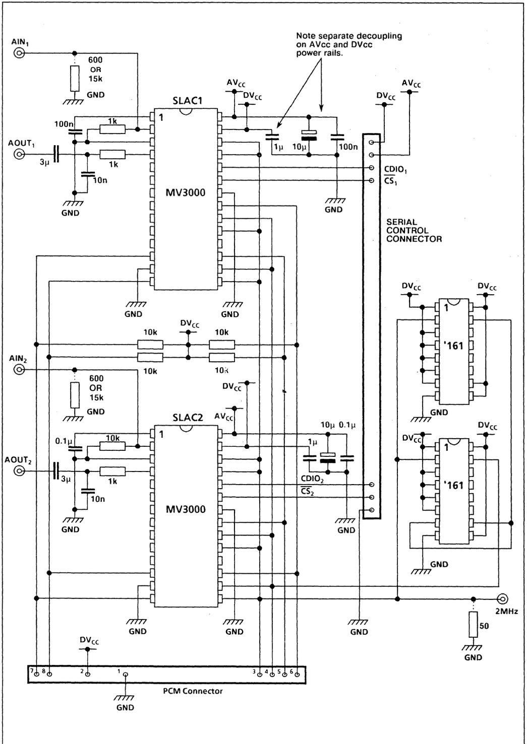
Fig.1 MV3000 evaluation board circuit diagram
