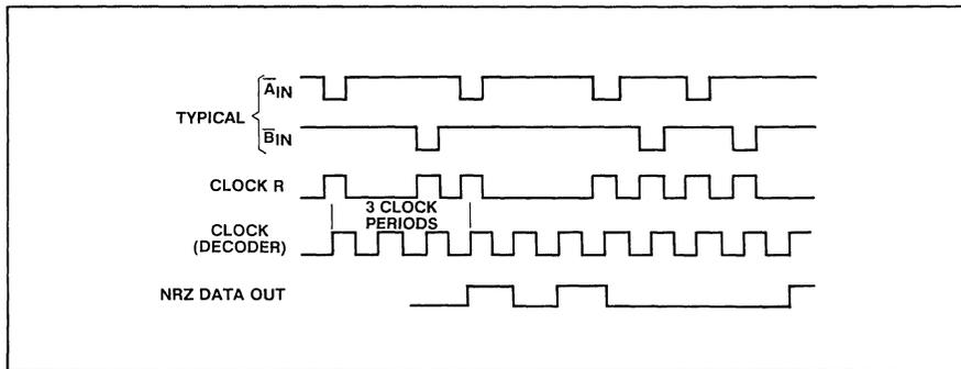
Fig. 3 Decode waveforms
