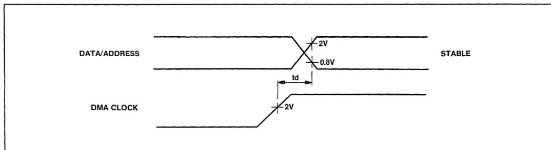
Fig.10 DMA timing
