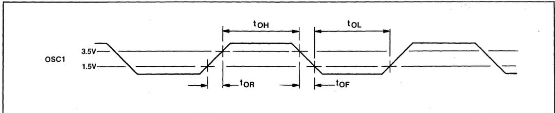
Fig.13 Timing - external oscillator input
