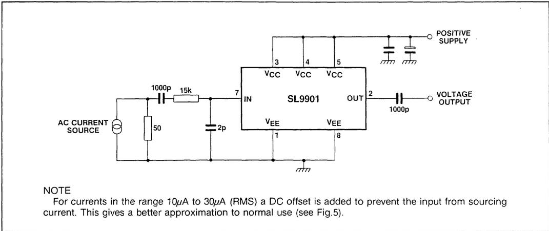
Fig.4 Test circuit
