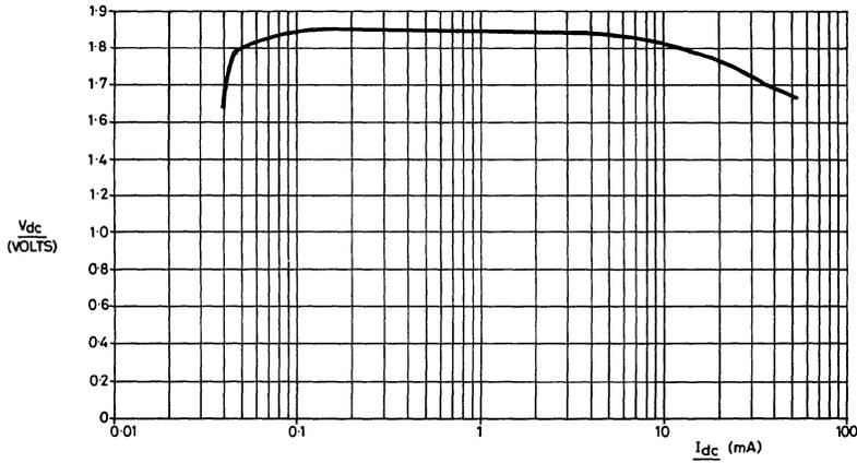
Fig.11 DC voltage v current (ZN483Z)
