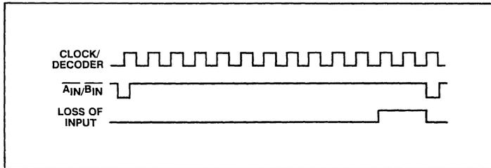
Fig.9 Loss of input waveforms
