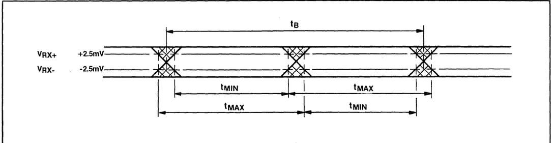
Fig.8 Timing - receive data
