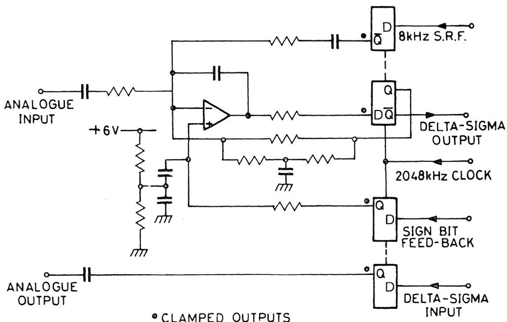
Fig. 2. Modulator/Demodulator Circuit
