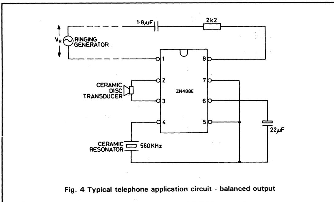
Fig. 4 Typical telephone application circuit - balanced output
