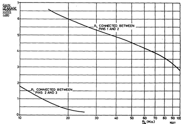
Fig.18 Gain leakage loss v leakage resistance (ZN483Z)
