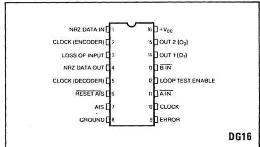
Fig. 1 Pin connections
