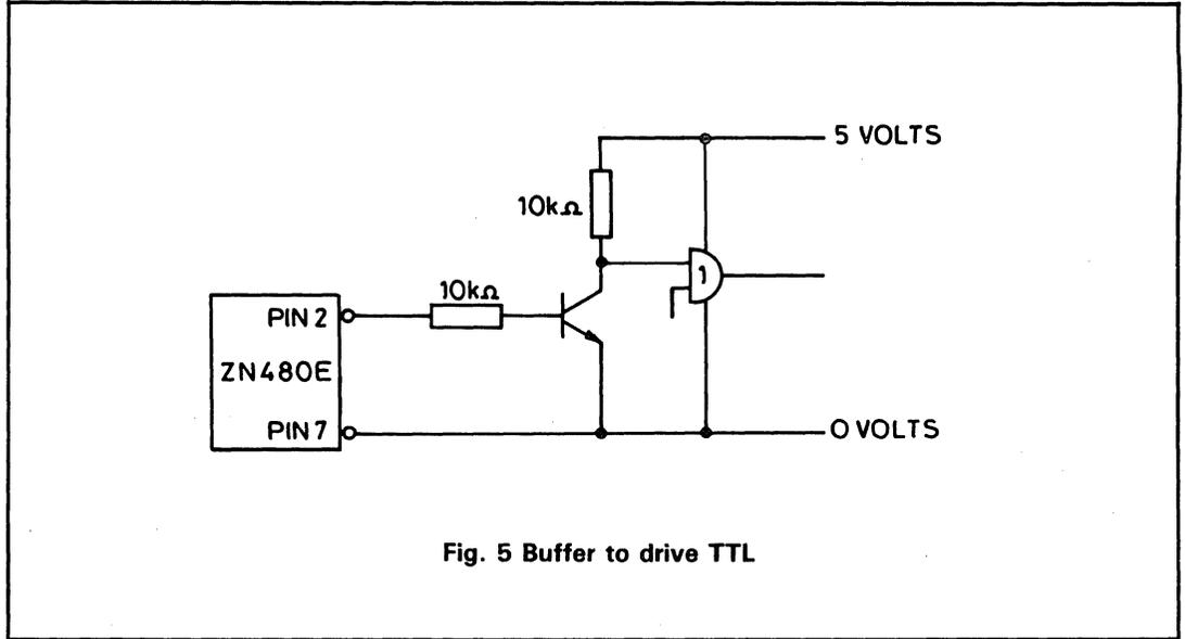
**Fig. 5 Buffer to drive TTL**
