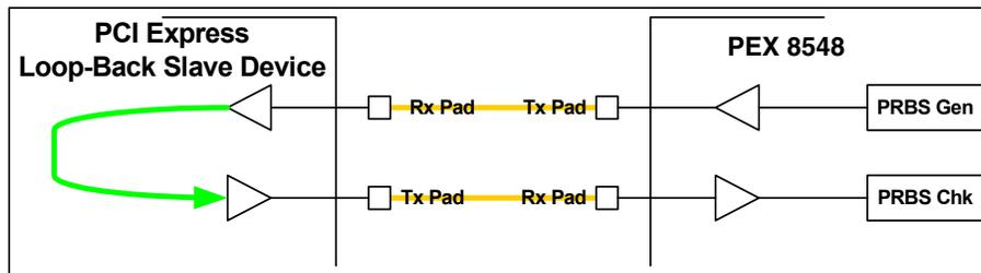
**Figure 15-3. Cable Loopback**
