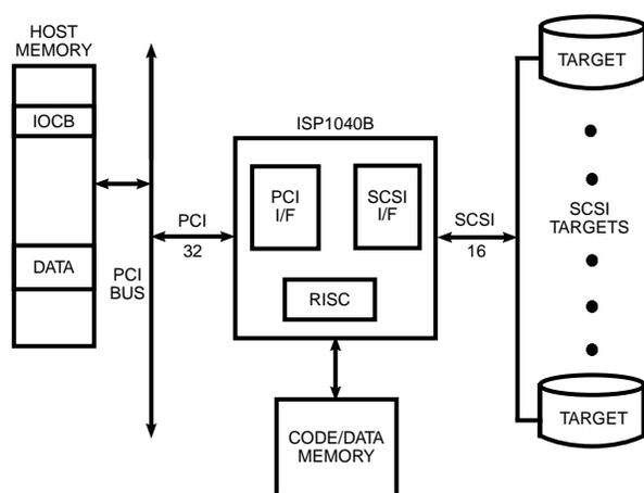
**Figure 2. I/O Subsystem Design Using the ISP1040B**
