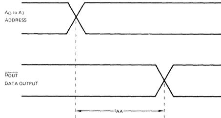
(ALL TIME MEASUREMENTS REFERENCED TO 1.5 V)
