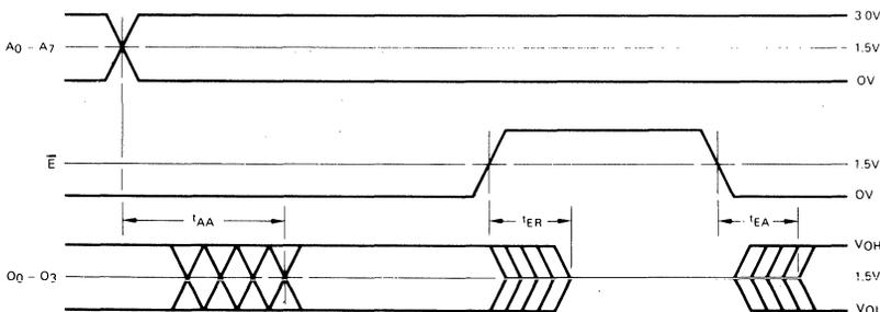
Note: Level on output while E is HIGH is determined externally.
