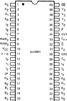
Note: Pin 1 is marked for orientation.
