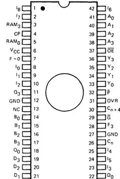
Note: Both grounds (pins 12 and 27) must be connected.
