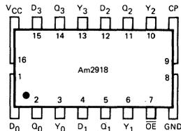
Note: Pin 1 is marked for orientation.
