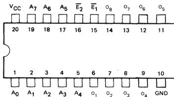
Note: Pin 1 is marked for orientation.
