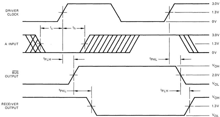
Note: Bus to Receiver output delay is measured by clocking data into the driver register and measuring the BUS to R combinatorial delay.
