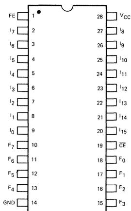
Note: Pin 1 is marked for orientation.
