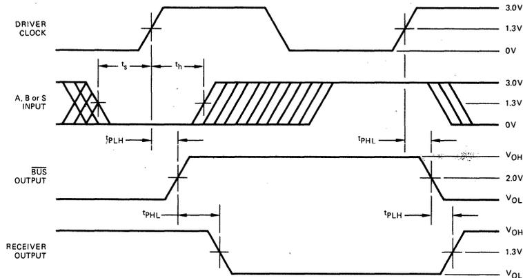
Note: Bus to Receiver output delay is measured by clocking data into the driver register and measuring the  $\overline{\text{BUS}}$  to R combinatorial delay.
