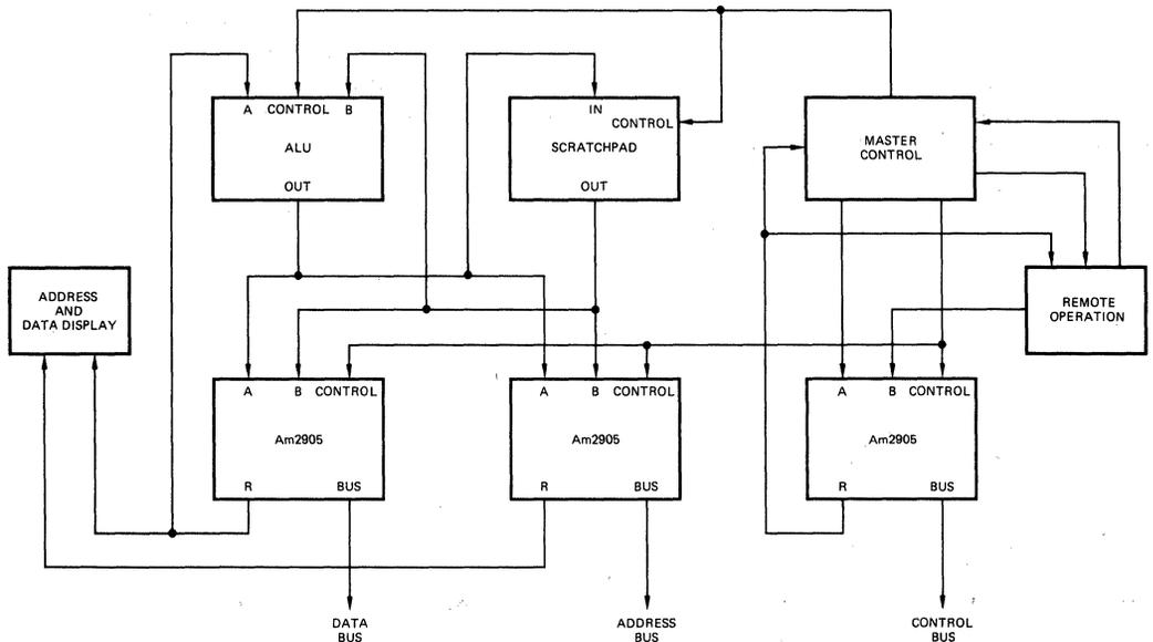
The Am2905 is a universal Bus Transceiver useful for many system data, address, control and timing input/output interfaces.
