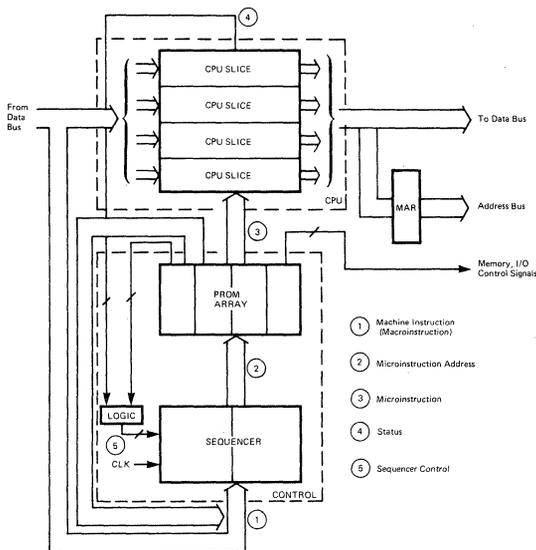
Figure 2. Typical Bit-Slice Implementation for CPU and Control.
