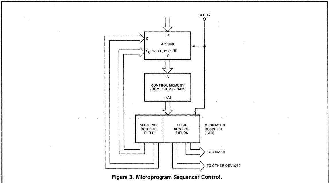
Figure 3. Microprogram Sequencer Control.
