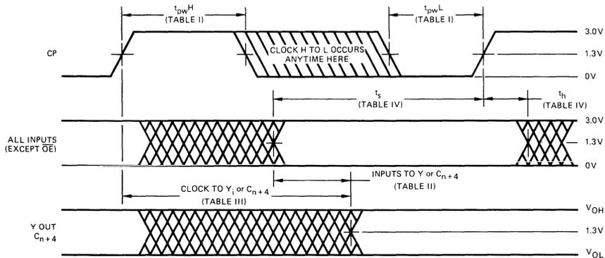
Figure 1. Switching Waveforms. See Tables for Specific Values.
