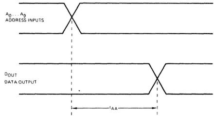
(All time measurements referenced to 1.5 V)
