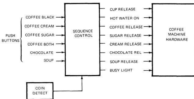
Figure 1. Coffee Machine Block Diagram.
