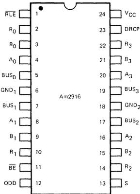
Note: Pin 1 is marked for orientation.
