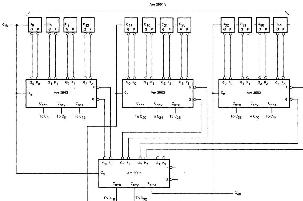
Figure 18. Carry Lookahead Scheme for 48-Bit CPU using 12 Am2901's. The Carry-Out Flag (C<sub>48</sub>) Should be Taken from the Lower Am2902 Rather than the Right-Most Am2901 for Higher Speed.
