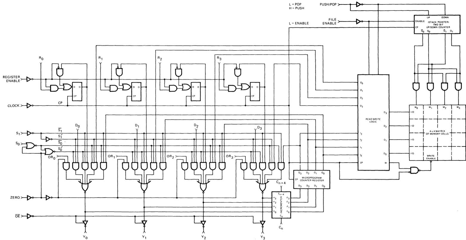
Note:  $R_i$  and  $D_i$  connected together on Am2911 and  $OR_i$  removed.
