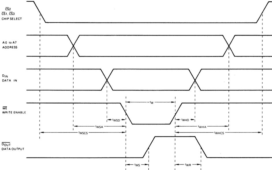
(ALL TIME MEASUREMENTS REFERENCED TO 1.5 V)
