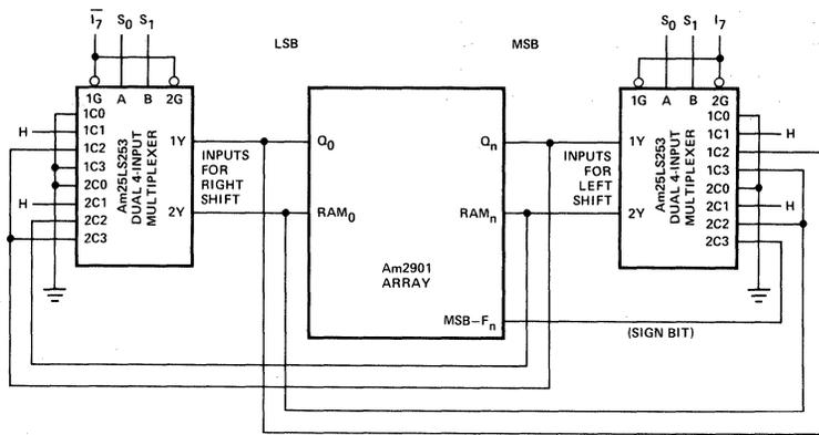
Figure 19. Three-State Multiplexers Used on Shift I/O Lines.
