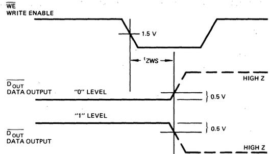
(All  $t_{ZXXX}$  parameters are measured at a delta of 0.5 V from the logic level and using Load C.)
