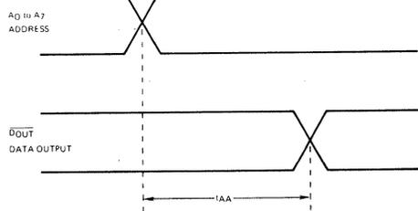
(ALL TIME MEASUREMENTS REFERENCED TO 1.5 V)
