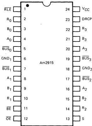
Note: Pin 1 is marked for orientation.
