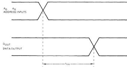
(ALL TIME MEASUREMENTS REFERENCED TO 1.5 V)
