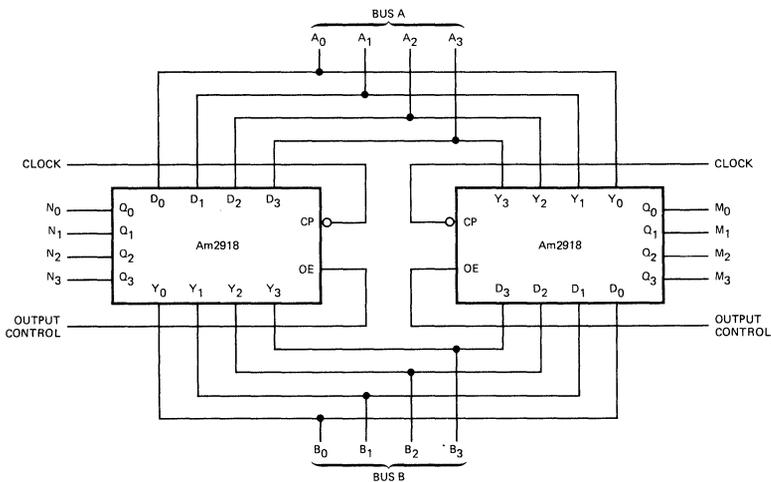
The Am2918 can be connected for bi-directional interface between two buses. The device on the left stores data from the A-bus and drives the A-bus. The device on the right stores data from the B-bus and drives the A-bus. The output control is used to place either or both drivers in the high-impedance state. The contents of each register are available for continuous usage at the N and M ports of the device.
