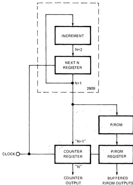
Figure 11. 2909 Pipelined System.
