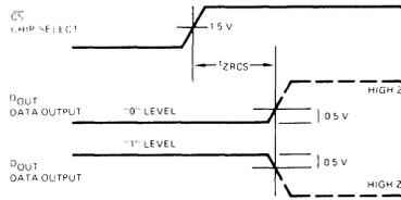
(All  $t_{zxxx}$  parameters are measured at a delta of 0.5 V from the logic level and using Load C.)
