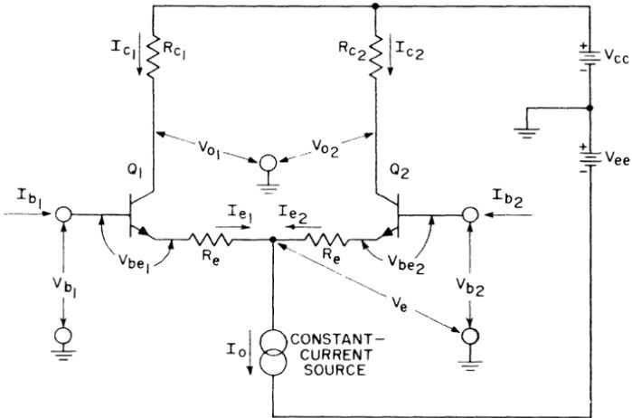
Fig. 23 — Schematic of the basic differential amplifier in which emitter degeneration is employed.
