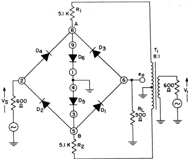
Fig. 291 — Series-shunt gate using the CA3019.
