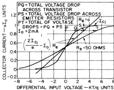
Fig. 24 — Effect of emitter degeneration on the transfer characteristics of the basic differential amplifier.
