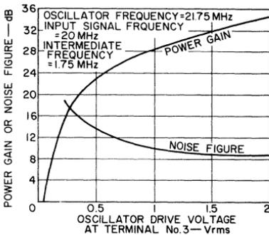
Fig. 191 — Power gain and noise figure as a function of oscillator drive voltage for the CA3005 or CA3006 balanced mixer.
