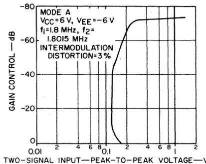
Fig. 112 — Third-order intermodulation characteristics of the CA3002 as a function of agc.
