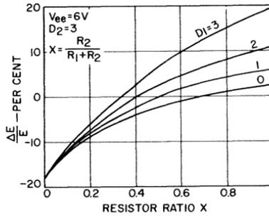
Fig. 45 — Effect of the number of diodes  $D_1$  on the variations in the voltage  $E$  as a function of the ratio  $X$  for a temperature increase of  $100^\circ\text{C}$  and a supply voltage  $V_{ee}$  of 6 volts when three diodes  $D_2$  are used.
