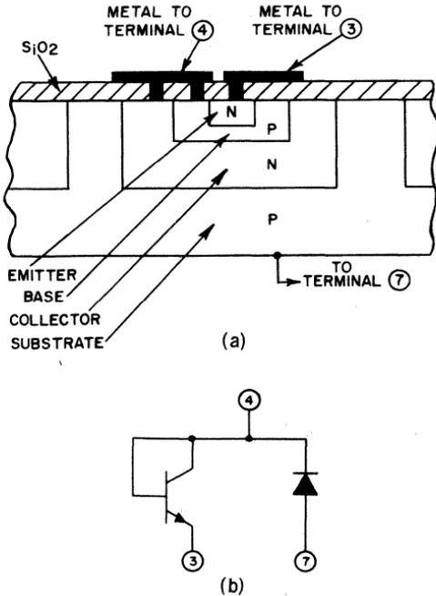
Fig. 284 — Diagram and equivalent circuit of the monolithic array.
