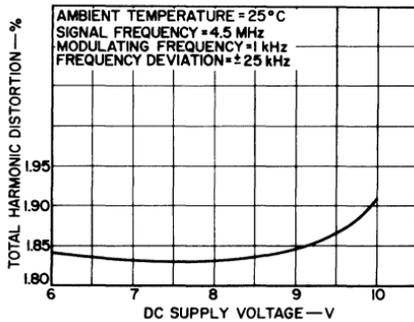
Fig. 260 — Total harmonic distortion as a function of dc supply voltage.
