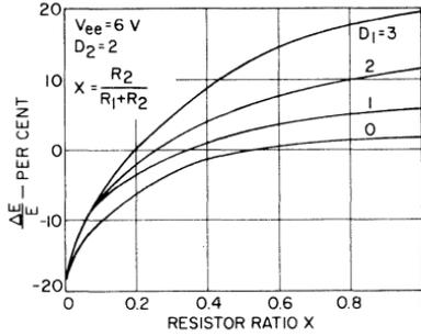
Fig. 43 — Effect of the number of diodes  $D_1$  on the variations in the voltage  $E$  as a function of the ratio  $X$  for a temperature increase of  $100^\circ\text{C}$  and a supply voltage  $V_{ee}$  of 6 volts when two diodes  $D_2$  are used.
