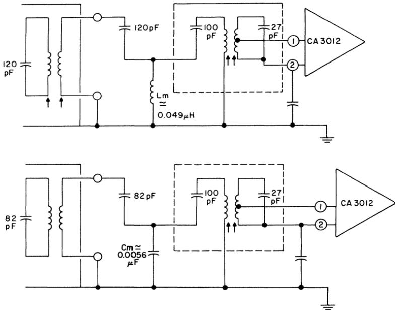
Fig. 267 — Configurations of two quadruple-tuned interstage filters.
