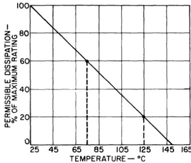
Fig. 240 — Temperature derating curve for the CA3020.
