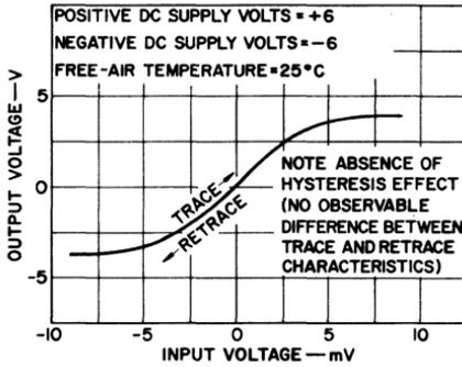
Fig. 202 — Output voltage as a function of input voltage for an open-loop operational amplifier.
