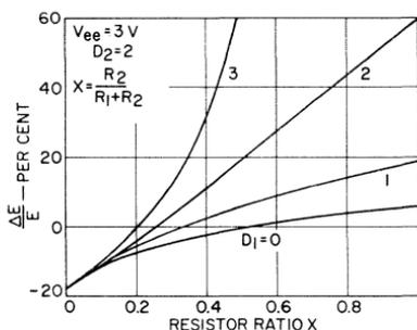
Fig. 42 — Effect of the number of diodes  $D_1$  on the variation in the voltage  $E$  as a function of the ratio  $X$  for a temperature increase of  $100^\circ\text{C}$  and a supply voltage  $V_{ee}$  of 3 volts when two diodes  $D_2$  are used.
