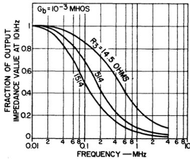
Fig. 53 — Effect of the emitter resistor ( $R_s$ ) of the current-sink transistor on the change in output impedance with frequency.
