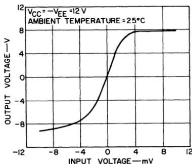
Fig. 226 — Open-loop transfer characteristics.
