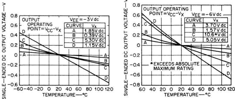
Fig. 73 — Theoretical curves of dc output voltage as a function of temperature for negative-supply voltages of -3 and -6 volts (calculated for  $\beta = 35$  at  $20^\circ C$ ).
