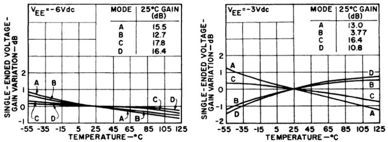
Fig. 95 — Voltage gain of the CA3001 (normalized to the 25°C gain) as a function of temperature for  $V_{EE}$  supplies of  $-3$  and  $-6$  volts.
