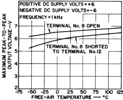
Fig. 205 — Output-swing capabilities as a function of temperature.
