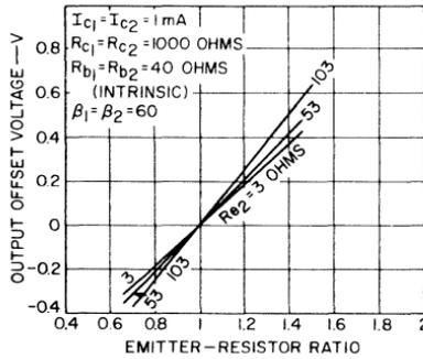
Fig. 34 — Effect of absolute values and ratios of the emitter resistors of the differential pair of transistors on the output offset voltage.
