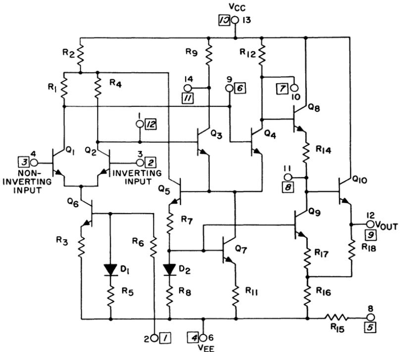
Fig. 197 — Schematic diagram for the  $\pm 6$ -volt integrated-circuit operational amplifiers (CA3008, CA3008A, CA3010, CA3010A, CA3029, CA3029A, CA3037, and CA3037A).
