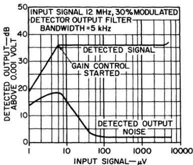
Fig. 179 — Output signal-to-noise ratio as a function of the input signal for the 12-MHz gain-controlled amplifier shown in Fig. 176 when gain control is used in only the first stage.
