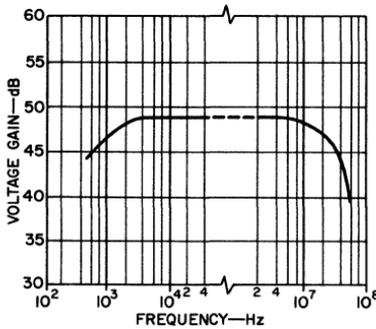
Fig. 298 — Voltage gain as a function of frequency for the broadband video amplifier of Fig. 297.
