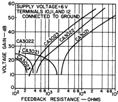
Fig. 127 — Voltage gain of the CA3021, CA3022, and CA3023 as a function of feedback resistance.
