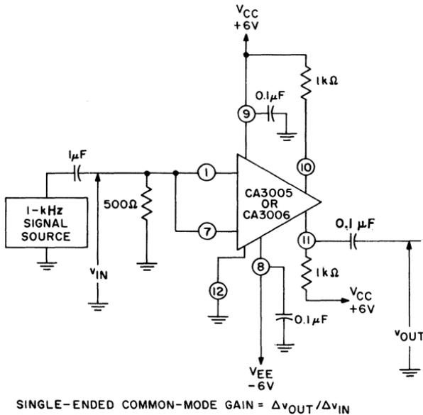
Fig. 158 — Test circuit used to determine single-ended common-mode gain.
