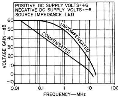
Fig. 212 — Open-loop gain as a function of frequency for both phase-compensated and uncompensated operational amplifiers.
