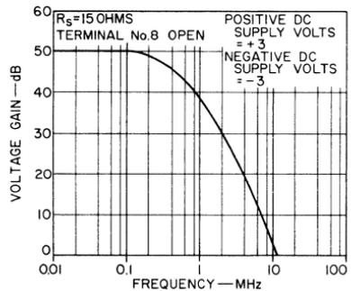
Fig. 201 — Voltage gain as a function of frequency.
