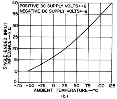
Fig. 207 — Input impedance as a function of temperature: (a) for CA3008; (b) for CA3008A.
