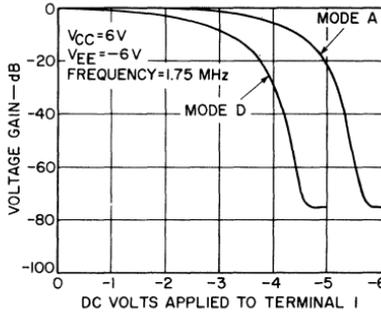
Fig. 111 — Voltage gain of the CA3002 as a function of negative dc supply voltage applied at terminal 1 (normalized to a gain of 26 dB).
