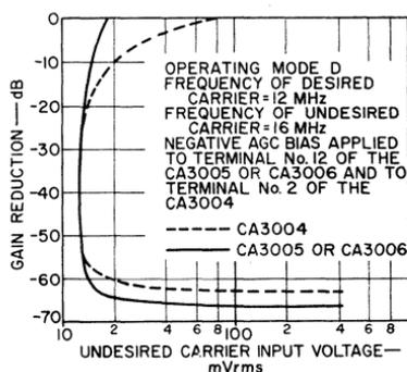
Fig. 163 — Gain control as a function of an undesired-carrier voltage that produces cross-modulation distortion of 10 per cent for balanced differential-amplifier operation of the CA3004, CA3005, and CA3006 when the gain-control voltage is applied to the bias network of the constant-current transistor  $Q_3$ .
