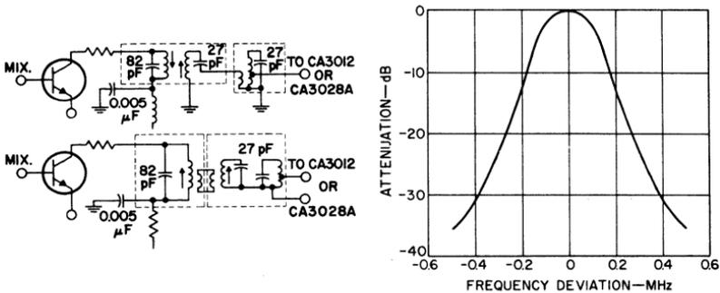
Fig. 266 — Configurations and response curve for triple-tuned interstage filter.
