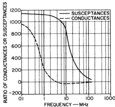
Fig. 148 — Ratio of real (conductance) and imaginary (susceptance) parts of the reverse-transfer admittance for a common-emitter stage to those for a cascode stage as a function of frequency.
