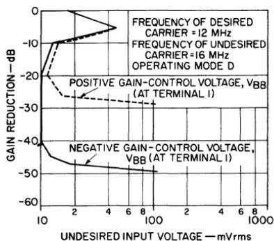
Fig. 164 — Gain control as a function of an undesired-carrier voltage that produces cross-modulation distortion of 10 per cent for balanced differential-amplifier operation of the CA3005 and CA3006 when gain control is provided by application of an offset voltage to the differential pair of transistors.
