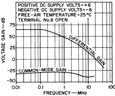
Fig. 203 — Differential and common-mode gain as a function of frequency.
