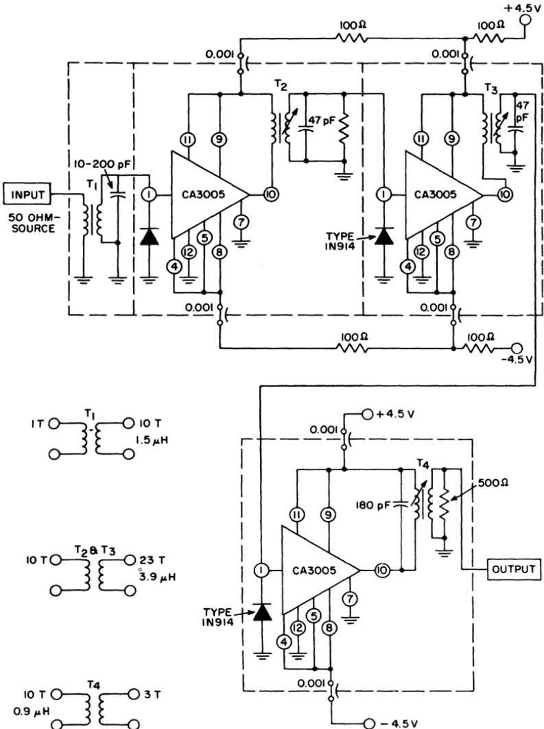
Notes: 1. Transformer  $T_1$  is a Ferramic Q-2 Type (unloaded  $Q = 200$ ).
