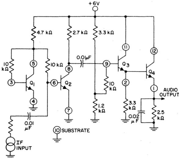
Fig. 303 — Schematic diagram for a CA3018 final if amplifier and second detector.
