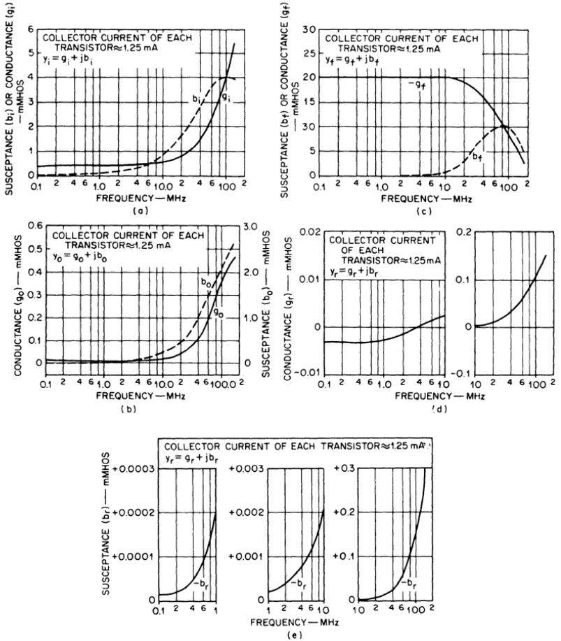
Fig. 150 — Admittance parameters of a CA3005 or CA3006 differential amplifier as a function of frequency.
