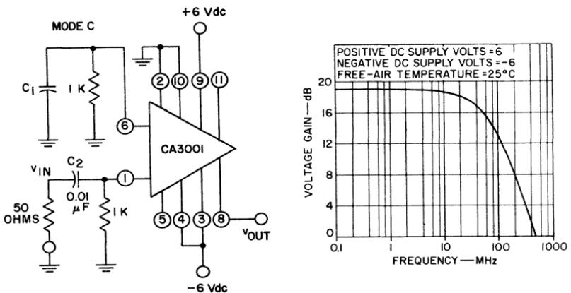
Fig. 96 — Frequency response of the CA3001 in the test circuit shown.
