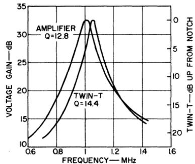
Fig. 233 — Circuit diagram and response for a band-pass amplifier using a twin-T network.
