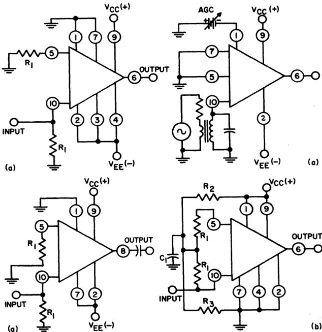
Fig. 105 — Circuit configurations for the CA3002 with (a) dual voltage supplies and (b) a single supply.
