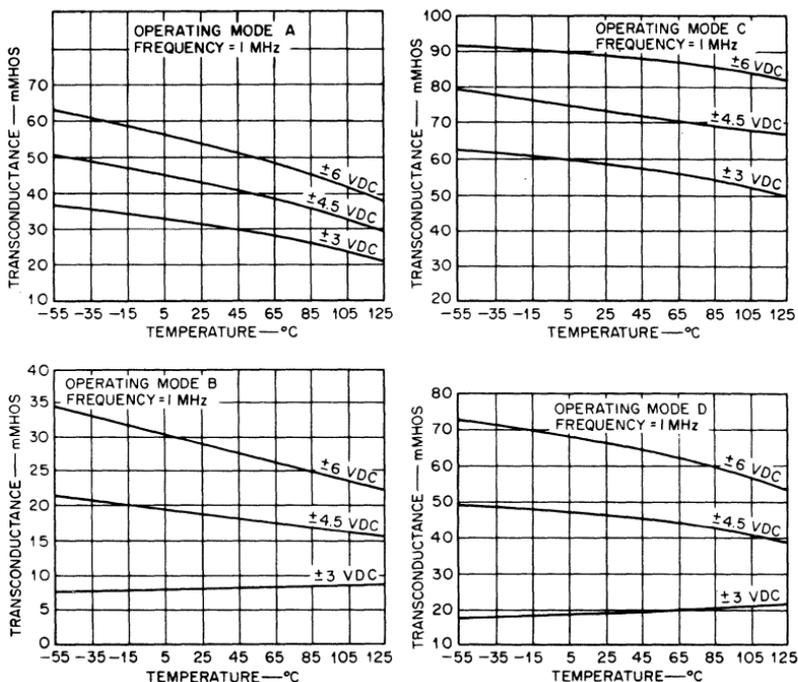
Fig. 146 — Transconductance of the CA3005 or CA3006 in a cascode configuration as a function of temperature for each operating mode.
