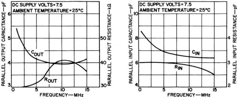
Fig. 258 — Input and output impedance as a function of frequency.
