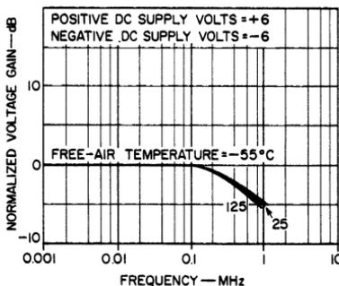
Fig. 78 — Normalized gain-frequency curves for the CA3000 at three different temperatures.
