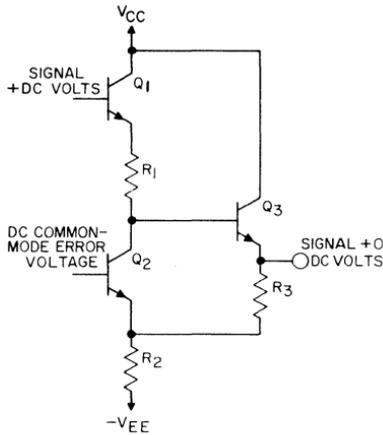
Fig. 9 — Output circuit used in linear integrated circuits to compensate for a shift in dc voltage level between output and input.
