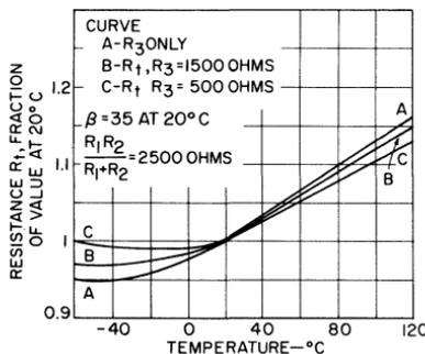
Fig. 39 — Resistance ratio  $R_t$  as a function of temperature for several values of the emitter resistor ( $R_3$ ) of the current-sink transistor.
