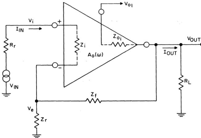
Fig. 59 — Noninverting-feedback operational-amplifier configuration.
