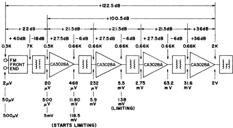
Fig. 275 — Voltage gain and impedance values for if-amplifier strip of Fig. 274.
