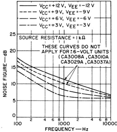
Fig. 196 — Noise figure for the "A"-version integrated-circuit operational amplifiers for operation from  $\pm 6$ -volt and  $\pm 12$ -volt supply voltages.
