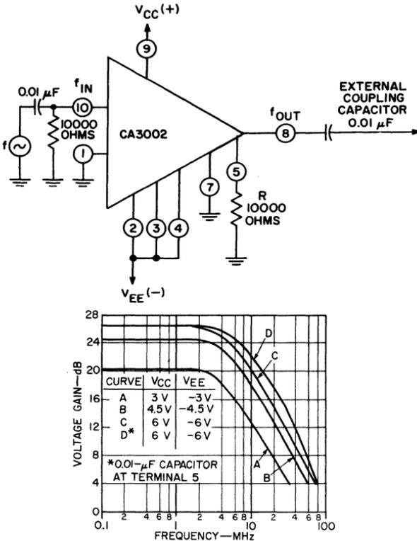
Fig. 110 — Effective single-state response characteristics for CA3002 if amplifier using 0.01-microfarad coupling capacitors. Curve D represents operation with 0.01-microfarad bypass capacitor connected at terminal 5 (not shown).
