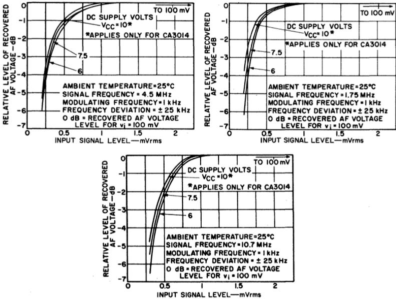
Fig. 259 — Input limiting voltage (knee) and recovered audio-frequency voltage for operation of amplifier-discriminator at 1.75, 4.5, and 10.7 MHz.
