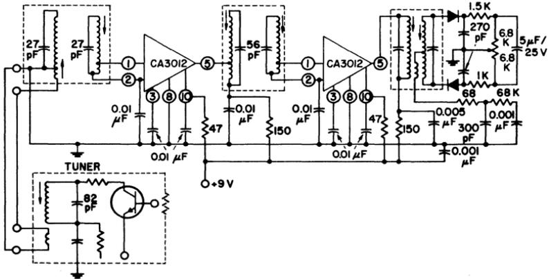
Fig. 269 — Complete 10.7 MHz if-amplifier strip using two CA3012 integrated circuits.
