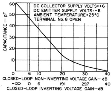
Fig. 213 — Amount of phase-compensating capacitance required to obtain a flat ( $\pm 1$ -dB) gain-frequency response.
