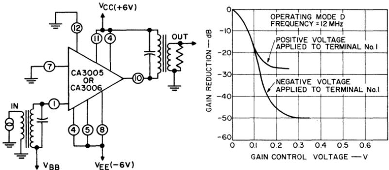
Fig. 160 — Gain control characteristics of the CA3005 or CA3006 as a function of the dc offset voltage  $V_{BB}$  applied to the differential pair of transistors  $Q_1$  and  $Q_2$ .
