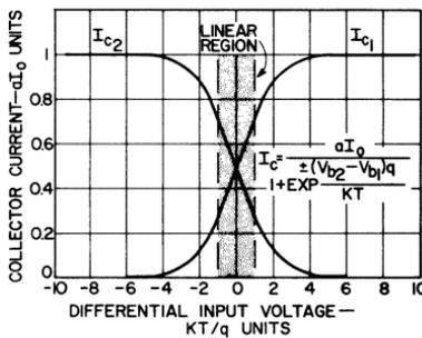
Fig. 21 — Transfer characteristics of the basic differential-amplifier circuit.
