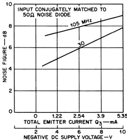
Fig. 155 — Representative noise performance of the CA3005 or CA3006 operated in a cascode configuration (operating mode D).
