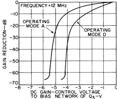
Fig. 159 — Gain-control characteristics of the CA3005 or CA3006 as a function of the dc gain-control voltage applied to the bias network of transistor  $Q_3$ .
