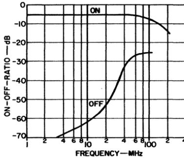
Fig. 289 — On-to-off ratio of the series gate of Fig. 288 as a function of frequency.
