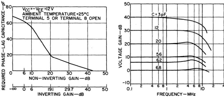
Fig. 228 — Amount of phase-lag capacitance required to obtain a flat ( $\pm 1$ -dB) response and typical response characteristics.
