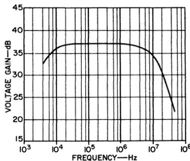
Fig. 300 — Voltage gain as a function of frequency for the cascode amplifier of Fig. 299.
