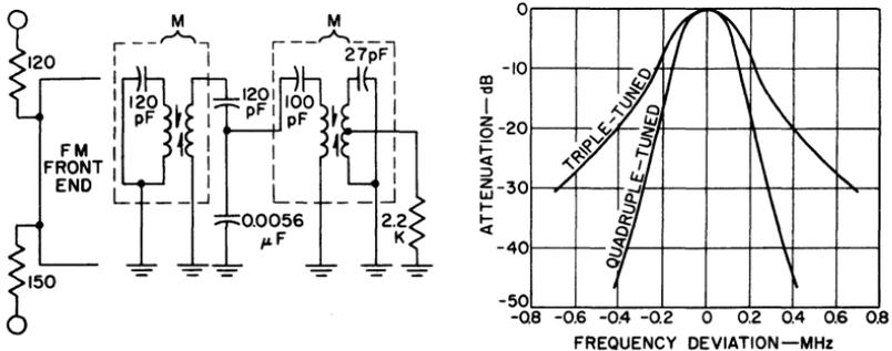
Fig. 268 — Response curve obtained with quadruple-tuned filter.
