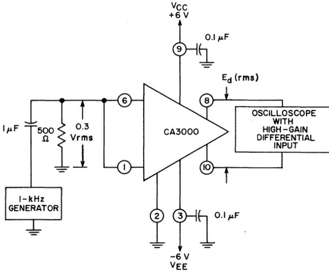
$$\text{COMMON-MODE REJECTION RATIO (CMR)} = 20 \log \frac{(A^*)(2)(0.3)}{E_d(\text{rms})}$$
