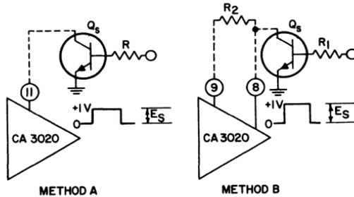
Fig. 244 — Methods of applying squelch to the CA3020.
