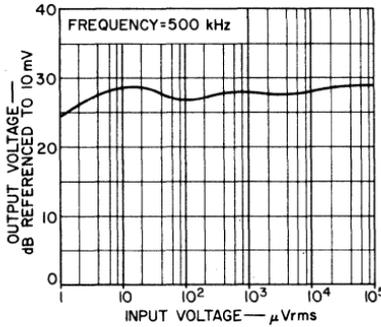
Fig. 137 — Schematic diagram and limiting performance of two-stage 500-kHz limiter-amplifier using the CA3021.
