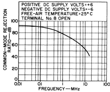
Fig. 204 — Common-mode rejection as a function of frequency.
