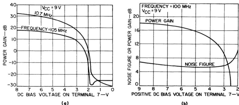
Fig. 162 — AGC characteristics of the CA3028A operated in a differential-amplifier configuration: (a) power gain as a function of agc voltage at 10.7 and 105 MHz; (b) power gain and noise figure as a function of agc voltage at 100 MHz.
