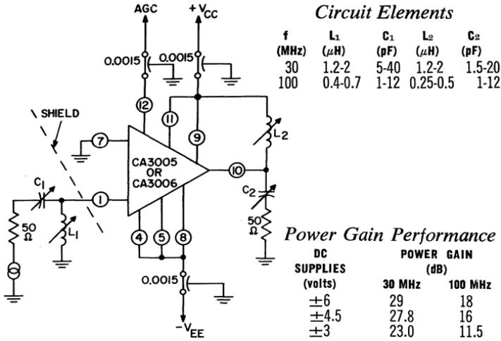
Fig. 173 — Test circuit used to evaluate rf-performance capabilities of CA3005 or CA3006 in a differential-amplifier configuration.
