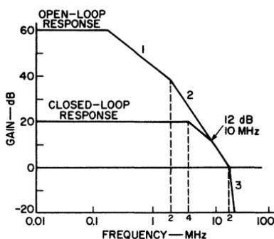
Fig. 64 — Basic integrating response characteristics of an operational amplifier.
