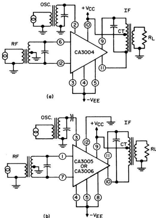
Fig. 185 — Circuit diagrams for use of (a) the CA3004 and (b) the CA3005 or CA3006 as mixers (operating mode D).
