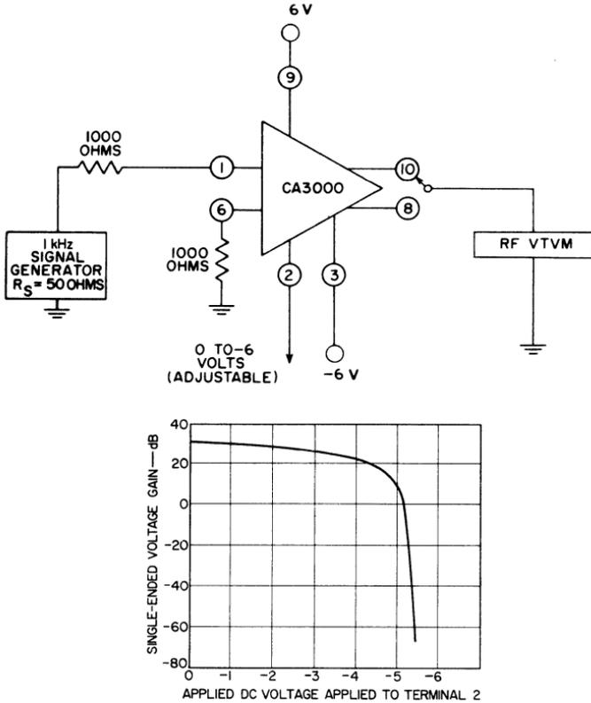
Fig. 79 — AGC characteristics of the CA3000 in test circuit shown at a frequency of 1 kHz.
