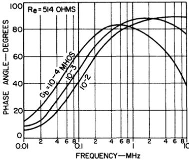
Fig. 54 — Output-impedance phase angle of the current-sink transistor as a function of frequency for several values of base-termination conductance.
