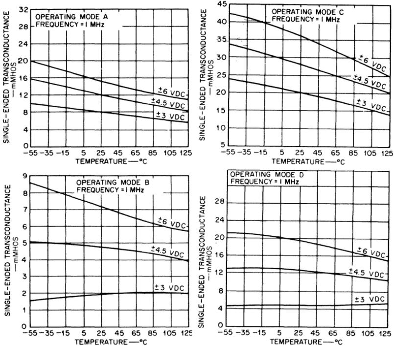
Fig. 145 — Single-ended transconductance of the CA3005 or CA3006 in a differential-amplifier configuration as a function of temperature for each operating mode.
