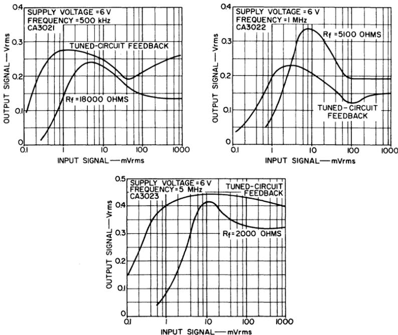
Fig. 133 — Limiting characteristics of the CA3021, CA3022, and CA3023.
