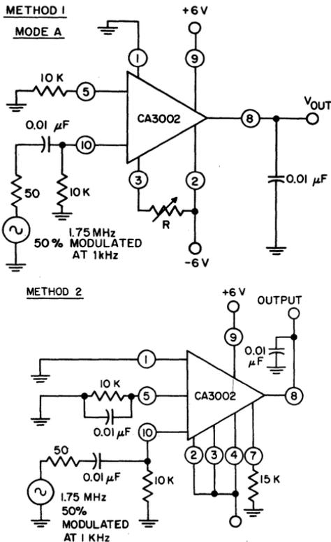
Fig. 115 — Envelope detectors using CA3002 integrated circuits.
