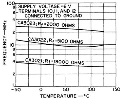
Fig. 125 — Upper 3-dB frequency shift with temperature for the CA3021, CA3022, and CA3023.
