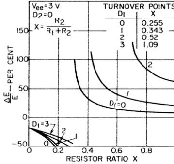
Fig. 40 — Effect of the number of diodes  $D_1$  on the variation in the voltage  $E$  as a function of the ratio  $X$  for a temperature increase of  $100^\circ\text{C}$  and a supply voltage  $V_{ee}$  of 3 volts when no diodes  $D_2$  are used.
