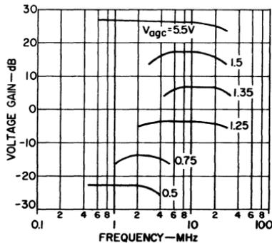
Fig. 129 — Effect of gain control on response characteristics of the CA3021, CA3022, and CA3023.
