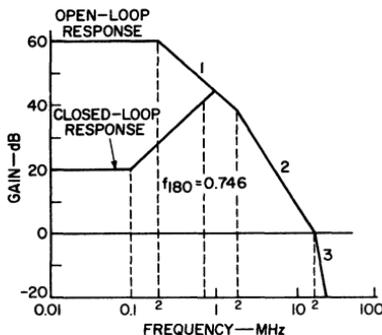
$$A_o(\omega) = \frac{1000}{\left(1 + j \frac{f}{0.2 \text{ MHz}}\right) \left(1 + j \frac{f}{2 \text{ MHz}}\right) \left(1 + j \frac{f}{20 \text{ MHz}}\right)}$$
