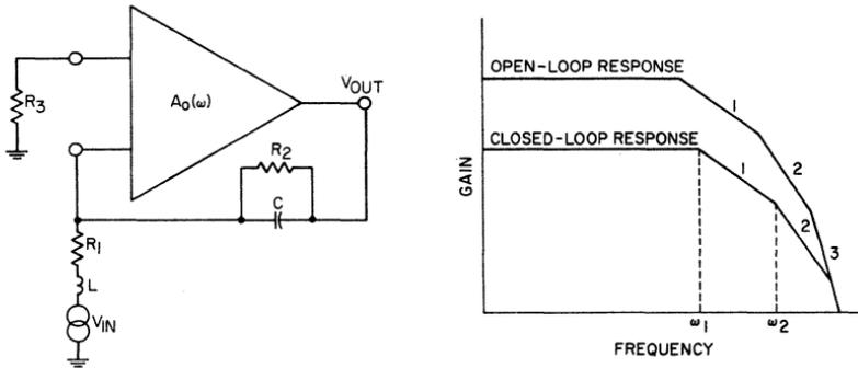
$$R_3 = R_1 \parallel R_2$$
