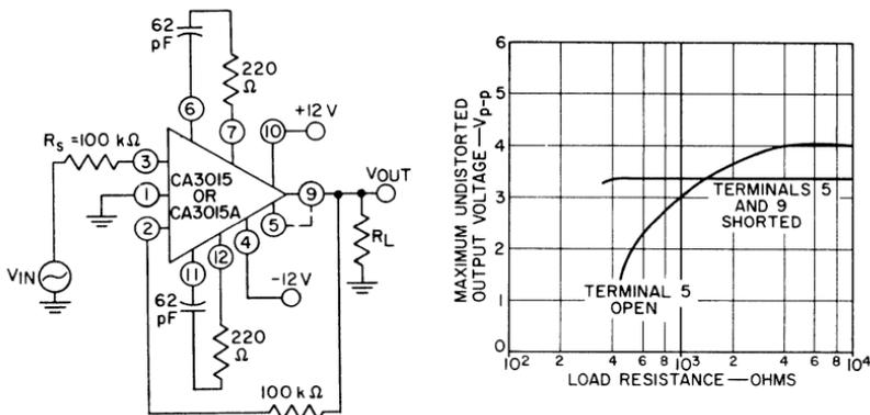
Fig. 235 — Circuit diagram for a voltage follower driven from a 100,000-ohm source, and curve showing maximum undistorted output voltage as a function of load resistance.
