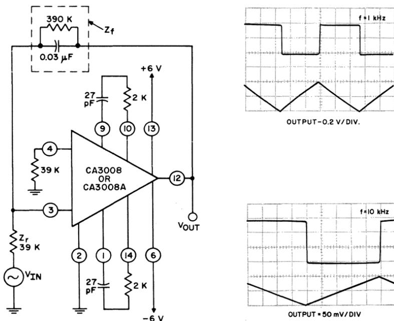
Fig. 222 — Circuit diagram and the input and output waveforms for an operational amplifier used as an integrator.
