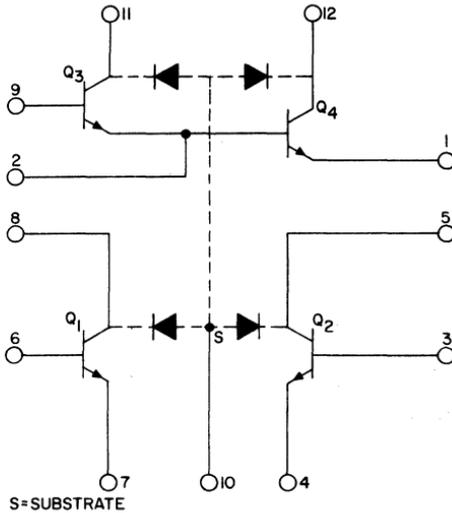
Fig. 296 — Schematic diagram for the CA3018 integrated-circuit transistor array.
