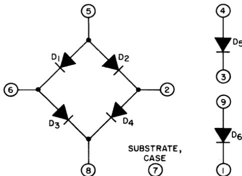
Fig. 283 — Schematic diagram of the CA3019 integrated-circuit diode array.
