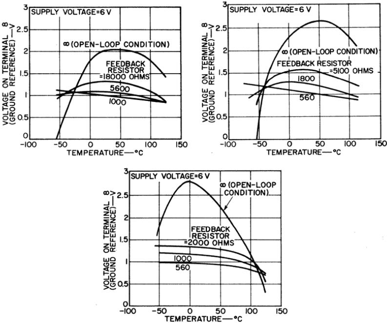
Fig. 122 — Output operating point of the CA3021, CA3022, and CA3023 as a function of temperature for various values of feedback resistance.
