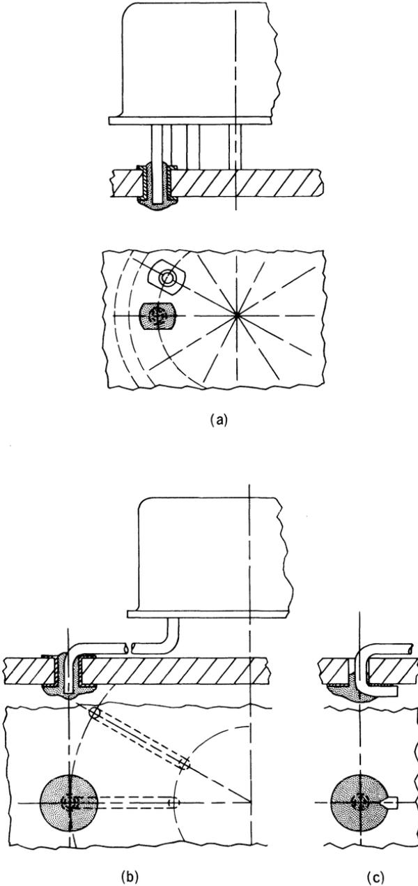
Fig. 15 — Mounting methods for RCA TO-5 style packages: (a) straight-through method; (b) straight-through method with leads radially offset; (c) radially offset leads with clinched-lead option.
