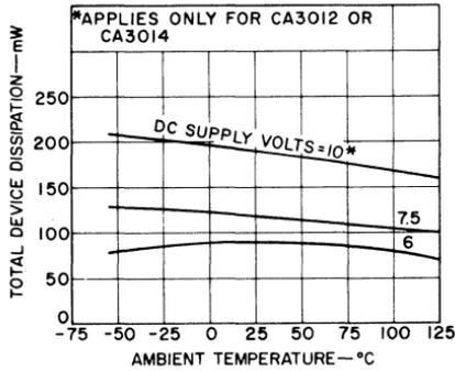
Fig. 255 — Total dissipation as a function of temperature.
