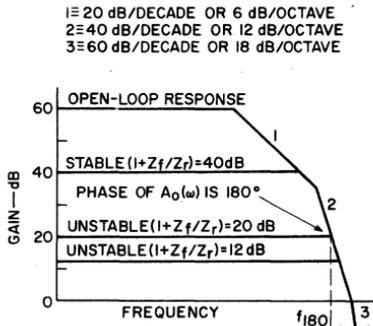
Fig. 62 — Open-loop response and stability characteristics of an operational amplifier.
