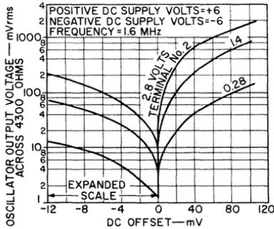
Fig. 188 — Cancellation of the oscillator signal at the output of a CA3004 mixer as a function of dc offset voltage.
