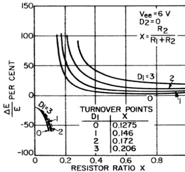
Fig. 41 — Effect of the number of diodes  $D_1$  on the variation in the voltage  $E$  as a function of the ratio  $X$  for a temperature increase of  $100^\circ\text{C}$  and a supply voltage  $V_{ee}$  of 6 volts when no diodes  $D_2$  are used.
