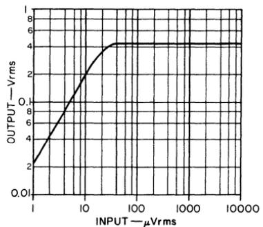
Fig. 178 — Limiting characteristics of the 12-MHz limiting amplifier shown in Fig. 175.
