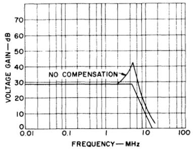
Fig. 215 — Circuit diagram and gain-frequency response of the 30-dB noninverting video amplifier operated without phase compensation.
