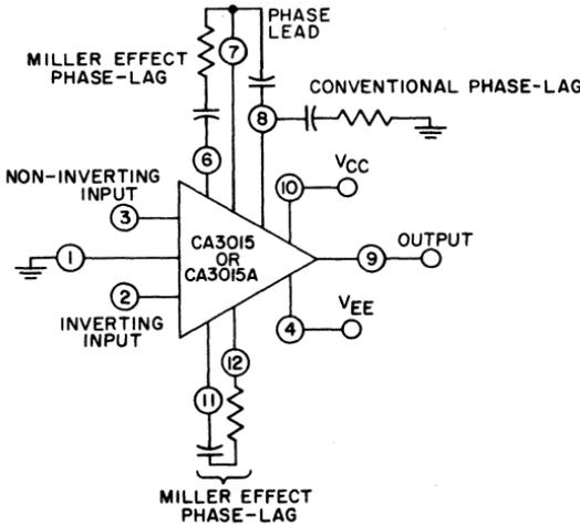
Fig. 227 — Terminal connections for phase-lag and phase-lead compensation of the CA3015 or CA3015A.
