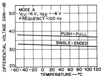
Fig. 76 — Measured values of single-ended and push-pull gain for mode A operation with symmetrical power supplies of  $\pm 6$  volts.
