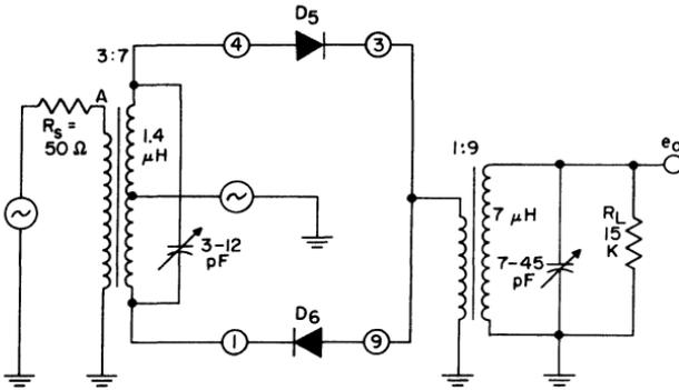
Fig. 292 — Balanced mixer using the CA3019.
