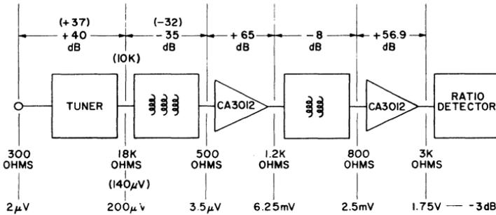
Fig. 270 — Voltage gain and impedance values for if-amplifier strip of Fig. 269.
