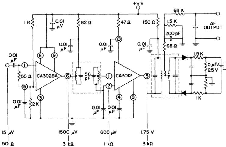
Fig. 274 — IF-amplifier strip using CA3028A and CA3012 integrated circuits.
