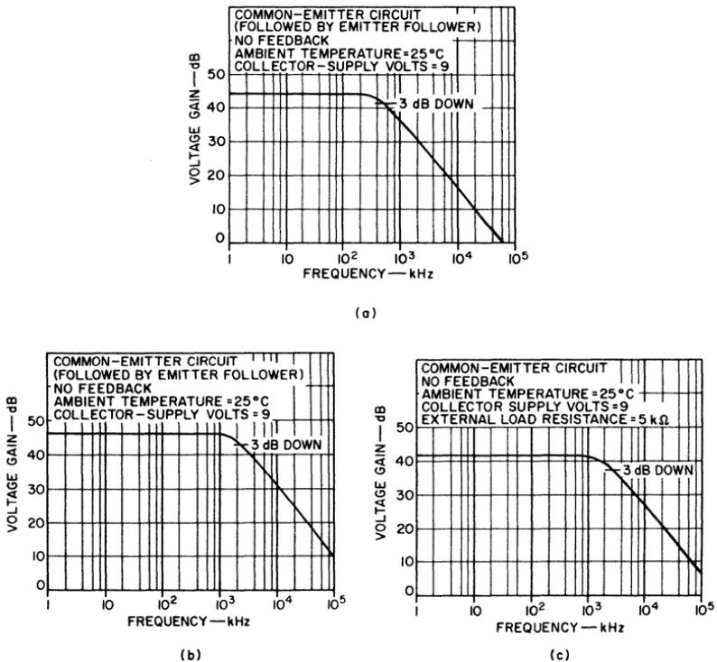
Fig. 281 — Typical gain-frequency response of the three amplifier stages in the CA3035 or CA3035V1 array: (a) first stage; (b) second stage; (c) third stage.
