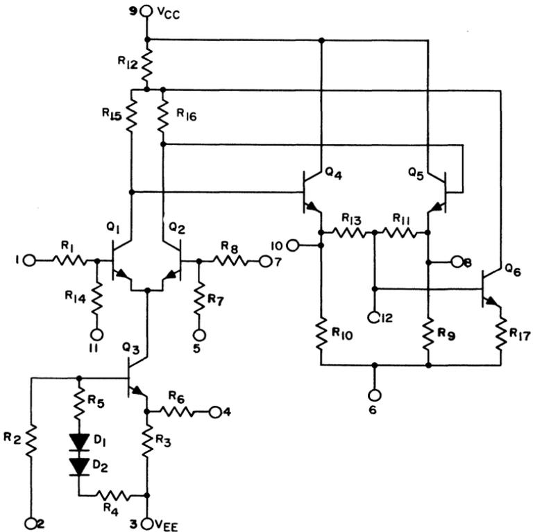
Fig. 89 — Schematic diagram of CA3007 integrated-circuit audio driver.
