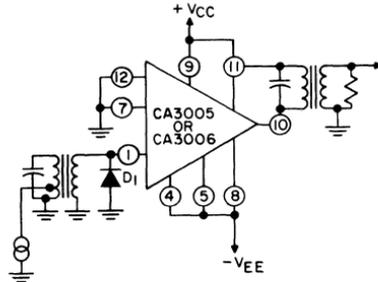
Fig. 169 — CA3005 or CA3006 differential-amplifier limiter that uses a diode to provide overload protection.
