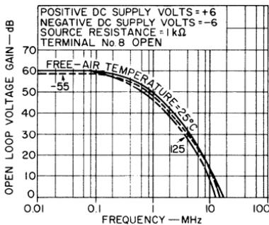
Fig. 200 — Open-loop gain as a function of frequency.
