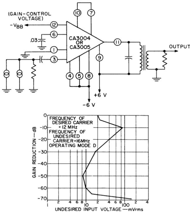
Fig. 166 — Gain control of the CA3005 or CA3006 in a cascode configuration as a function of an undesired-carrier voltage that produces cross-modulation distortion of 10 per cent when gain control is provided by a negative bias voltage applied to the base of transistor  $Q_3$ .
