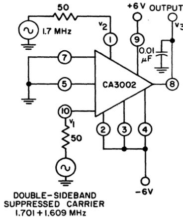
Fig. 117 — Product-detector circuit using the CA3002.
