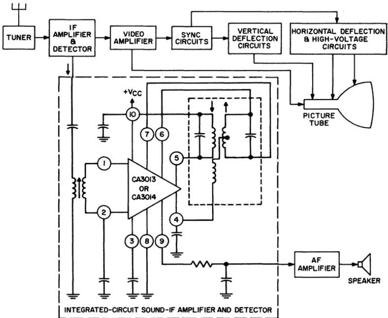
Fig. 261 — Block diagram of typical television receiver using CA3013 or CA3014 integrated-circuit sound-if amplifier and detector section.
