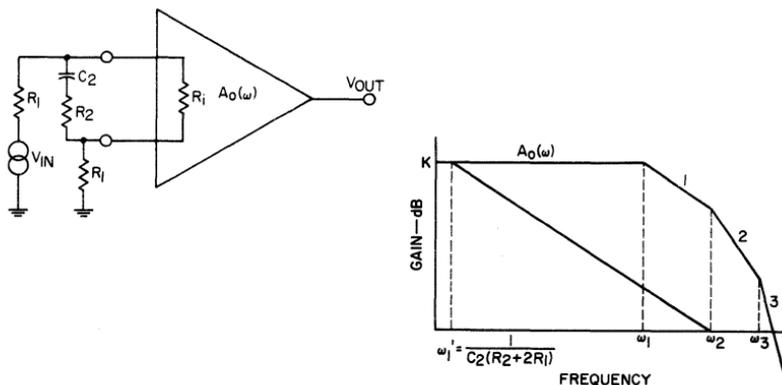
$A_o(\omega)$  = uncompensated open-loop gain
