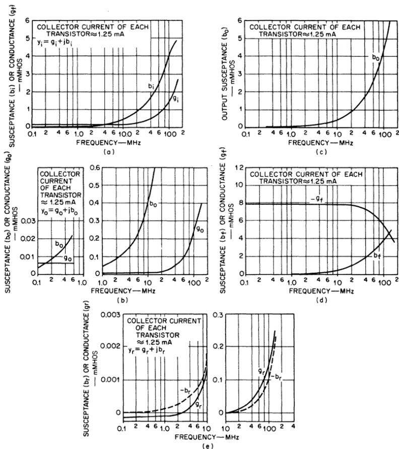
Fig. 149 — Admittance parameters of the CA3004 differential amplifier as a function of frequency.
