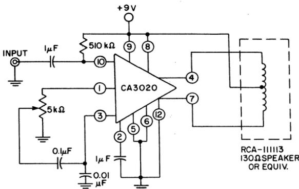
Fig. 246 — 310-milliwatt audio amplifier without transformers.
