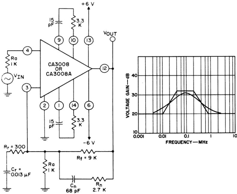
Fig. 220 — Circuit diagram and response of a noninverting type of operational amplifier used to synthesize peaked-response transfer functions.
