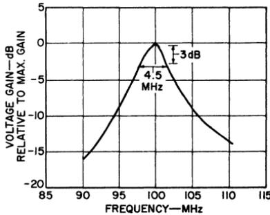
Fig. 306 — Response characteristics of 100-MHz amplifier of Fig. 305.
