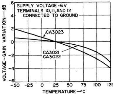
Fig. 124 — Voltage-gain variation with temperature for the CA3021, CA3022, and CA3023 (feedback adjusted to provide gain of approximately 40 dB at 25°C).
