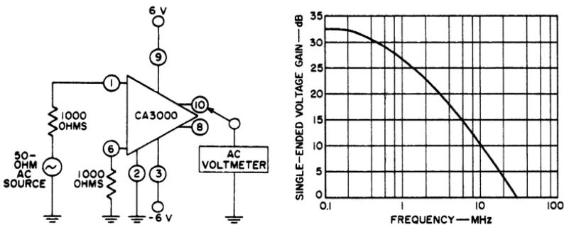
Fig. 77 — Single-ended voltage gain of the CA3000 as a function of frequency in test circuit shown.
