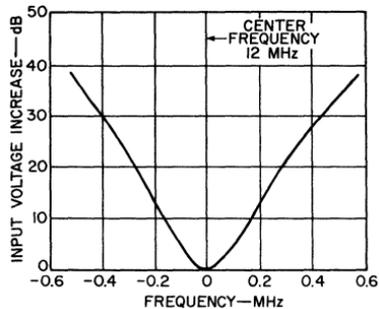
Fig. 180 — Frequency-response characteristics of the 12-MHz gain-controlled amplifier shown in Fig. 176.
