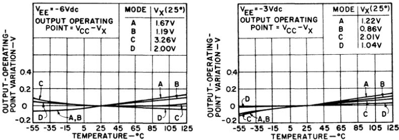
Fig. 94—Output operating point of the CA3001 (normalized to the  $25^\circ\text{C}$  operating point) as a function of temperature for  $V_{EE}$  supplies of  $-3$  and  $-6$  volts.
