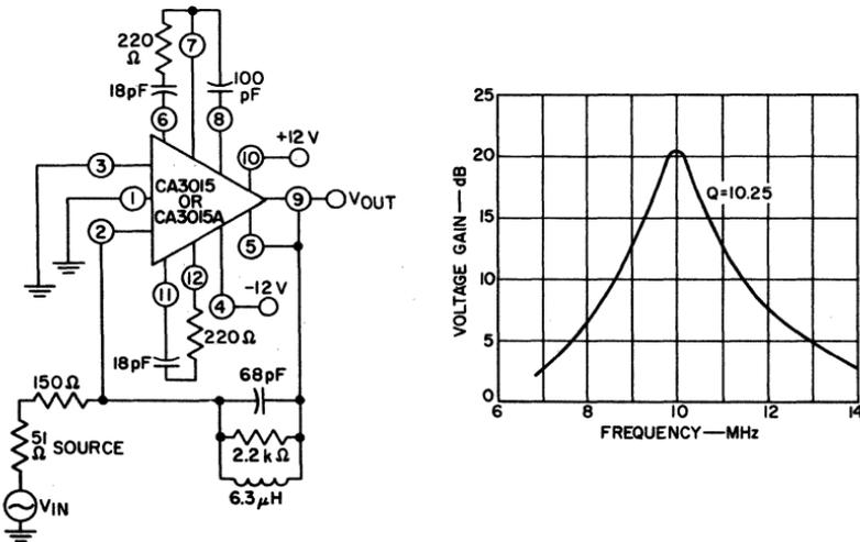
Fig. 234 — Circuit diagram and response for a 10-MHz band-pass amplifier.
