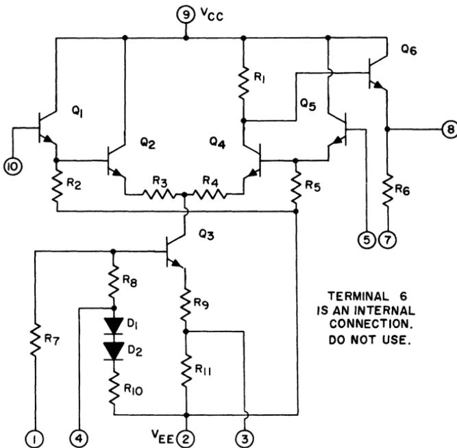
Fig. 104 — Schematic diagram of the CA3002 integrated-circuit if amplifier.
