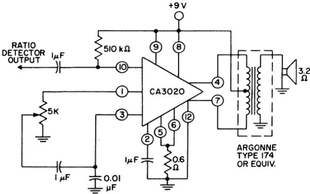
*Fig. 247 — 545-milliwatt amplifier driving a low-impedance speaker.*
