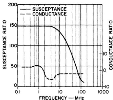
Fig. 147 — Ratio of real (conductance) and imaginary (susceptance) parts of the reverse-transfer admittance for a common-emitter stage to those for a differential-amplifier stage as a function of frequency.
