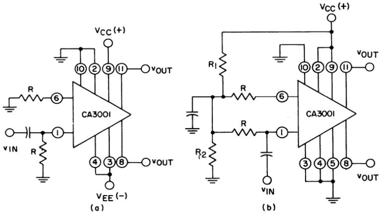
Fig. 93 — Circuit connections for the CA3001 for (a) separate positive and negative supplies and (b) a single supply.
