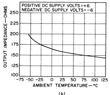
Fig. 208 — Output impedance as a function of temperature: (a) for CA3008; (b) for CA3008A.
