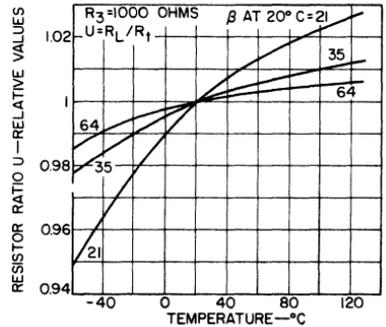
Fig. 49 — Resistor ratio  $U$  as a function of temperature for several values of the beta for the current-sink transistor.
