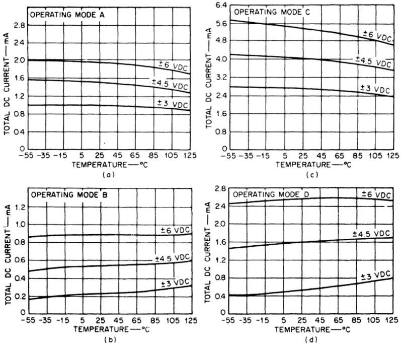
Fig. 143 — Operating current of the CA3004, CA3005, or CA3006 as a function of temperature for each operating mode.
