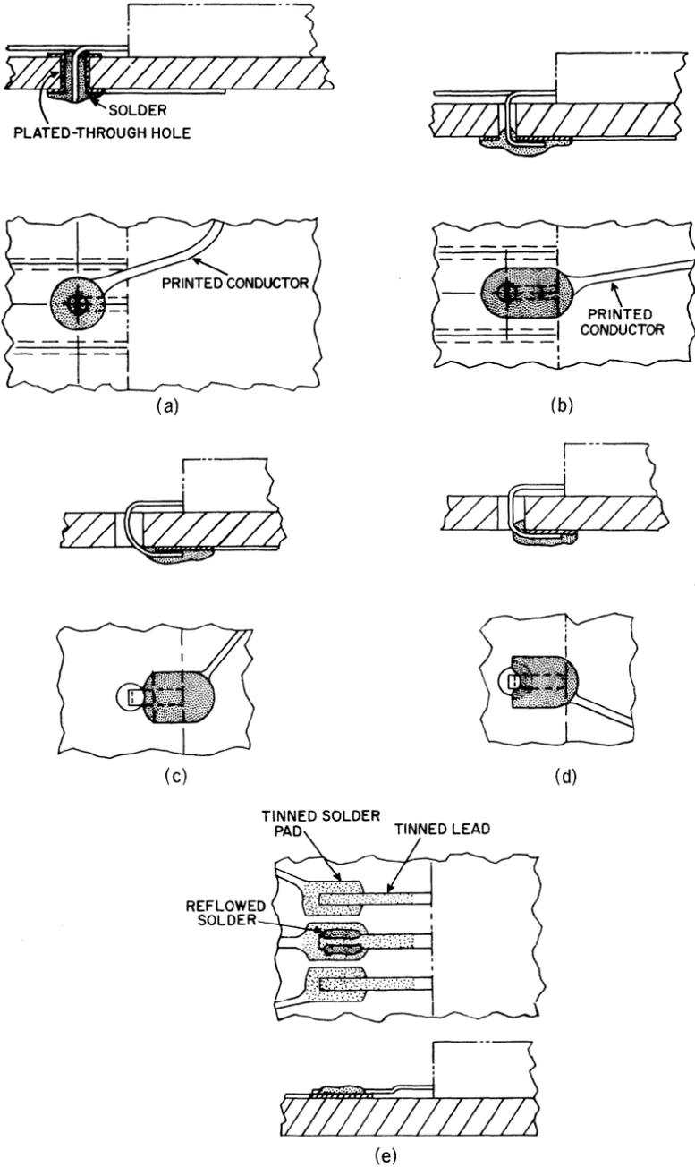
Fig. 11 — Interconnection methods for RCA 14-terminal ceramic flat packs: (a) straight-through method; (b) clinched-lead full-pad method; (c) clinched-lead offset-pad method; (d) clinched-lead half-pad method; (e) surface connection method (reflow soldering).
