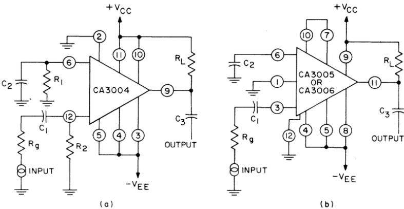
Fig. 195 — Video amplifiers using (a) the CA3004 in a differential-amplifier configuration and (b) the CA3005 or CA3006 in a cascode configuration.
