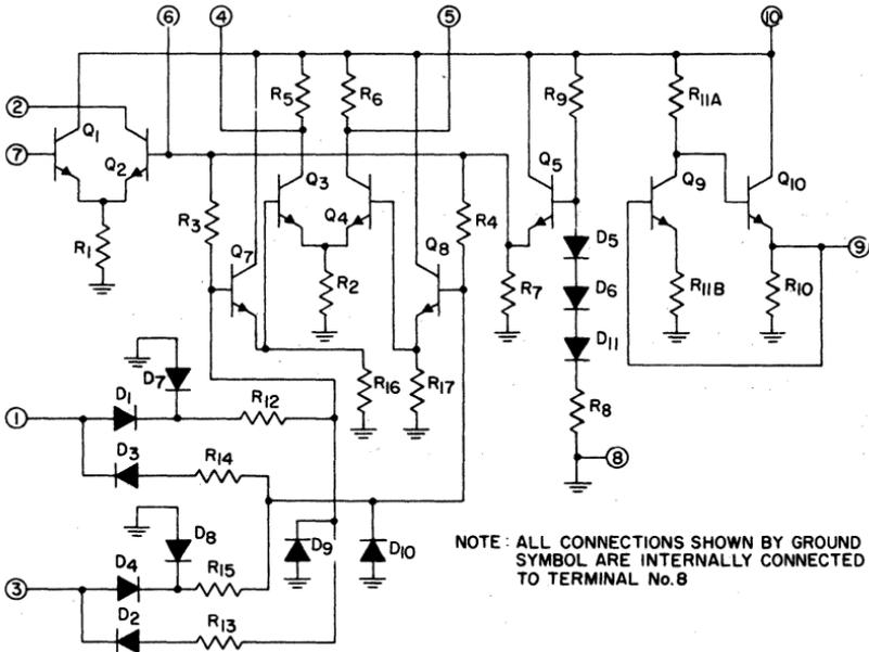
Fig. 278 — Schematic diagram of the CA3034 or CA3034V1 integrated-circuit wide-band amplifier/phase detector.
