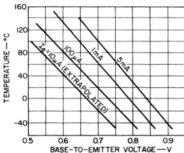
Fig. 29 — Effect of temperature and emitter current on the base-to-emitter voltage of an integrated-circuit transistor.
