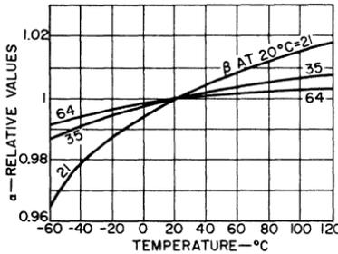
Fig. 46 — Relative values of the alpha for the current-sink transistor as a function of temperature for several beta values.
