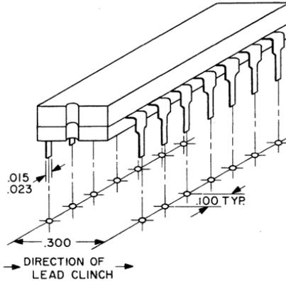
Fig. 18 — Mounting arrangement for RCA dual-in-line packages.
