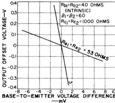
Fig. 35 — Output offset voltage as a function of the difference in the base-to-emitter voltages of the differential pair of transistors for several values of the total emitter resistance (internal + external) of each transistor.
