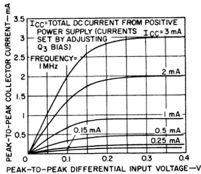
Fig. 140 — Dynamic transfer and limiting characteristics of the CA3005 or CA3006 operated in the differential-amplifier configuration.
