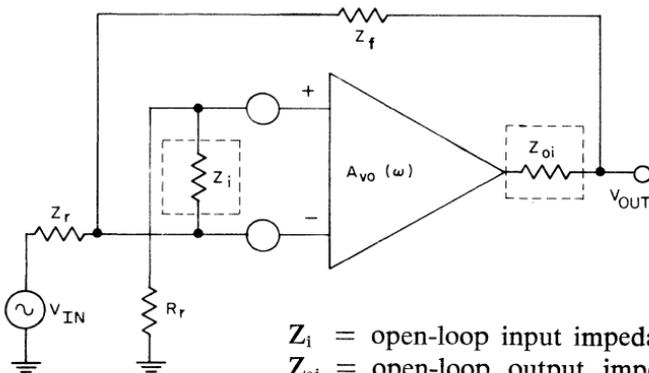
$Z_i$  = open-loop input impedance
