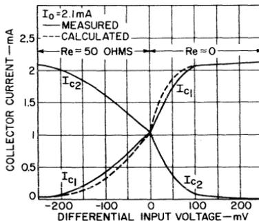
Fig. 26 — DC characteristics of the basic differential amplifier with and without emitter degeneration for a source current of  $I_o$  of 2.1 milliamperes.
