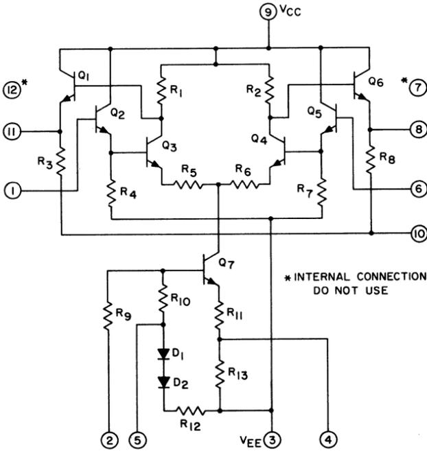
Fig. 92 — Schematic diagram of CA3001 integrated-circuit video amplifier.
