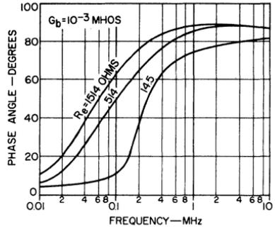
Fig. 55 — Output-impedance phase angle of the current-sink transistor as a function of frequency for several values of emitter resistance.
