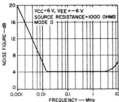
Fig. 113 — Noise figure of the CA3002 as a function of frequency.
