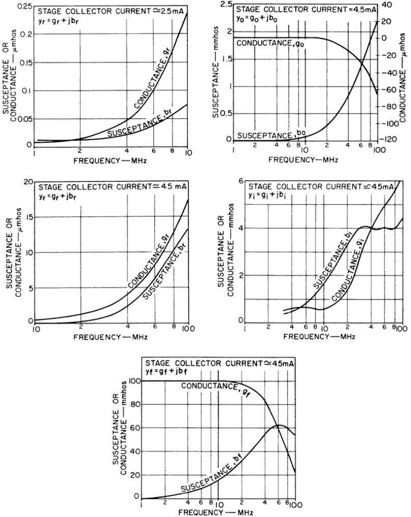
Fig. 153 — Admittance parameters of a CA3028A cascode amplifier as a function of frequency.
