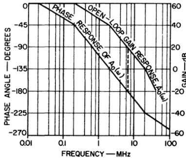
Fig. 61 — Gain and phase response of an open-loop operational amplifier operated without phase compensation.
