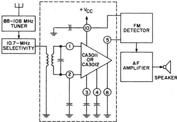
Fig. 263 — Block diagram of typical FM receiver using CA3011 or CA3012 integrated-circuit wide-band amplifier.
