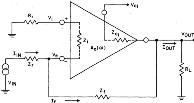
Fig. 58 — Inverting-feedback operational-amplifier configuration.
