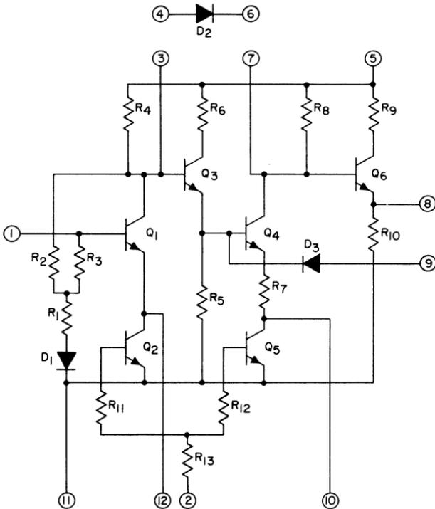
Fig. 119 — Schematic diagram for the CA3021, CA3022, and CA3023 integrated circuits.
