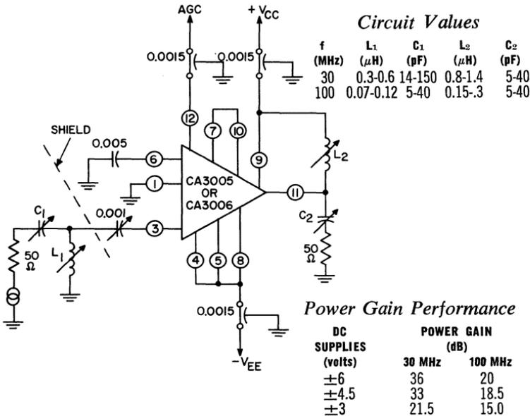
Fig. 174 — Test circuit used to evaluate rf-performance capabilities of a CA3005 or CA3006 in a cascode configuration.
