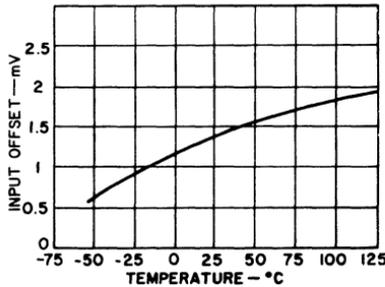
Fig. 81 — Input offset voltage of CA3000 as a function of temperature in test circuit shown.
