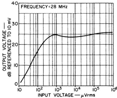
Fig. 136 — Schematic diagram and limiting performance of two-stage limiter-amplifier using the CA3023.
