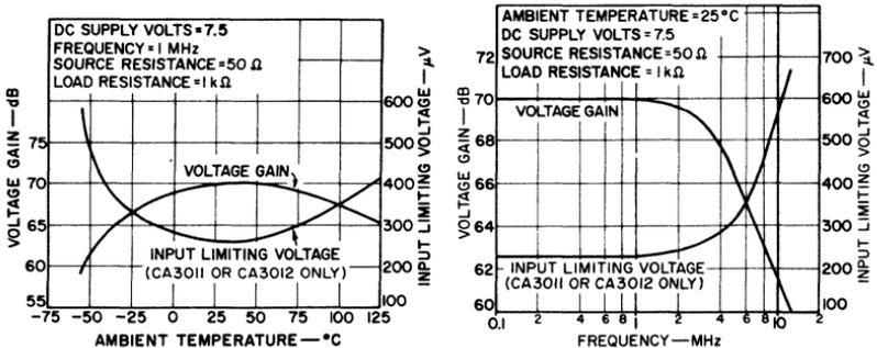
Fig. 257 — Voltage gain and input limiting voltage as a function of temperature and of frequency.
