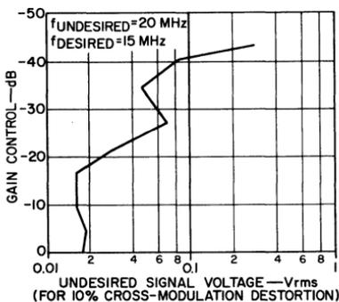
Fig. 302 — In-band cross-modulation characteristic of the 15-MHz amplifier of Fig. 301 (data taken with untuned input).
