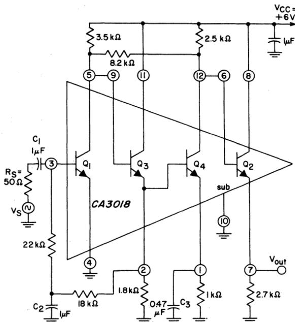
Fig. 297 — Schematic diagram for a CA3018 broadband video amplifier.
