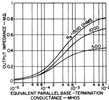
Fig. 51 — Low-frequency output impedance of the current-sink transistor as a function of the equivalent parallel base-termination conductance for several values of the emitter resistance.
