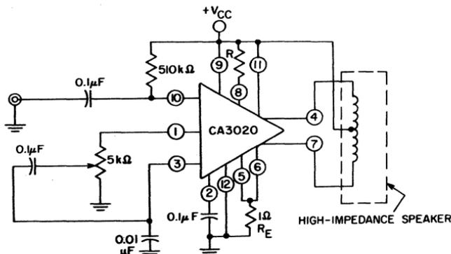
Fig. 242 — CA3020 connection optimized for low distortion.
