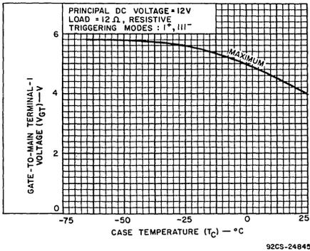
Fig. 10 - DC gate-trigger voltage vs. case temperature.
