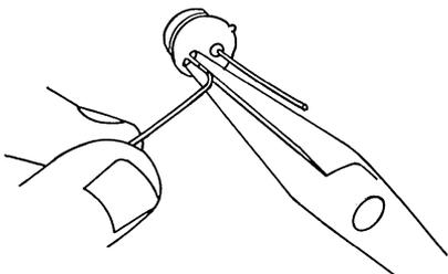
Fig. 5 - Method of bending leads on thyristor package.
