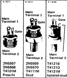
These RCA triacs are gate-controlled, full-wave silicon ac switches. They are designed to switch from an off-state to an on-state for either polarity of applied voltage with positive or negative gate triggering voltages.
