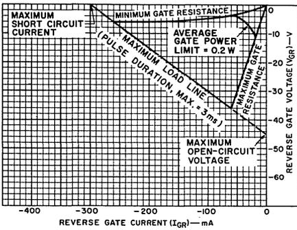
Fig. 14—Reverse gate voltage vs. reverse gate current.
