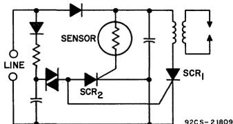
Fig. 26 - Line-charged ignition circuit.
