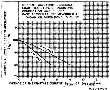
Fig. 6—Maximum allowable case temperature vs. on-state current.
