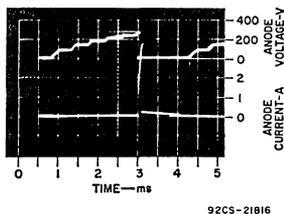
Fig. 19 — SCR voltage (top) and current (bottom) as a function of time (oscilloscope sweep triggered at instant ignition breaker points are closing; 4000 r/min;  $V_{CC} = 12$  V).
