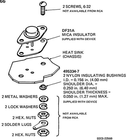
Note: Maximum torque applied to mounting flange is 12 in.-lb.
