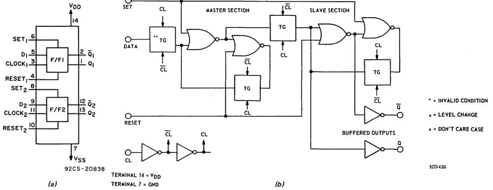
Fig. 13— Logic and block diagram of the CD4013A.
