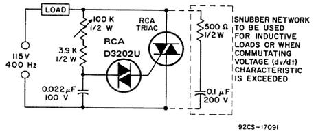
**NOTE:** For incandescent lamp loads which produce burnout current surges with  $I^2t$  values greater than 2.5 ampere<sup>2</sup> seconds, connect a 10-ohm resistor of appropriate power rating in series with the load. This rating can be determined as follows:
