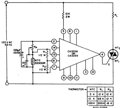
Fig. 11 - CA3058 or CA3059 on-off controller with hysteresis.
