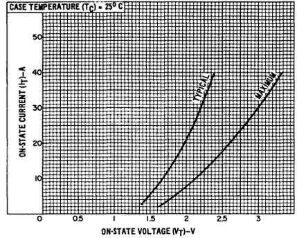
Fig. 4—Instantaneous on-state current vs. on-state voltage.
