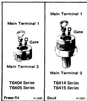
These RCA triacs are gate-controlled full-wave silicon ac switches. They are designed to switch from an off-state to an on-state for either polarity of applied voltage with positive or negative gate triggering voltages. They are intended for operation at 400 Hz with resistive or inductive loads and nominal line voltages of 115 and
