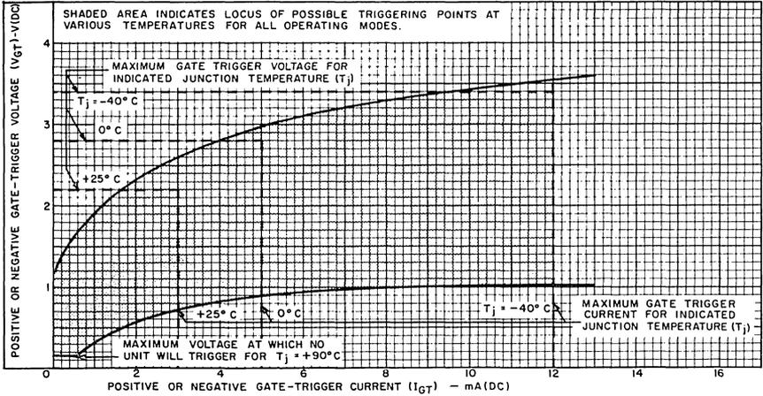
Fig. 16 - Gate characteristics for T2300 and T2310 series.
