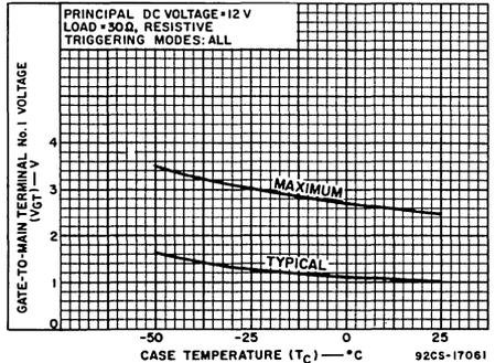
Fig. 10 - DC gate-trigger voltage vs. case temperature.
