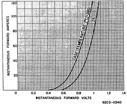
Fig.5— Surge-current rating chart for all types and corresponding reverse-polarity versions.
