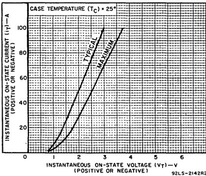
Fig. 5 — On-state current vs. on-state voltage.
