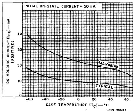
Fig. 18—DC holding current (positive) vs. case temperature.
