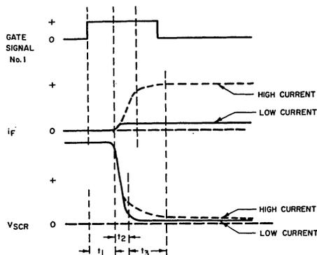
Fig.3 - Actual SCR wave shapes during turn-on.
