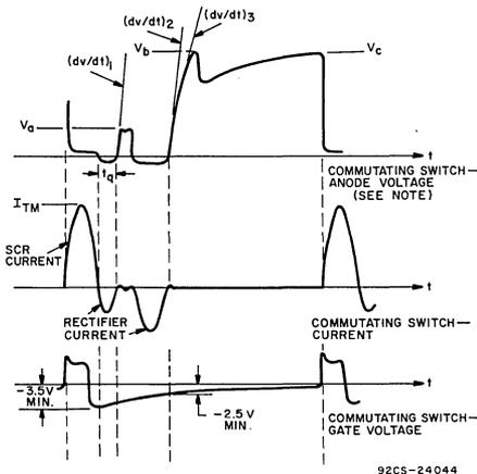
NOTE: "Commutating Switch-Anode Voltage" oscilloscope display has been modified graphically to enhance the measurement points of  $dv/dt$ .
