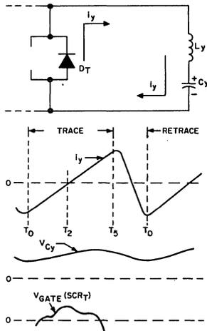
Fig. 4—Effective configuration of the deflection circuit during the first half of the trace interval, time  $T_0$  to  $T_2$ , and operating voltage and current waveforms for the complete trace-retrace cycle.
