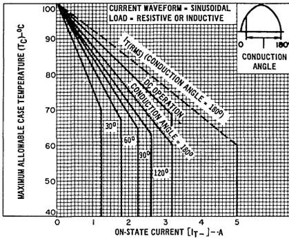
Fig. 2 - Maximum allowable case temperature vs. on-state current.
