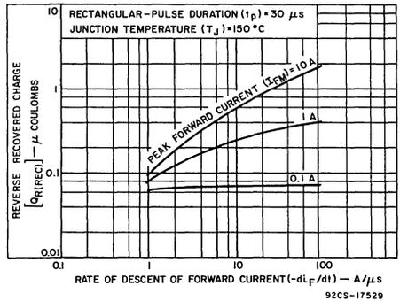
Fig. 13 - Reverse recovered charge vs. rate of descent of forward current for all types.
