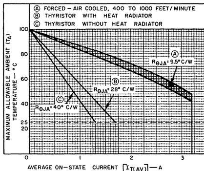
Fig. 1— Maximum allowable ambient temperature vs. on-state current.
