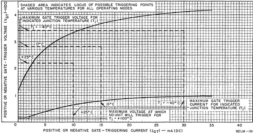
Fig. 17 - Gate characteristics for T2302 and T2312 series.
