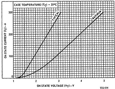
Fig. 6 - Variation of on-state current with on-state voltage.
