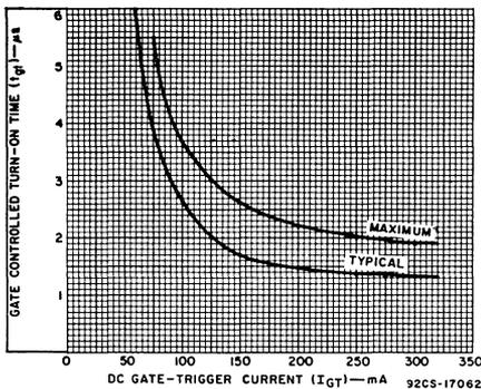
Fig. 11 - Turn-on time vs. gate trigger current.
