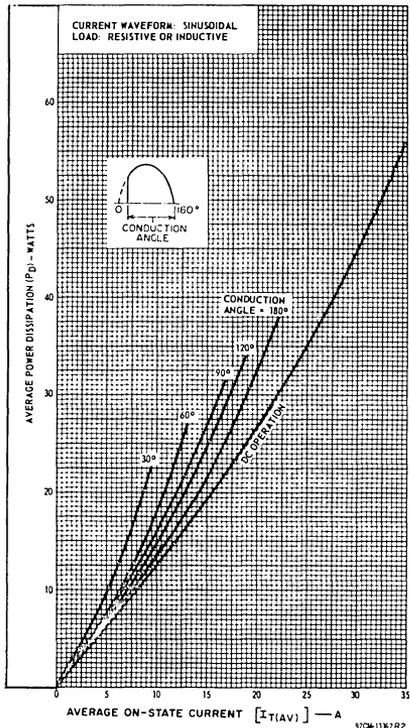
Fig. 2—Power dissipation vs. on-state current.
