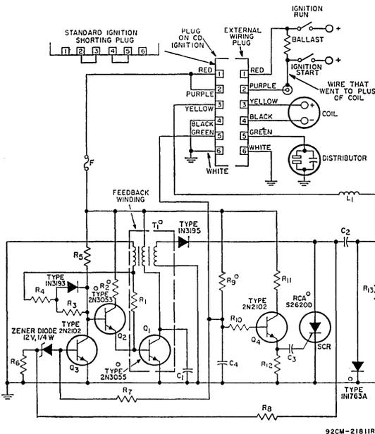
Fig. 14 - An SCR capacitive-discharge automotive ignition circuit.
