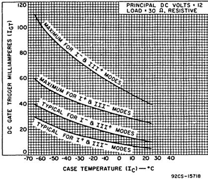
Fig. 11 — DC gate-trigger current vs. case temperature.
