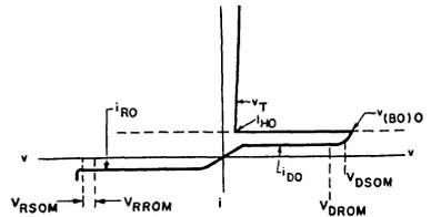
Fig. 2 - Principal voltage-current characteristic for S3705M and S3706E.
