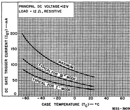
Fig. 10 - DC gate-trigger current (for I<sup>-</sup> and III<sup>+</sup> triggering modes) vs. case temperature for T2800 series only.
