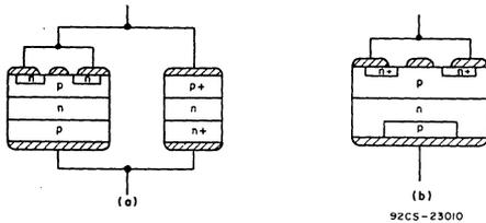
Fig. 2—(a) Separate SCR and rectifier, (b) combined device.
