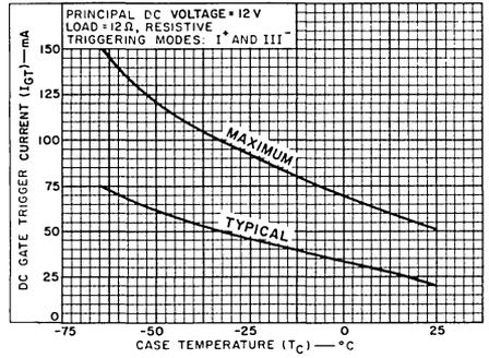
Fig. 8 - DC gate-trigger current vs. case temperature (I<sup>+</sup> & III<sup>+</sup> modes).
