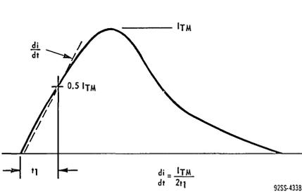
Fig. 15 - Rate-of-change of on-state current with time (defining  $di/dt$ ).
