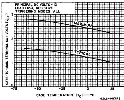
Fig. 14 — DC gate-trigger voltage vs. case temperature.
