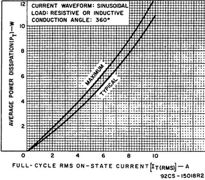
Fig. 2 — Power dissipation vs. on-state current.
