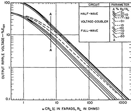
Fig. 11 - RMS ripple voltage of capacitor-input circuits.
