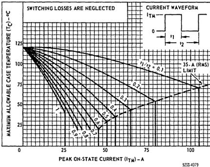
Fig. 5 - Maximum allowable case-temperature vs. peak on-state current.
