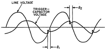
Fig. 7 – Voltage waveforms of double-time-constant control circuit.
