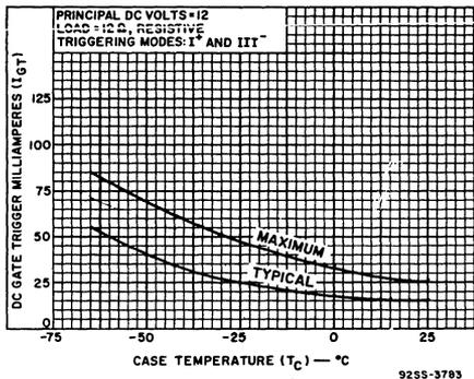
Fig. 12 — DC gate-trigger current (for I<sup>+</sup> and III<sup>-</sup> triggering modes) vs. case temperature.
