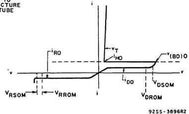
Fig. 2 - Principal voltage-current characteristic for S3702S and S3703SF.
