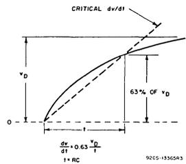
Fig. 16—Rate of rise of off-stage voltage with time (defining critical dv/dt).
