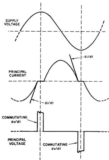
Fig. 14 — Waveshapes of commutating  $dv/dt$  characteristics.
