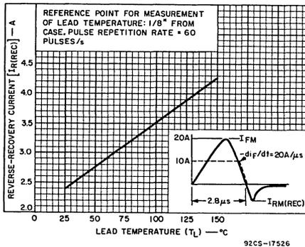
Fig. 9 — Reverse-recovery current vs. lead temperature.
