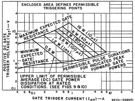
Fig. 12—Typical forward-biased gate characteristics.
