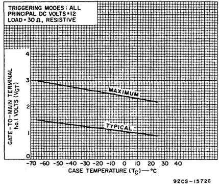
Fig. 12 — DC gate-trigger voltage vs. case temperature.
