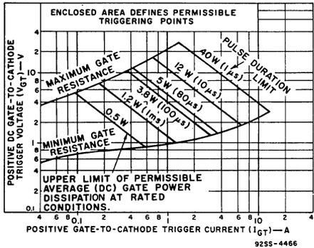
Fig. 14—Typical forward-biased gate trigger characteristics.
