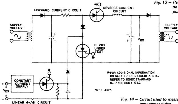
Fig. 14 - Circuit used to measure turn-off time ( $t_q$ ), rectangular pulse.
