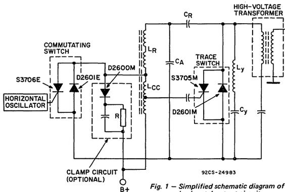
Fig. 1 - Simplified schematic diagram of horizontal output circuit.
