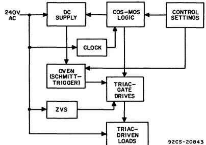
Fig. 11—Block diagram of a central-processor control.
