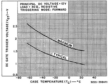
Fig. 10—DC gate-trigger voltage (forward) vs. case temperature.
