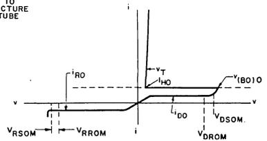
Fig. 2 - Principal voltage-current characteristic for S3702S and S3703SF.
