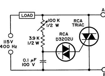
NOTE: For incandescent lamp loads which produce burnout current surges with  $I^2t$  values greater than 2.5 ampere<sup>2</sup> seconds, connect a 10-ohm resistor of appropriate power rating in series with the load. This rating can be determined as follows:
