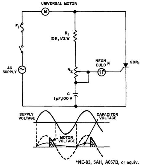
Fig.4 - Half-wave motor control with no regulation.
