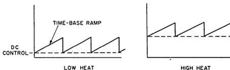
Fig. 20 — Proportional-controller waveshapes.
