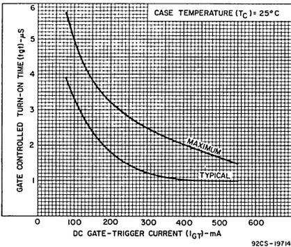
Fig. 11 - Turn on time vs. gate-trigger current.
