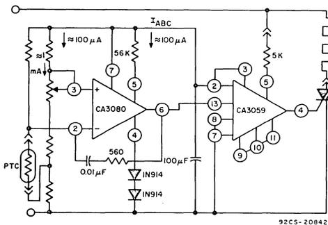
Fig. 7—Schematic diagram of circuit for use with low-resistance sensor.
