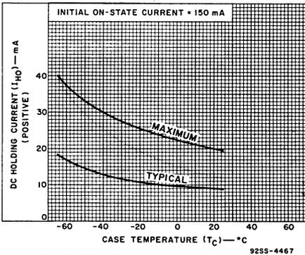
Fig. 15—DC holding current vs. case temperature.
