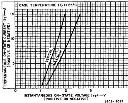
Fig. 7 — On-state current vs. on-state voltage (surge condition).
