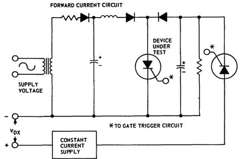
RE-APPLIED FORWARD BLOCKING VOLTAGE SUPPLY
