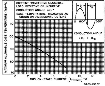
Fig. 3 — Allowable case temperature vs. on-state current.
