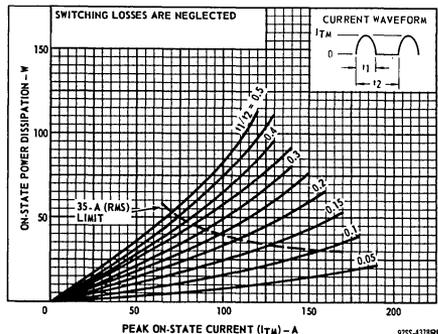
Fig. 2 — Power dissipation vs. peak on-state current.
