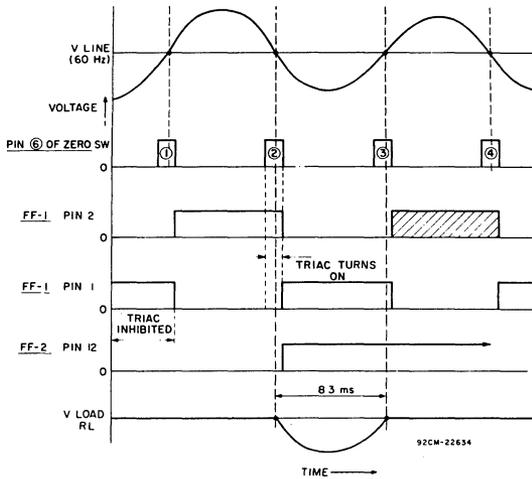
Fig. 53 - Timing diagram for the power one-shot control.
