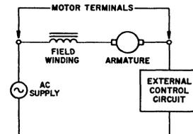
Fig.1 - Schematic diagram for a series-wound universal motor.
