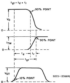
Fig. 15 — Relationship between off-state voltage, on-state current, and gate-trigger voltage showing reference points for definition of turn-on time (t<sub>gt</sub>).
