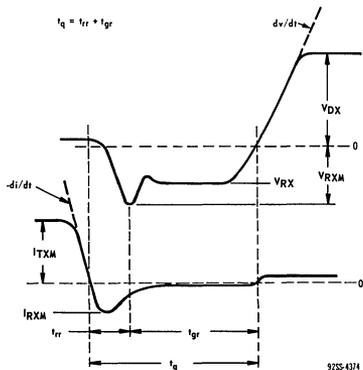
Fig. 8—Relationship between off-state voltage, reverse voltage, on-state current, and reverse current showing reference points defining turn-off time ( $t_q$ ).
