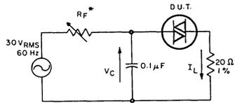
\* ADJUST FOR ONE FIRING IN HALF CYCLE
