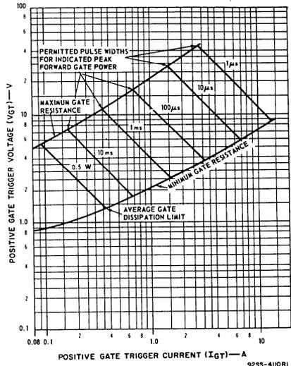
Fig.8—Gate pulse characteristics for forward triggering mode.
