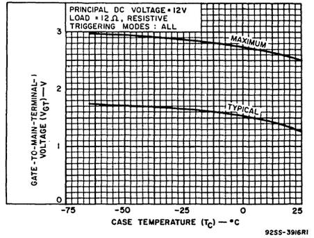
Fig. 14 - DC gate-trigger voltage vs. case temperature.
