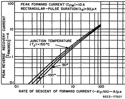
Fig. 11 — Typical peak reverse-recovery current vs. rate of descent of forward current for D2600M, D2601E, and D2601M.
