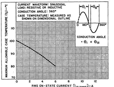
Fig. 3 - Allowable case temperature vs. on-state current.
