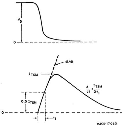
Fig. 16—Rate-of-change of on-state current with time (defining  $di/dt$ ).
