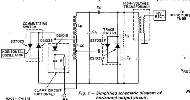
Fig. 1 - Simplified schematic diagram of horizontal output circuit.
