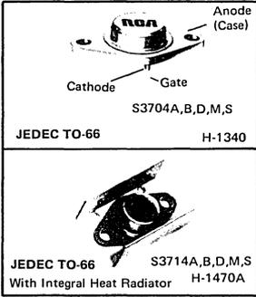
RCA-S3704 and S3714-series types are all-diffused, silicon controlled rectifiers (reverse-blocking triode thyristors) designed for inverter applications such as ultrasonics, choppers, regulated power supplies, induction heaters, cycloconverters, and fluorescent lighting. These types may be used at frequencies up to 25 kHz.
