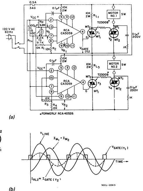
Fig. 32 - Dual output, over-temperature controller (a) circuit, (b) voltage and current waveforms.
