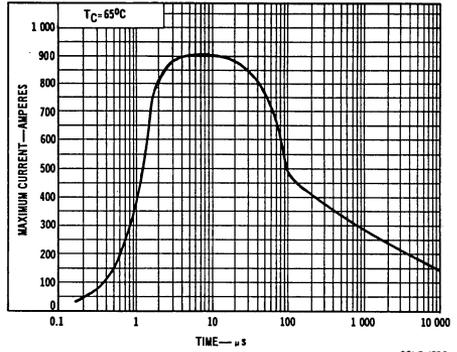
Fig. 7—Maximum current as a function of time.
