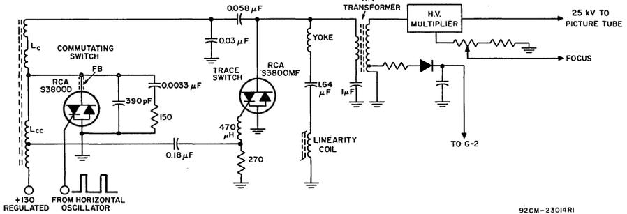
Fig. 6—System designed to operate from a regulated supply of approximately 130 volts.
