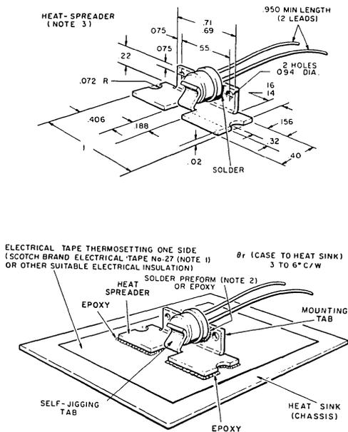
*Fig.7 - Self-jigging heat spreader.*
