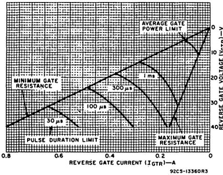
Fig. 8—Reverse gate voltage vs. reverse gate current.
