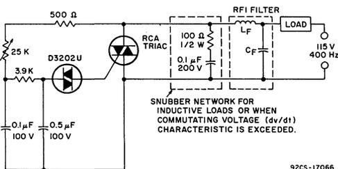
Fig. 16 — Typical phase-control circuit for operation at 400 Hz.
