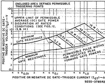
Fig. 11 - Gate-pulse characteristics for all triggering modes.
