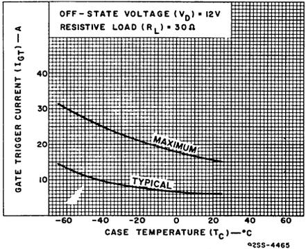
Fig. 12—DC gate-trigger current (forward) vs. case temperature.
