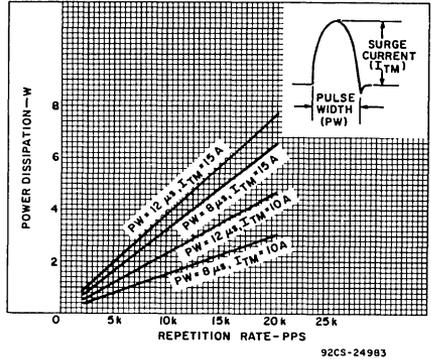
Fig. 7 - Dissipation vs. repetition rate for S3702S and S3703SF
