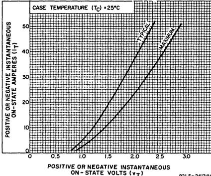
Fig. 7 - On-state current vs. on-state voltage.
