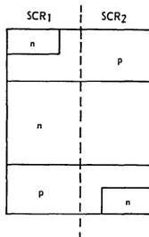
Fig. 12 - Structure of a triac.
