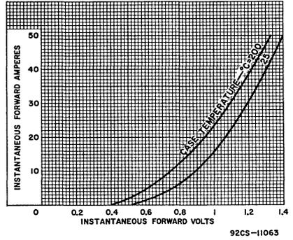
Fig. 5 - Current-Multiplying-Factor Chart for Polyphase and DC operation for all Types and corresponding reverse-polarity versions. Fig. 6 - Typical Forward Characteristics for all Types and corresponding reverse-polarity versions.
