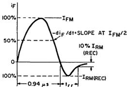
Fig. 8 - Oscilloscope display and test circuit for measurement of reverse-recovery time for D2101S, D2103S, and D2103SF.
