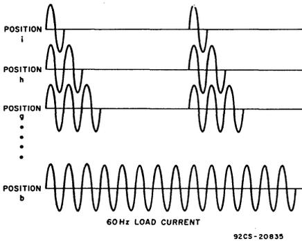
Fig. 16— Power-output waveforms for the circuit of Fig. 12.
