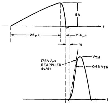
$I_{TM} = 8$  A,  $V_{TM} = V_{DROM}$ , reapplied  $dv/dt = 175$  V/ $\mu s$  (measured from 0 to 0.63 of  $V_{TM}$ ), negative gate voltage source = -24 V, source impedance = 15  $\Omega$ . 92CS-24045
