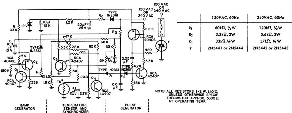
NOTE: ALL RESISTORS 1/2 W .510% UNLESS OTHERWISE SPECIFIED. THERMISTOR APPROX. 3000 Ω AT OPERATING TEMP.
