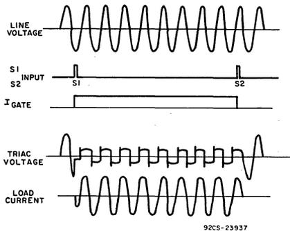
Fig. 3—Triac current and voltage waveforms as a function of control-circuit inputs for resistive load.
