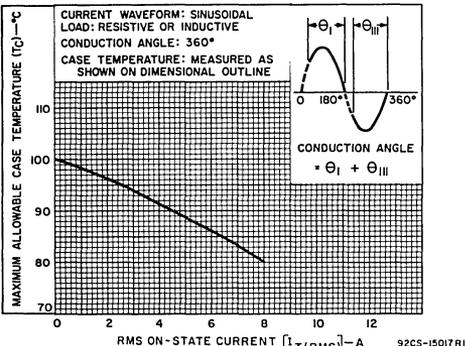
Fig. 3 - Maximum allowable case temperature vs. on-state current.
