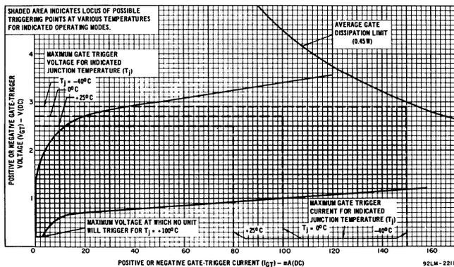
Fig. 11—Gate characteristics for  $I^-$  and  $III^t$  triggering modes.
