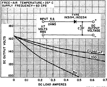
Fig.6— Typical operation characteristics of types 1N3194 and 1N3254 in half-wave rectifier service.
