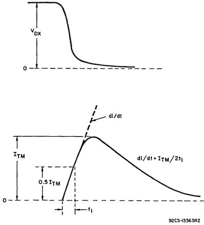
Fig. 1—Waveshape of di/dt rating test.
