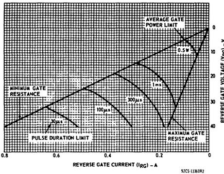
Fig. 5—Reverse gate voltage vs. reverse gate current.
