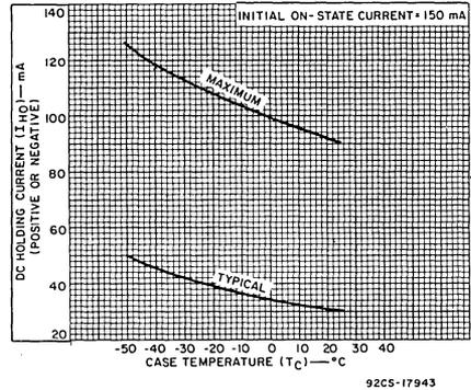
Fig. 6 - DC holding current vs. case temperature.
