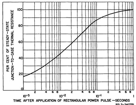
Fig. 12 - Transient junction-to-case thermal resistance vs. time.
