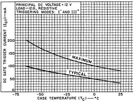
Fig. 9 - DC gate-trigger current vs. case temperature (I<sup>+</sup> & III<sup>+</sup> modes).
