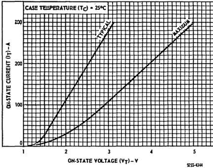
Fig. 13—Variation of on-state current with on-state voltage.
