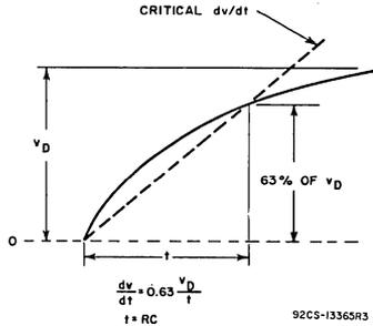
Fig. 15—Rate of rise of off-state voltage with time (defining critical  $dv/dt$ ).
