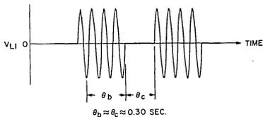
Fig. 15— Timing of thyristor flasher.
