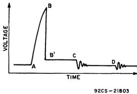
Fig. 1 - Ignition-voltage waveshape.
