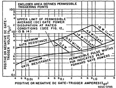
Fig. 10 - Gate pulse characteristics for all triggering modes.
