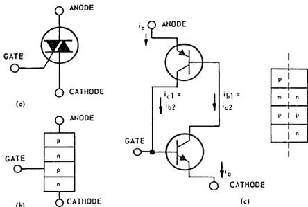
Fig. 1 - Two-transistor analogy of an SCR: (a) schematic symbol of SCR; (b) p-n-p structure represented by schematic symbol; (c) two-transistor model of SCR.
