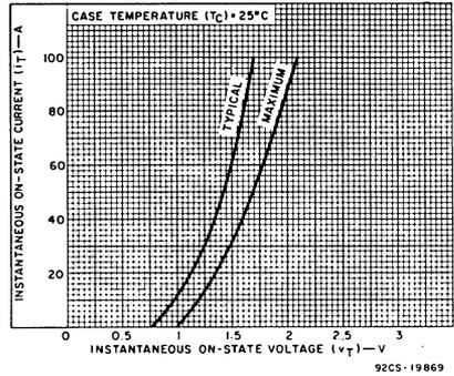
Fig.6—Instantaneous on-state current vs. on-state voltage.
