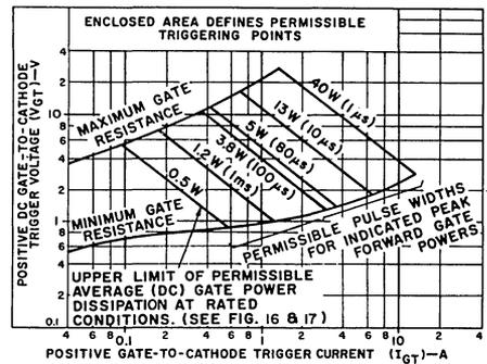
Fig. 15—Gate pulse characteristics for forward triggering mode.
