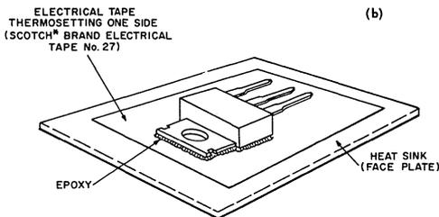
Fig.13 - Examples of isolated mounting of triacs.
