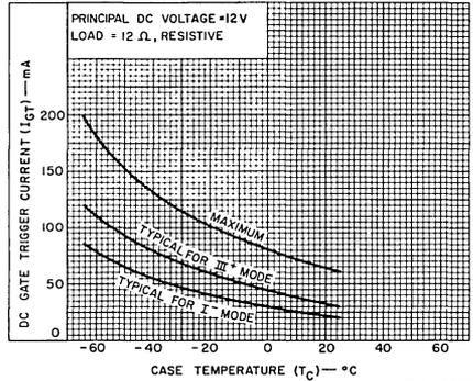
Fig. 13—DC gate-trigger current (for I<sup>-</sup> and III<sup>+</sup> triggering modes) vs. temperature.
