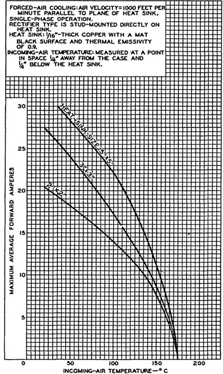
Fig. 3 - Rating Chart III for Types 1N248-C, 1N249-C, 1N250-C, 1N1195-A, 1N1196-A, 1N1197-A, 1N1198-A, and corresponding reverse-polarity versions.
