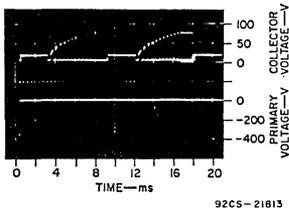
Fig. 16 — Collector voltage of the inverter output transistor Q1 (top) and ignition-coil primary voltage (bottom) as functions of time (2000 r/min;  $V_{CC} = 12$  V).
