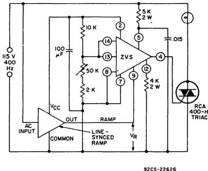
Fig. 45 — Circuit diagram for 400-Hz zero-voltage-switched lamp dimmer.
