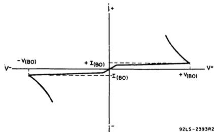
Fig.1—Voltage-current characteristic for both types.
