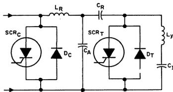
Fig. 12 — Circuit configuration showing the addition of auxiliary capacitor  $C_A$  and current and voltage waveforms showing the effect of this capacitor.
