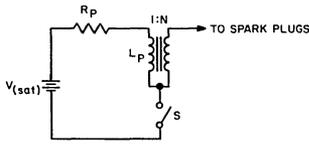
Fig. 2 - Basic inductive-discharge ignition circuit (Kettering system).
