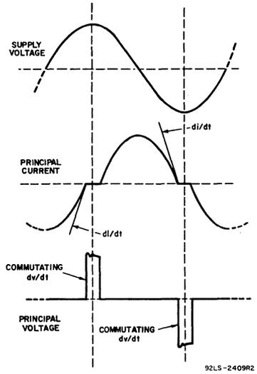
Fig. 5 - Oscilloscope display of commutating dv/dt.
