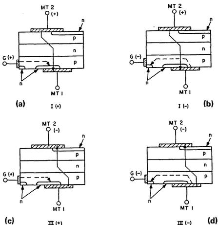
Fig. 7 - Current flow in a triac.
