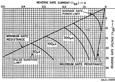
Fig. 13—Reverse gate voltage vs. reverse gate current.
