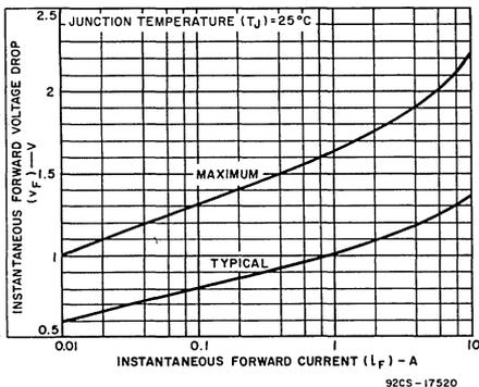
Fig. 3 — Forward-voltage drop vs. forward current.
