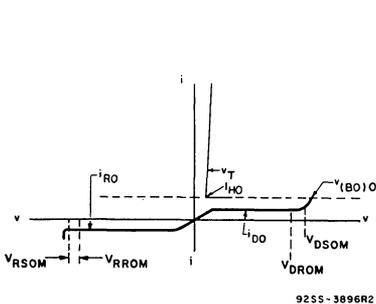
Fig. 1 — Principal voltage-current characteristic.
