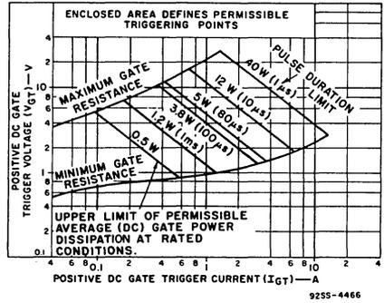
Fig. 7—Gate pulse characteristics for forward triggering mode.
