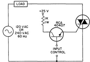
Fig. 12 — AC Triac Switch Control From DC Input: at 120 VAC, Y = T2700B; at 240 VAC, Y = T2700D.
