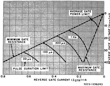
Fig.9—Reverse gate voltage vs. reverse gate current.
