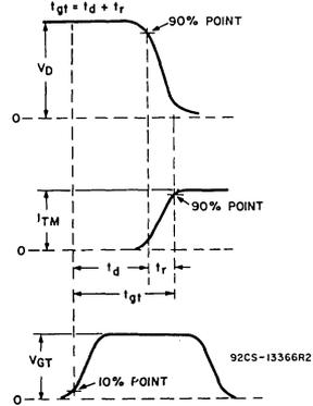
Fig. 15 - Relationship between off-state voltage, on-state current, and gate-trigger voltage showing reference points for definition of turn-on time ( $t_{gt}$ ).
