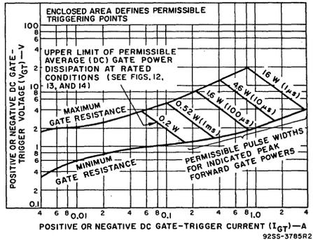
Fig. 10—Gate pulse characteristics for all triggering modes.
