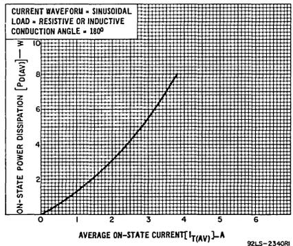
Fig. 2— Power dissipation vs. average on-state current.
