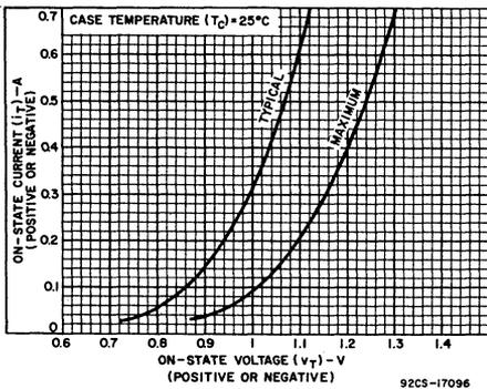
Fig. 6 — On-state current vs. on-state voltage (steady-state condition).
