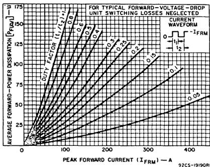
Fig.6—Average forward-power dissipation for typical forward-voltage-drop unit.
