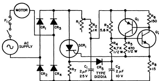
Q<sub>1</sub>, Q<sub>2</sub> - Complementary pair of general-purpose p-n-p and n-p-n transistor
