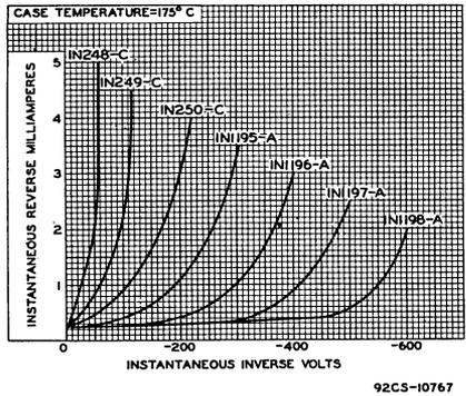
Fig. 7 - Typical Reverse Characteristics for Types 1N248-C, 1N249-C, 1N250-C, 1N1195-A, 1N1196-A, 1N1197-A, 1N1198-A, and corresponding reverse-polarity versions.
