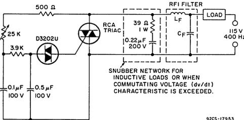
Fig. 17 — Typical phase-control circuit for operation at 400 Hz.
