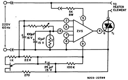
Fig. 17 - Schematic diagram of proportional zero-voltage-switching control.
