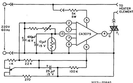
Fig. 9—Schematic diagram of proportional zero-voltage switching control.
