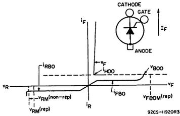
Fig. 1 - Typical E-I Characteristic of Silicon Controlled-Rectifier.
