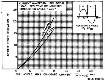
Fig. 7— Power dissipation curve.
