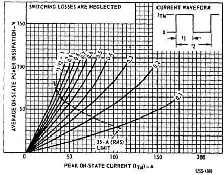
Fig. 4 - Power dissipation vs. peak on-state current.
