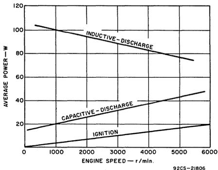
Fig. 6 — Ignition power requirements
