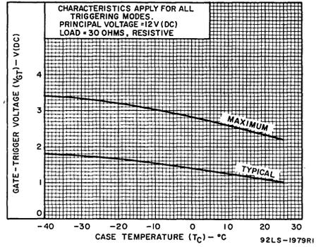
Fig. 11 — DC Gate-trigger voltage characteristics for all types.
