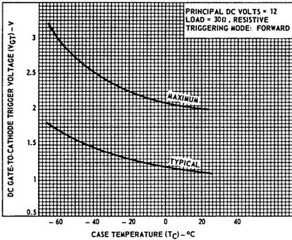
Fig. 13—DC gate-trigger voltage vs. case temperature.
