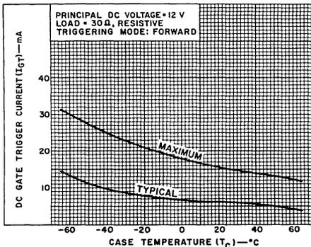
Fig. 16—DC gate-trigger current (forward) vs. case temperature.
