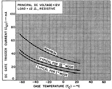
Fig. 12 - DC gate-trigger current (for I<sup>+</sup> and III<sup>-</sup> triggering modes) vs. case temperature.
