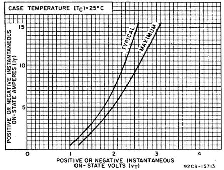
Fig. 7 — On-state current vs. on-state voltage.
