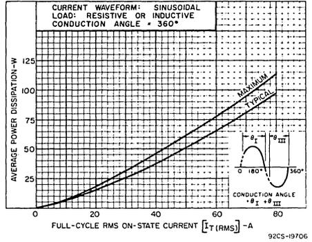
Fig. 2 - Power dissipation vs. on-state current.
