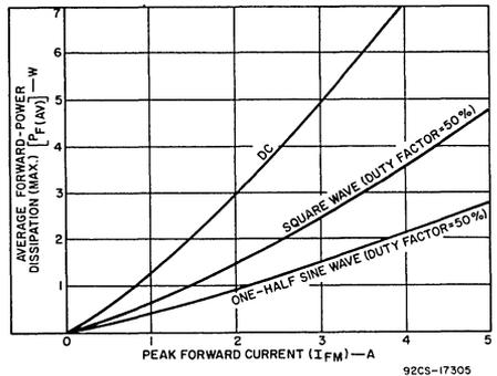
Fig. 2 - Variation of peak forward-power dissipation with peak forward current.
