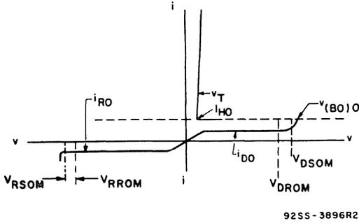
Fig. 1—Principal voltage-current characteristics.
