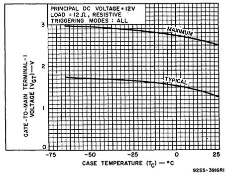
Fig. 11 - DC gate-trigger voltage vs. case temperature.
