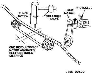
Fig. 39 — Step-and-punch machine.
