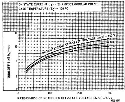
Fig. 14 - Typical variation of turn-off time with rate-of-rise of reapplied off-state voltage (rectangular pulse).
