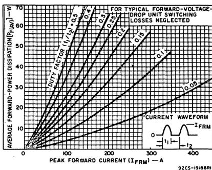
Fig.4—Average forward-power dissipation for typical forward-voltage-drop unit.
