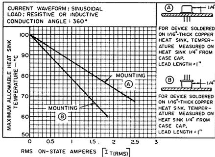
Fig. 4 - Maximum allowable heat-sink temperature vs. on-state current.
