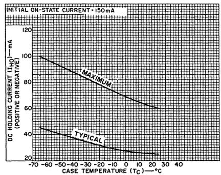
Fig. 6 - DC holding current vs. case temperature.
