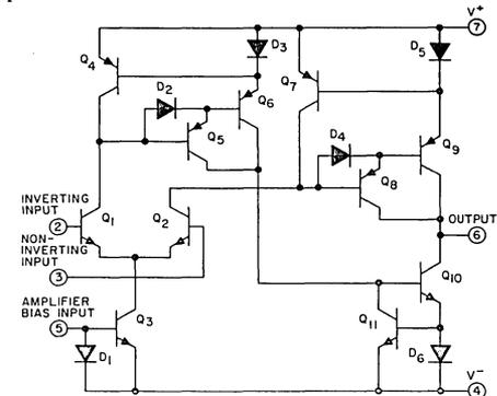
Fig. 8—Schematic diagram of the CA3080. 92CS-17587
