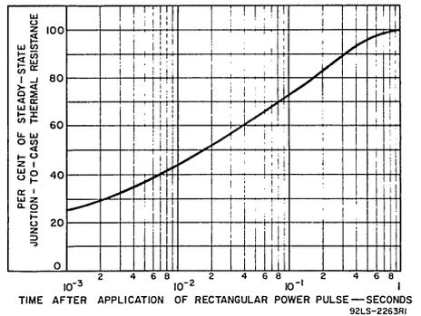
Fig. 16 — Transient junction-to-case thermal resistance vs. time.
