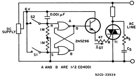
Fig. 2—Two dual-input NOR gates connected to form set-reset flip-flop.
