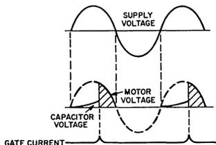
Fig.5 - Half-wave motor control with no regulation.
