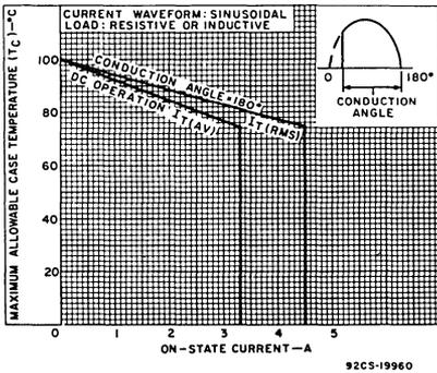
Fig. 3—Maximum allowable case temperature vs. on-state current.
