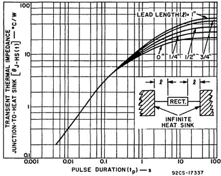
Fig. 5—Typical variation of transient thermal impedance with pulse duration for several lead lengths.
