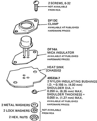
Note: Maximum torque applied to mounting flange is 12 in.-lb.
