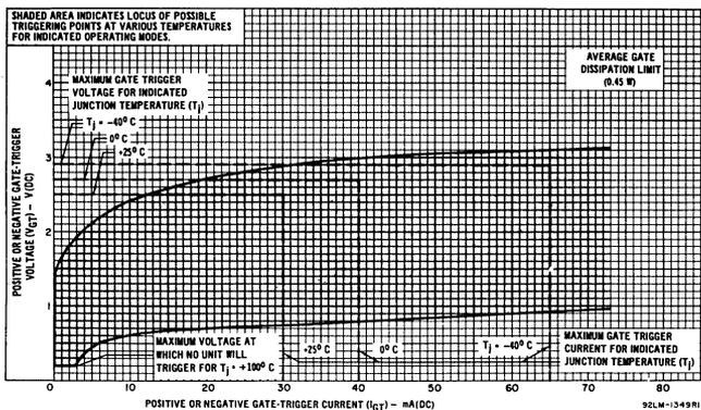
Fig. 10—Gate characteristics for  $I^t$  and  $III^t$  triggering modes.
