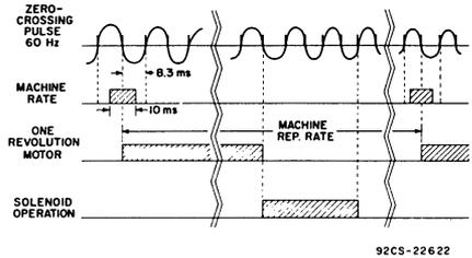
Fig. 41 — Timing diagram for proposed solid-state machine control.
