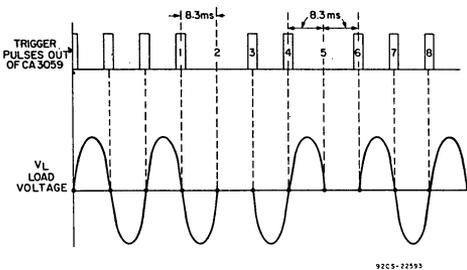
Fig. 10 - Half-cycling phenomenon in the zero-voltage switch.
