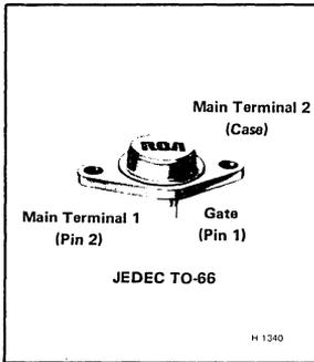
RCA T4700B and T4700D\* are gate-controlled full-wave ac silicon switches. They are designed to switch from an off-state to a conducting state for either polarity of applied voltage with positive or negative gate triggering.
