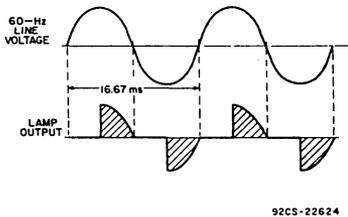
Fig. 43 — Waveforms for 60-Hz phase-controlled lamp dimmer.
