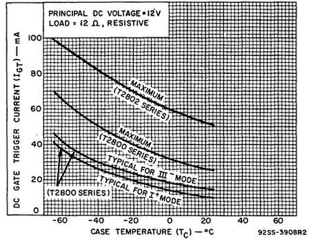
Fig. 9 - DC gate-trigger current (for I<sup>+</sup> and III<sup>-</sup> triggering modes) vs. case temperature.
