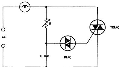
Fig. 27 - Basic triac-diac light-dimmer control circuit.
