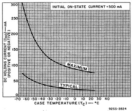
Fig. 6 - DC holding current vs. case temperature.
