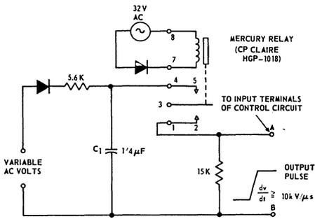
Fig. 15 - Circuit used to generate fast rising transients.
