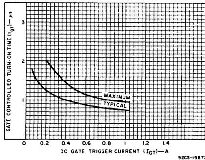
Fig.12—Gate-controlled turn-on time vs. gate trigger current.
