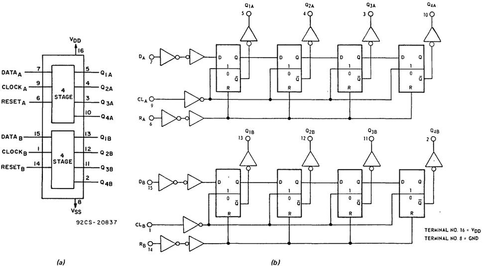
Fig. 14— Logic and block diagram of the CD4015A.
