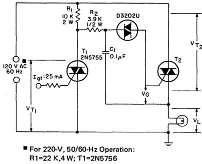
Fig. 12— Negative-logic bulb-switching circuit.
