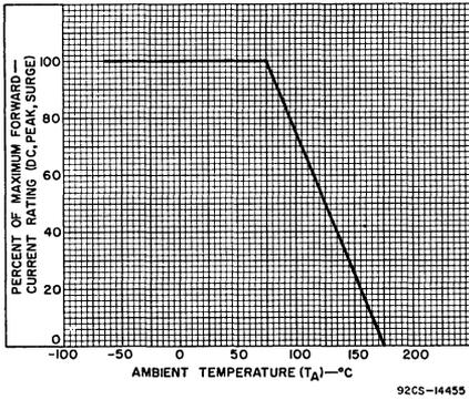
Fig. 1 - Rating Chart for Types 1N5211 through 1N5218.
