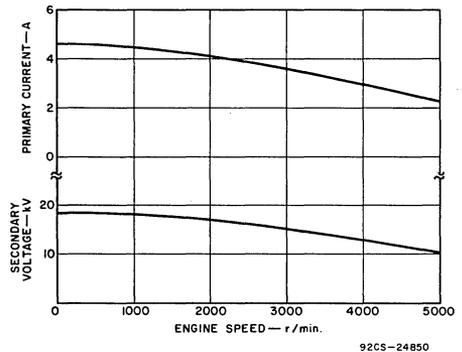
Fig. 3 - Performance of conventional inductive-discharge ignition system.
