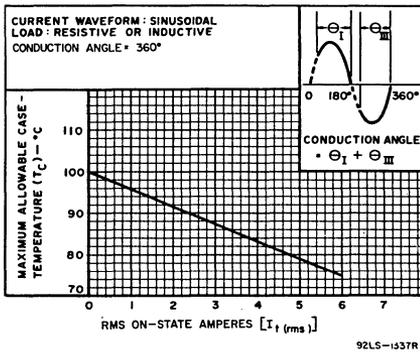
Fig. 3 - Allowable case temperature vs. on-state current.
