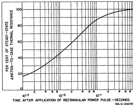
Fig. 15 — Transient thermal resistance (junction-to-case vs. time).
