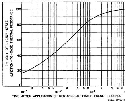
Fig. 12 - Transient thermal resistance vs. time (junction-to-case).
