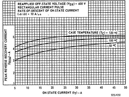
Fig. 10 - Typical variation of peak reverse-recovery current with on-state current (rectangular pulse).
