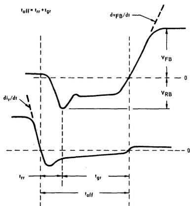
Fig. 10 - Waveshapes illustrating thyristor turn-off time.
