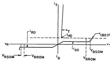
Fig. 2—Principal voltage-current characteristics.
