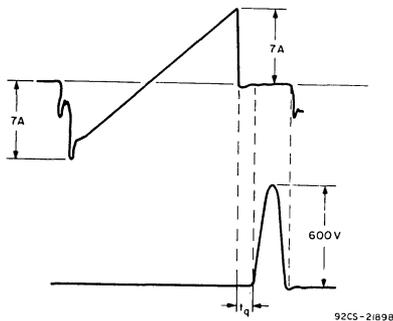
Fig. 4— Circuit-commutated turn-off time in trace ITR.
