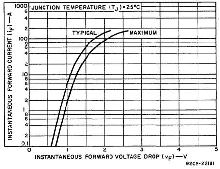
Fig.4 — Forward current vs. forward voltage drop.
