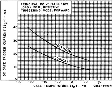
Fig. 9—DC gate-trigger current (forward) vs. case temperature.
