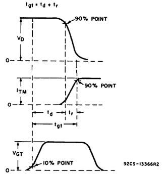
Fig. 13—Relationship between off-state voltage, on-state current, and gate-trigger voltage showing reference points for definition of turn-on time ( $t_{gt}$ ).
