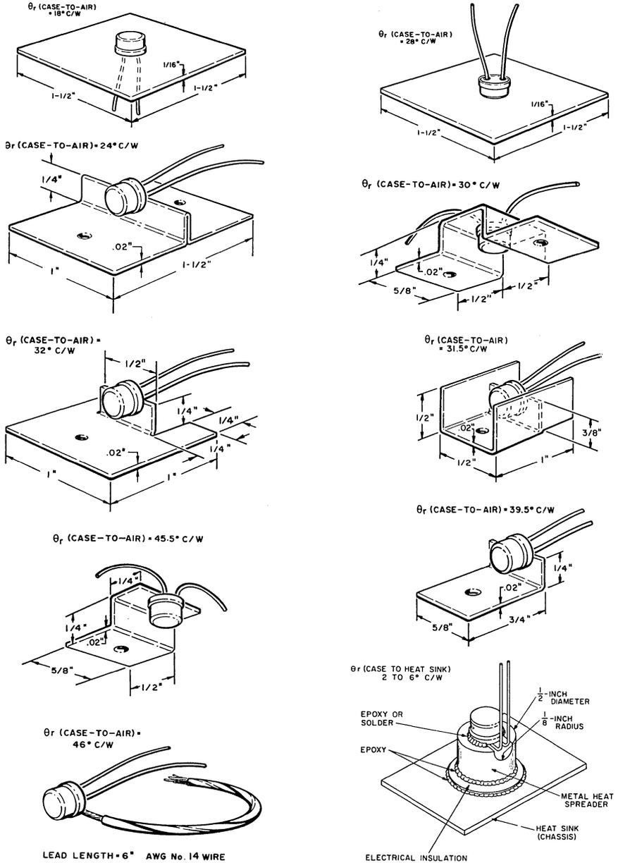
Fig.6 - Typical heat-sink heat-spreader configurations.
