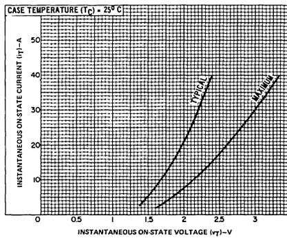
Fig.5 - Instantaneous on-state current vs. on-state voltage for S3705M and S3706E. 92LS2344R1
