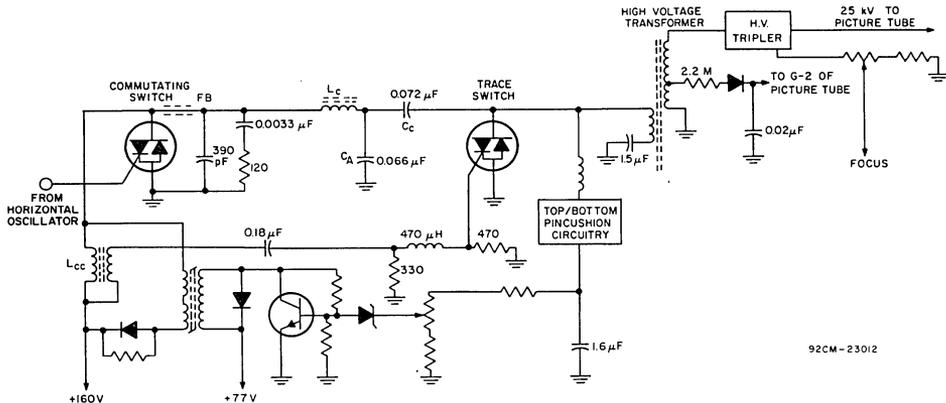
Fig. 4— ITR's in a deflection circuit originally developed to use separate SCR's and rectifiers.
