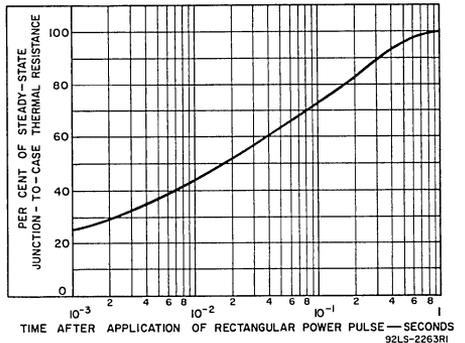
Fig. 12 - Transient junction-to-case thermal resistance vs. time.
