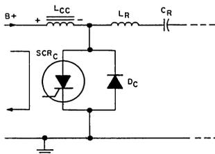
Fig. 10 — Circuit elements and current path used to supply energy to the charging choke  $L_{CC}$  during period from the start of retrace switching action to the end of the first half of the retrace interval, time  $T_3$  to  $T_1$ .
