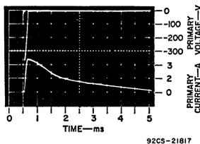
Fig. 20 — Primary voltage (top) and current (bottom) as a function of time (1-mH coil used in place of standard ignition coil, 2000 r/min;  $V_{CC} = 12$  V).
