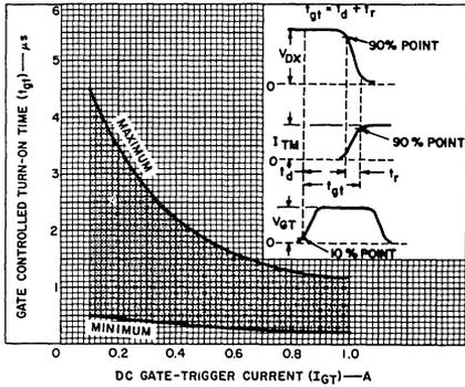
Fig. 10 - Turn-on time vs. gate-trigger current.
