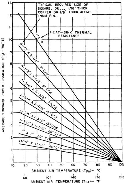
Fig. 3 - Guide to heat-sink area determination.
