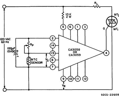
Fig. 27 – CA3058 or CA3059 on-off temperature controller.
