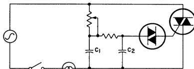
Fig.29 - "Double-time-constant" light-control circuit.
