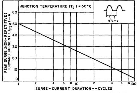
Fig. 3 - Peak surge (non-repetitive) forward current vs. surge-current duration for all types.
