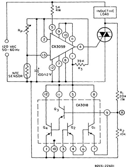
Fig. 8—Use of CA3058 or CA3059 together with CA3018 for switching inductive loads.
