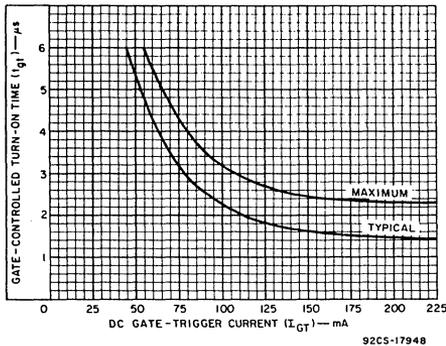
Fig. 11 - Turn-on time vs. gate trigger current.
