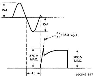
Fig. 2— Circuit-commutated turn-off time in commutating ITR.
