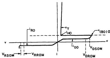
Fig. 2 - Principal voltage-current characteristic for S3705M and S3706E.
