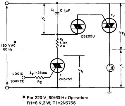
Fig. 10— Positive-logic bulb-switching circuit.
