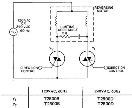
Fig. 15 — Reversing motor control.
