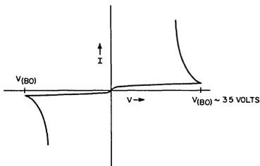
Fig. 2 - Voltage-current characteristic of a diac.
