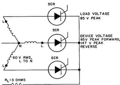
Fig. 7 shows a three-phase, half-wave circuit that uses three SCR's. In this application, the firing angle can be varied continuously from 30 to 145 degrees. It is desired to determine the resulting variation in the attainable load power. Current and voltage waveforms for SCR's in three-phase, half-wave circuits are shown in Fig. 8.
