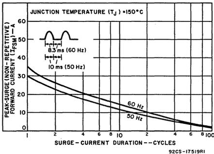
Fig. 9 - Peak-surge (non-repetitive) forward current vs. surge-current duration for D2600M, D2601E, and D2601M.
