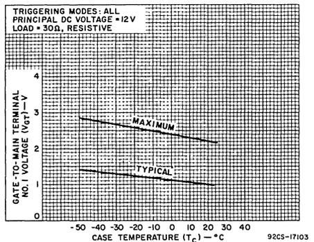
Fig. 13 — DC gate-trigger voltage vs. case temperature.
