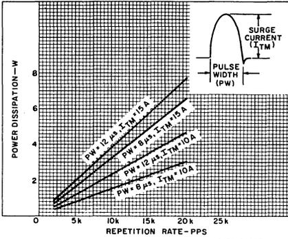
Fig. 3—Dissipation vs. repetition rate.
