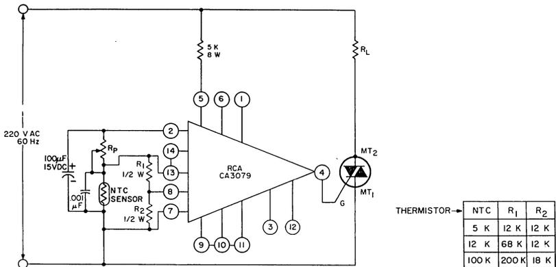
Fig. 6—CA3079 on-off controller with hysteresis.
