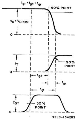
Fig. 2—Waveshapes of  $t_{gt}$  characteristics test.
