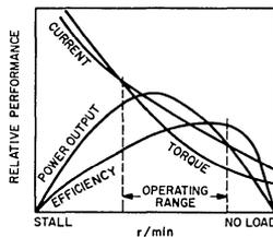
Fig. 2 - Typical performance curves for a universal motor.
