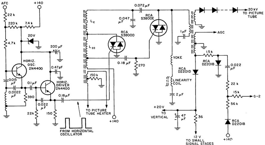
Fig. 7—Schematic diagram of a deflection circuit for a black and white receiver operating from a simple half-wave line rectifier with no regulation.
