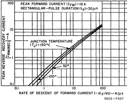
Fig. 11 — Typical peak reverse recovery current vs. rate of descent of forward current for D2101S, D2103S, and D2103SF.
