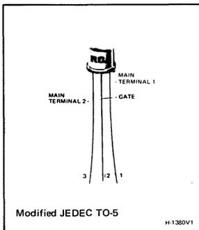
RCA T2304- and T2305-series triacs are gate-controlled full-wave silicon ac switches. They are designed to switch from an off-state to an on-state for either polarity of applied voltage with positive or negative gate triggering voltages.
