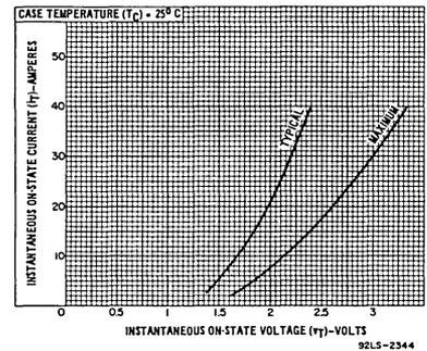
Fig. 13—On-state characteristics.
