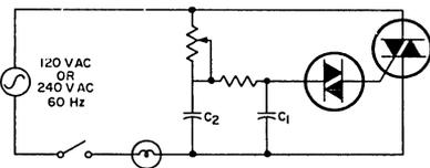
Fig. 6 - "Double-time-constant" light-control circuit.
