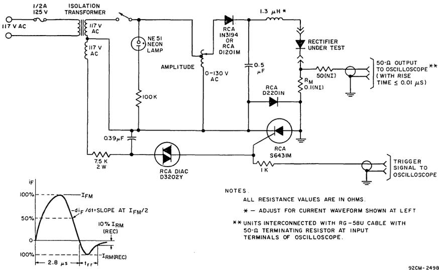
Fig. 8 — Oscilloscope display and test circuit for measurement of reverse-recovery time for D2600M, D2601E, and D2601M.
