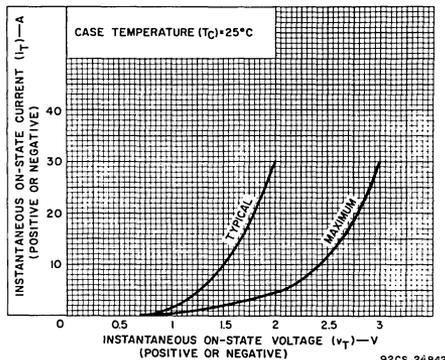
Fig. 6 - On-state current vs. on-state voltage.
