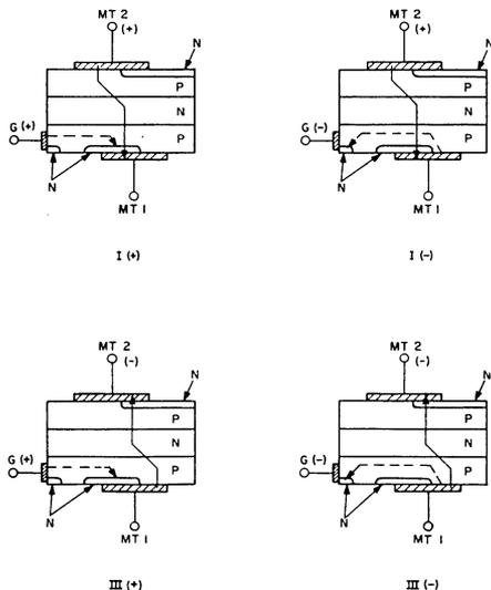
Fig. 2 — Current flow in a triac.
