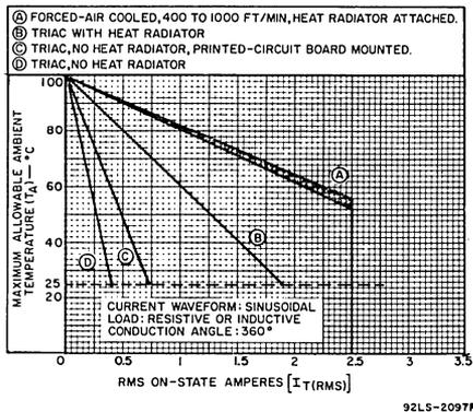
Fig. 5 - Maximum allowable ambient temperature vs. on-state current.
