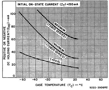
Fig. 7 - DC holding current vs. case temperature.
