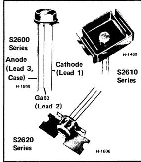
The S2600, S2610, and S2620 series are all-diffused, silicon controlled rectifiers (reverse-blocking triode thyristors) for capacitor-discharge ignition systems, high-voltage generators, and power-switching and control applications.
