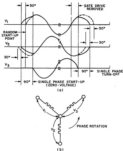
Fig. 4—Voltage phase relationship for a three-phase resistive load when the application of load power is controlled by zero-voltage switching: (a) voltage waveforms, (b) load-circuit orientation of voltages. (The dashed lines indicate the normal relationship of the phases under steady-state conditions. The deviation at start-up and turn-off should be noted.)
