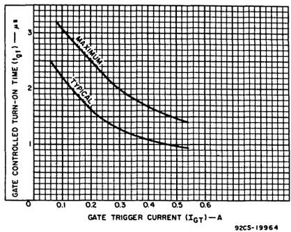
Fig. 11—Gate-controlled turn-on time vs. gate-trigger current.
