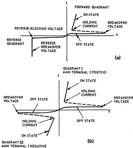
Fig. 4 - Principal voltage-current characteristics of SCR's and triacs.
