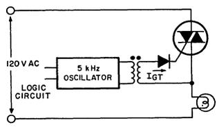
Fig. 18— Isolation transformer gate control.
