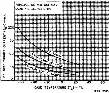
Fig. 13 - DC gate-trigger current for I<sup>-</sup> and III<sup>+</sup> triggering modes) vs. case temperature.
