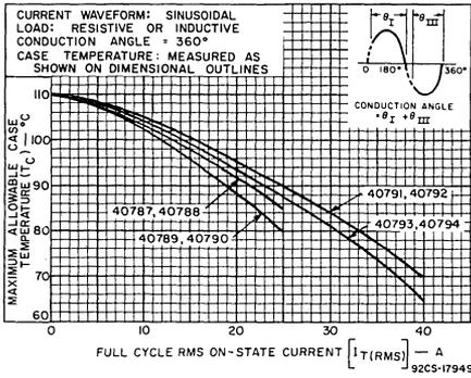
Fig. 3 - Maximum allowable case temperature vs. on-state current.
