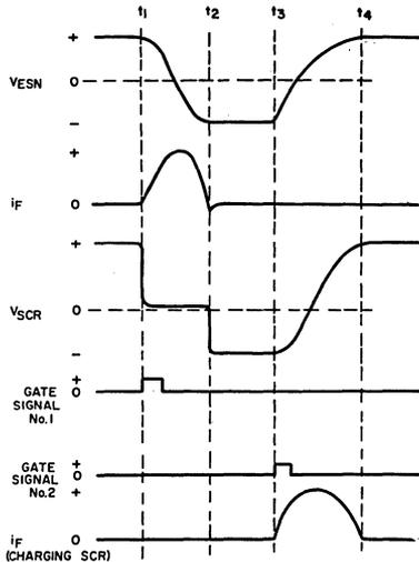
Fig.2 - Idealized waveforms for pulse-discharge circuit.
