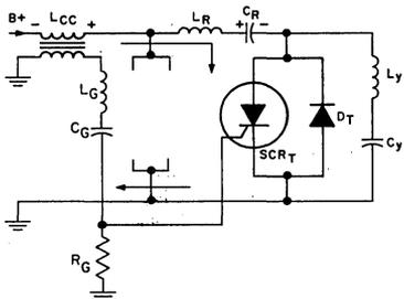
Fig. 11 — Effective configuration of the deflection circuit for resetting (application of forward bias to) the trace  $SCR_T$  and recharging the retrace capacitor  $C_R$ , during time interval from  $T_1$  to  $T_3$ .
