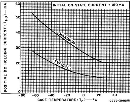
Fig. 11—Holding current (positive) vs. case temperature.
