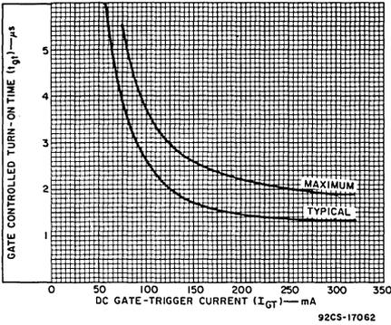
Fig. 12 - Turn-on time vs. gate-trigger current.
