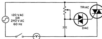
Fig. 3 - Basic triac-diac light-control circuit.
