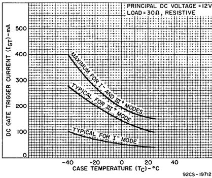
Fig. 9 - DC gate-trigger current vs. case temperature ( $I^-$  and  $I^{11-}$  modes).
