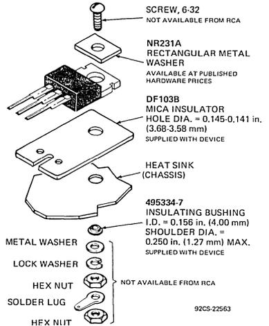
Note: Maximum torque applied to mounting flange is 8 in.-lb.
