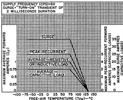
Fig.1 - Rating Chart for RCA-1N1763A and 1N1764A
