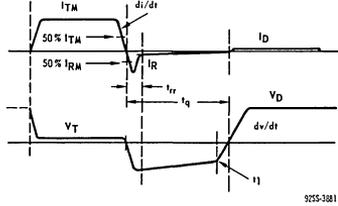
Fig. 5—Oscilloscope display for measurement of circuit commutated turn-off time ( $t_g$ ).
