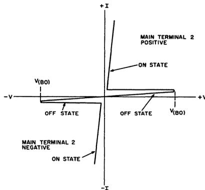
Fig. 1 - Voltage-current characteristic of a triac.
