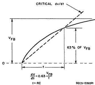
Fig. 1—Waveshape of critical  $dv/dt$  rating test.
