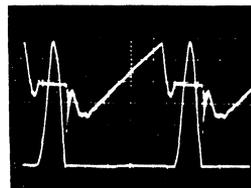
Fig. 5— Typical deflection-circuit waveforms for trace ITR.
