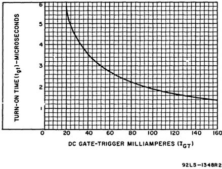
Fig. 9 - Typical turn-on time vs. gate-trigger current.
