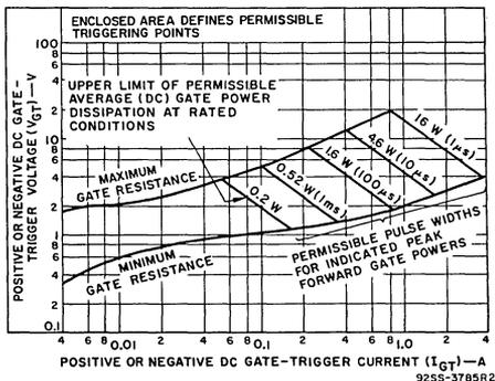
Fig. 5 - Gate pulse characteristics for all triggering modes.
