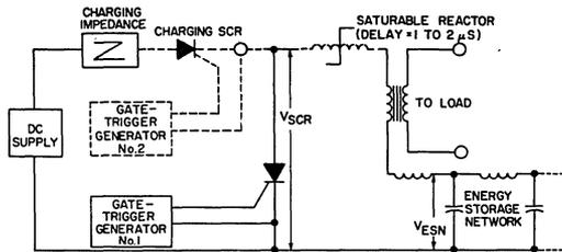
Fig.1 - Basic pulse modulator circuit.
