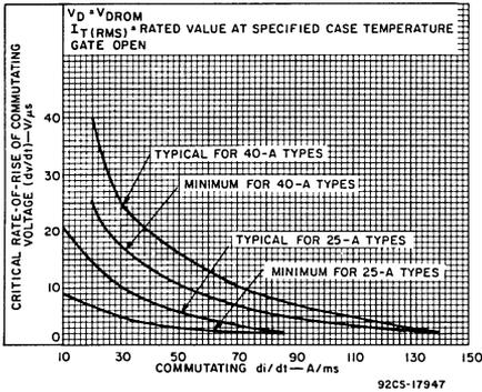
Fig. 13 — Commutating voltage vs. commutating current.
