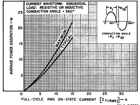
Fig. 2 - Power dissipation vs. on-state current.
