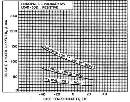
Fig. 8 - DC gate-trigger current vs. case temperature ( $I^+$  and  $I^{11+}$  modes).
