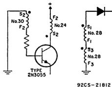
Fig. 15 - Details of inverter transformer (T<sub>1</sub>) shown in Fig. 14.
