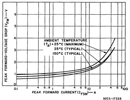
Fig. 2—Peak forward-voltage drop vs. peak forward current.
