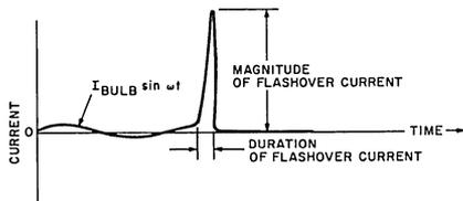
Fig. 3— Flashover current at peak voltage point.
