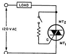
Fig. 2— Example of  $I_+$ ,  $III_-$  gating of triac.
