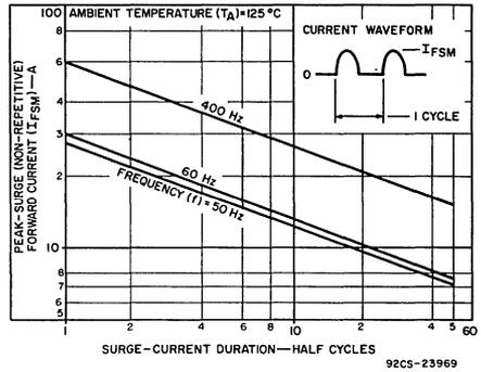
Fig. 2 - Peak-surge (non-repetitive) forward current vs. surge-current duration.
