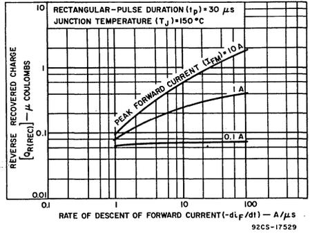
Fig. 12 - Reverse-recovered charge vs. rate of descent of forward current.
