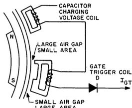
Fig. 12 - Magnetic advance for flywheel-charged capacitive-discharge system.
