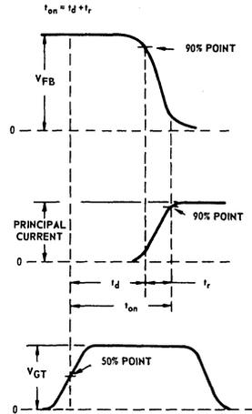
Fig. 8 - Waveshapes illustrating thyristor turn-on time.
