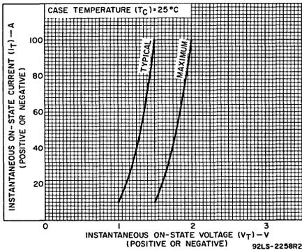
Fig. 5—On-state current vs. on-state voltage.
