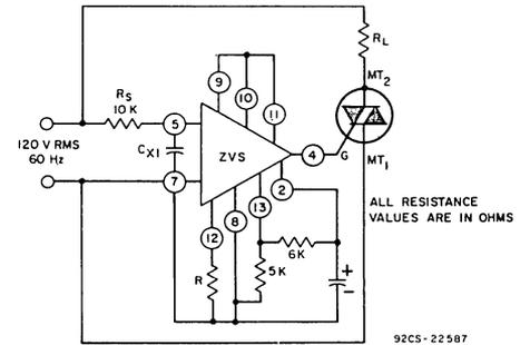
Fig. 4 — Use of a capacitor between terminals 5 and 7 to delay the output pulse of the zero-voltage switch.
