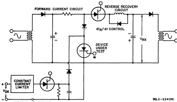
Fig. 8—Conventional turn-off-time test circuit.
