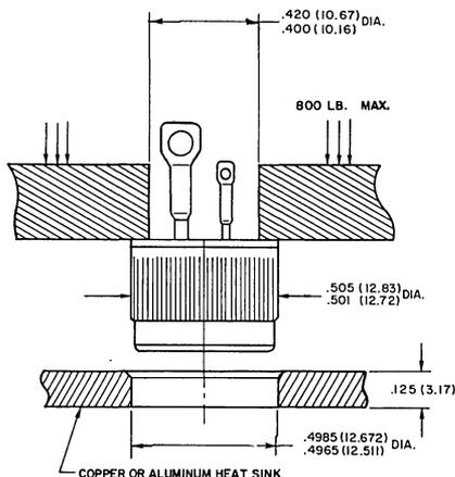
NOTE: Dimensions in parentheses are in millimeters
