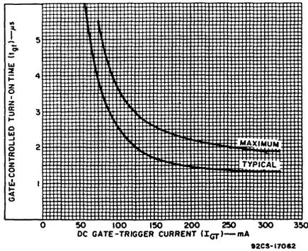
Fig. 15 - Typical turn-on time vs. gate-trigger current.
