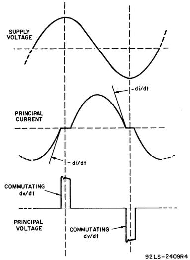
Fig. 5 — Oscilloscope display of commutating dv/dt.
