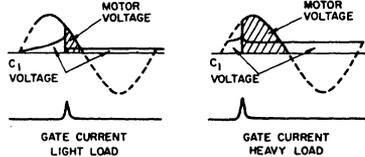
Fig.10 - Full-wave motor control with regulation.
