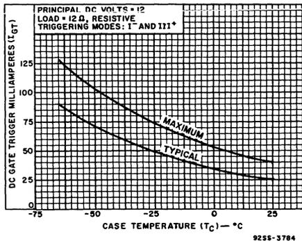
Fig. 13 — DC gate-trigger current (for I<sup>-</sup> and III<sup>+</sup> triggering modes) vs. case temperature.
