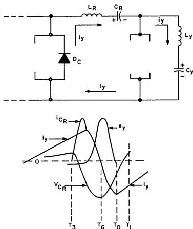
Fig. 8 — Effective configuration of the deflection circuit and operating voltage and current waveforms during the second half of retrace, time  $T_0$  to  $T_0$ .
