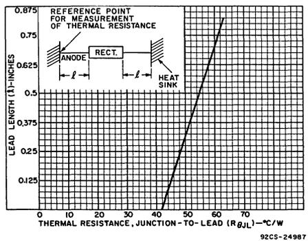
Fig. 14 — Junction-to-lead thermal resistance vs. lead length for D2600M, D2601E, and D2601M.
