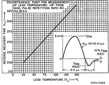
Fig. 9 - Typical variation of reverse recovery time with lead temperature for all types.
