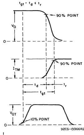
Fig. 12 - Relationship between off-state voltage, on-state current, and gate-trigger voltage showing reference points for definition of turn-on time ( $t_{gt}$ ).
