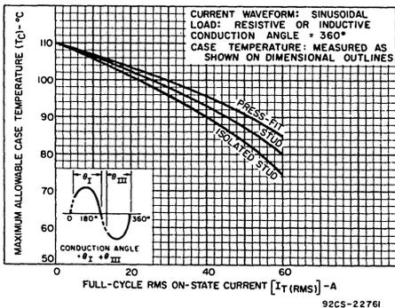
Fig. 3 - Maximum allowable case temperature vs. on-state current.
