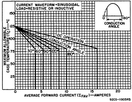
Fig. 2 - Rating Chart for Types 2N1842A through 2N1850A.
