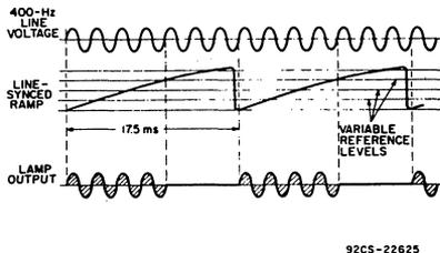
Fig. 44 — Waveforms for 400-Hz zero-voltage-switched lamp dimmer.
