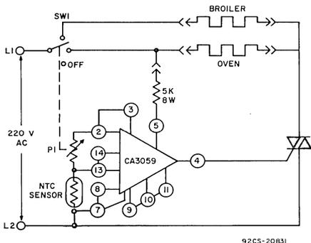
Fig. 3— Schematic diagram of basic oven control.
