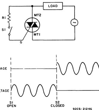
Fig. 4 - ON/OFF control, non-synchronized.
