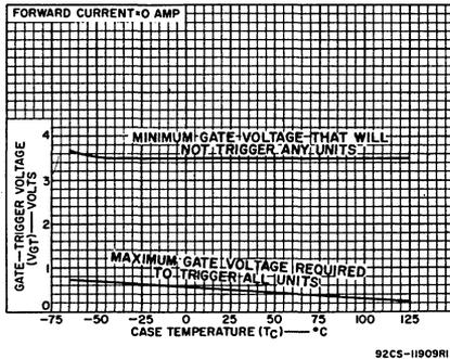
Fig. 8 - Gate Trigger-Voltage Characteristics for Types 2N1842A through 2N1850A.
