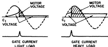
Fig.7 - Half-wave motor control using two-transistor regenerative triggering with regulation.
