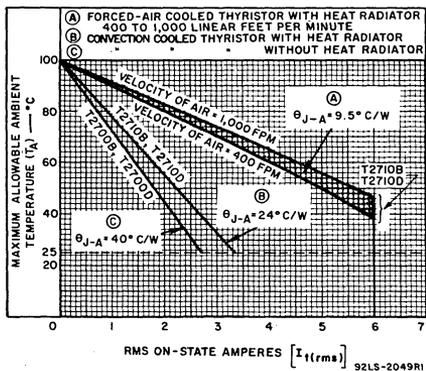
Fig. 16 — Maximum allowable ambient temperature vs. on-state current.
