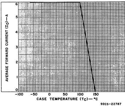
Fig. 1 — Average forward current vs. case temperature.
