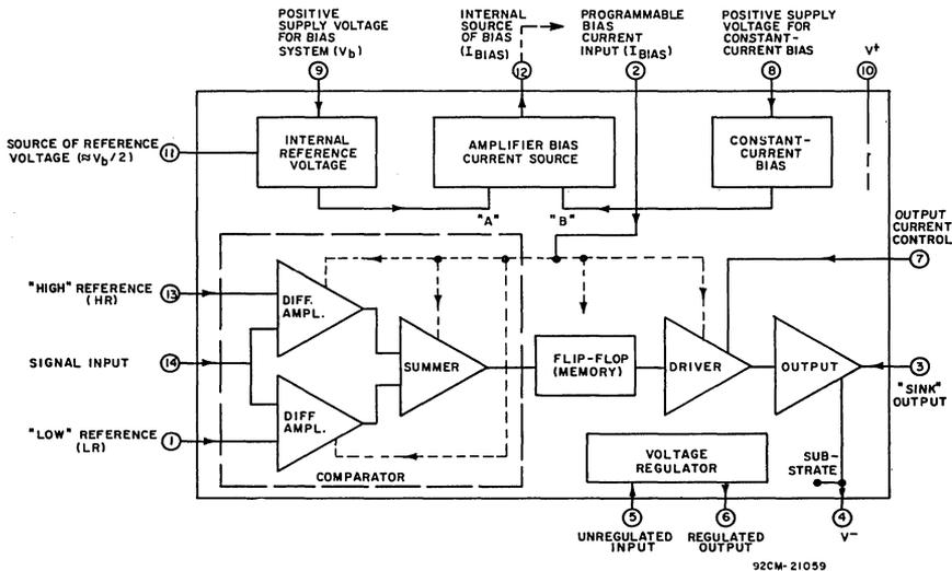
Fig. 14 - Block diagram of CA3099E integrated-circuit programmable comparator.
