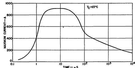
Fig.9- Maximum permissible current as a function of time after the initiation of turn-on.
