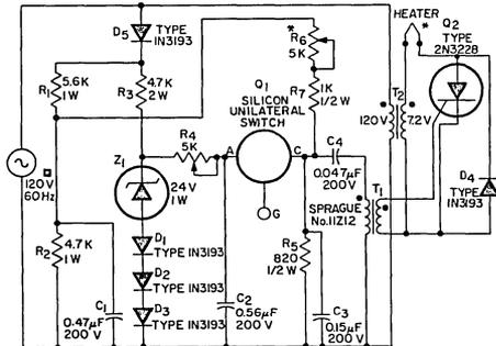
\*In the closed-loop regulator,  $R_6$  is replaced by a photo cell, and a potentiometer in series with a 6-volt incandescent lamp is connected in parallel with the heater terminals
