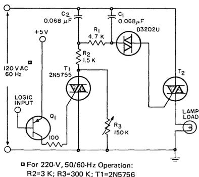
Fig. 8— A circuit including a filament pre-heat arrangement.
