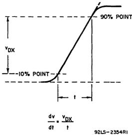
Fig. 12 - Rate-of-rise of off-state voltage with time (defining dv/dt).
