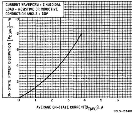
Fig. 4 - Power dissipation vs. average on-state current.
