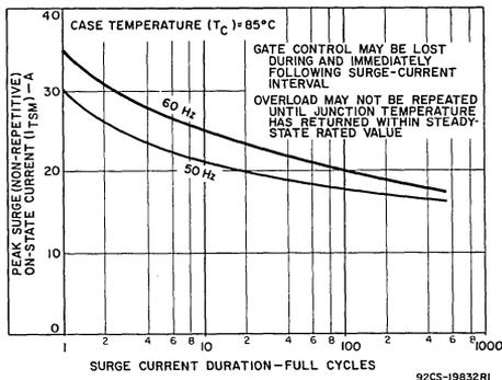
Fig. 6—Peak surge on-state current vs. surge cycles for all series.
