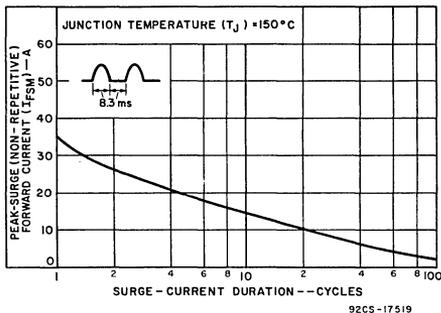
Fig. 2 — Peak-surge (non-repetitive) forward current vs. surge-current duration.
