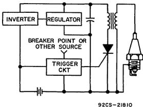
Fig. 13 - Block diagram of an inverter-charged ignition system.
