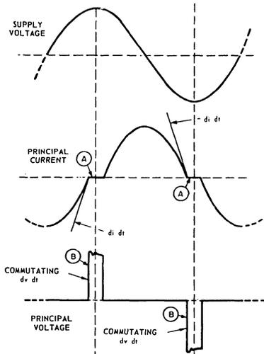
Fig. 13 - Waveshapes of commutating  $dv/dt$  characteristics.
