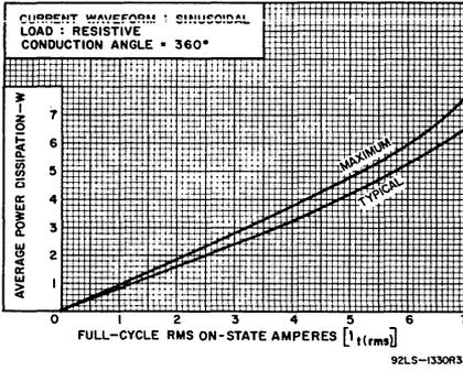
Fig. 2 - Power dissipation vs. on-state current.
