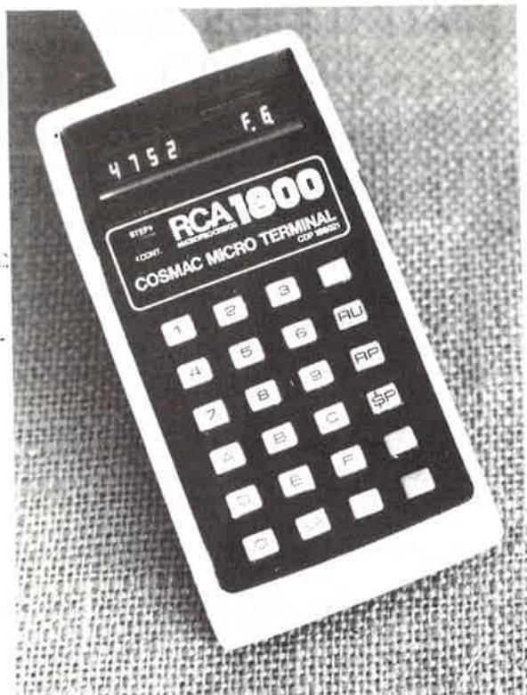
Fig. 16 – Photograph of RCA COSMAC Microterminal CDP18S021.
