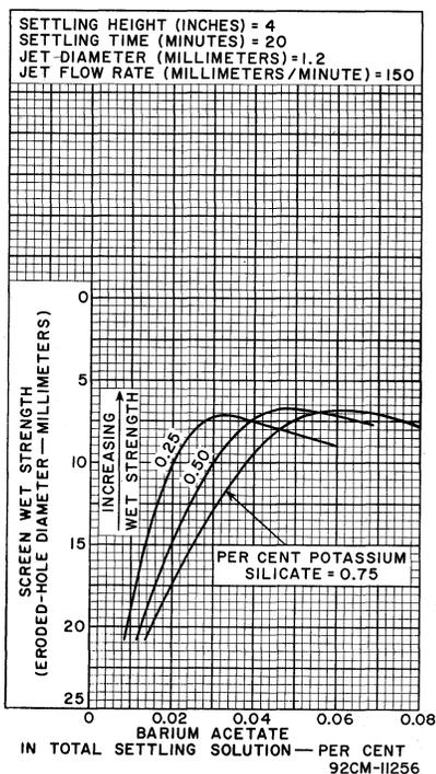
SCREEN REWET STRENGTH P4-SULFIDE PHOSPHOR BLEND RCA No.33-Z-387
