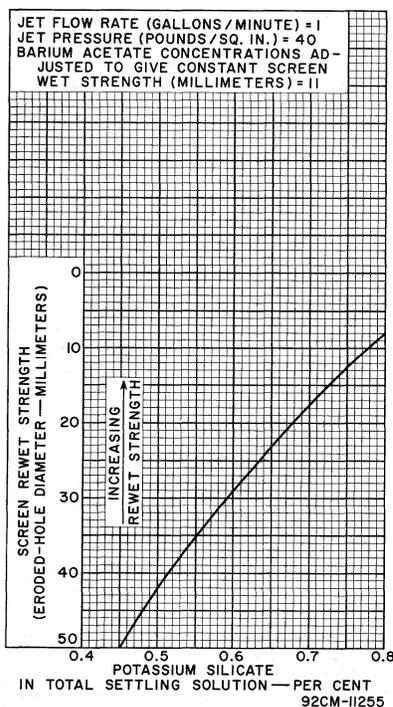
SCREEN WET STRENGTH P4-SULFIDE PHOSPHOR BLEND RCA No.33-Z-290
