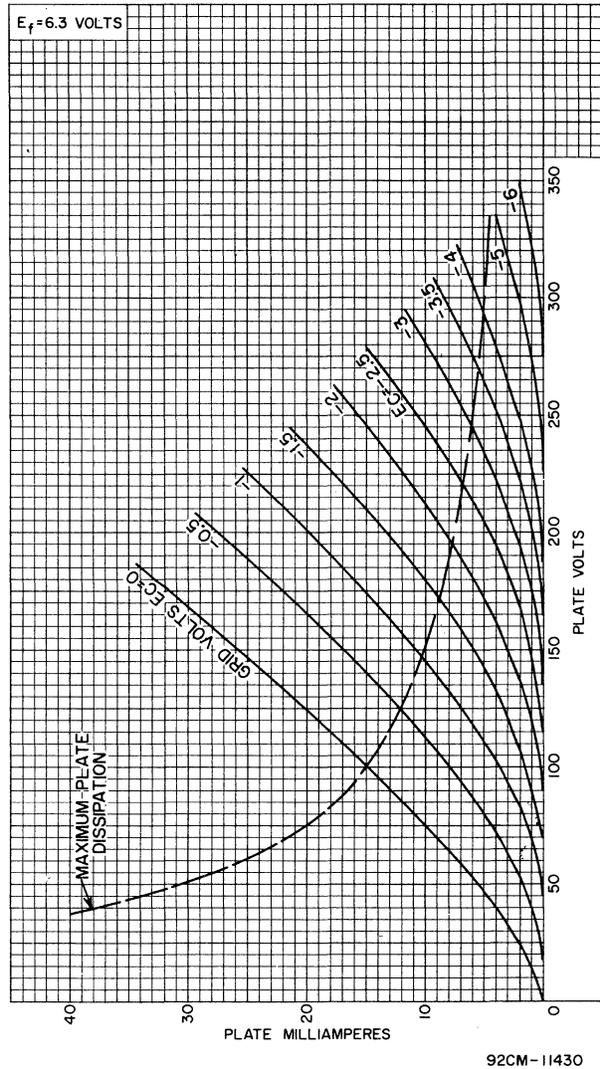
Fig. 2 - Average Plate Characteristics for Type 8058.
