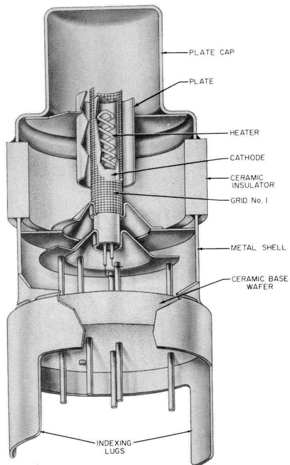
*Fig. 5 - Illustration of a double-ended nuvistor triode showing cylindrical electrodes and tripod-like supports.*
