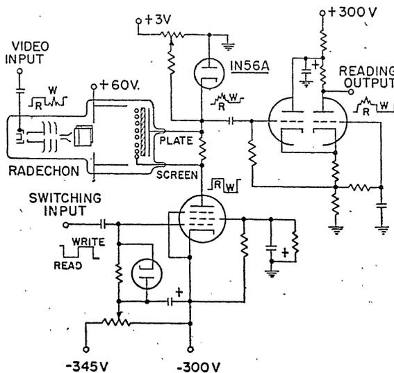
Fig. 5—Crystal output circuit.
