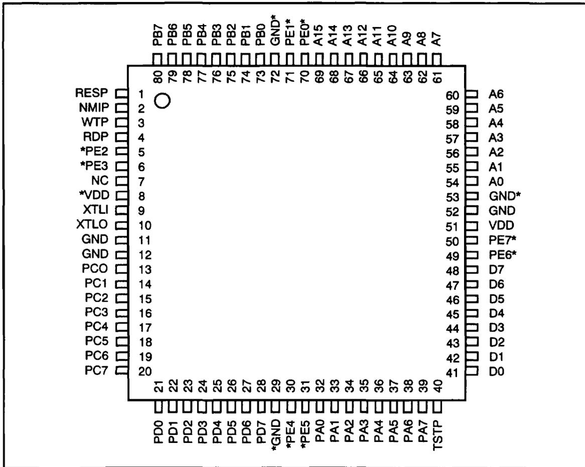
NOTE: \* Indicates pins not bonded in the 68 pin PLCC package.
