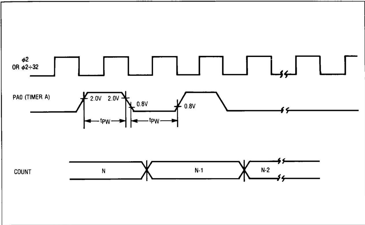
Figure 3-12. Event Counter (Mode 2) Waveforms
