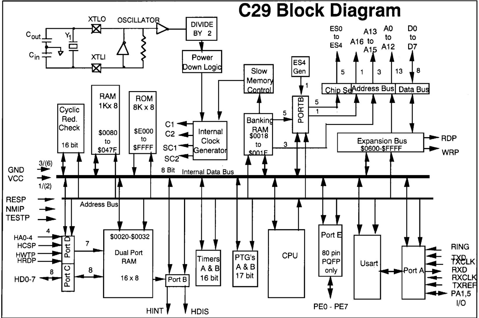
Figure 3-1a. C29 Block Diagram
