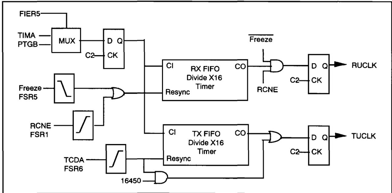
Figure 3-20. FIFO UART Timing Simulator
