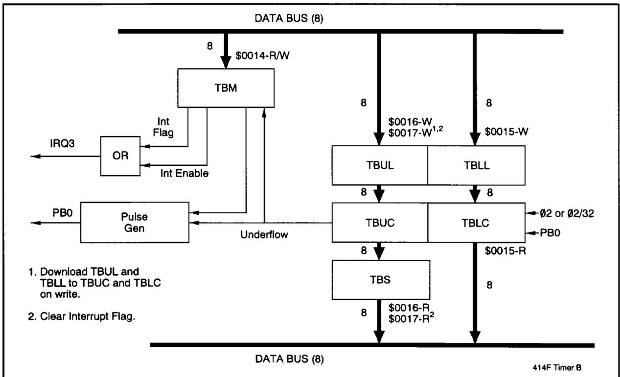
Figure 3-9 . Counter/Timer B Block Diagram
