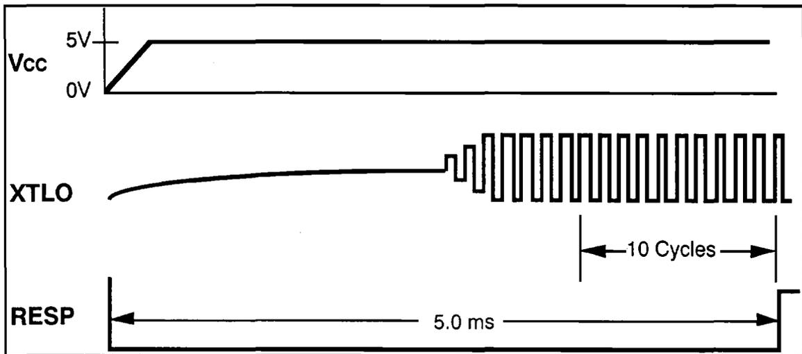
Figure 5-8. Power On RESP Timing
