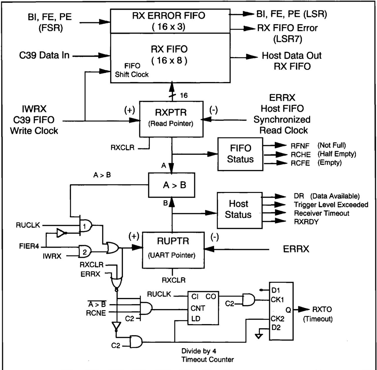
Figure 3-21. RX FIFO Block Diagram
