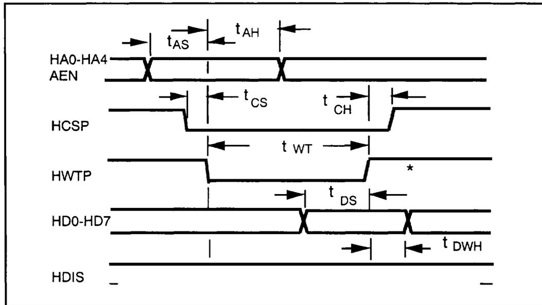
\* Following any Host write, a minimum delay of 2 times the internal MCU clock cycle time (200 ns at 10 MHz) is required from the rising edge of HWTP to the falling edge of the next selected Host HWTP or HRDP clock.
