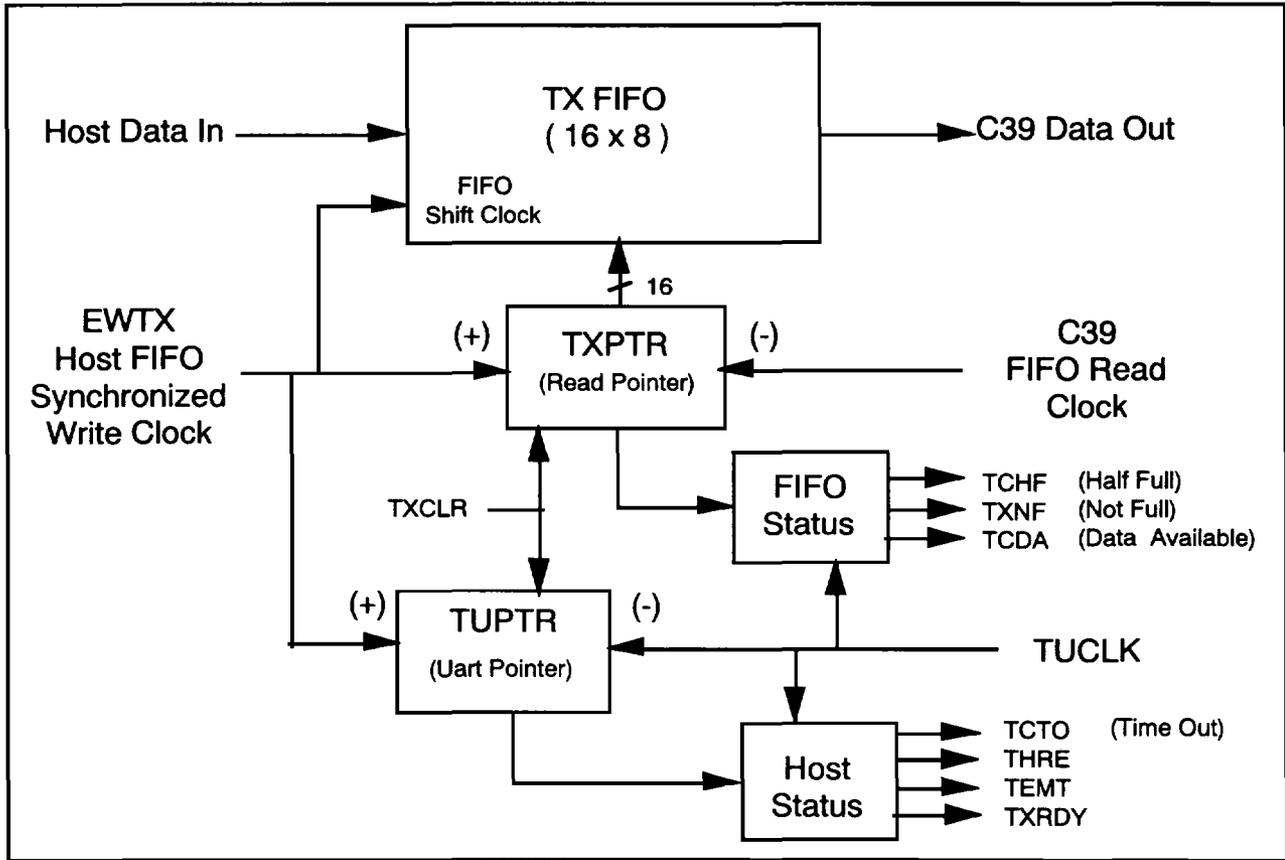
Figure 3-19. TX FIFO Block Diagram
