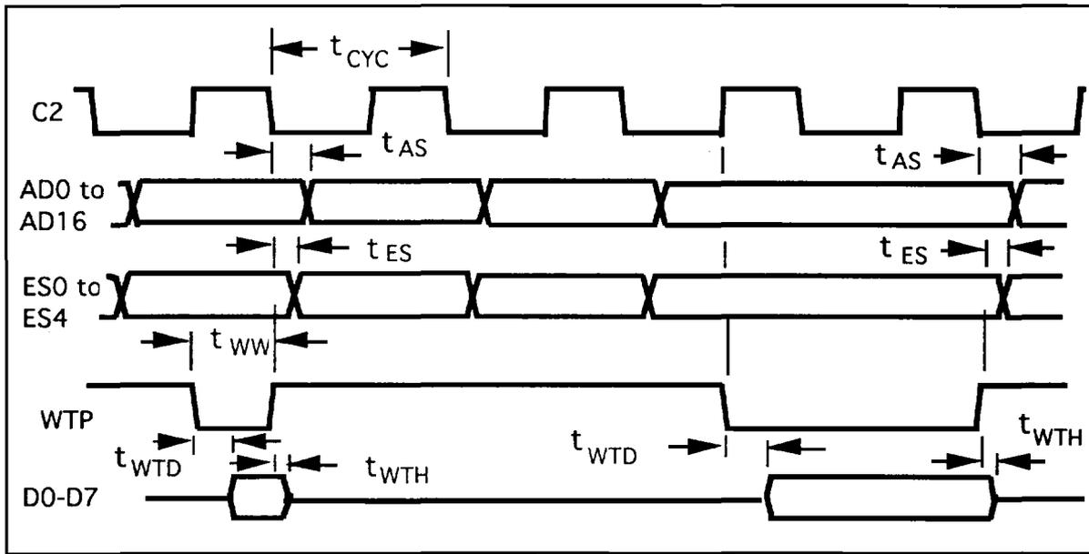
Figure 5-6. Expansion Bus Write Waveforms
