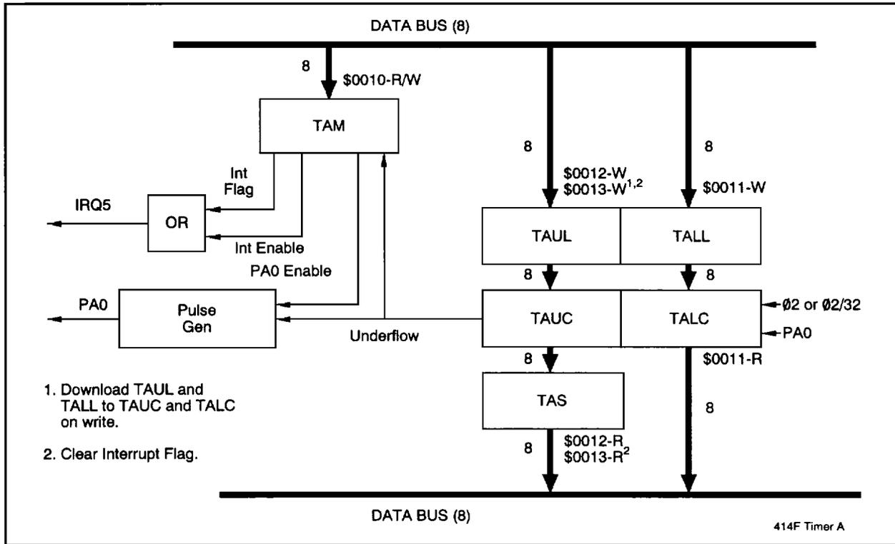
Figure 3-8. Counter/Timer A Block Diagram
