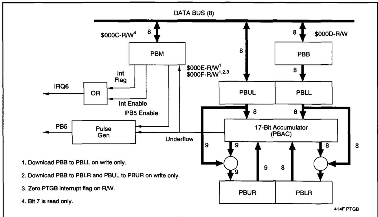
Figure 3-15. Precision Time Generator B Block Diagram
