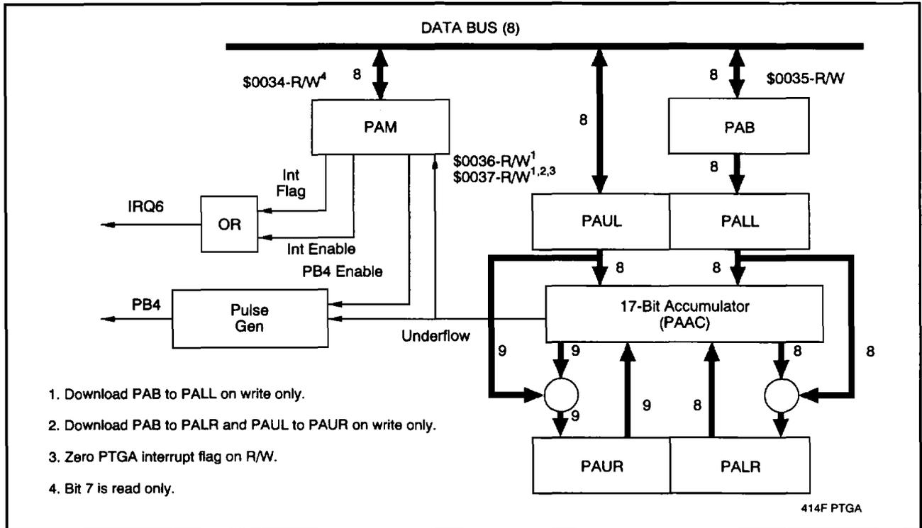
Figure 3-14. Precision Time Generator A Block Diagram
