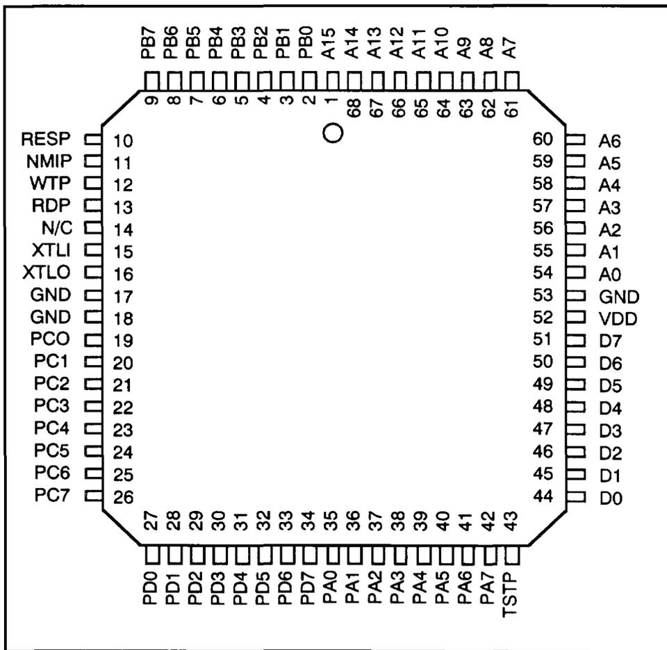
NOTE: Pin 14 is SYNC on C29; NC on C39.
