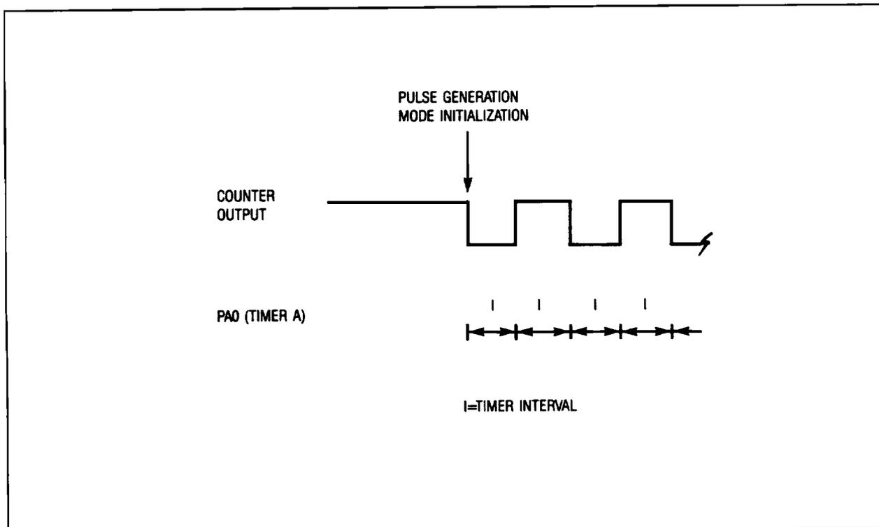
Figure 3-11. Pulse Generator (Mode 1) Waveforms
