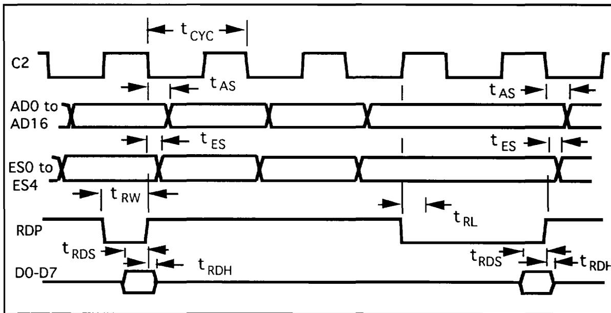
Figure 5-5. Expansion Bus Read Waveforms
