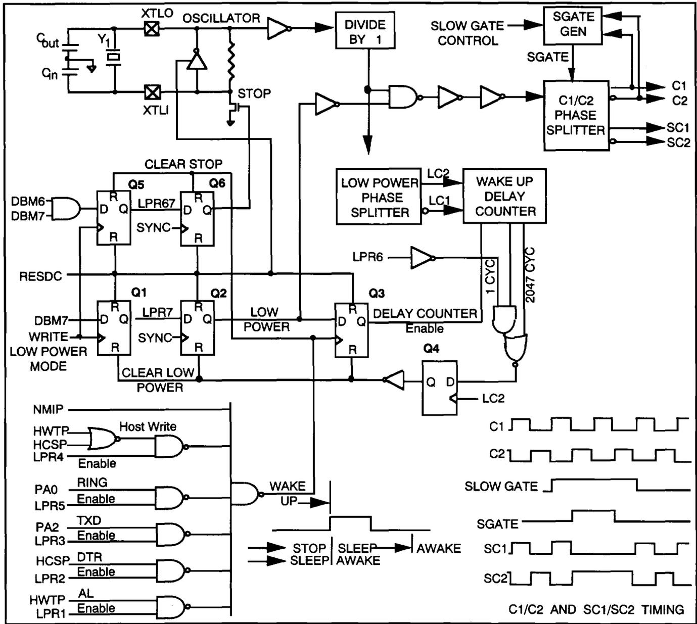
Figure 3-22. Low Power Mode Logic and Timing
