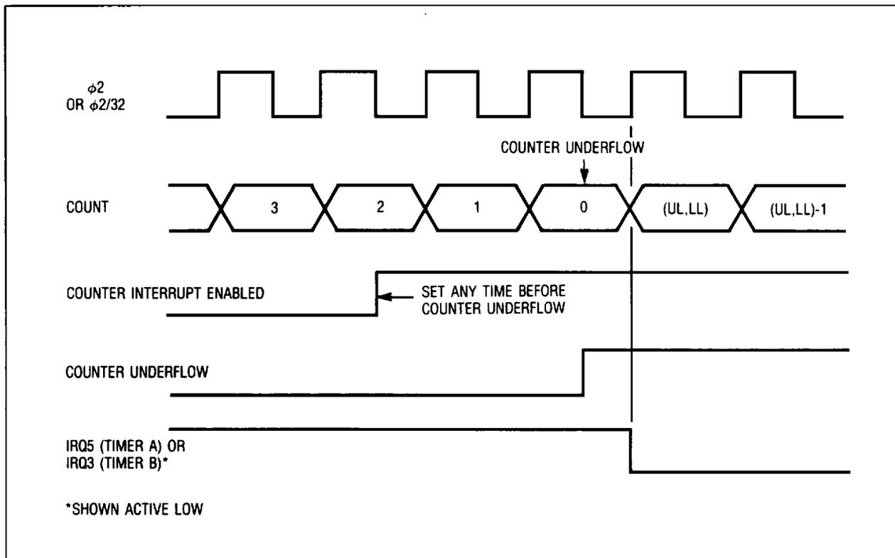
Figure 3-10. Interval Timer (Mode 0) Waveforms
