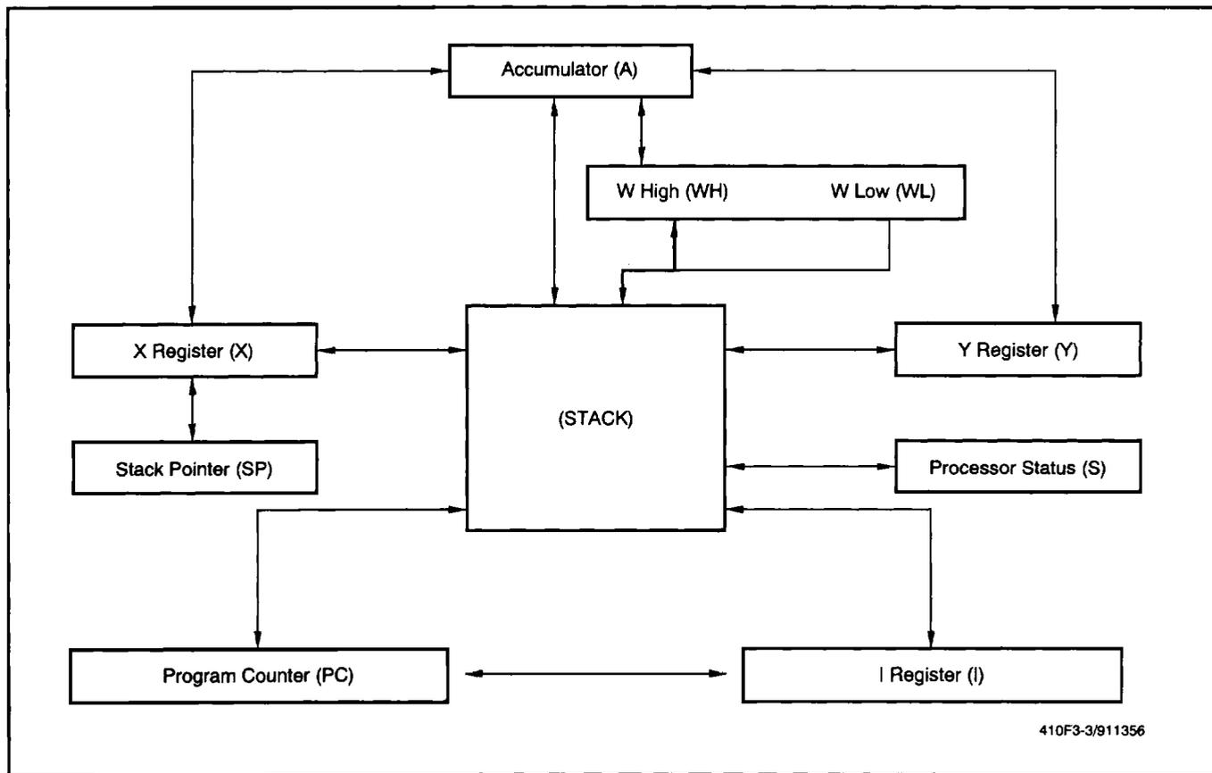
Figure 3-3. CPU Registers and Data Flow
