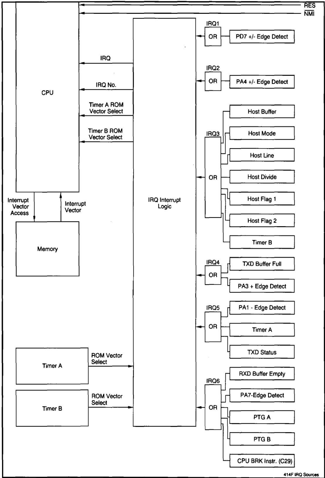
Figure 3-5. IRQ Interrupt Logic Interface
