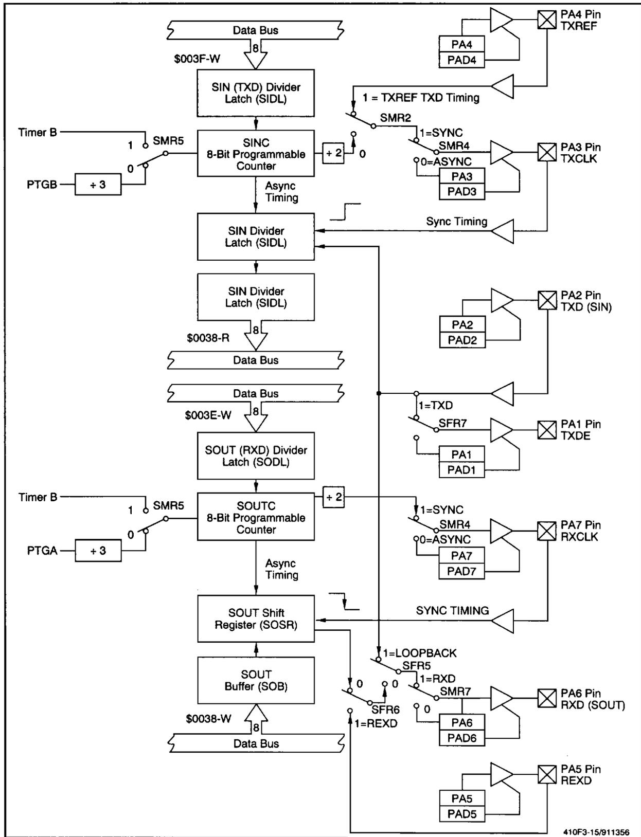
Figure 3-16. USART Block Diagram
