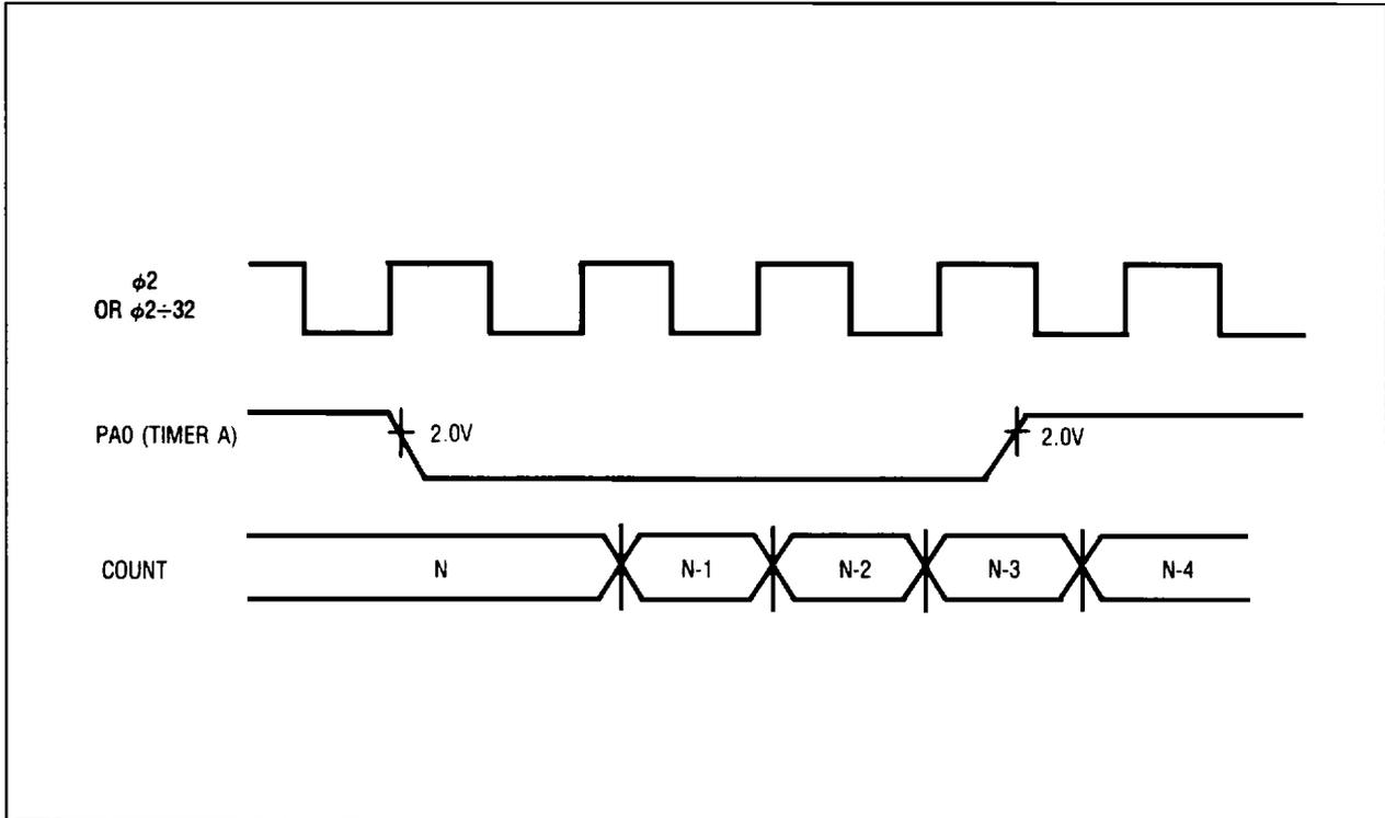
Figure 3-13. Pulse Width Measurement (Mode 3) Waveforms
