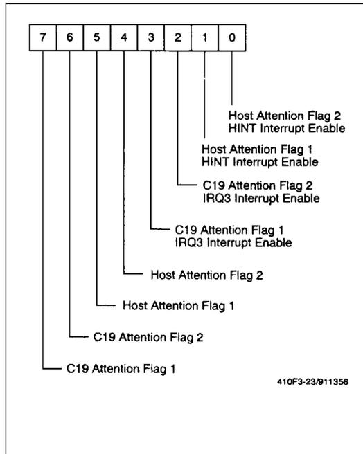
Figure 3-23. Host Handshake Register (HHR) - \$002F
