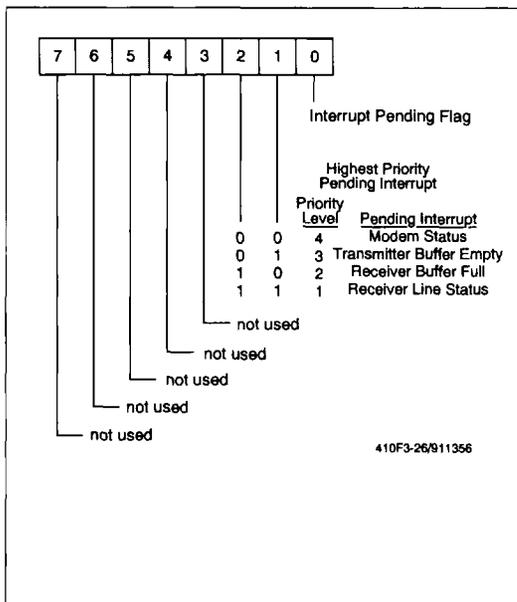
Figure 3-26. Interrupt Identifier Register (SLR)
