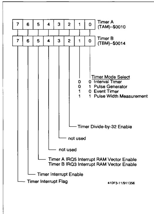
Figure 3-11. Timer A and Timer B Mode Registers
