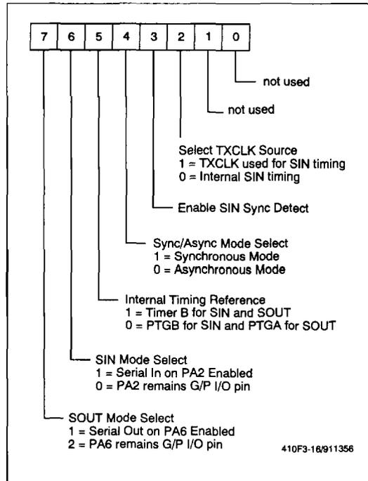
Figure 3-16. Serial Mode Register (SMR) - \$003A
