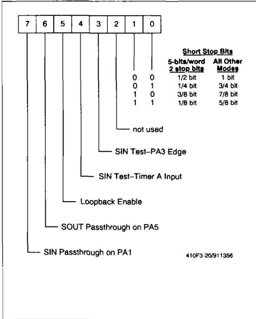
Figure 3-20. Serial Form Register (SFR) - \$003D
