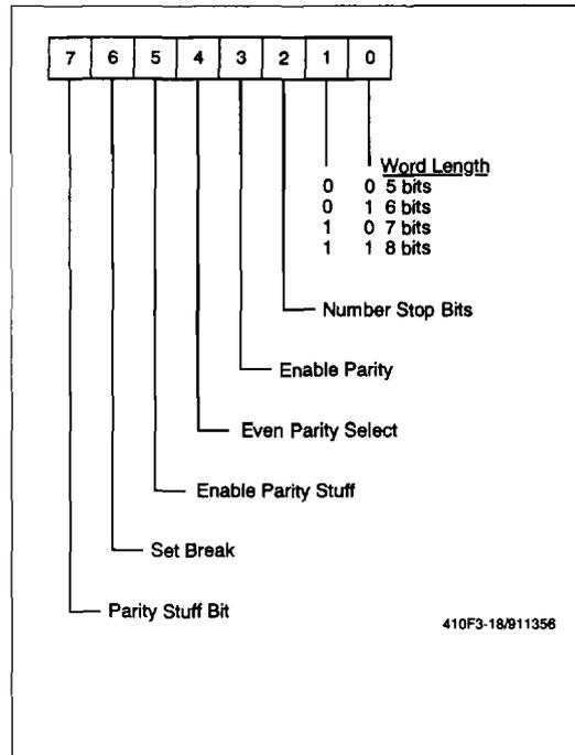
Figure 3-18. Serial Line Register (SLR) - \$003B
