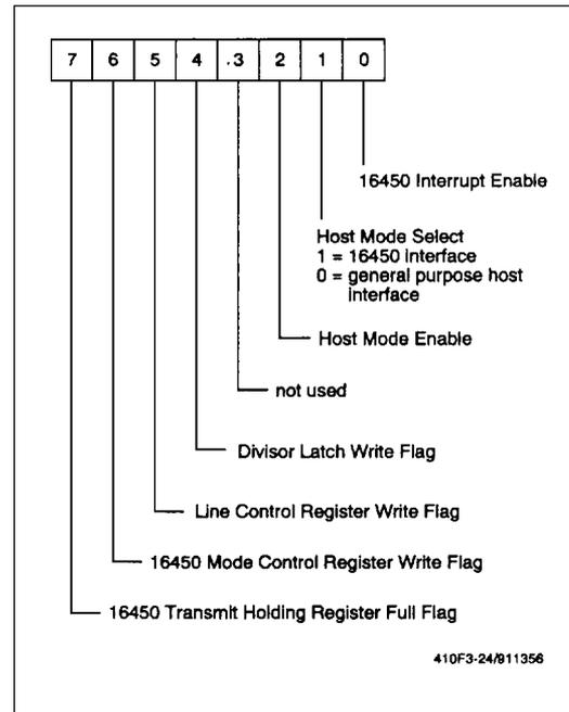
Figure 3-24. Host Control Register (HCR) - \$0032
