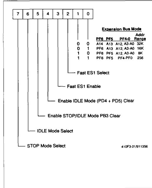
Figure 3-21. Bus Control Register (BCR) - \$0009
