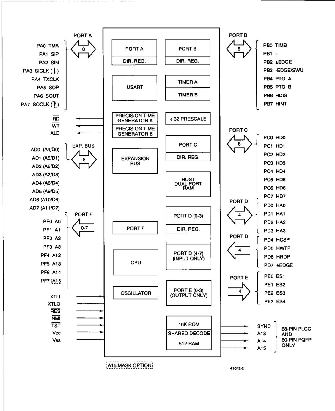
Figure 2-2. R65C19 Internal Functions and I/O Signals
