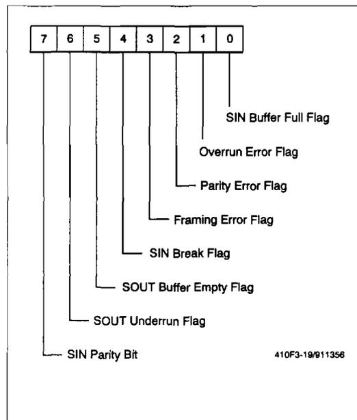
Figure 3-19. Serial Status Register (SSR) - \$003C
