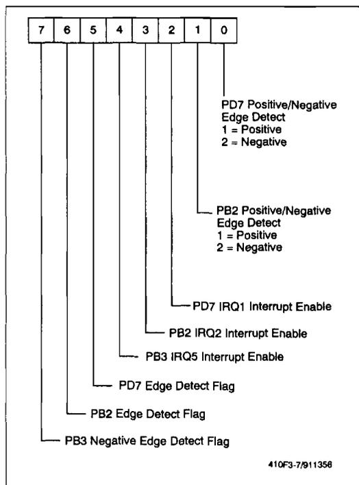
Figure 3-7. External Interrupt Register (EIR) - \$000A
