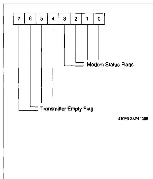
Figure 3-28. Modem Status Register (MSR) - \$0031
