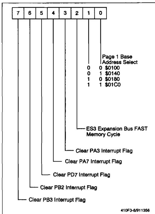
Figure 3-8. Clear Interrupt Register (CIR) - \$000B
