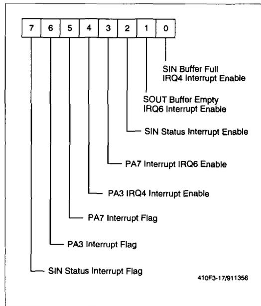
Figure 3-17. Serial Interrupt Register (SIR) - \$0039
