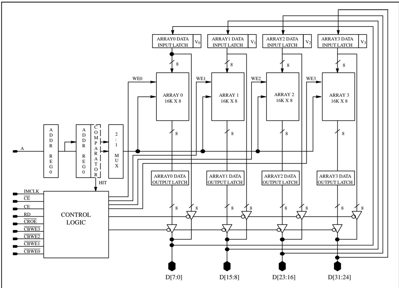
**Figure 4. RT627 Block Diagram**
