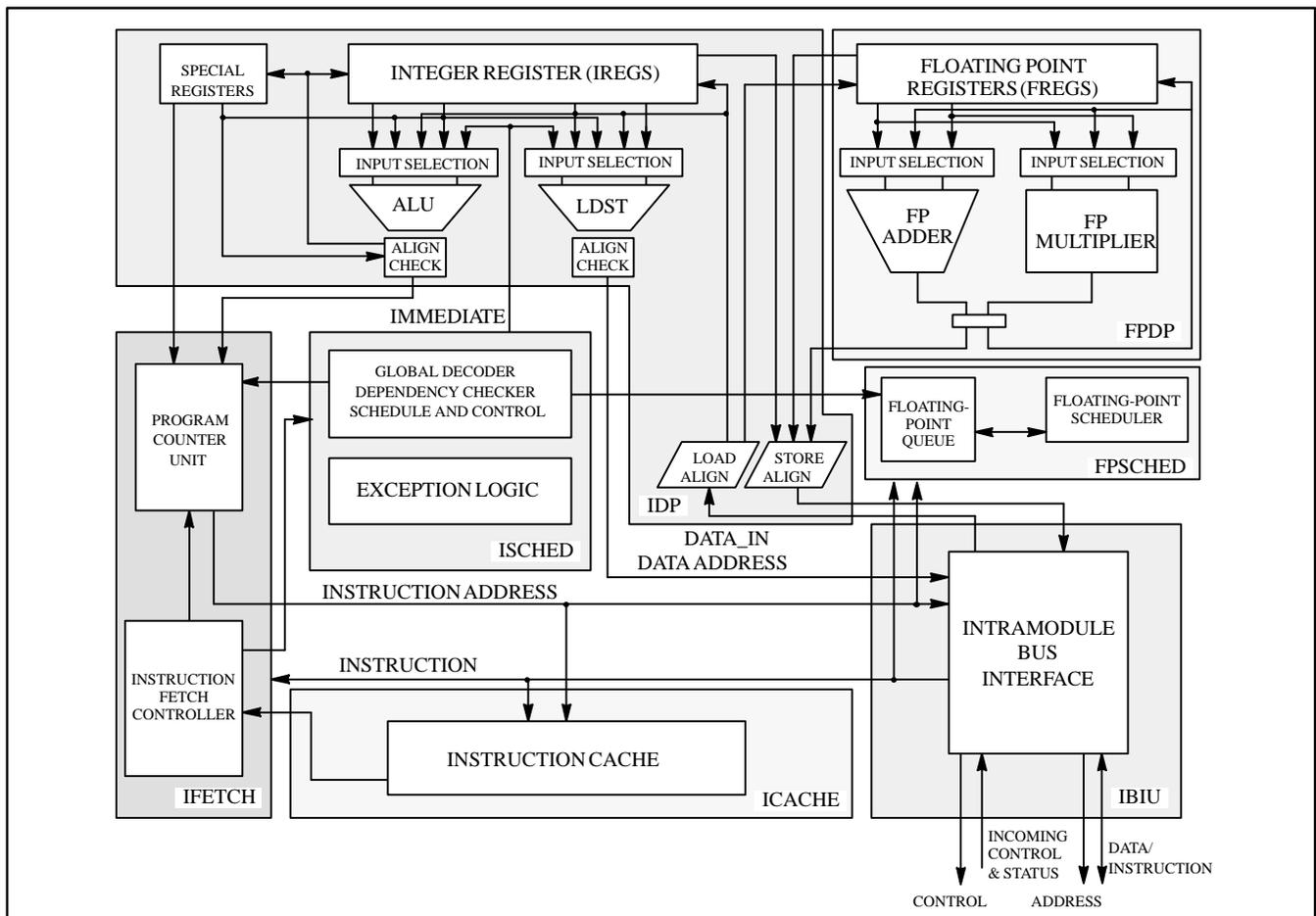
Figure 2. RT620 CPU Logic Block Diagram
