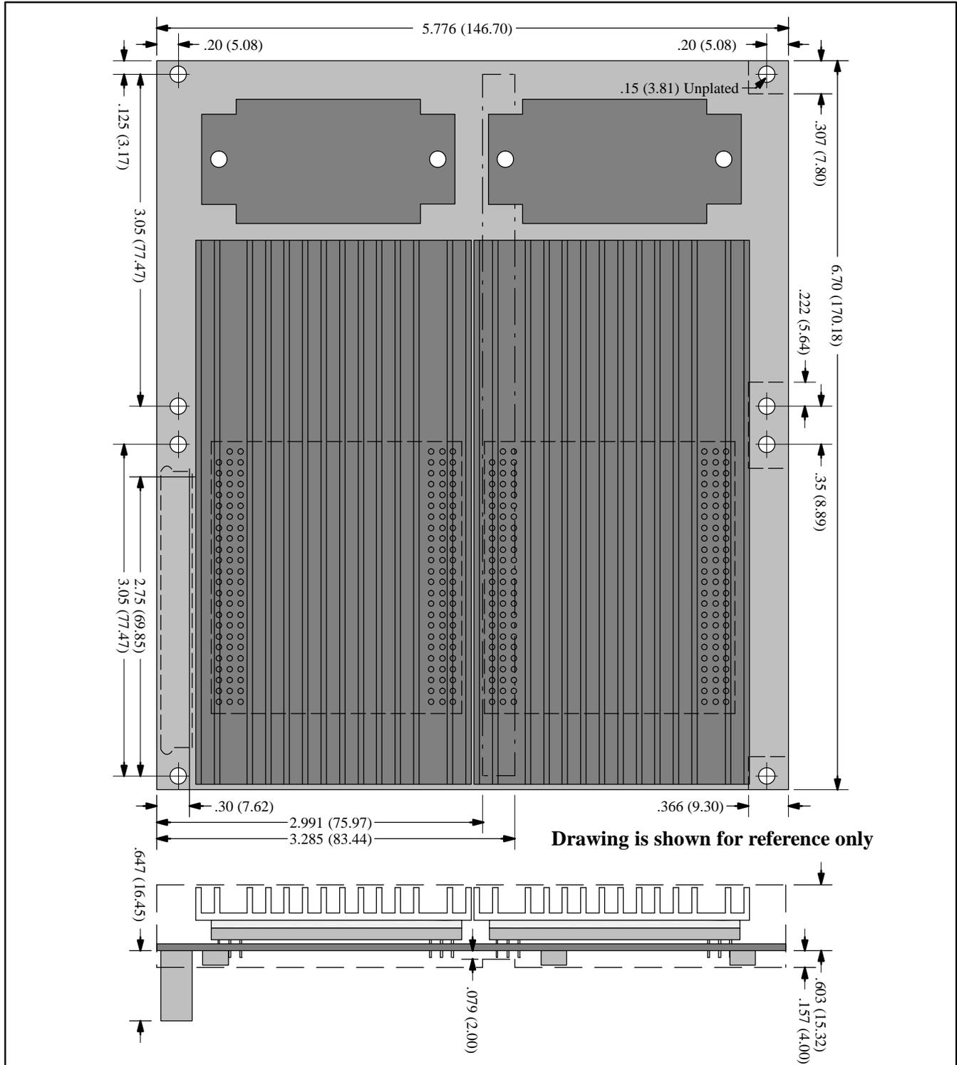
**Figure 6. RT6226M Mechanical Dimensions**
