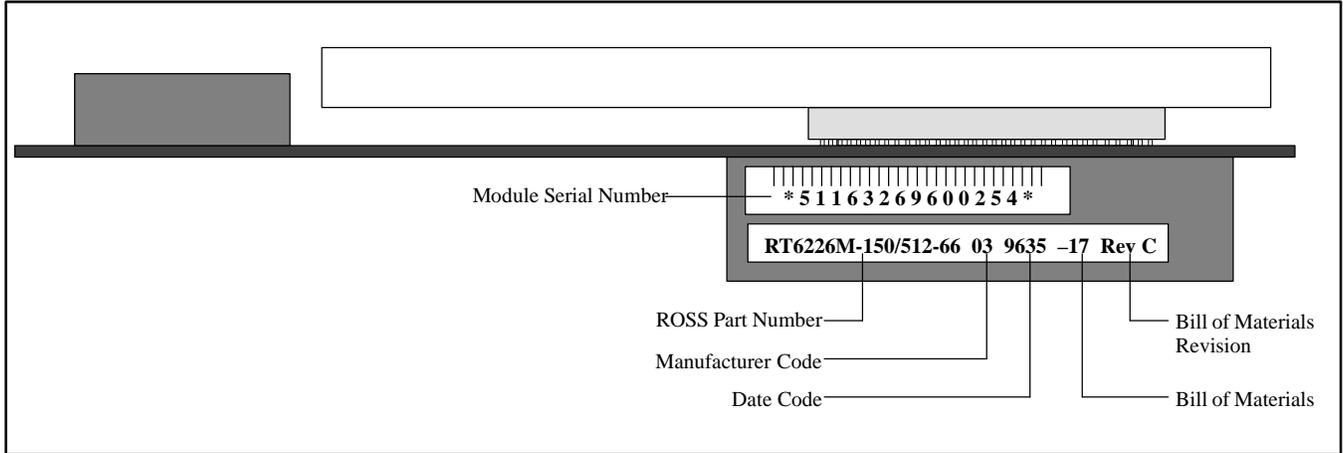
**Figure 7. RT6226M Module Labeling**
