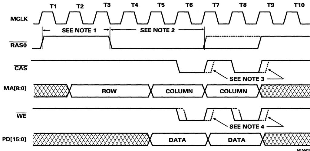
Figure 6-10. Fast Page Mode Write Cycle
