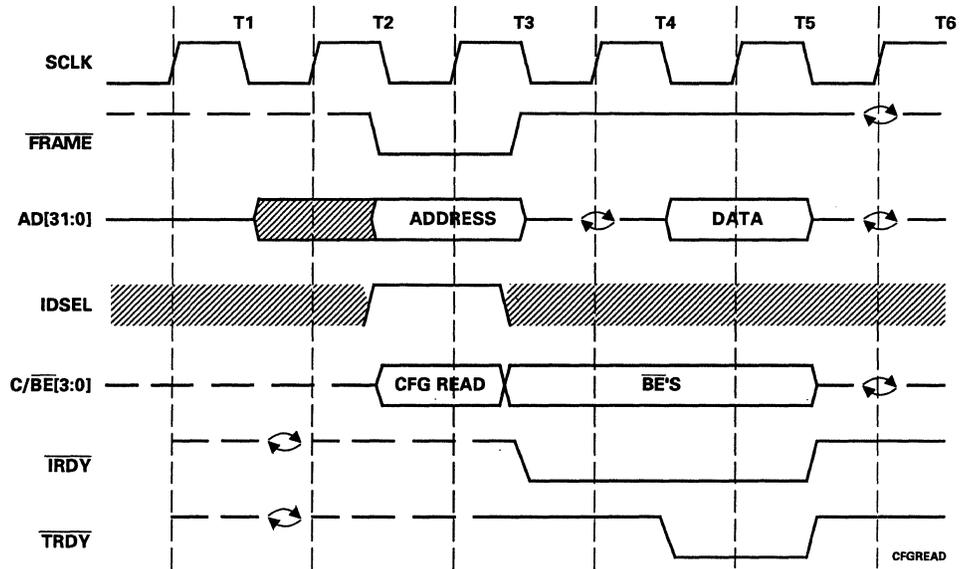
Figure 6-5. PCI Configuration Read Cycle
