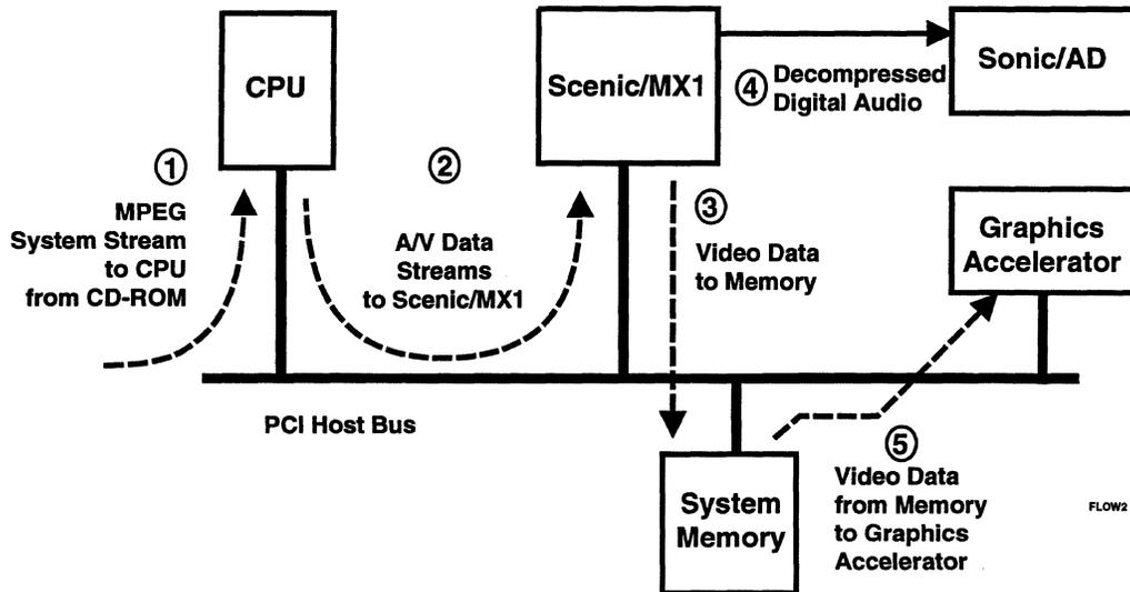
Figure 7-2. Data Flow with Graphics Accelerator
