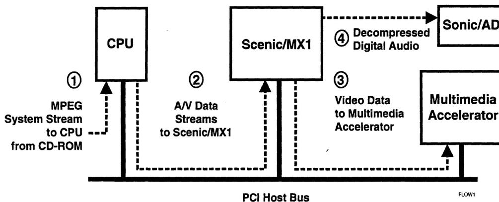
Figure 7-1. Data Flow with Multimedia Accelerator
