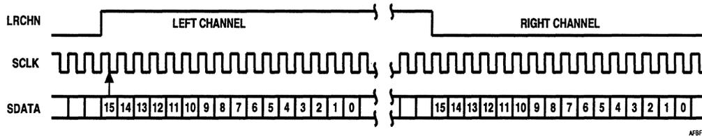
**Figure 6-13. First Audio Bits Latched on Rising Edge**
