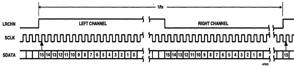
**Figure 6-12. First Audio Bits Latched on Rising Edge**
