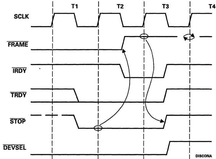
Figure 6-3. PCI Disconnect Example A
