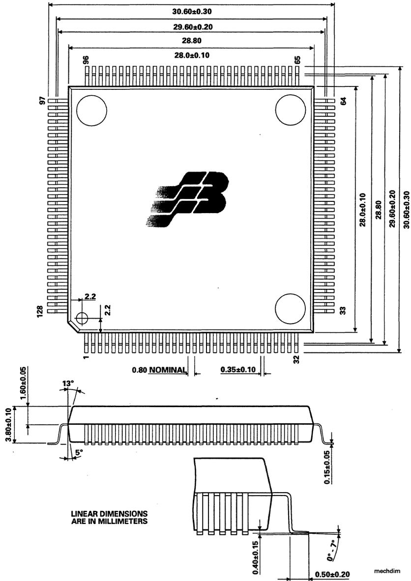
Figure 2-1. 128-pin PQFP Mechanical Dimensions
