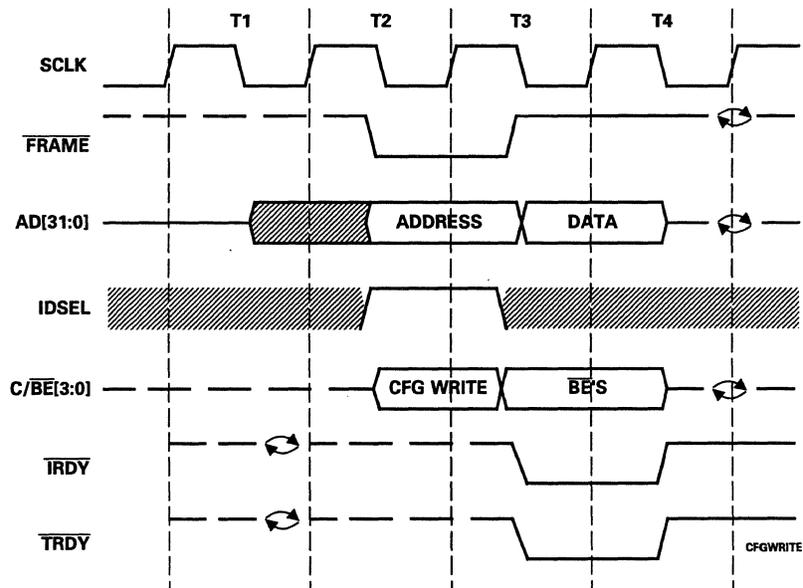
Figure 6-6. PCI Configuration Write Cycle
