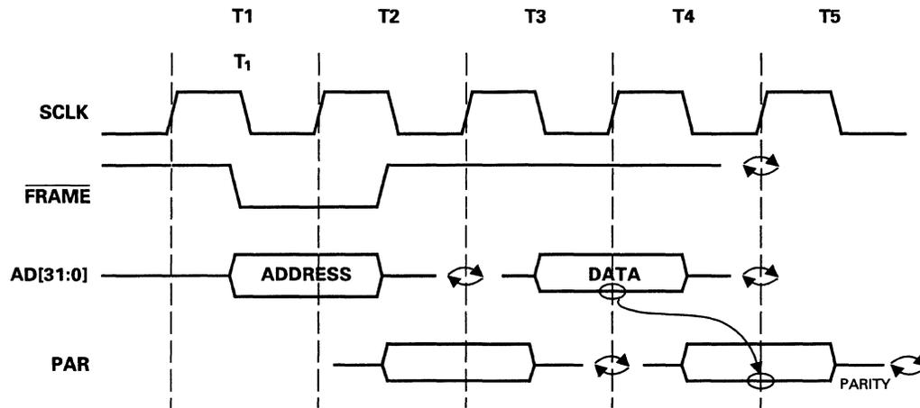
Figure 6-7. Read Parity Operation
