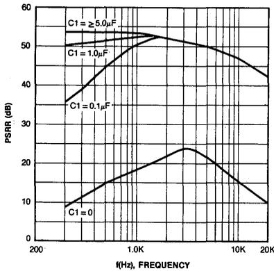
Fig. 14 PSRR vs FREQUENCY ( $C_2 = 0$ )
