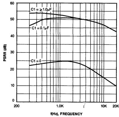
Fig. 13 PSRR vs FREQUENCY ( $C_2 = 1.0\mu\text{F}$ )
