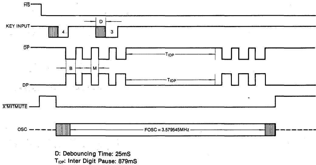
**TIMING DIAGRAM** (for Switching Mode Operation by MODE SELECT Input)
