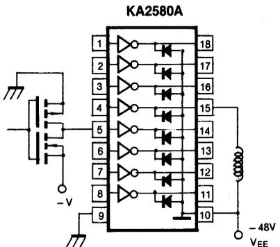
TELECOMMUNICATION RELAY DRIVER (NEGATIVE LOGIC)
