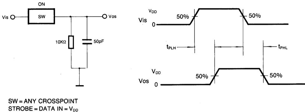
FIG. 3 OFF ISOLATION MEASUREMENT (FEEDTHROUGH)
