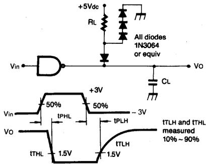
$C_L = 15pF$  = total parasitic capacitance, which includes probe and wiring capacitances
