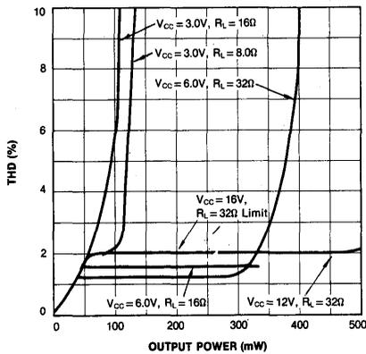
Fig. 22 DISTORTION vs POWER (f = 1,3KHz, AvD = 12dB)
