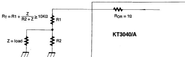
Receive Filter Output Gain Adjustment
