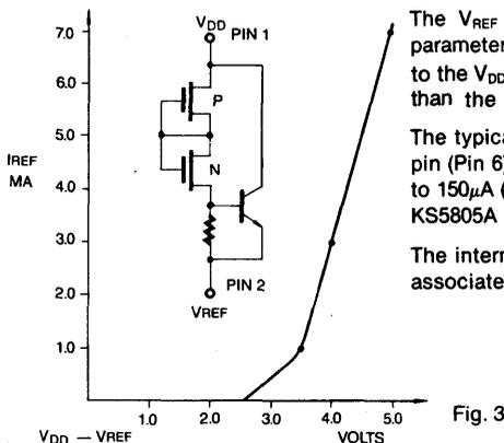
The V<sub>REF</sub> output provides a reference voltage that tracks internal parameters of the KS5805A. V<sub>REF</sub> provides a negative voltage reference to the V<sub>DD</sub> supply. Its magnitude will be approximately 0.6 volts higher than the minimum operating voltage of a particular KS5805A.
