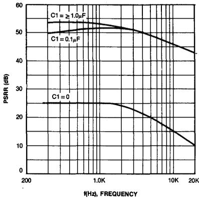
Fig. 12 PSRR vs FREQUENCY ( $C_2 = 5.0\mu\text{F}$ )
