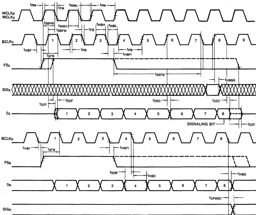
Fig. 3 Long Frame Sync Timing
