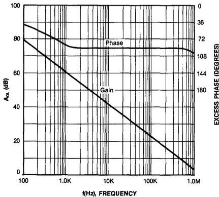
Fig. 8 DIFFERENTIAL GAIN vs FREQUENCY
