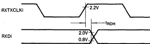
Fig. 5 Receive Data Hold Time (+1 Mode)
