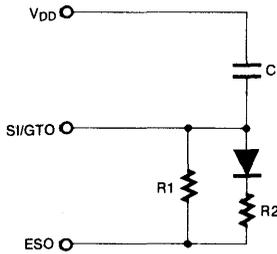
$$t_{GTP} = (R1C) \ln(V_{DD}/V_{DD} - V_{TST})$$
