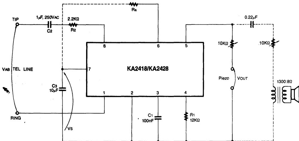
$$f_1 = \frac{3.22 \cdot 10^4}{R_1 \text{ (K}\Omega\text{)}} \text{ (KA2418)}, f_1 = \frac{2.66 \cdot 10^4}{R_1 \text{ (K}\Omega\text{)}} \text{ (KA2428)}, f_2 = \frac{5}{7} f_1, f_{\text{sweep}} = \frac{1000}{C_1 \text{ (nF)}}$$
