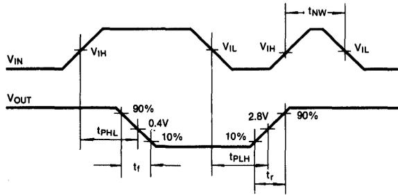
Fig. 2 Switching Waveforms
