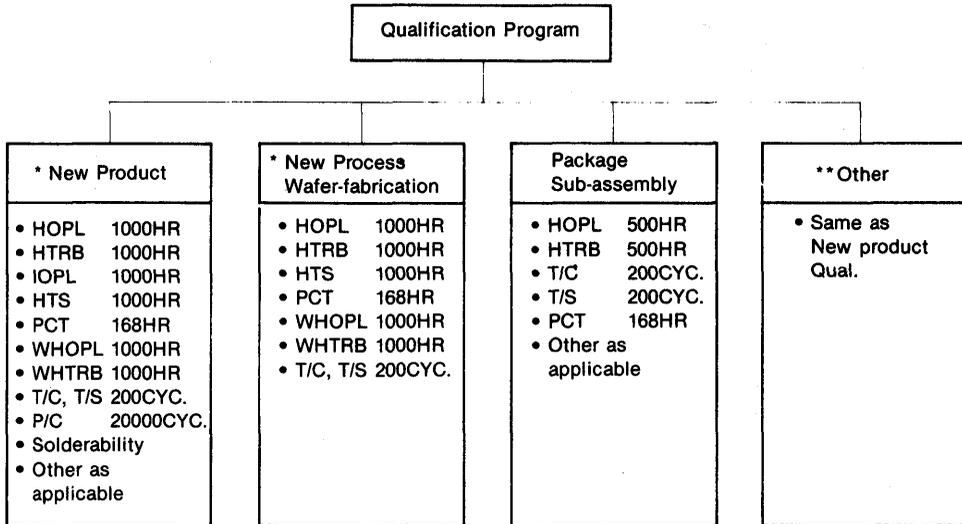
\*Testing time for each test items depends on the grade (group) of devices. (see the device group list 2.1 2))
