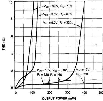
Fig. 21 DISTORTION vs POWER (f = 3KHz, AvD = 34dB)
