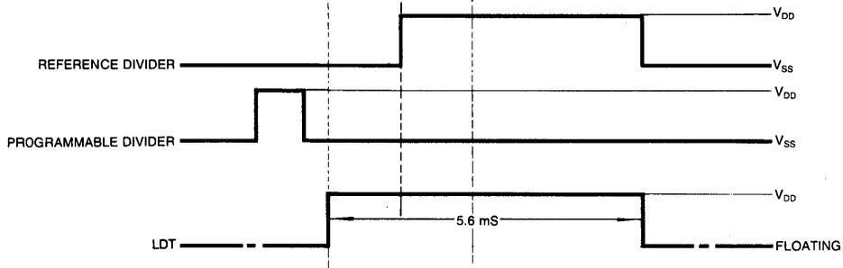
Note) When the phase difference of programmable divider & reference divider exceeds  $T_D$  than LDT output is high.
