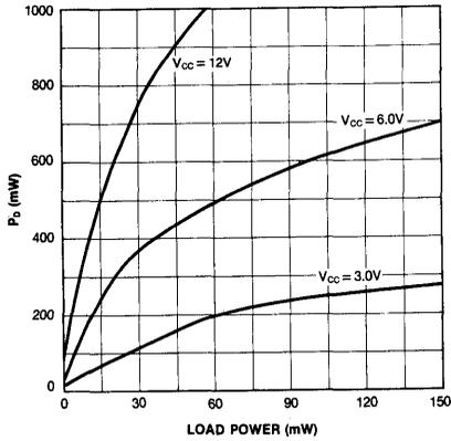
Fig. 18 POWER DISSIPATION (16Ω LOAD)
