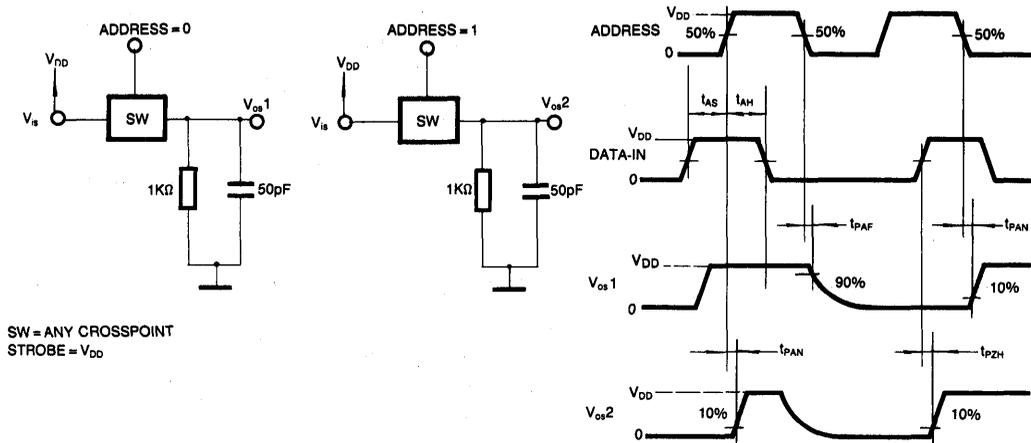
**FIG. 8. WAVE FORMS FOR CROSSTALK (CONTROL INPUT TO SIGNAL OUTPUT)**
