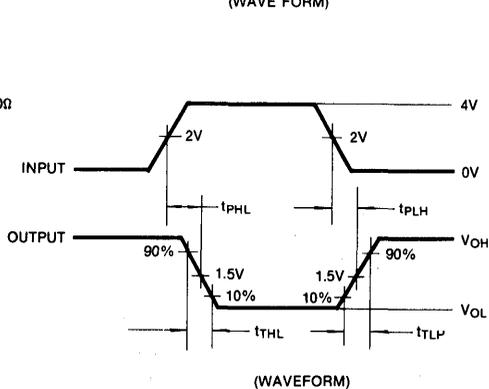
Note) 3. The pulse generator has the following characteristics:  $Z_{OUT} = 50\Omega$ ,  $t_w = 500ns$ ,  $t_r = t_f \geq 5ns$
