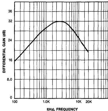
Fig. 7 OPEN LOOP GAIN & PHASE (AMP 1)
