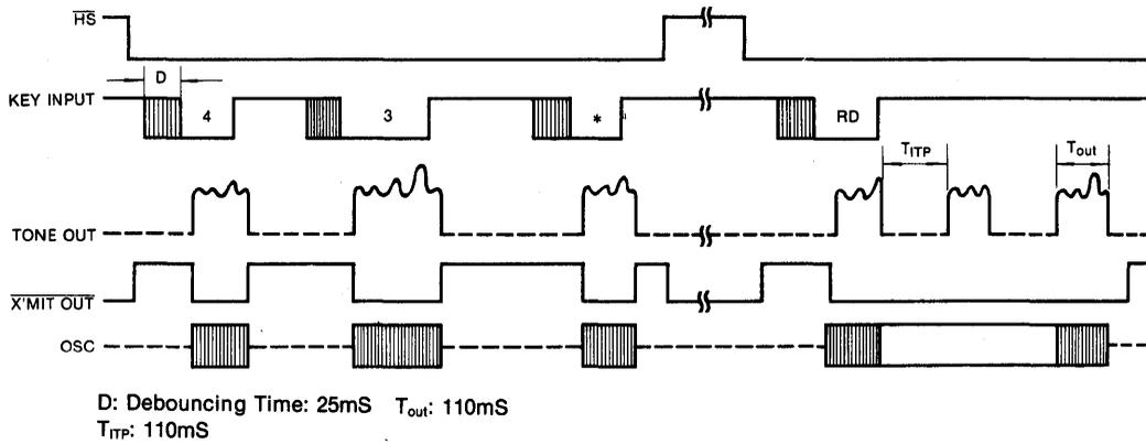
**PULSE MODE TIMING** (MODE SELECT =  $V_{DD}$ )
