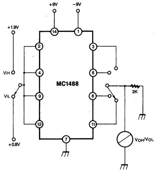
FIGURE 3 OUTPUT SHORT CIRCUIT CURRENT
