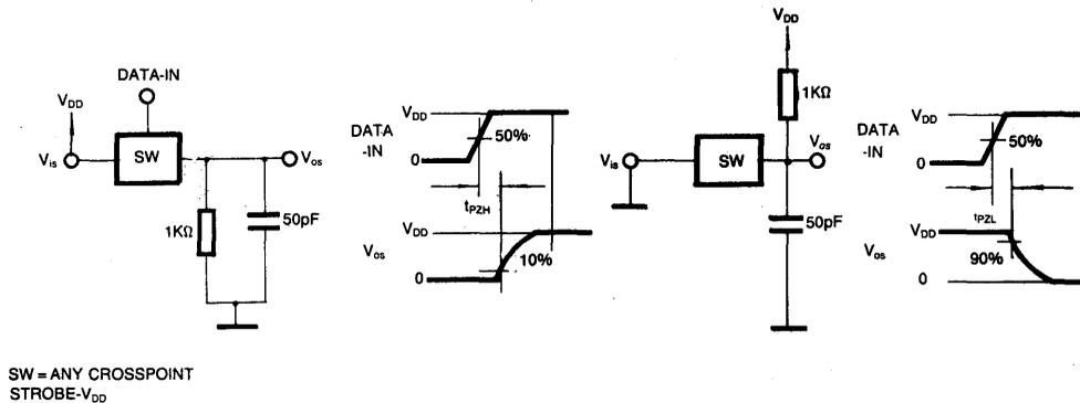
**FIG. 7. PROPAGATION DELAY TIME & WAVE FORMS (ADDRESS TO SIGNAL OUTPUT, SWITCH TURN-ON OR TURN-OFF)**
