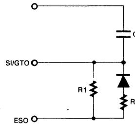
$$t_{GTP} = (RpC) \ln(V_{DD}/V_{DD} - V_{TST})$$
