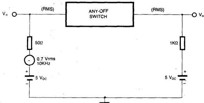
$$I_o = 20 \text{ Log}(V_{os}/V_{is}) \text{ dB}$$
