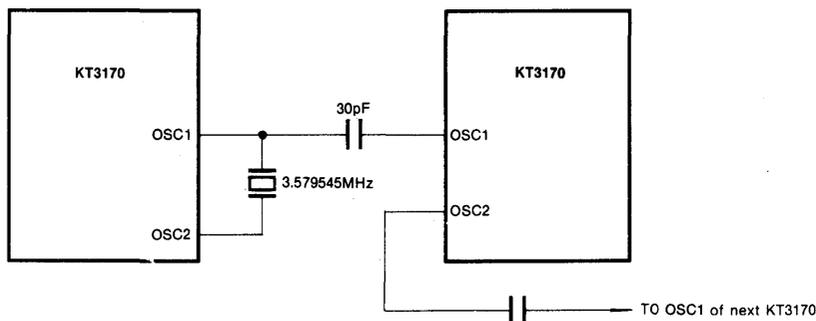
Fig. 4 Oscillator Connection
