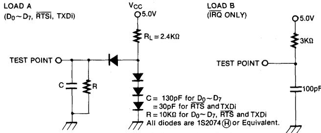
Fig. 9 Bus Timing Test Loads
