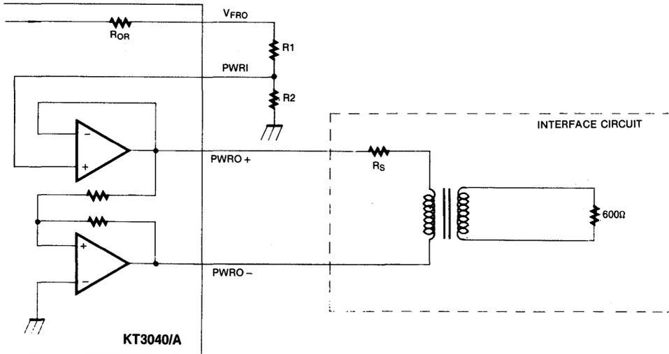
Typical Connection of Output Driver Amp
