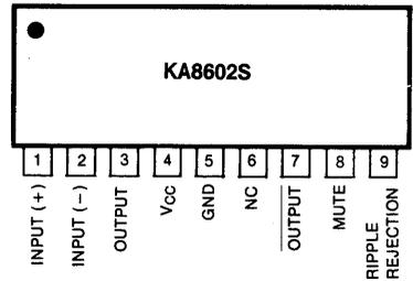
Fig. 1 AUDIO AMPLIFIER (HIGH INPUT IMPEDANCE)
