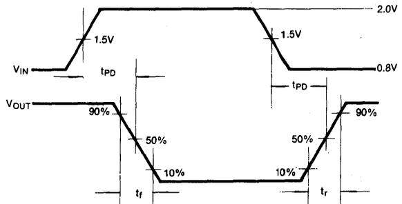
Fig. 2 Switching Waveforms
