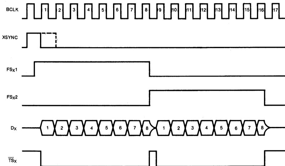
**Fig. 1 Transmit Data Timing**
