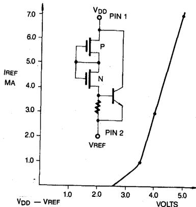
The  $V_{REF}$  output provides a reference voltage that tracks internal parameters of the KS58C05. The  $V_{REF}$  provides a negative voltage reference to the  $V_{DD}$  supply. Its magnitude will be approximately 0.6 volts higher than the minimum operating voltage of a particular KS58C05.
