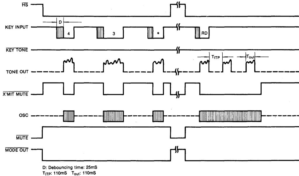
**PULSE MODE TIMING** (MODE SELECT =  $V_{DD}$ )
