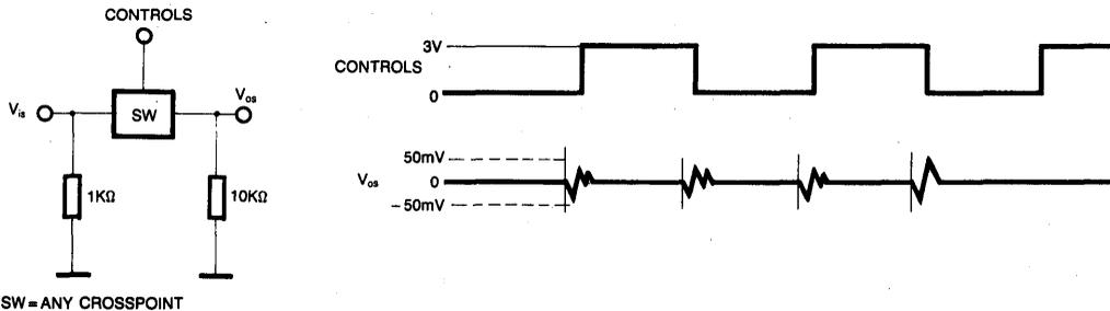
**FIG. 9. PROPAGATION DELAY TIME & WAVE FORM (RESET TO OUTPUT SIGNAL)**
