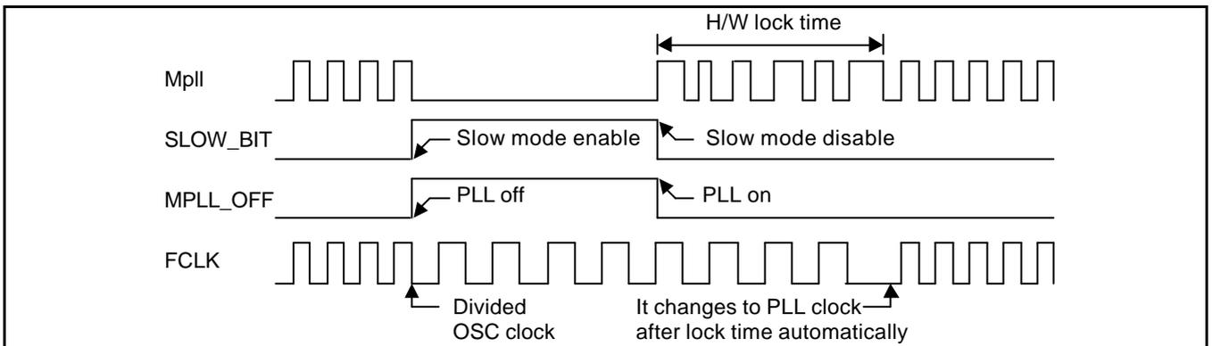
Figure 6-13. The case that the Exit\_from\_Slow\_mode command and the instant PLL\_on command is issued simultaneously.
