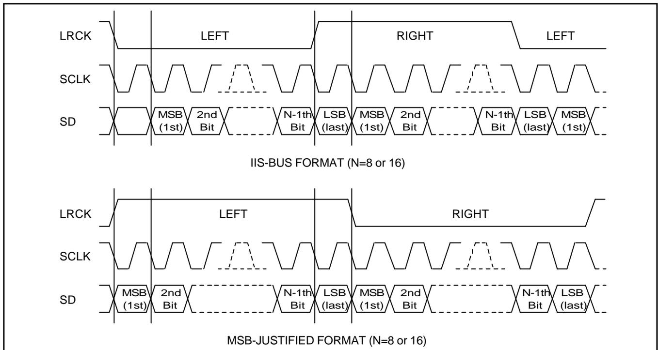
Figure 21-2. IIS-Bus and MSB(Left)-justified Data Interface Formats
