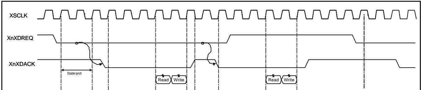
Figure 8-4. Single service, Demand Mode, Single Transfer Size
