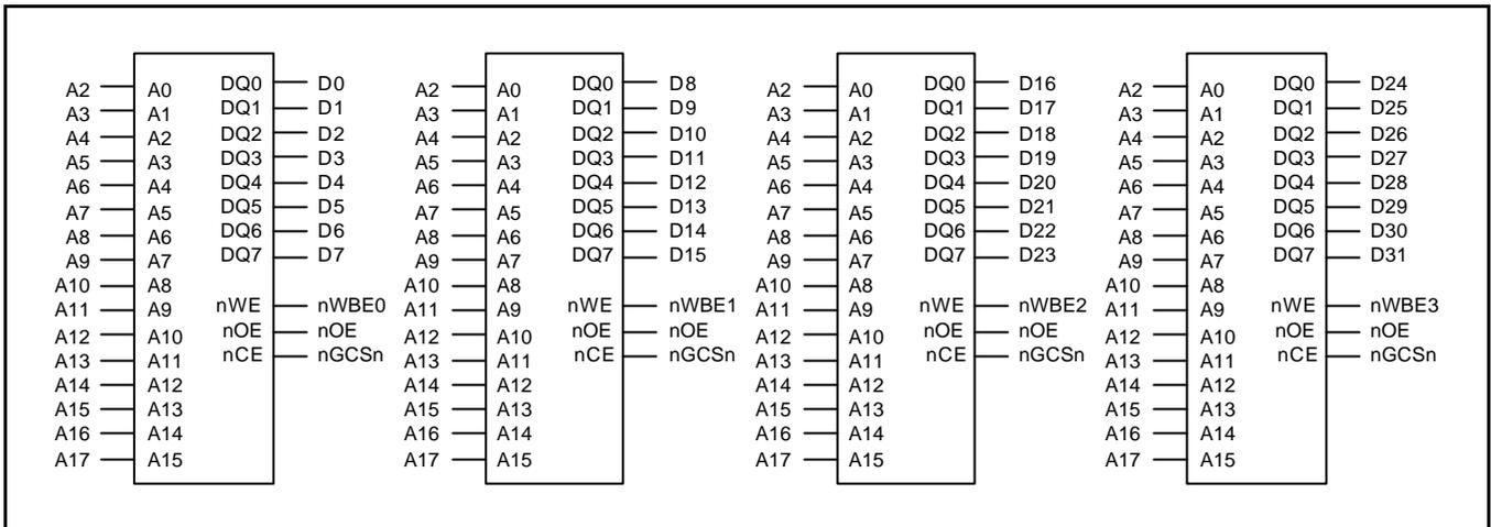
Figure 5-6. Memory Interface with 8bit ROM x 4
