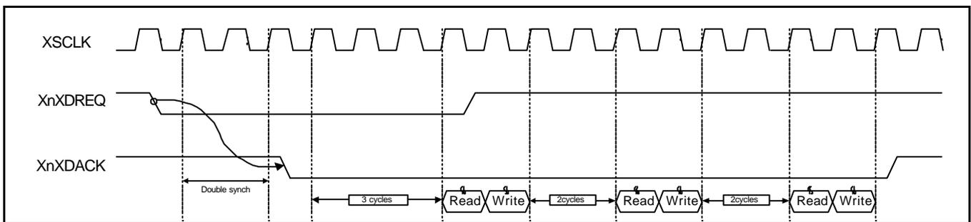
Figure 8-6. Whole service, Handshake Mode, Single Transfer Size
