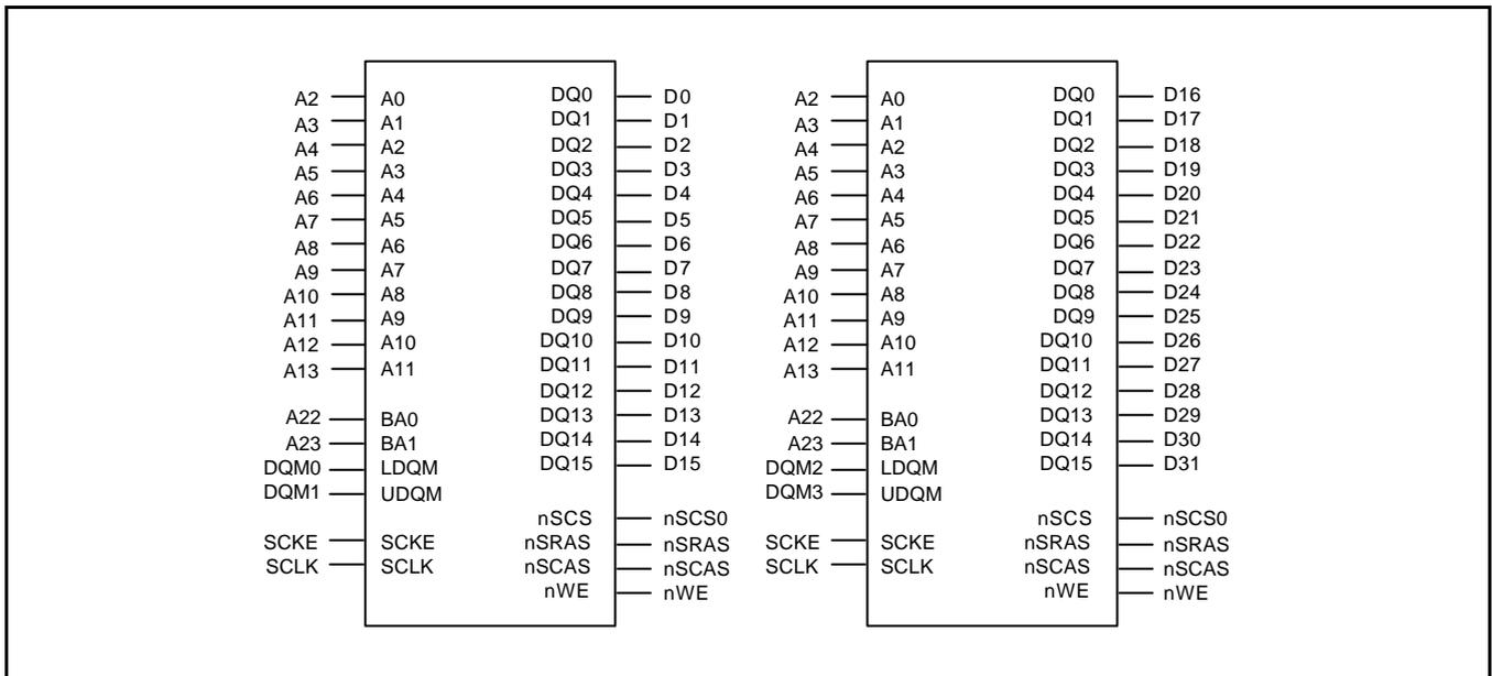
Figure 5-11. Memory Interface with 16bit SDRAM(4Mx16 \* 2ea, 4bank)
