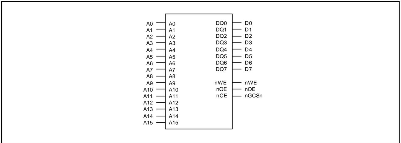
Figure 5-4. Memory Interface with 8bit ROM
