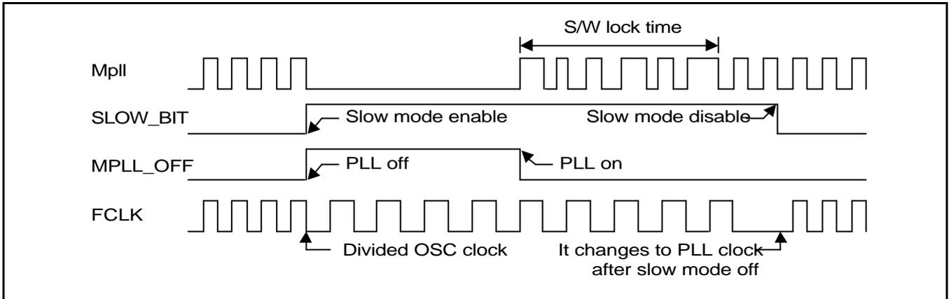
Figure 6-12. The case that Exit\_from\_Slow\_mode command is issued after lock time is end
