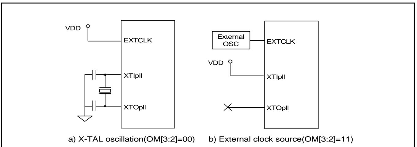
Figure 6-3. Main Oscillator Circuit Examples
