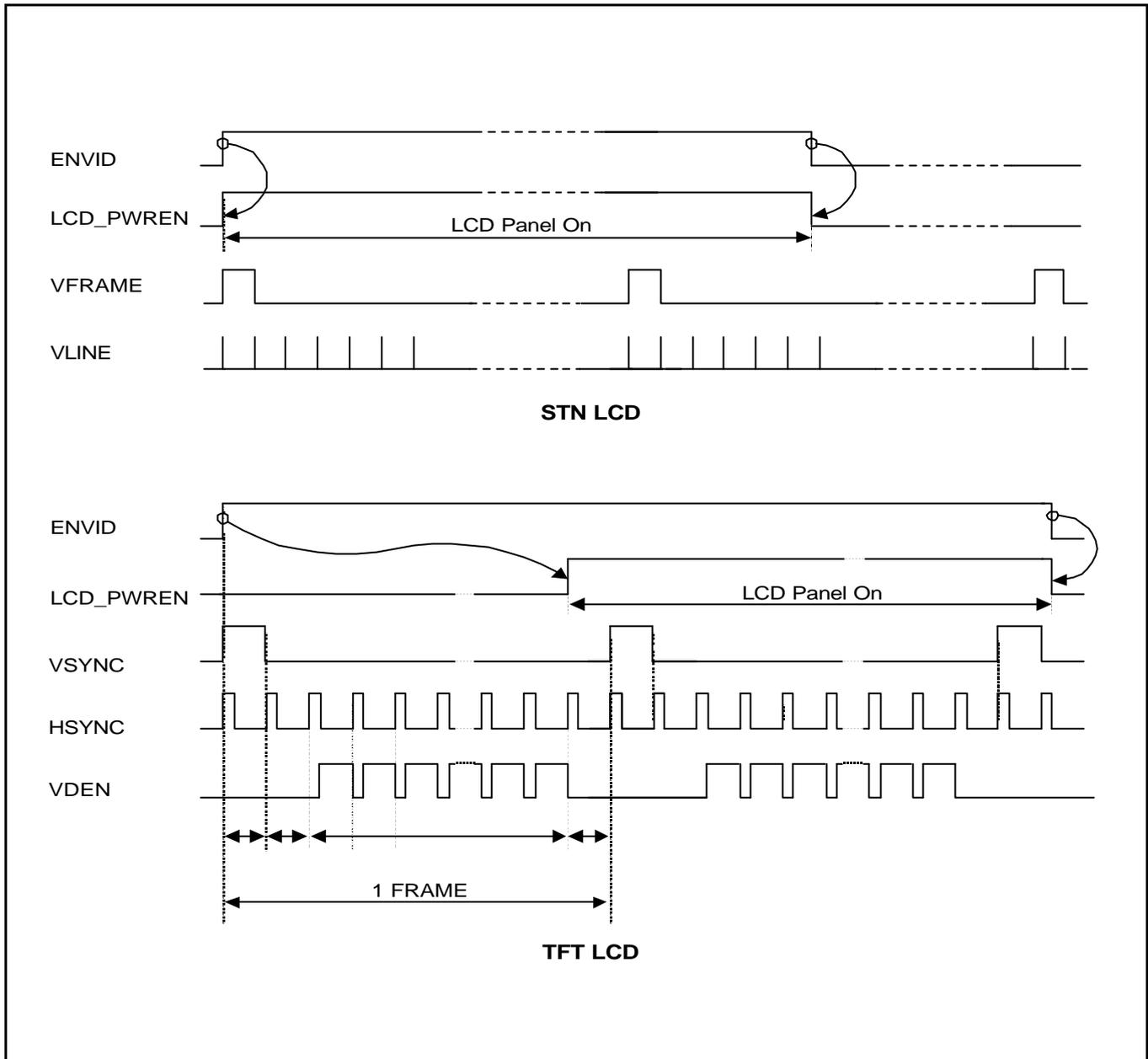
Figure 15-8. Example of PWREN function (PWREN=1, INVPWREN=0)
