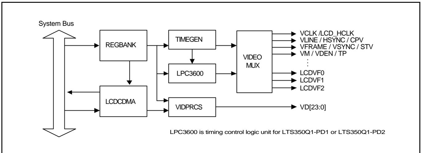
Figure 15-1. LCD Controller Block Diagram
