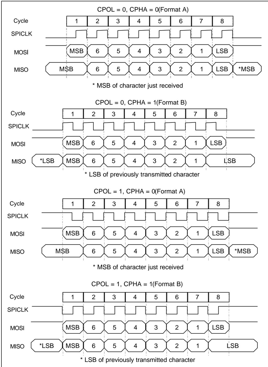
Figure 22-2. SPI Transfer Format
