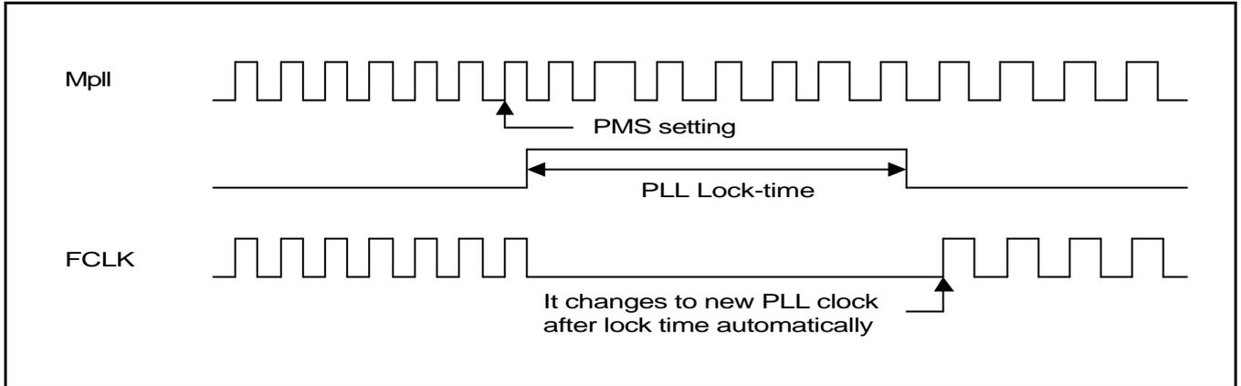
**Figure 6-5. The case that changes Slow clock by setting PMS value**
