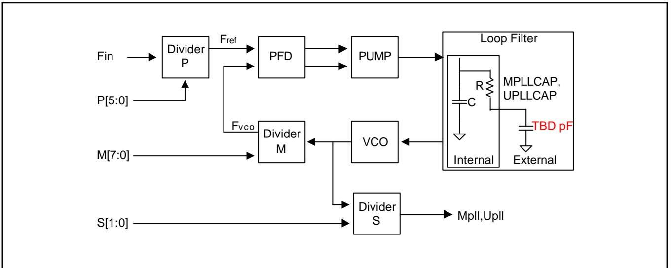
Figure 6-2. PLL (Phase-Locked Loop) Block Diagram
