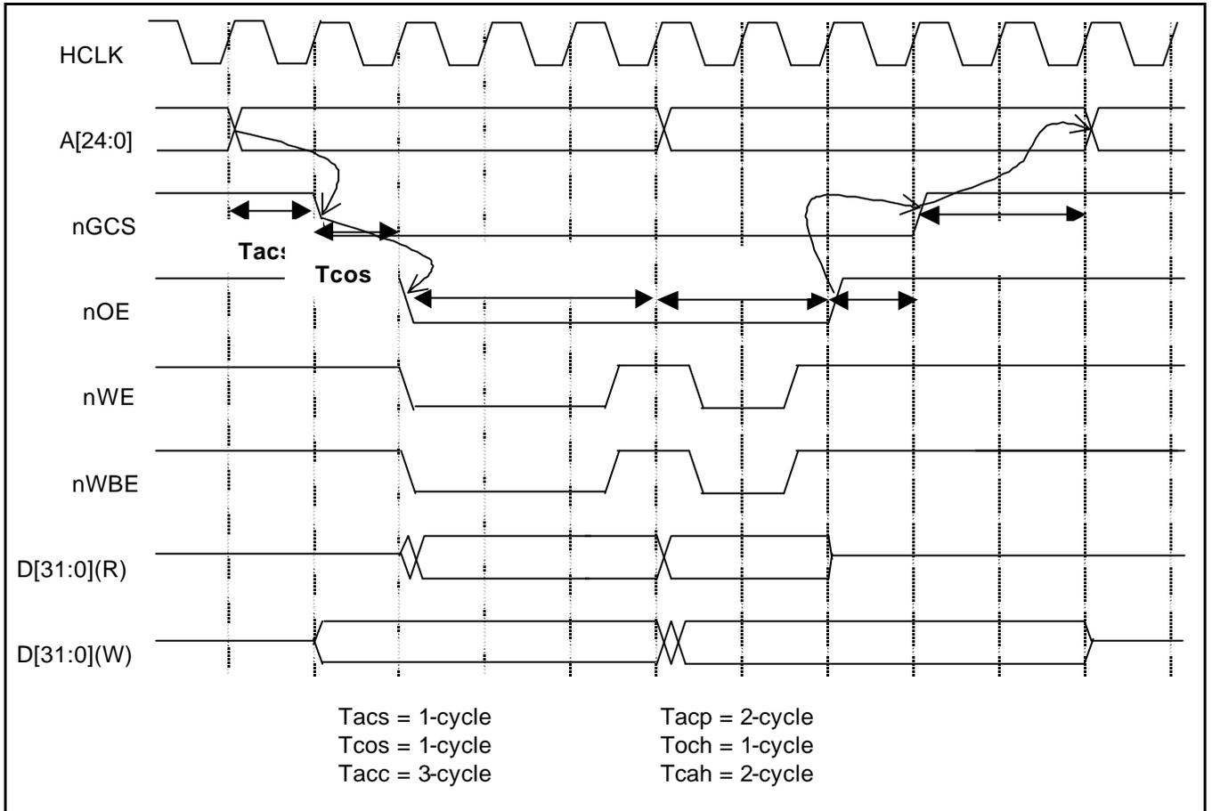
Figure 5-12. S3C2410X01 nGCS Timing Diagram.
