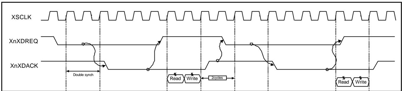
Figure 8-5. Single service, Handshake Mode, Single Transfer Size
