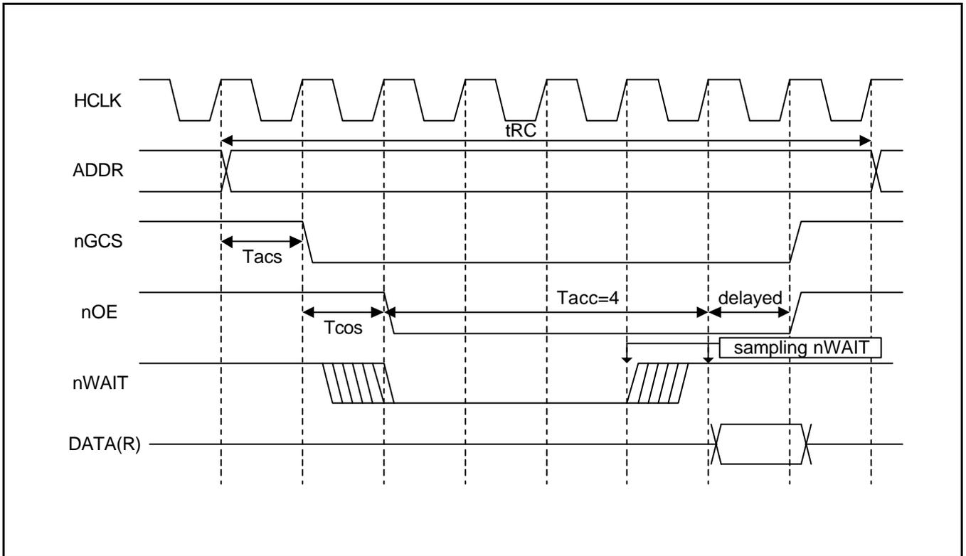
**Figure 5-2. S3C2410X01 External nWAIT Timing Diagram.(Tacc=4)**
