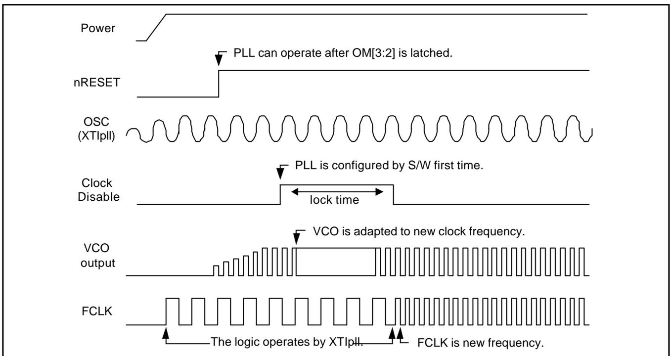
**Figure 6-4. Power-On Reset Sequence(When the external clock source is a crystal oscillator.)**
