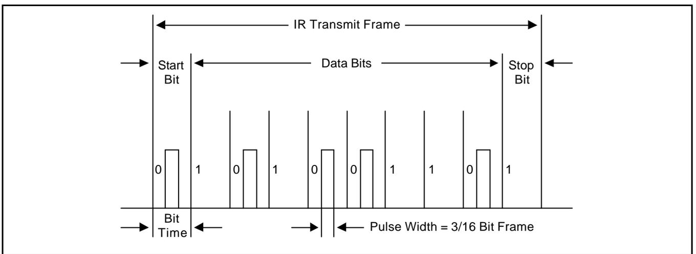
Figure 11-5. Infra-Red Transmit Mode Frame Timing Diagram
