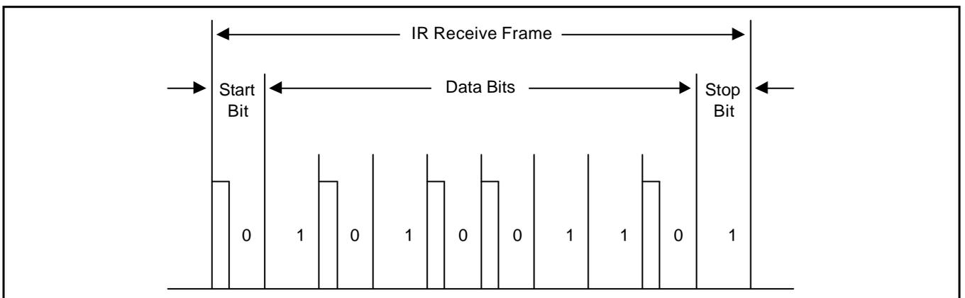
Figure 11-6. Infra-Red Receive Mode Frame Timing Diagram
