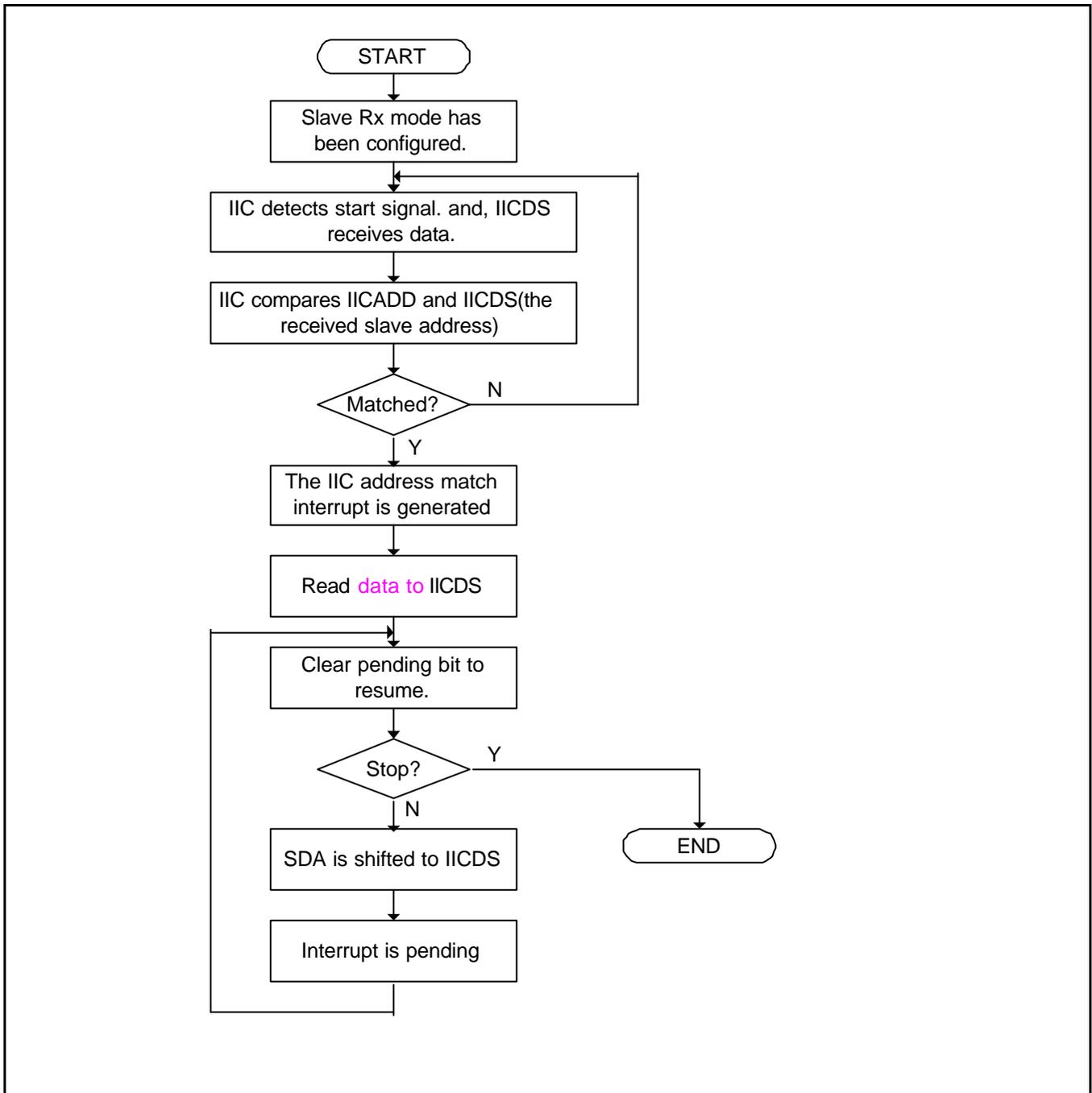
Figure 20-9 Operations for Slave / Receiver Mode
