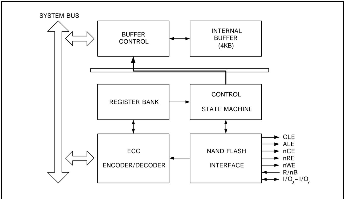
**Figure 23-1. NAND Flash Controller Block Diagram**
