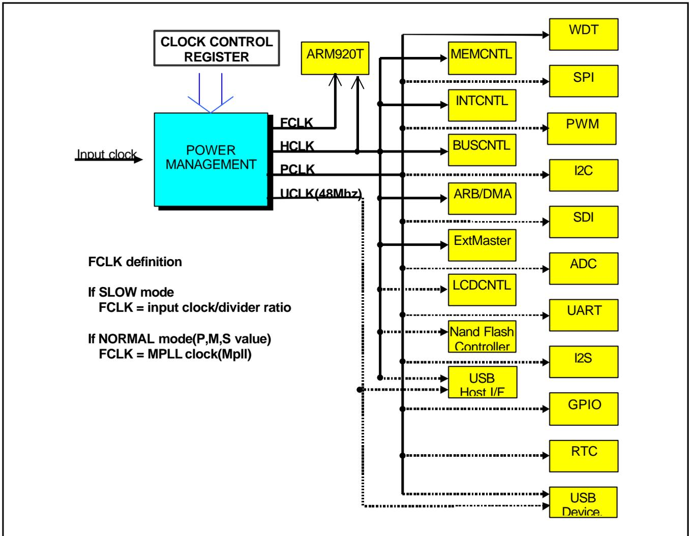
Figure 6-7. The Clock Distribution Block Diagram
