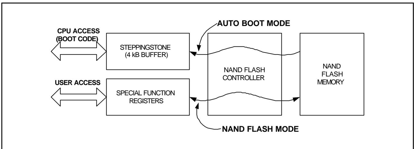
**Figure 23-2. NAND Flash Operation Scheme**
