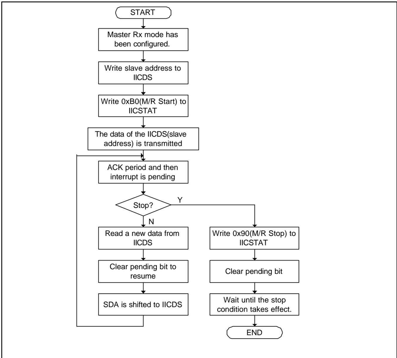
Figure 20-7 Operations for Master / Receiver Mode
