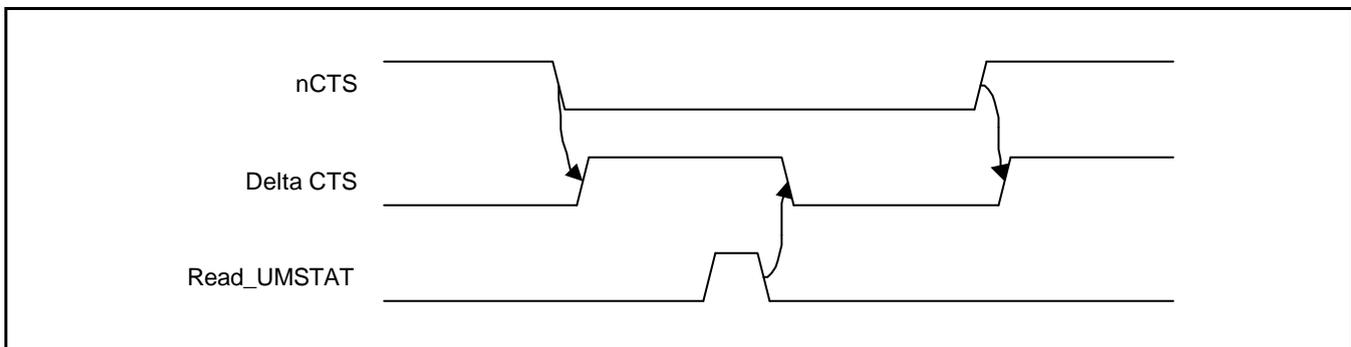
Figure 11-7. nCTS and Delta CTS Timing Diagram
