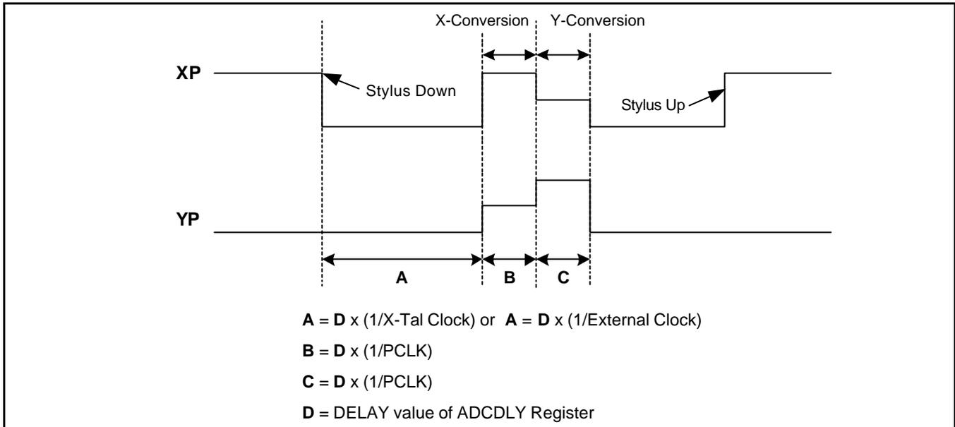
Figure 16-3 Timing Diagram at Auto (Sequential) X/Y Position Conversion Mode
