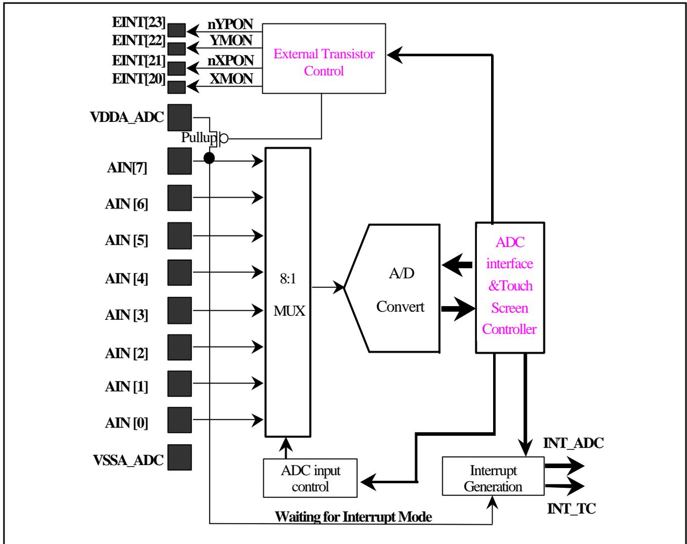
Figure 16-1. ADC and Touch Screen Interface Functional Block Diagram
