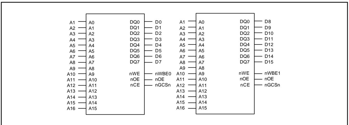
Figure 5-5. Memory Interface with 8bit ROM x 2
