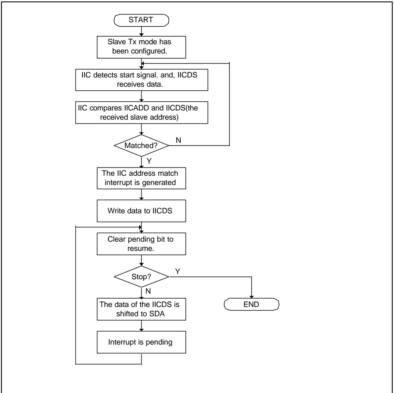
Figure 20-8 Operations for Slave / Transmitter Mode
