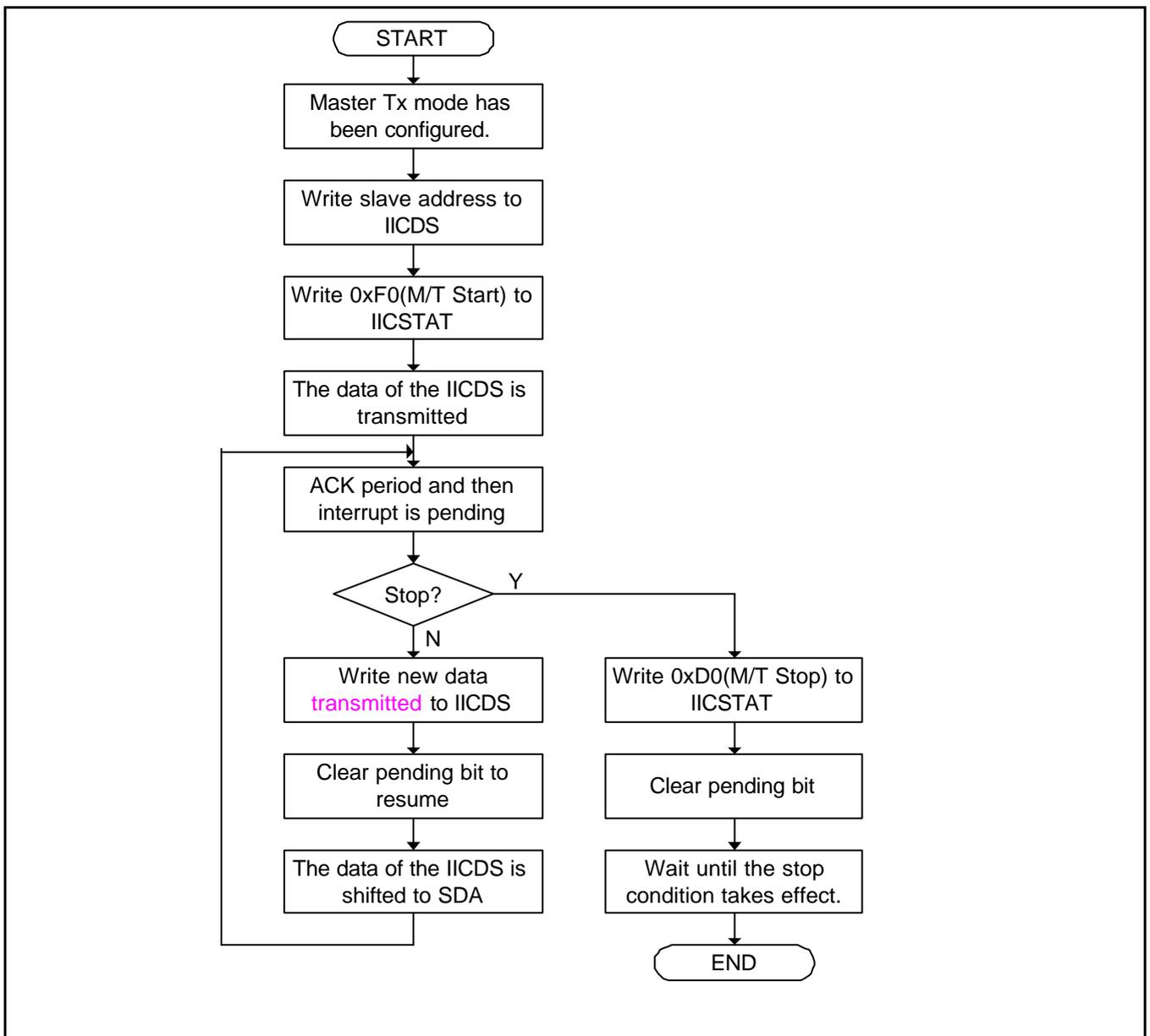
Figure 20-6 Operations for Master / Transmitter Mode
