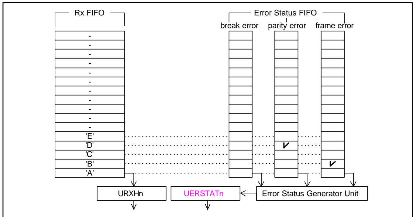
**Figure 11-3. Example showing UART Receiving 5 Characters with 2 Errors**
