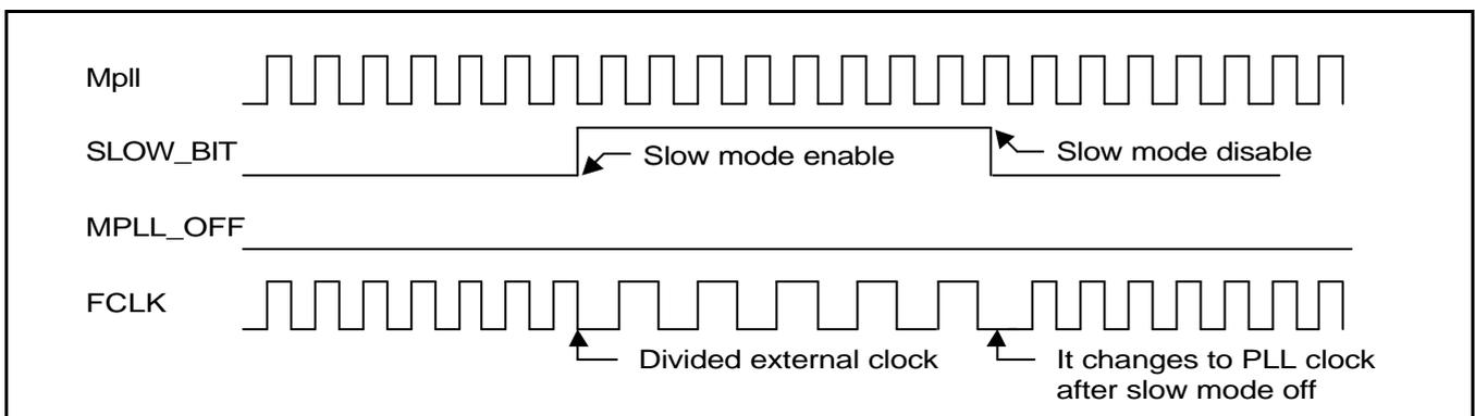
**Figure 6-11. The case that Exit\_from\_Slow\_mode command is issued in PLL on state**
