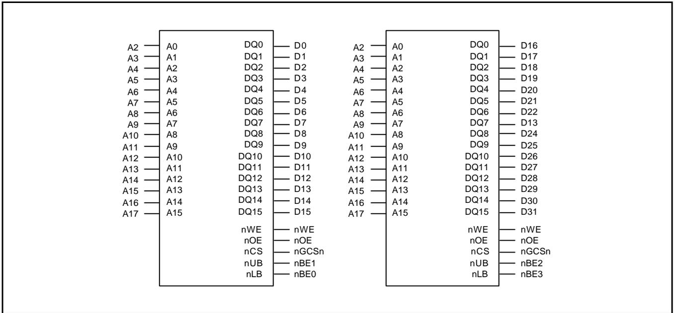
Figure 5-9. Memory Interface with 16bit SRAM x 2
