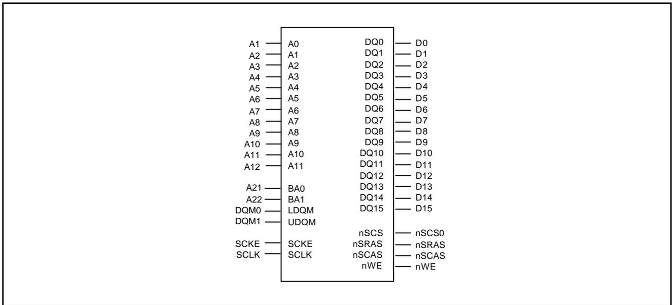
Figure 5-10. Memory Interface with 16bit SDRAM(4Mx16, 4bank)
