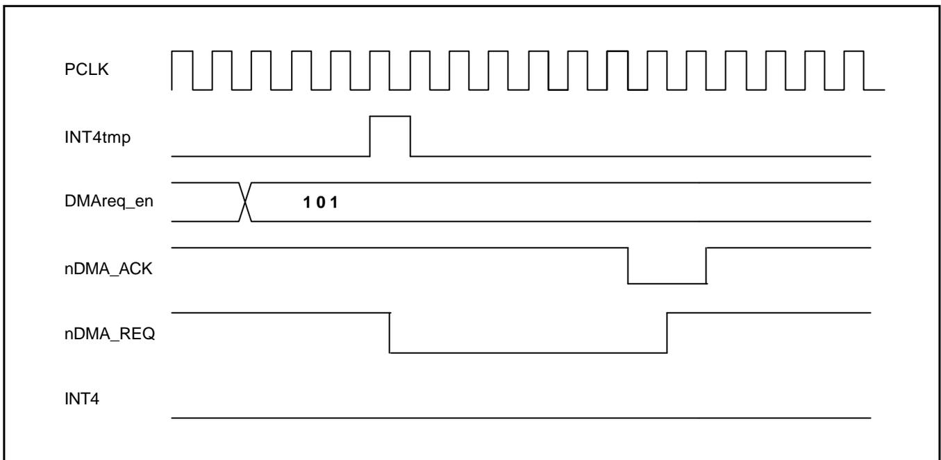
**Figure 10-8. The Timer4 DMA mode operation**
