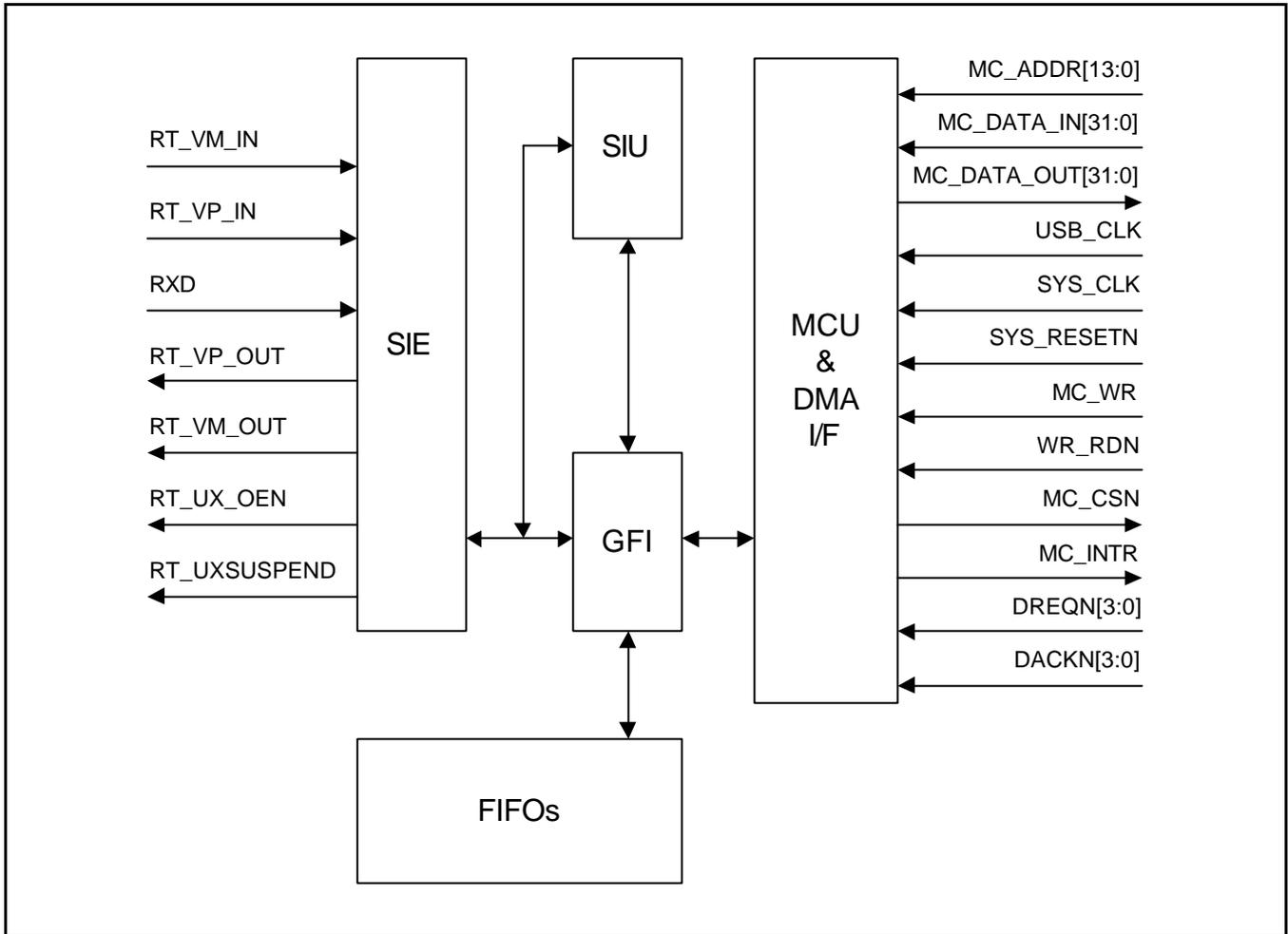
Figure 13-1. USB Device Block Diagram
