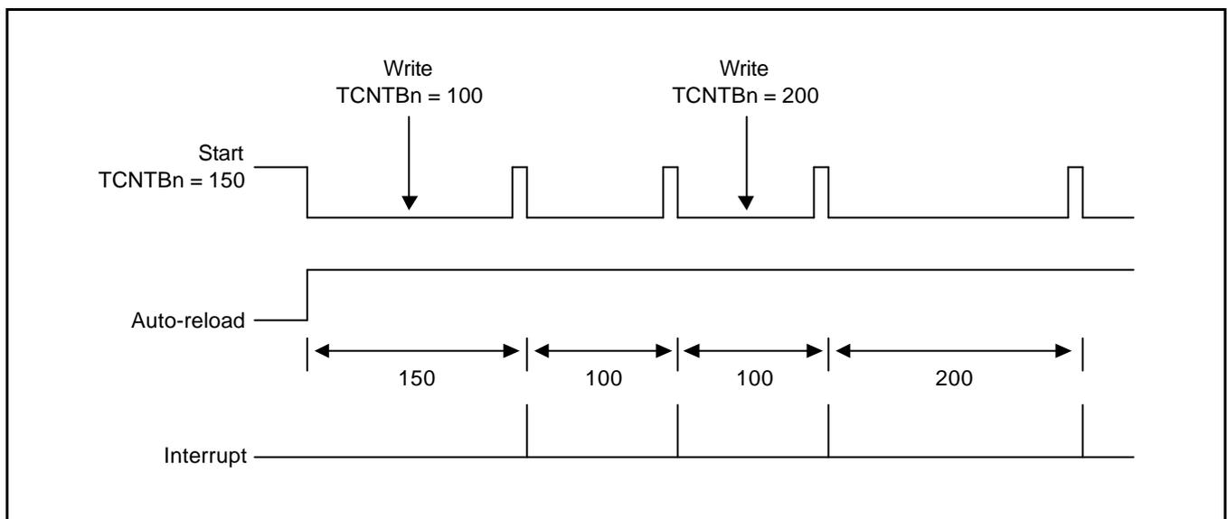
**Figure 10-3. Example of Double Buffering Feature**
