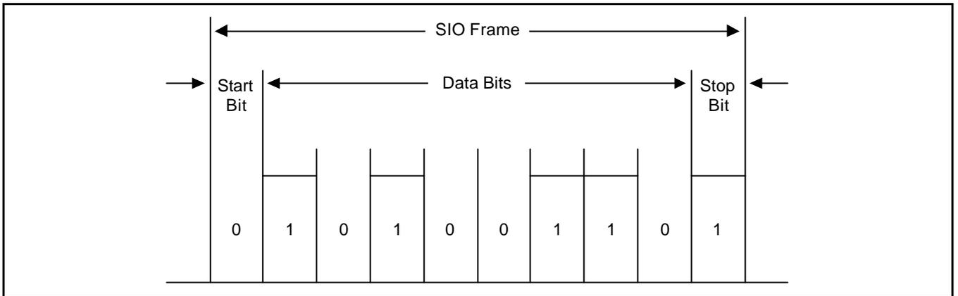
Figure 11-4. Serial I/O Frame Timing Diagram (Normal UART)
