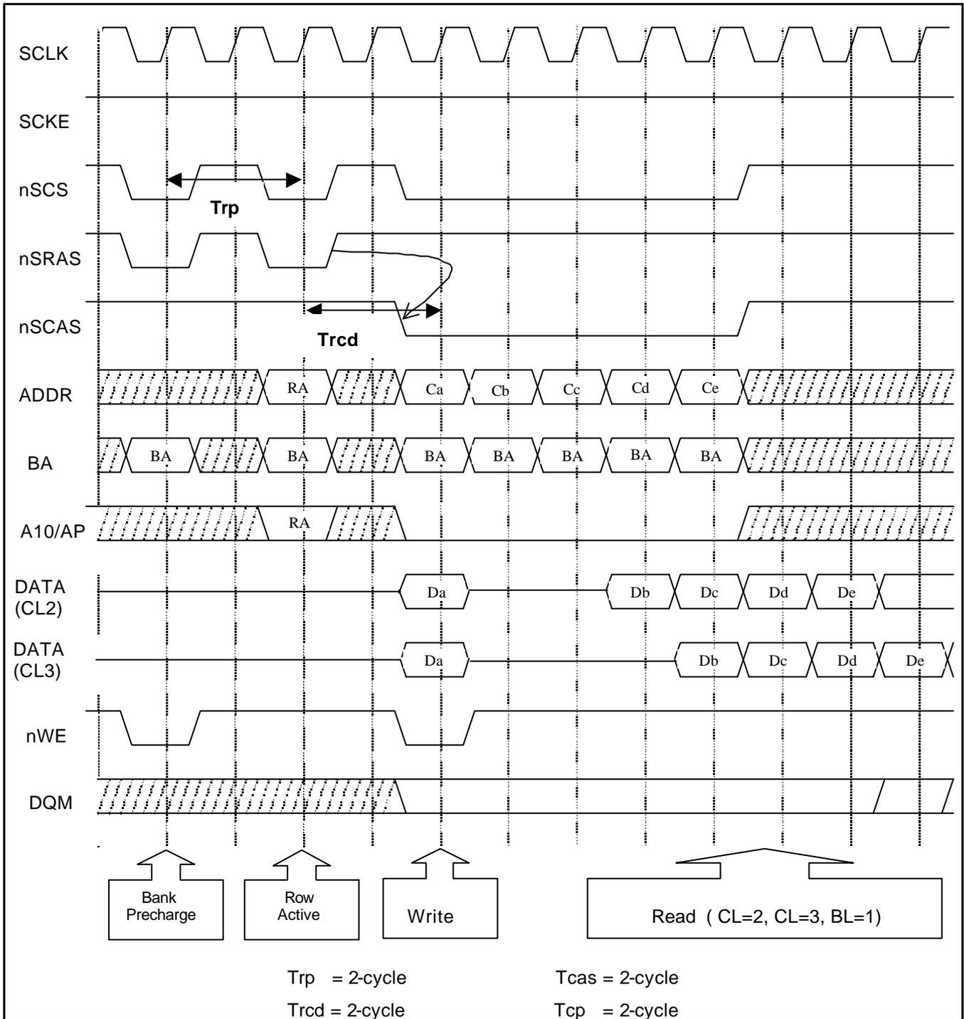
Figure 5-13. S3C2410X01 SDRAM Timing Diagram
