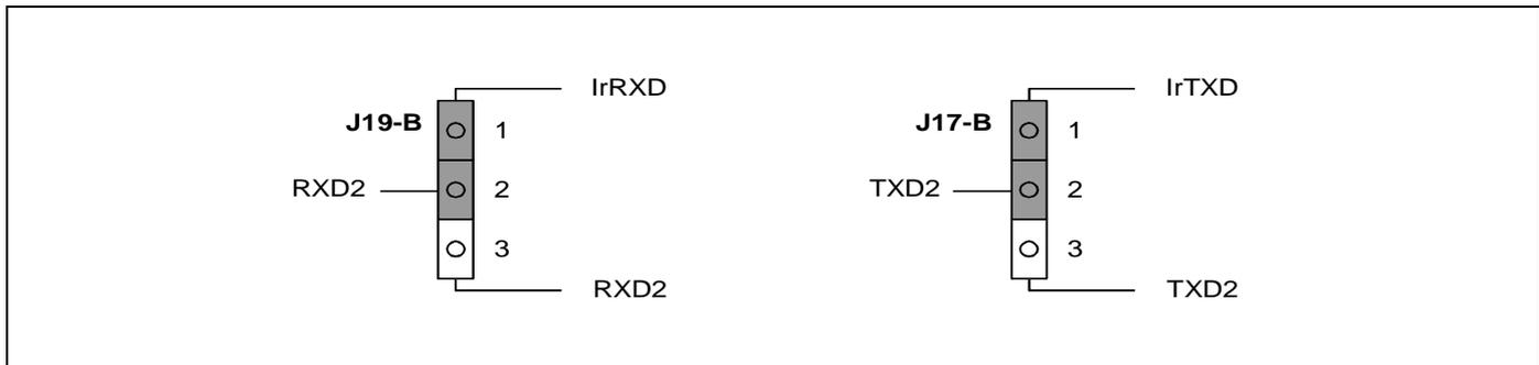
Figure 1-11. SMDK2440 Board IrDA Configurations
