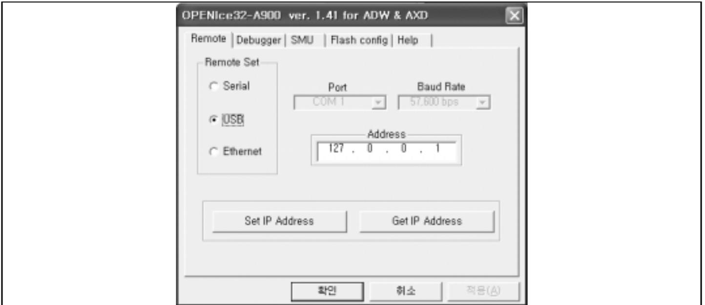
Figure 2-15. OPENice32-A900 Configuration: Communication Setting Page
