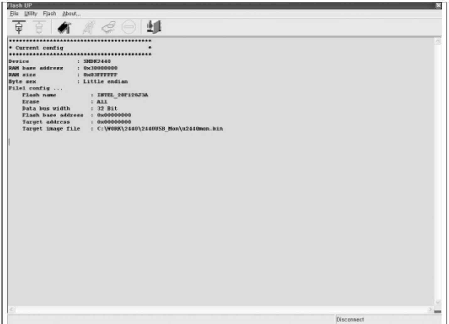
7. Select Write from the Flash Menu. Then it starts to erase the specified area of Intel Strata Flash and write the image to the Flash memory. It takes about 10 second.
