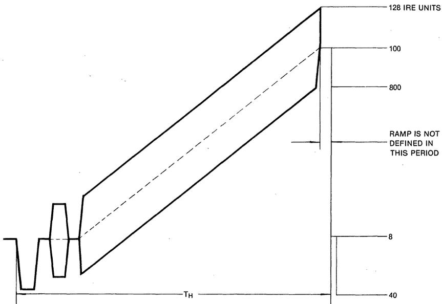
Fig. 2 Modulated Ramp Test Signal
