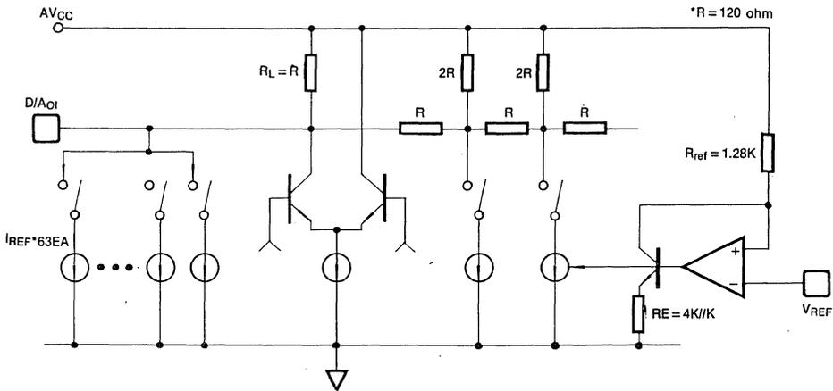
Fig. 6 Pin 6, 8, Reference Voltage and Analog Output
