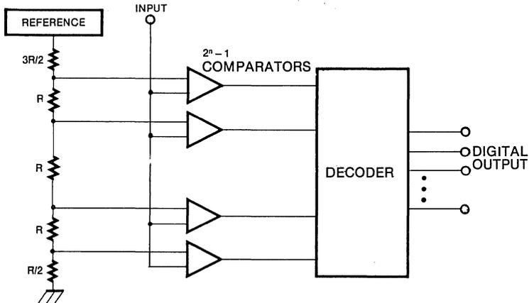
Fig. 4 Functional Block Diagram of Flash A/D Converter
