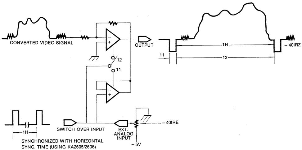
Add horizontal sync. pulse of video signal to the converted composited signal; result is the stabilized sync. pulse
