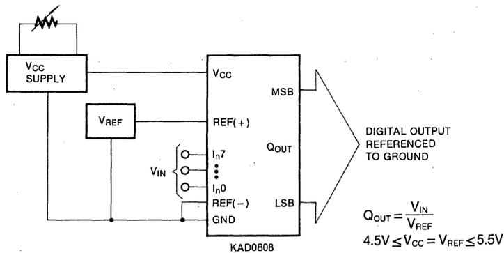
Fig. 10 Ground Referenced Conversion System Using Trimmed Supply
