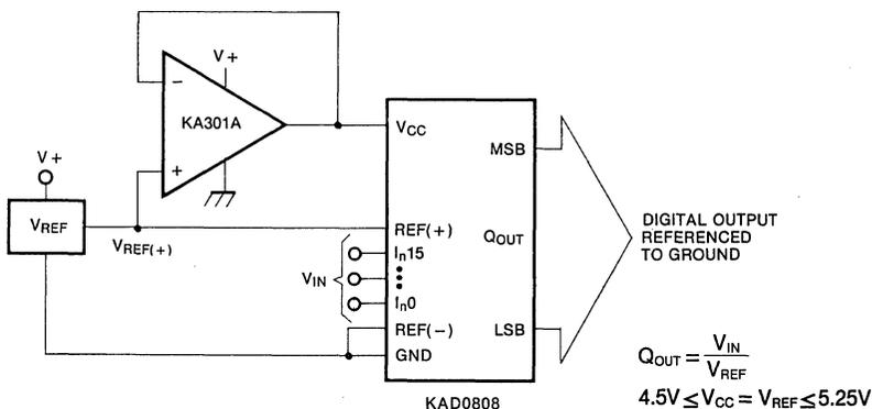
Fig. 6 Ground Referenced Conversion System with Reference Generating  $V_{CC}$  Supply
