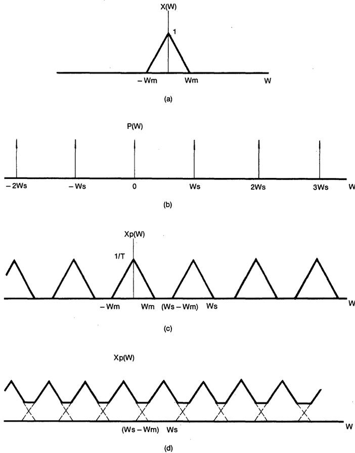
**Fig 3.** Effect in the frequency domain of sampling in the time domain:
