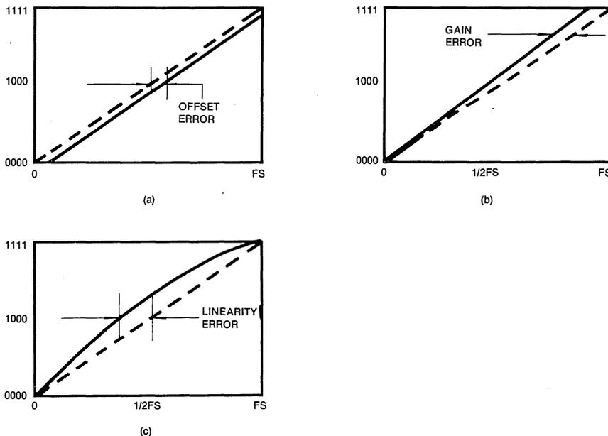
Fig. 1 Errors for an A/D Converter; (a) Offset; (b) Gain; (c) Linearity
