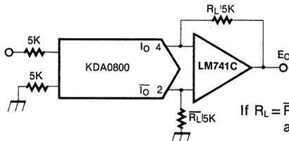
If  $R_L = \bar{R}_L$  within  $\pm 0.05\%$ , output is symmetrical about ground
