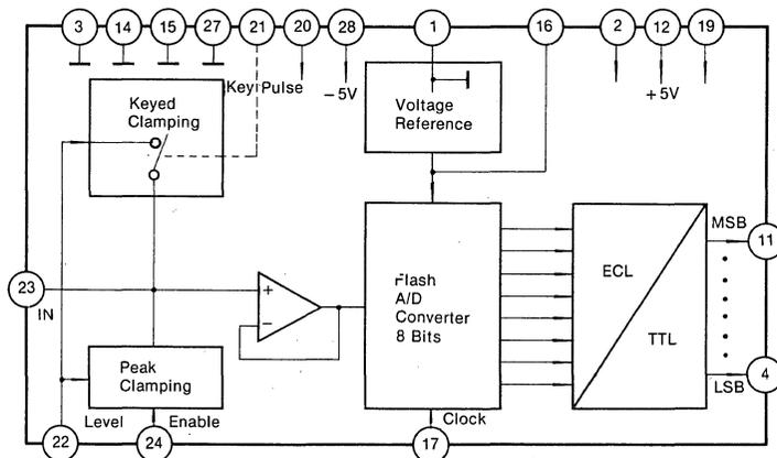
Fig. 4 KSV3208 Block Diagram
