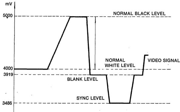
Fig. 10 With Inverse Signal Input
