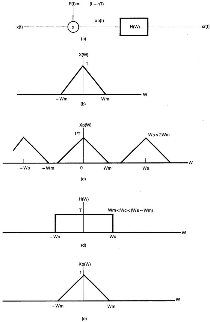
Fig. 4 Recovery of a original signal from its samples using an ideal lowpass-filter.
