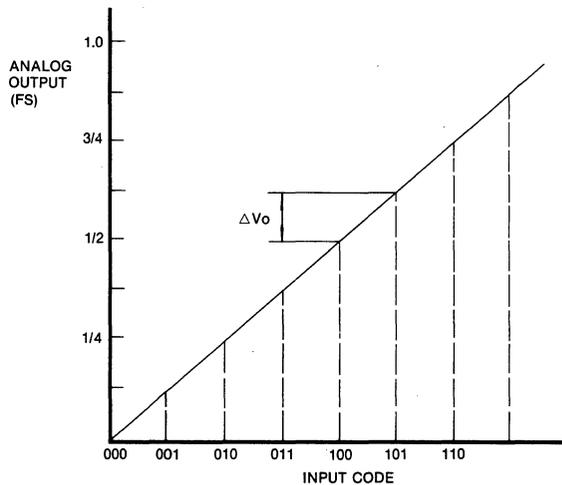
**Fig. 9 Transfer Function of Ideal 3-bit D/A Converter**
