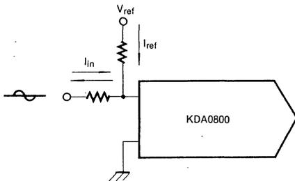
(b)  $+V_{ref}$  must be above peak positive swing of  $V_{IN}$
