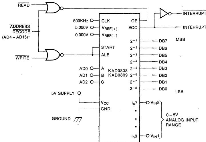
\* Address latches needed for 8085 and SC/MP interfacing the KAD0808 to a microprocessor
