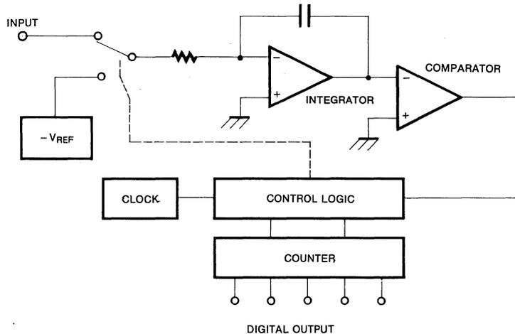
Fig. 6 Functional Block Diagram of Dual-Slope A/D Converter.
