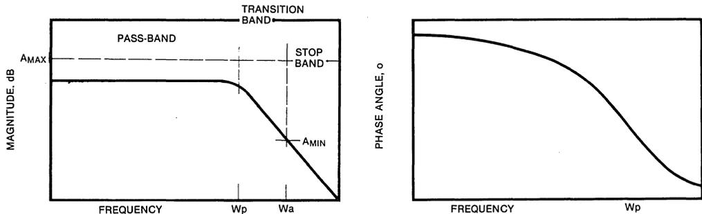
**Fig. 6** Typical filter magnitude and phase versus frequency response
