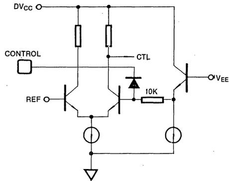
Fig. 5 Pin 3, 4, 5 & Pin 18, Control Signal & Clock Input
