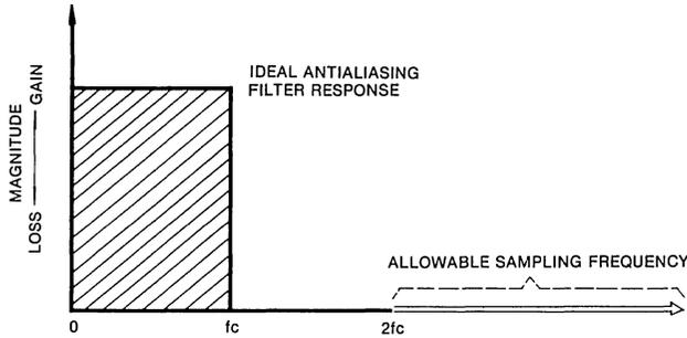
Fig. 2 Shown in the shaded area is an ideal, low pass, anti-aliasing filter response.
