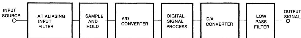
Fig. 5 Generalized single channel sample data system
