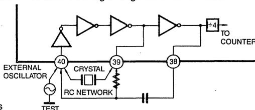
Fig. 8: Clock Circuits
