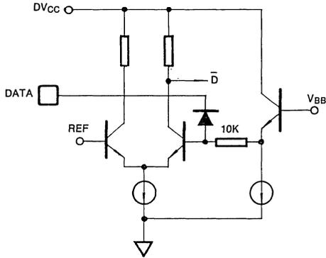
Fig. 4 Pin 19-26, Digital Input
