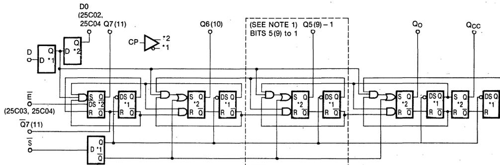
NOTE 1: Cell logic is repeated for register stages Q5 to Q1 KS25C02, KS25C03
