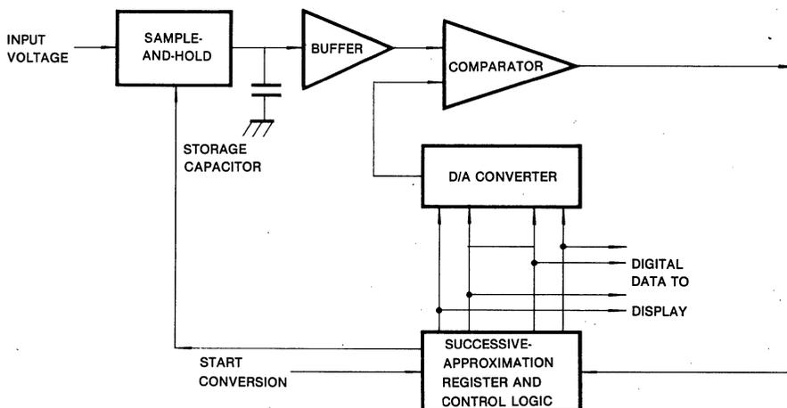
Fig. 9 Successive Approximation A/D Converter
