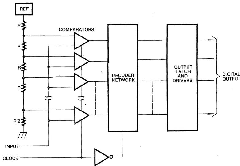
Fig. 1 Flash (Parallel) A/D Converter
