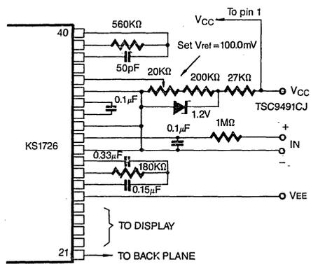
Figure 15: KS7126 with an External Band-Gap Reference (1.2V Typ) IN- is tied to Common. Values Shown are for One Reading Per Second.
