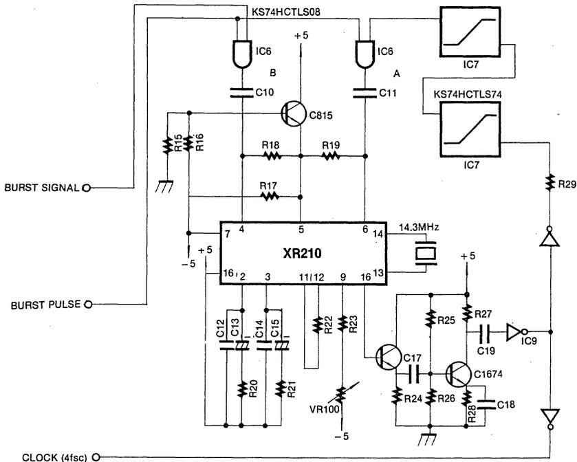
(The Clock Generator Circuit)
