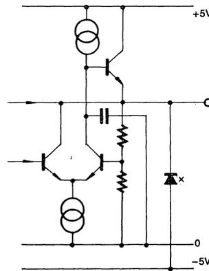
Fig. 8: Pin 25, Reference Voltage Pin
