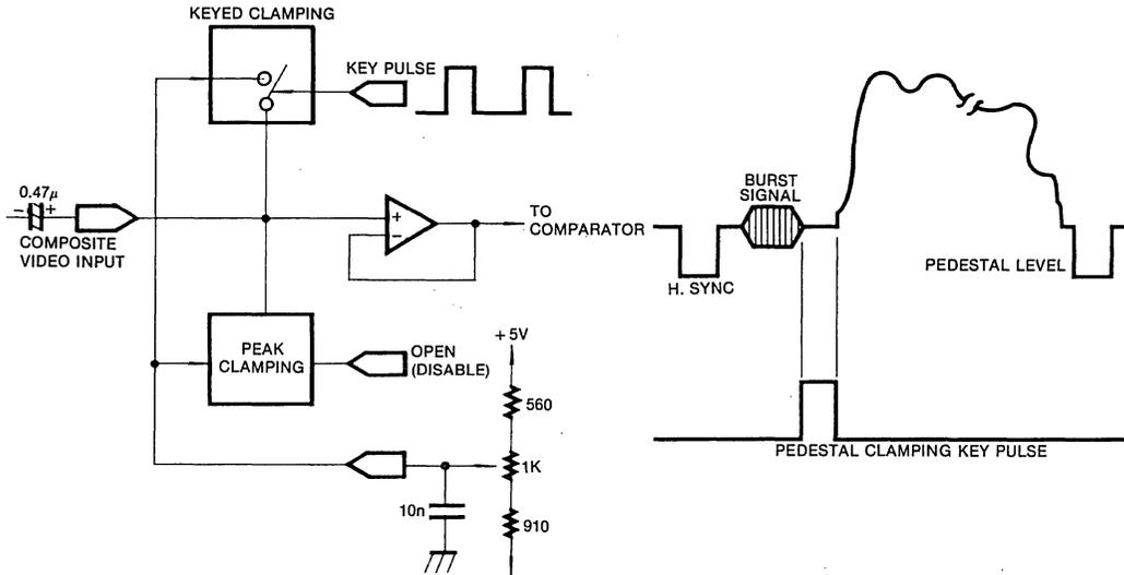
Fig. 7 Operating Keyed Clamping
