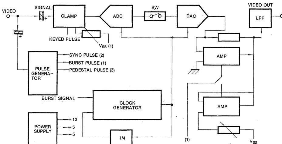
This demo board is a fully assembled and tested circuit board designed to aid the demonstration of KSV3110, 8 bit ADC and 10 bit DAC. The board contains circuitry for pulse generator, clock generator with KSV3110. The KSV3110 Demo Board consists of six functional sections, such as pulse generator, clock generator, clamp part, ADC, DAC, feed-in amp. The more detailed information is on the following pages.
