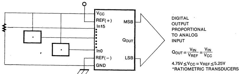
Fig. 4 Ratiometric Conversion System
