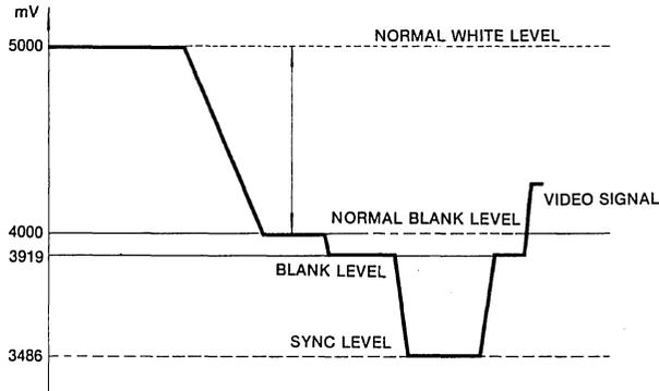
Fig. 9 Without Inverse Signal Input
