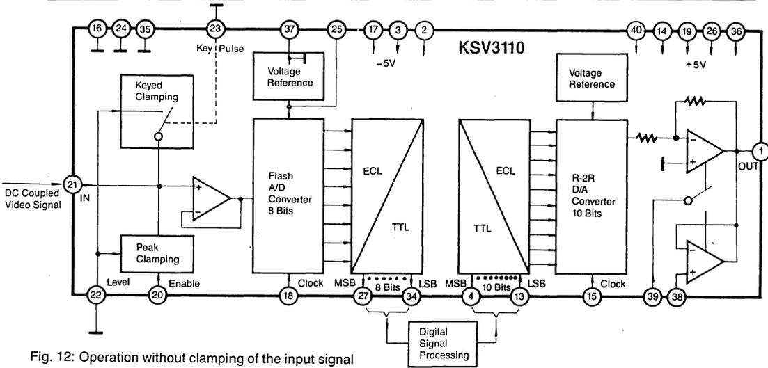
Fig. 12: Operation without clamping of the input signal
