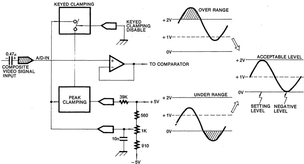
Input signal is clamped automatically to the negative peak value
