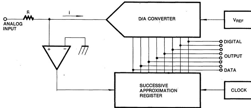
Fig. 2 Functional Block Diagram of Successive-Approximation A/D Converter.
