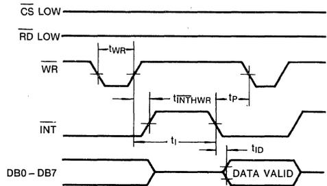
Fig. 4 WR-RD Mode (Pin 7 is High)
