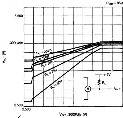
GRAPHICS PLOT ( $V_{REF}$  VS  $AV_{OUT}$  WITH BLANK, SYNC)
