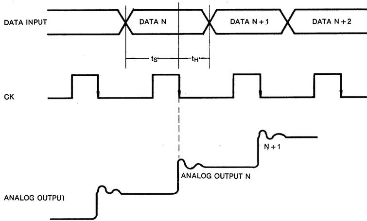
Fig. 11 KSV3110 Timing Diagram (D/A)
