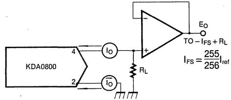
For complementary output (operation as a negative logic DAC) connect non-inverting input of op amp to  $I_0$  (pin 2); connect  $I_0$  (pin 2); connect  $I_0$  (pin 4) to ground.
