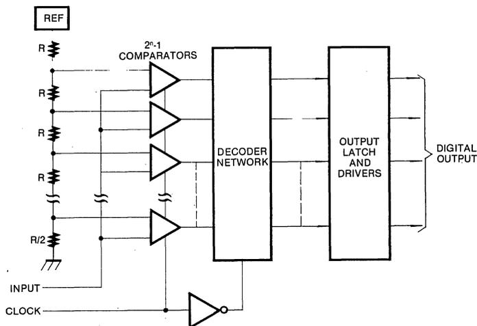
Fig. 3 Flash (Parallel) A/D Converter
