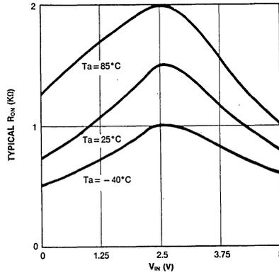
Fig. 7 Multiplexer  $R_{ON}$  vs  $V_{IN}$  ( $V_{CC} = V_{REF} = 5V$ )
