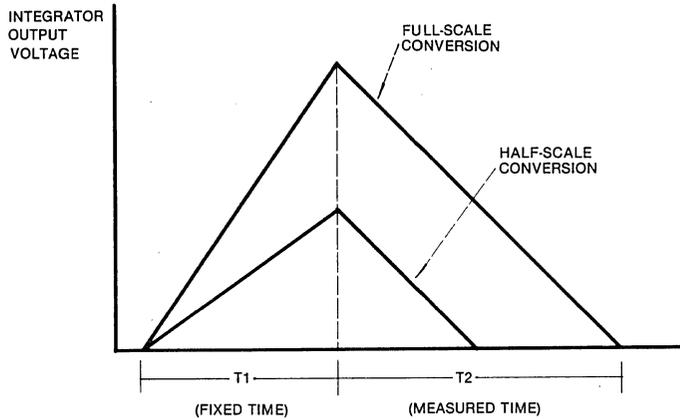
Fig. 7 Integrator Output Waveform for Dual-Slop A/D Converter
