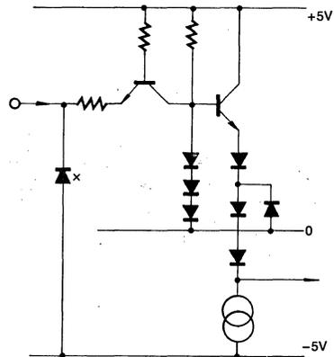
Fig. 5: Pins 4 to 13, 15, 18, 23 and 39, Inputs
