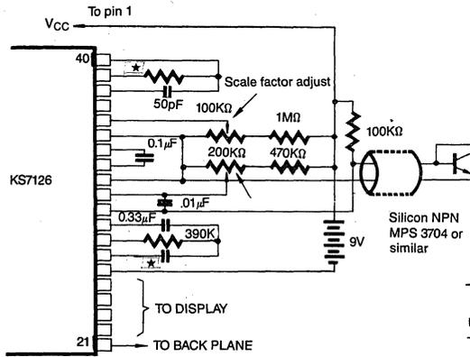
Figure 16: KS7126 Used as a Digital Centigrade Thermometer. A Silicon Diode-Connected Transistor Has a Temperature Coefficient of About 2mV/°C.
