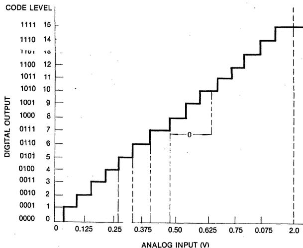
Fig. 2 The Quantizer Transfer Function for a 4-Bit Parallel A/D Converter
