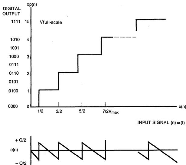
Fig. 8 Quantization characteristics.
