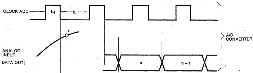
(The Timing Diagram of A/D Part)
