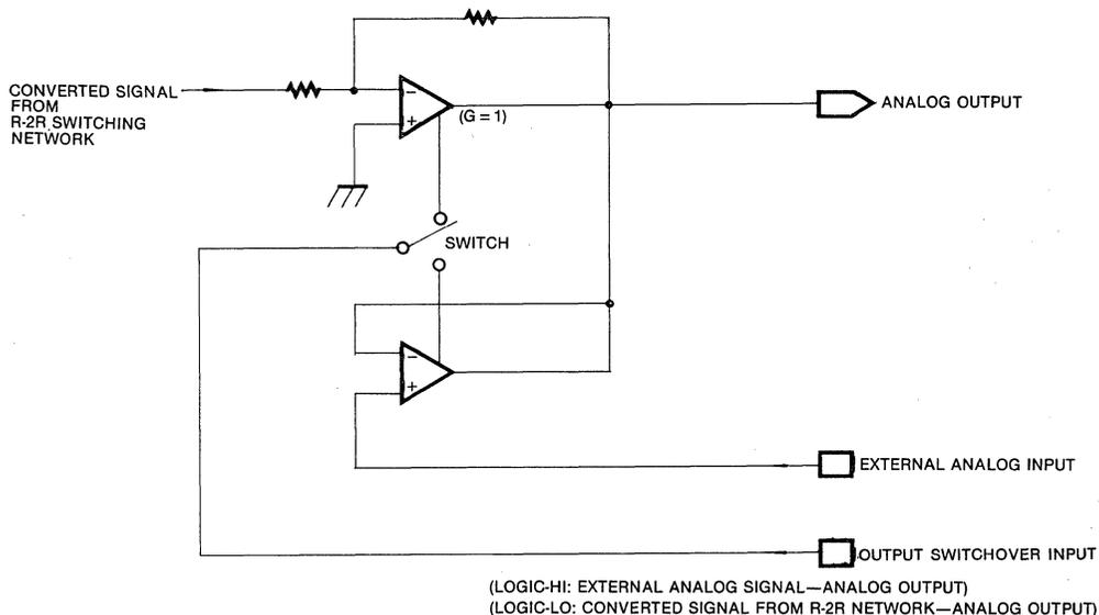
Fig. 8 KSV3110-DA Output Signal Switchover Circuit
