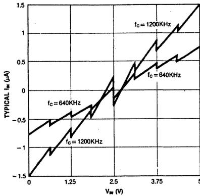
Fig. 1 Comparator  $I_{IN}$  vs  $V_{IN}$  ( $V_{CC} = V_{REF} = 5V$ )
