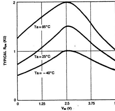
Fig. 2 Multiplexer  $R_{ON}$  vs  $V_{IN}$  ( $V_{CC} = V_{REF} = 5V$ )
