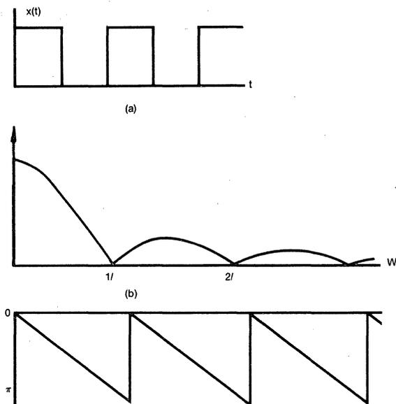
Fig. 11 (b) Magnitude and (c) phase frequency response of the sampling pulse (a).
