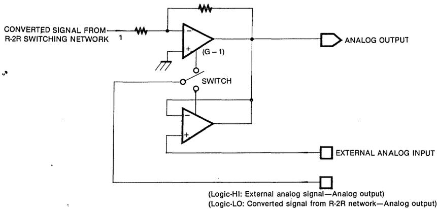
When the pin 39 of KSV3110 is high, the external signal which is connected to the pin 38 is out and when the pin 39 of KSV3110 is low, the converted signal is out. In the KSV3110 Demo Board, this block is used for adding the horizontal sync pulse to the converted composite video signal.
