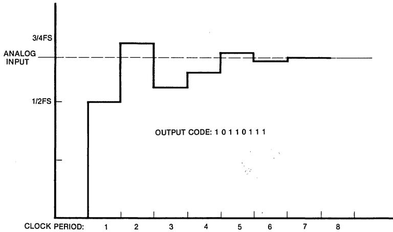
Fig. 3 D/A Output for 8-Bit Successive-Approximation Conversion
