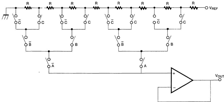
Fig. 12 3-Bit D/A Converter Example Using Voltage-Scaling Principle
