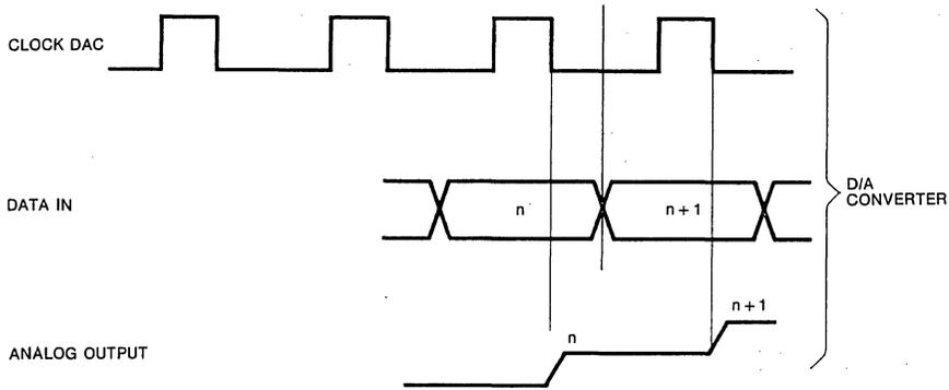
(The Timing Diagram of D/A Part)
