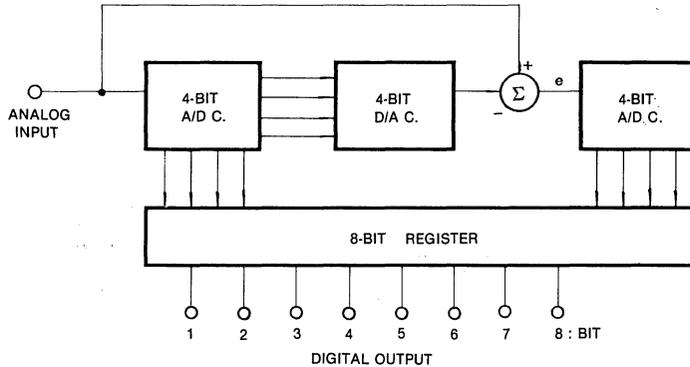
Fig. 5 Functional Block Diagram of Subranging A/D Converter
