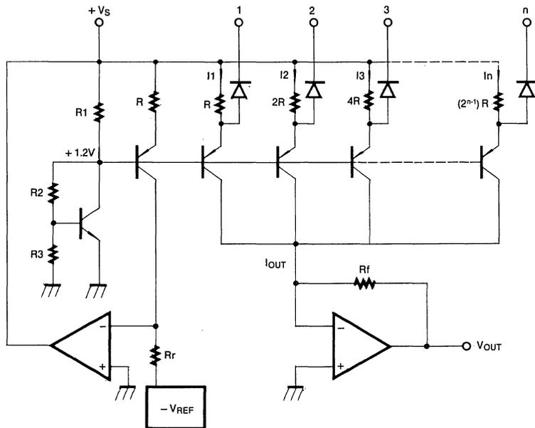
Fig. 10 Weighted Current Source D/A Converter
