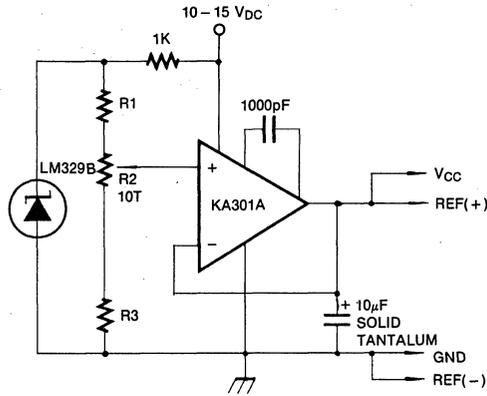
Fig. 7 Typical Reference and Supply Circuit
