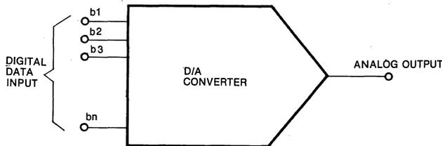
**Fig. 8 Functional Block Diagram of a Basic D/A Converter**
