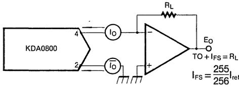
For complementary output (operation as negative logic DAC), connect inverting input of op amp to  $\bar{I}_0$  (pin 2), connect  $I_0$  (pin 4) to ground.
