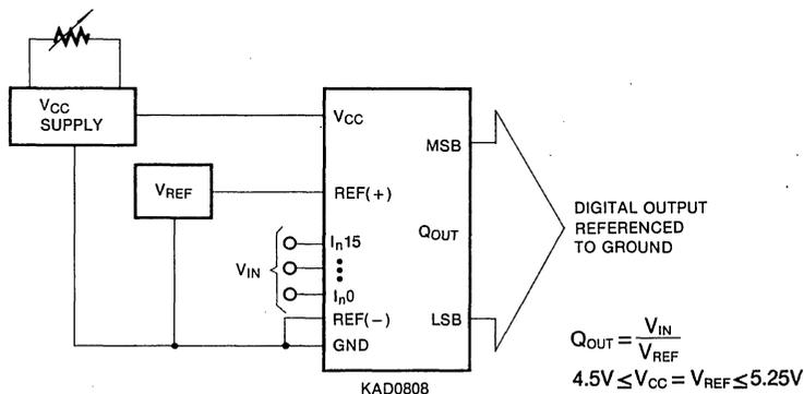
Fig. 5 Ground Referenced Conversion System Using Trimmed Supply
