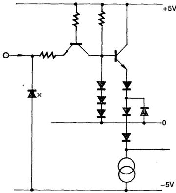
Fig. 5: Pins 4 to 13, 15, 18, 23 and 39, Inputs
