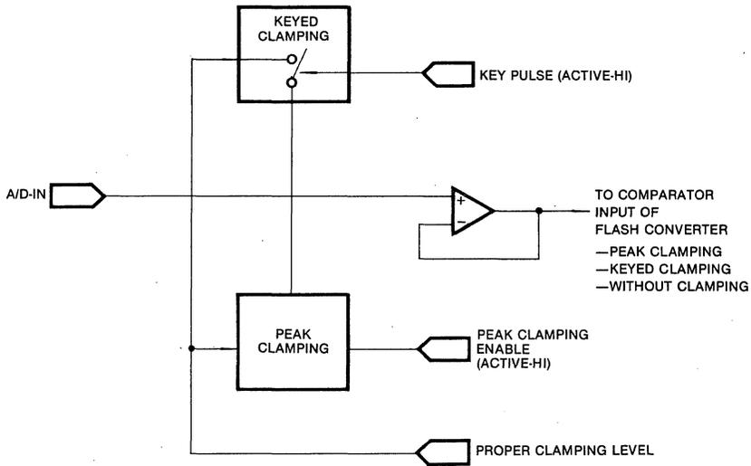
Fig. 5 KSV3208, KSV3110 Clamping Circuit for A/D Input
