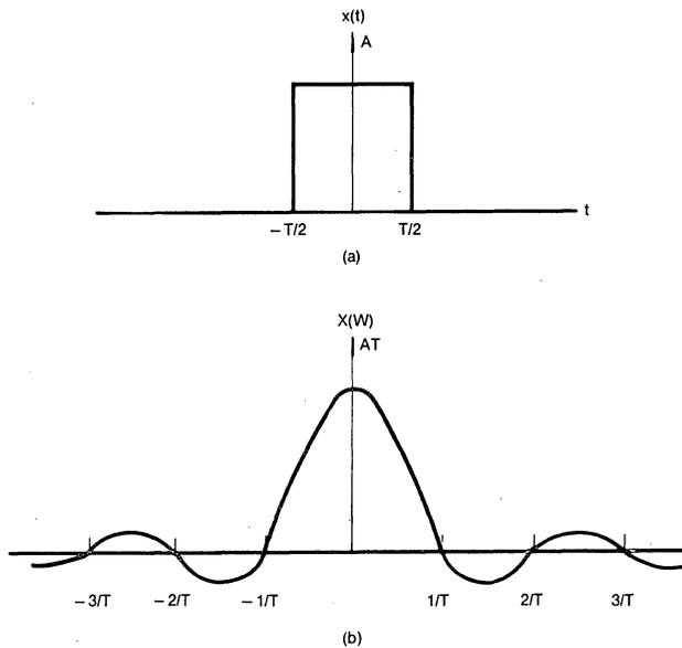
Fig. 10 The Fourier transform of the rectangular pulse (a) is shown in (b).
