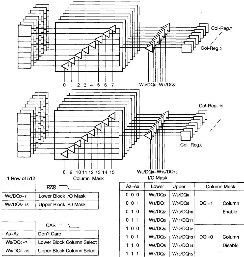
Figure 5. Block Write Scheme
