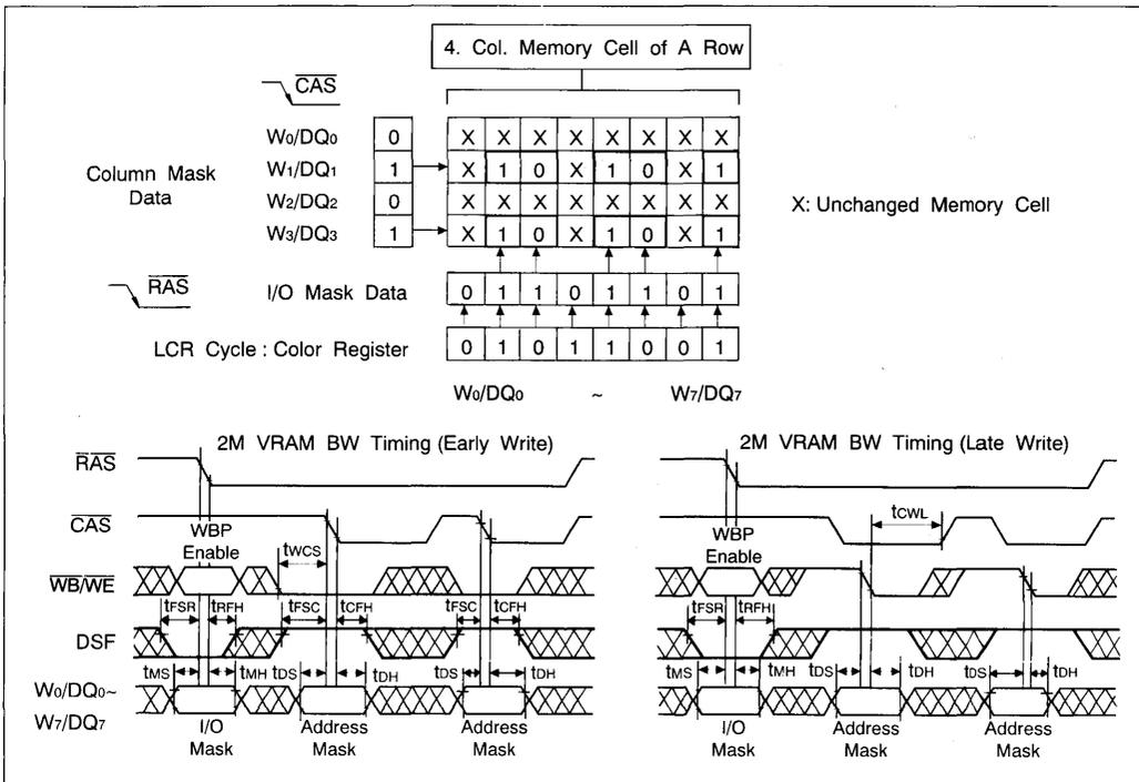
Figure 5. Block Write Example and Timing
