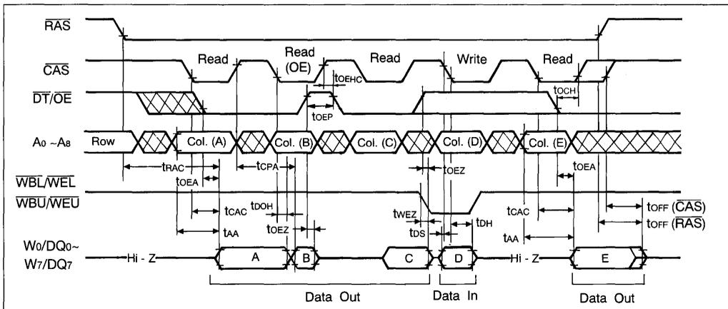
Figure 1. Extended Data Output Example
