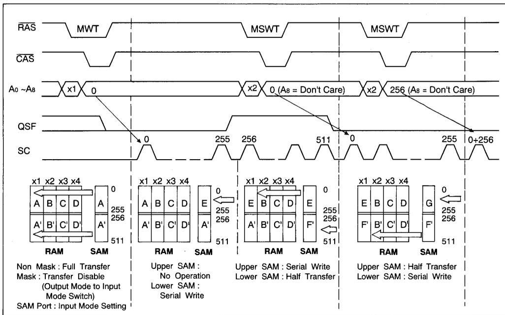
Figure 11. Masked Split Write Transfer Normal Usage
