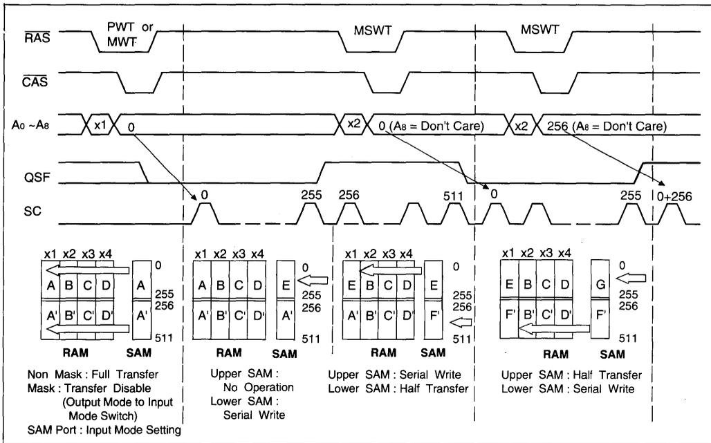
Figure 10. Masked Split Write Transfer Normal Usage
