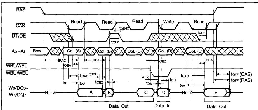
Figure 1. Extended Data Output Example
