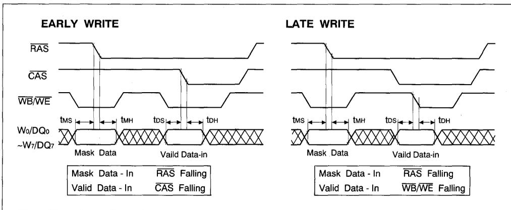
Figure 2. New Mask Write Cycle Example 1 (Early Write & Late Write)
