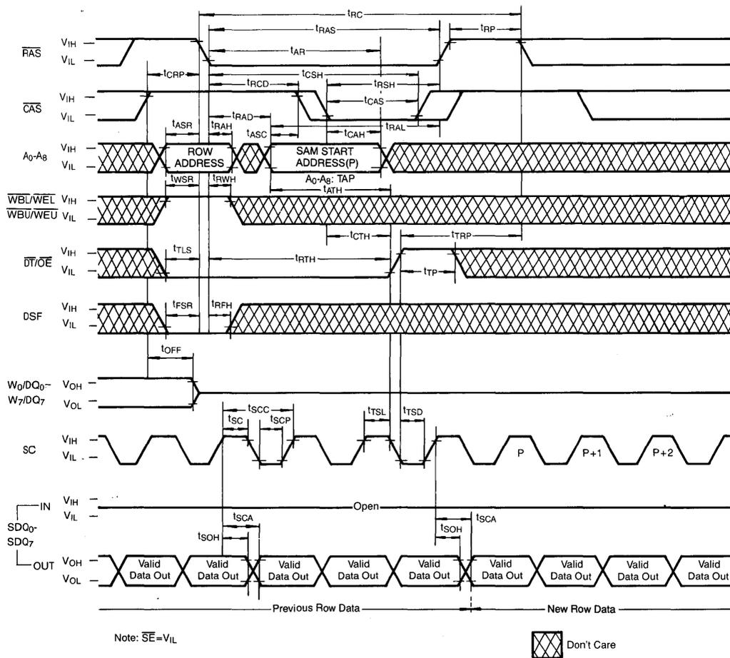
**MASKED WRITE TRANSFER CYCLE (Output Mode to Input Mode Switch)**
