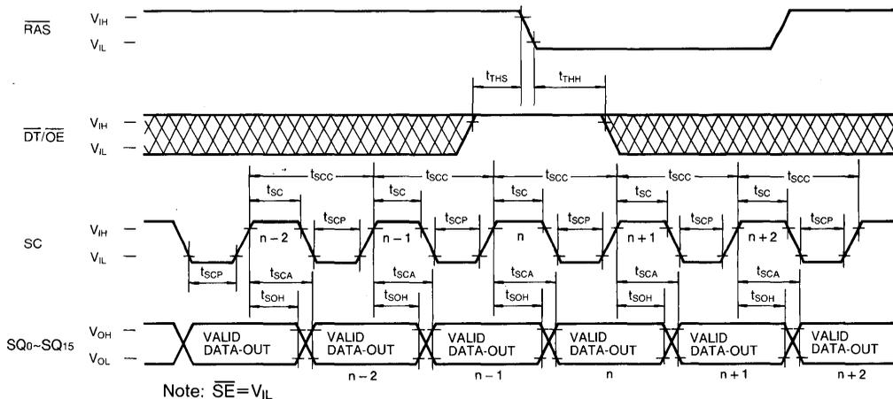
**SERIAL READ CYCLE ( $\overline{SE}$  Controlled Outputs)**
