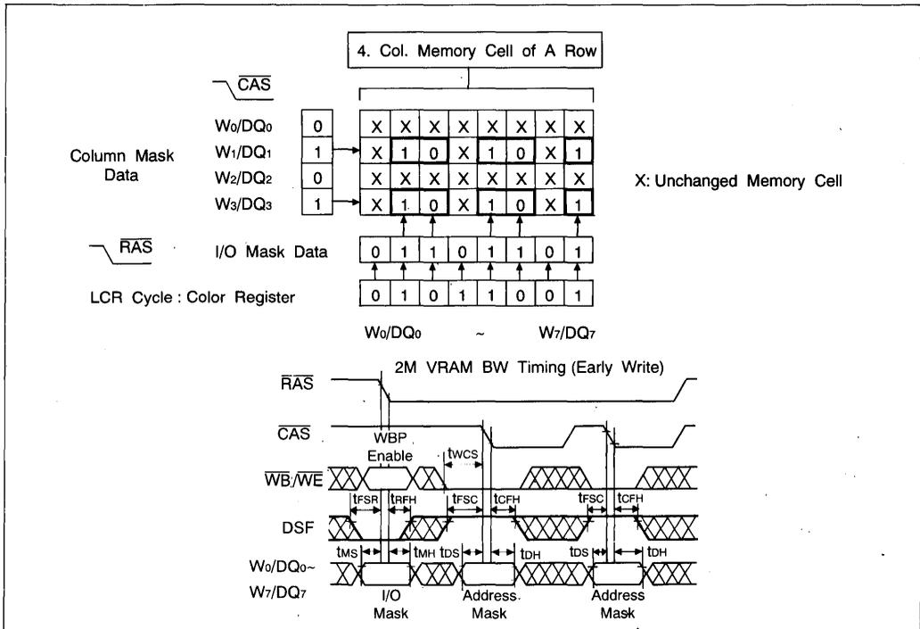
Figure 4. Block Write Example and Timing
