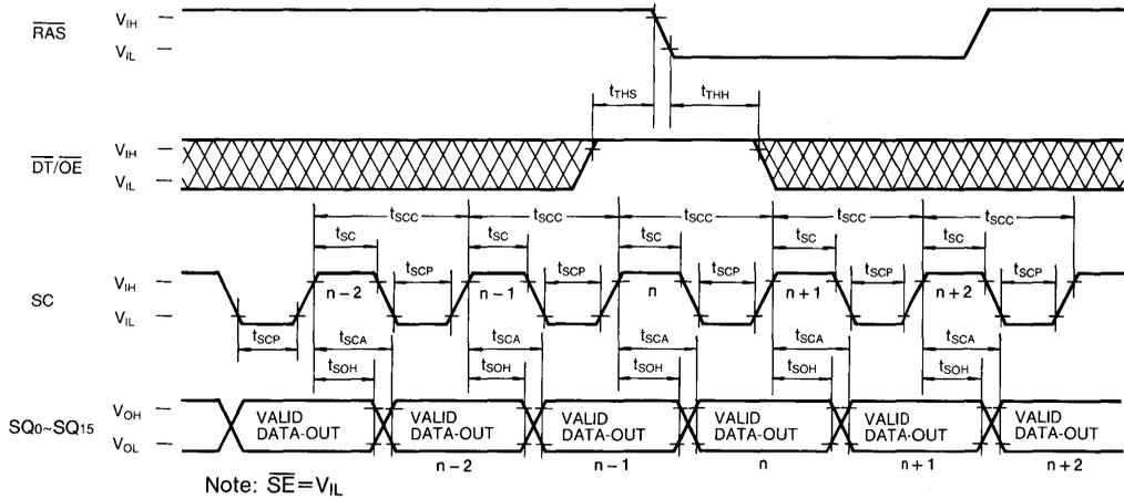
SERIAL READ CYCLE ( $\overline{SE}$  Controlled Outputs)
