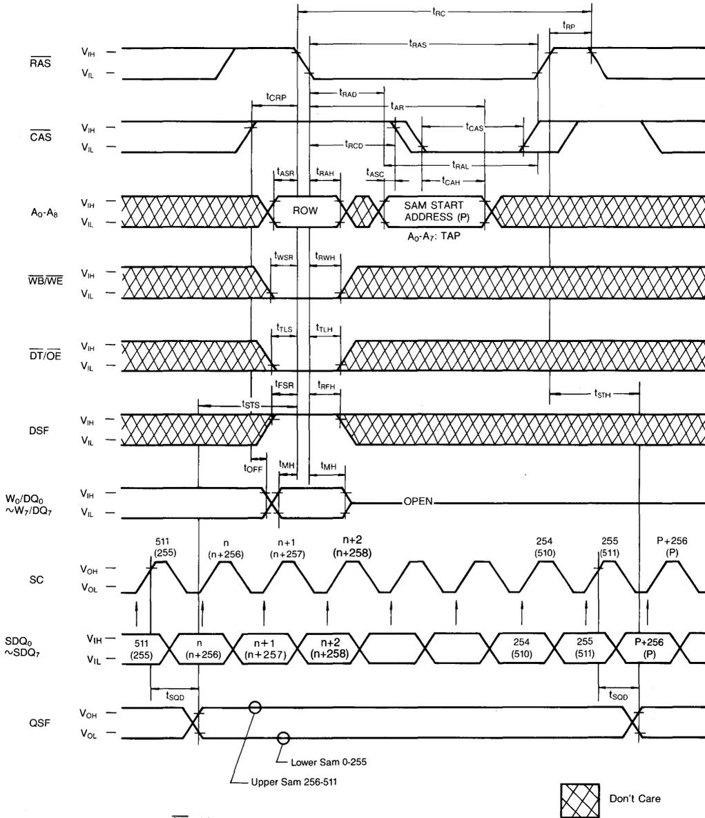
**SERIAL READ CYCLE ( $\overline{SE} = V_{IL}$ )**
