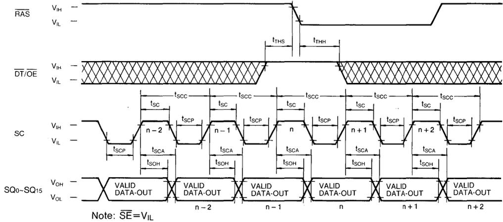
SERIAL READ CYCLE ( $\overline{SE}$  Controlled Outputs)
