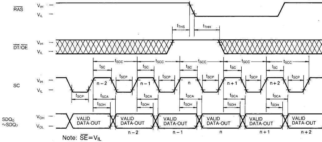
SERIAL READ CYCLE ( $\overline{SE}$  Controlled Outputs)
