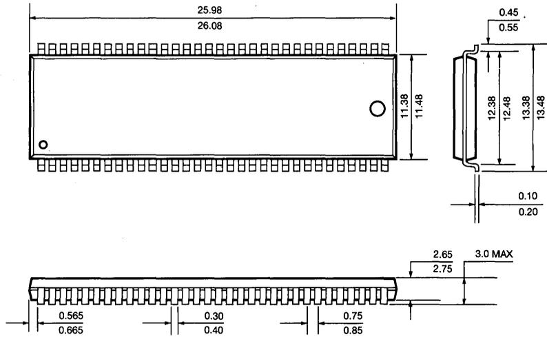
**70(64) Pin Plastic Thin Small Out Line Package (Type II Forward)**
