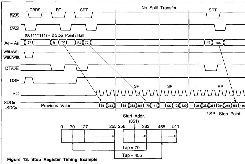
**Figure 13. Stop Register Timing Example**
