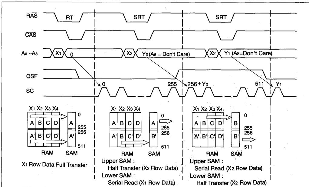
Figure 7. Split Read Transfer Normal Usage (Case1)
