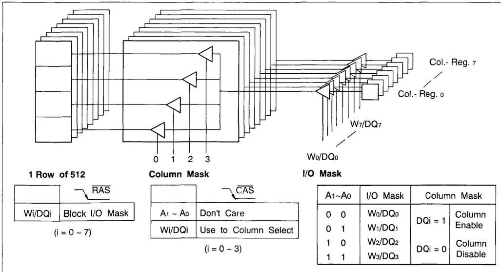
Figure 4. Block Write Scheme
