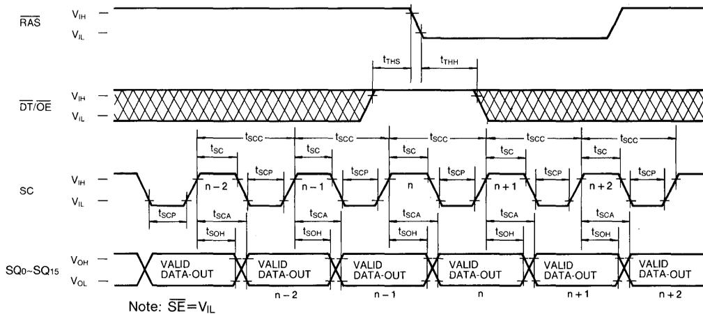
SERIAL READ CYCLE ( $\overline{SE}$  Controlled Outputs)
