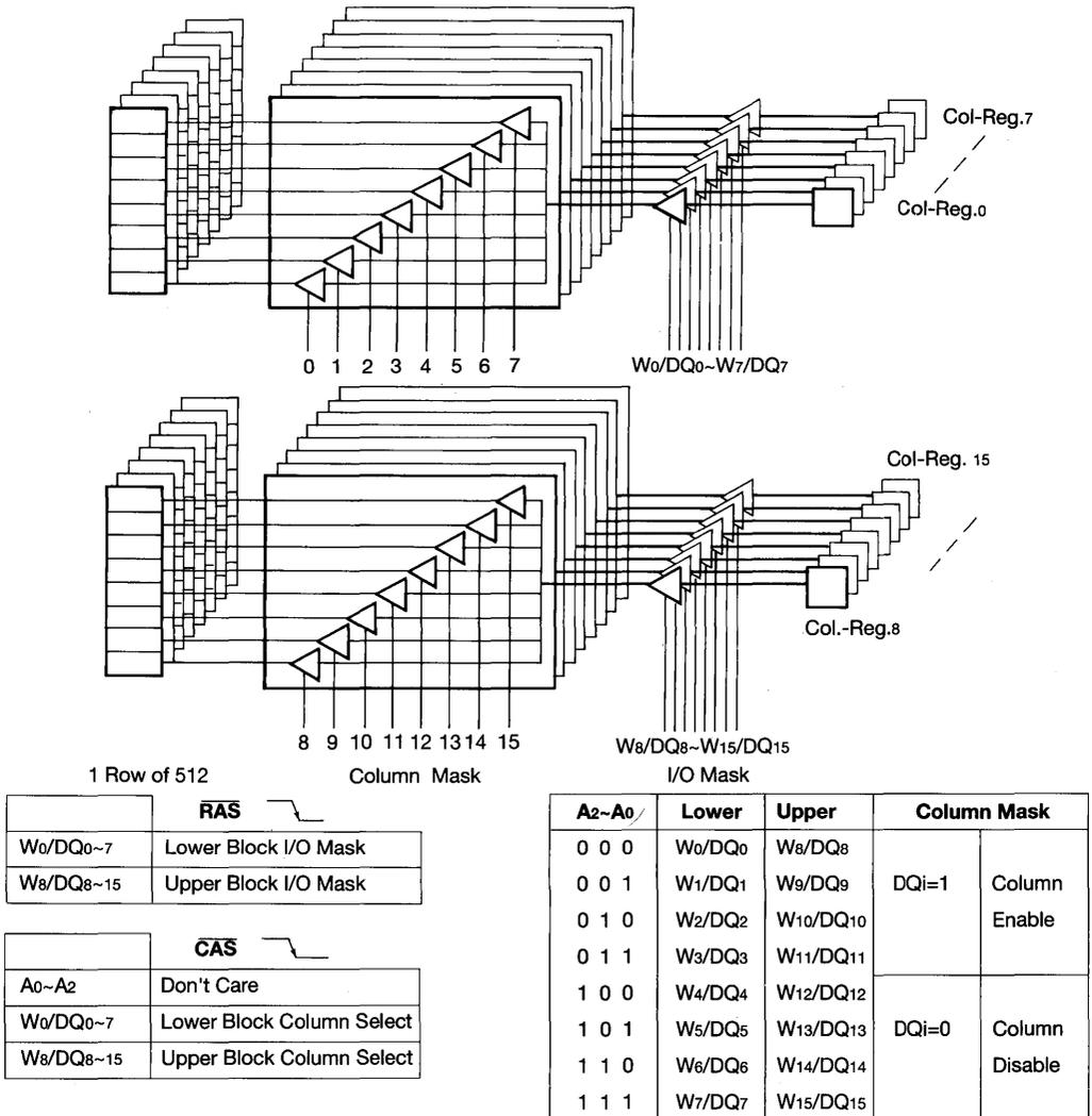
Figure 5. Block Write Scheme
