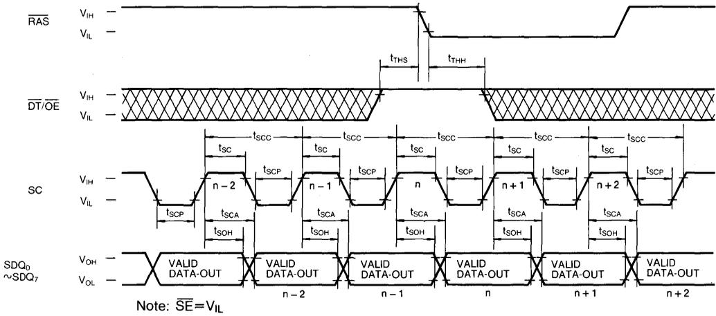
SERIAL READ CYCLE ( $\overline{SE}$  Controlled Outputs)
