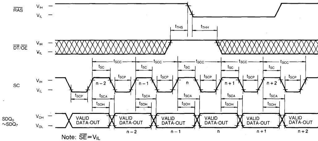
SERIAL READ CYCLE ( $\overline{SE}$  Controlled Outputs)
