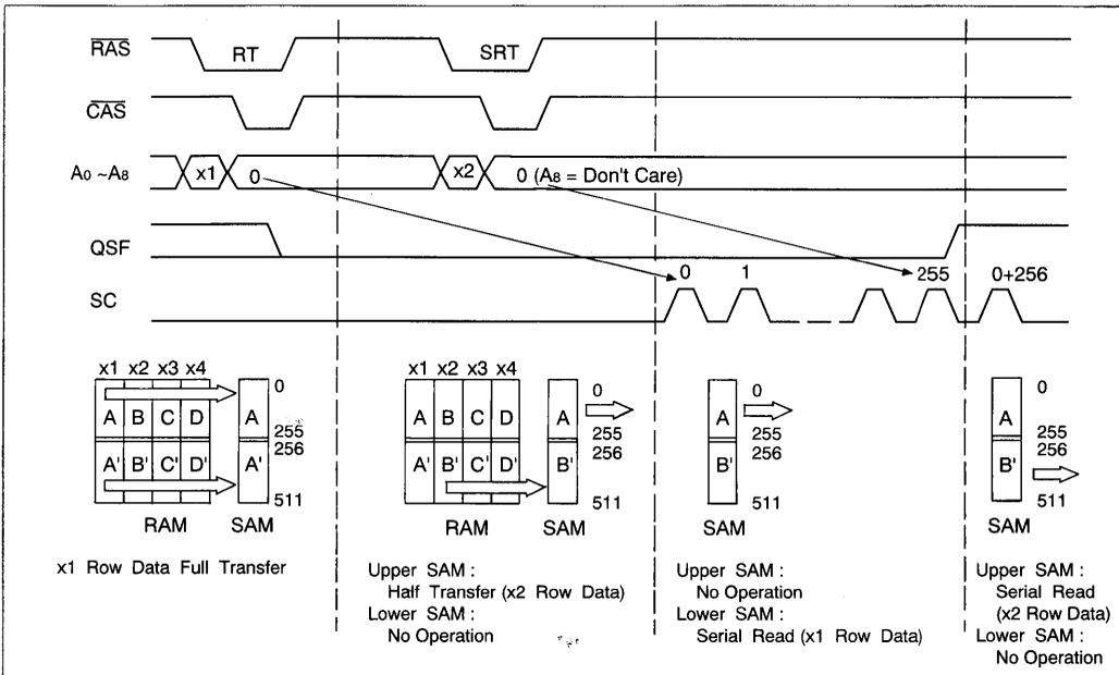
Figure 7. Split Read Transfer Normal Usage
