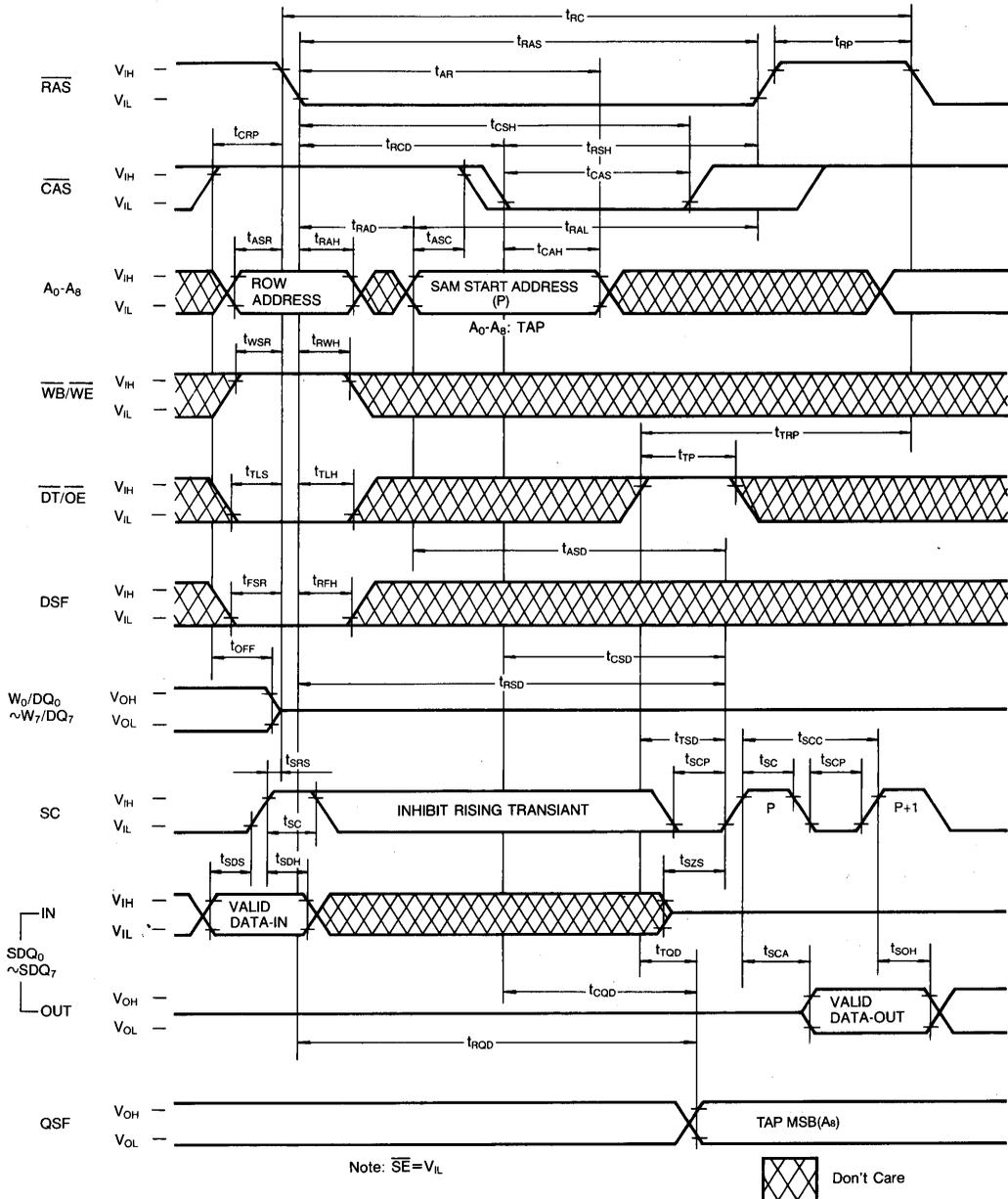
**MASKED WRITE TRANSFER CYCLE (Output Mode to Input Mode Switch)**
