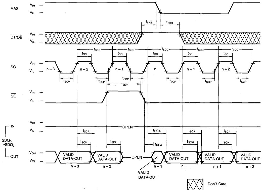
SERIAL WRITE CYCLE ( $\overline{SE}$  Controlled Inputs)
