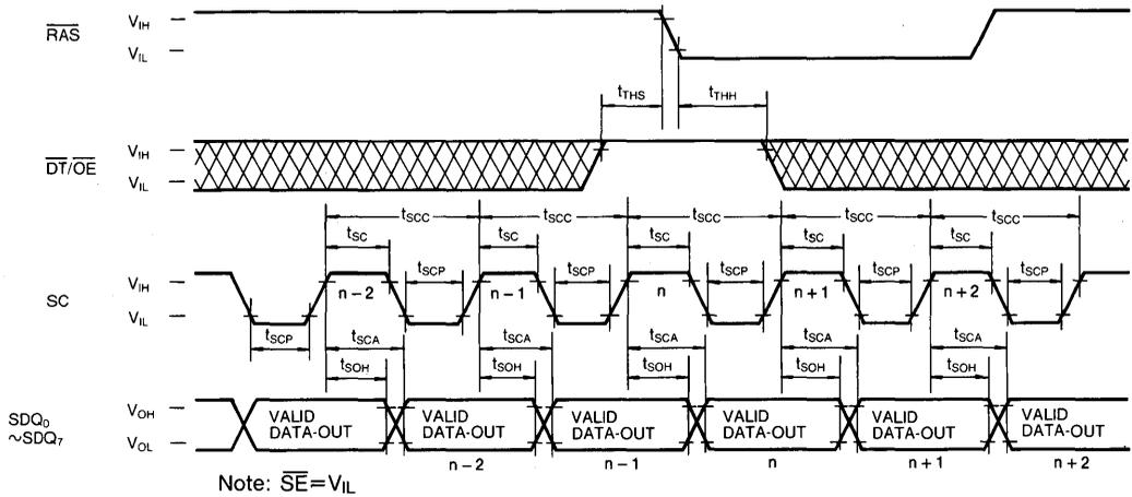
SERIAL READ CYCLE ( $\overline{SE}$  Controlled Outputs)
