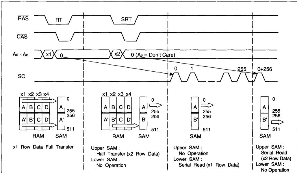
Figure 8. Split Read Transfer Normal Usage
