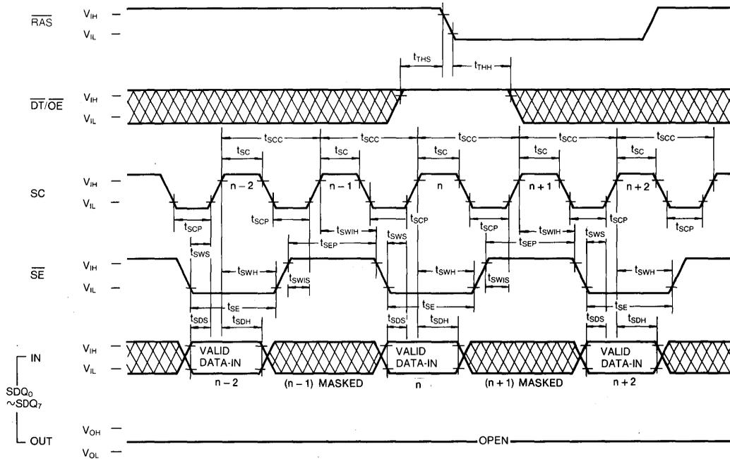
**SERIAL WRITE CYCLE ( $\overline{SE} = V_{IL}$ )**
