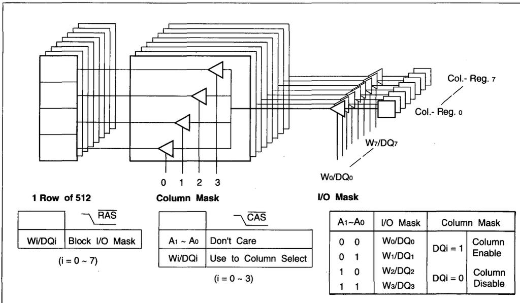
Figure 3. Block Write Scheme
