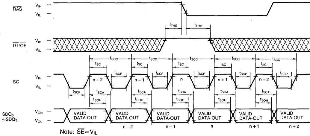
SERIAL READ CYCLE ( $\overline{SE}$  Controlled Outputs)
