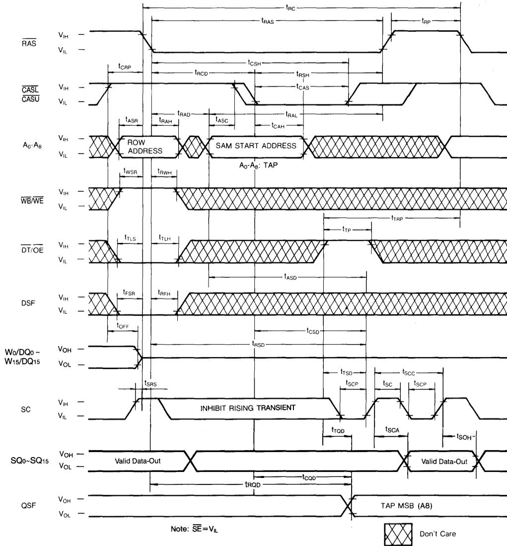
SERIAL READ CYCLE ( $\overline{SE} = V_{IL}$ )
