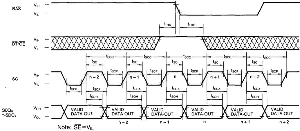
**SERIAL READ CYCLE ( $\overline{SE}$  Controlled Outputs)**
